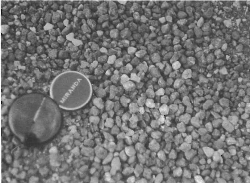
Figure 24. Three sizes of coarse aggregate were used. This is the small size cut on the 1/2" screen.
