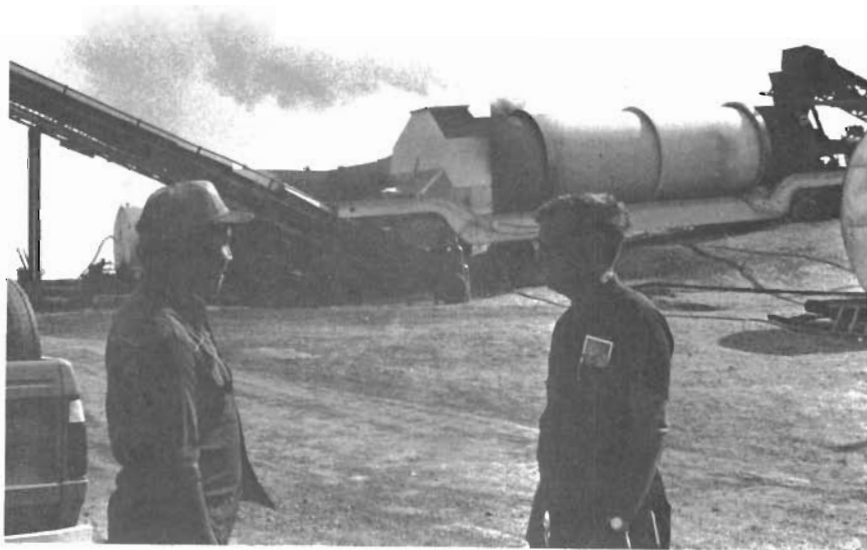
Figure 11. M. Israel, employee of Motheral Contractors and John Nixon observe a large plume that developed during the use of flux oil in the recycling of the old pavement before proper adjustment was made.
