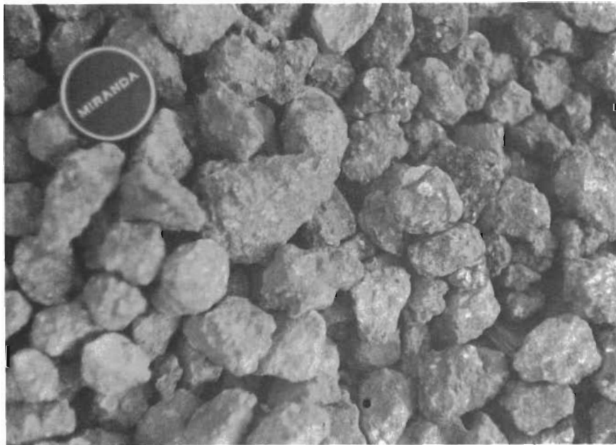
Figure 26. Maximum size was anything over the 7/8" screen which included some 2" material from the old base.
