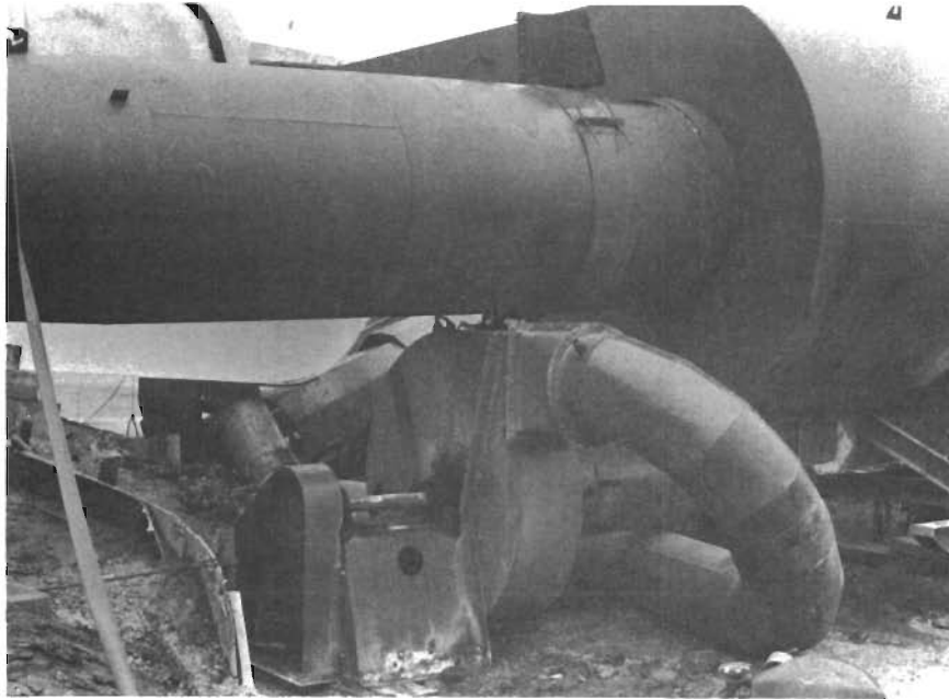
Figure 19. Dust collector system showing the main pipe to the stack and the larger particle return line to the materials output end.
