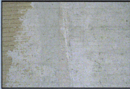
EucoSpeed- cracks at boundaries
