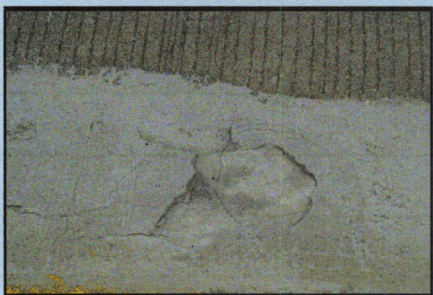
MgKrete- cracking and spalling
