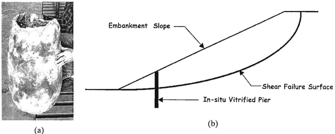
**Figure 1** – (a) A Column of Vitrified Soil Exhumed from a Field Demonstration Site, (b) Use of In-Situ Vitrification for Slope Stabilization
