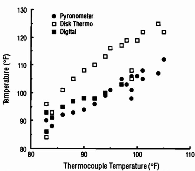
Fig 3.6. Temperatures for each device; slab thickness = 6 inches, aggregate = river gravel.
