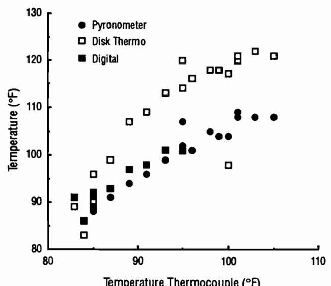
Fig 3.11. Temperatures for each device; slab thickness = 14 inches, aggregate = limestone.
