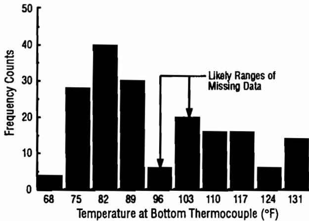
Fig 4.15. Frequency counts of temperature at bottom thermocouple.
