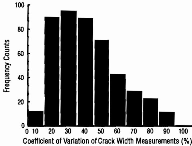
Fig 4.11. Frequency counts of the observed coefficients of variation of crack width measurements.
