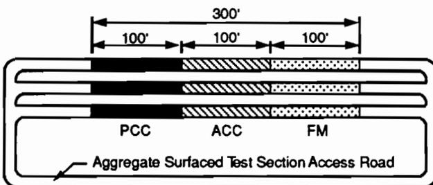
Fig 2.1. Layout of test site at Balcones Research Center (Ref 3).
