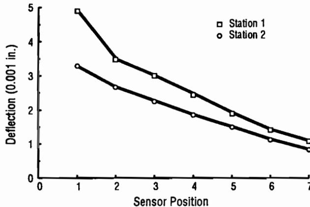
Fig 4.9. Deflection basins in a typical overlaid subsection.
