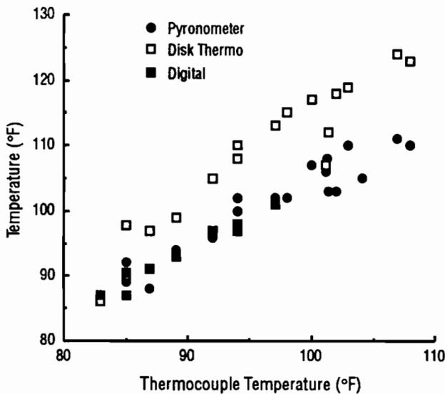
Fig 3.7. Temperatures for each device; slab thickness = 6 inches, aggregate = limestone.
