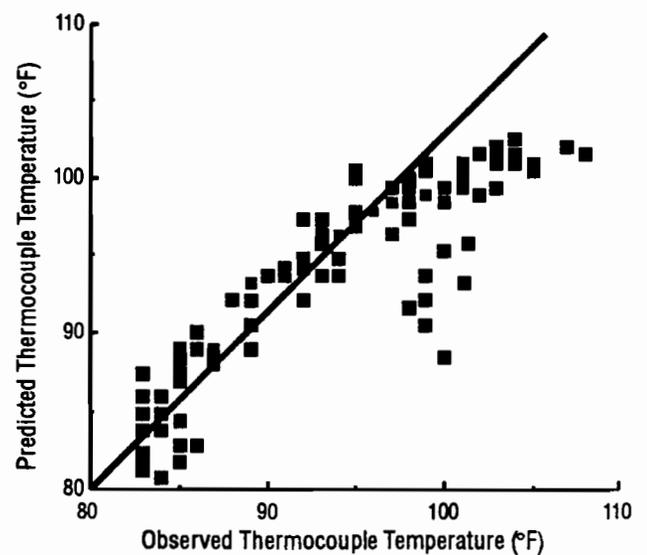
Fig 3.17. Predicted versus actual plot, disk linear model.
