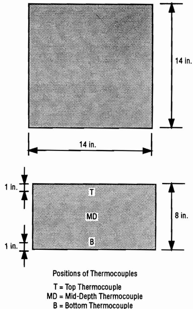
Fig 3.1. Scheme of the portable slabs.
