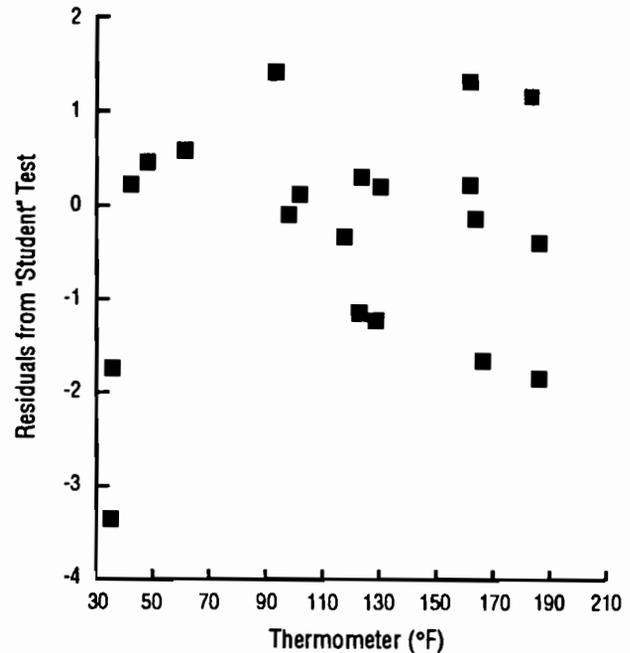
Fig 3.5. Residual plot of the calibration curve.
