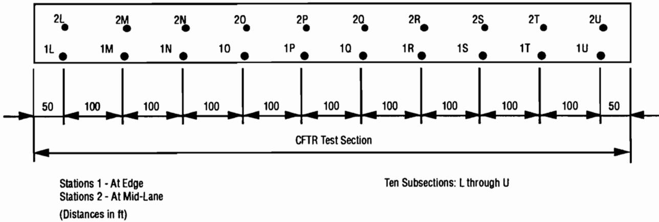
Fig 4.4. Overlaid test section: subsections and stations.
