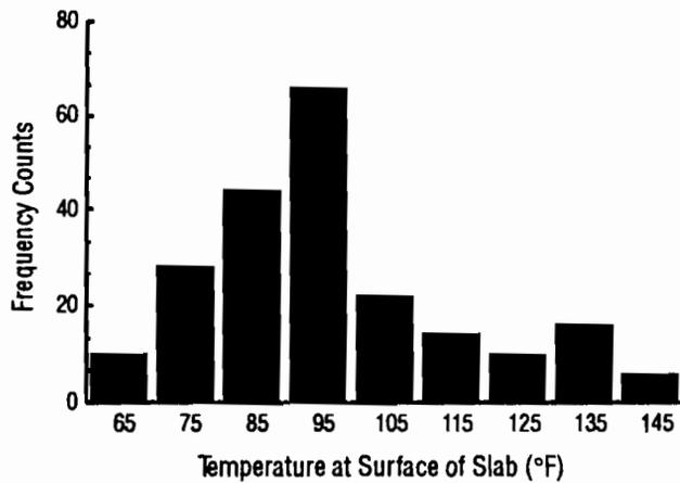
Fig 4.12. Frequency counts of temperature taken at surface.
