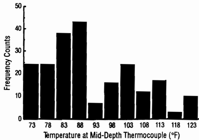
Fig 4.14. Frequency counts of temperature at middepth thermocouples.
