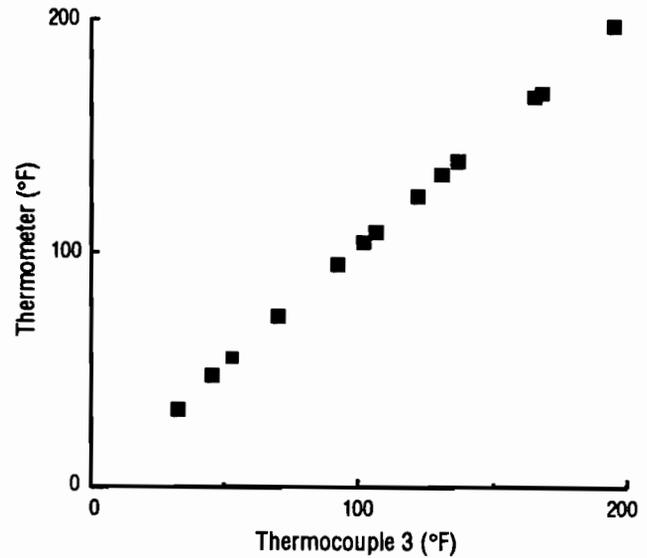
Fig 3.4. Thermometer vs. thermocouple 3.
