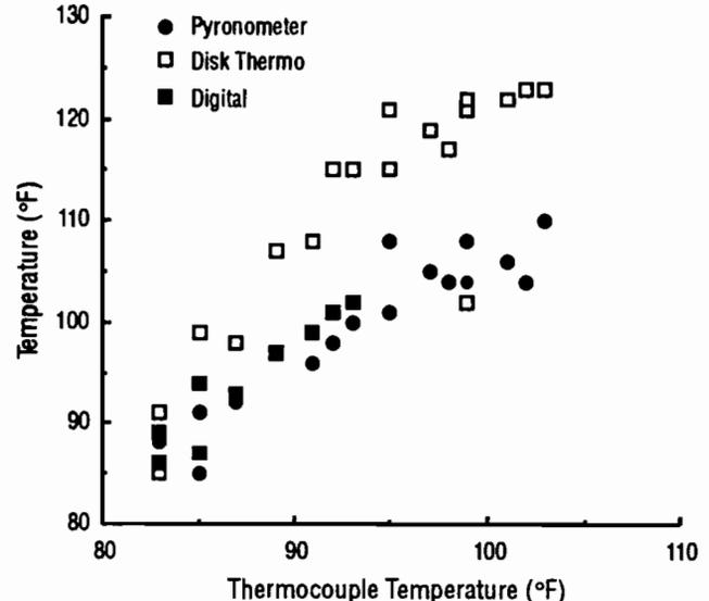
Fig 3.10. Temperatures for each device; slab thickness = 14 inches, aggregate = river gravel.
