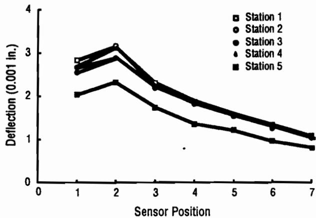
Fig 4.8. Deflection basins in a typical non-overlaid subsection.
