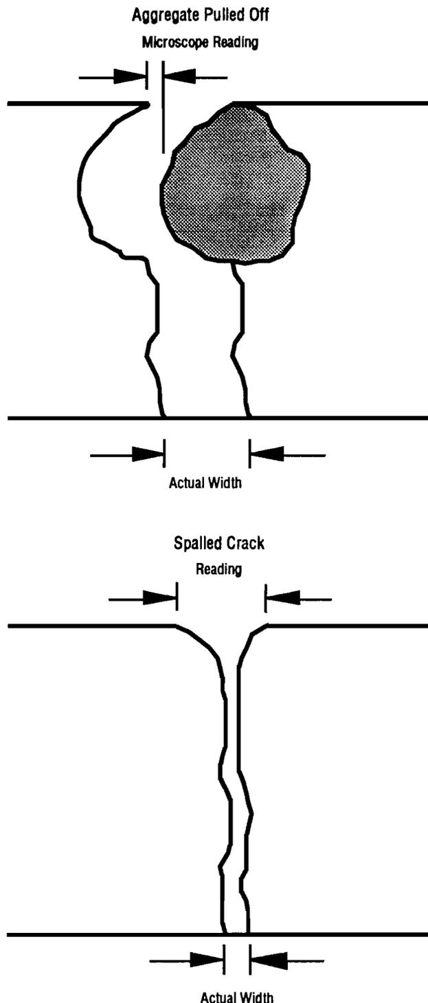
Fig 2.2. Situations to avoid in crack width readings.
