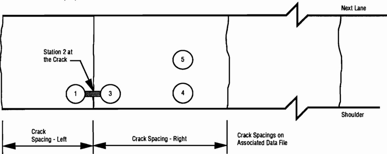
Fig 4.3. Non-overlaid test section: subsections and stations.
