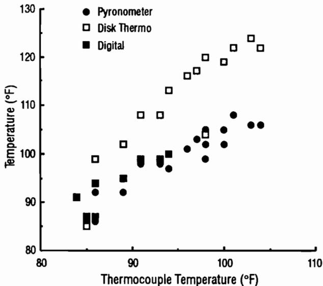
Fig 3.8. Temperatures for each device; slab thickness = 10 inches, aggregate = river gravel.
