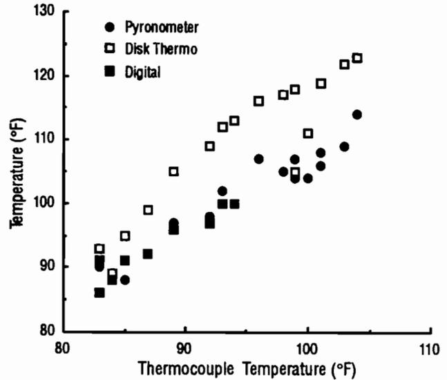
Fig 3.9. Temperatures for each device; slab thickness = 10 inches, aggregate = limestone.
