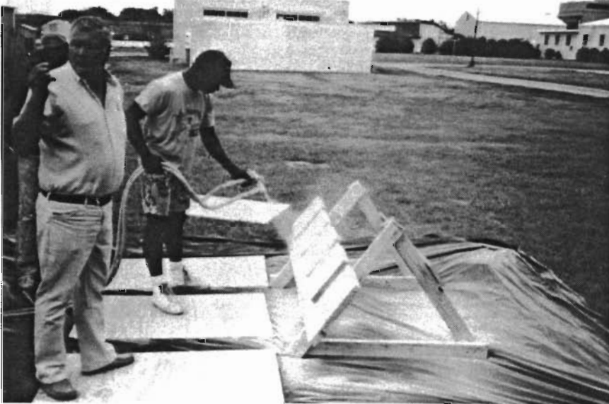
Fig 4.1. Application of coatings to test panels.
