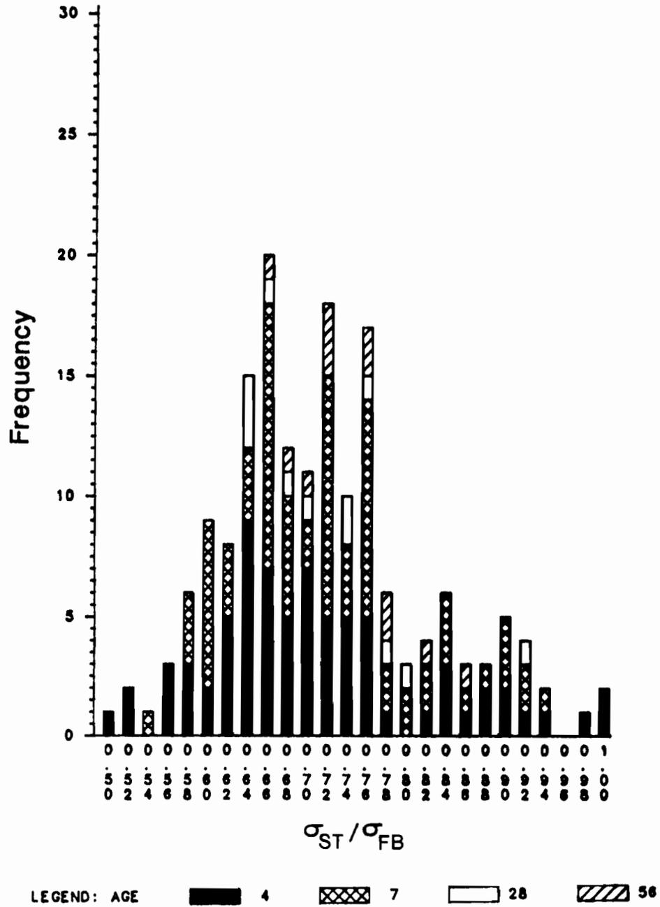
Fig 6.5. Distribution of splitting tensile versus flexural stress ratios for 4 x 8-inch cylinders, histogram form.
