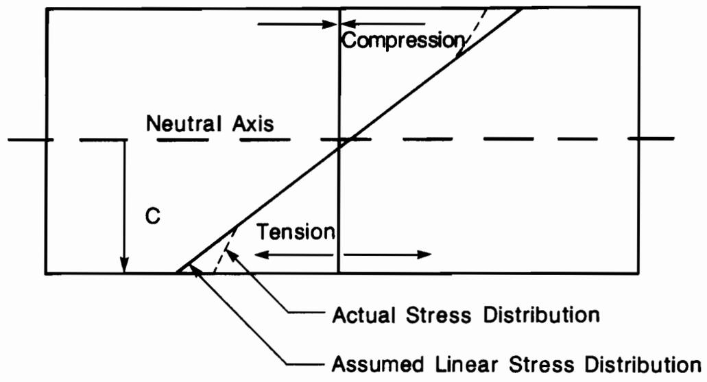
Fig 2.3. Stress distribution in the flexure beam test.
