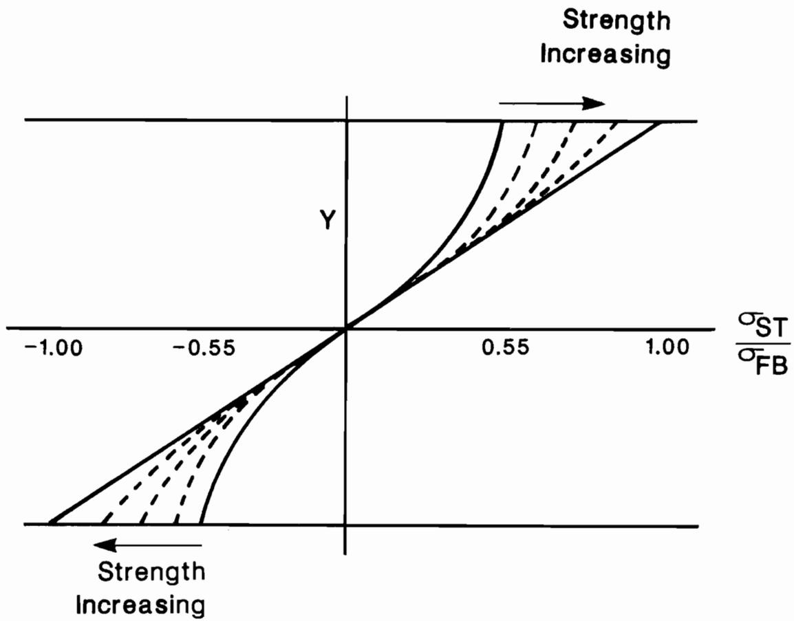
Fig 6.7. Change in stress distribution in the flexure beam specimen as the strength of the concrete increases.
