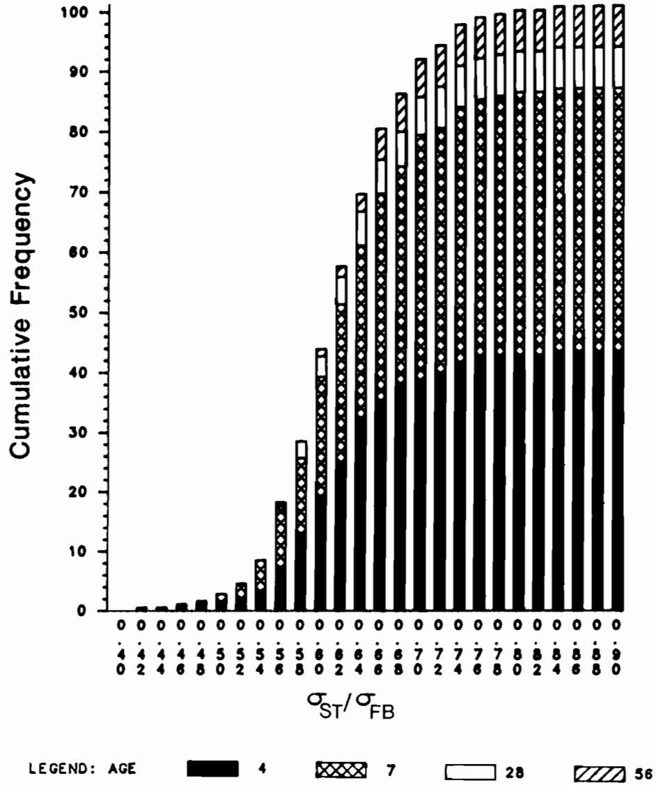
Fig 6.4. Distribution of splitting tensile versus flexural stress ratios for 6 x 12-inch cylinders, cumulative form.
