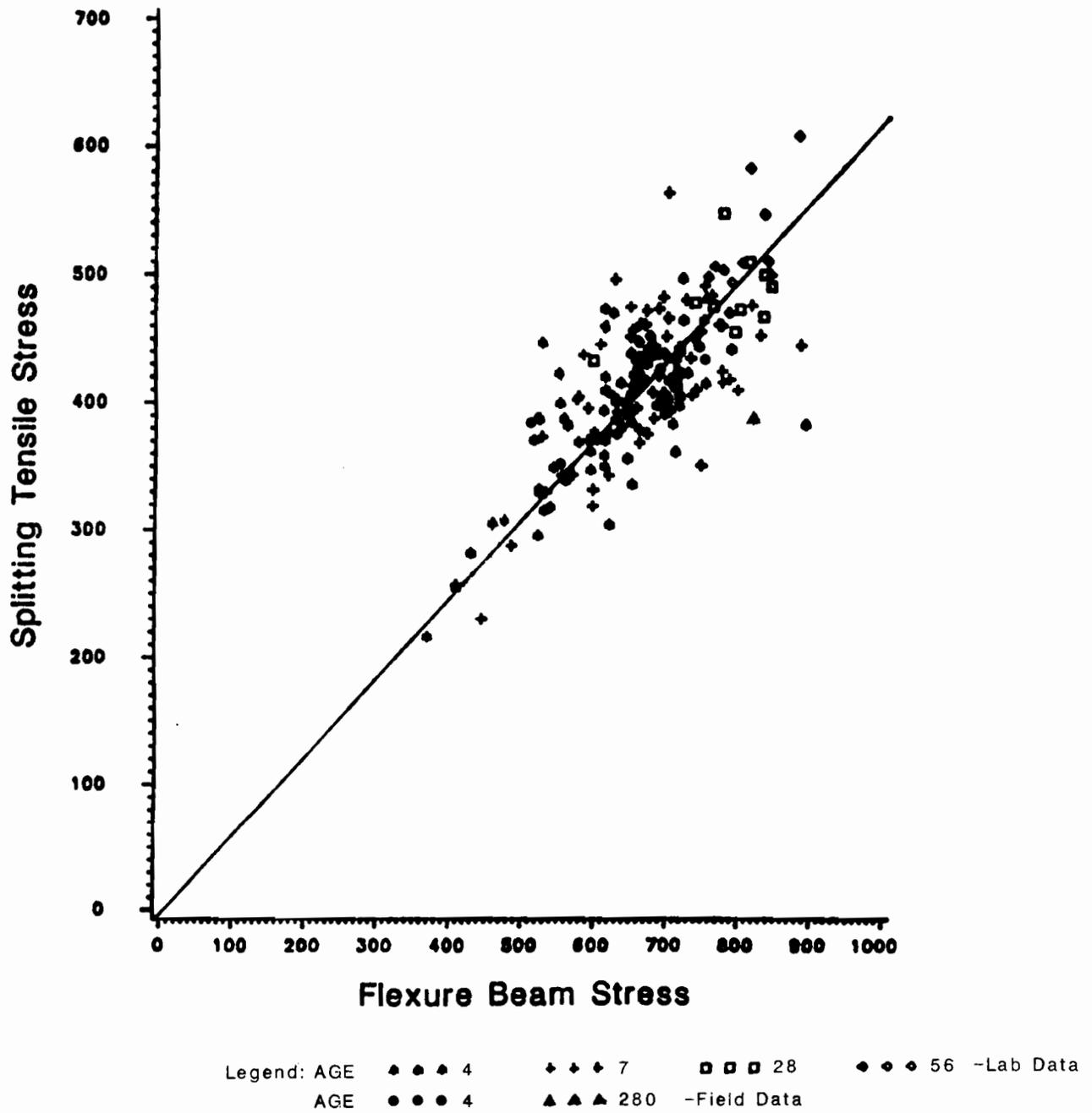
Fig 6.8 . Comparison between lab and field splitting tensile and flexural strength for 6 x 12-inch cylinders.
