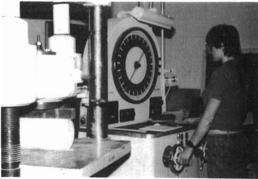
Fig 3.3. Loading 6 x 12-inch cylinder specimen.
