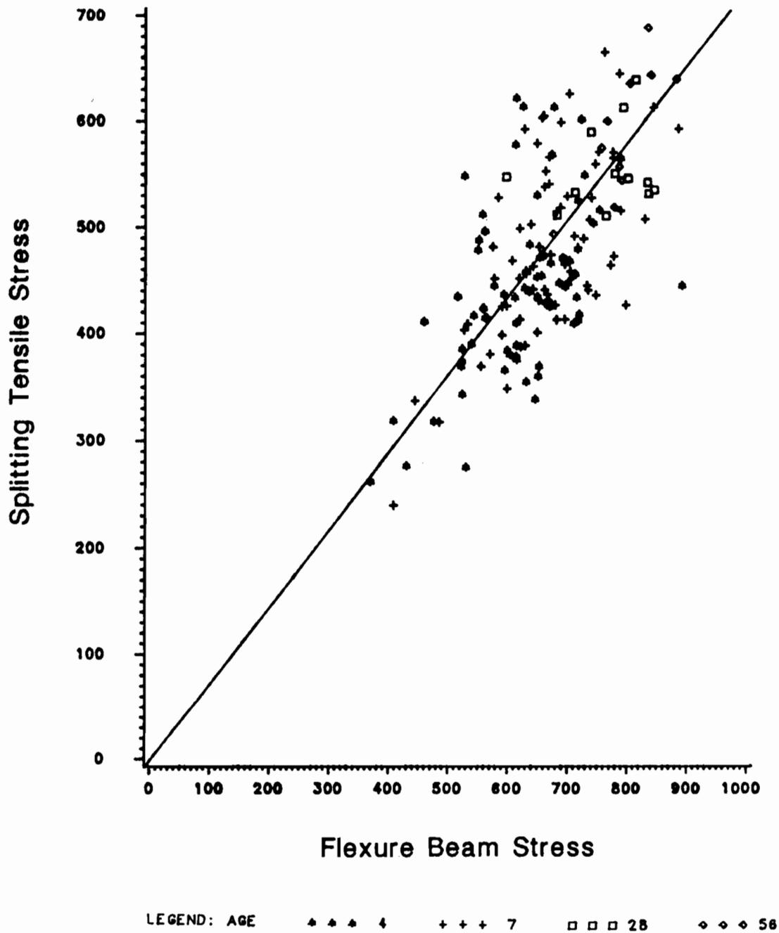
Fig 6.2. Relationship between splitting tensile strength and flexural strength for 4 x 8-inch cylinders.
