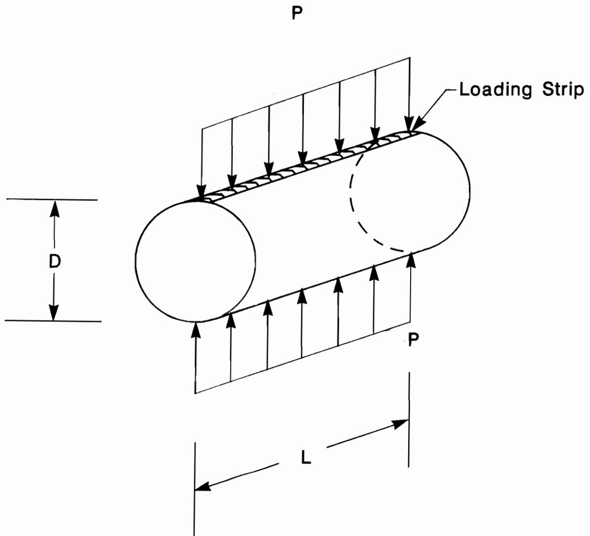
Fig 3.1. Isometric of splitting tensile test.
