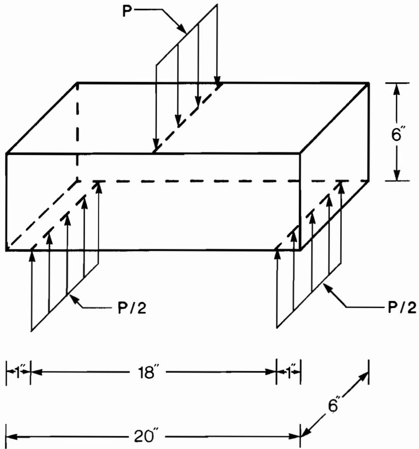
Fig 2.1. Isometric of flexure beam test.
