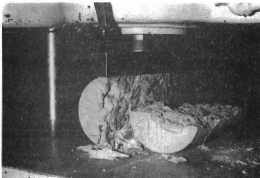
Fig 3.4. Typical fracture place of splitting tensile test specimen.
