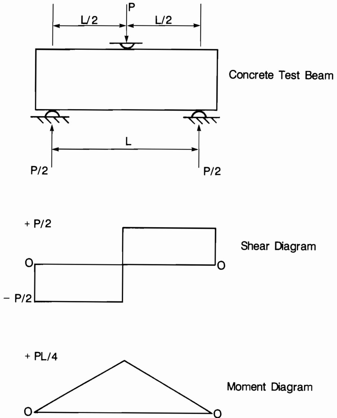
Fig 2.2. Shear and moment diagrams for center point flexure beam test.
