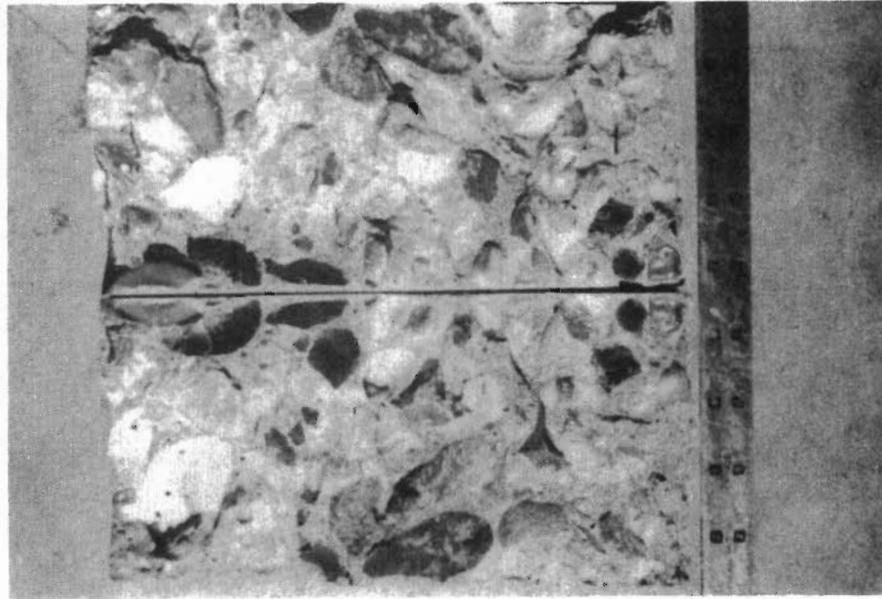
Fig 3.5. Close-up of typical fracture plane of splitting tensile test specimen.
