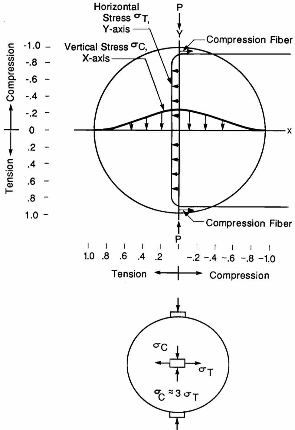
Fig 3.2. Relative stress distributions and center element showing biaxial state of stress for the splitting tensile test (Ref 11).
