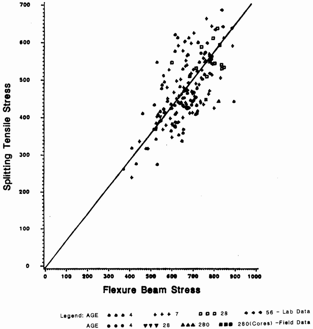
Fig 6. 9 . Comparison between lab and field splitting tensile and flexural strength for 4 x 8-inch cylinders.
