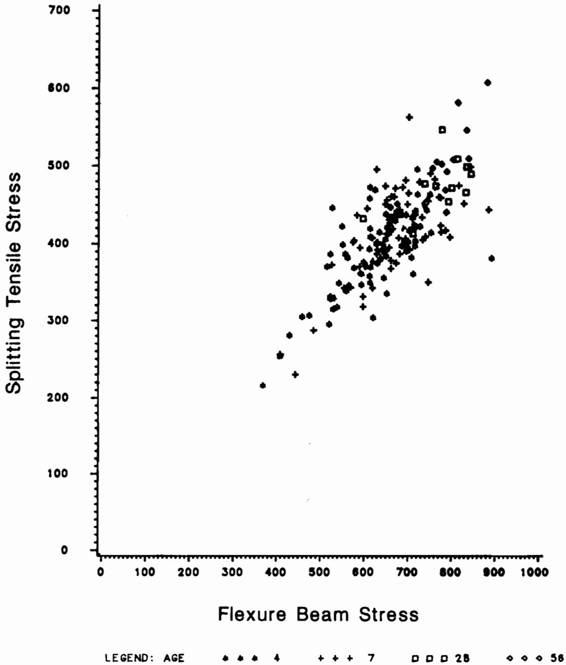
Fig 6.1. Relationship between splitting tensile strength and flexural strength for 6 x 12-inch cylinders.
