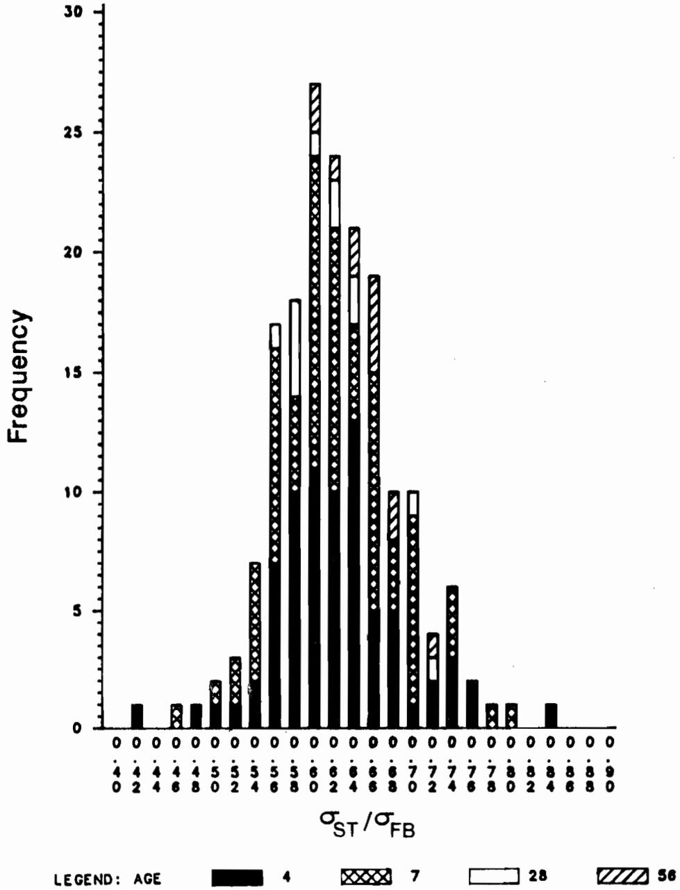
Fig 6.3. Distribution of splitting tensile versus flexural stress ratios for 6 x 12-inch cylinders, histogram form.
