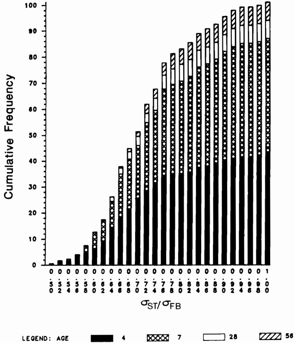
Fig 6.6. Distribution of splitting tensile versus flexural stress ratios for 4 x 8-inch cylinders, cumulative form.
