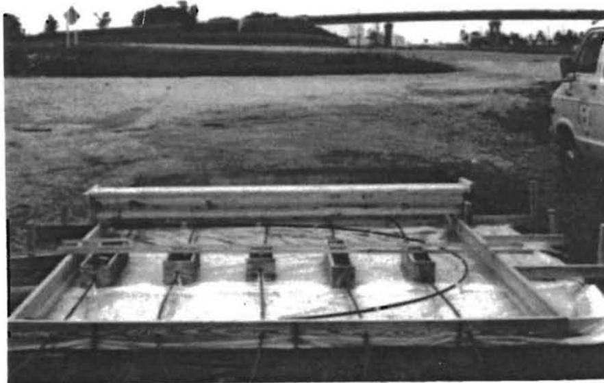
Fig 2.7. Layout of Test Slab No. 1 before the concrete was cast.
