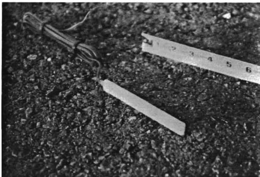
Fig 2.6. Embedment gage used for measuring concrete strain.
