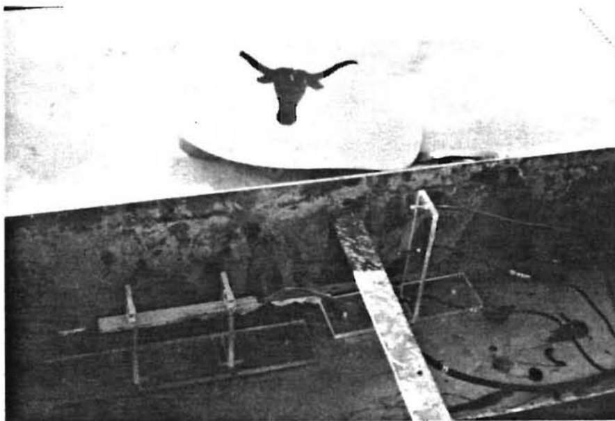
Fig 3.12. Close-up view of thermocouples and embedment strain gages in block-out.
