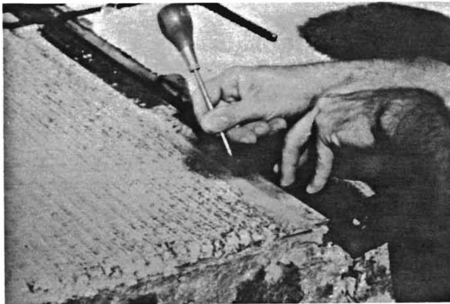
Fig 3.31. Etching of scribe marks used for measuring changes in joint opening width.
