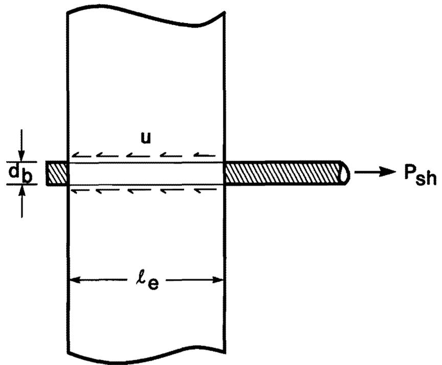
Fig. A.2 Shear-bond failure
