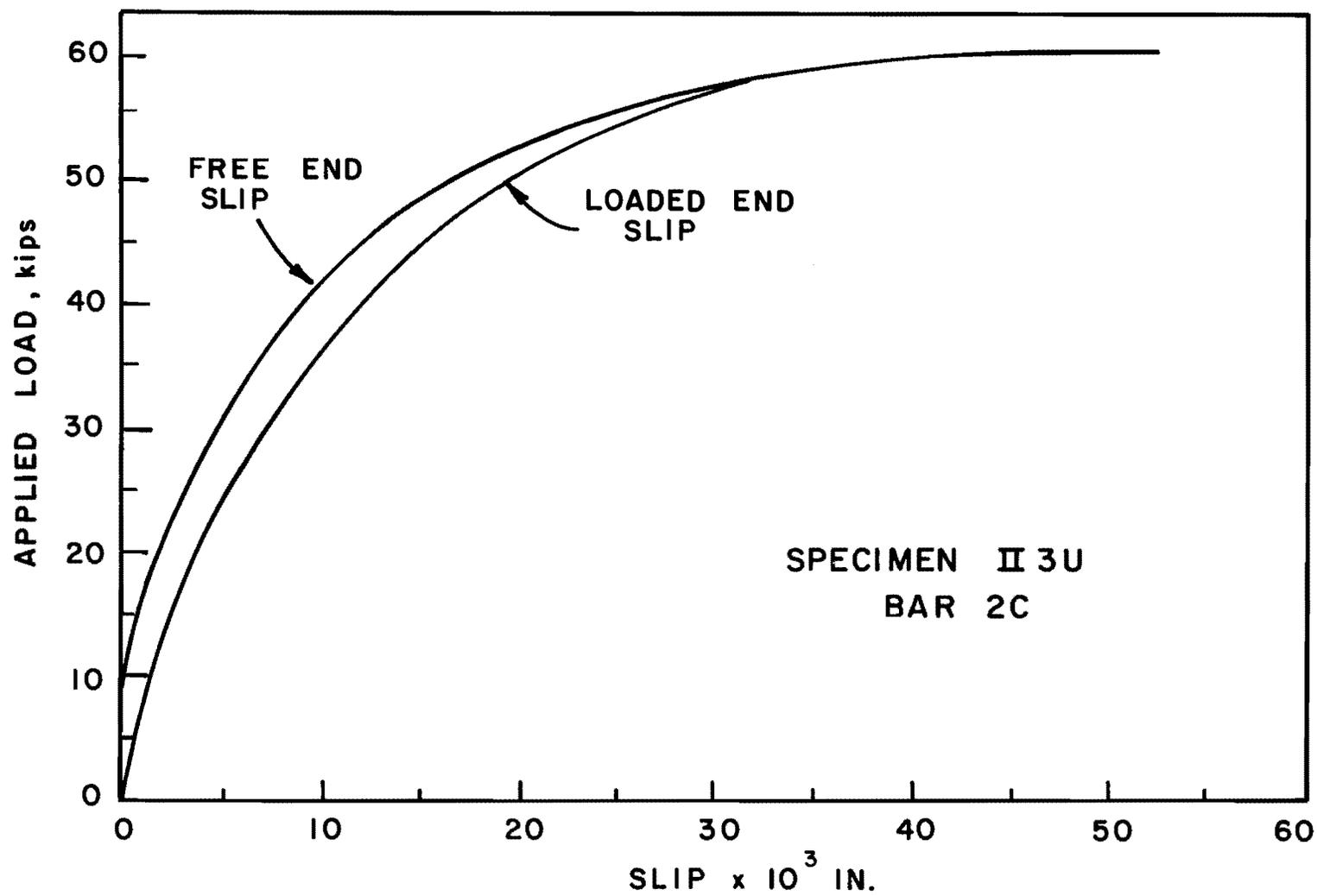
Fig. 4.9 Typical load-slip curve
