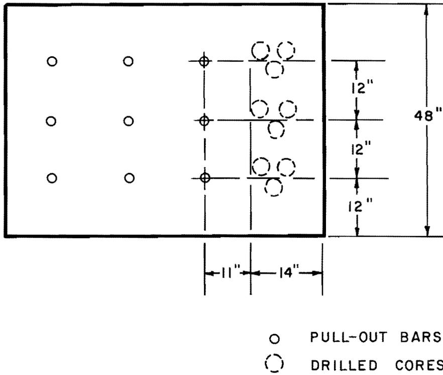
Fig. 3.8 Location of drilled cores
