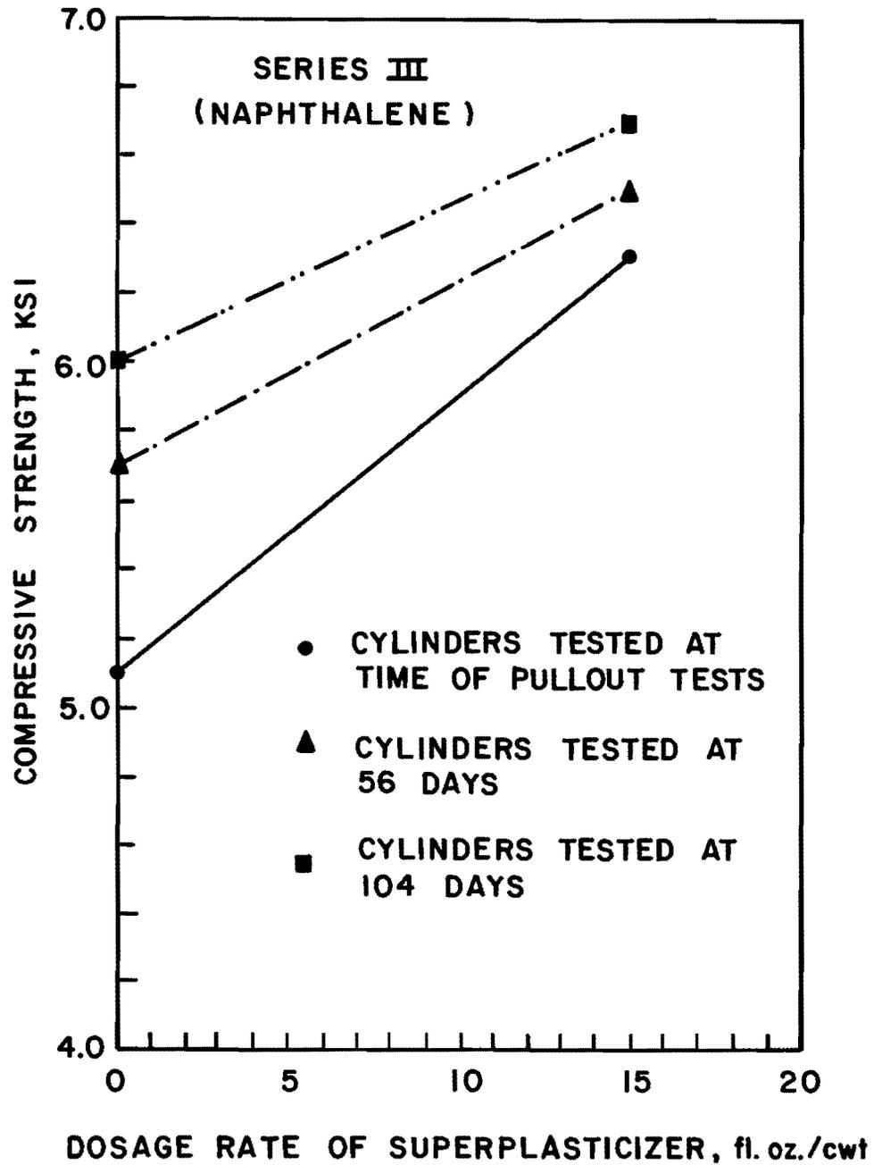
Fig. 6.24 Effect of addition of superplasticizer on compressive strength of concrete for Series III
