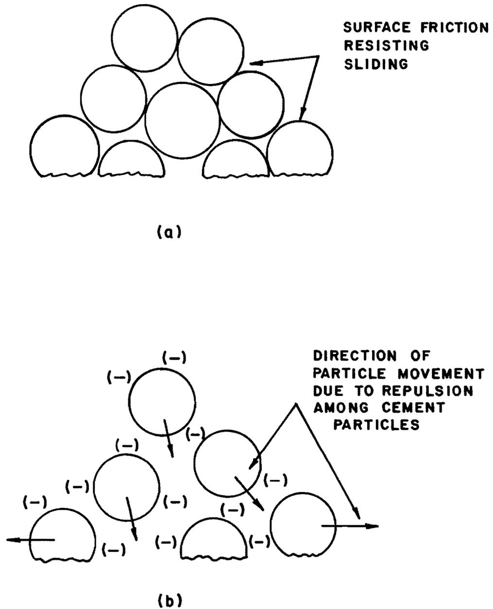
Fig. 6.13 Process by which naphthalene-based superplasticizer increases slump of concrete: (a) stacking of cement particles due to surface friction; (b) sliding of cement particles after addition of superplasticizer
