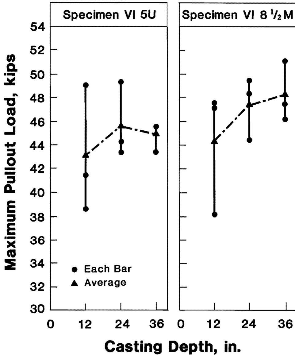
Fig. 6.37 Maximum pullout load versus casting depth for bars from Series VI
