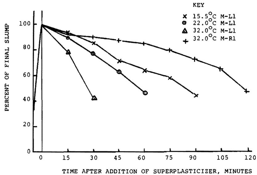
Fig. 2.14 Effect of temperature variation on slump loss [19]
