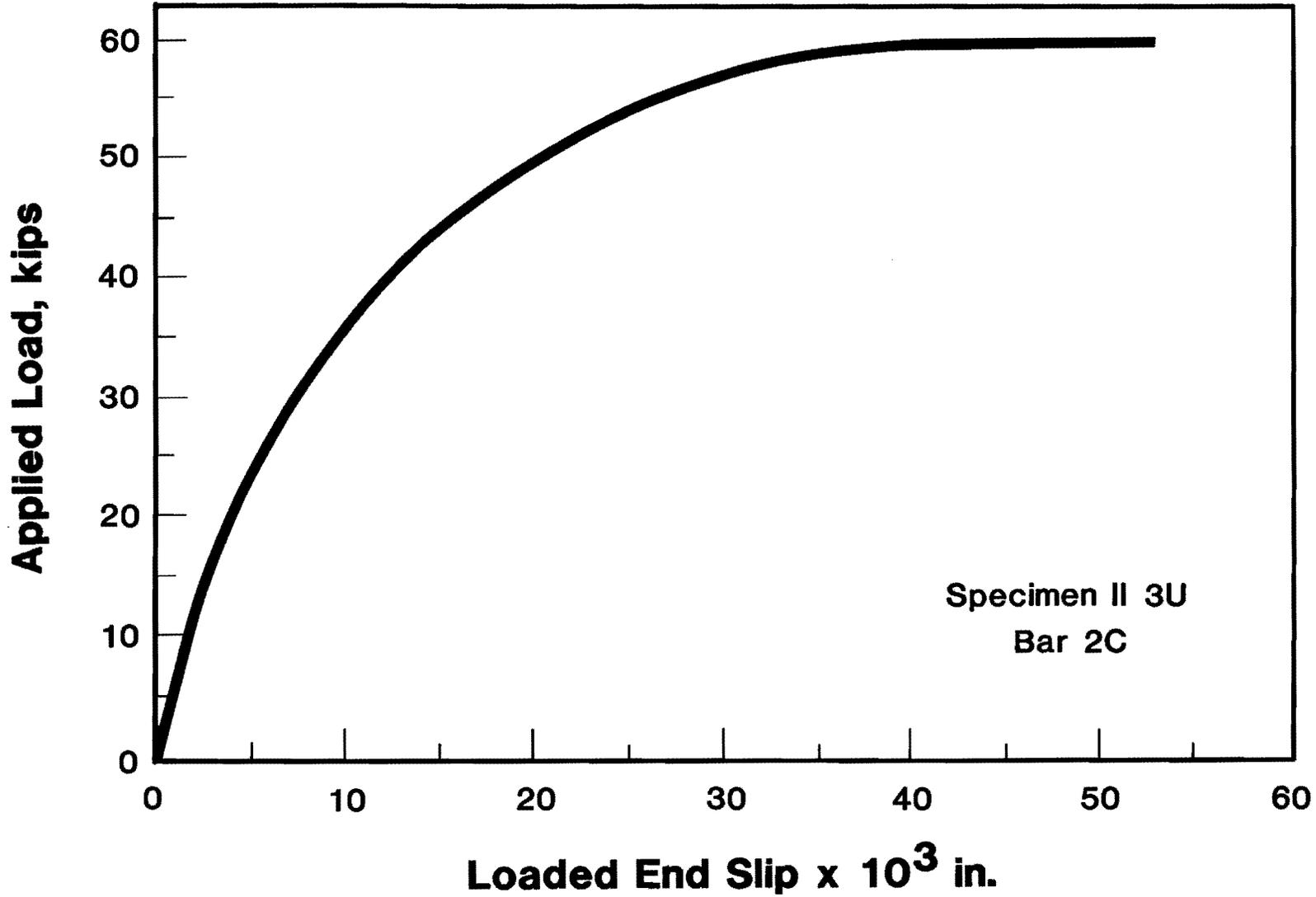
Fig. B.3 Corrected loaded end slip curve
