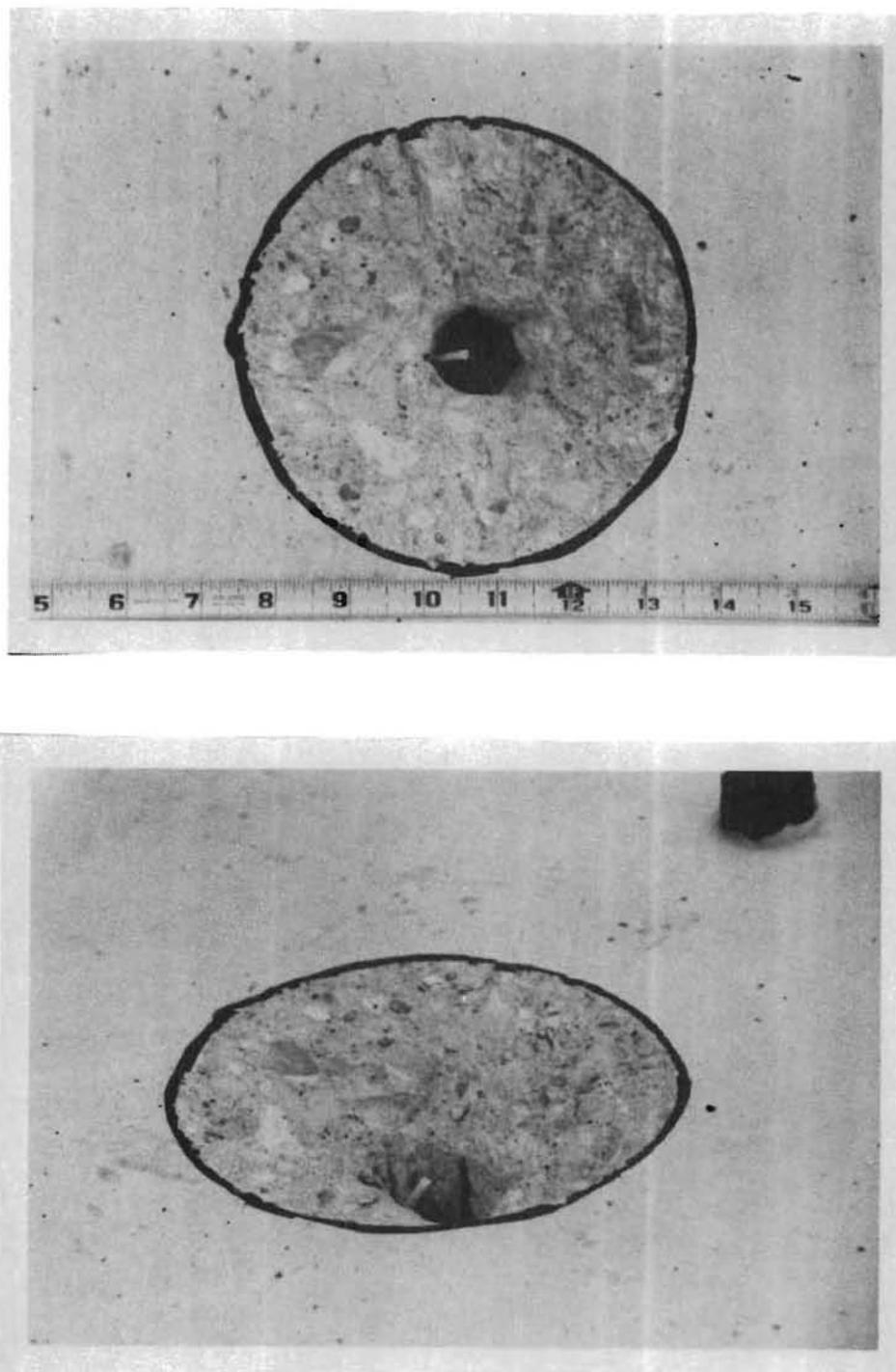
Fig. 4.14 Appearance of failure surface resulting from pullout test
