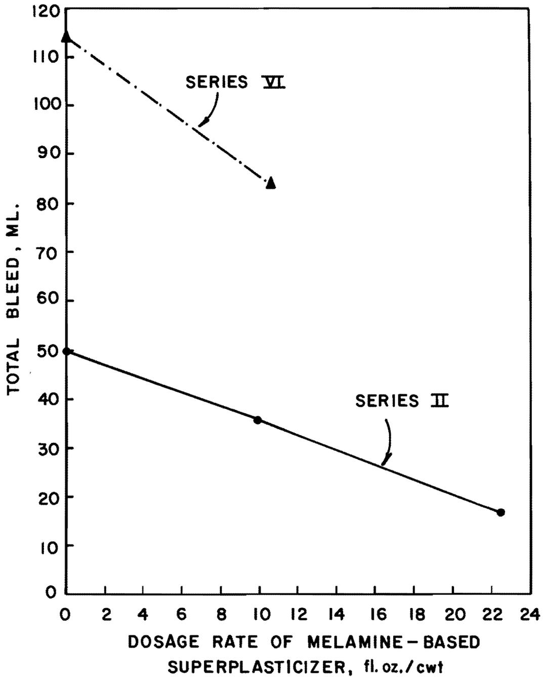
Fig. 6.22 Effect of melamine-based superplasticizer on the bleeding of concrete
