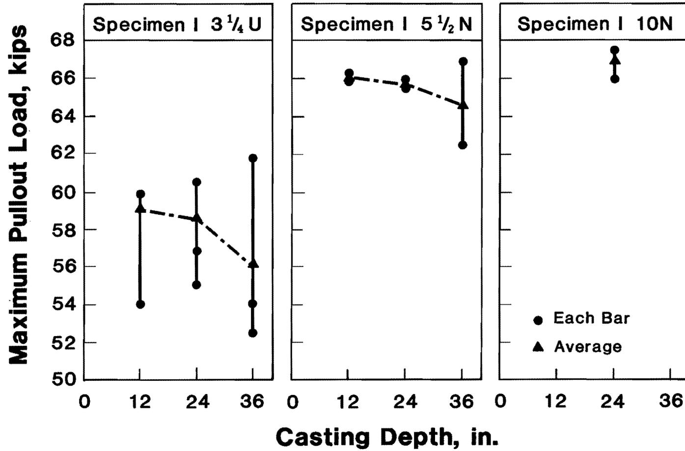
Fig. 6.32 Maximum pullout load versus casting depth for bars from Series I
