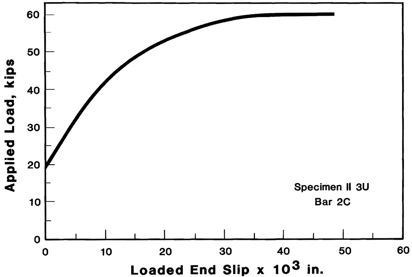
Fig. B.1 Loaded end slip curve before correction
