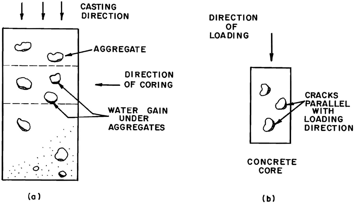
Fig. 6.29 Discontinuities in concrete caused by bleeding of concrete:
