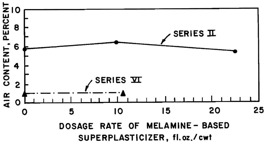
Fig. 6.20 Effect of melamine-based superplasticizer on air content of concrete
