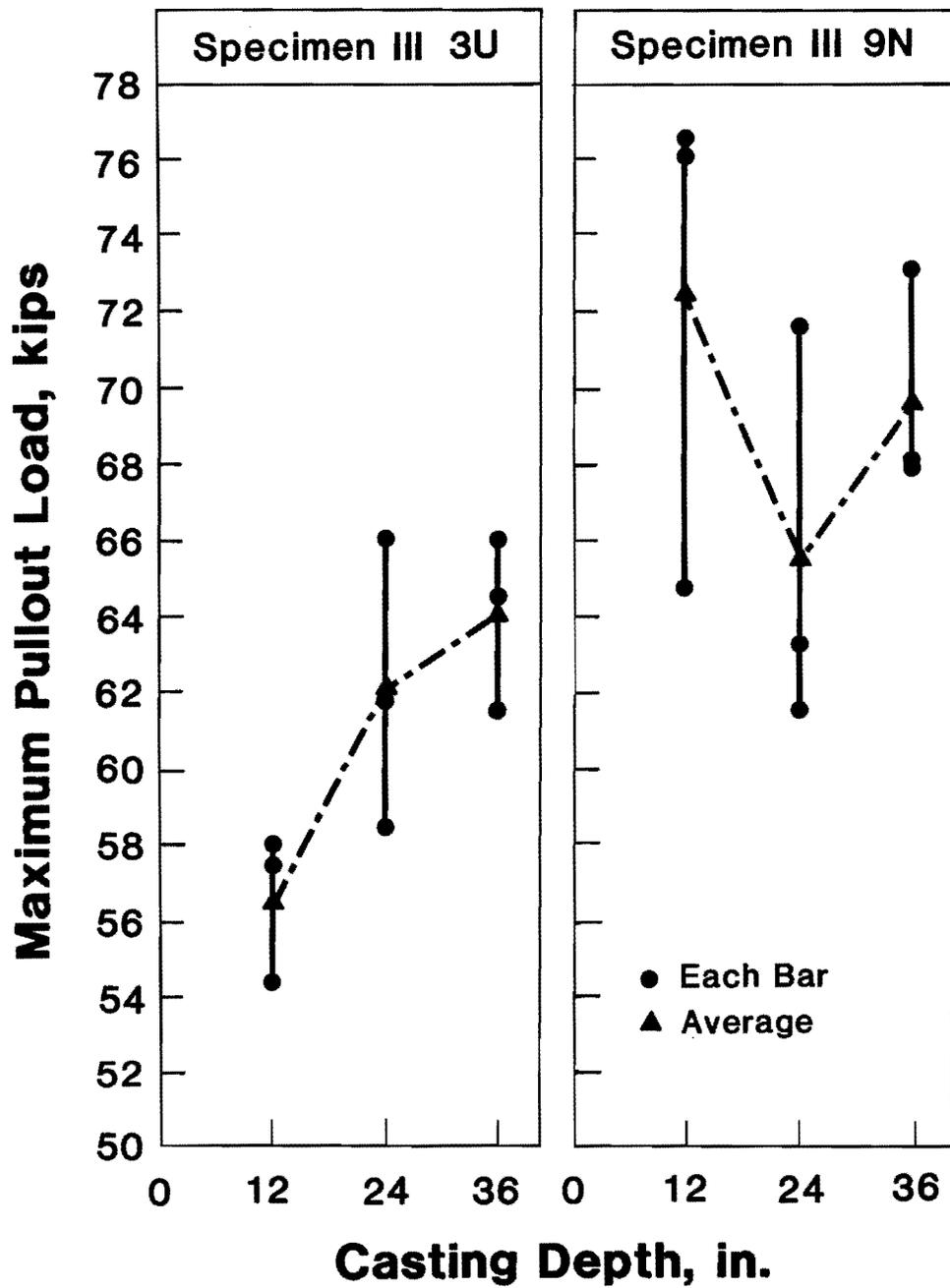
Fig. 6.34 Maximum pullout load versus casting depth for bars from Series III
