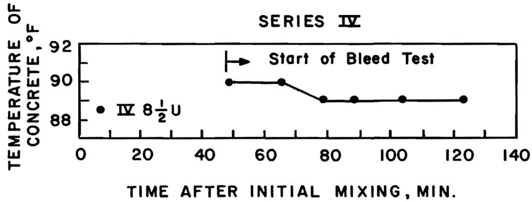
Fig. 6.18d Temperature of concrete with time during bleed tests for Series IV
