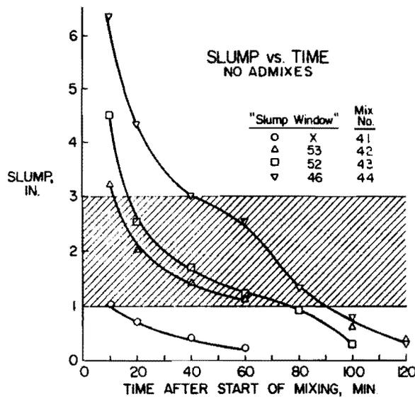
Fig. 2.11 "Slump windows" for concretes with various initial slump values [25]
