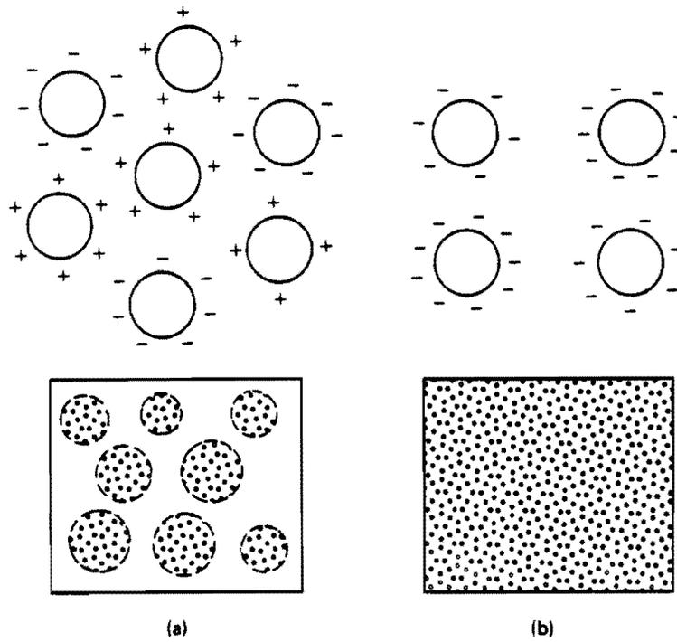
Fig. 2.7 Dispersing action of superplasticizer (schematic representation): (a) flocculated paste; (b) dispersed paste [23]
