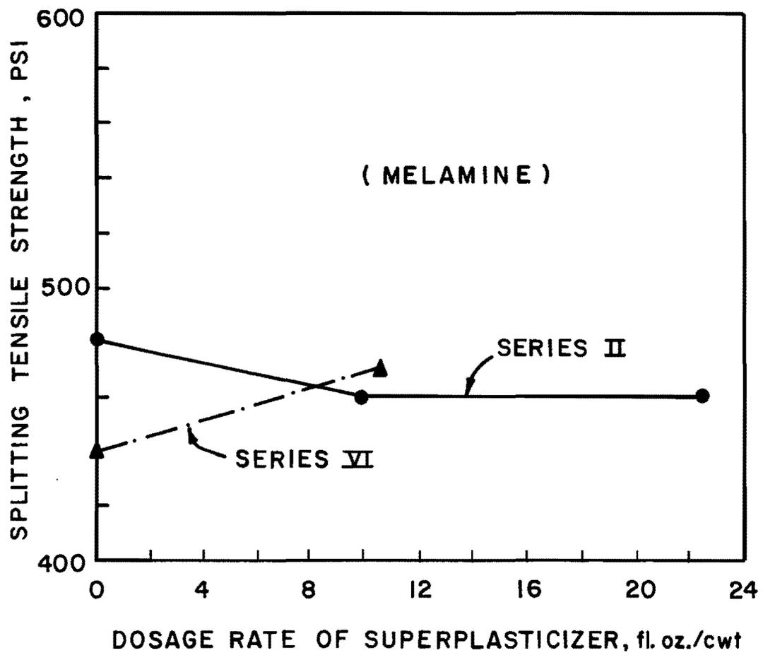
Fig. 6.31 Effect of dosage rate of melamine-based superplasticizer on splitting tensile strength of concrete
