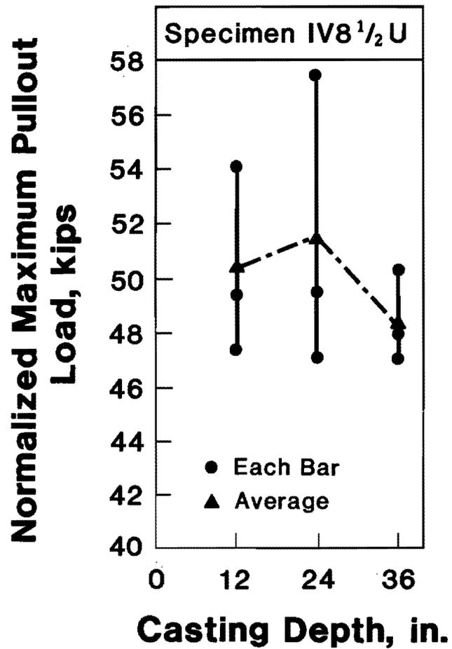
Fig. 6.43 Normalized maximum pullout load versus casting depth for bars from Series IV
