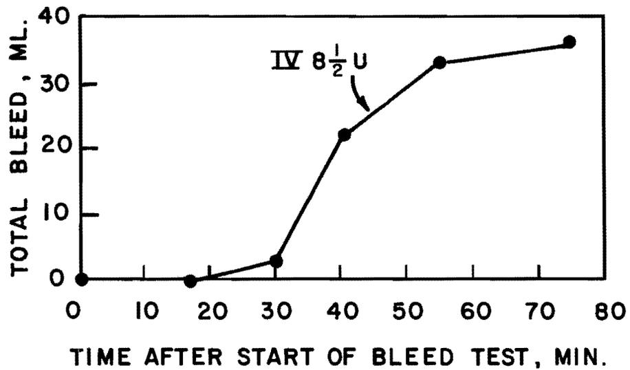
Fig. 4.4 Bleed versus time curve for specimen of Series IV
