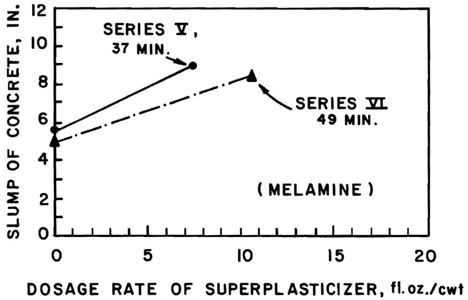
Fig. 6.17 Slump of concrete versus dosage rate of superplasticizer for Series V and VI
