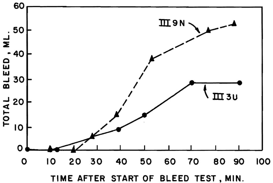
Fig. 4.3 Bleed versus time curves for specimens of Series III
