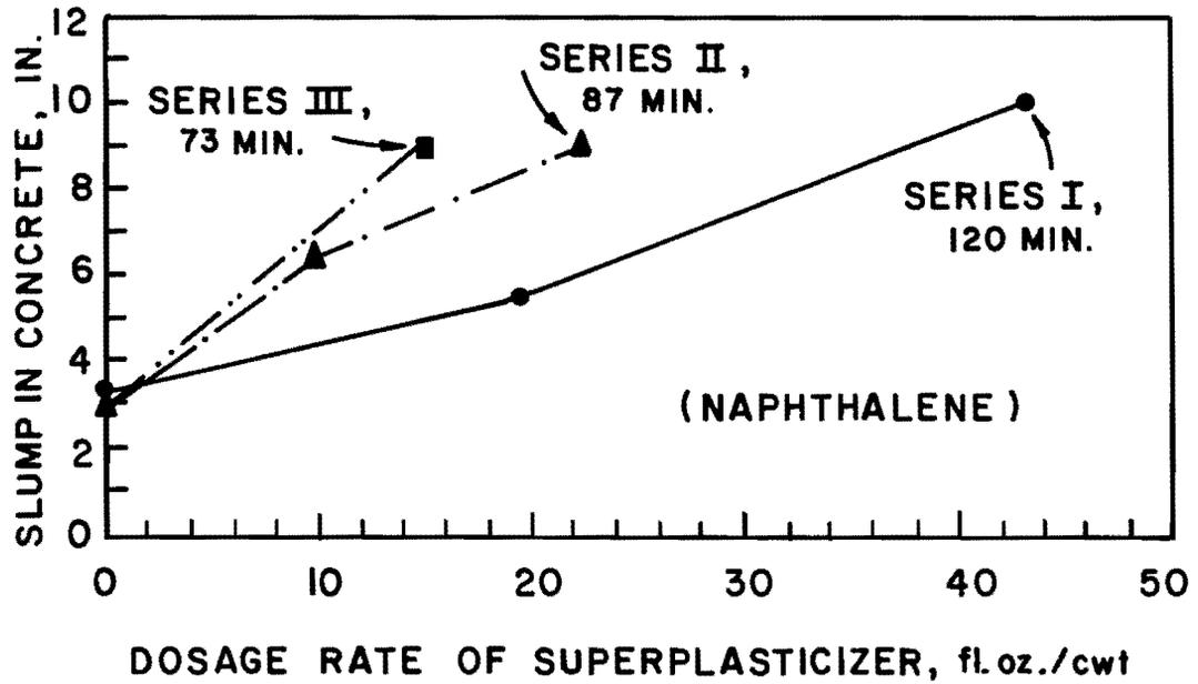
Fig. 6.16 Slump of concrete versus dosage rate of superplasticizer for Series I, II, and III
