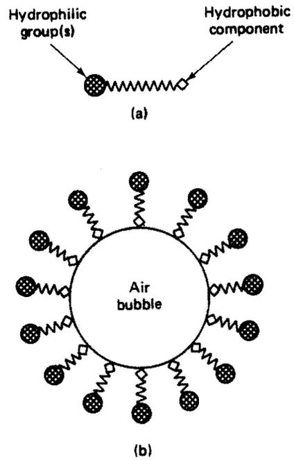
Fig. 2.2 Schematic representation of air entrainment by surface active molecules: (a) surface-active molecule; (b) stabilized air bubble [23]
