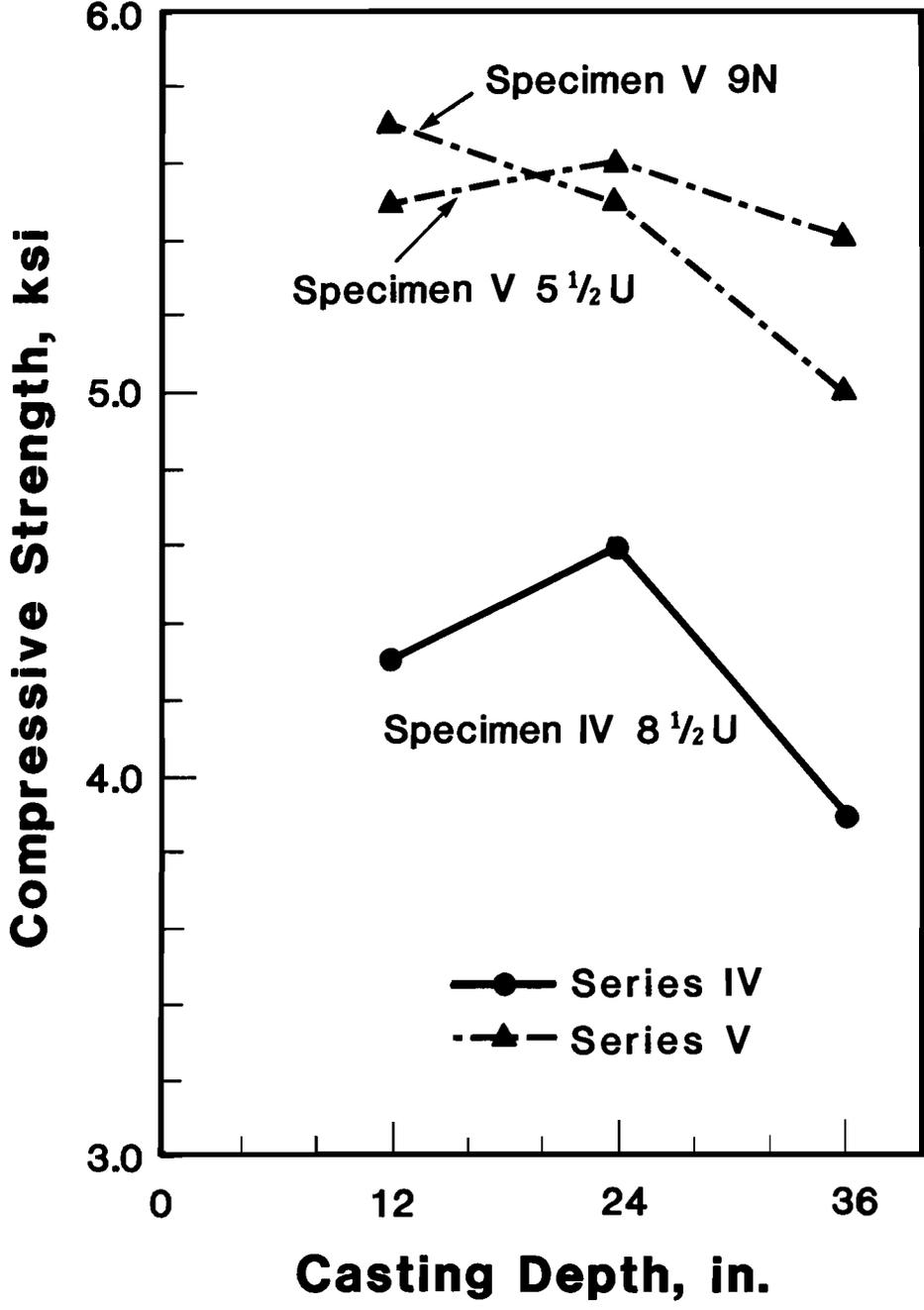
Fig. 6.28 Core compressive strength as a function of casting depth
