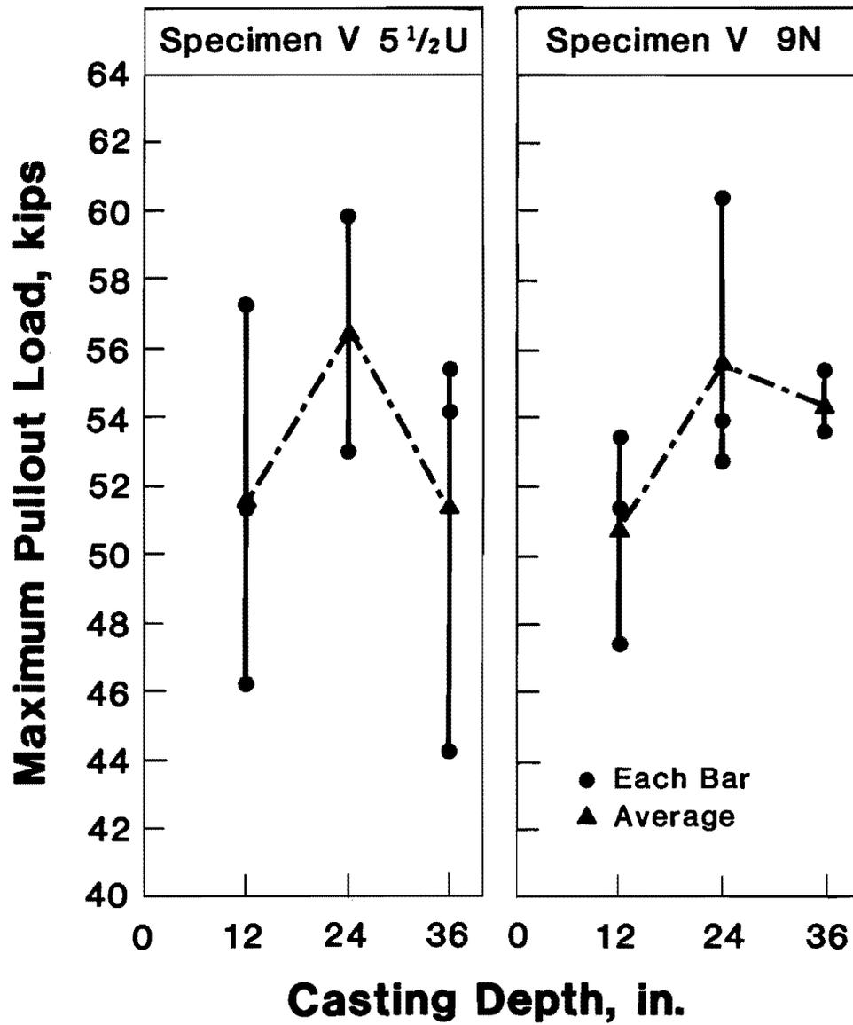
Fig. 6.36 Maximum pullout load versus casting depth for bars from Series V
