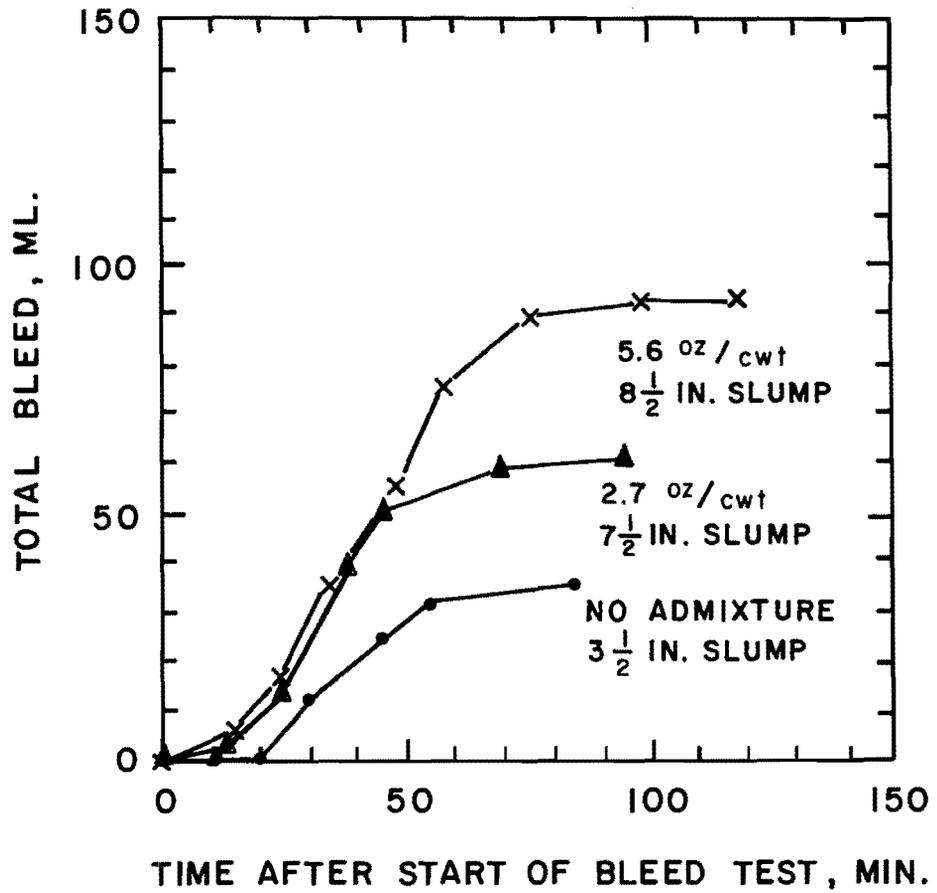
Fig. 2.19 Effect of melamine-based superplasticizer on bleeding of concrete for various dosage rates [24]
