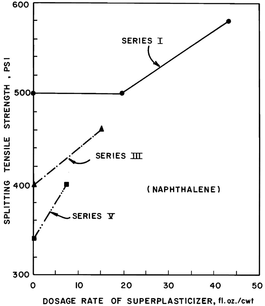
Fig. 6.30 Effect of dosage rate of naphthalene-based superplasticizer on splitting tensile strength of concrete
