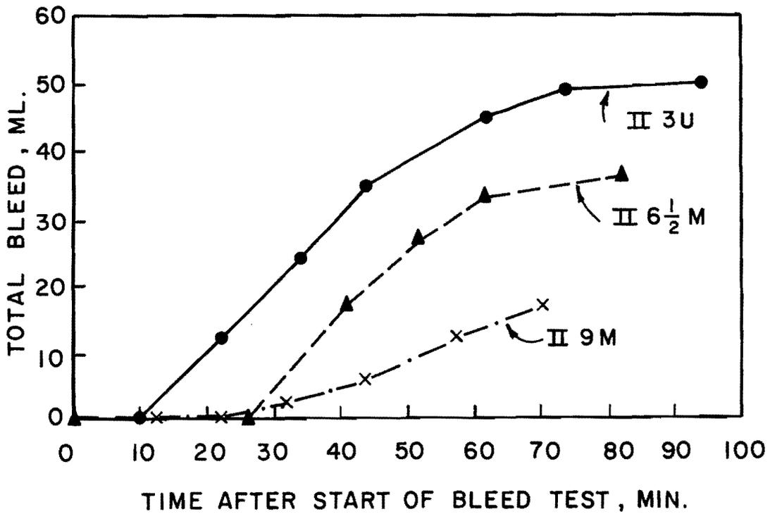
Fig. 4.2 Bleed versus time curves for specimens of Series II
