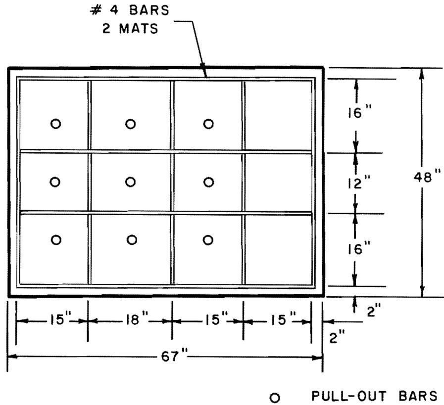
Fig. 3.5 Location of steel reinforcement
