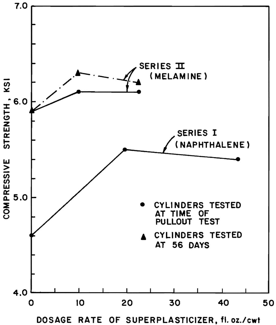
Fig. 6.23 Effect of addition of superplasticizer on compressive strength of concrete for Series I and II
