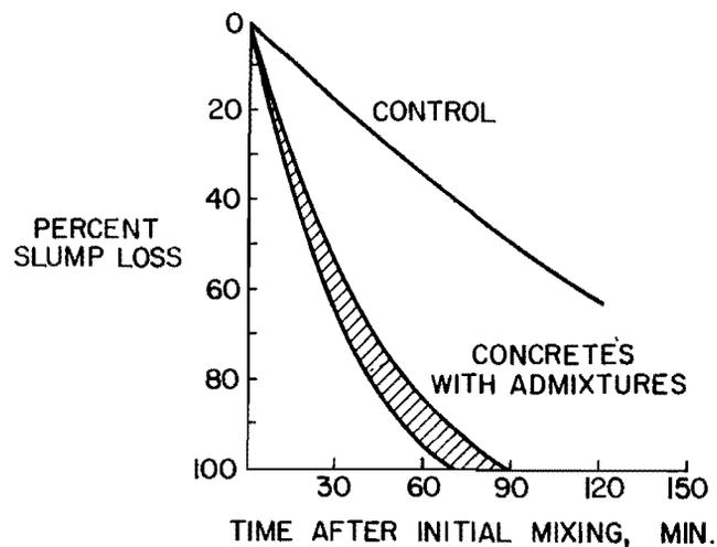
Fig. 2.9 Slump loss versus time for concrete containing 658 lbs cement per cubic yard [25]
