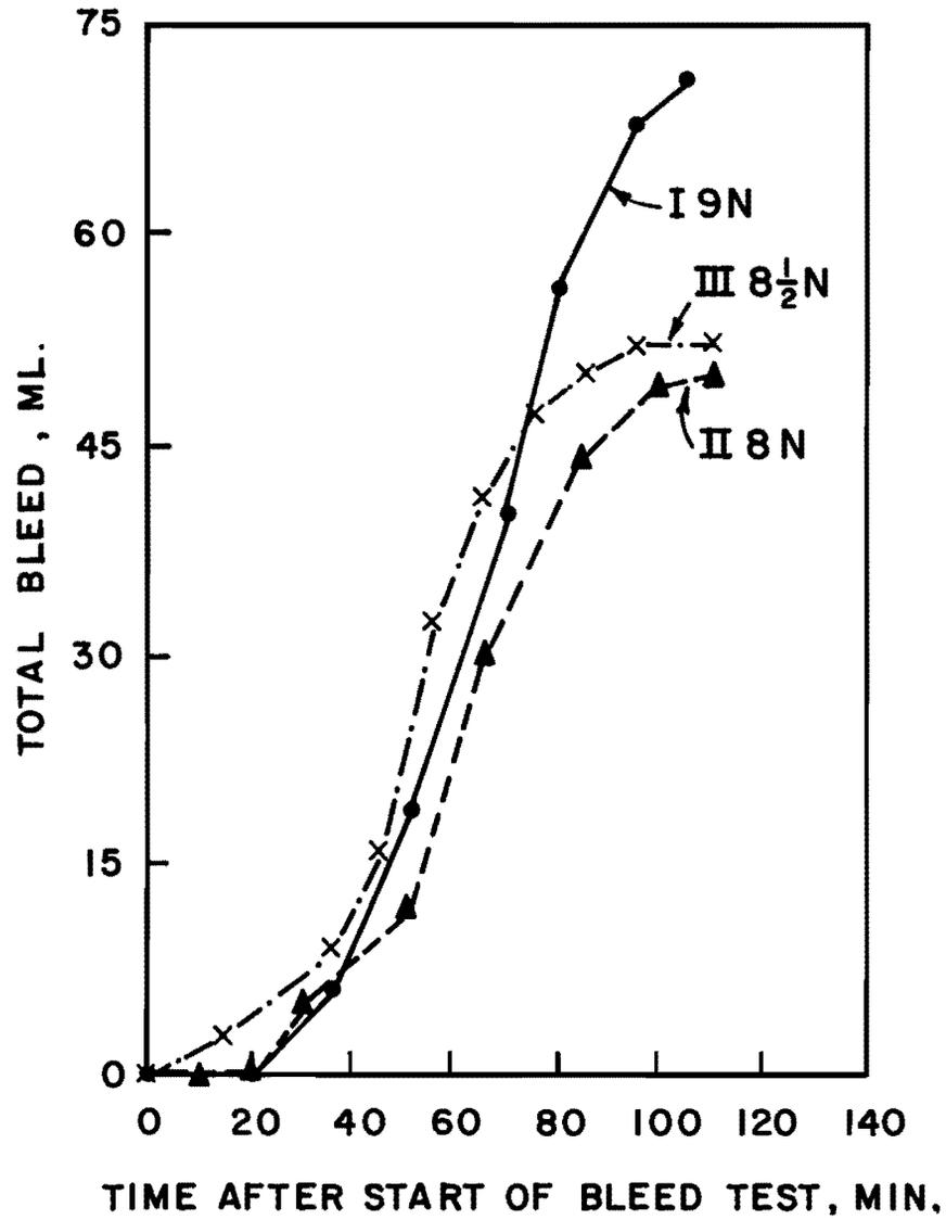
Fig. 5.6 Effect of concrete age on the bleeding of concrete containing superplasticizer
