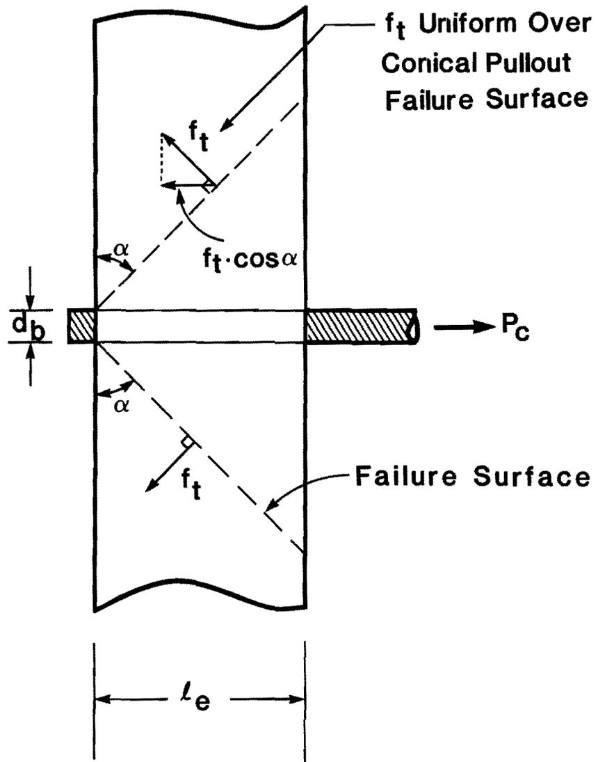
Fig. A.1 Schematic representation of conical pullout failure surface
