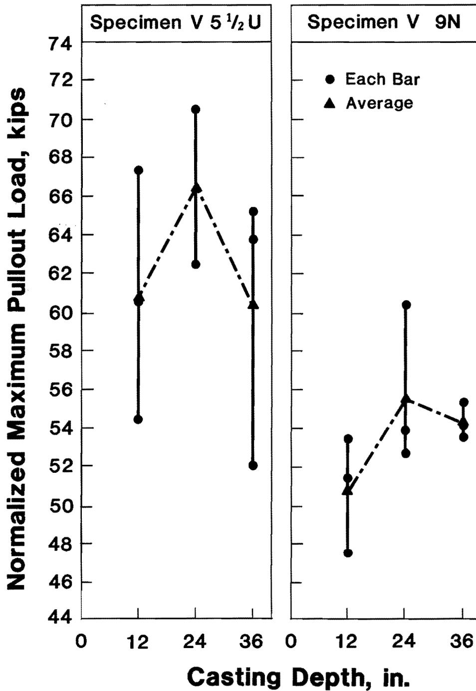
Fig. 6.41 Normalized maximum pullout load versus casting depth for bars from Series V
