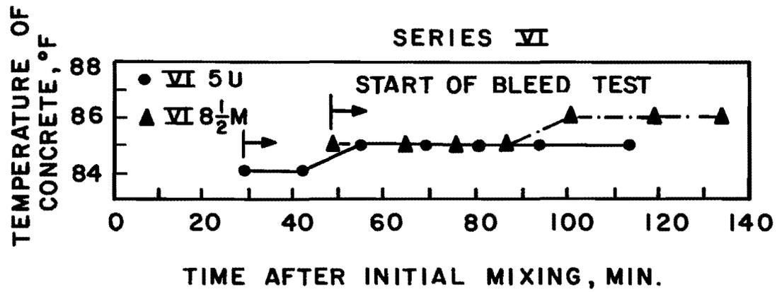
Fig. 6.18f Temperature of concrete with time during bleed tests for Series VI
