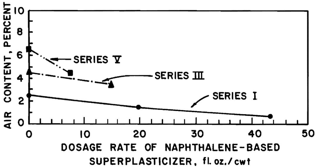
Fig. 6.19 Effect of naphthalene-based superplasticizer on air content of concrete
