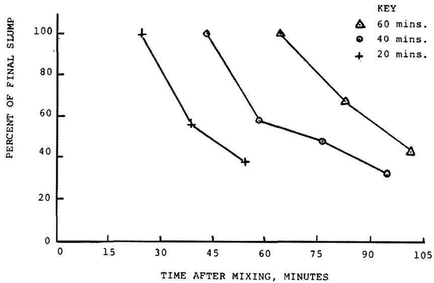
Fig. 2.15 Effect of time of addition of superplasticizer on slump loss [19]
