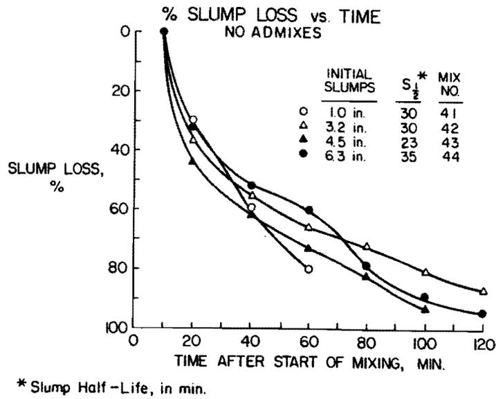
Fig. 2.10 Percent slump loss versus time for various initial slump values [25]
