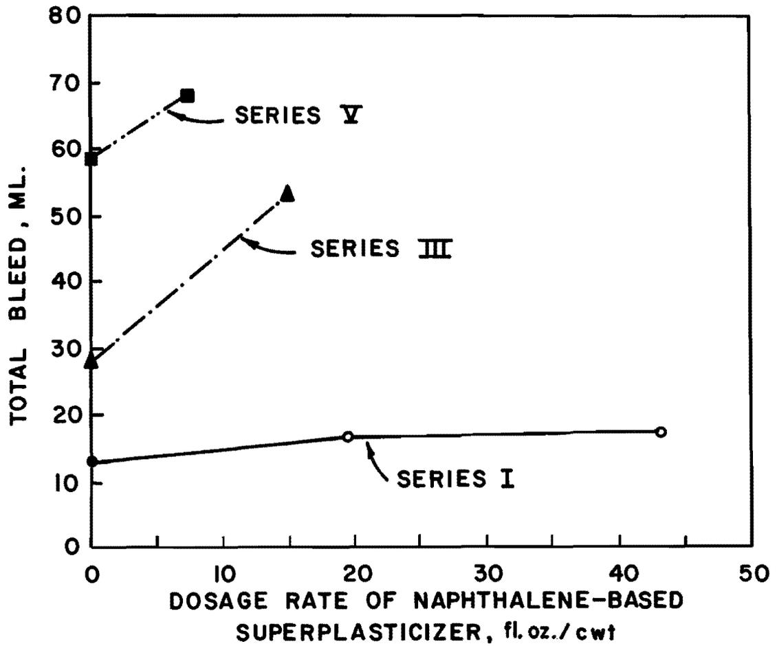
Fig. 6.21 Effect of naphthalene-based superplasticizer on the bleeding of concrete
