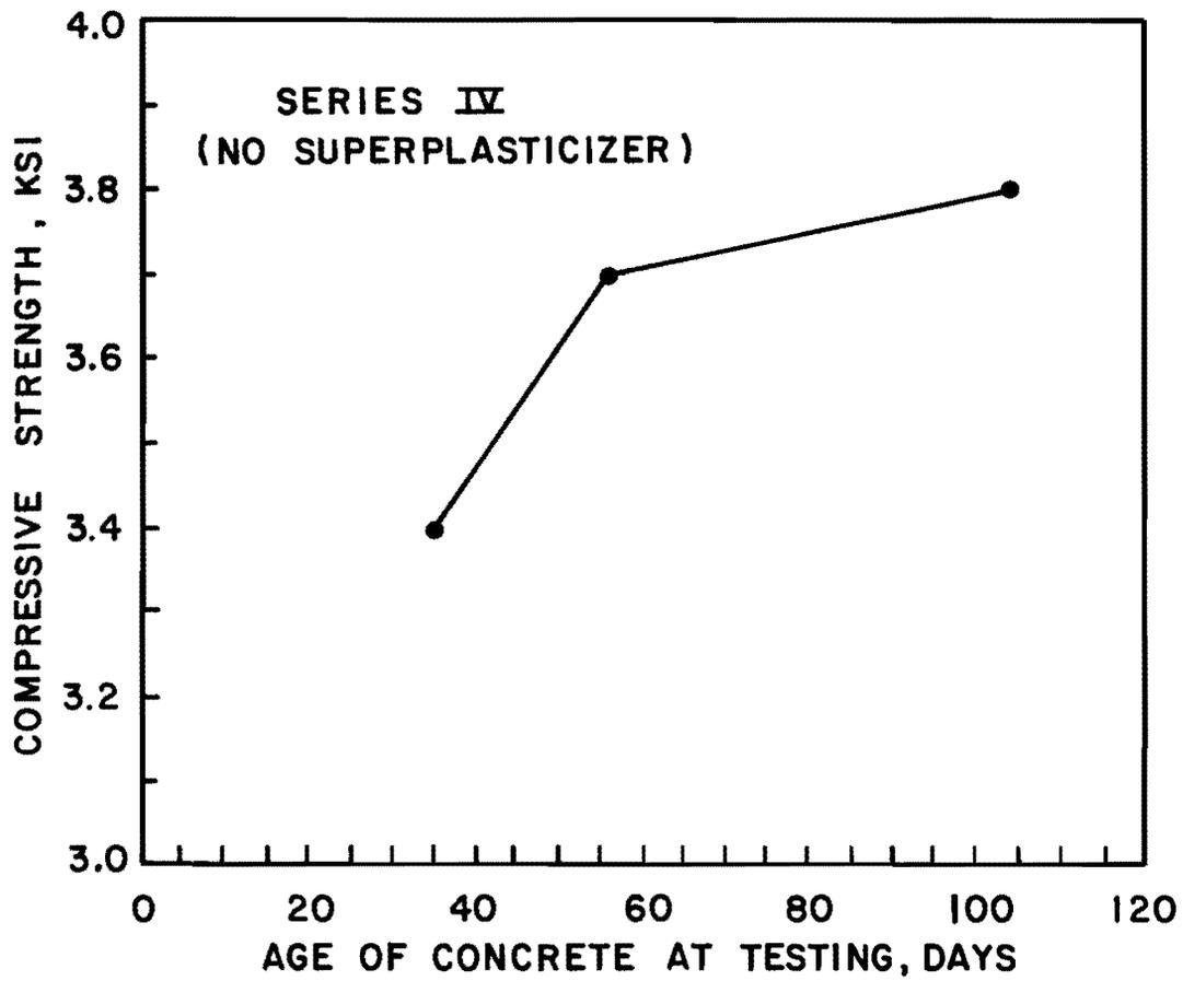
Fig. 6.25 Compressive strengths of cylinders from Series IV
