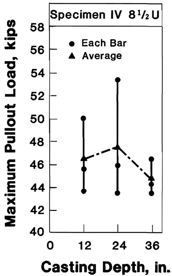
Fig. 6.35 Maximum pullout load versus casting depth for bars from Series IV
