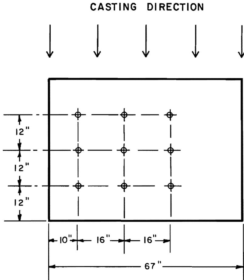
Fig. 3.2 Casting depth and casting direction
