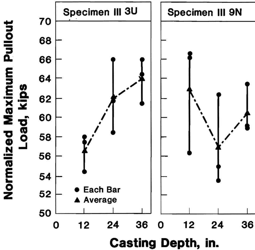
Fig. 6.40 Normalized maximum pullout load versus casting depth for bars from Series III
