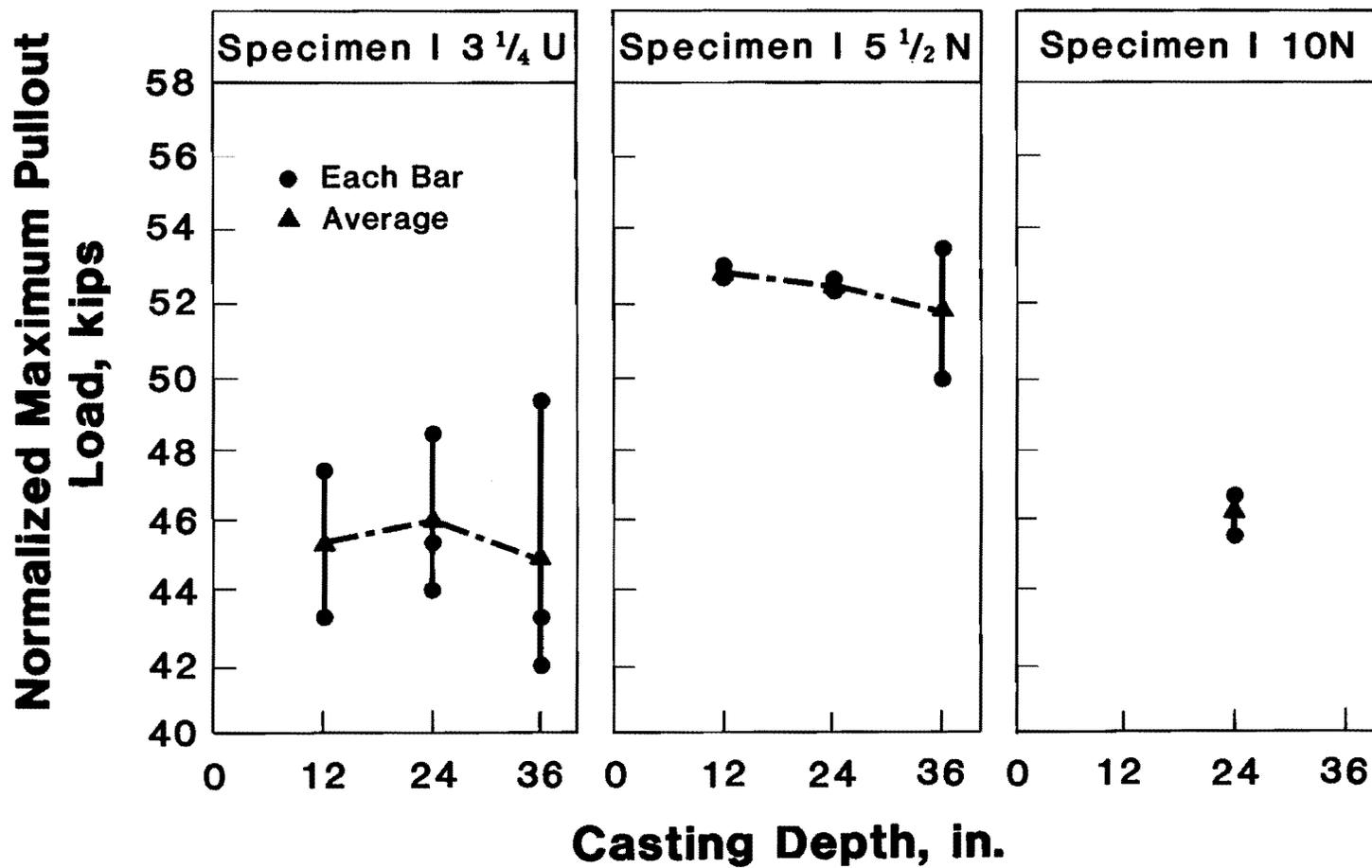
Fig. 6.38 Normalized maximum pullout load versus casting depth for bars from Series I
