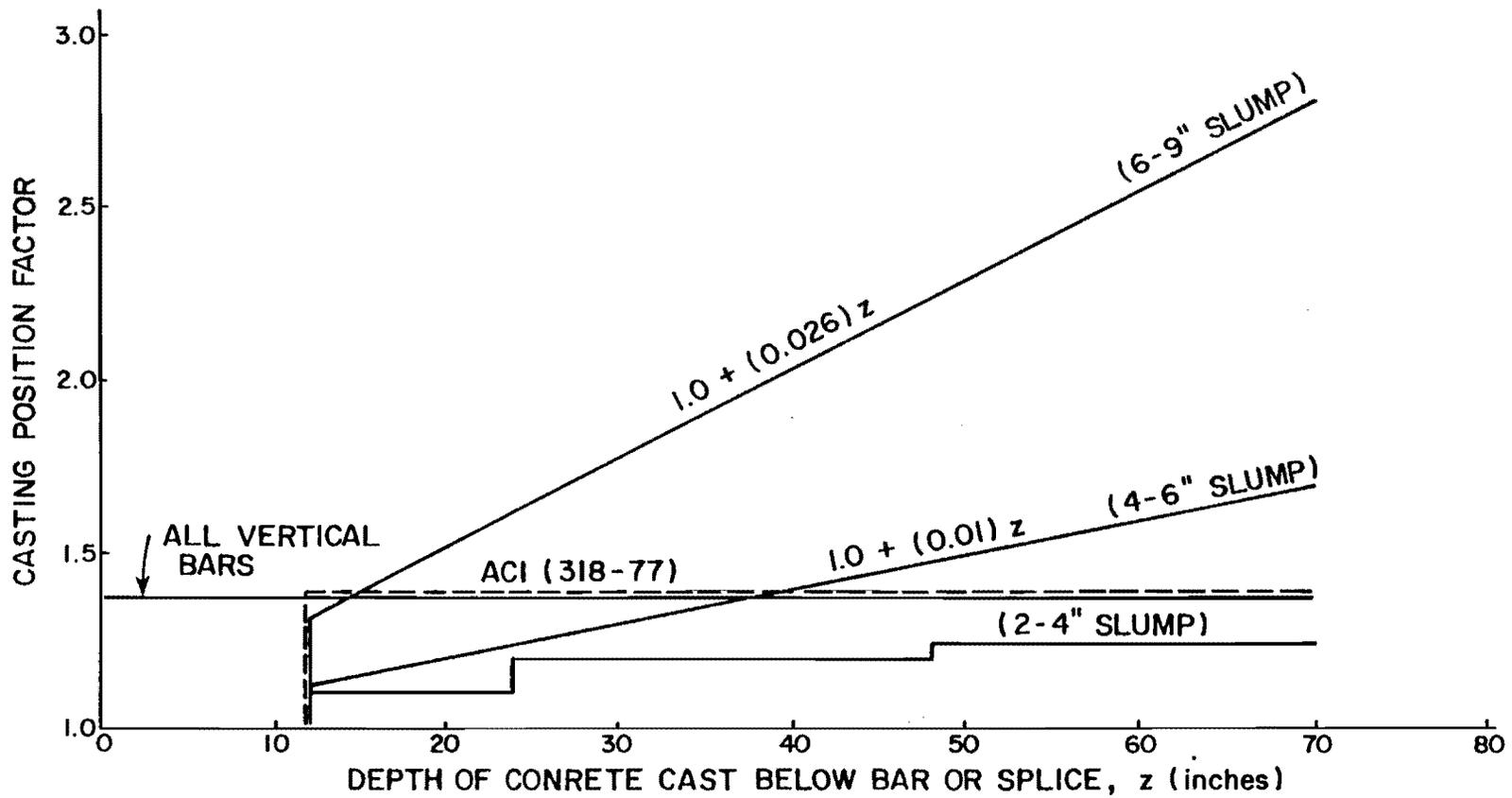
Fig. 2.6 Recommended casting position factors for all ranges of slump investigated [17]
