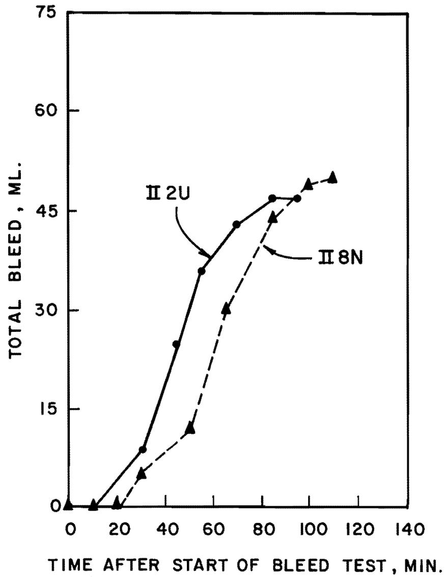
Fig. 5.3 Bleed test results for time of addition of 55 minutes
