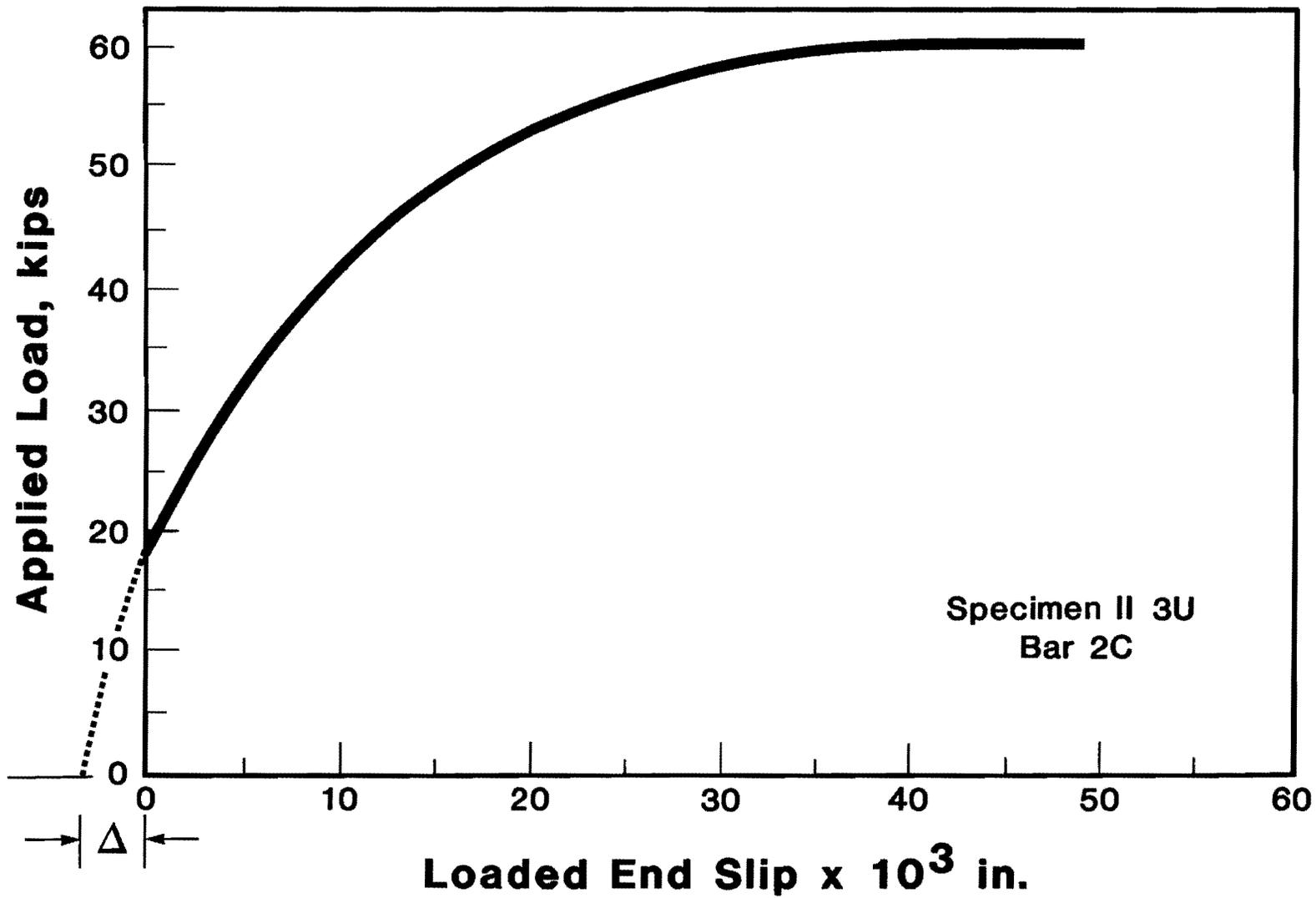
Fig. B.2 Correction to loaded end slip curve
