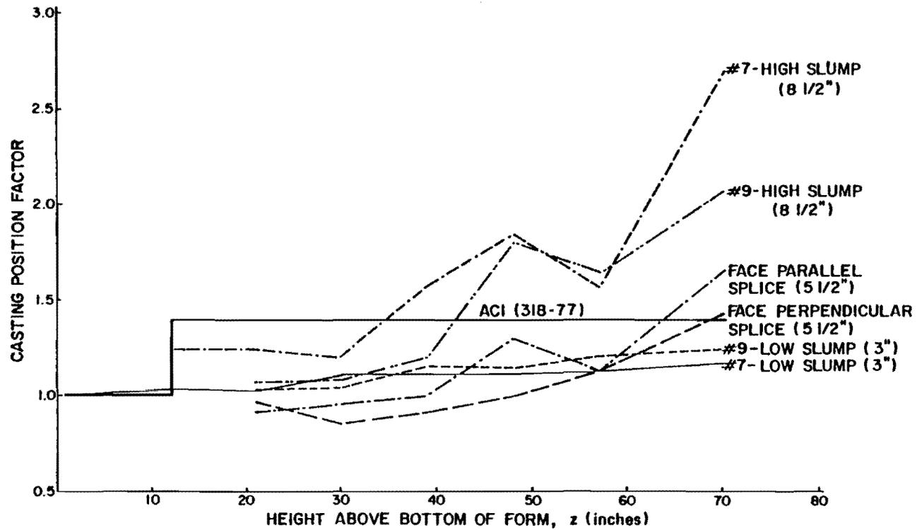
Fig. 2.5 Casting position factor versus bar height for all tests [17]
