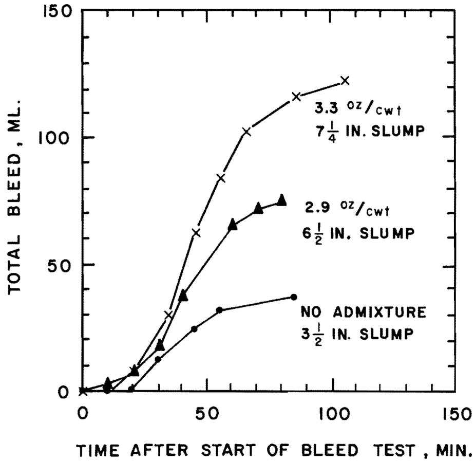
Fig. 2.18 Effect of naphthalene-based superplasticizer on bleeding of concrete for various dosage rates [24]
