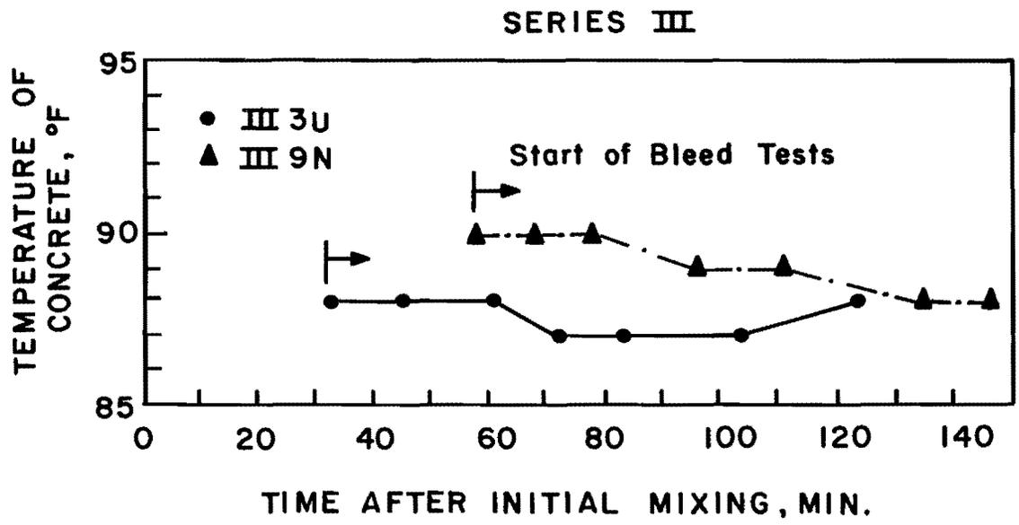
Fig. 6.18c Temperature of concrete with time during bleed tests for Series III
