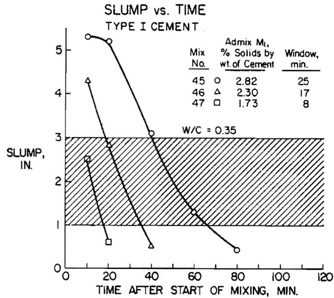
Fig. 2.12 "Slump windows" for concretes with various admixture dosages [25]
