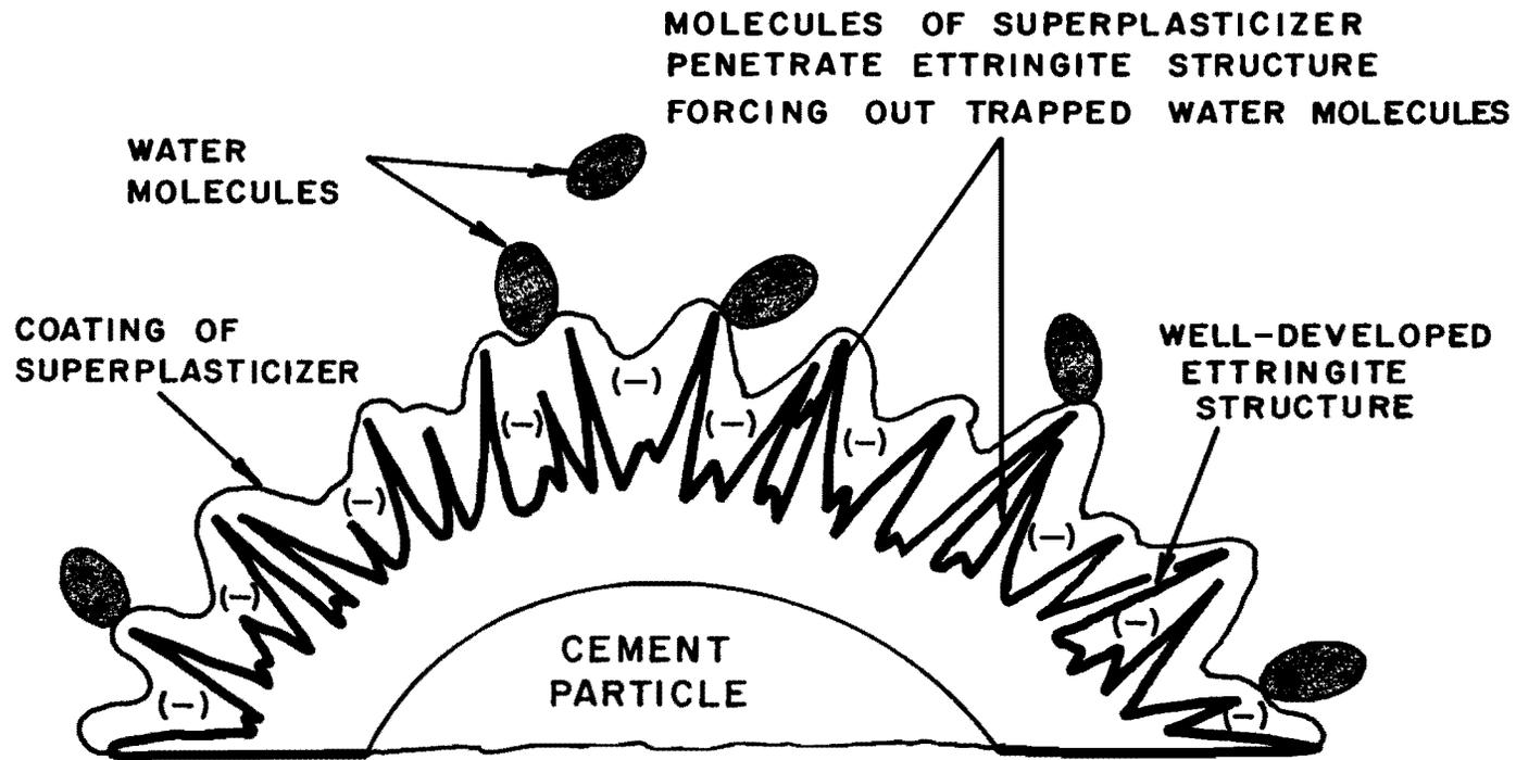
Fig. 6.15 Proposed action of a naphthalene-based superplasticizer when added to concrete 85 minutes after initial mixing
