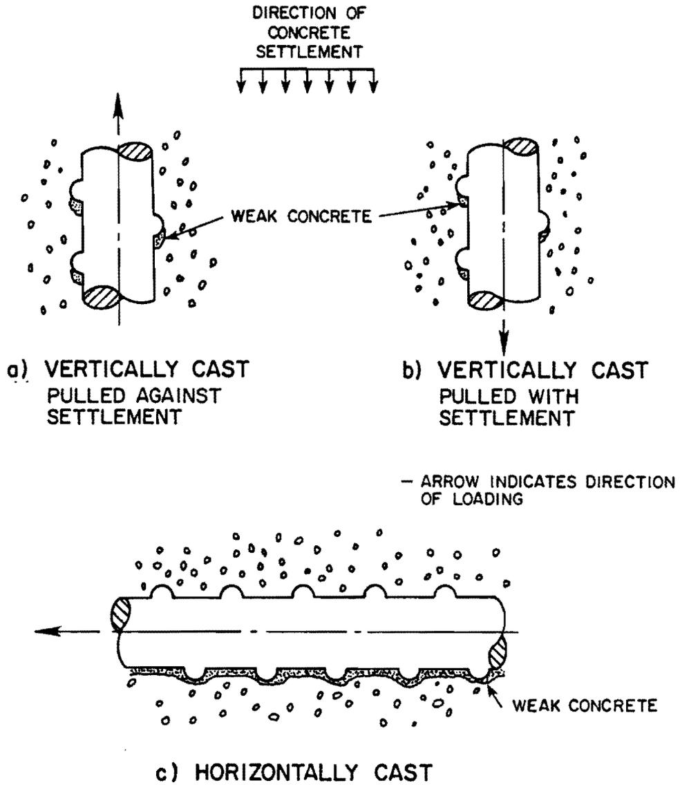
Fig. 1.1 Definition of casting position [17]
