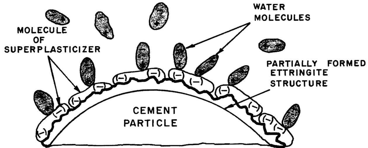
Fig. 6.12 Proposed action of a naphthalene-based superplasticizer when added to concrete 30 minutes after initial mixing
