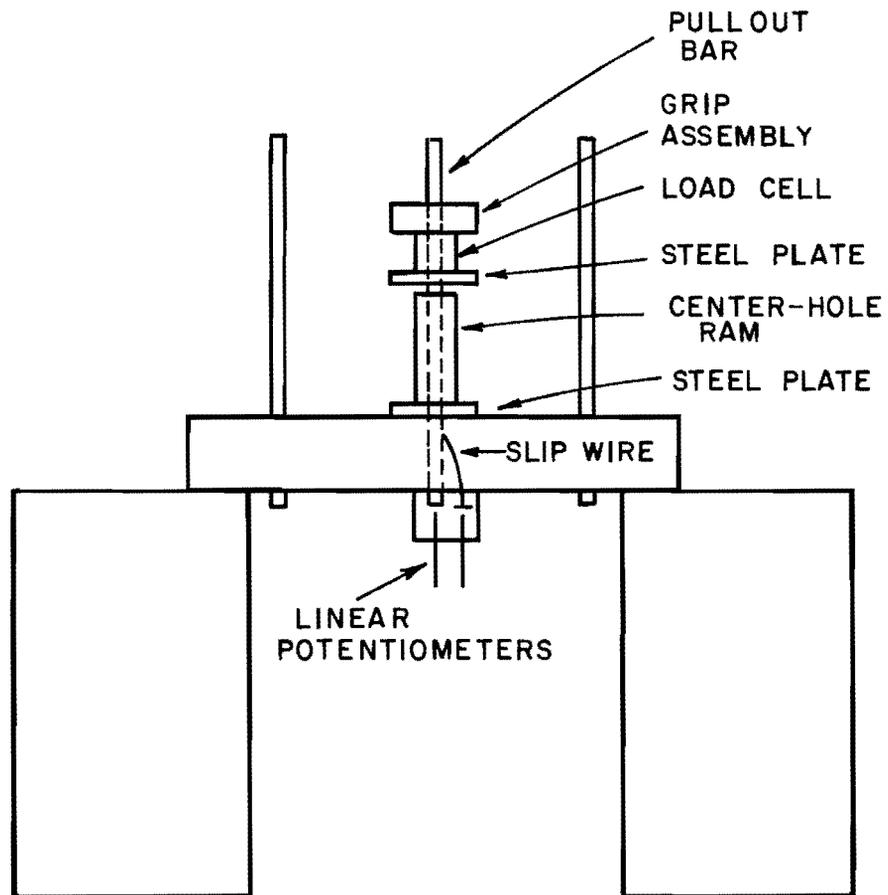
Fig. 3.10 Specimen in place prior to testing
