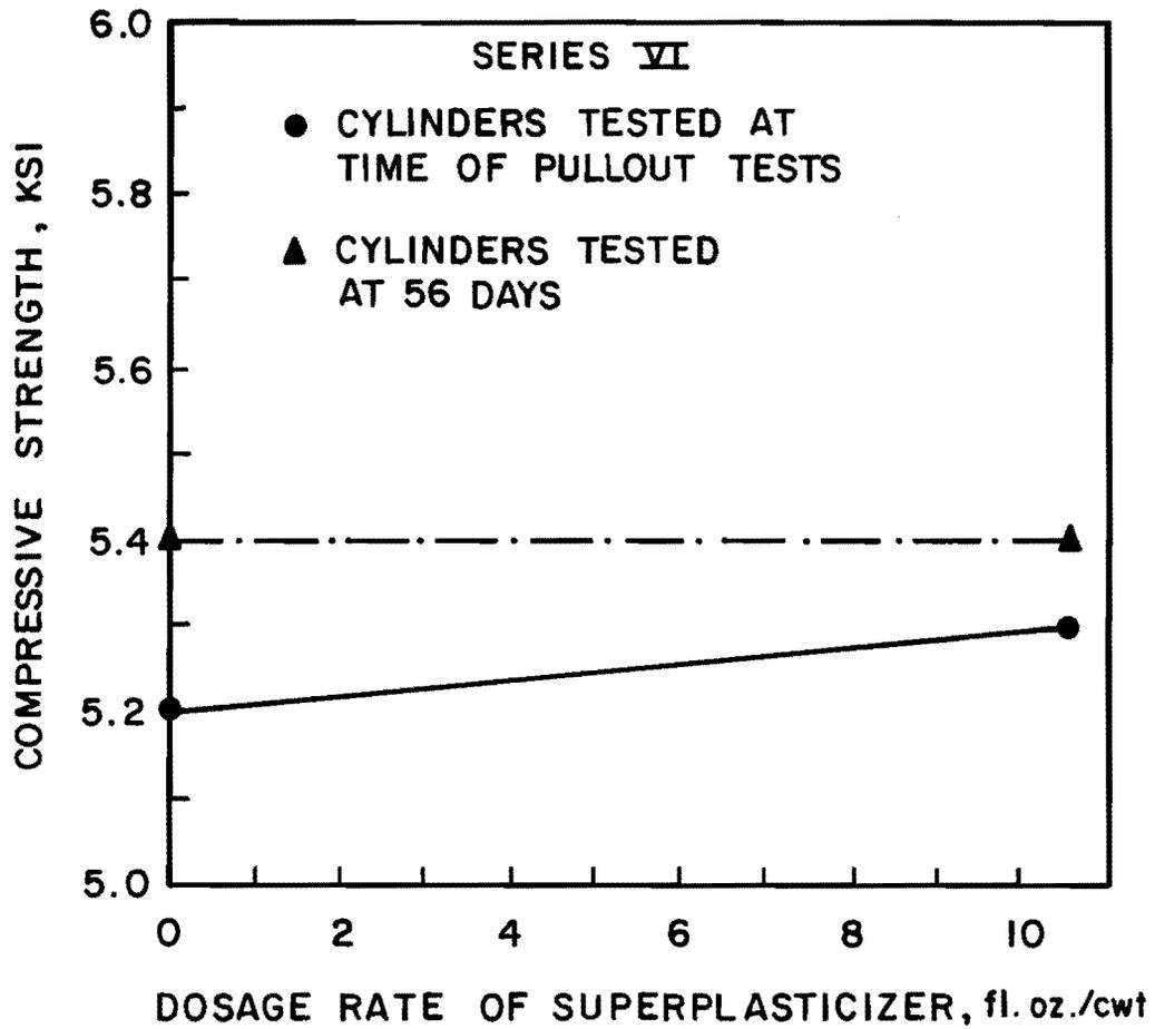
Fig. 6.27 Effect of addition of superplasticizer on compressive strength of concrete for Series VI
