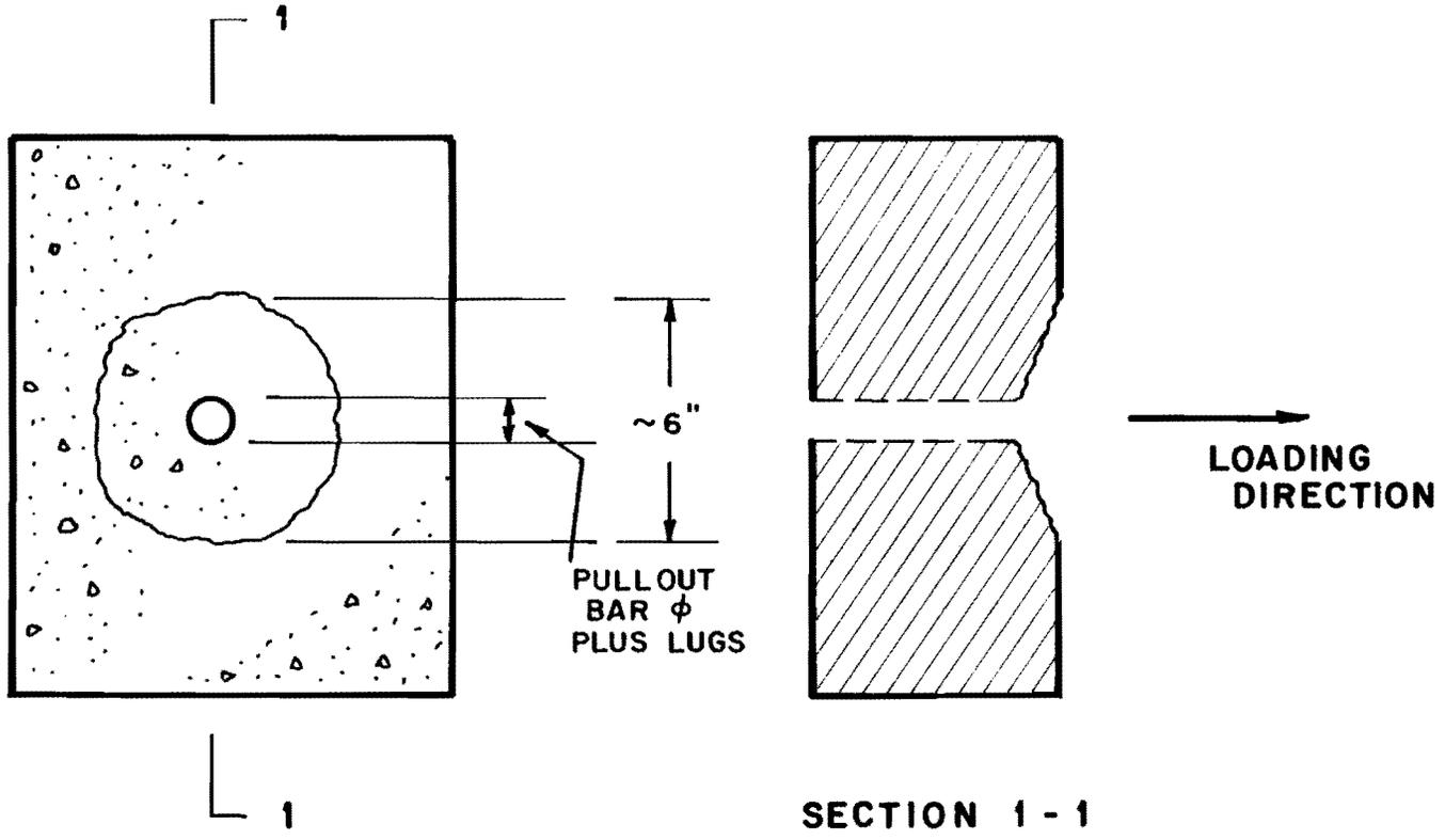
Fig. 4.13 Appearance of failure surface resulting from pullout test
