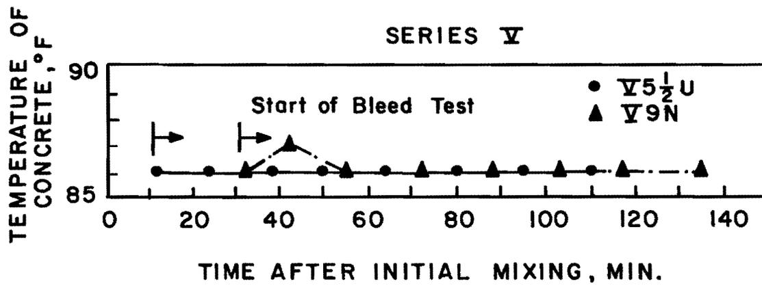
Fig. 6.18e Temperature of concrete with time during bleed tests for Series V
