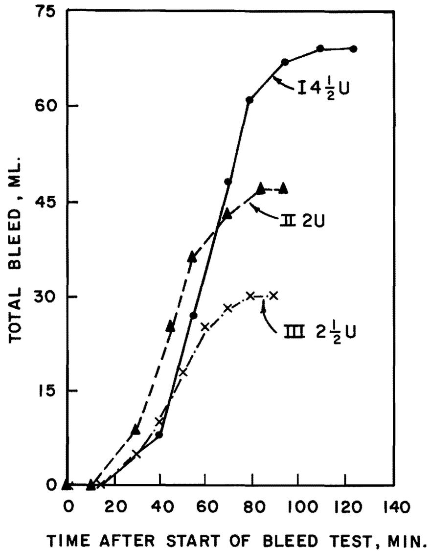
Fig. 5.5 Effect of concrete age on its bleed characteristics (no superplasticizer added)
