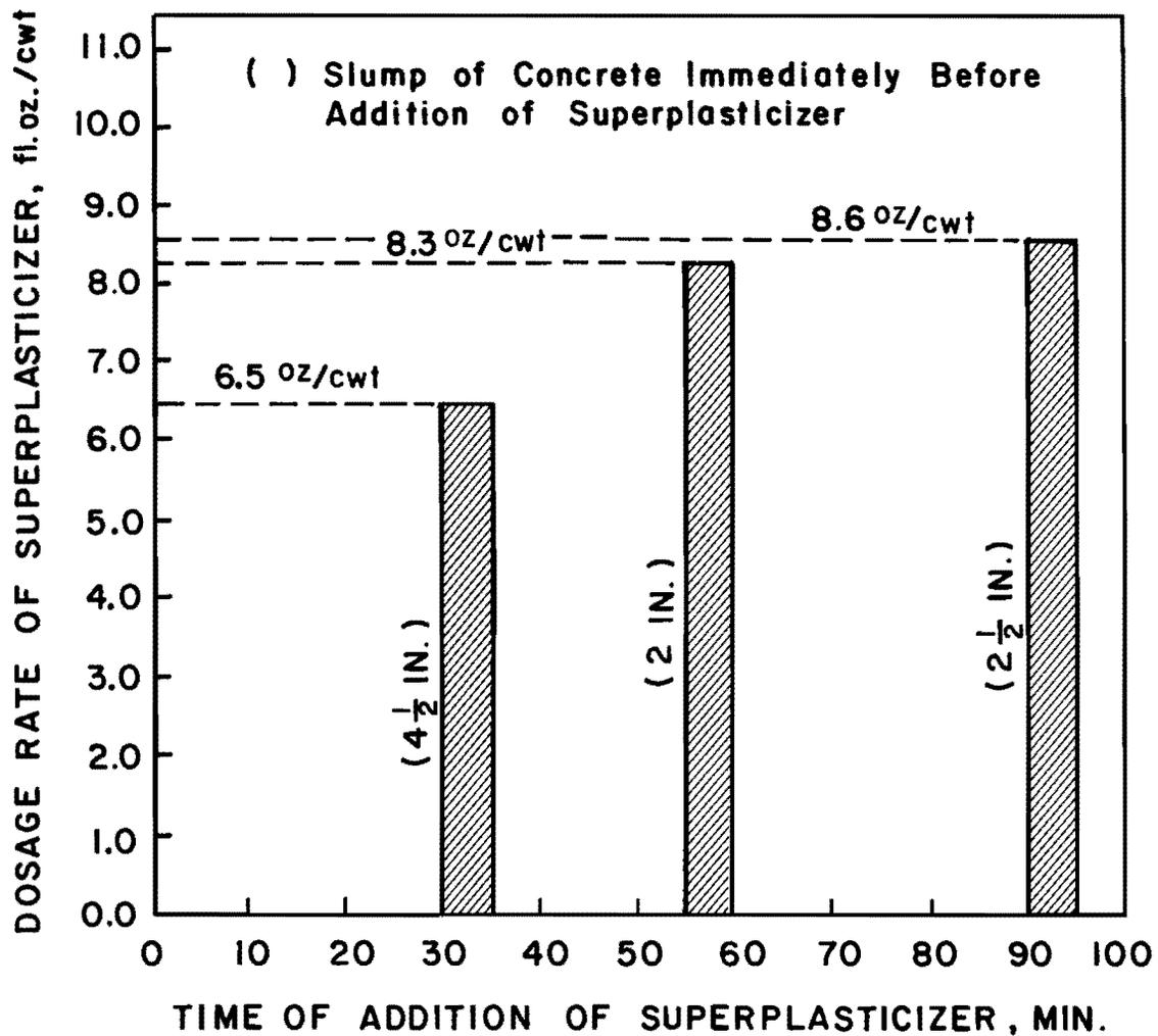
Fig. 6.2 Dosage rate of superplasticizer required to increase the concrete slump to 8-1/2 in.  $\pm$  1/2 in. as a function of time of addition
