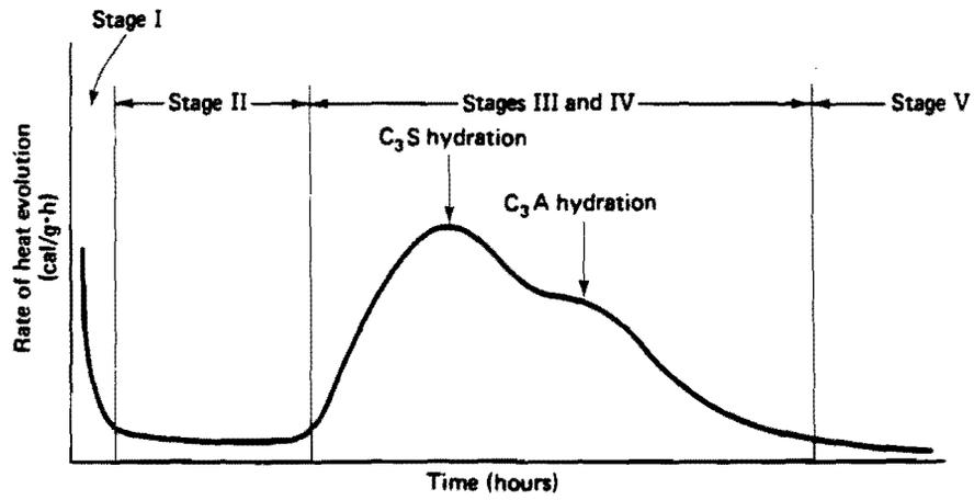
Fig. 5.1 Rate of heat evolution during the hydration of portland cement [23]
