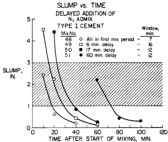
Fig. 2.13 "Slump windows" for concretes with various delay periods [25]
