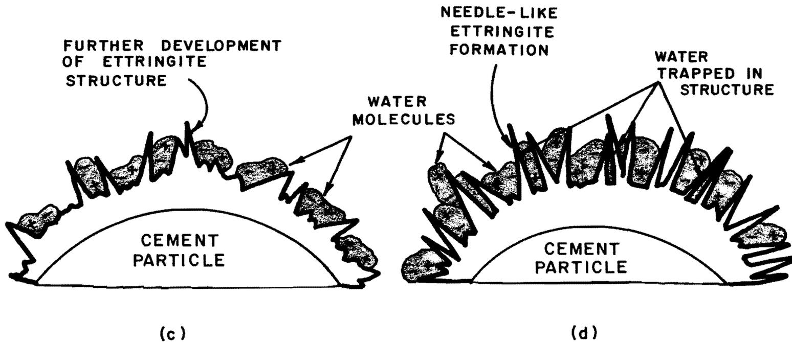
Fig. 6.9 Proposed appearance of cement particle surface:
