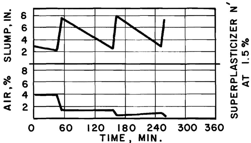
Fig. 2.20 Changes in plastic properties of concrete W/C = 0.42 due to repeated dosages of superplasticizer [27]
