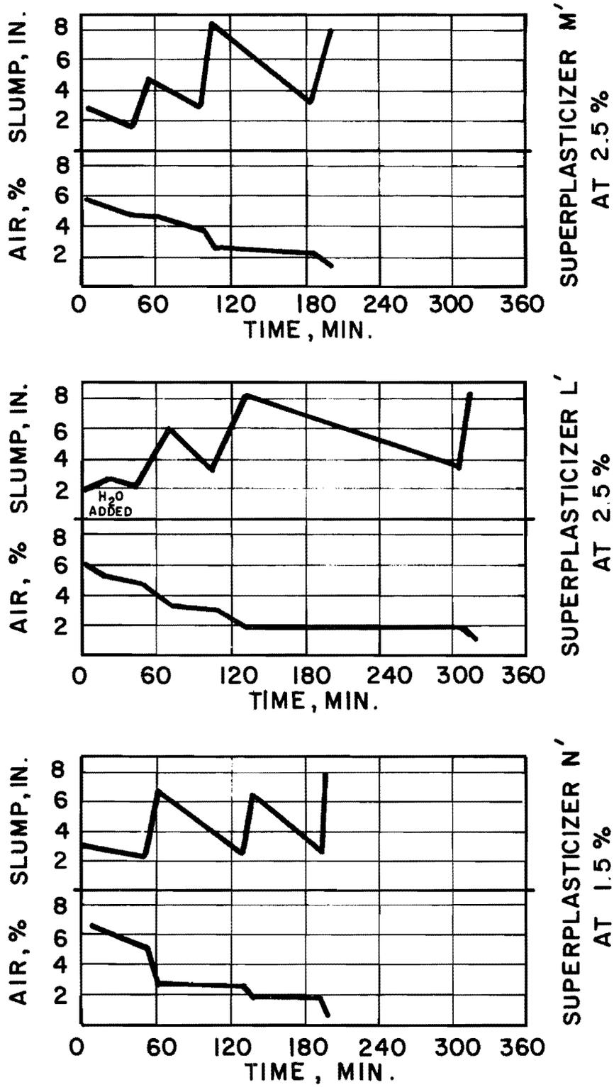
Fig. 2.21 Changes in plastic properties of concrete W/C = 0.55 due to repeated dosages of superplasticizer [27]
