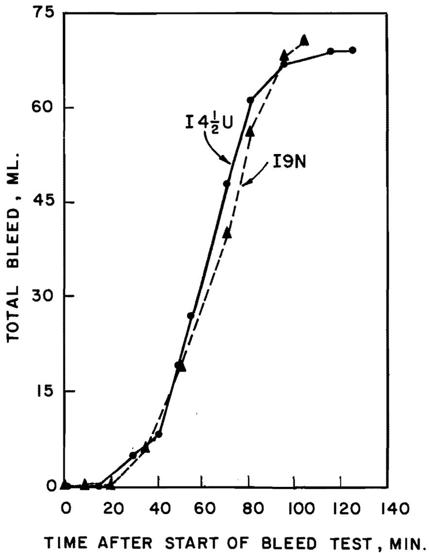
Fig. 5.2 Bleed test results for time of addition of 30 minutes
