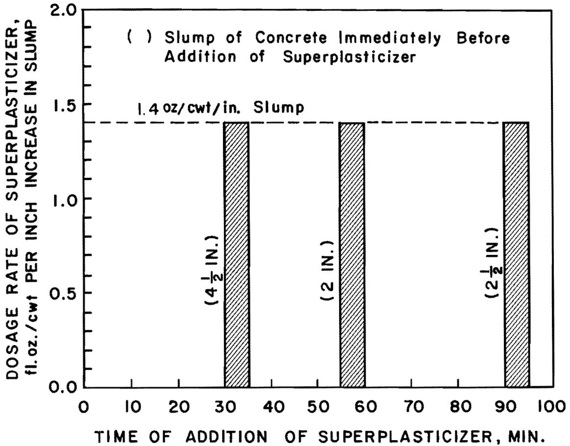
Fig. 6.3 Dosage rate of superplasticizer required per inch increase in slump to increase the concrete slump to  $8\frac{1}{2}$  in.  $\pm$   $\frac{1}{2}$  in. as a function of time of addition
