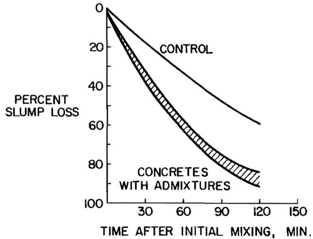
Fig. 2.8 Slump loss versus time for concrete containing 376 lbs cement per cubic yard [25]
