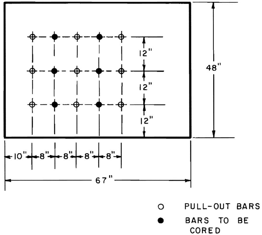
Fig. 3.6 Location of bars to be cored
