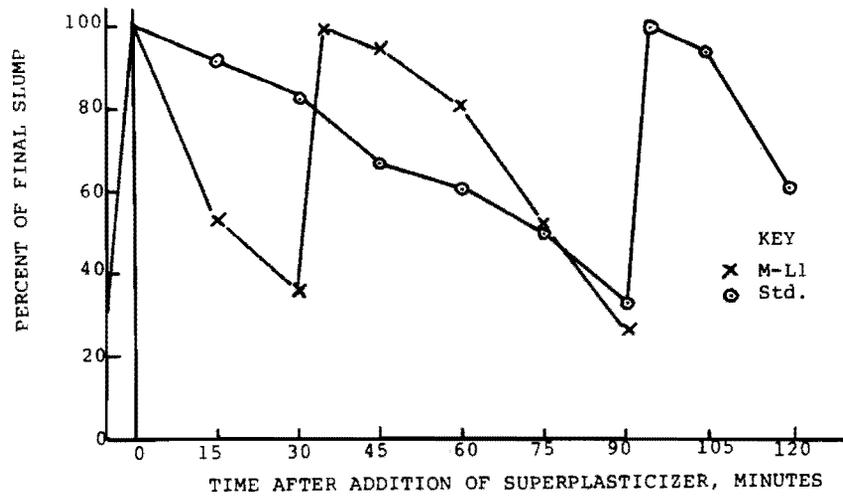
Fig. 2.17 Effect of redosage on slump loss [19]
