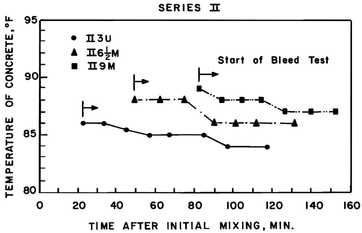
Fig. 6.18b Temperature of concrete with time during bleed tests for Series II
