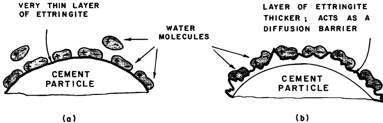
Fig. 6.9 Proposed appearance of cement particle surface:
