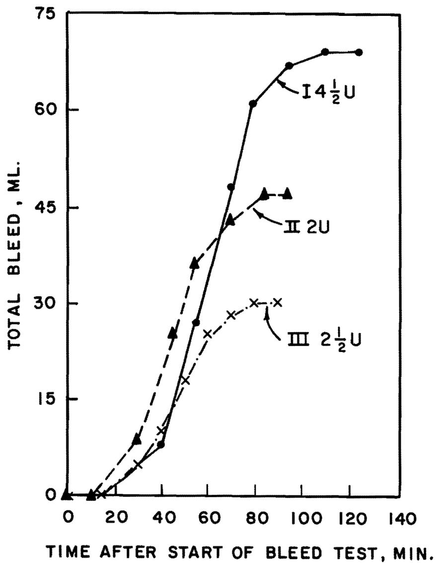
Fig. 6.5 Effect of concrete age on its bleed characteristics (no superplasticizer added)
