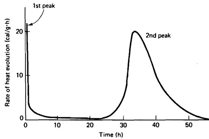
Fig. 6.10 Rate of heat evolution during the hydration of tricalcium aluminate with gypsum [23]
