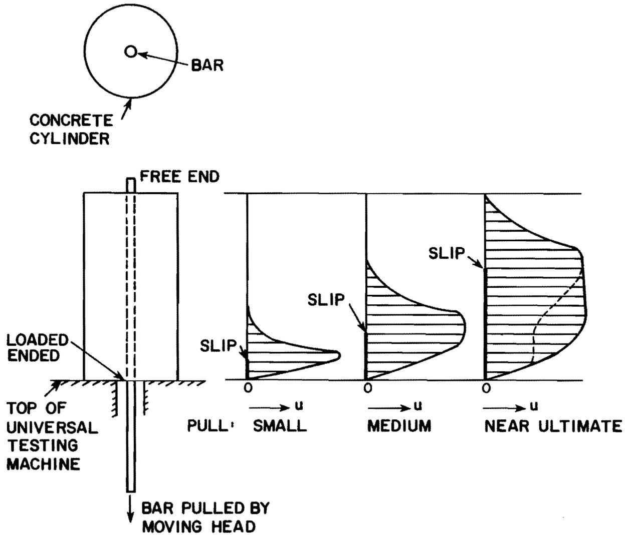
Fig. 2.3 Bond pullout test with bond stress distribution [9]
