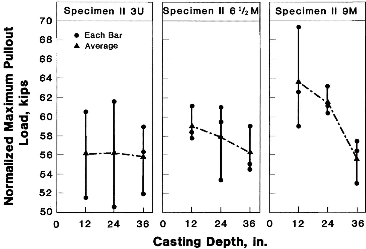
Fig. 6.39 Normalized maximum pullout load versus casting depth for bars from Series II
