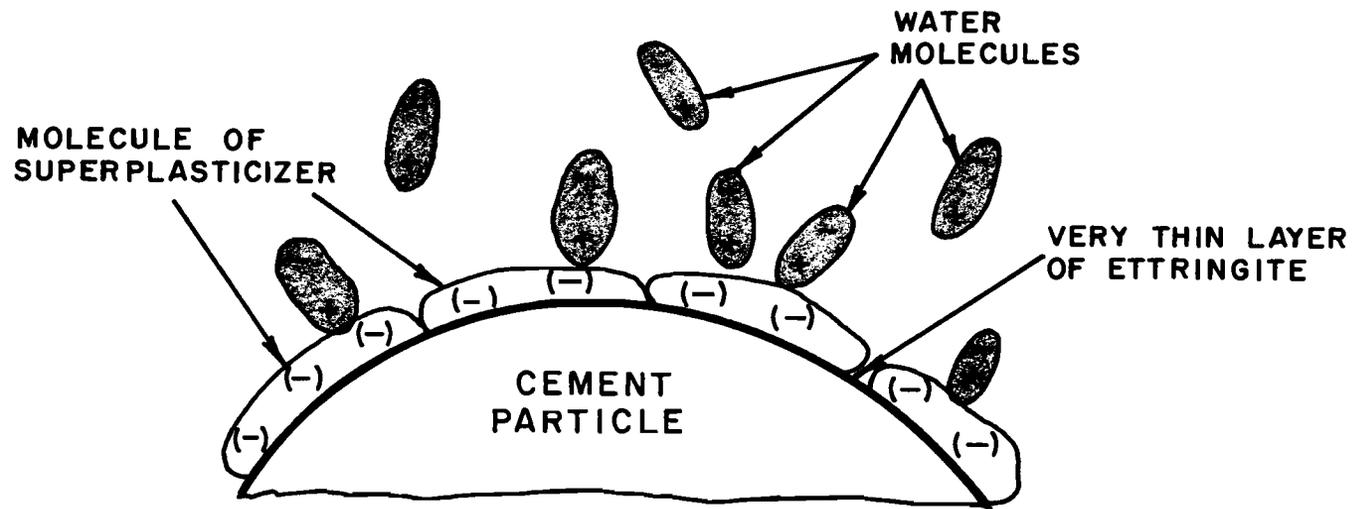
Fig. 6.11 Proposed action of a naphthalene-based superplasticizer when added to concrete immediately after initial mixing
