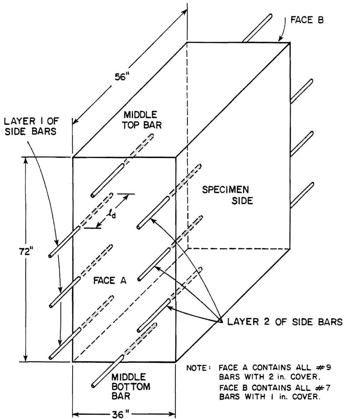
Fig. 2.4 Schematic representation of specimen for high slump tests [17]
