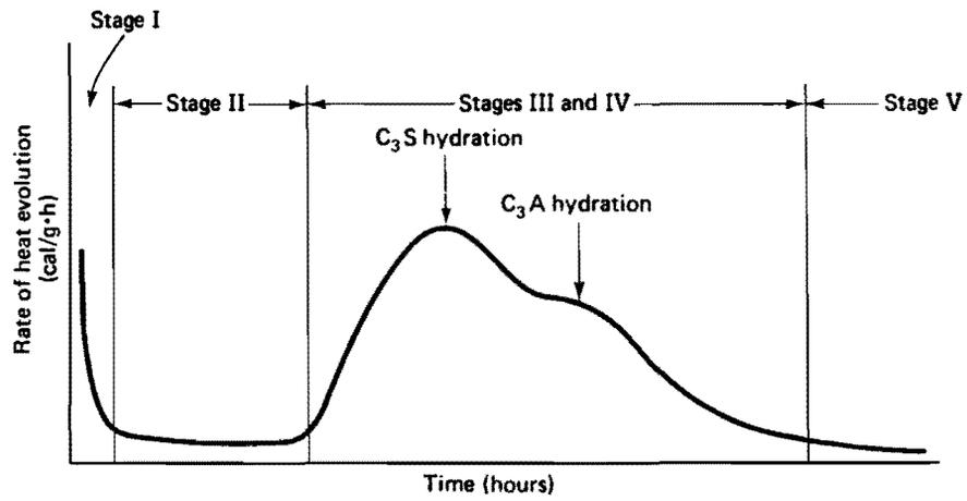
Fig. 6.8 Rate of heat evolution during the hydration of portland cement [23]
