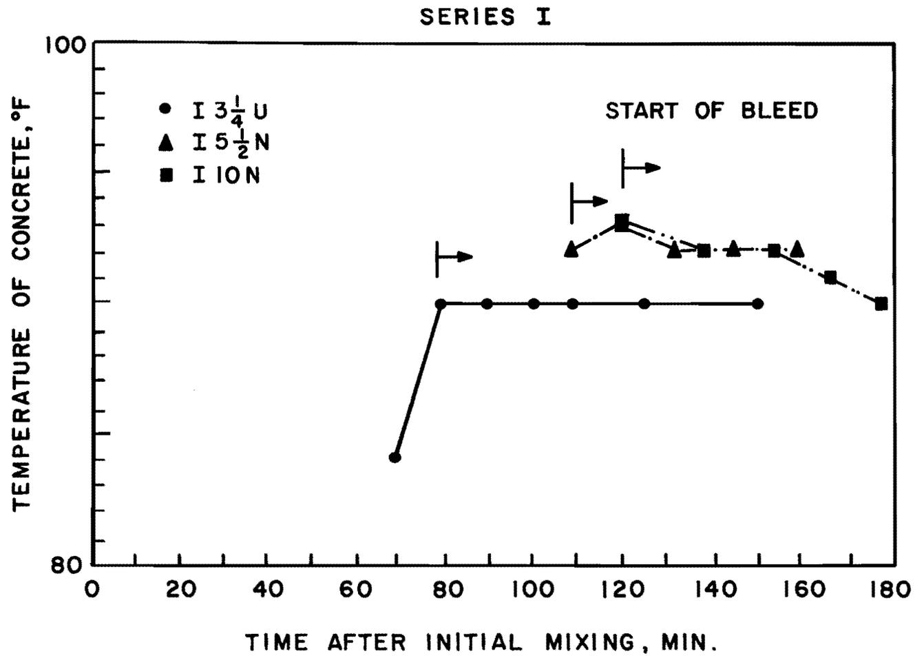
Fig. 6.18a Temperature of concrete with time during bleed tests for Series I
