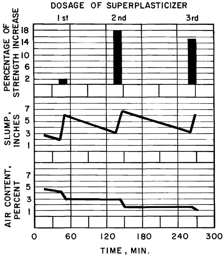
Fig. 2.22 Effect of repeated dosages of superplasticizer on slump, air content, and compressive strength of concrete [14]
