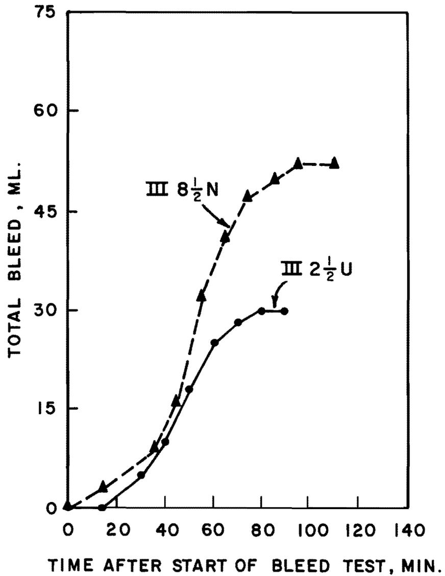
Fig. 5.4 Bleed test results for time of addition of 85 minutes
