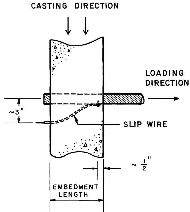
Fig. 3.3 Location of slip wire within specimen
