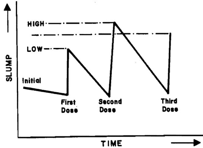
Fig. 2.16 Effect of repeated dosages of superplasticizer on slump of concrete [27]
