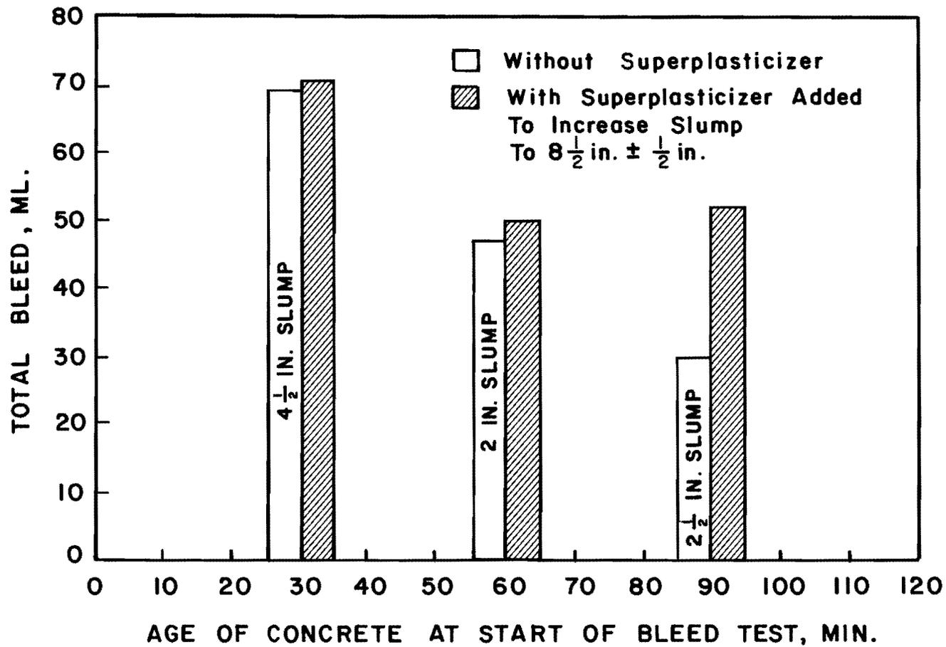
Fig. 6.7 Effect of time of addition of superplasticizer on bleeding of concrete
