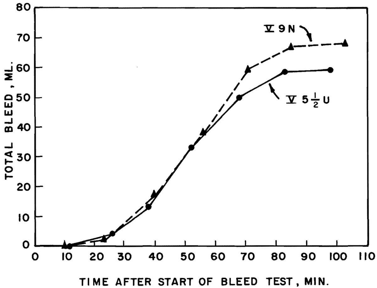
Fig. 4.5 Bleed versus time curves for specimens of Series V
