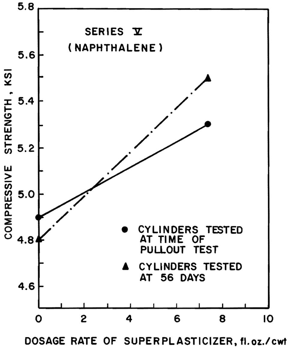
Fig. 6.26 Effect of addition of superplasticizer on compressive strength of concrete for Series V
