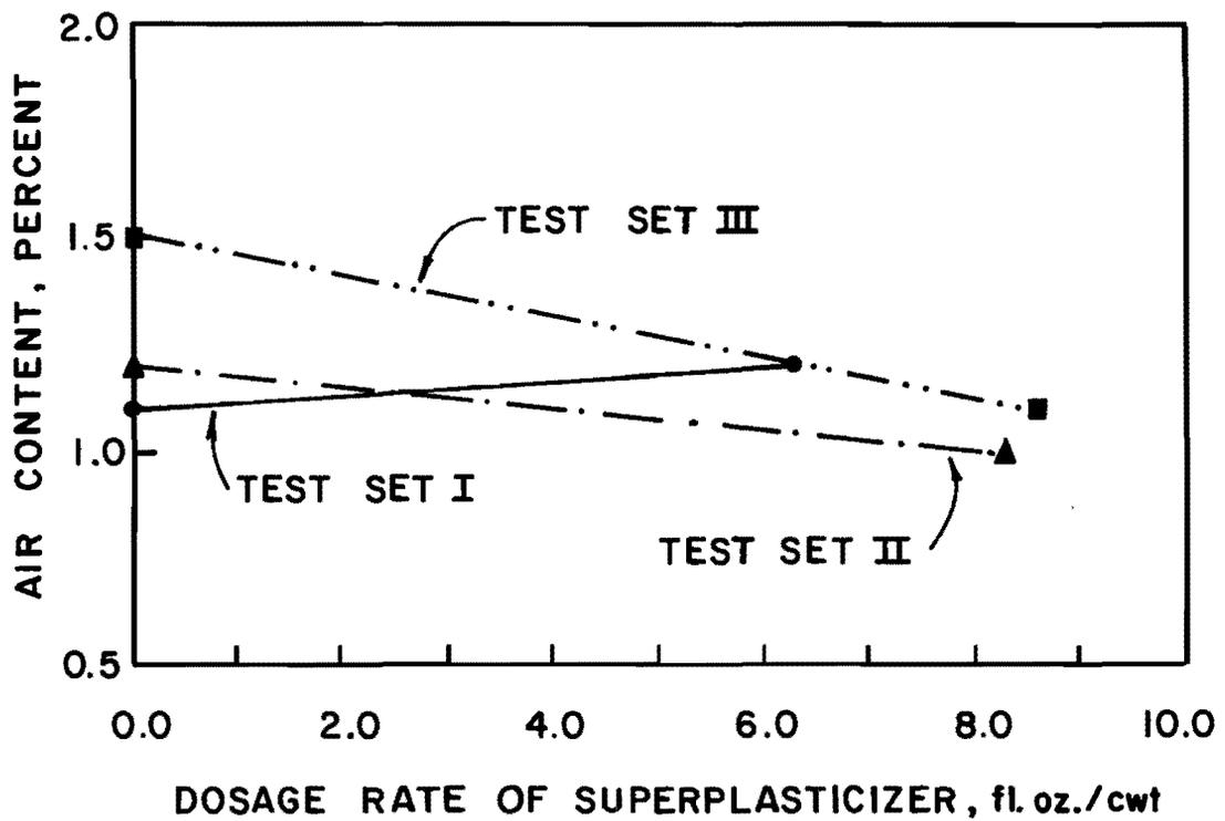
Fig. 6.4 Air content of concrete as a function of dosage rate of superplasticizer
