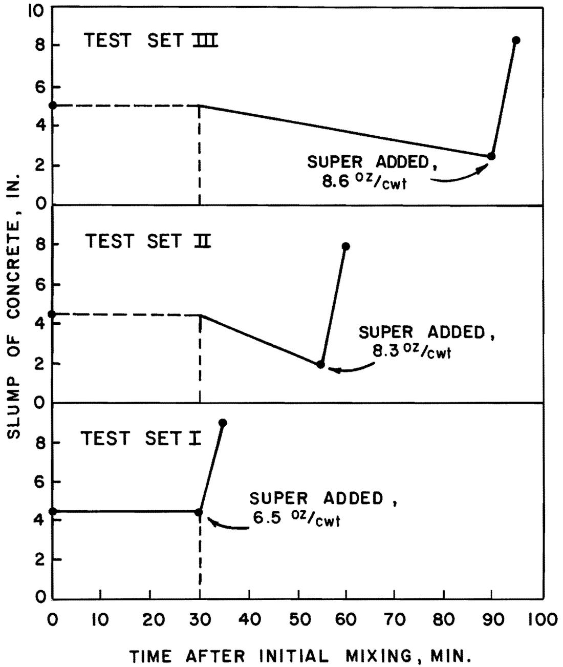
Fig. 6.1 Slump behavior of concrete from time of initial mixing to time of addition of superplasticizer for each test set
