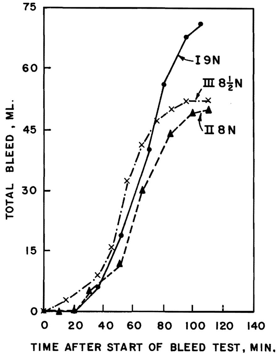
Fig. 6.6 Effect of concrete age on the bleeding of concrete containing superplasticizer
