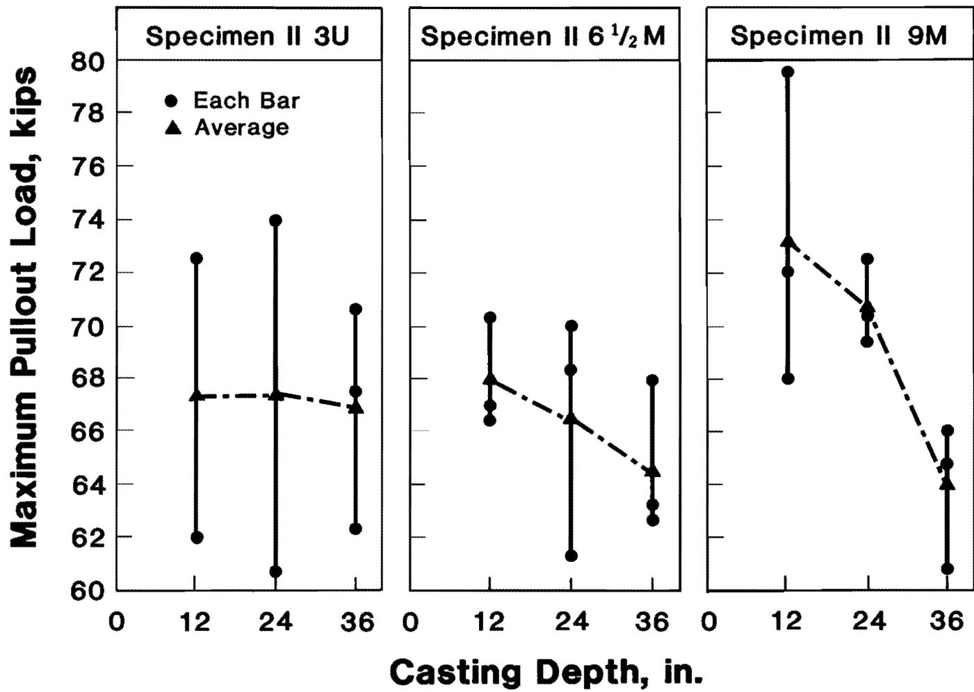
Fig. 6.33 Maximum pullout load versus casting depth for bars from Series II
