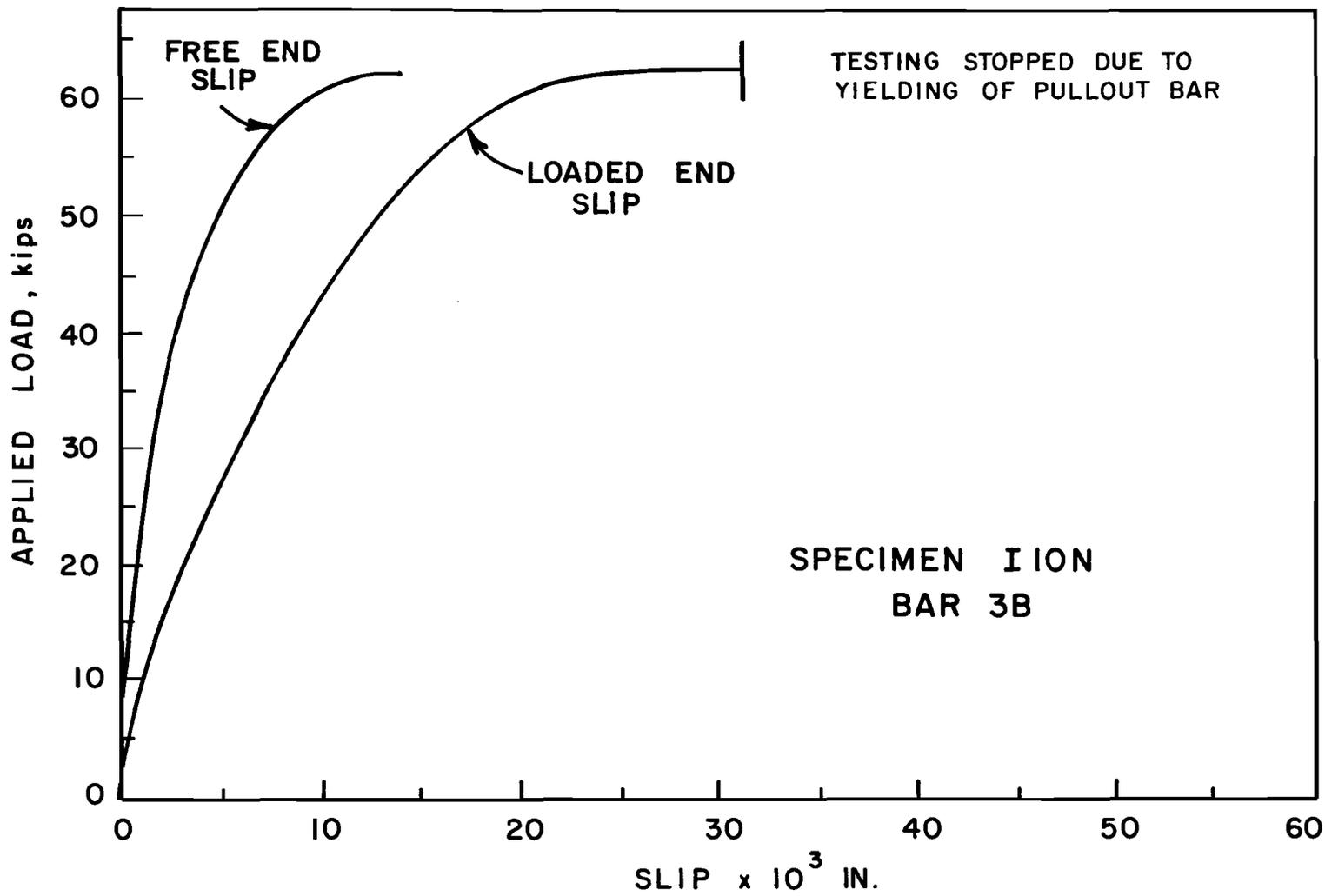
Fig. 4.8 Typical load-slip curve
