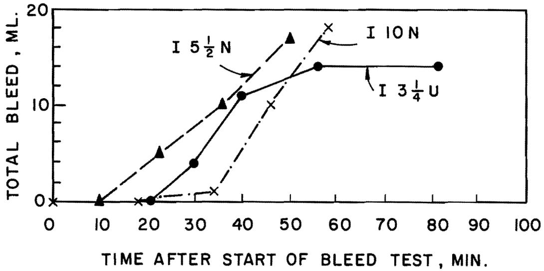
Fig. 4.1 Bleed versus time curves for specimens of Series I
