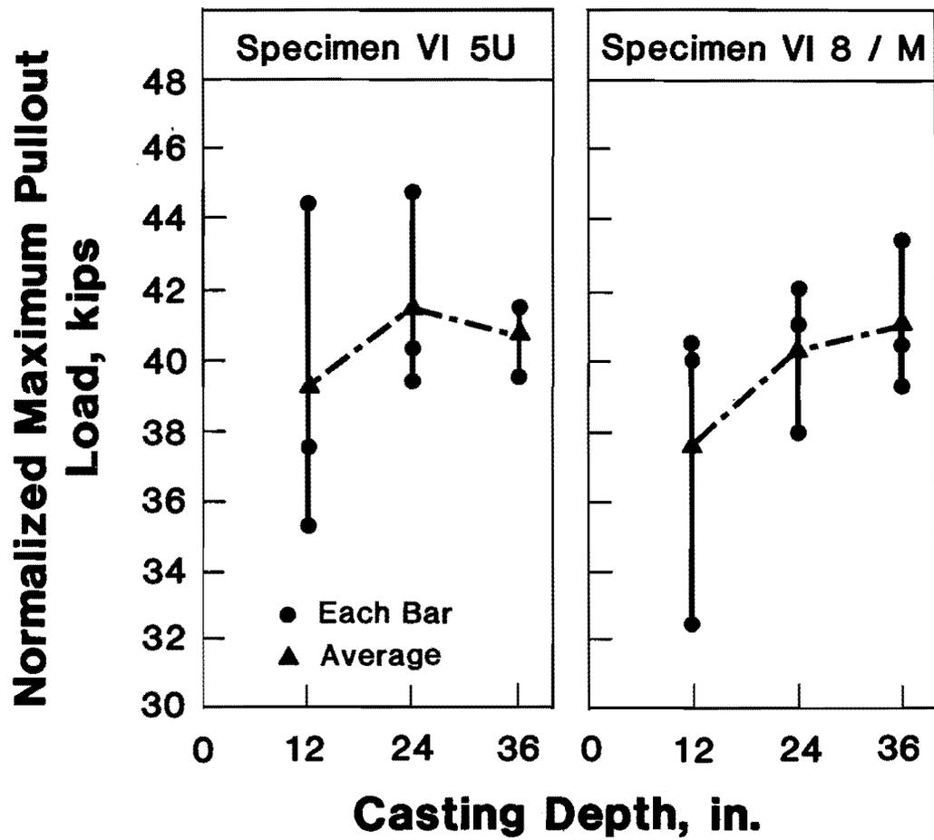
Fig. 6.42 Normalized maximum pullout load versus casting depth for bars from Series VI
