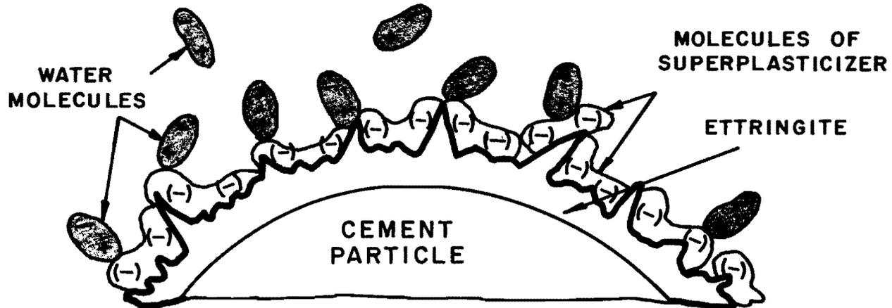
Fig. 6.14 Proposed action of a naphthalene-based superplasticizer when added to concrete 55 minutes after initial mixing
