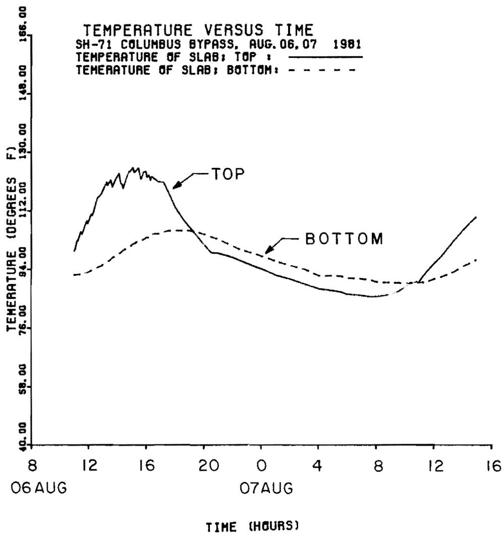
Fig 2.23. Temperature of top and bottom of concrete slab versus time, Summer 1981.
