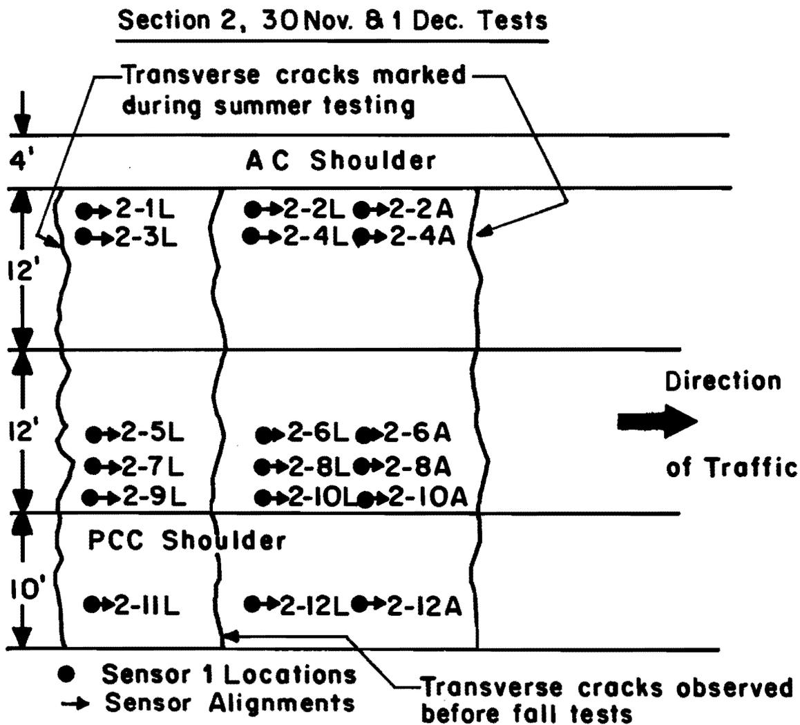
Fig 2.20. Layout plan of test locations in Fall 1981, section no. 2.
