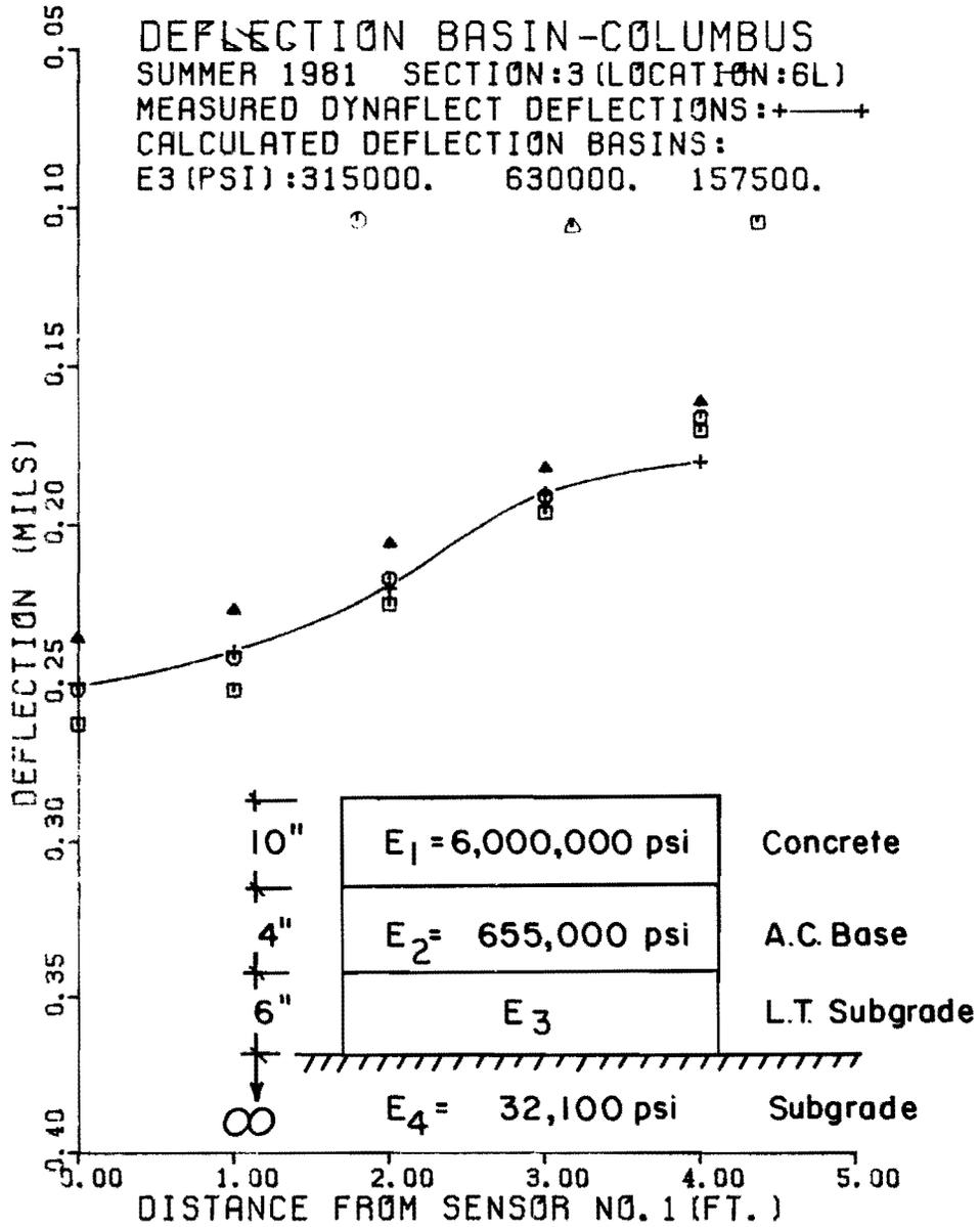
Fig 5.6. Effect of change of  $E_3$  on calculated basin (infinite subgrade).
