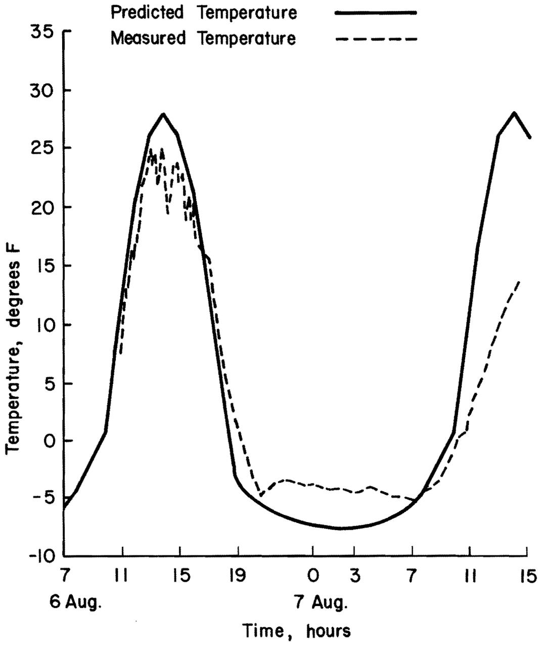
Fig 4.11(a). Variation in temperature differential based on Summer 1981 data, Columbus Bypass, SH-71.
