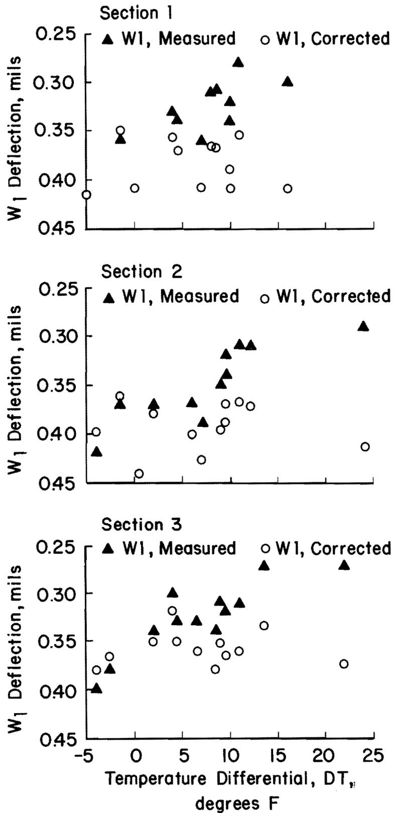
Fig E.2. Measured and corrected  $W_1$  deflections at location 1L, Columbus bypass, SH-71 (1981 data).
