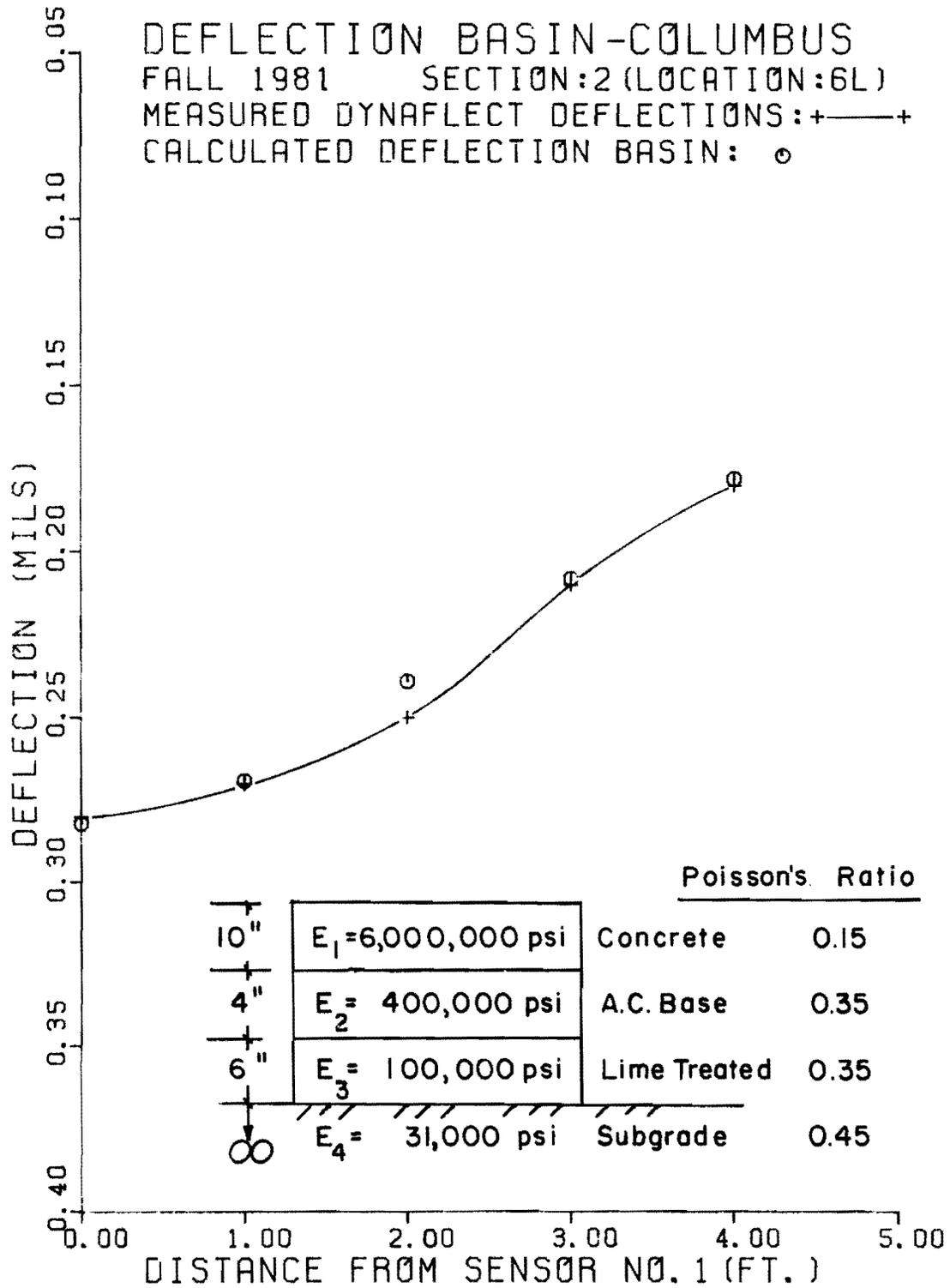
Fig F.7. Measured and calculated deflection basins (Example 5).
