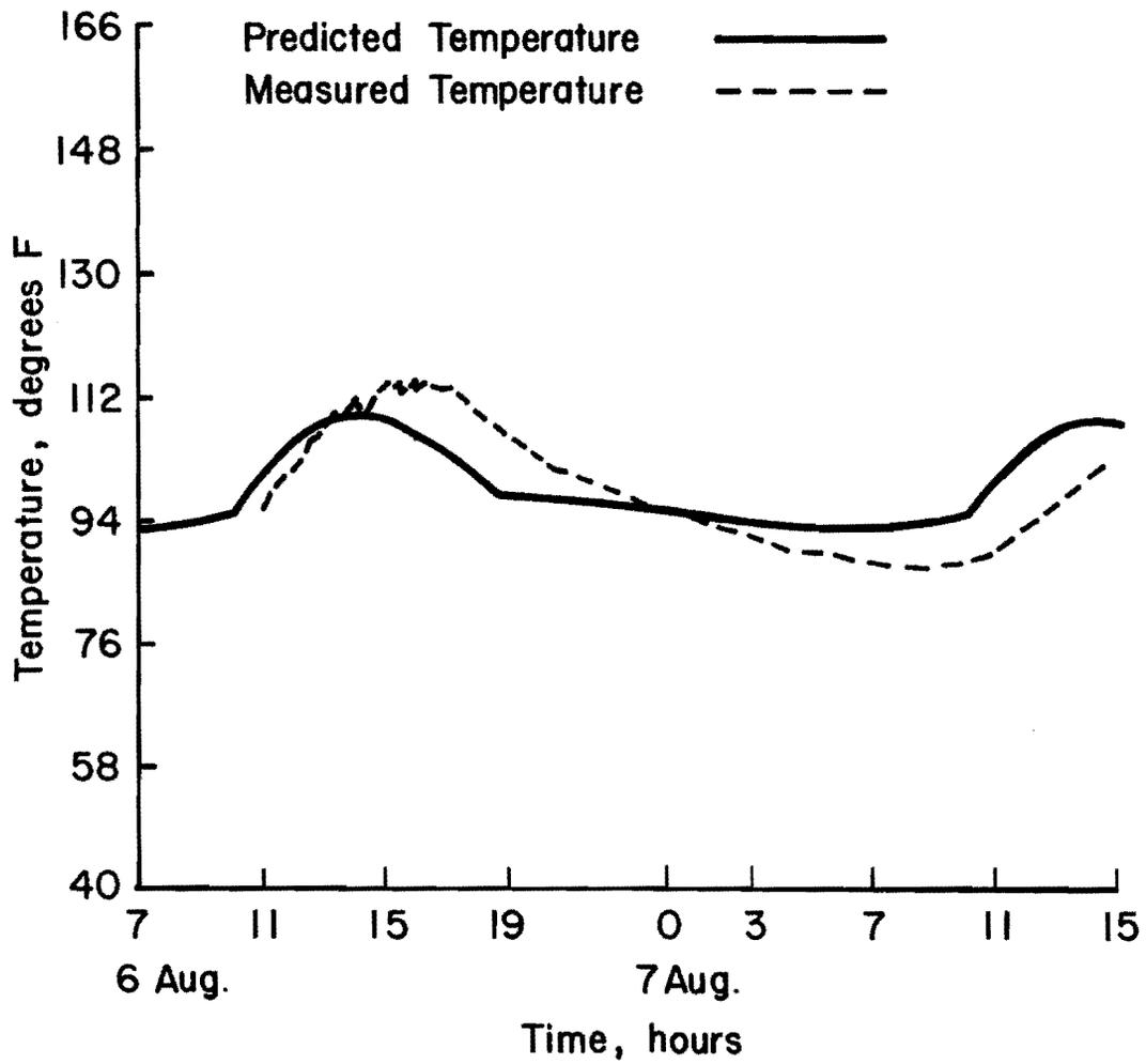
Fig 4.12(a). Variation in mid-depth temperature based on Summer 1981 data, Columbus Bypass, SH-71.
