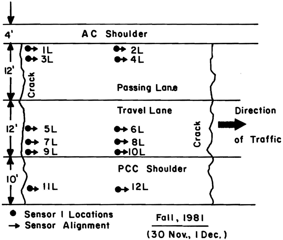
Fig 2.21. Layout plan of test locations in Fall 1981, section no. 3.
