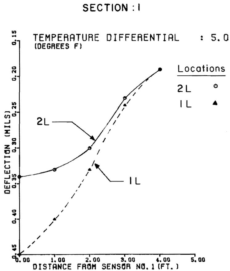
Fig 2.34(a). Comparison of deflection basins in mid-span and at crack locations measured at low temperature differential.
