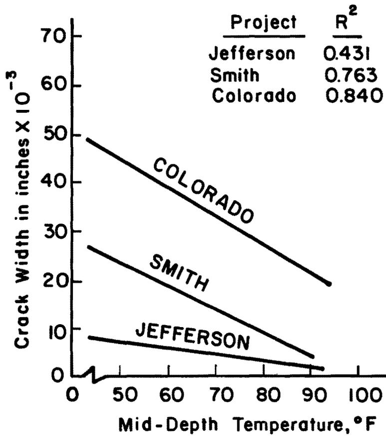
Fig 2.7. Crack width versus mid-depth temperature (Ref 7).
