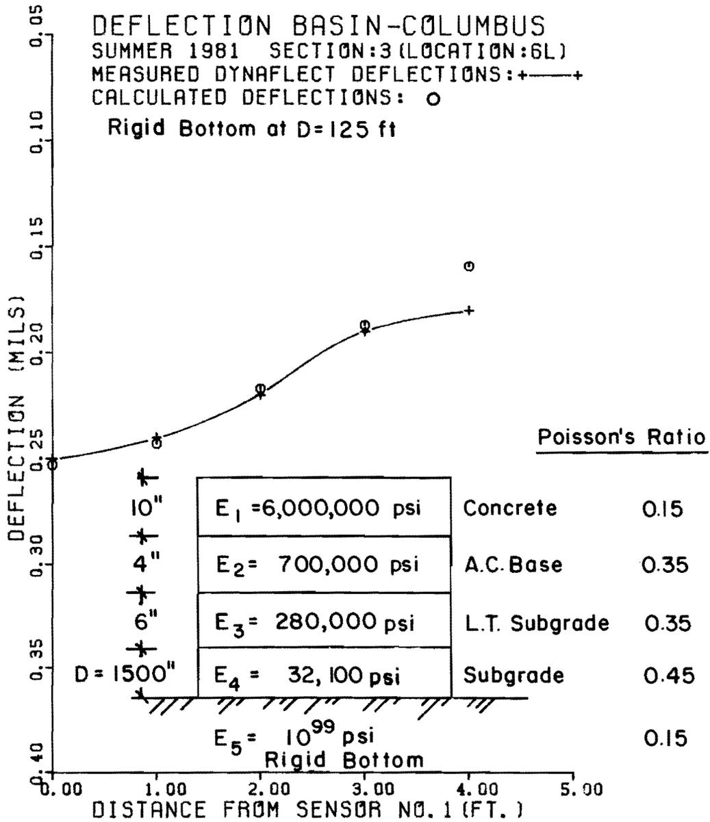
Fig 5.10. The back calculated Young's moduli (case of rigid bottom under 125 ft. of natural subgrade).
