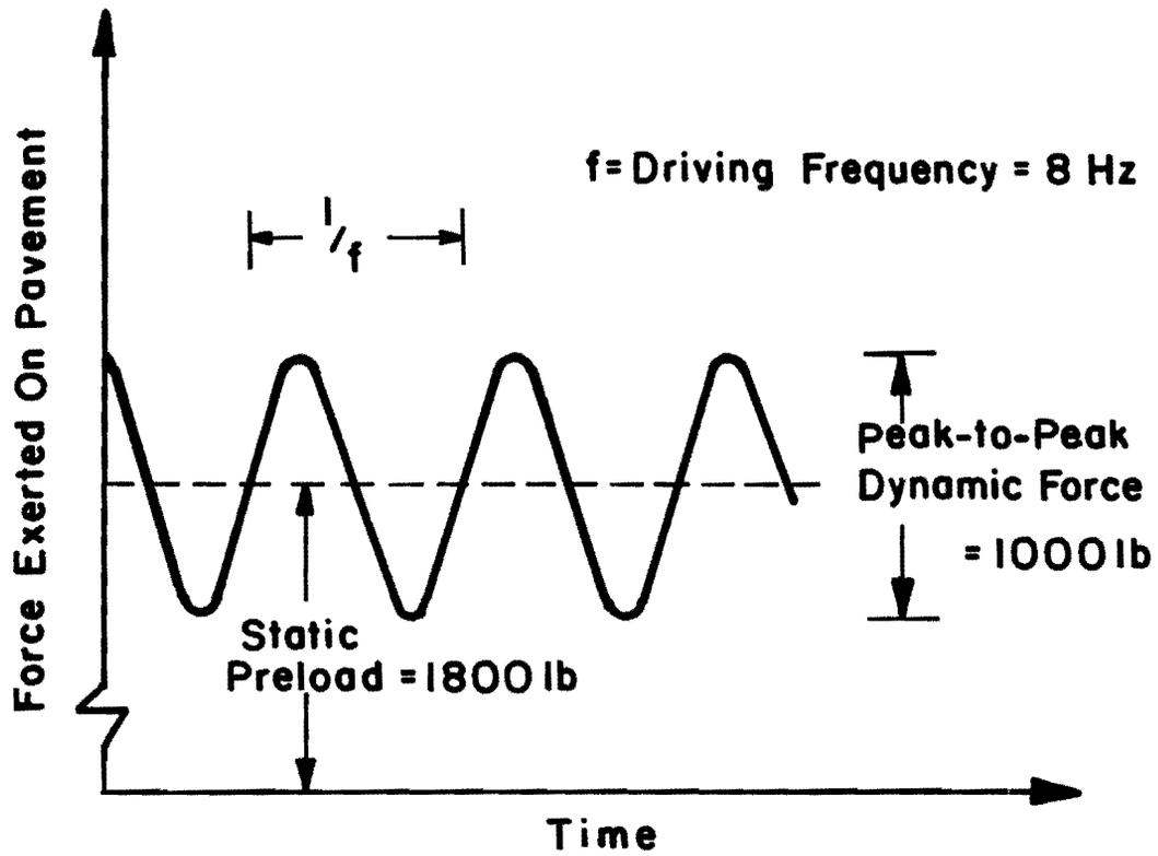
Fig 2.11. Typical dynamic force output signal of Dynaflect.
