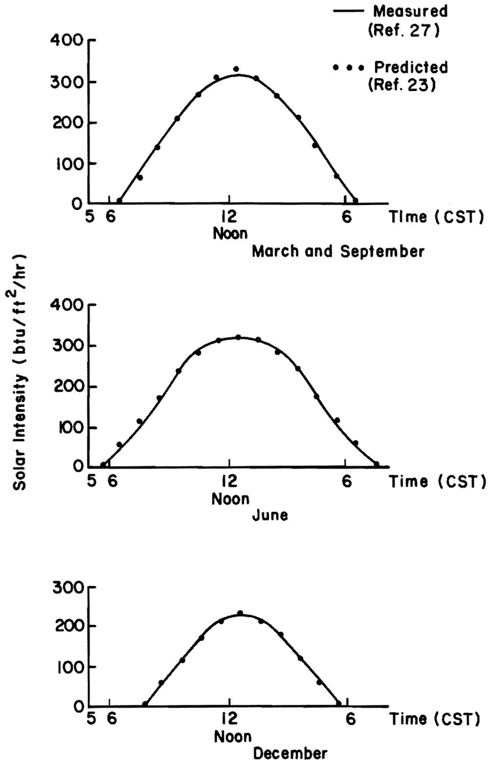
Fig 4.3. Hourly distributions of solar radiation intensity for a clear day, latitude 30° North.
