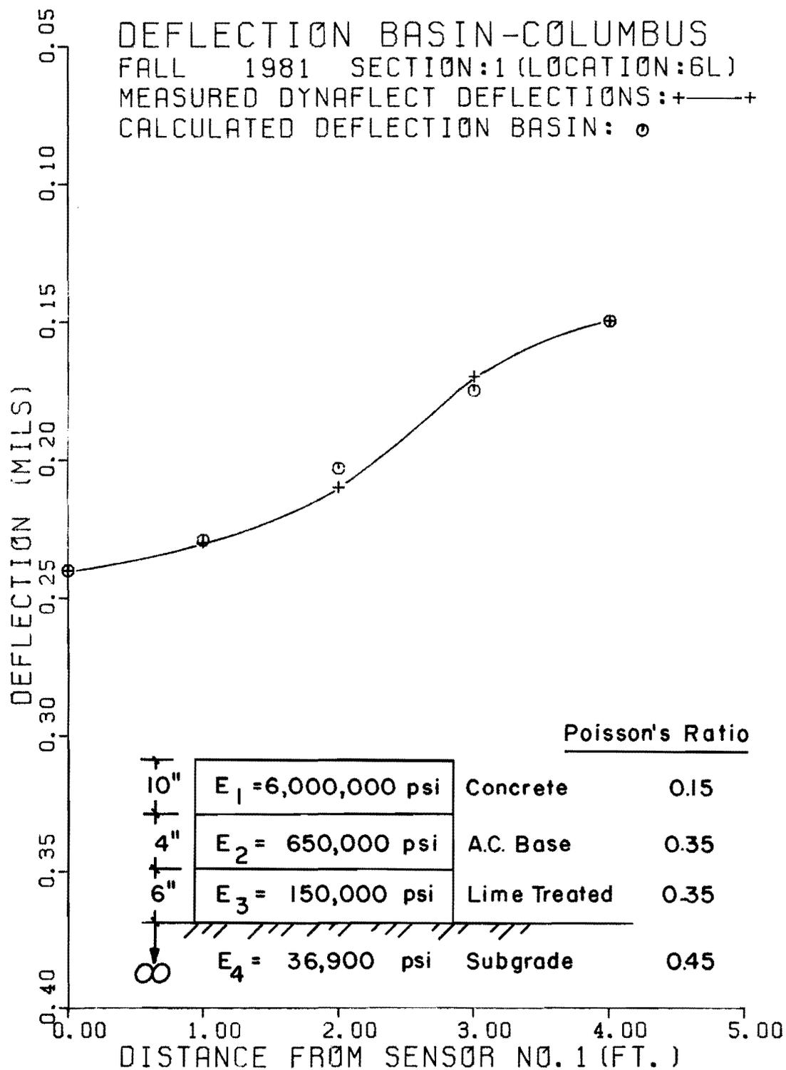
Fig F.4. Measured and calculated deflection basins (Example 2).
