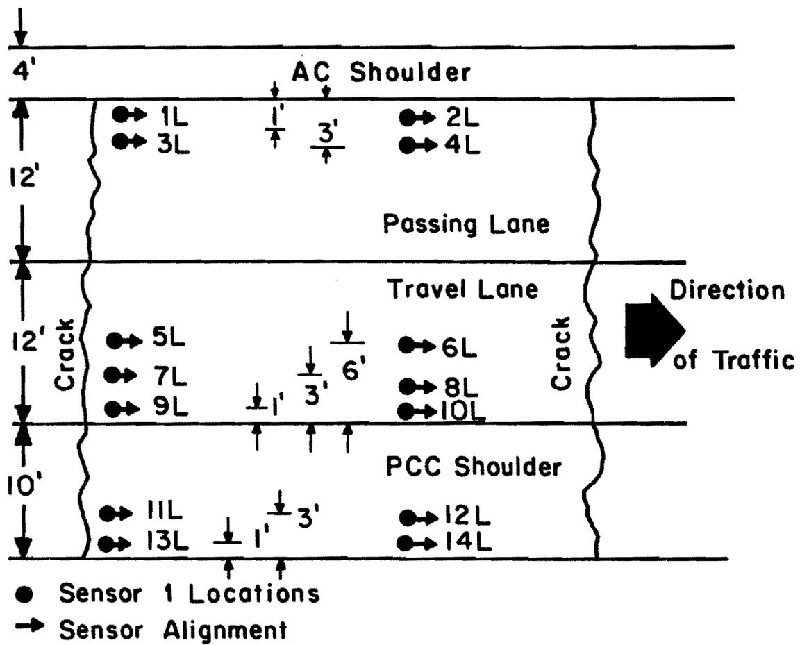
Fig 2.18. Layout plan of selected test locations in Summer 1981, sections nos. 1, 2, and 3.
