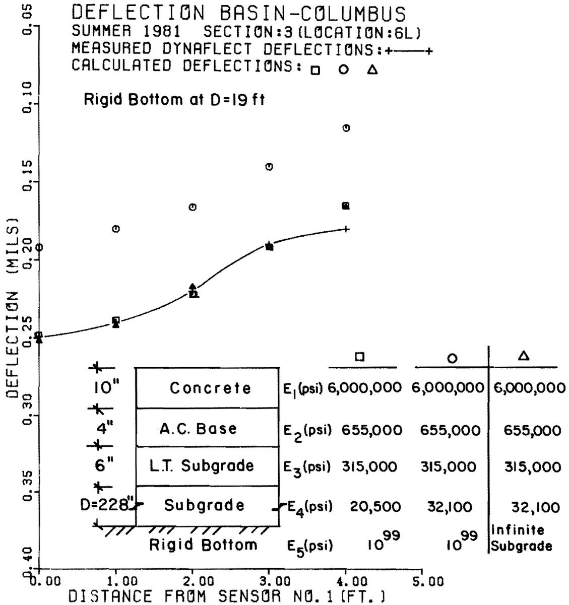
Fig 5.9. Reduction in subgrade modulus assuming a rigid bottom at some finite depth.
