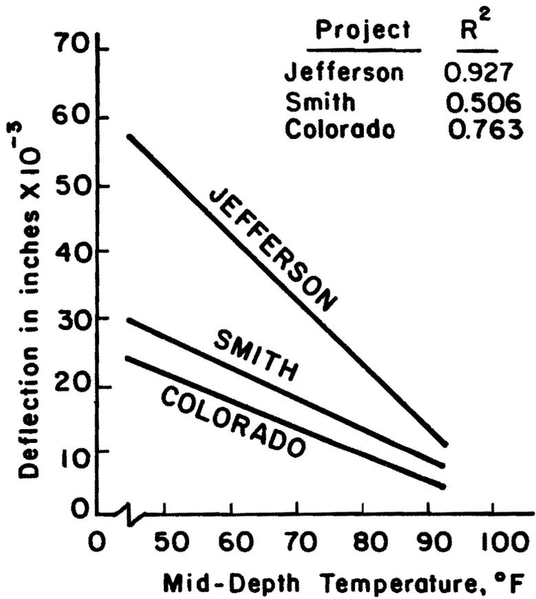
Fig 2.8. Deflection versus mid-depth temperature (Ref 7).
