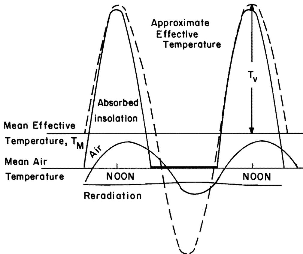
Fig 4.6. Comparison between effective temperature and air temperature (Ref 4).
