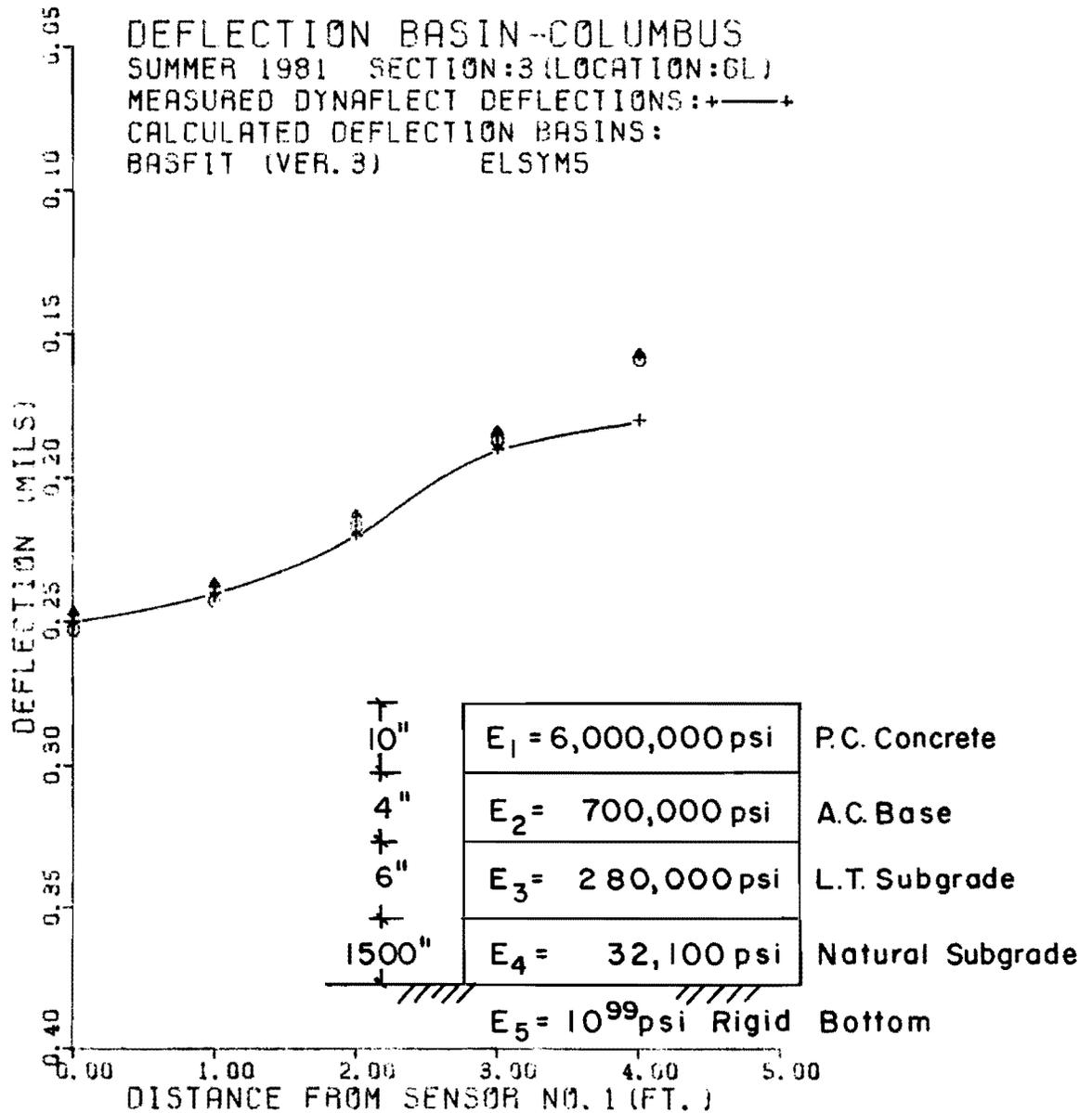
Fig F.2. Comparison of calculated deflection basins (case of rigid bottom).
