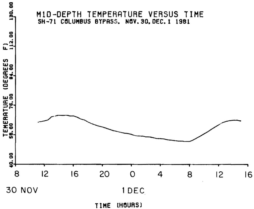
Fig 2.28. Mid-depth temperature of concrete slab versus time relationship, Summer 1981.
