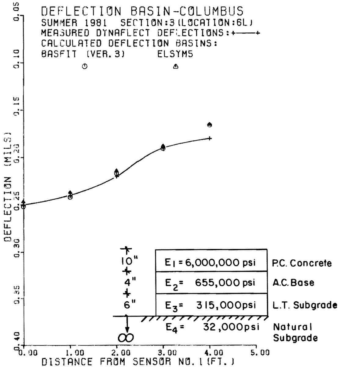
Fig F.1. Comparison of calculated deflection basins (infinite subgrade).
