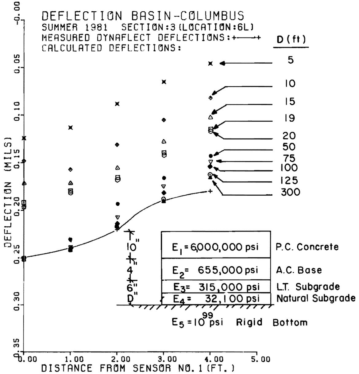
Fig 5.8. Effect of consideration of rigid bottom on calculated deflection basin.
