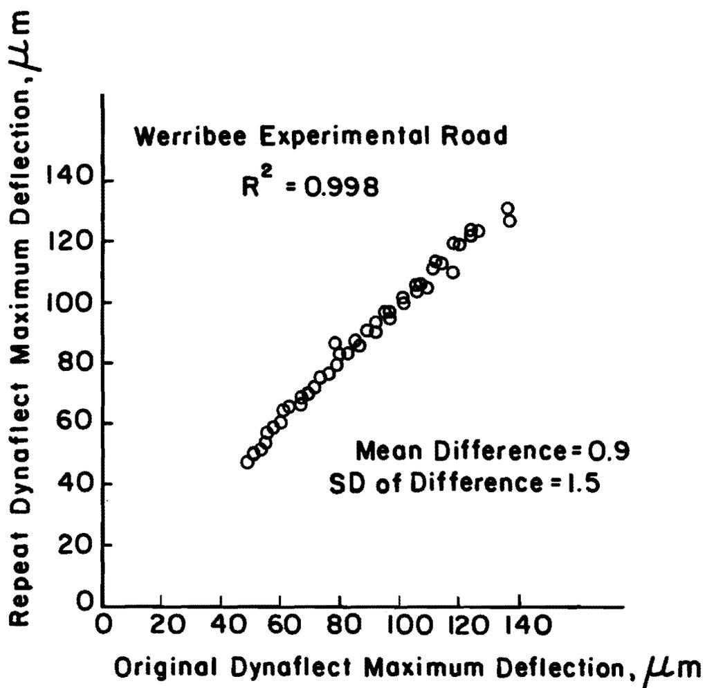
Fig 2.13. Original and repeat Dynaflect sensor 1 deflections without moving the Dynaflect from it's original position (Ref 16).
