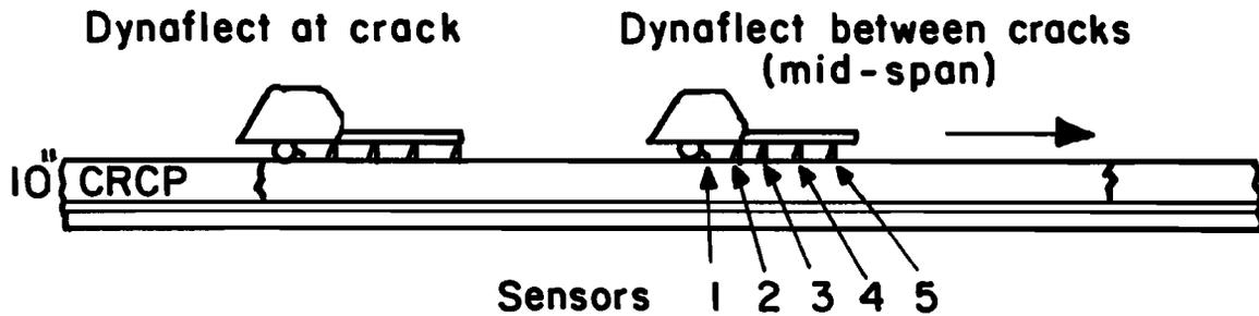
Fig 2.17. Dynaflect positions with respect to transverse cracks.
