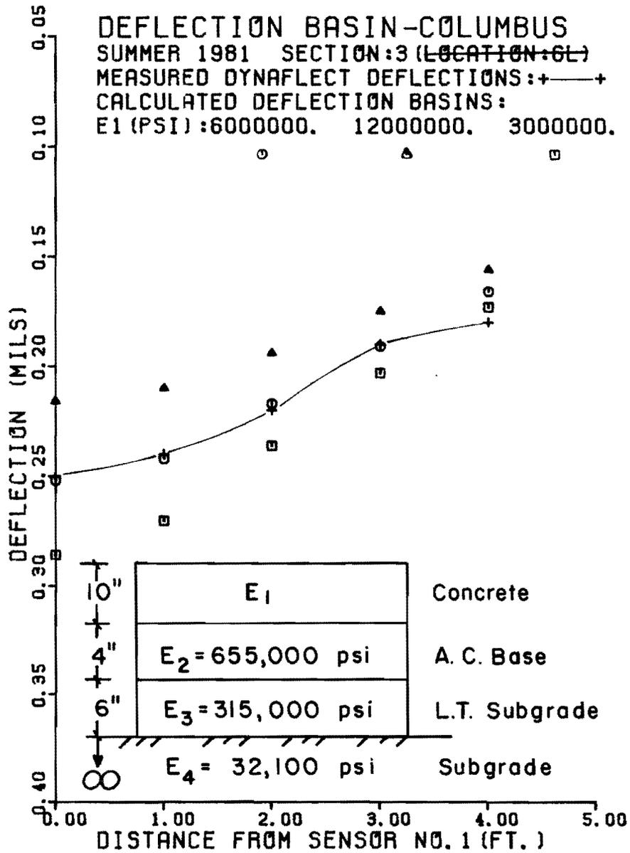
Fig 5.4. Effect of change of E<sub>1</sub> on calculated basin (infinite subgrade).
