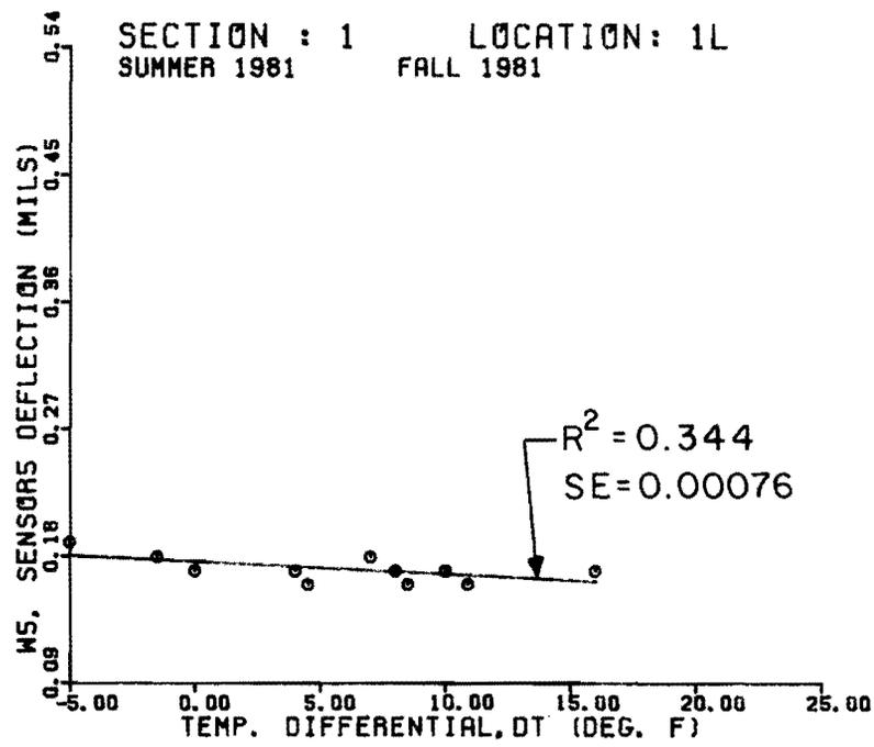
Fig 2.31(a). Sensor 5 deflection ( $W_5$ ) versus temperature differential relationship at location 1L, section 1.
