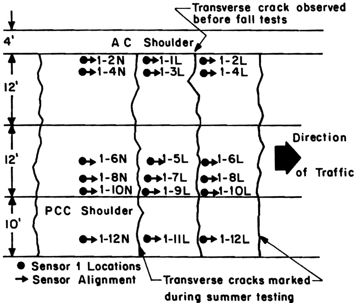
Fig 2.19. Layout plan of test locations in Fall 1981, section No. 1.
