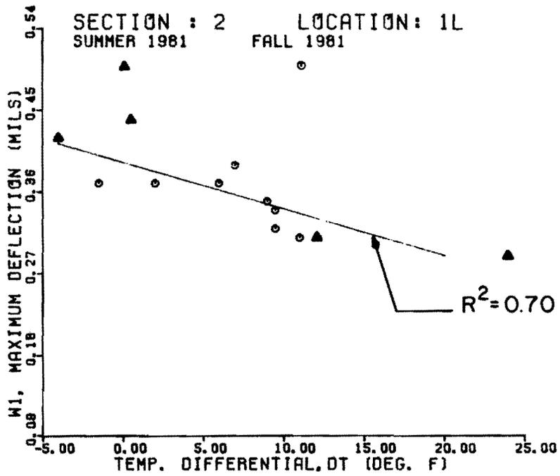
Fig 2.30(b). Maximum deflection ( $W_1$ ) versus temperature differential relationship at location 1L, section 2.
