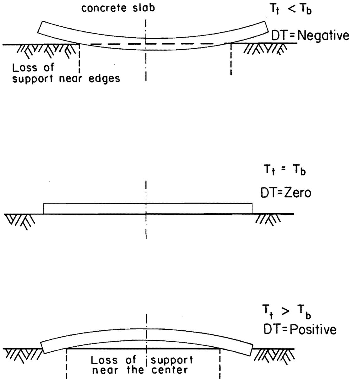
Fig 2.3. Conceptual illustration of curling in a concrete slab.
