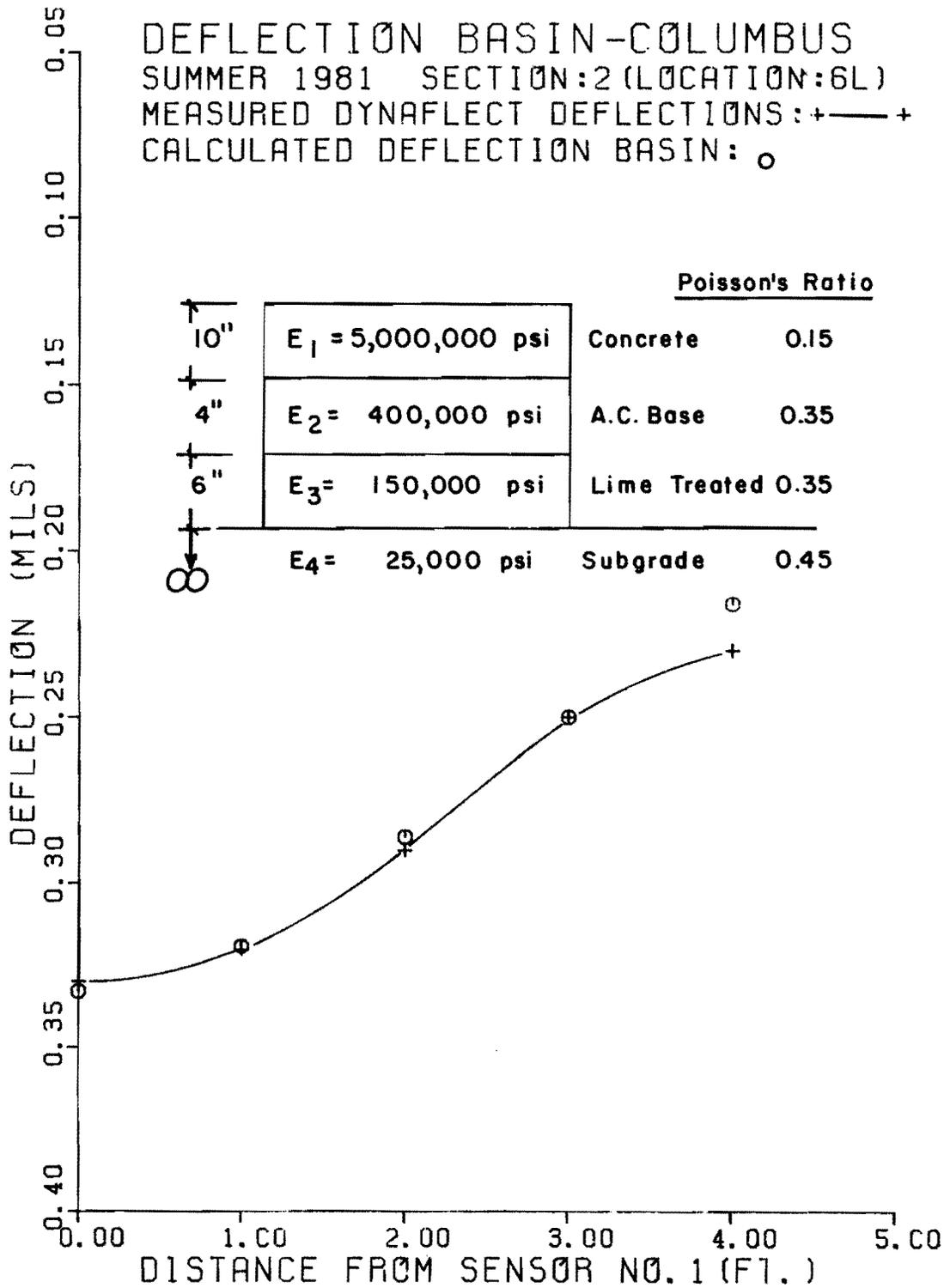
Fig F.6. Measured and calculated deflection basins (Example 4).
