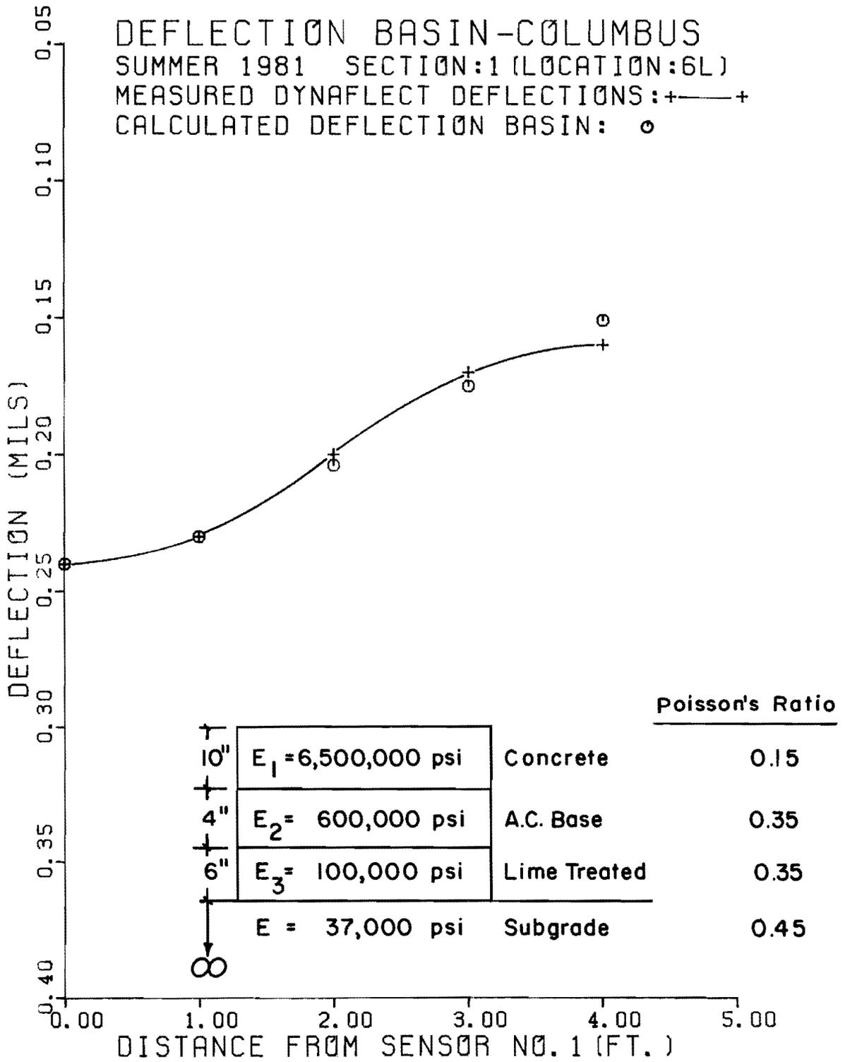
Fig F.3. Measured and calculated deflection basins (Example 1).
