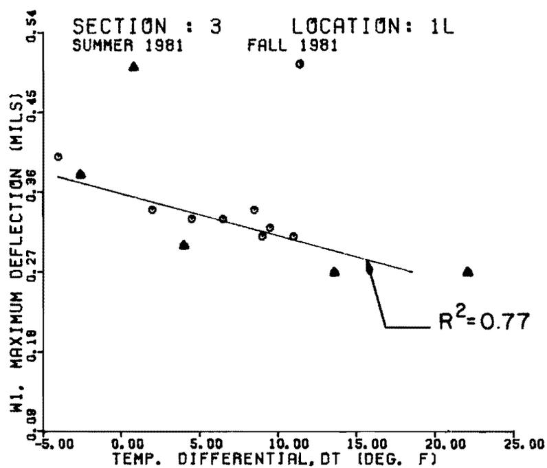
Fig 2.30(c). Maximum deflection ( $W_1$ ) versus temperature differential relationship at location 1L, section 3.
