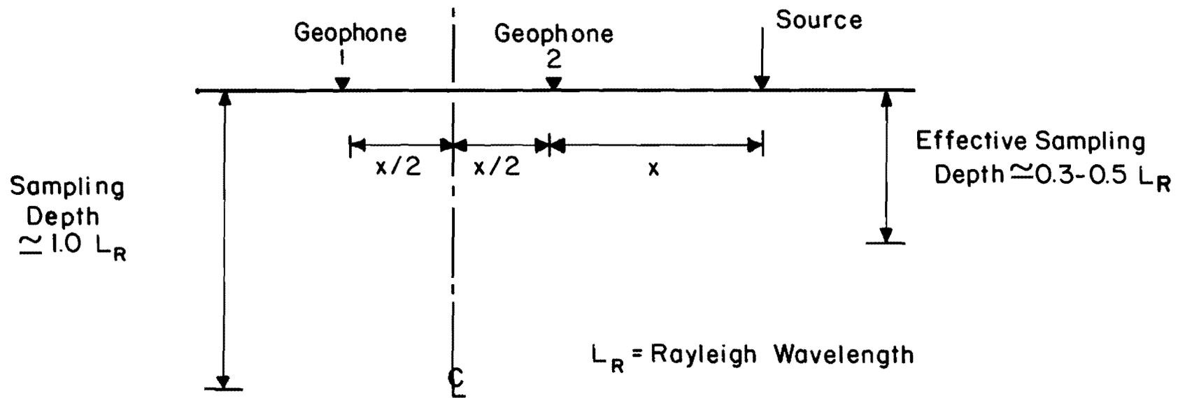
Fig 6.1. Schematic of Spectral-Analysis-of-Surface-Waves (SASW) Method.
