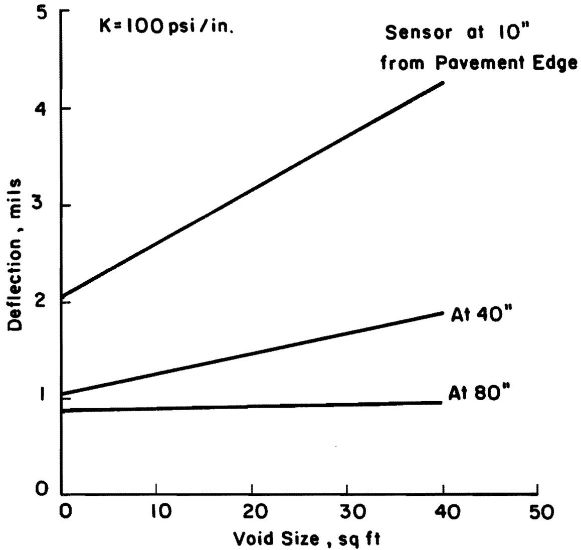
Fig 2.10. Effect of void size and Dynaflect position on pavement deflection (Ref 10).
