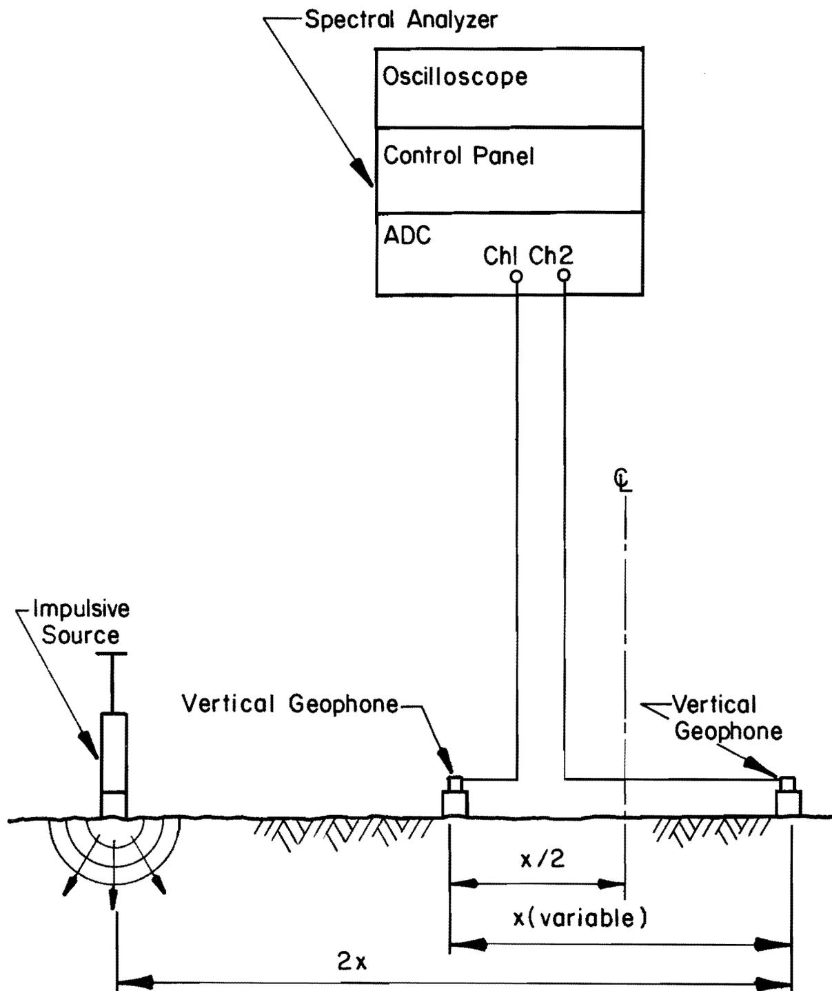
Fig 6.3. Schematic of Experimental Arrangement for SASW Tests.
