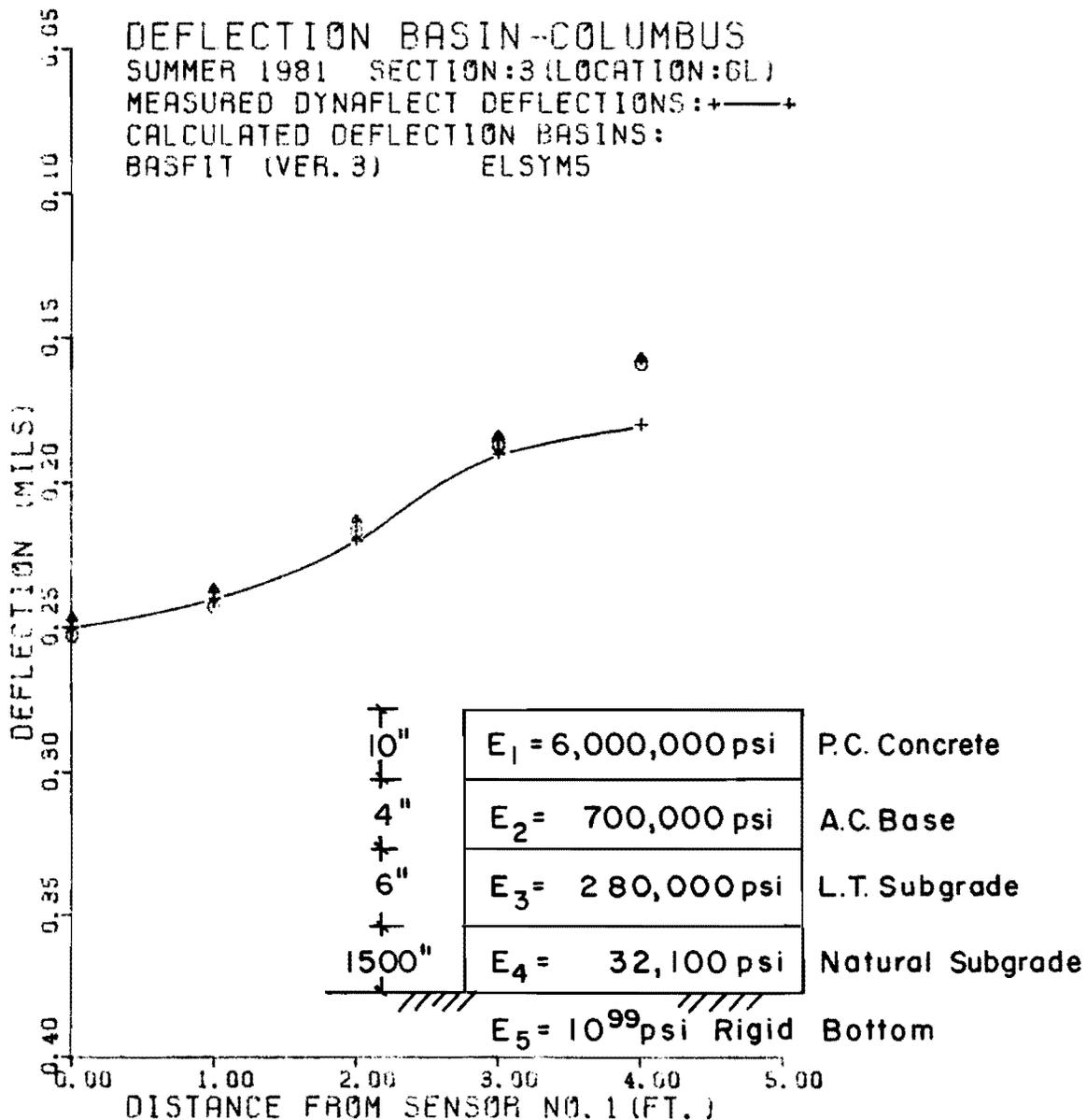
Fig F.2. Comparison of calculated deflection basins (case of rigid bottom).
