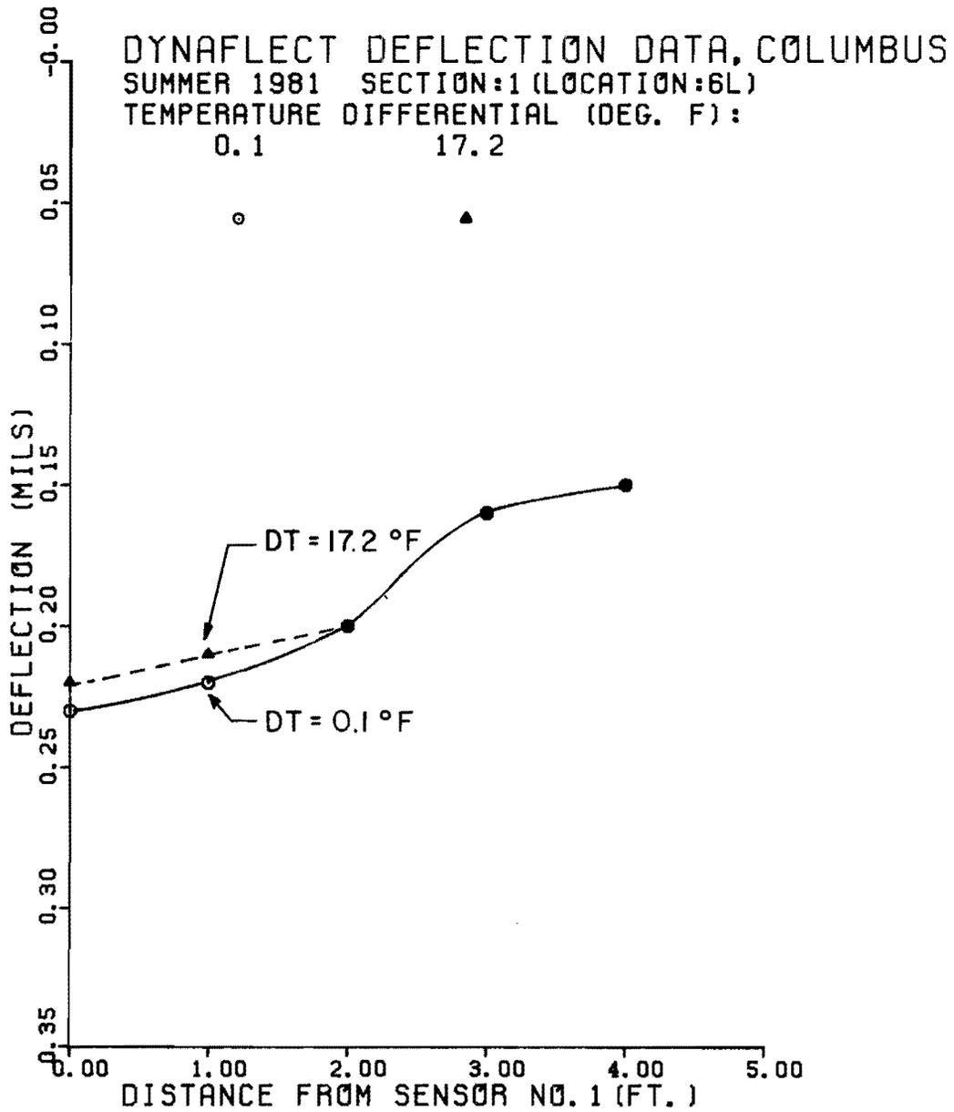
Fig 2.33. Deflection basins measured in mid span position (interior condition) at different temperature differentials.
