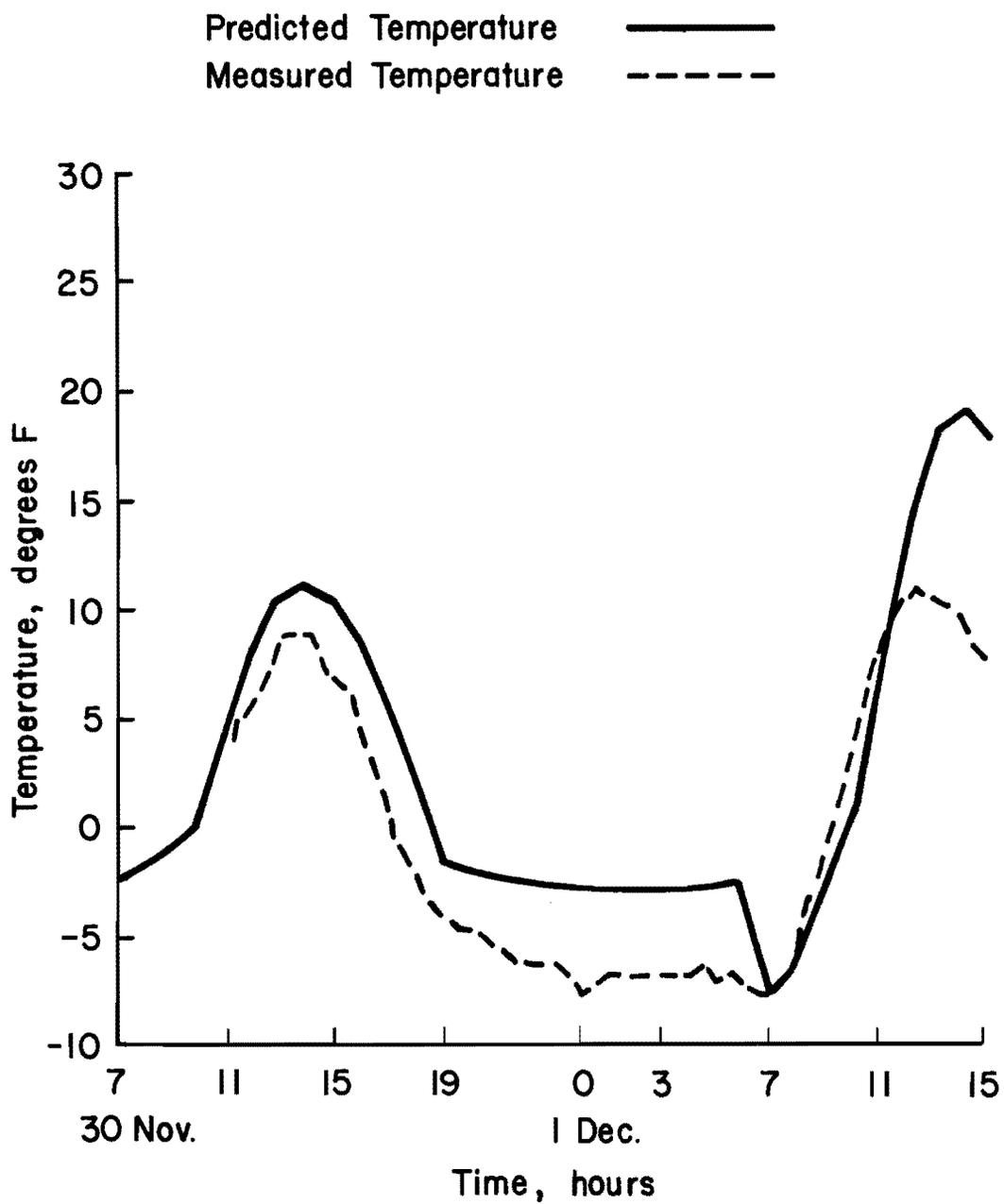
Fig 4.11(b). Variation in temperature differential based on Fall 1981 data, Columbus Bypass, SH-71.
