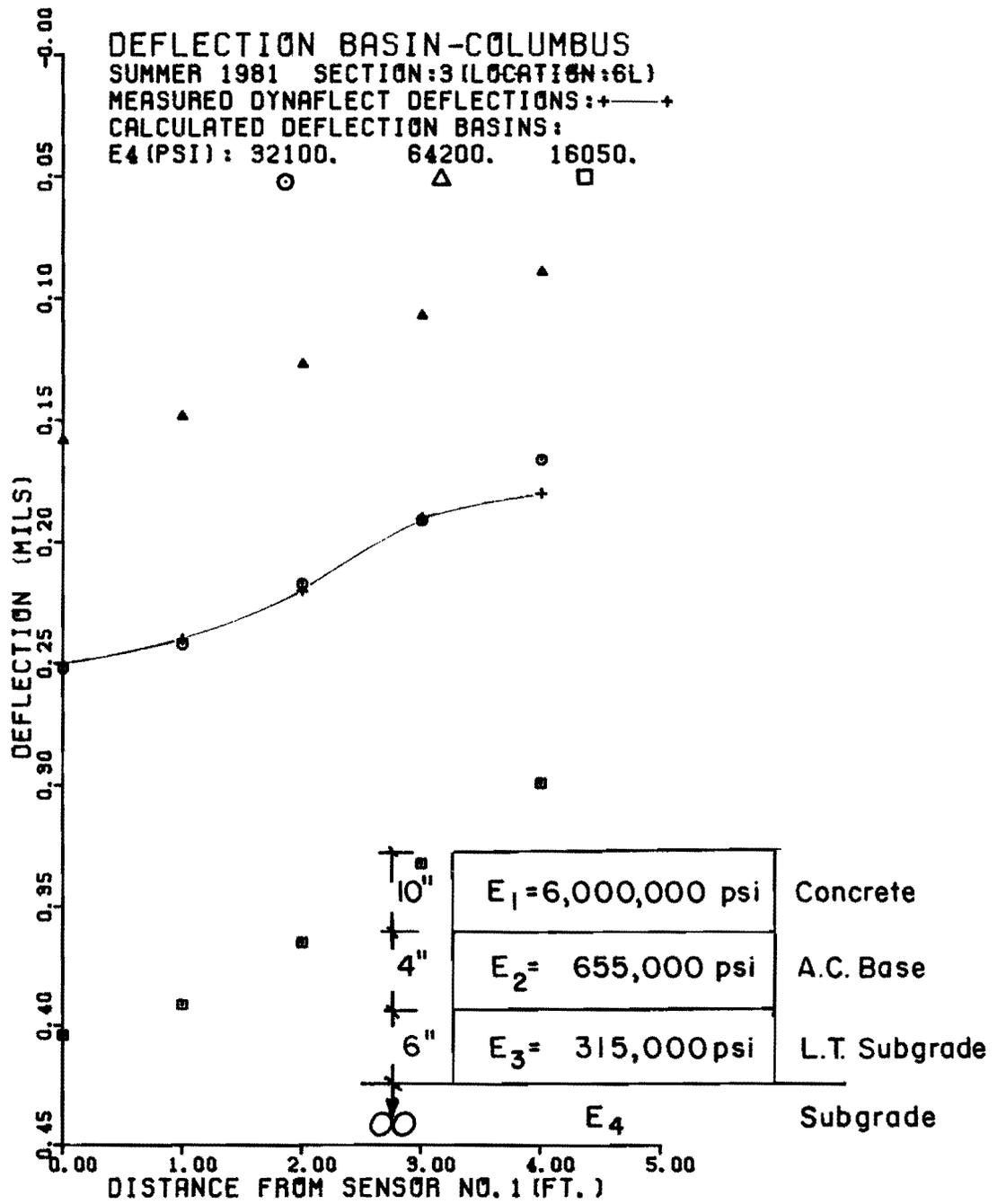
Fig 5.7. Effect of change of E<sub>4</sub> on calculated basin (infinite subgrade).
