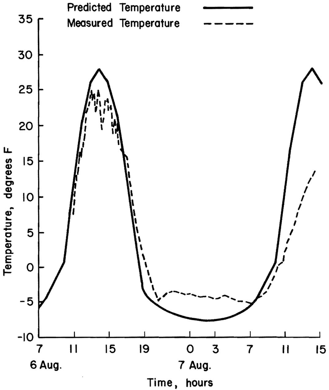
Fig 4.11(a). Variation in temperature differential based on Summer 1981 data, Columbus Bypass, SH-71.
