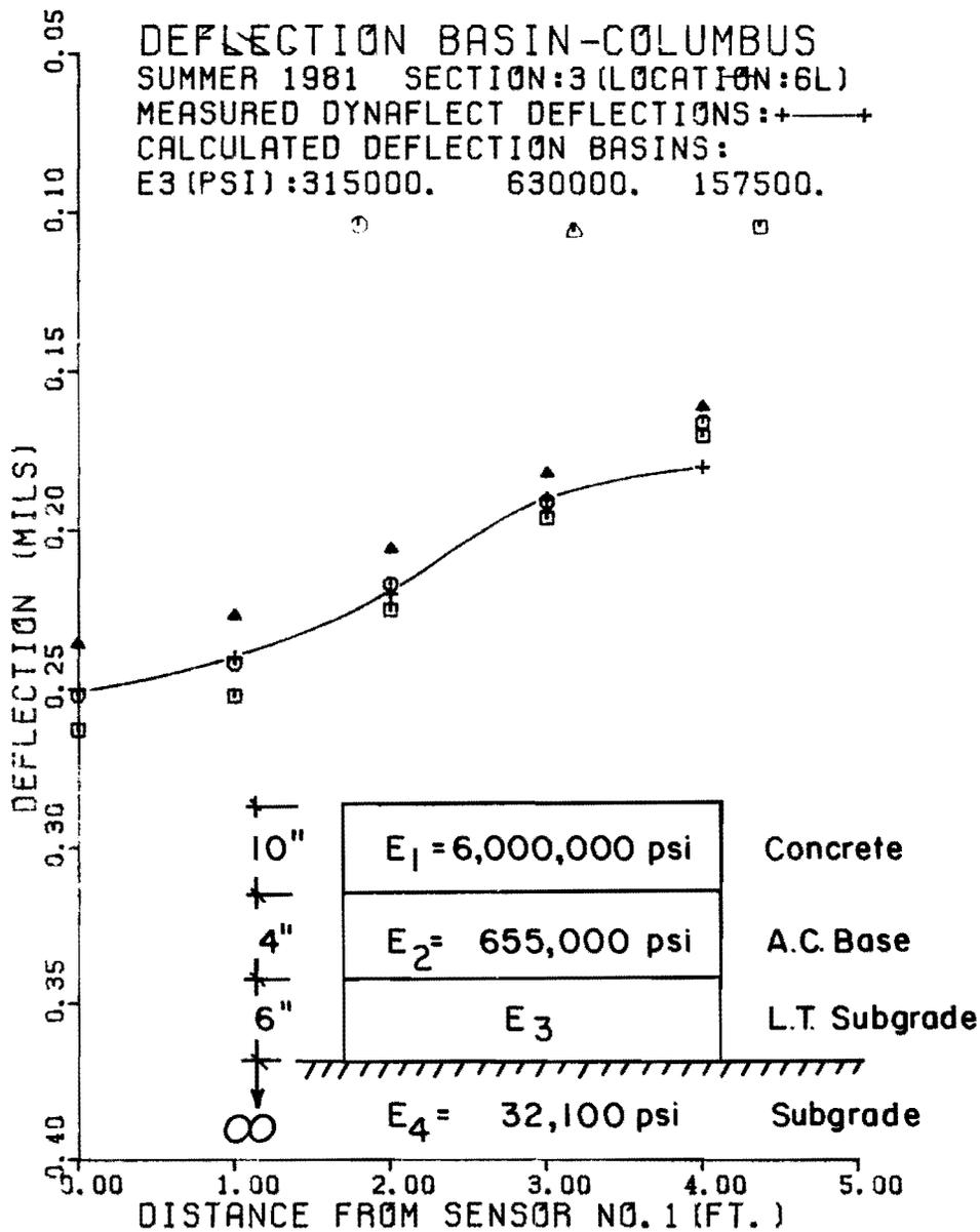
Fig 5.6. Effect of change of  $E_3$  on claculated basin (infinite subgrade).
