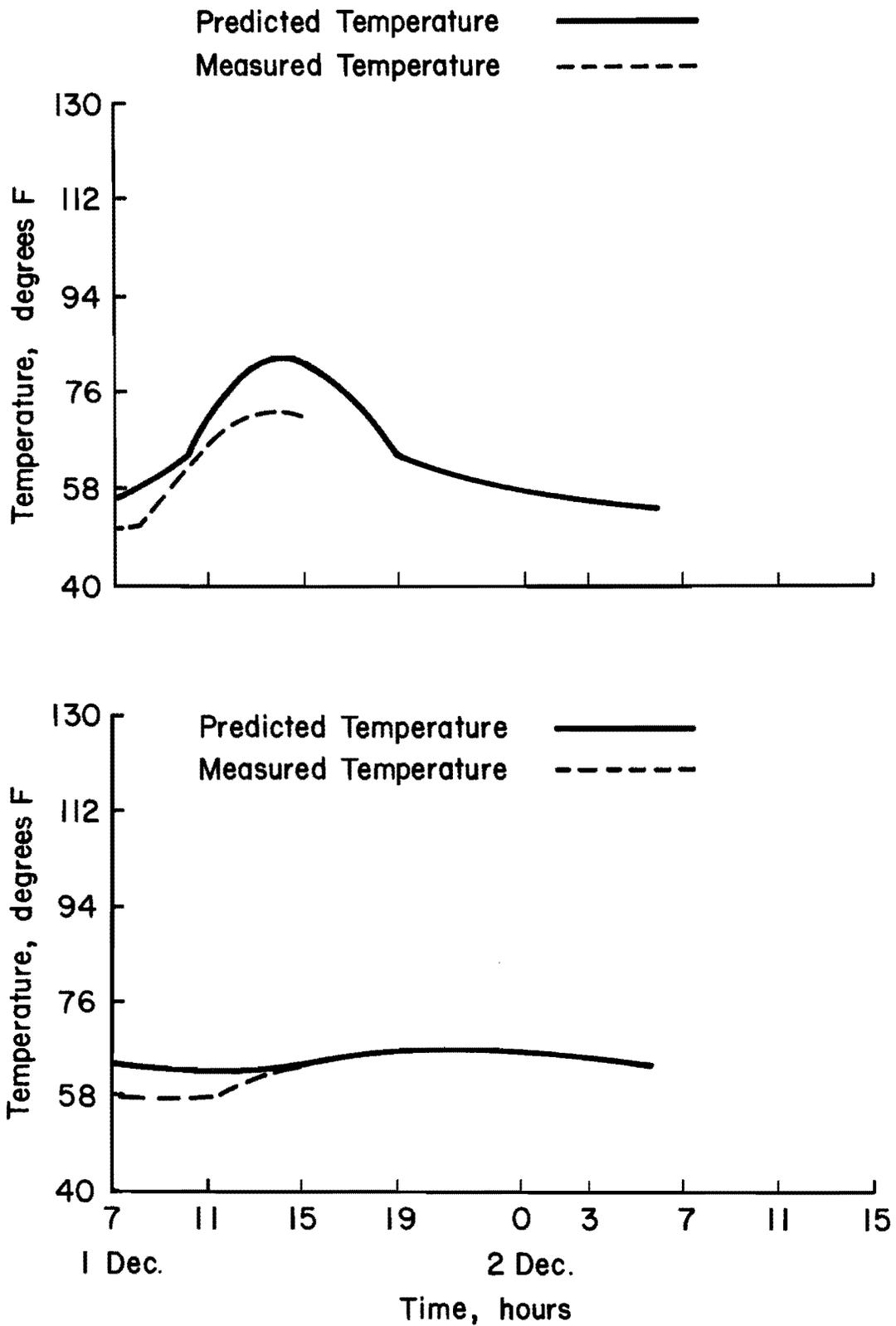
Fig 4.10. Variation in temperatures of concrete slab on 1, 2 Dec. 1981, Columbus Bypass, SH-71.
