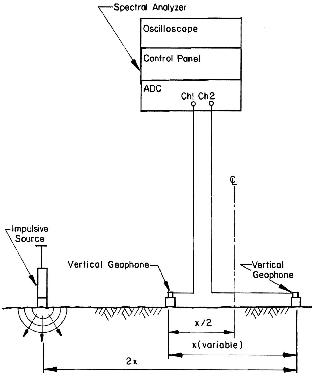
Fig 6.3. Schematic of Experimental Arrangement for SASW Tests.
