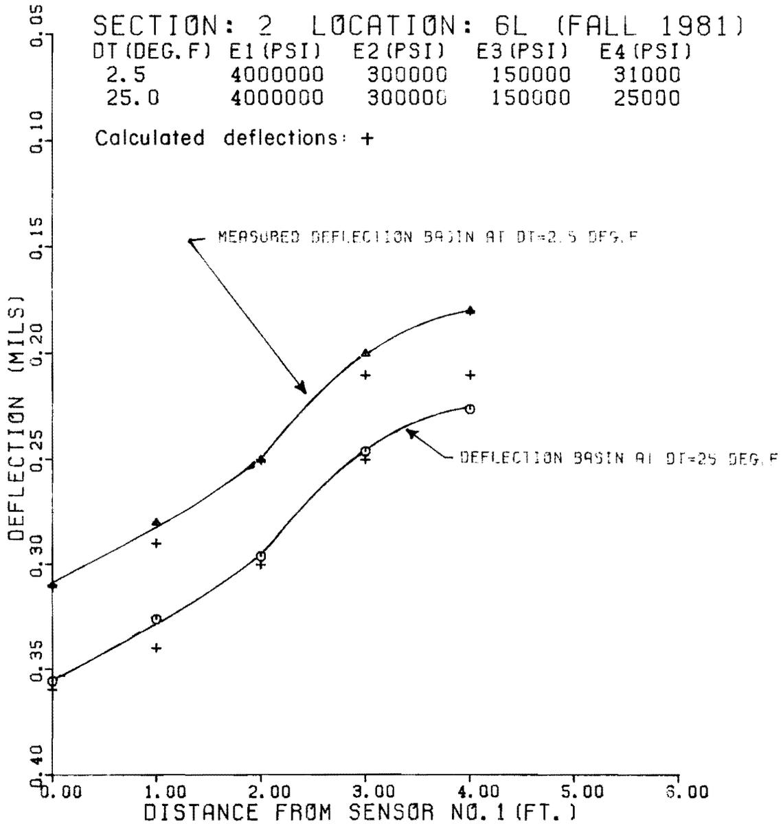
Fig 3.2. Effect of increase in positive temperature differential on the Dynaflect deflection basin and the back-calculated Young's moduli.
