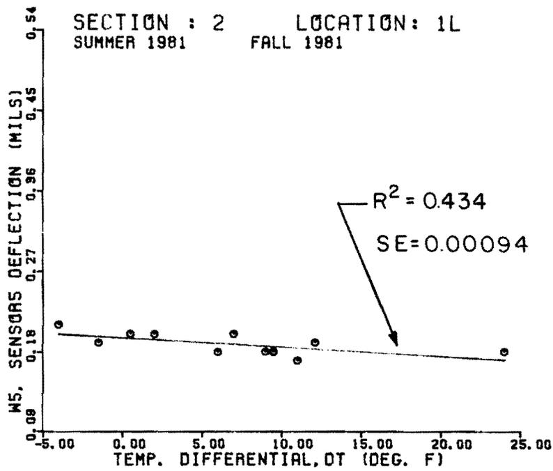
Fig 2.31(b). Sensor 5 deflection ( $W_5$ ) versus temperature differential relationship at location 1L, section 2.
