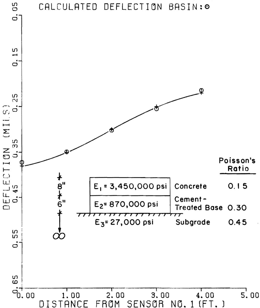
Fig F.11. Measured and calculated deflection basins (Example 9).
