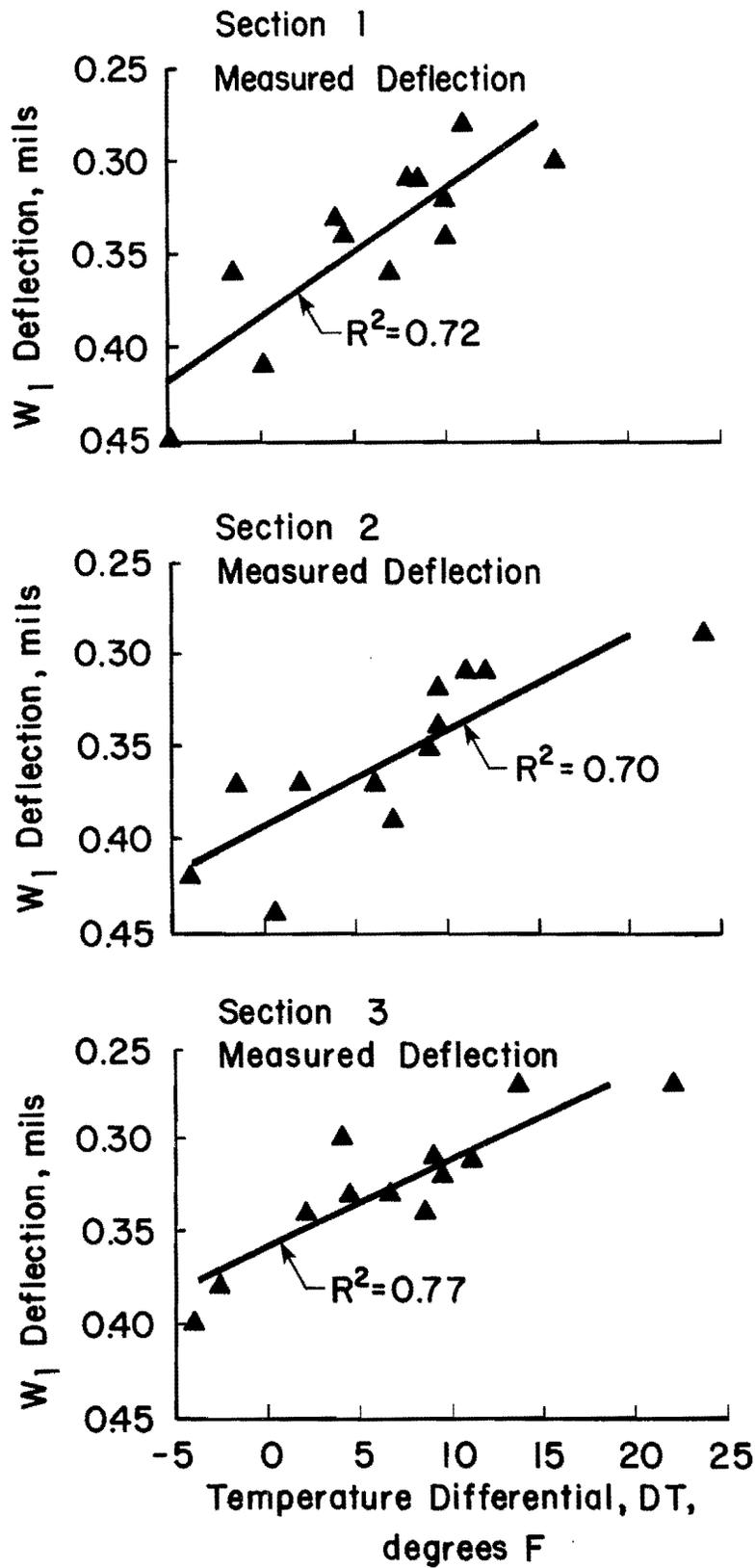
Fig E.1. Measured W<sub>1</sub> deflections versus temperature differential relationship at location 1L, Columbus bypass, SH-71 (1981 data).
