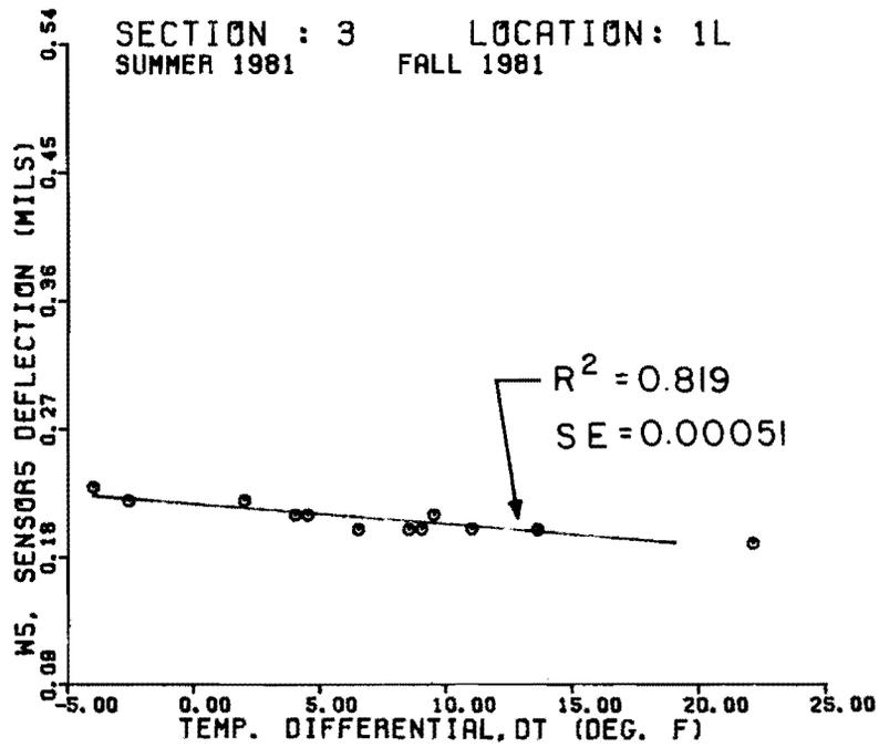
Fig 2.31(c). Sensor 5 deflection ( $W_5$ ) versus temperature differential relationship at location 1L, section 3.
