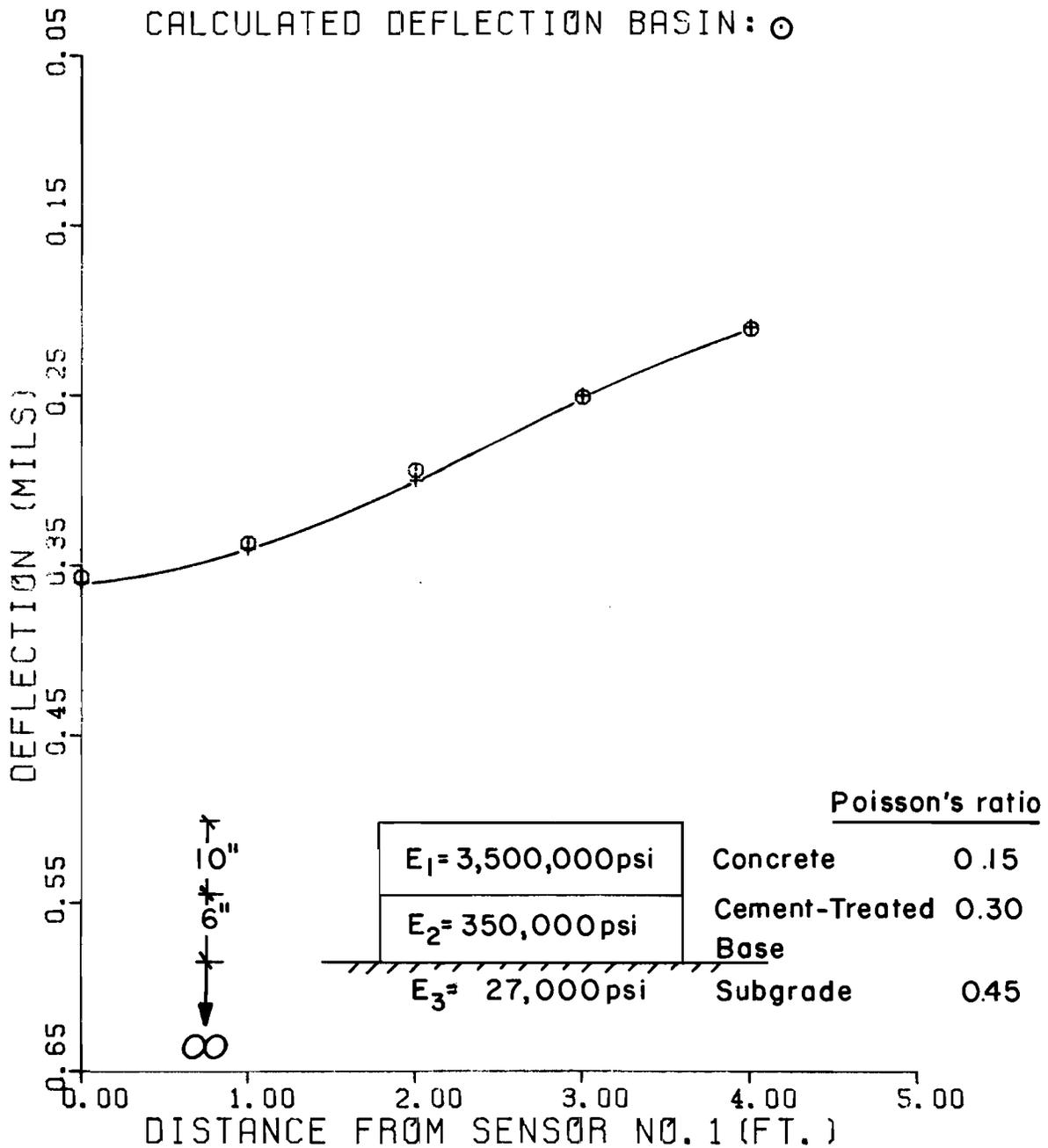
Fig F.8. Measured and calculated deflection basins (Example 6).
