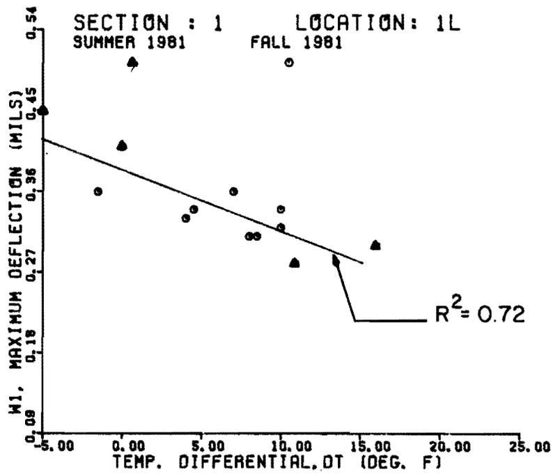
Fig 2.30(a). Maximum deflection ( $W_1$ ) versus temperature differential relationship at location 1L, section 1.
