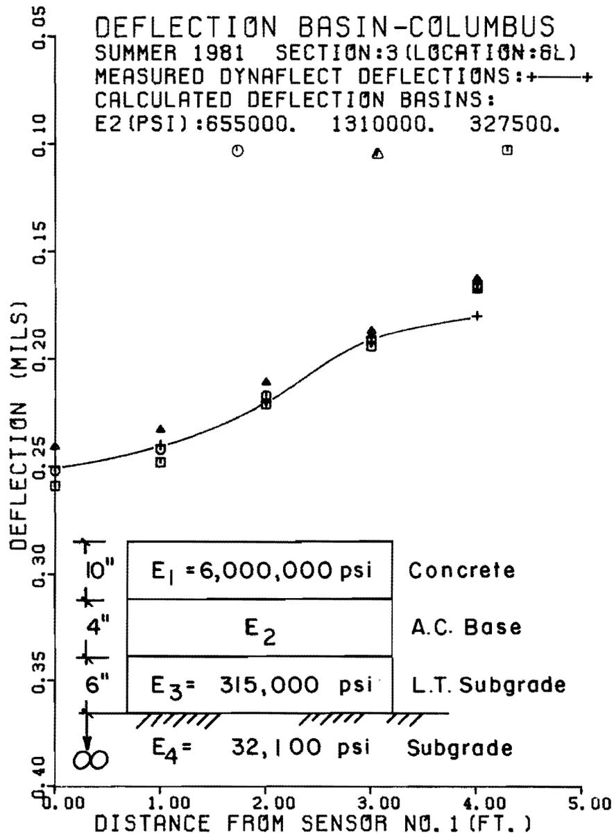
Fig 5.5. Effect of change of  $E_2$  on calculated basin (infinite subgrade).
