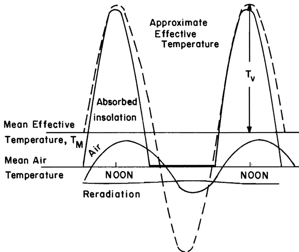
Fig 4.6. Comparison between effective temperature and air temperature (Ref 4).
