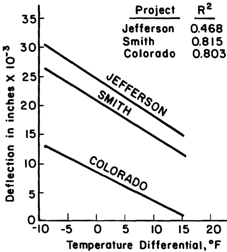
Fig 2.5. Edge deflection versus temperature differential (Ref 7).
