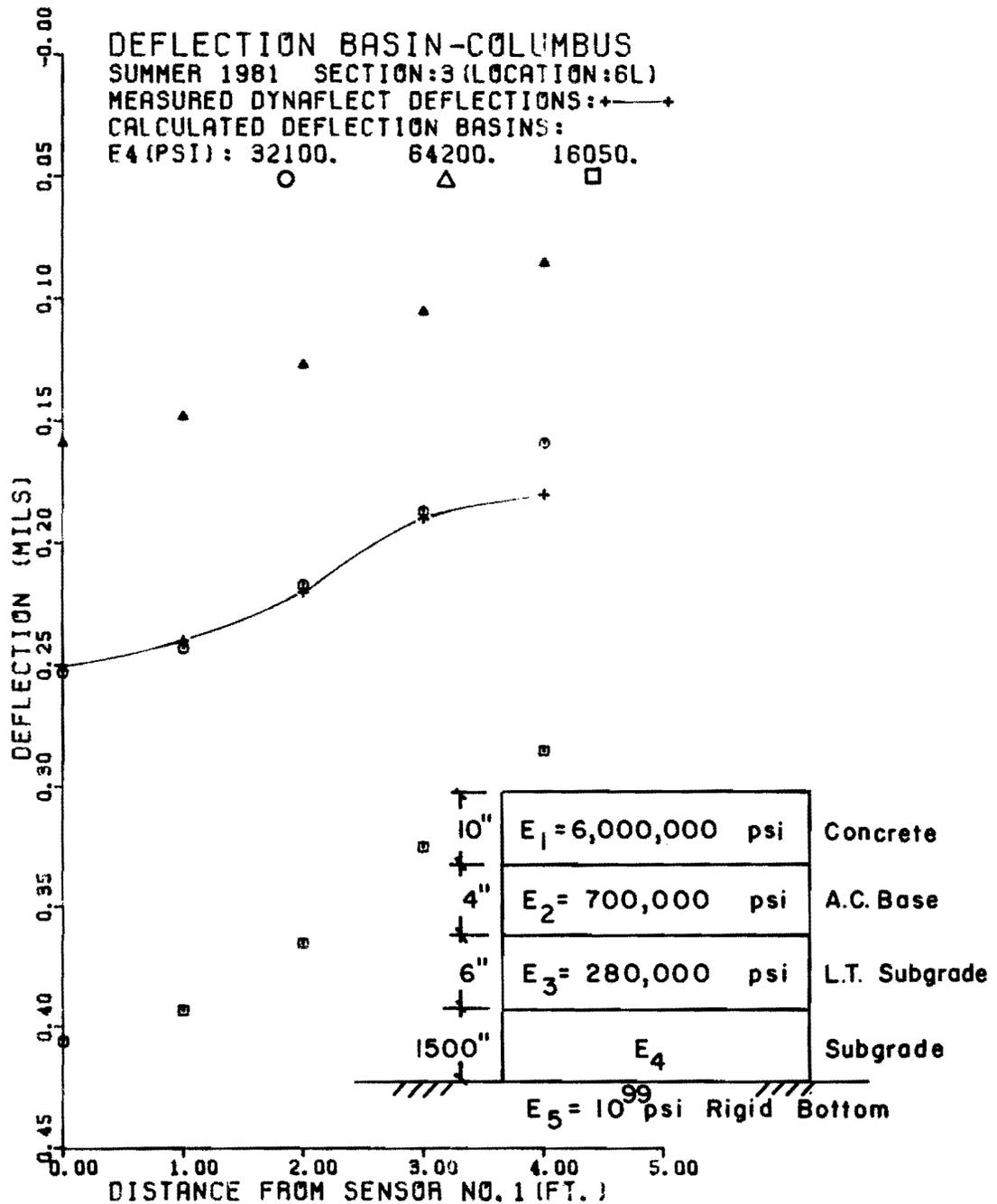
Fig 5.14. Effect of change of  $E_4$  on calculated basin (case of rigid bottom).
