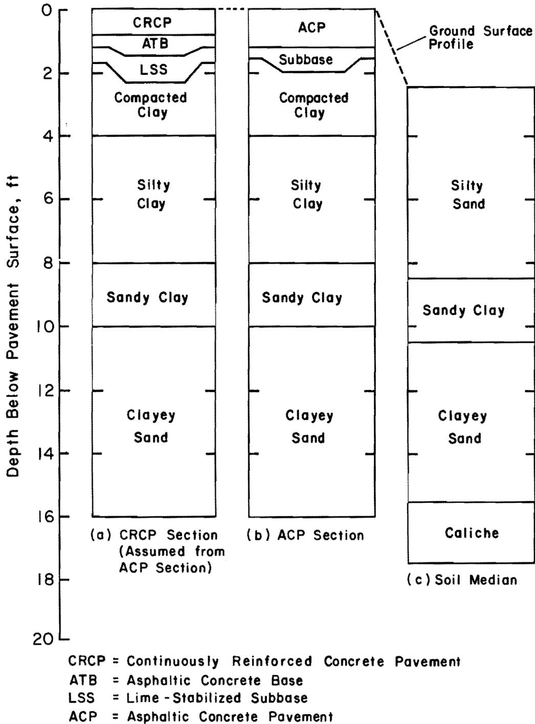
Fig 6.2. Soil profile under different test sections.
