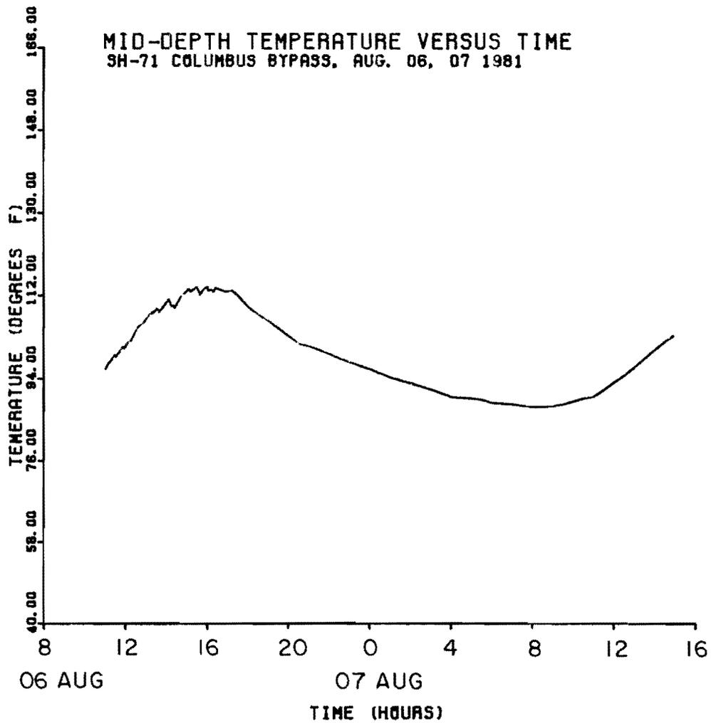
Fig 2.27. Mid-depth temperature of concrete slab versus time relationship, Fall 1981.
