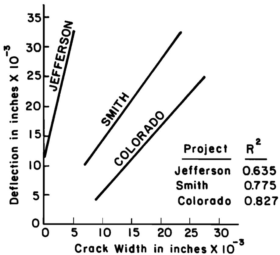
Fig 2.6. Deflection versus crack width (Ref 7).
