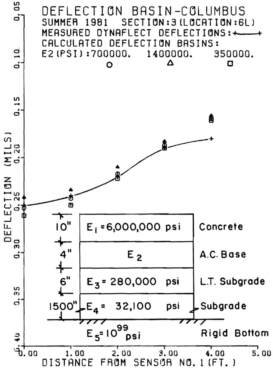
Fig 5.12. Effect of change of  $E_2$  on calculated basin (case of rigid bottom).
