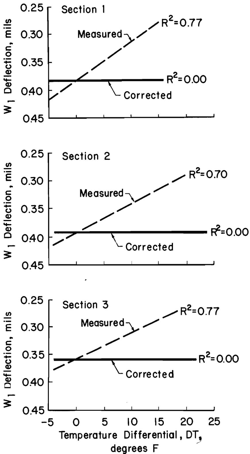
Fig E.3. Best fit lines for measured and corrected W<sub>1</sub> deflections at location 1L, Columbus bypass, SH-71 (1981 data).
