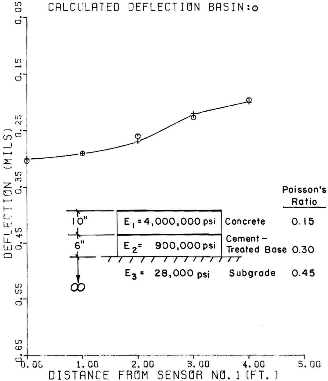
Fig F.9. Measured and calculated deflection basins (Example 7).
