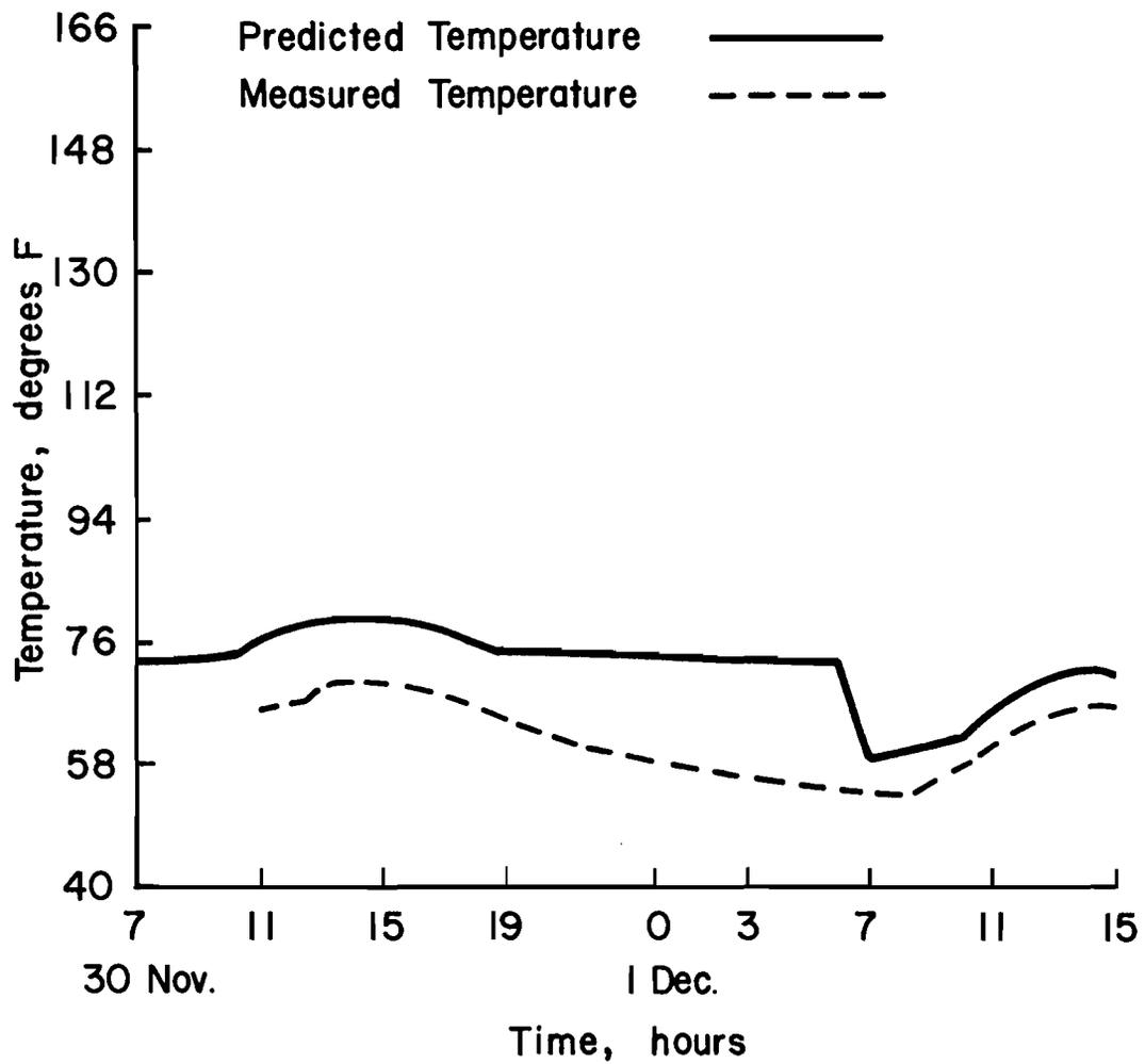
Fig 4.12(b). Variation in mid-depth temperature based on Fall 1981 data, Columbus Bypass, SH-71.
