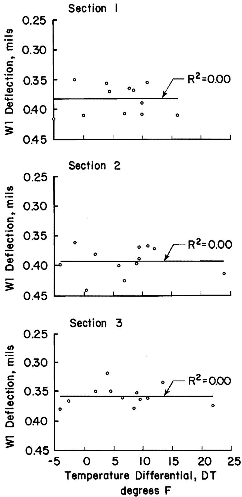
Fig 4.13. Corrected deflections at location IL after applying the temperature correction to the measured sensor 1 deflections, (Summer and Fall 1981 data).
