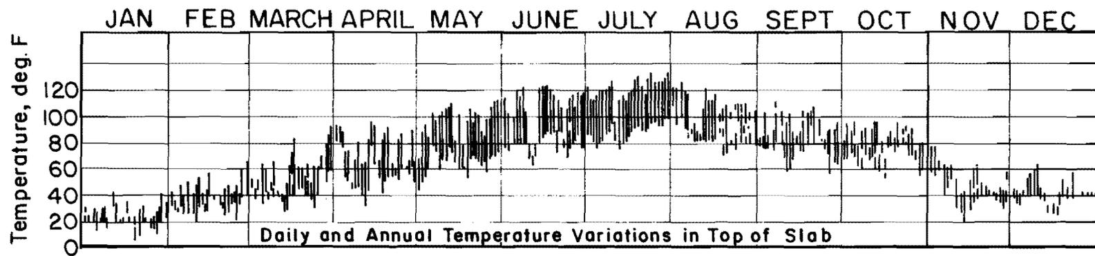
Fig 2.1(a). Temperature variations in top of P.C. concrete slab, Arkansas, 1940 (Ref 3).
