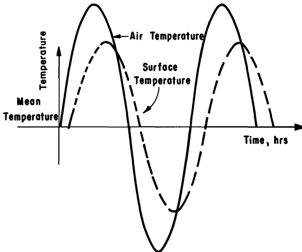
Fig 4.4. Surface temperature versus time relationship without the effects of solar radiation and wind (Ref 4).
