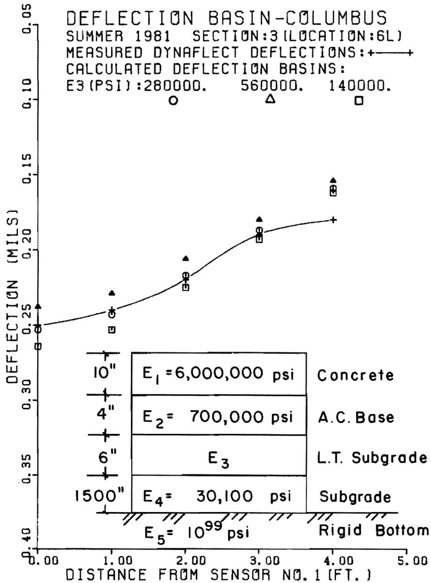
Fig 5.13. Effect of change of  $E_3$  on calculated basins (case of rigid bottom).
