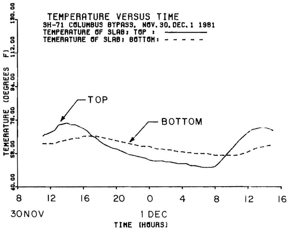
Fig 2.24. Temperature of top and bottom of concrete slab versus time, Fall 1981.
