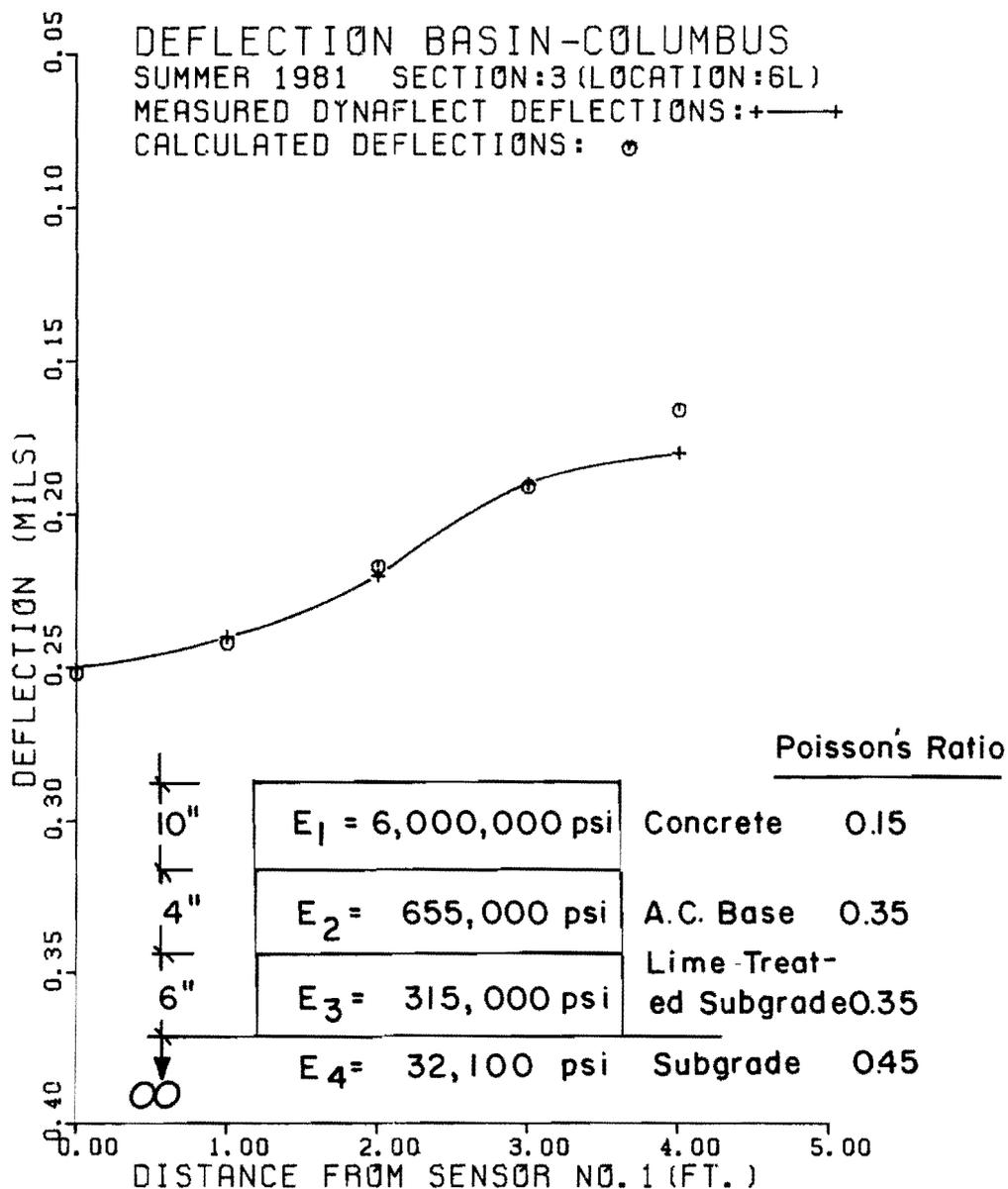
Fig 5.3. Back calculated Young's moduli assuming infinite subgrade.
