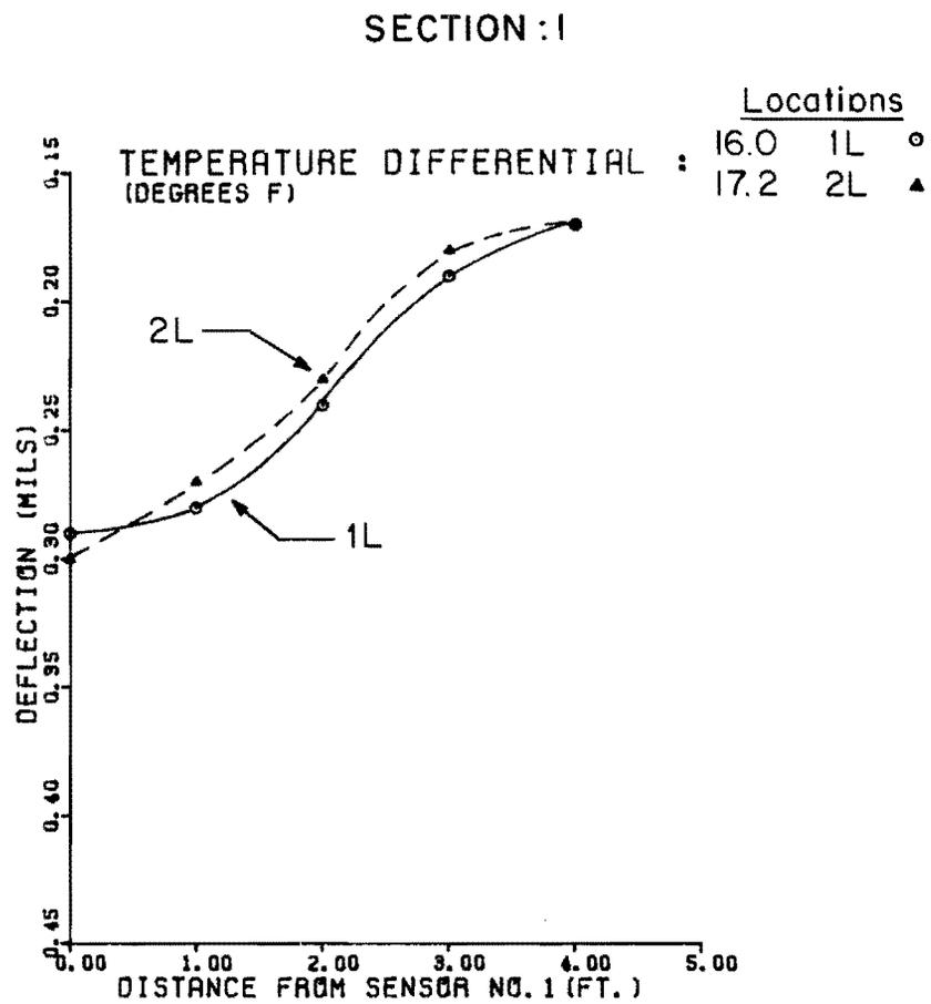
Fig 2.34(b). Comparison of deflection basins in mid-span and at crack locations measured at higher positive temperature differential.
