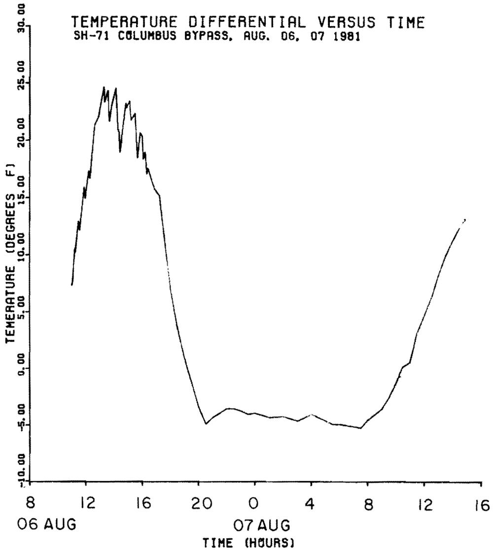
Fig 2.25. Temperature differential versus time relationship, Summer 1981.
