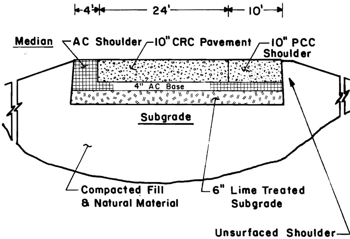
Fig 2.16. Typical details of CRC pavements, Columbus bypass (southbound direction only), Texas.
