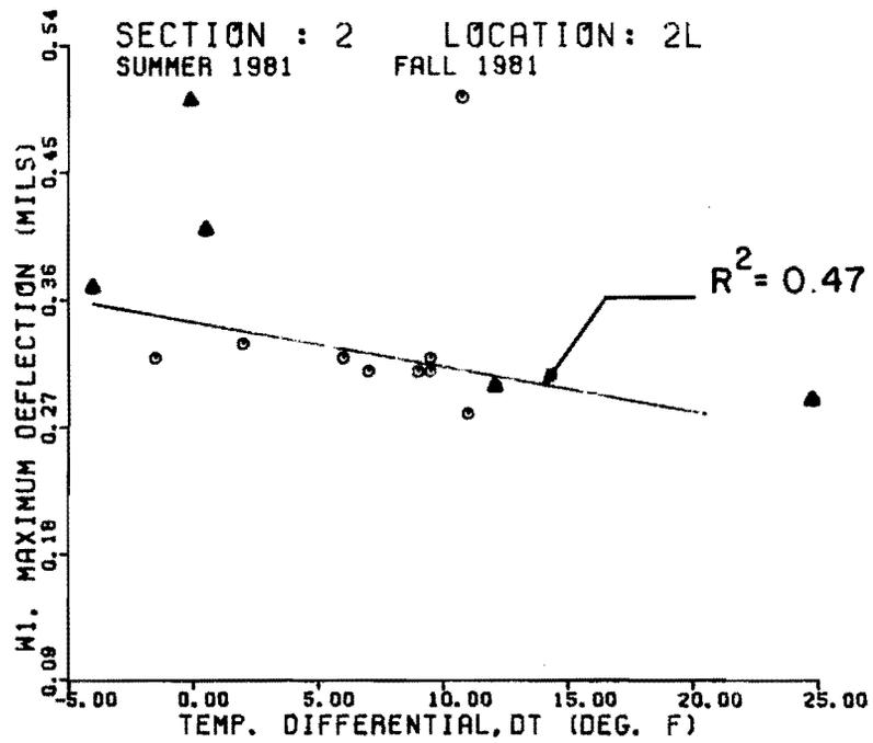
Fig 2.35(b). Maximum deflection ( $W_1$ ) versus temperature differential relationship at location 2L, section 2.
