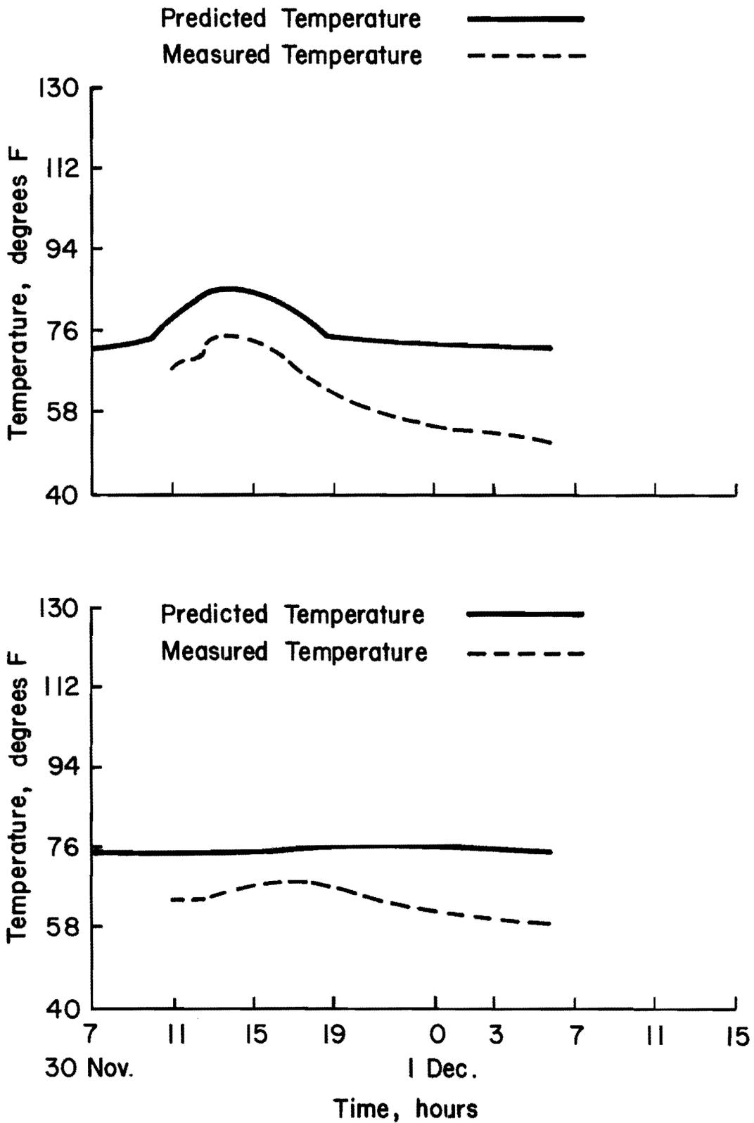
Fig 4.9. Variation in temperature of concrete slab on 30 Nov. - 1 Dec. 1981, Columbus Bypass, SH-71.
