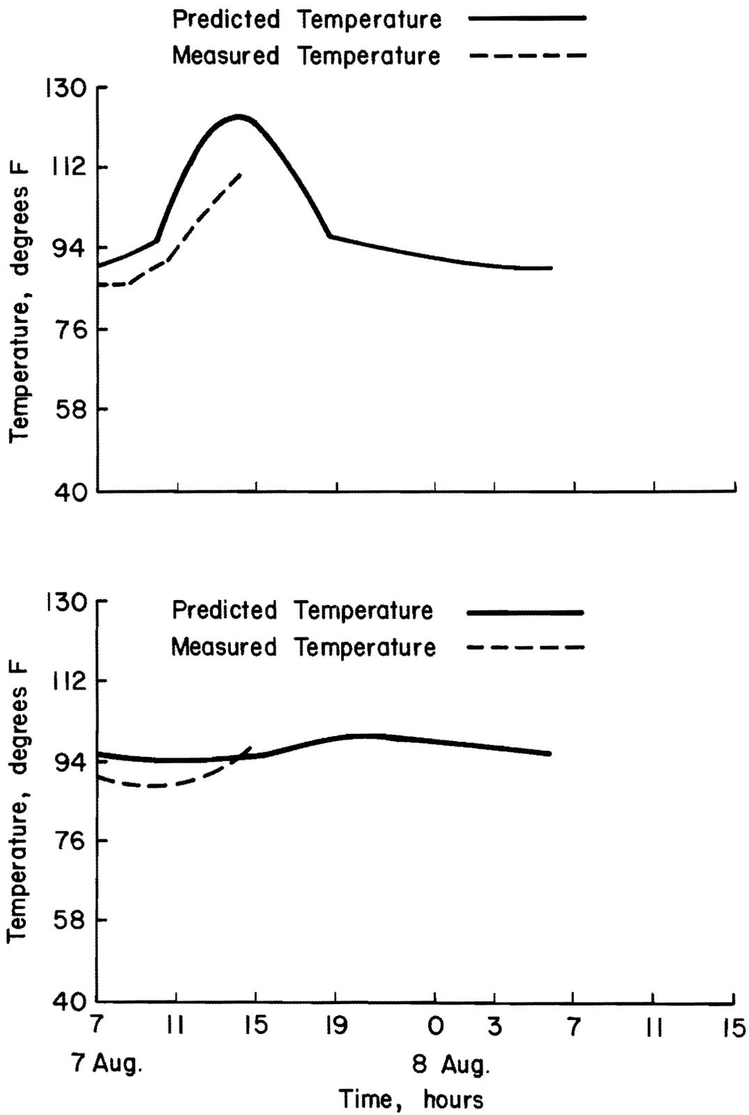
Fig 4.8. Variation in temperature of concrete slab on 7-8 Aug. 1981, Columbus Bypass, SH-71.
