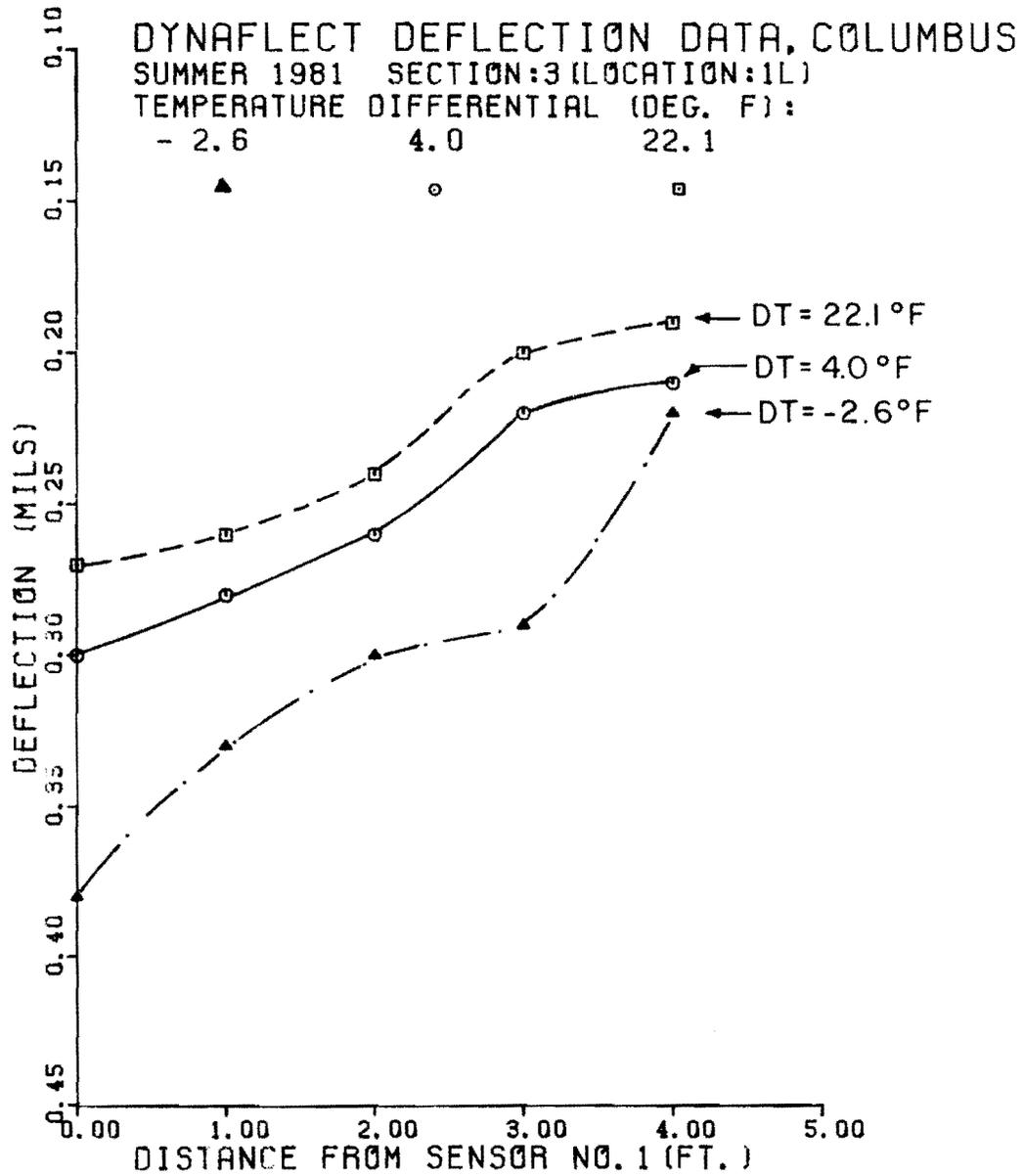
Fig 2.32. Deflection basins measured near the pavement edge at different temperature differentials.
