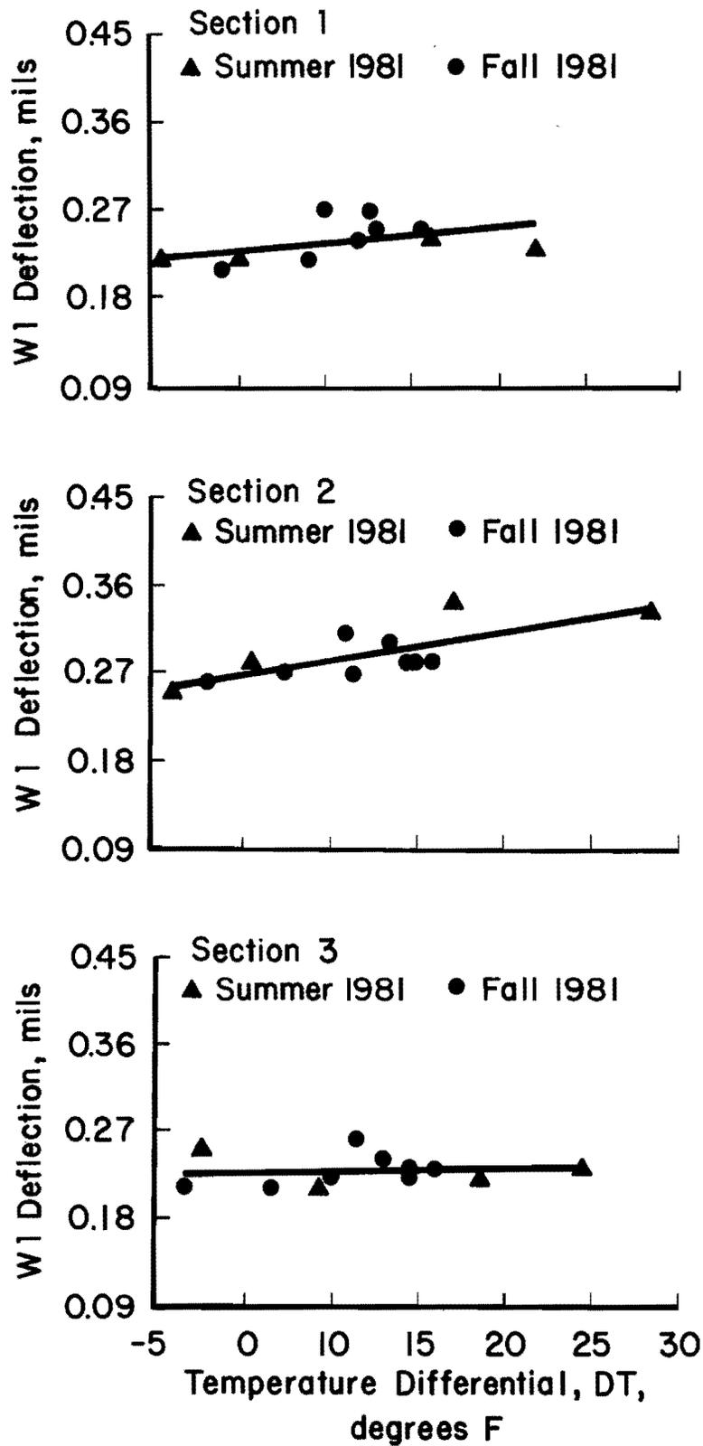
Fig B.1. The best fit lines estimated from simple linear regression analyses, (location 6L).
