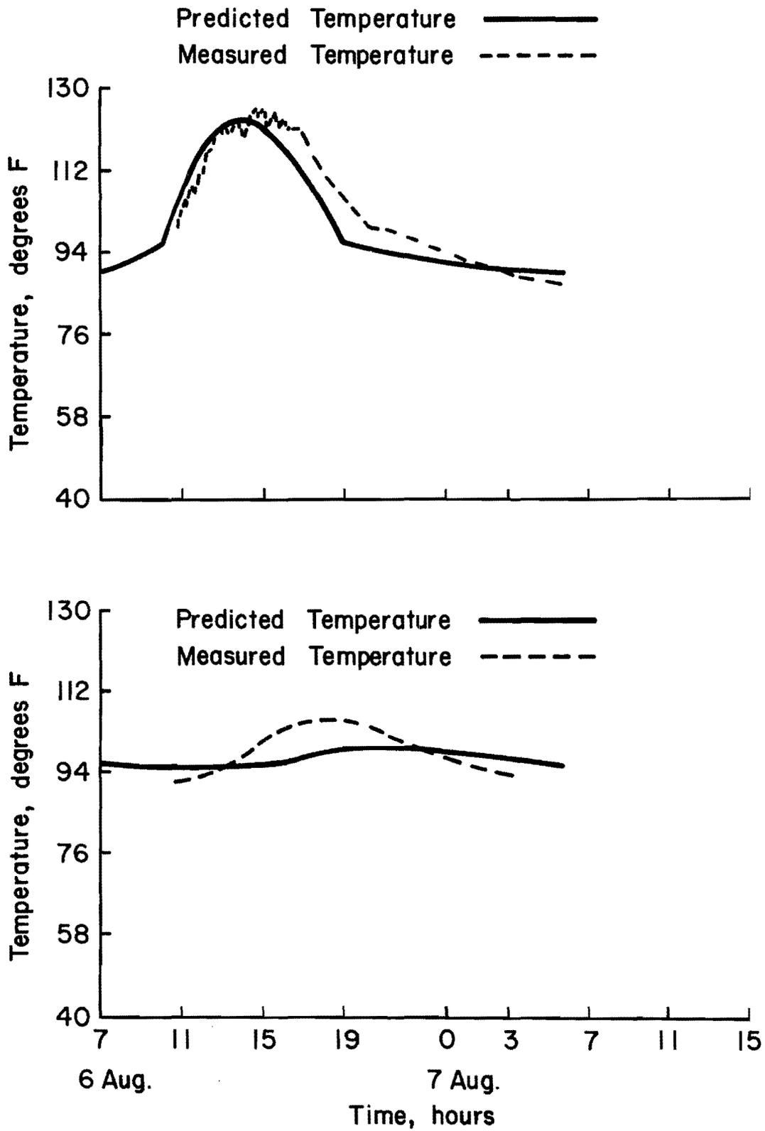
Fig 4.7. Variation in temperature of concrete slab on 6-7 Aug. 1981, Columbus Bypass, SH-71.
