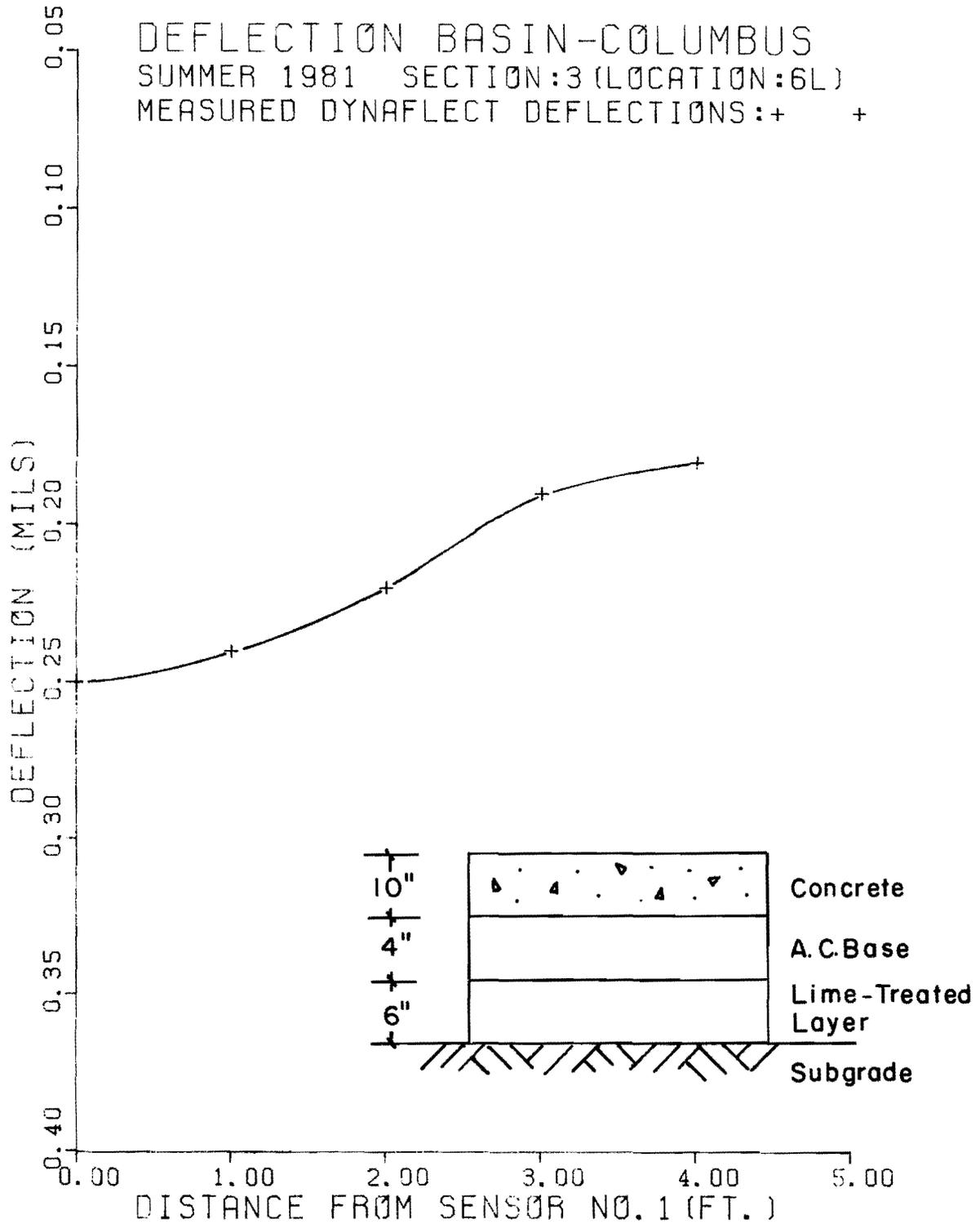
Fig 5.1. Measured deflection basin and pavement structure of the test section.
