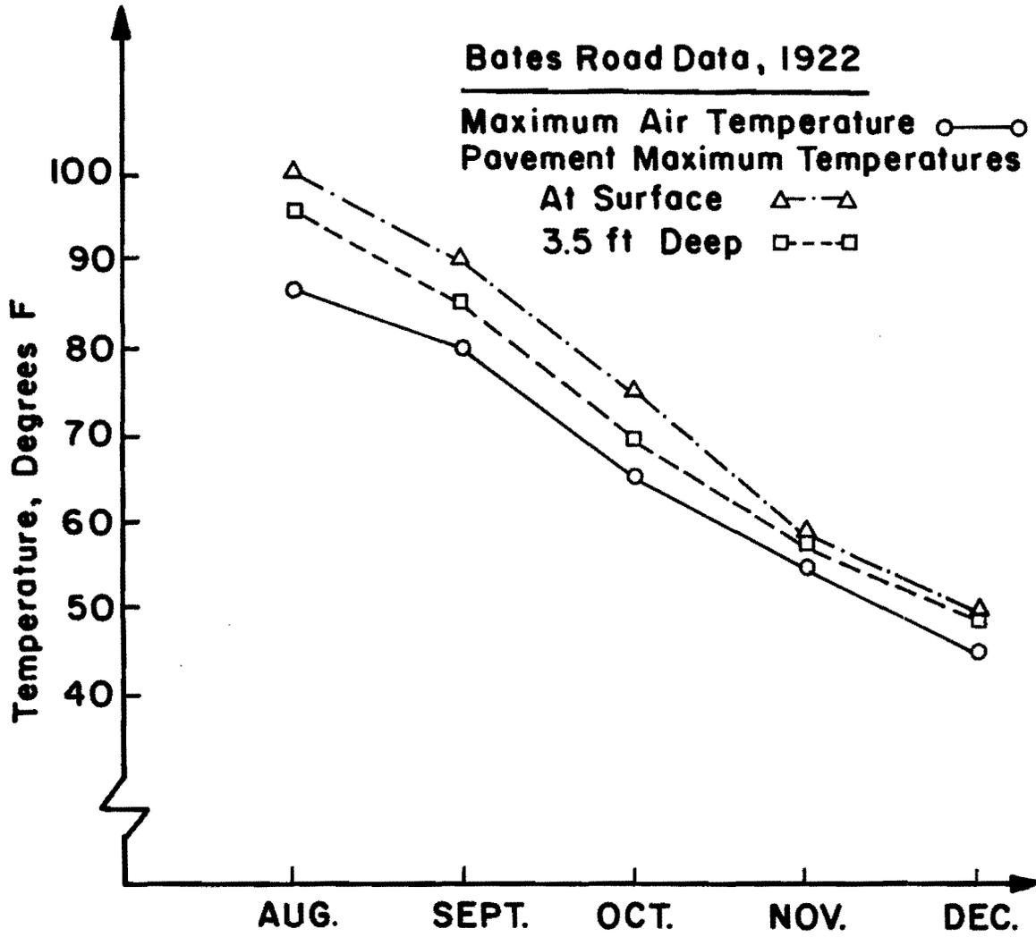
Fig 2.2. Monthly variation in air and concrete pavement temperatures - Bates Road Test (Ref 4).
