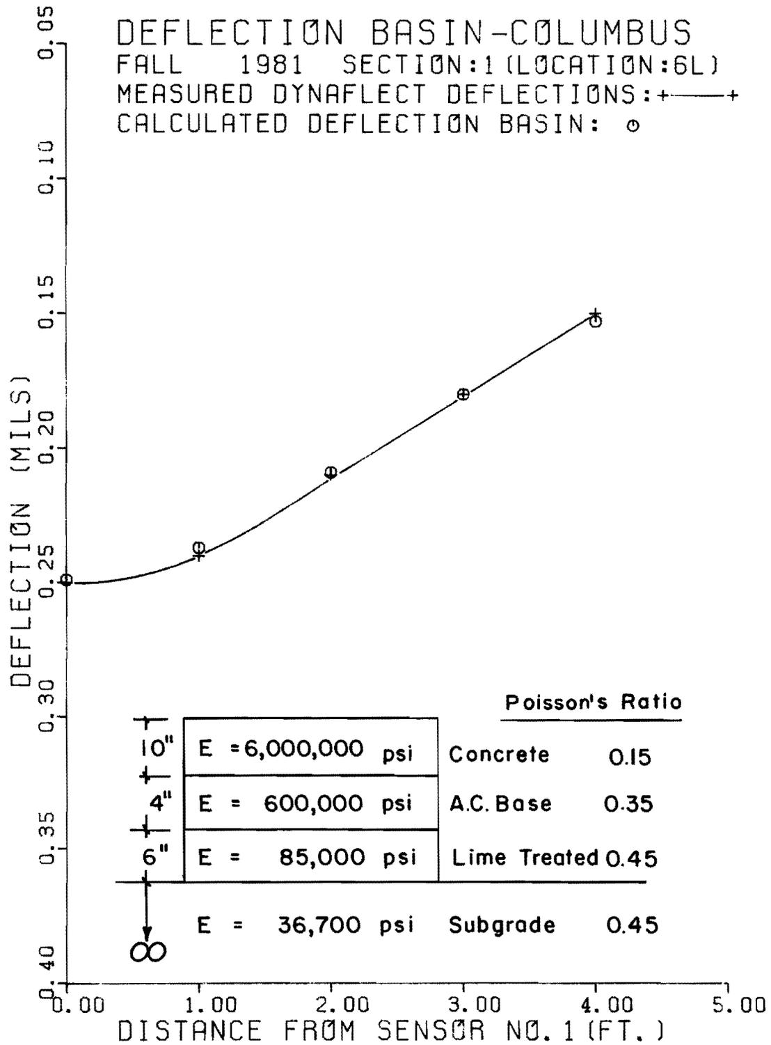
Fig F.5. Measured and calculated deflection basins (Example 3).
