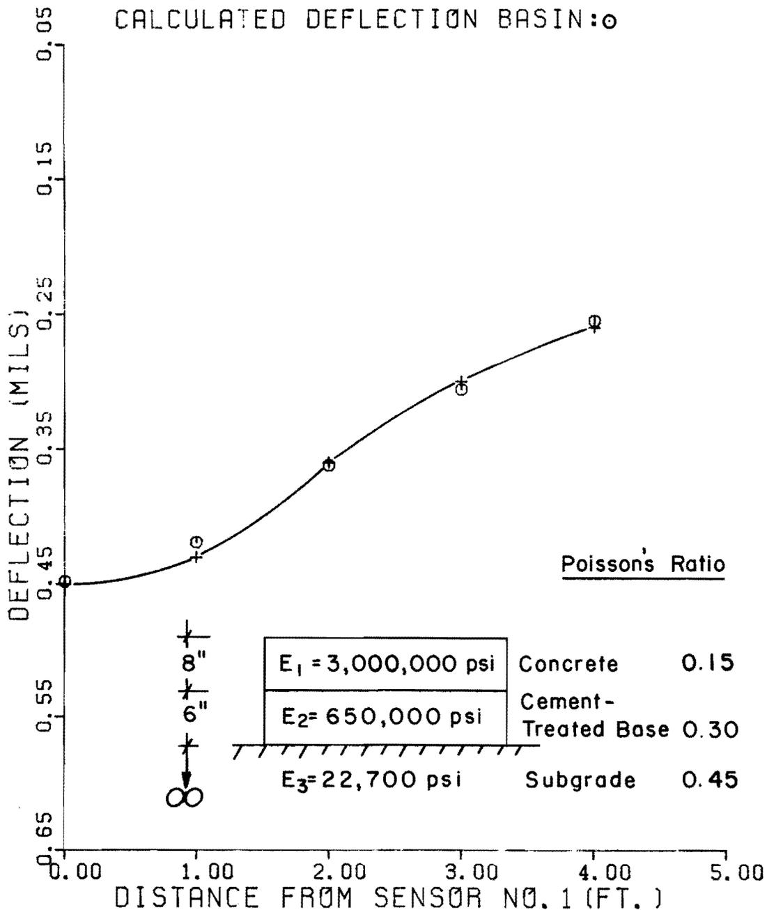
Fig F.10. Measured and calculated deflection basins (Example 8).
