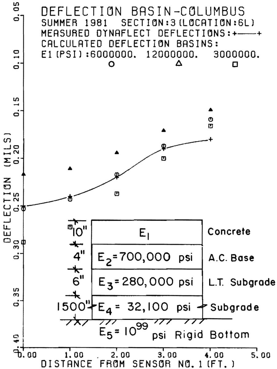
Fig 5.11. Effect of change of E<sub>1</sub> on calculated basin (case of rigid bottom).
