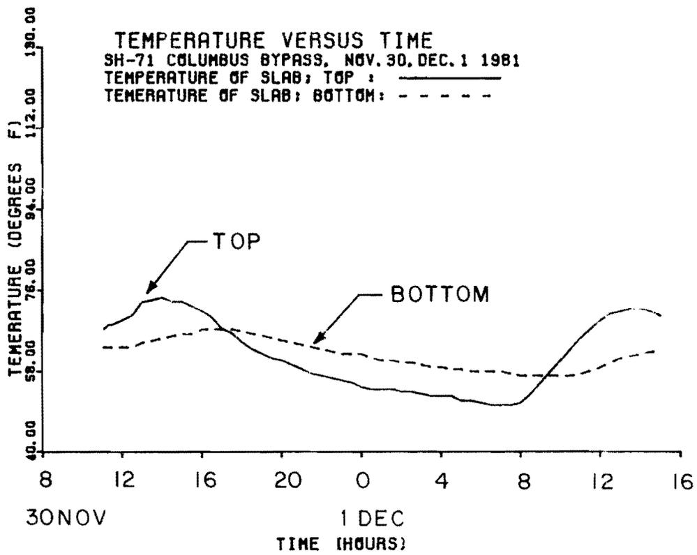
Fig 2.24. Temperature of top and bottom of concrete slab versus time, Fall 1981.
