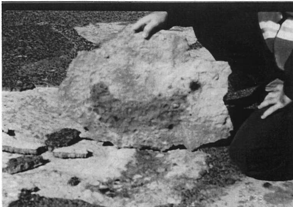
Figure 3. Large piece of debonded PUP mortar shows large dark area where material never bonded to the substrate.
