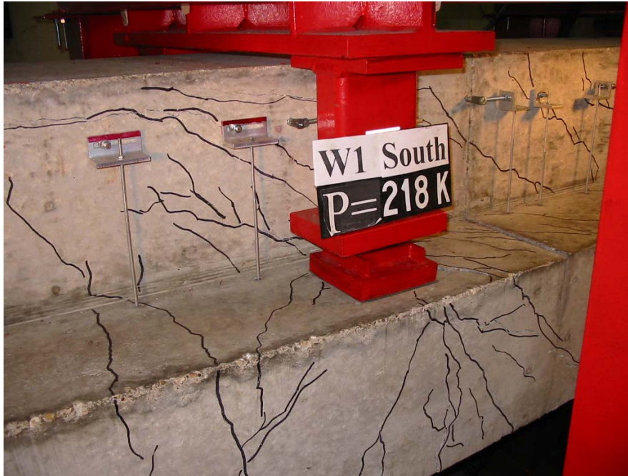
Fig. 4.2.4(c) LVDTs to study effective distribution width L_D along span
