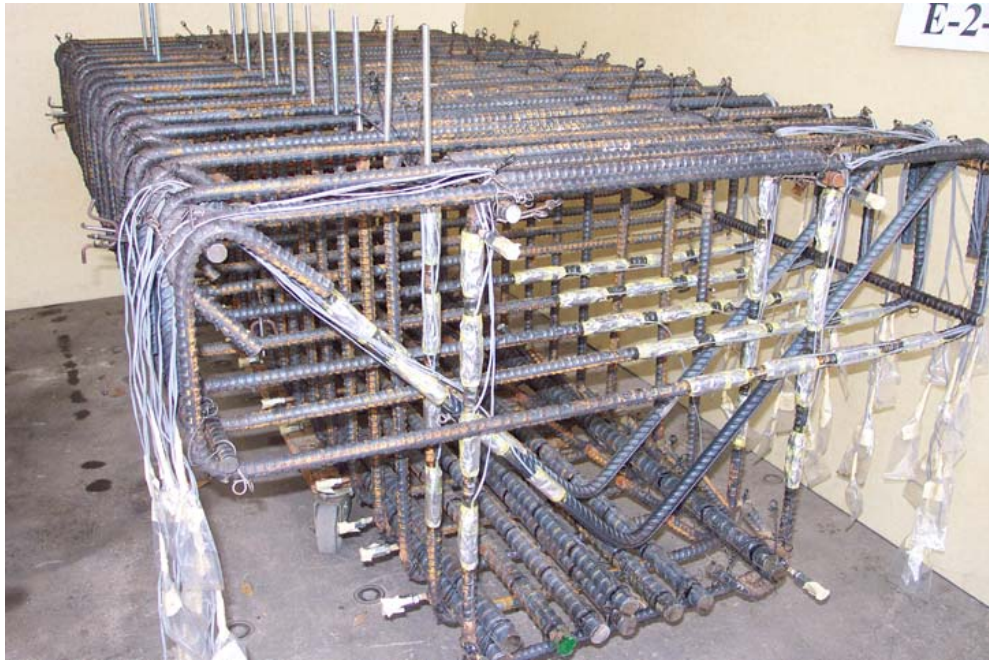
Fig. 3.1(d) Steel cage with two diagonal bars (Specimen E-2-6)
