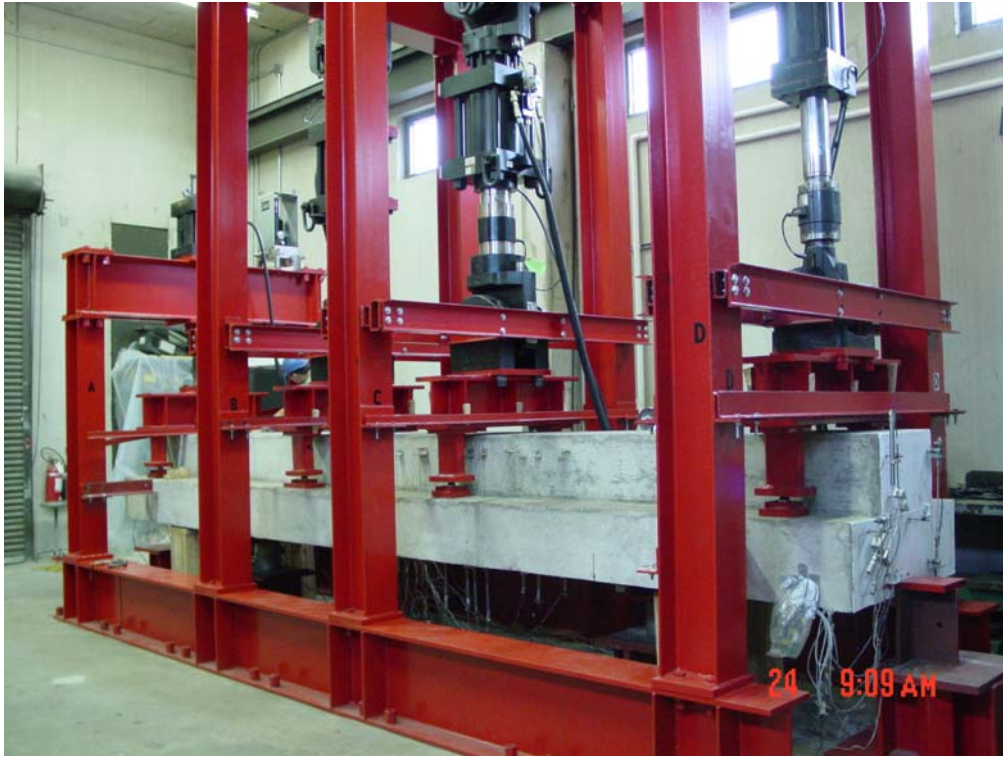
Fig. 4.2.2(a) Test frame setup with specimen
