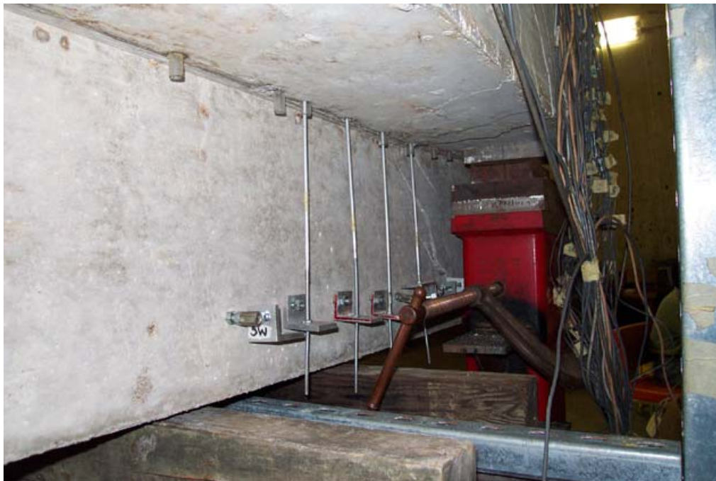
Fig. 3.1(e) LVDTs to study the variation of hanger steel strains along the span
