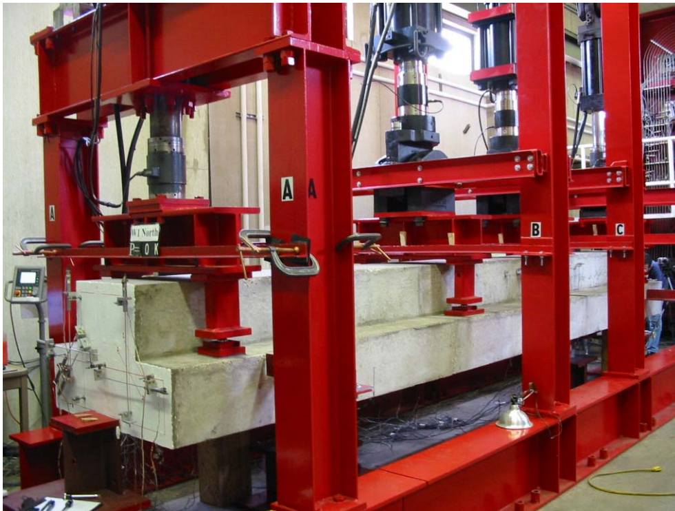
Fig. 4.2.2(b) Actuators A, B, C and D with whole specimen
