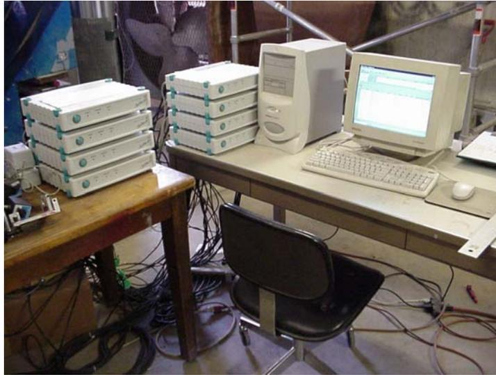
*Fig. 2.7 The HBM Spider 8 Data Acquisition System*
