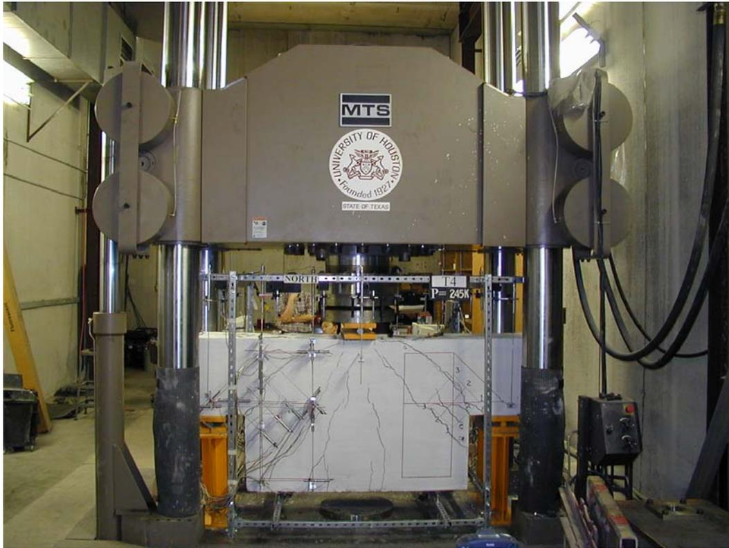
*Fig. 2.3 The MTS Test System and Testing Facility*
