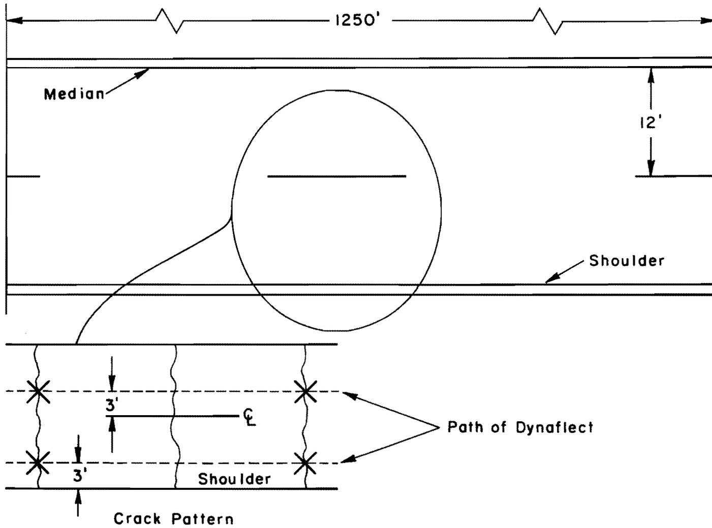
Fig 5. Layout of test sections for deflection testing.
