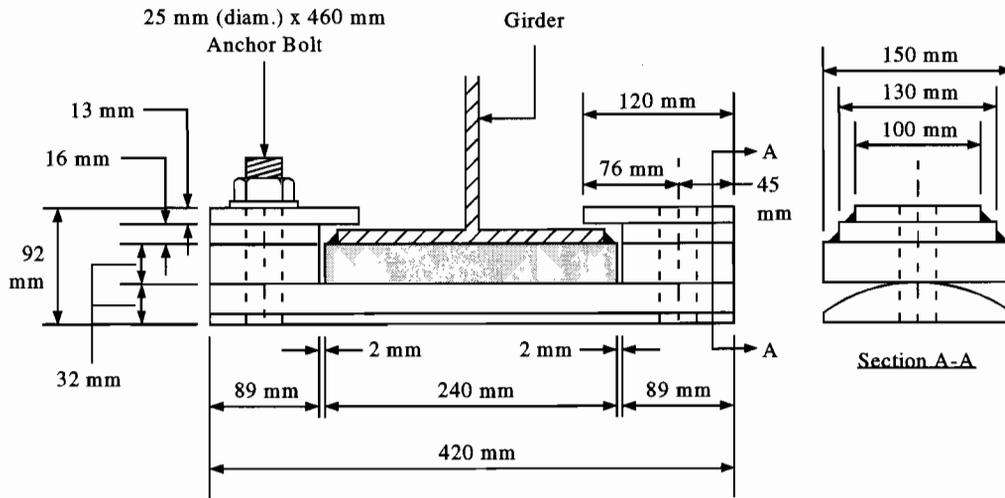
**Figure 4.7 Expansion Bearing Detail.**
