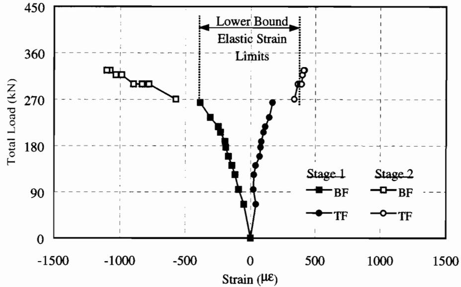
**Figure 6.10 Measured Strains on Bottom Flange (BF) and Top Flange (TF) of Girder 1 at Section d-d of Unit-N.**
