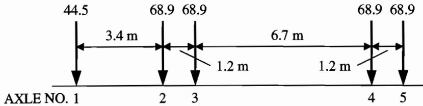
(c) TYPE 3-3: Unit Weight = 355.9 kN (80 kips)
