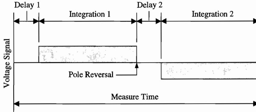
**Figure 3.12 Measurement Sequence for a Single Channel.**
