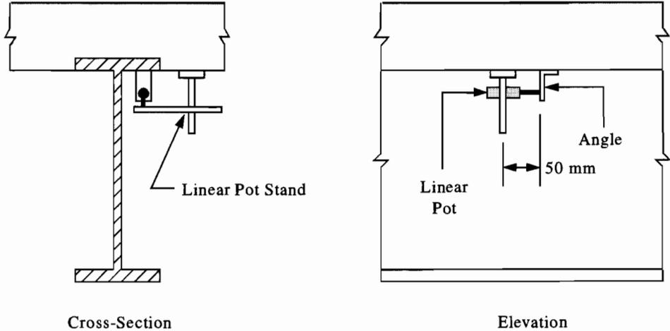
**Figure 5.13 Mounting Assembly for Typical Slip Transducer.**
