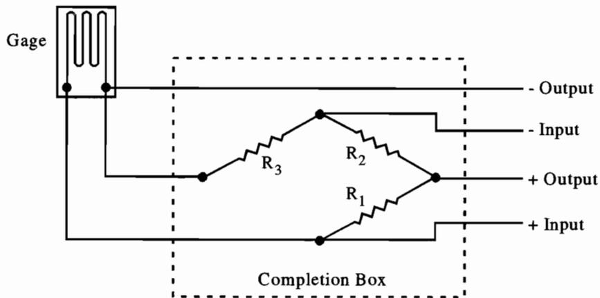
**Figure 3.11 Wiring Layout for Three-Wire, Quarter Bridge Circuit.**
