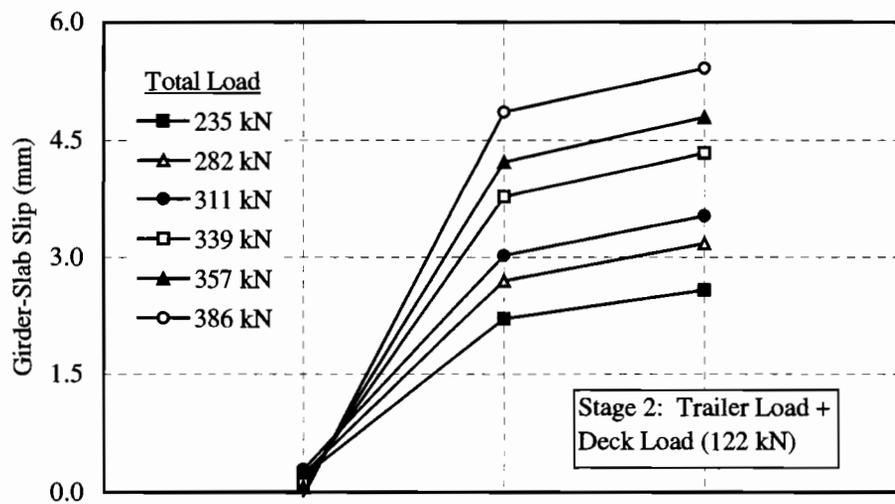
Figure 6.27 Slip Profile Along Length of Girder 2 at Unit-S for Load Position 4.
