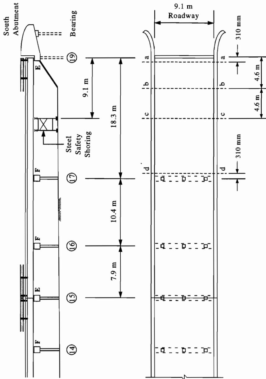
Figure 5.18 Instrumented Sections of Unit-S.
