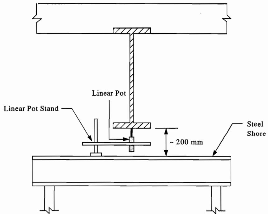
**Figure 5.14** *Mounting Assembly for Typical Deflection Transducer.*
