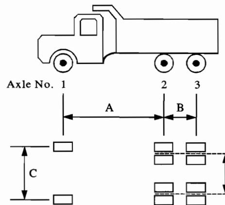
**Figure 5.11 Service Load Run in Progress and Measured Vehicle Configurations.**
