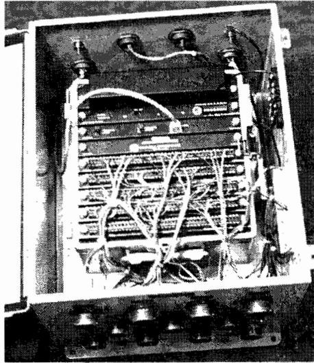
**Figure 3.4 CR9000C Data Logger in Steel Enclosure.**
