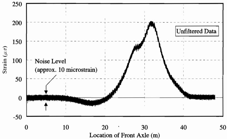
**Figure 6.3 Typical Service Load Strain Record before Filtering.**
