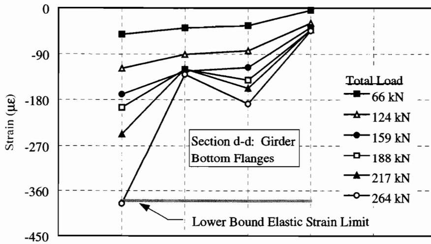
Figure 6.11 Girder Strain Profile at Section d-d of Unit-N during Stage 1 Loading.
