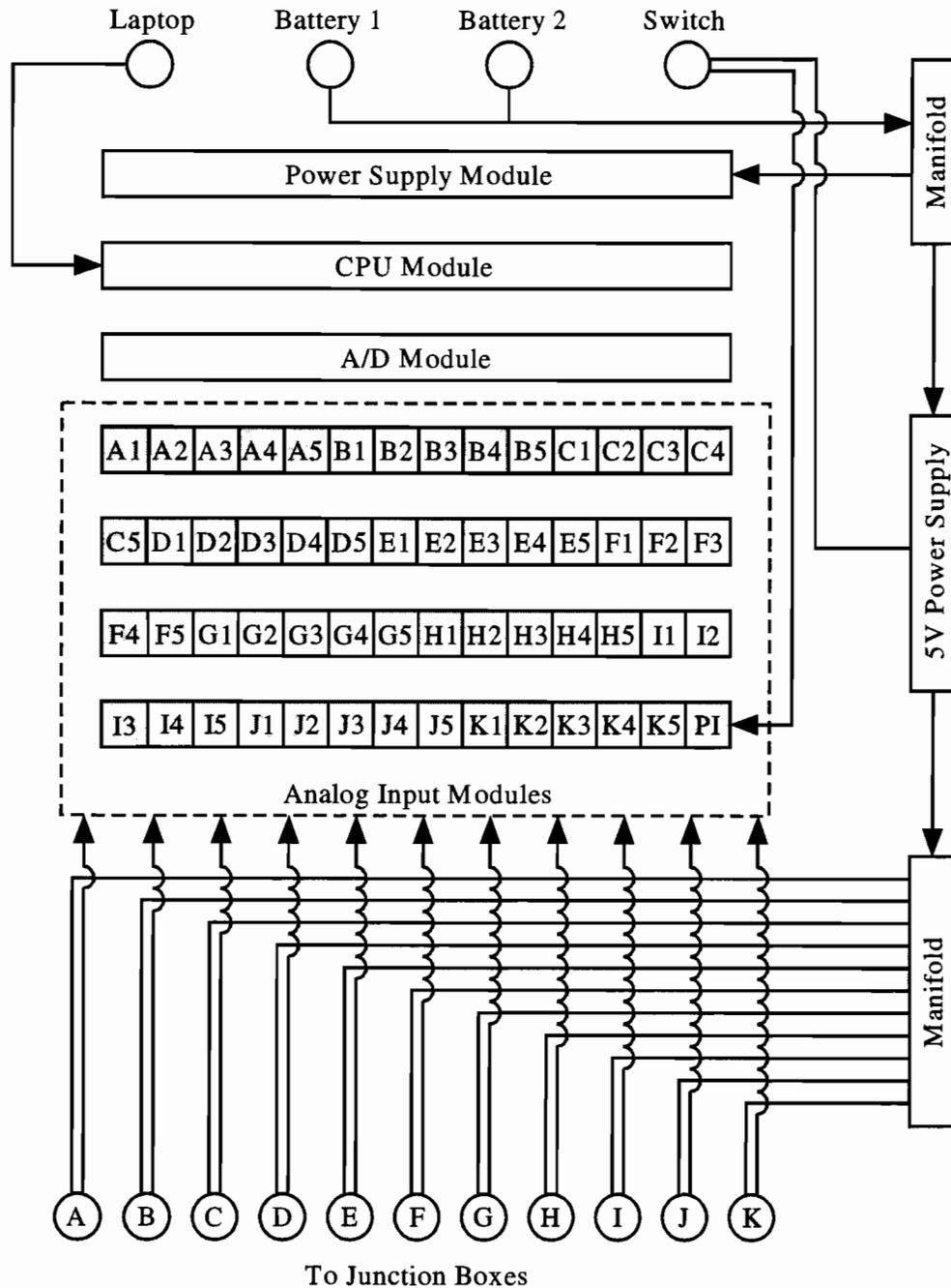
**Figure 3.7** *Wiring Layout Inside CR9000C Steel Enclosure.*
