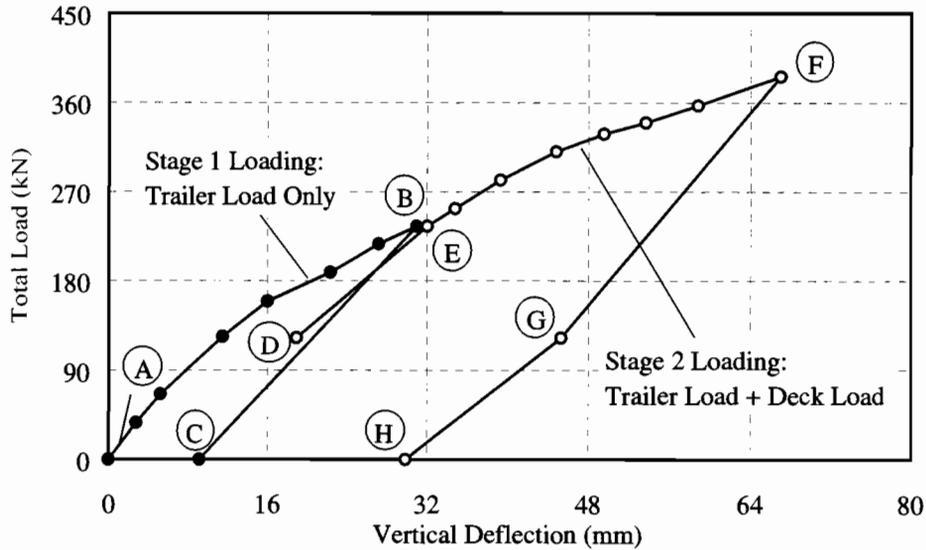
**Figure 6.7 Vertical Deflection Response for Girder 2 of Unit-S.**
