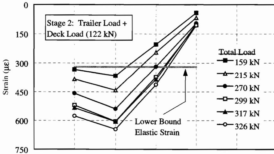
Figure 6.14 Bottom Flange Strains at Section c-c of Unit-N for Load Position 4.
