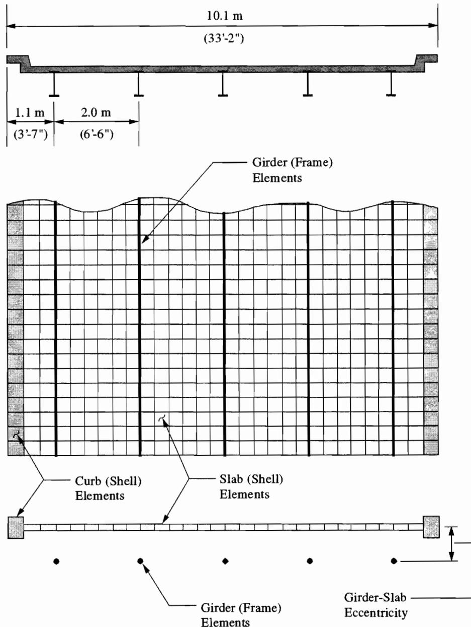
**Figure 8.1** *Finite Element Modeling of Marlin Bridge Units.*
