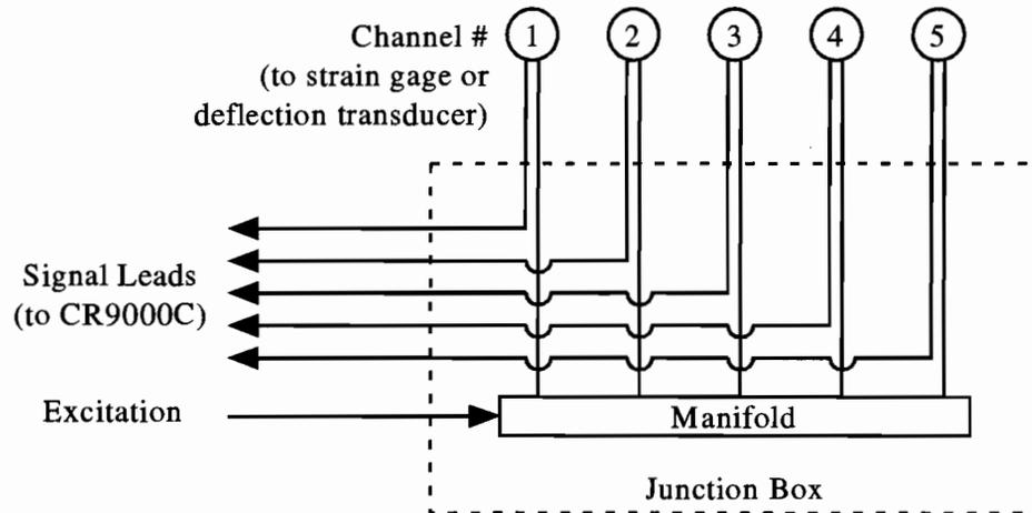
**Figure 3.9 Junction Box Wiring Layout.**
