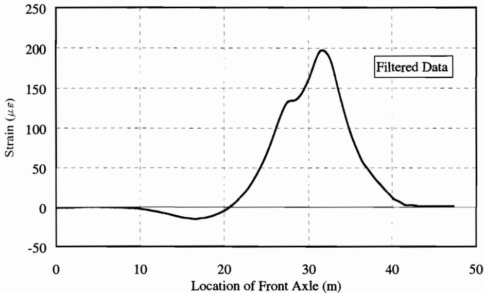
**Figure 6.4 Typical Service Load Strain Record after Filtering.**
