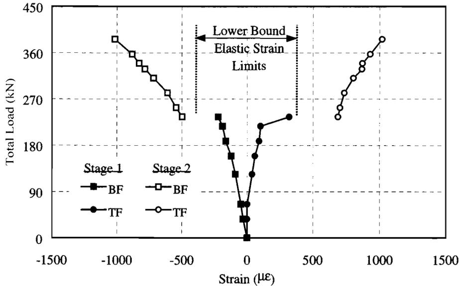
**Figure 6.15 Measured Strains on Bottom Flange (BF) and Top Flange (TF) of Girder 1 at Section d-d of Unit-S.**
