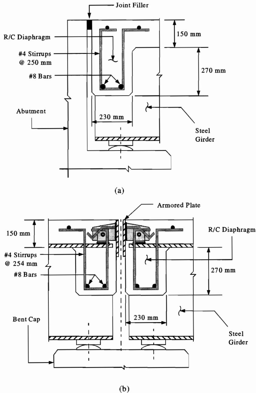
Figure 4.9 Expansion Joint Detail (a) At Abutment and (b) Between Units.
