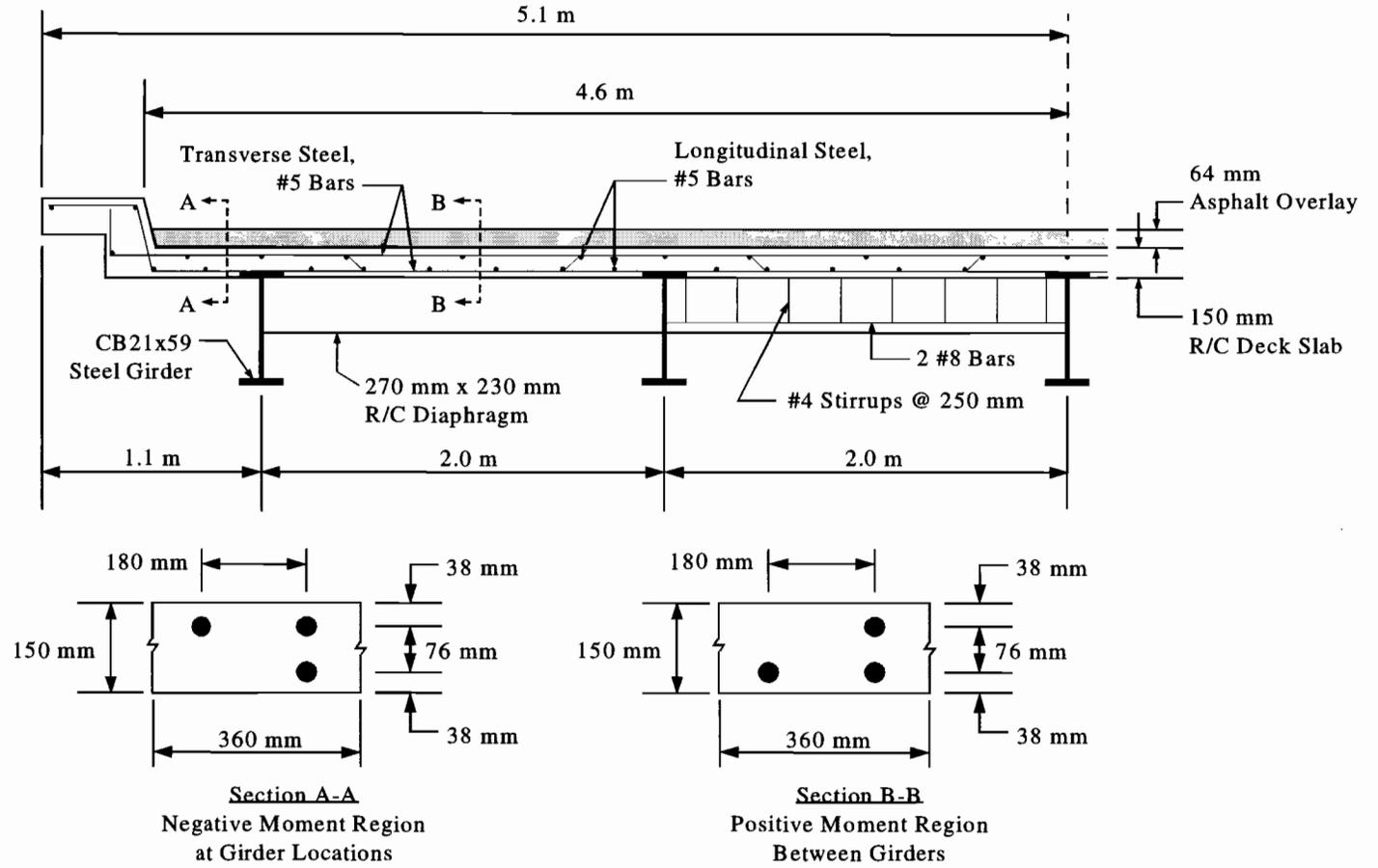
Figure 4.5 Curb and Railing Detail.
