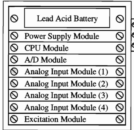
**Figure 3.3 Module Layout of CR9000C Data Logger.**
