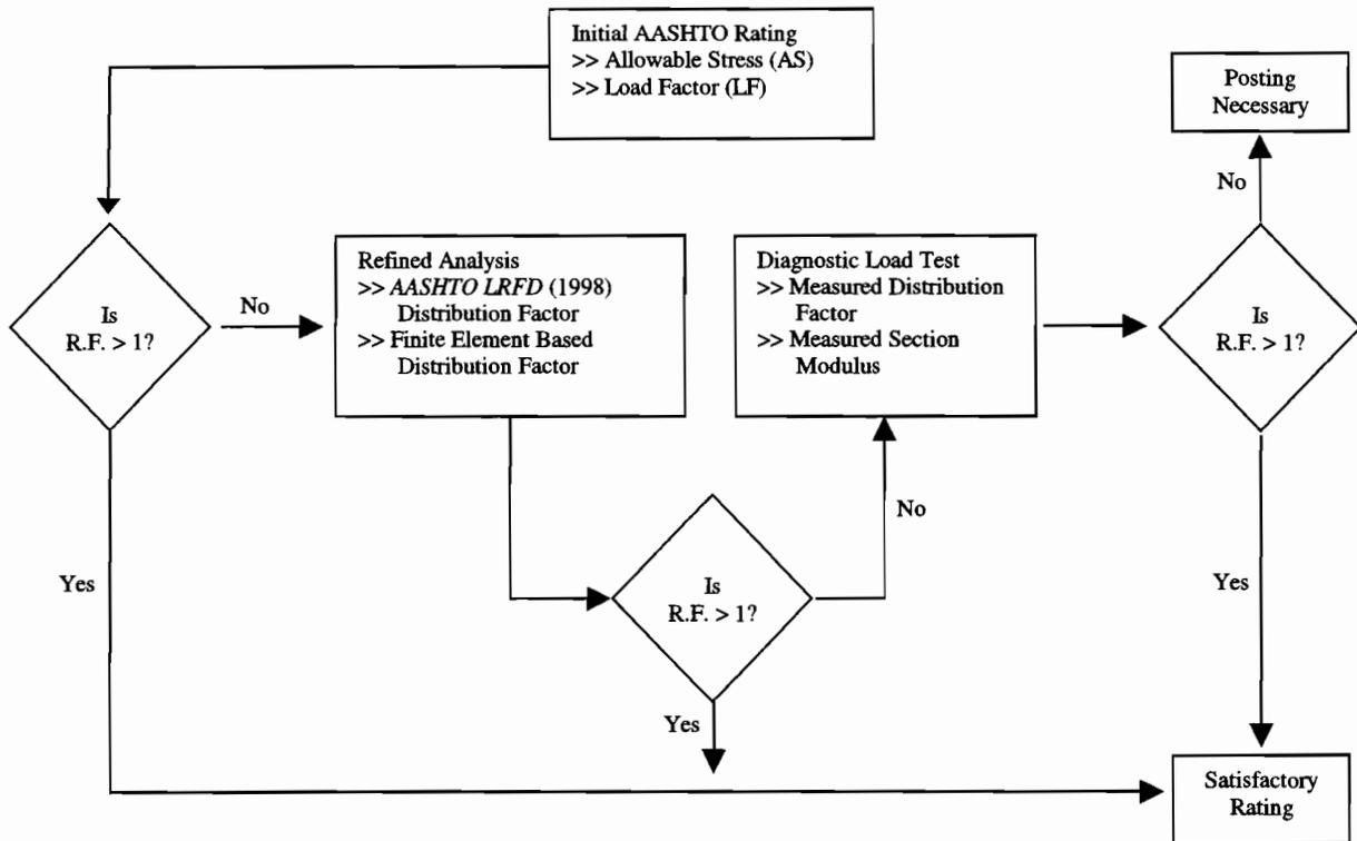
Figure 9.1 Flowchart of Experimental Bridge Rating Process.
