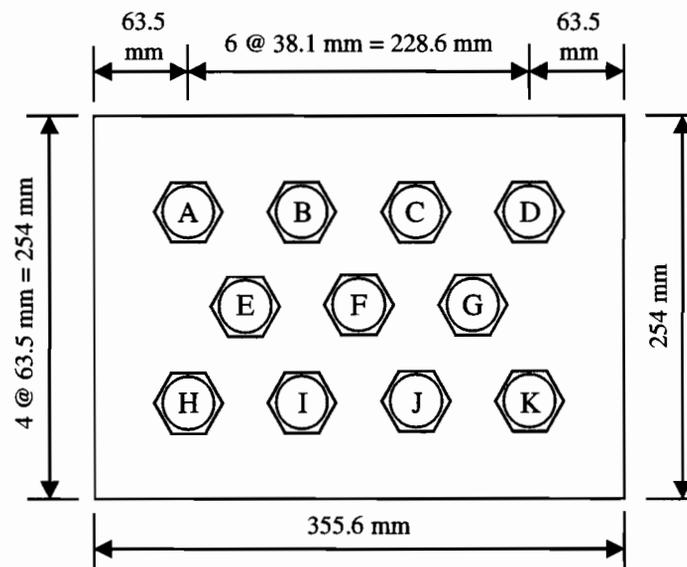
**Figure 3.5 Side 1 of Data Logger Enclosure.**
