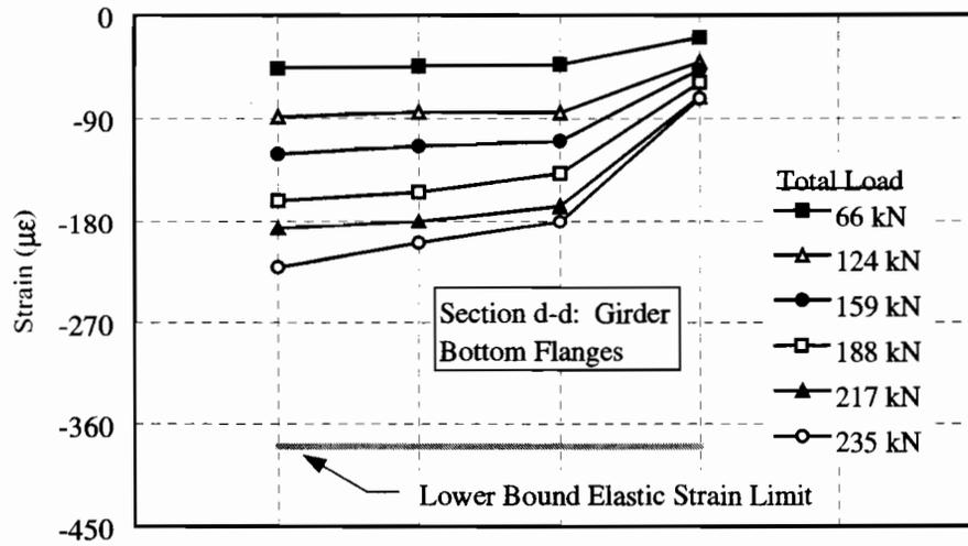
Figure 6.16 Girder Strain Profile at Section d-d of Unit-S during Stage 1 Loading.
