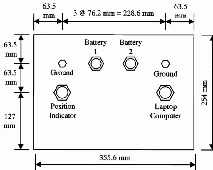
**Figure 3.6 Side 2 of Data Logger Enclosure.**
