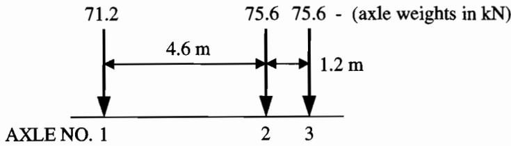
(b) TYPE 3S2: Unit Weight = 320.3 kN (72 kips)
