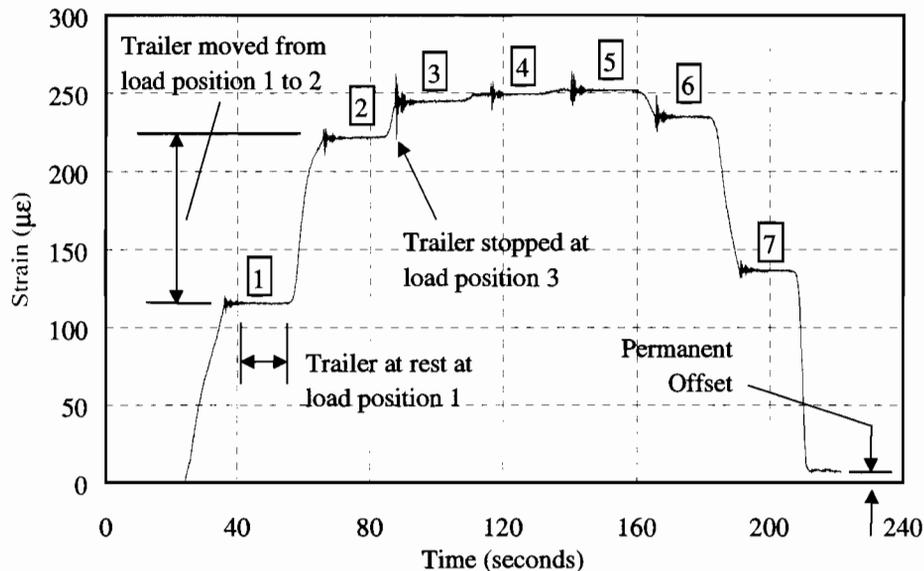
**Figure 6.1 Typical Strain History during Trailer Load Sequence.**
