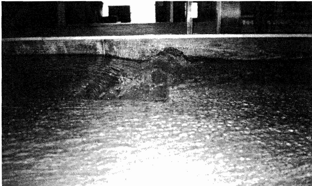
Figure C.12 Test Conducted on Drain 4, Illustrating Splash Occuring at the Shallow End of the Drain Pan
