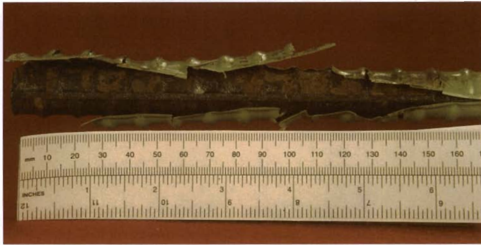
Figure 3.4 Coating debonding of splice bar (beam study).
