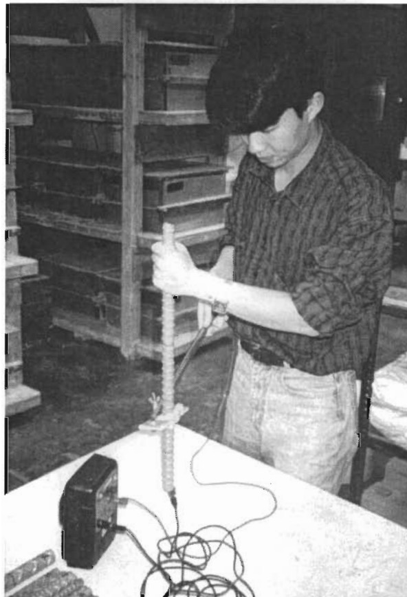
Figure 1.1 Operation of the holiday detector.
