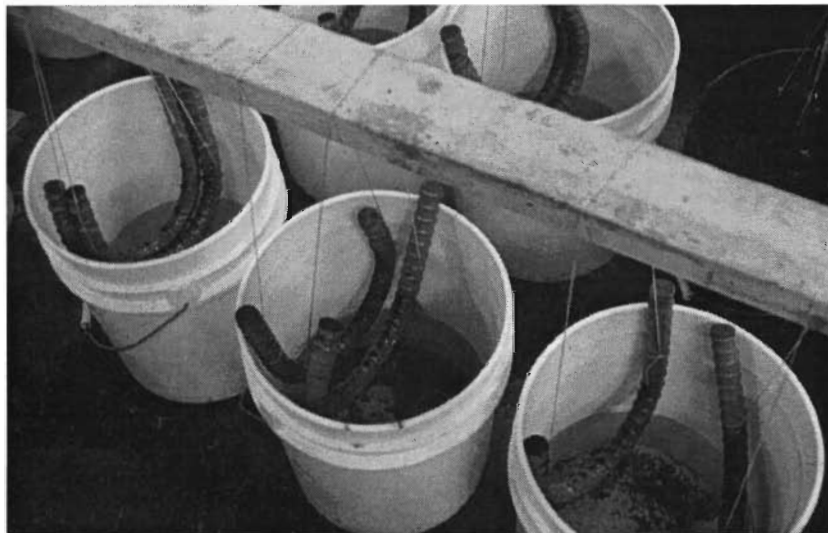
Figure 1.6 Test setup for immersion study.
