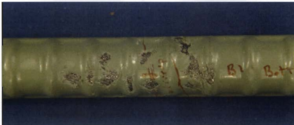
Figure 3.18 Coating adhered well throughout most portions of bars from beam B1.
