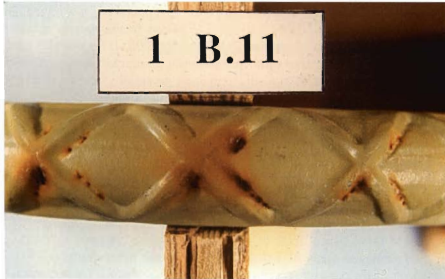
Figure 2.16 Corrosion at holidays not detected before immersion in 3.5% NaCl after about 8 months of exposure.
