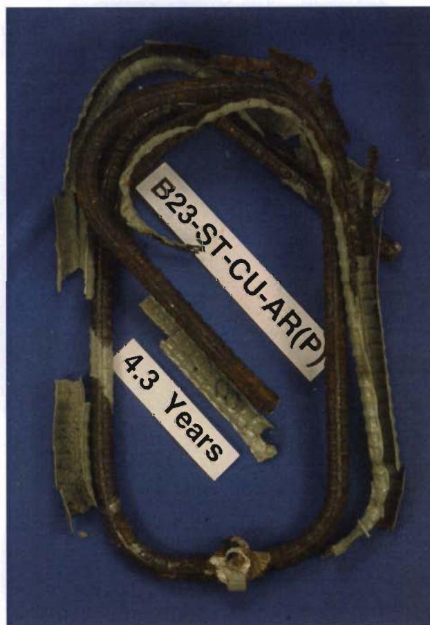
Figure 3.17 Coating extensively debonded on stirrups (beam study).
