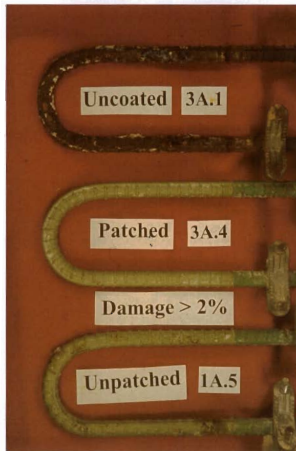
Figure 2.6 Comparative performance of uncoated and coated bars after 4.5 years of exposure (macrocell study).
