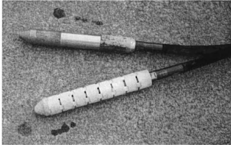
Figure 1.4 Metal (top) and rubber head vibrators.
