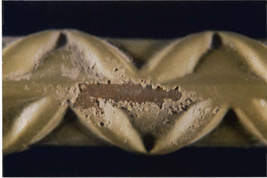
Figure 4.6 Damage to coating caused by metal head vibrator on test bar from Phase 1 study.
