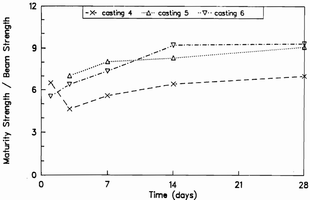
Fig B-31. Ratio of maturity method strengths to flexural strengths of wetroom-cured beams for castings 4, 5, and 6. Maturity curve based on cores drilled from slabs.
