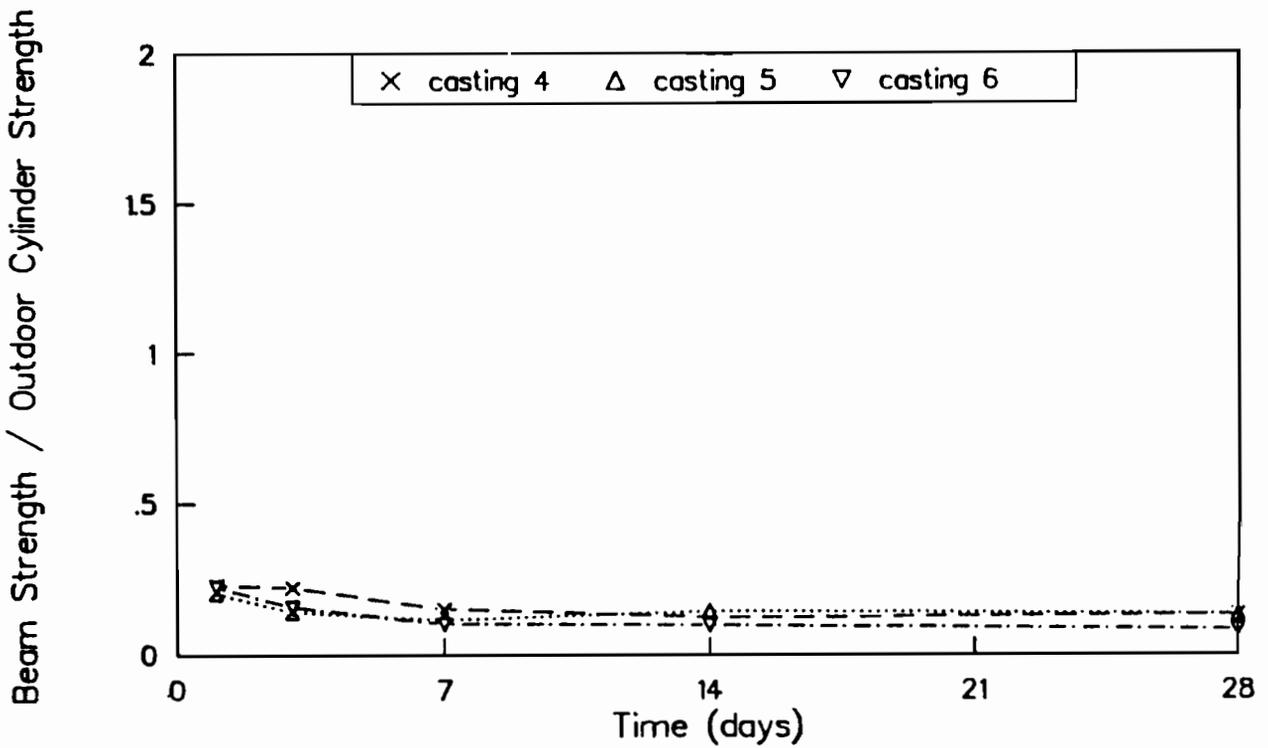
Fig B-15. Ratio of flexural strengths of outdoor-cured beams to strengths of outdoor-cured cylinders for castings 4, 5, and 6.
