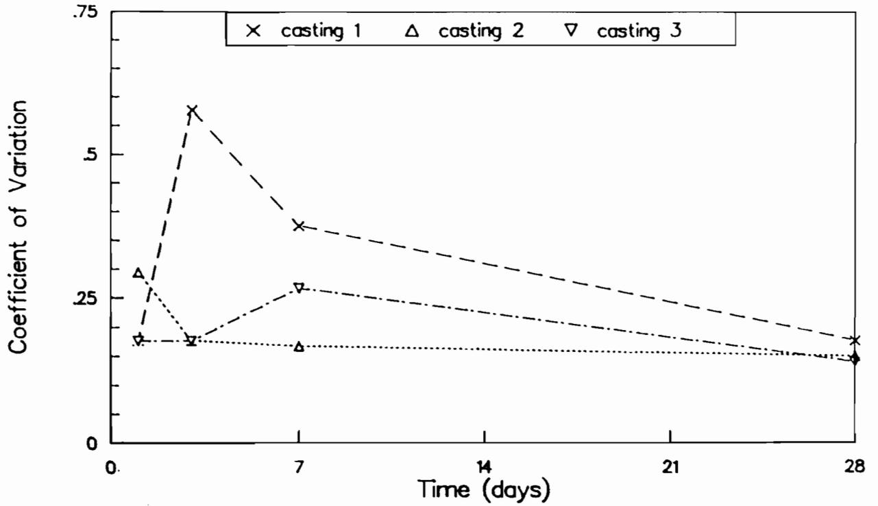
Fig A-18. Coefficient of variation of rebound number strengths for castings 1, 2, and 3.
