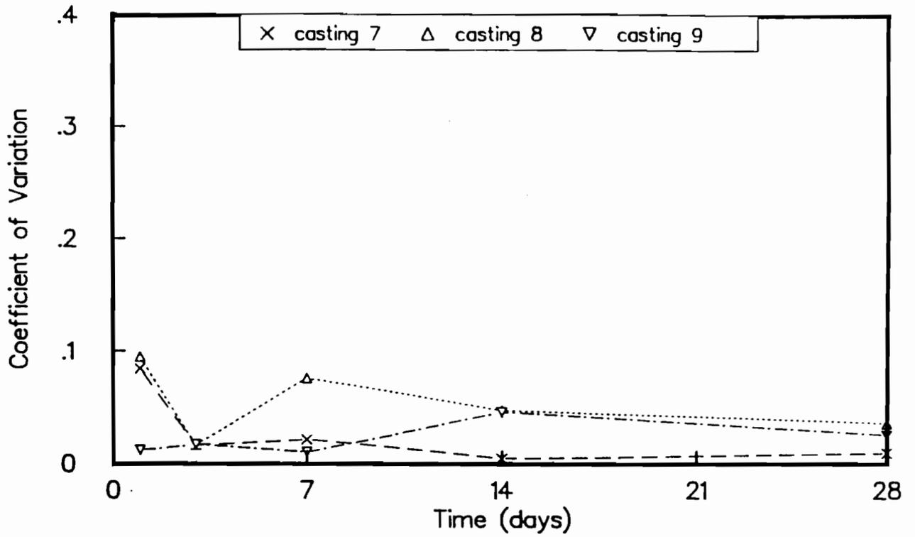
Fig C-45. Coefficient of variation of wetroom-cured cylinder strengths for castings 7, 8, and 9.
