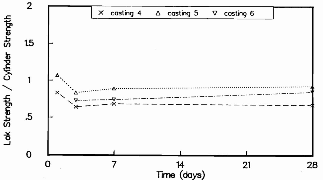
Fig B-5. Ratio of "Lok-Test" pullout strengths to strengths of wetroom-cured cylinders for castings 4, 5, and 6.
