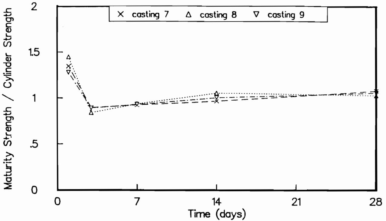
Fig C-7. Ratio of maturity method strengths to strengths of wetroom-cured cylinders for castings 7, 8, and 9. Maturity curve based on wetroom-cured cylinders.
