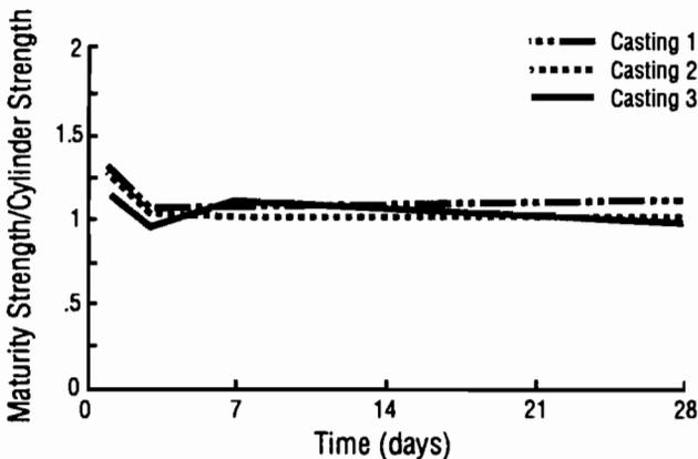
**Fig 5-10. Ratio of maturity method strength to strength of wetroom-cured cylinders for castings 1, 2, and 3.**
