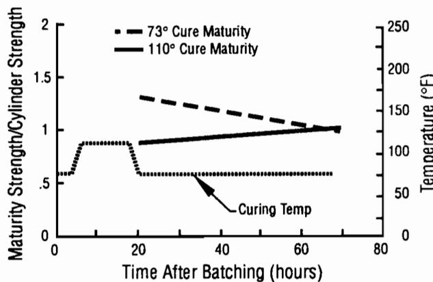
Fig 5-36. Ratio of maturity method strength to cylinder strength for casting 10.
