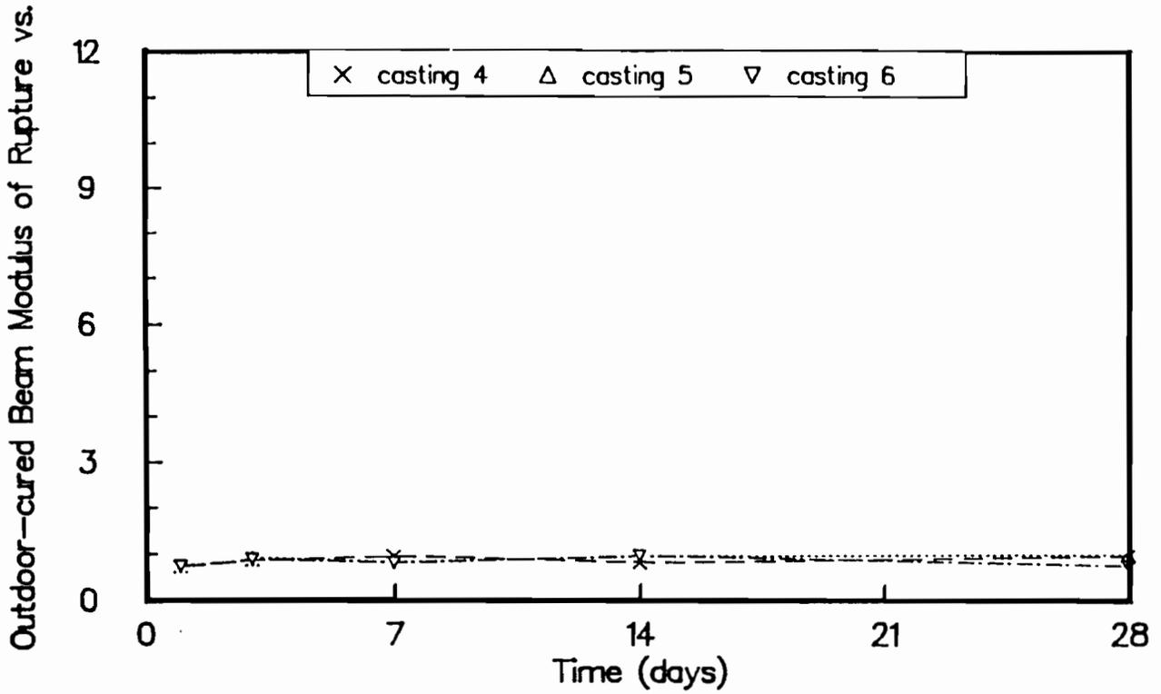
Fig B-26. Ratio of flexural strengths of outdoor-cured beams to flexural strengths of wetroom-cured beams for castings 4, 5, and 6.
