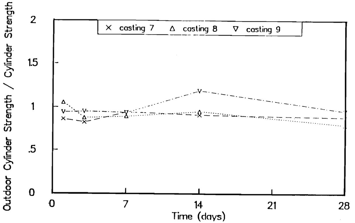
Fig C-1. Ratio of strengths of outdoor-cured cylinders to strengths of wetroom-cured cylinders for castings 7, 8, and 9.
