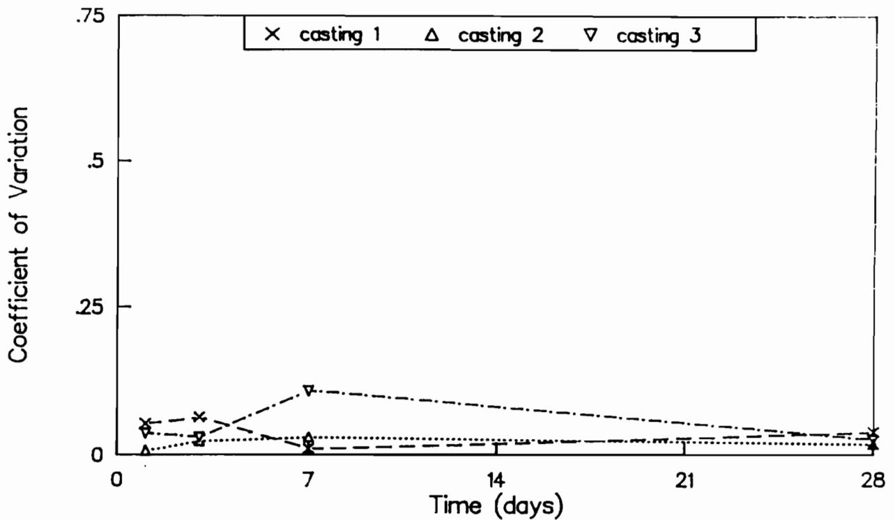
Fig A-13. Coefficient of variation of wetroom-cured cylinder strengths for castings 1, 2, and 3.
