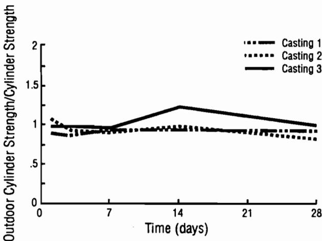
**Fig 5-17. Ratio of outdoor-cured cylinder strength to strength of wetroom-cured cylinders for castings 7, 8, and 9.**
