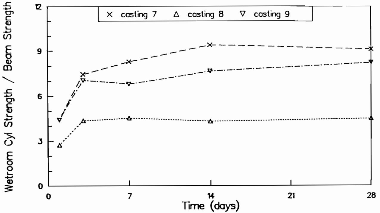
Fig C-23. Ratio of strengths of wetroom-cured cylinders to flexural strengths of wetroom-cured beams for castings 7, 8, and 9.
