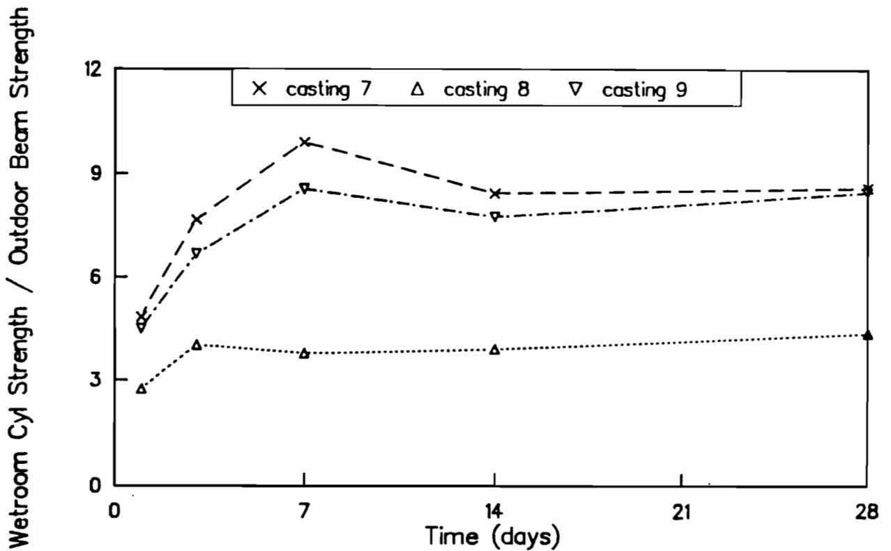
Fig C-34. Ratio of strengths of wetroom-cured cylinders to flexural strengths of outdoor-cured beams for castings 7, 8, and 9.
