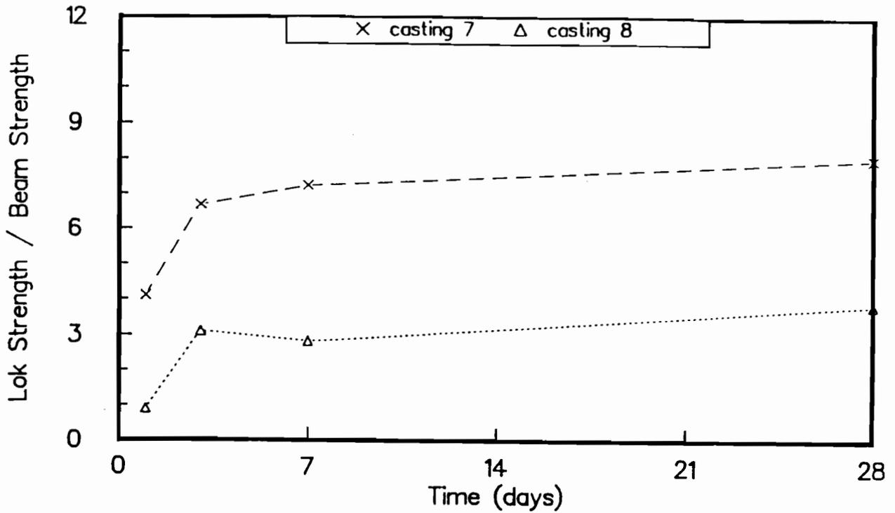
Fig C-27. Ratio of "Lok-Test" pullout strengths to flexural strengths of wetroom-cured beams for castings 7 and 8.
