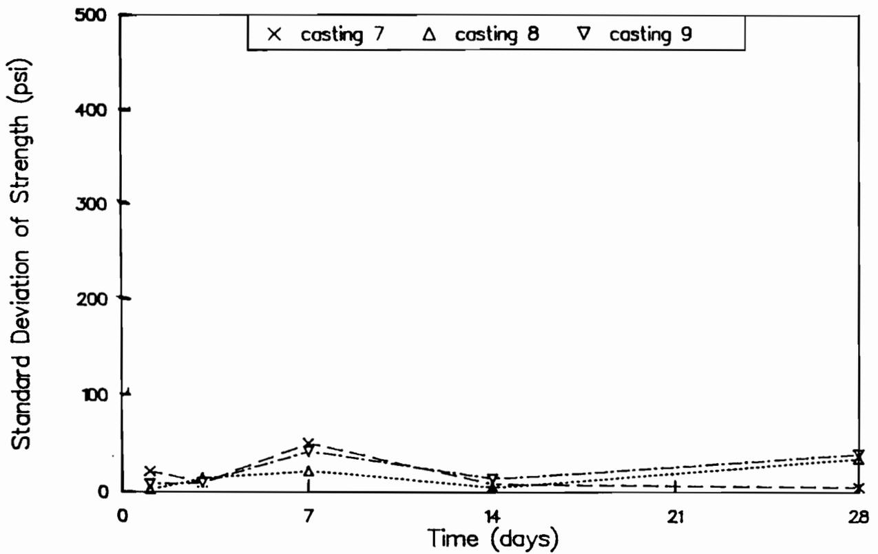
Fig C-60. Standard deviation of flexural strength of wetroom-cured beams for castings 7, 8, and 9.
