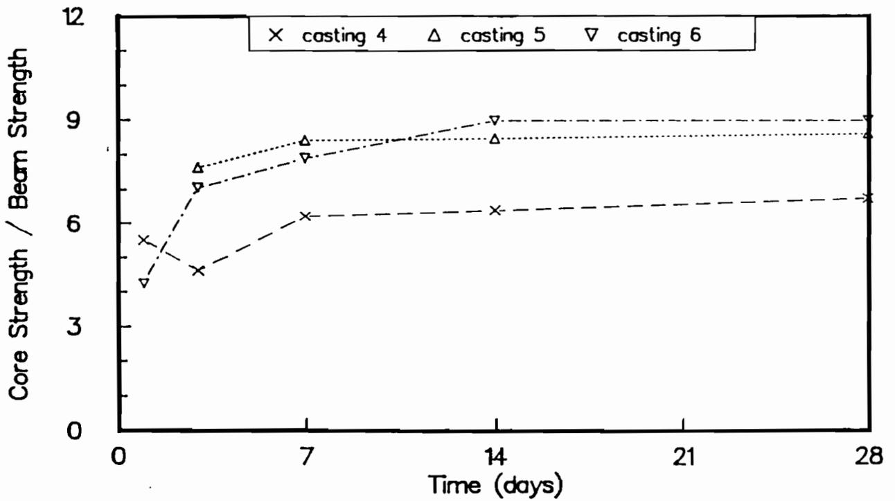
Fig B-25. Ratio of strengths of cores to flexural strengths of wetroom-cured beams for castings 4, 5, and 6.
