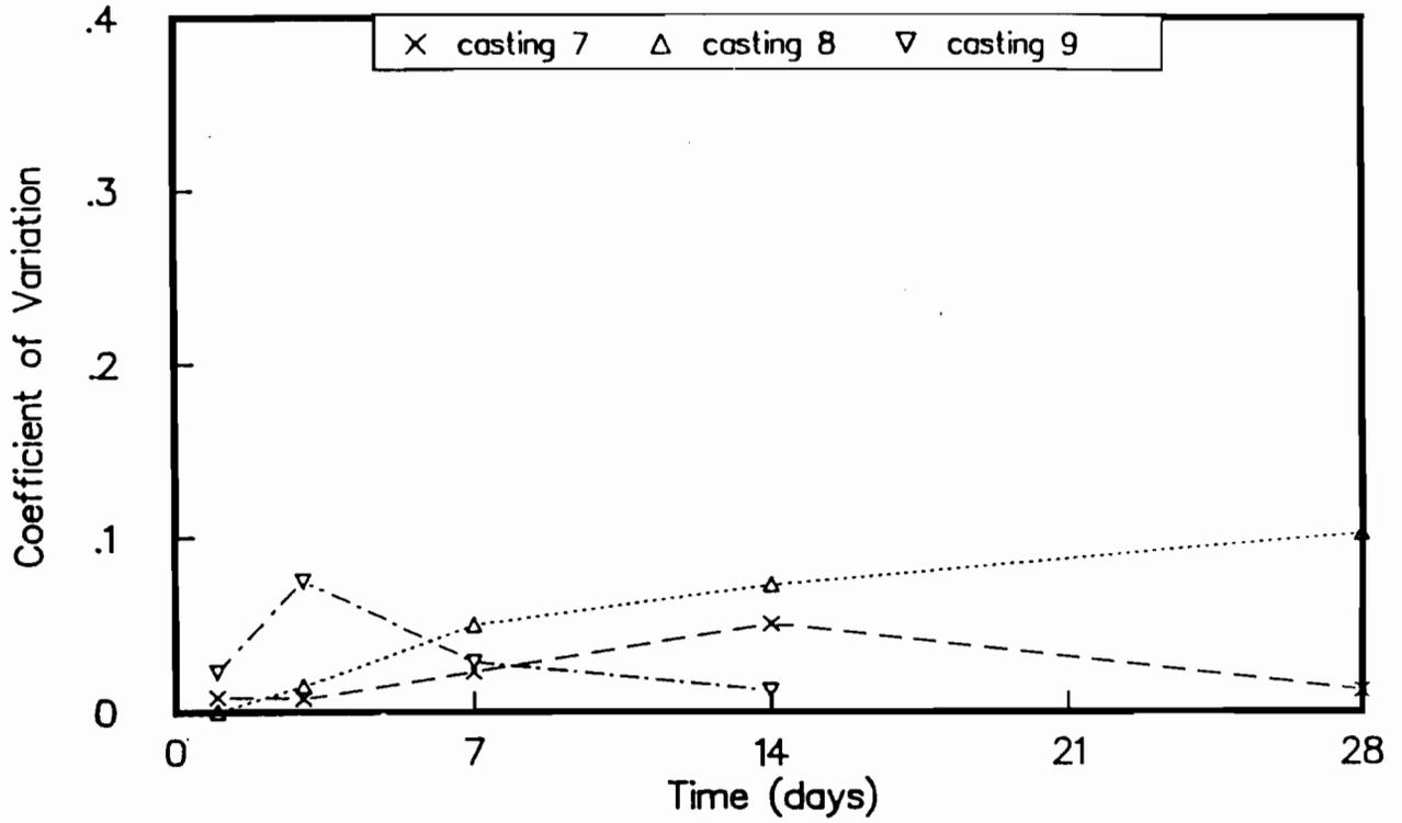
Fig C-47. Coefficient of variation of cores drilled from slabs for castings 7, 8, and 9.
