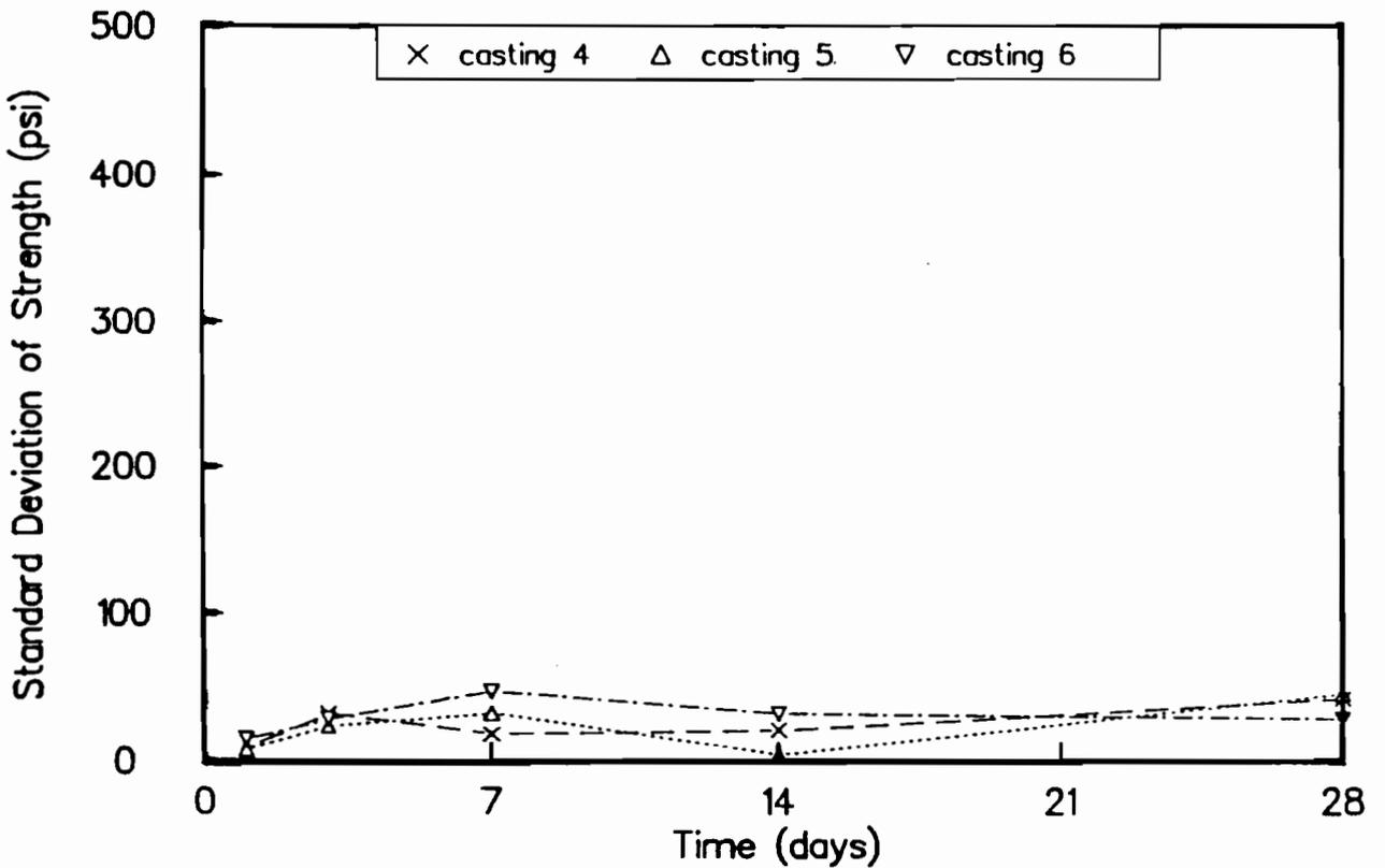
Fig B-61. Standard deviation of flexural strength of outdoor-cured beams for castings 4, 5, and 6.
