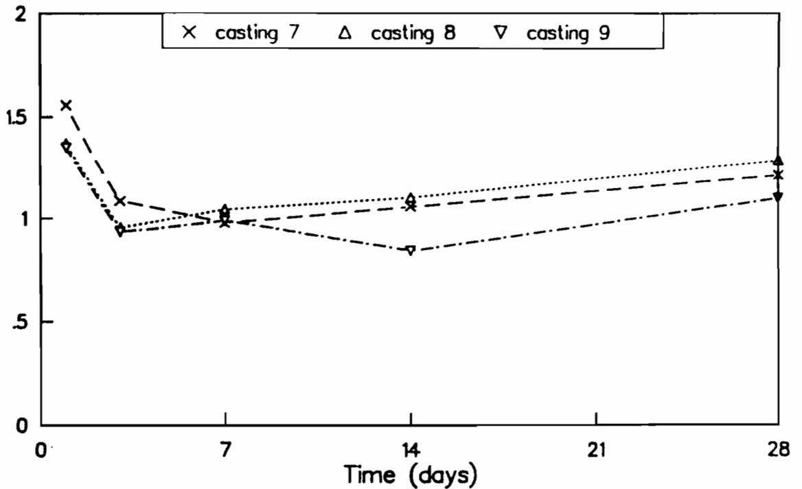
Fig C-18. Ratio of maturity method strengths to strengths of outdoor-cured cylinders for castings 7, 8, and 9. Maturity curve based on wetroom-cured cylinders.
