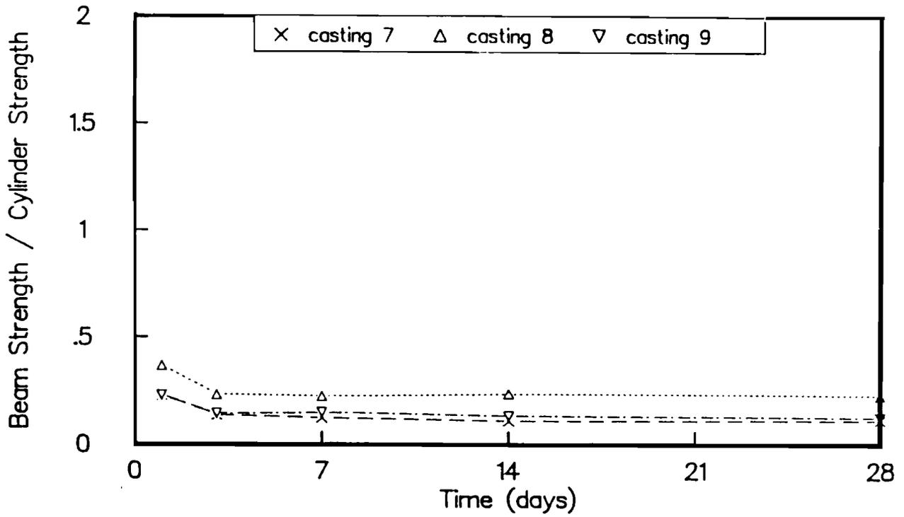
Fig C-3. Ratio of flexural strengths of wetroom-cured beams to strengths of wetroom-cured cylinders for castings 7, 8, and 9.
