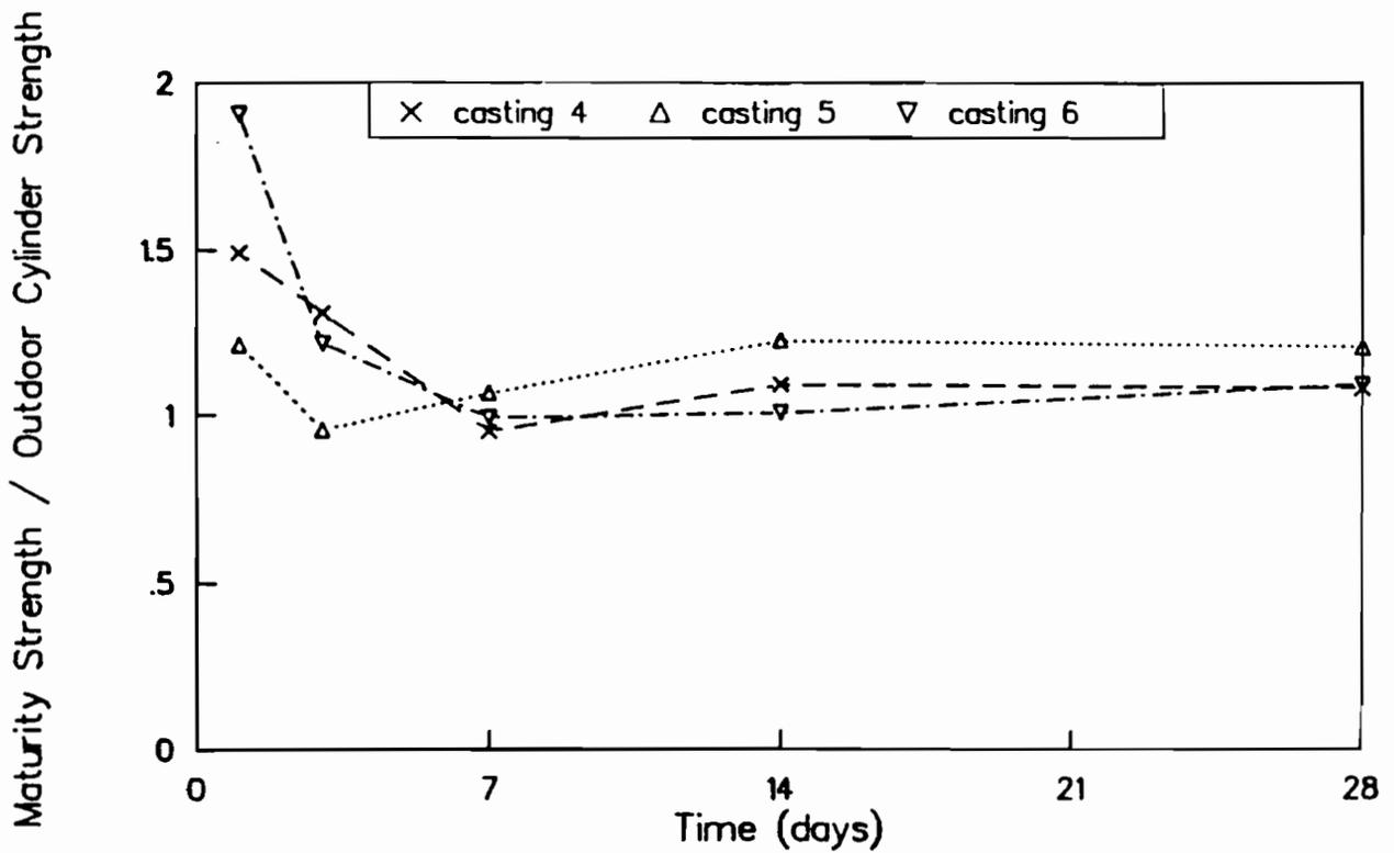
Fig B-18. Ratio of maturity method strengths to strengths of outdoor-cured cylinders for castings 4, 5, and 6. Maturity curve based on wetroom-cured cylinders.
