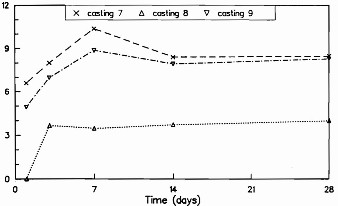
Fig C-36. Ratio of strengths of cores to flexural strengths of outdoor-cured beams for castings 7, 8, and 9.
