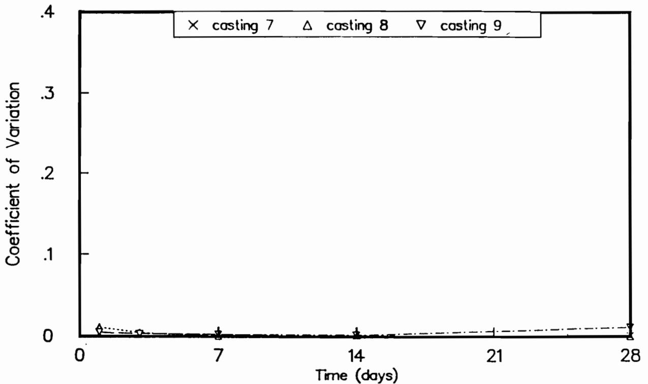
Fig C-56. Coefficient of variation of maturity method strengths for castings 7, 8, and 9. Maturity curve based on outdoor-cured beams.
