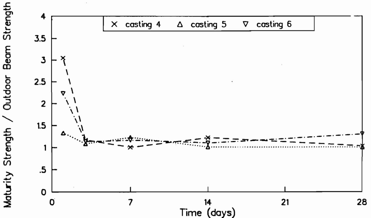
Fig B-43. Ratio of maturity method strengths to flexural strengths of outdoor-cured beams for castings 4, 5, and 6. Maturity curve based on wetroom-cured beams.
