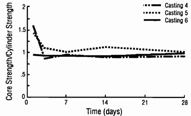
**Fig 5-18. Ratio of strength of cores drilled from slabs to strength of wetroom-cured cylinders for castings 4, 5, and 6.**
