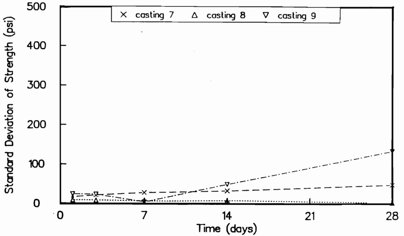
Fig C-65. Standard deviation of maturity method strengths for castings 7, 8, and 9. Maturity curve based on outdoor-cured cylinders.
