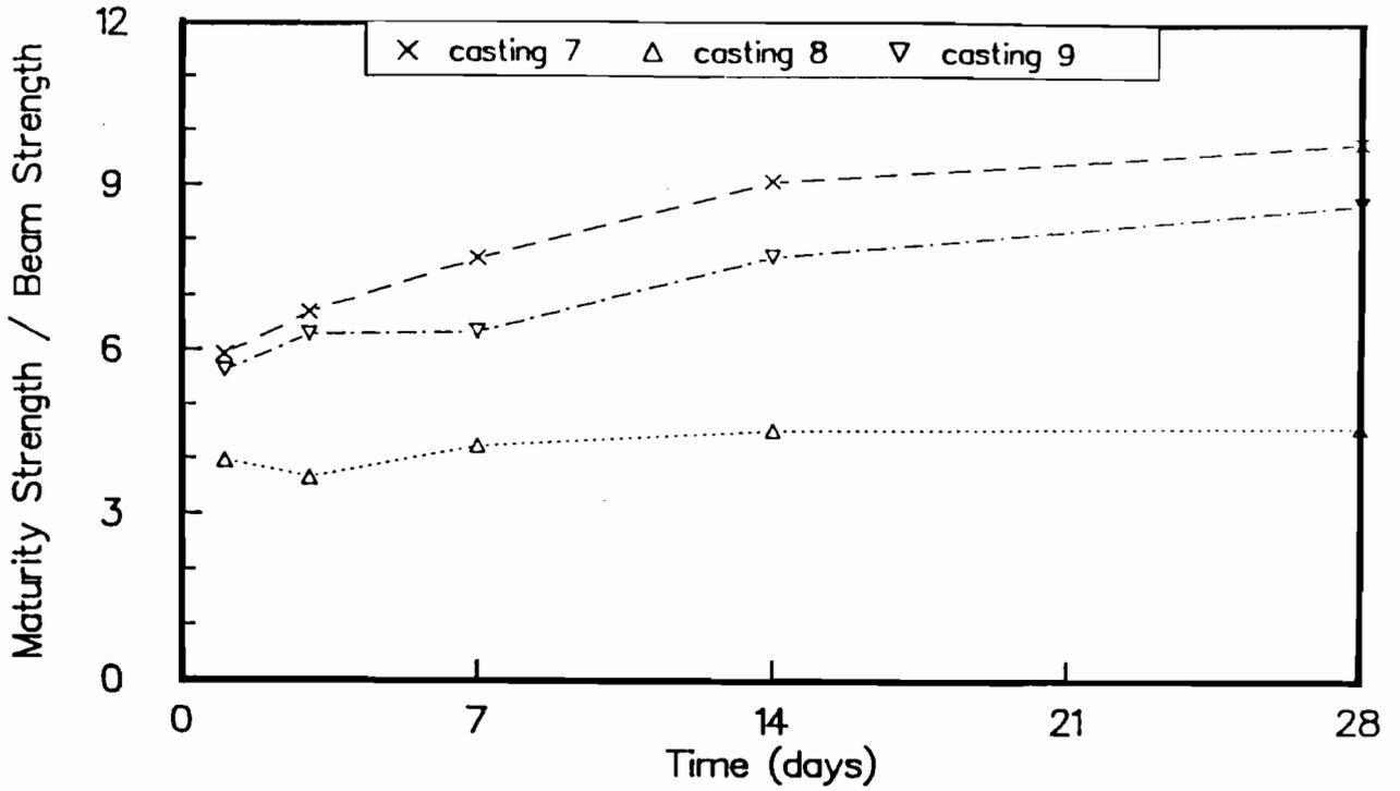
Fig C-29. Ratio of maturity method strengths to flexural strengths of wetroom-cured beams for castings 7, 8, and 9. Maturity curve based on wetroom-cured cylinders.
