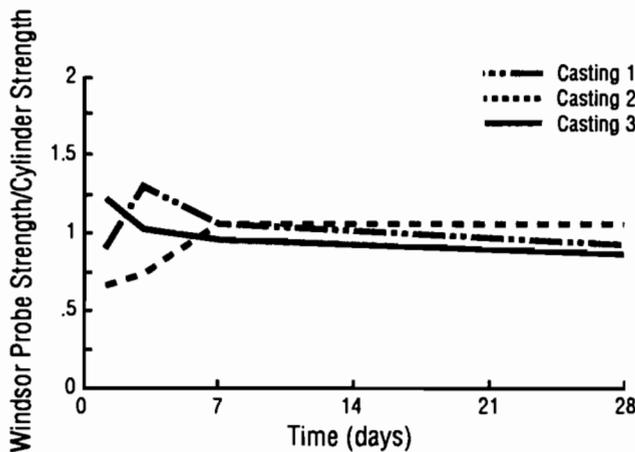
Fig 5-12. Ratio of Windsor probe penetration resistance strength to strength of wetroom-cured cylinders for castings 1, 2, and 3.
