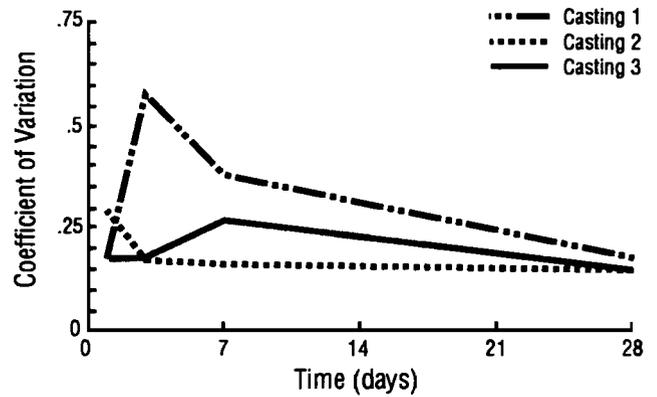
**Fig 5-8. Coefficient of variation of rebound number strengths for castings 1, 2, and 3.**
