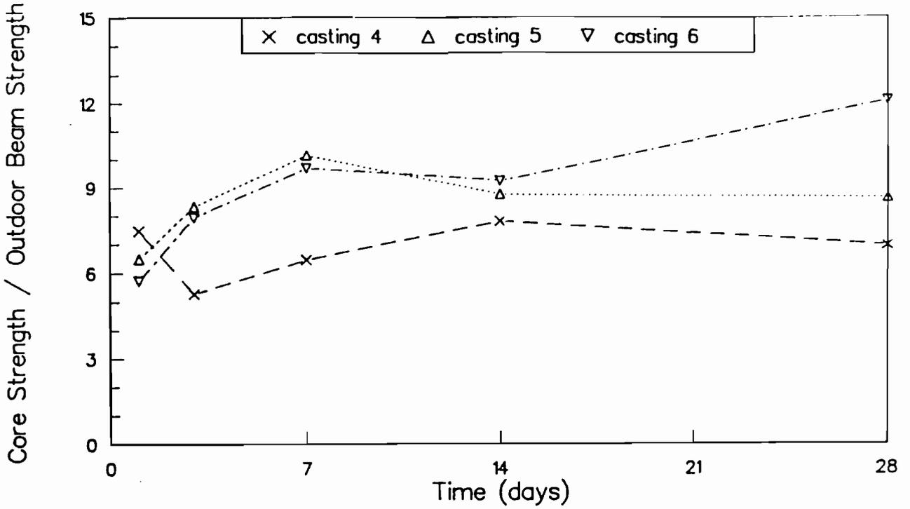
Fig B-36. Ratio of strengths of cores to flexural strengths of outdoor-cured beams for castings 4, 5, and 6.
