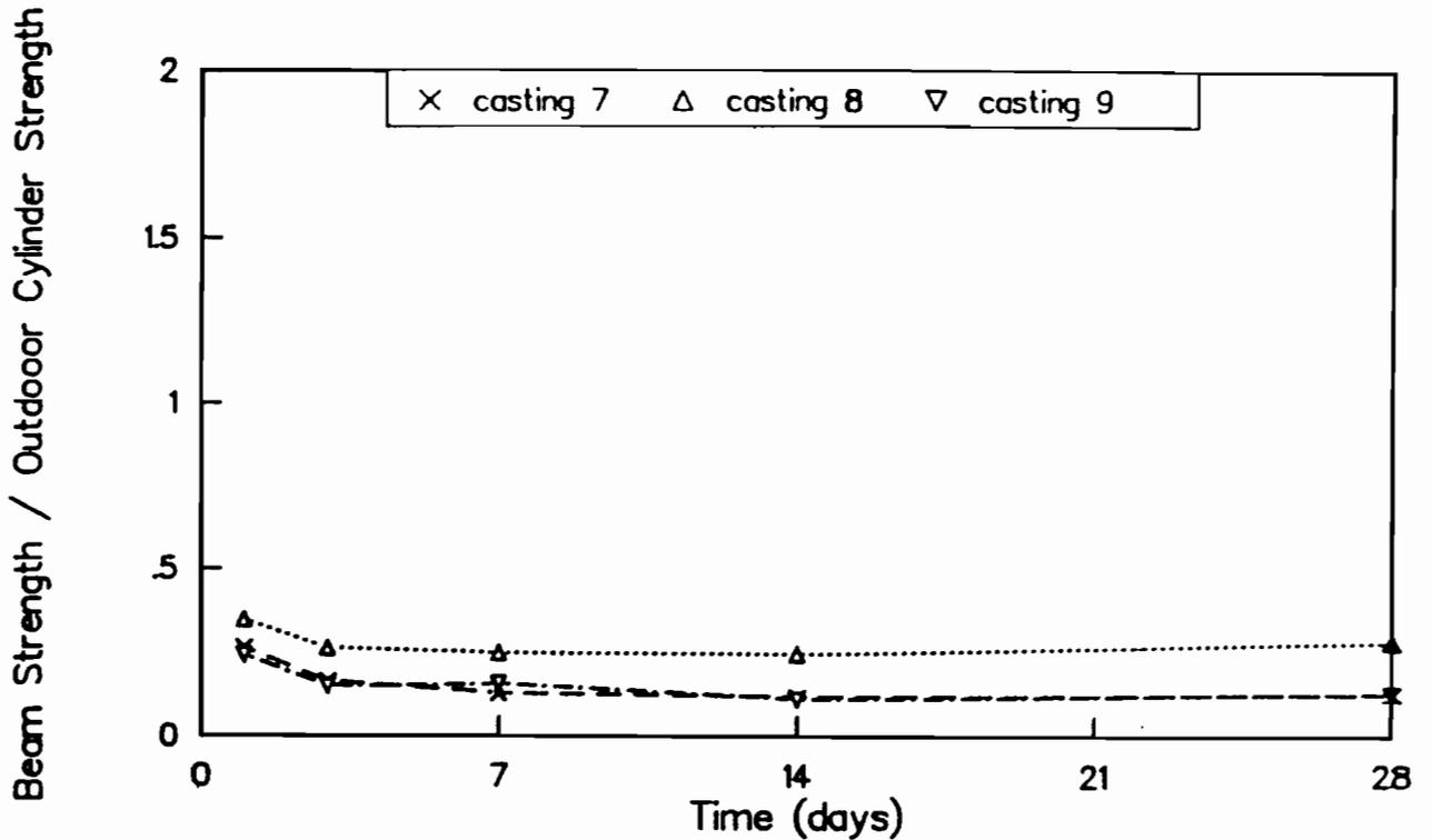
Fig C-14. Ratio of flexural strengths of wetroom-cured beams to strengths of outdoor-cured cylinders for castings 7, 8, and 9.
