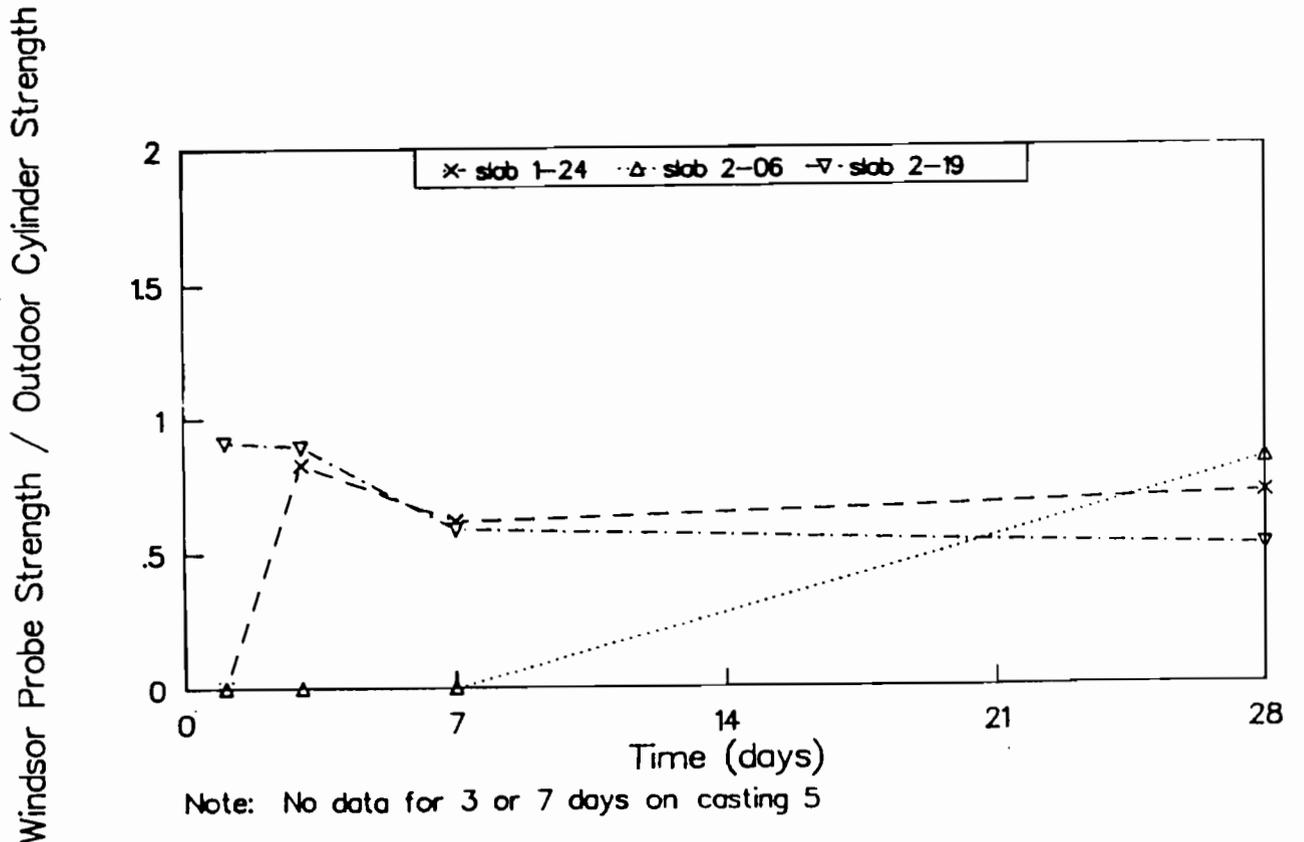
Fig B-17. Ratio of Windsor probe penetration resistance strengths to strengths of outdoor-cured cylinders for castings 4, 5, and 6.
