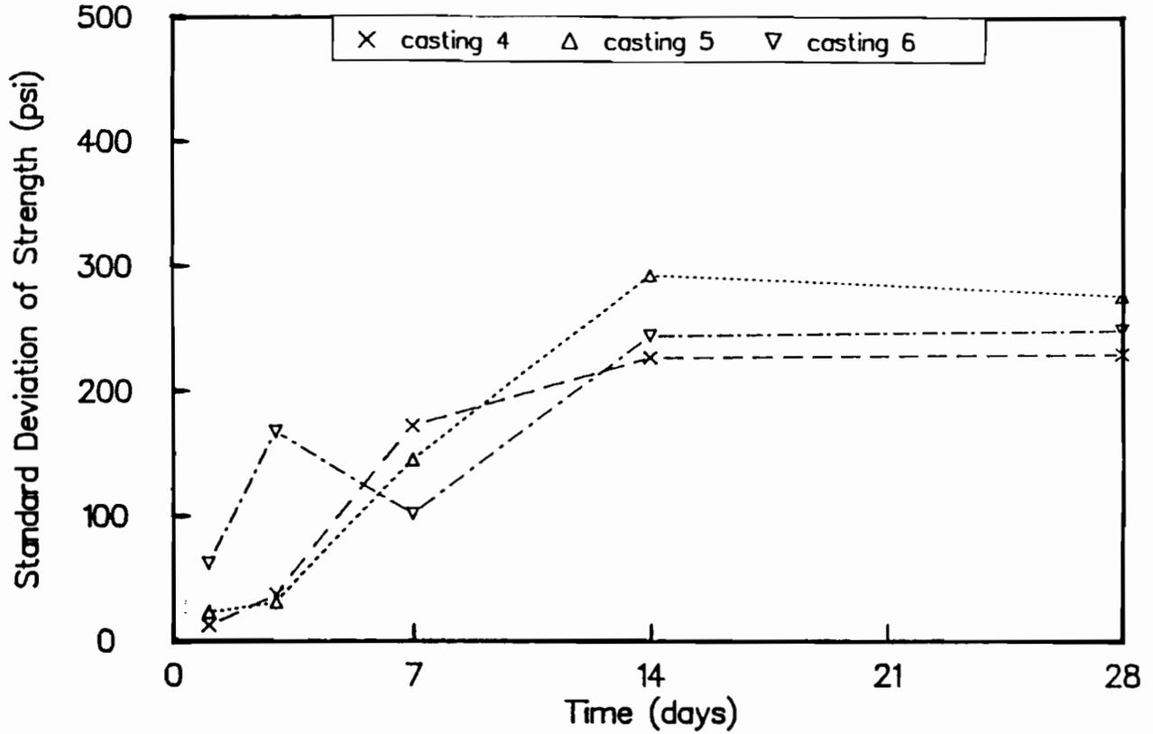
Fig B-58. Standard deviation of outdoor-cured cylinder strengths for castings 4, 5, and 6.
