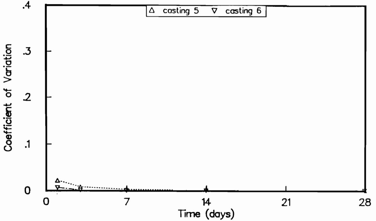
Fig B-52. Coefficient of variation of maturity method strengths for castings 5 and 6. Maturity curve based on wetroom-cured cylinders.
