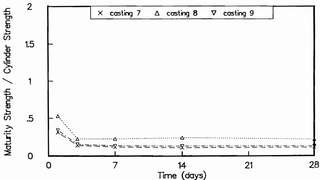
Fig C-10. Ratio of maturity method strengths to strengths of wetroom-cured cylinders for castings 7, 8, and 9. Maturity curve based on wetroom-cured beams.
