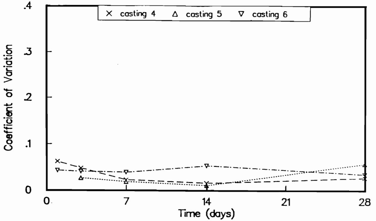
Fig B-48. Coefficient of variation of flexural strength of wetroom-cured beams for castings 4, 5, and 6.
