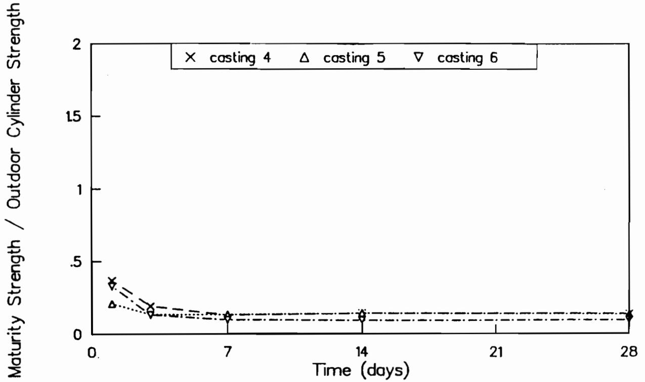
Fig B-22. Ratio of maturity method strengths to strengths of outdoor-cured cylinders for castings 4, 5, and 6. Maturity curve based on outdoor-cured beams.
