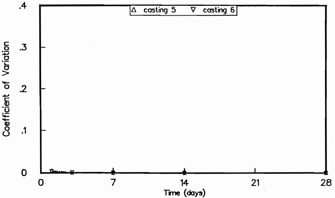
Fig B-55. Coefficient of variation of maturity method strengths for castings 5 and 6. Maturity curve based on wetroom-cured beams.
