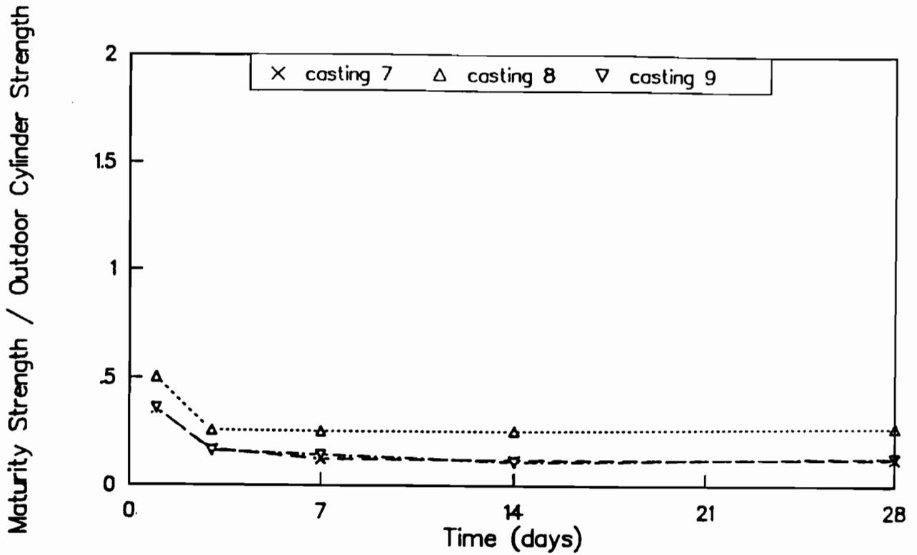
Fig C-21. Ratio of maturity method strengths to strengths of outdoor-cured cylinders for castings 7, 8, and 9. Maturity curve based on wetroom-cured beams.
