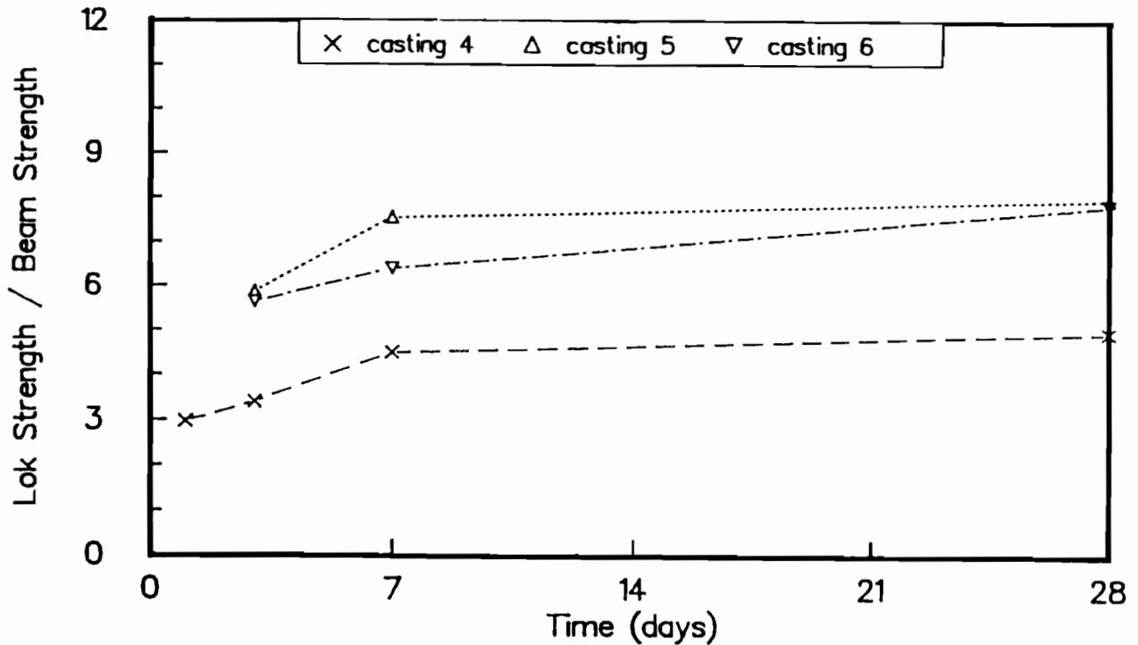
Fig B-27. Ratio of "Lok-Test" pullout strengths to flexural strengths of wetroom-cured beams for castings 4, 5, and 6.
