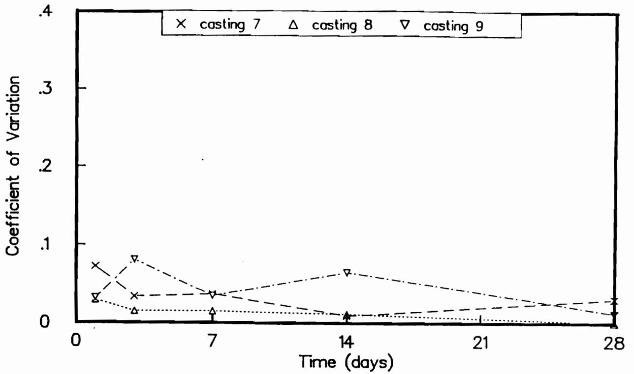
Fig C-49. Coefficient of variation of flexural strength of outdoor-cured beams for castings 7, 8, and 9.
