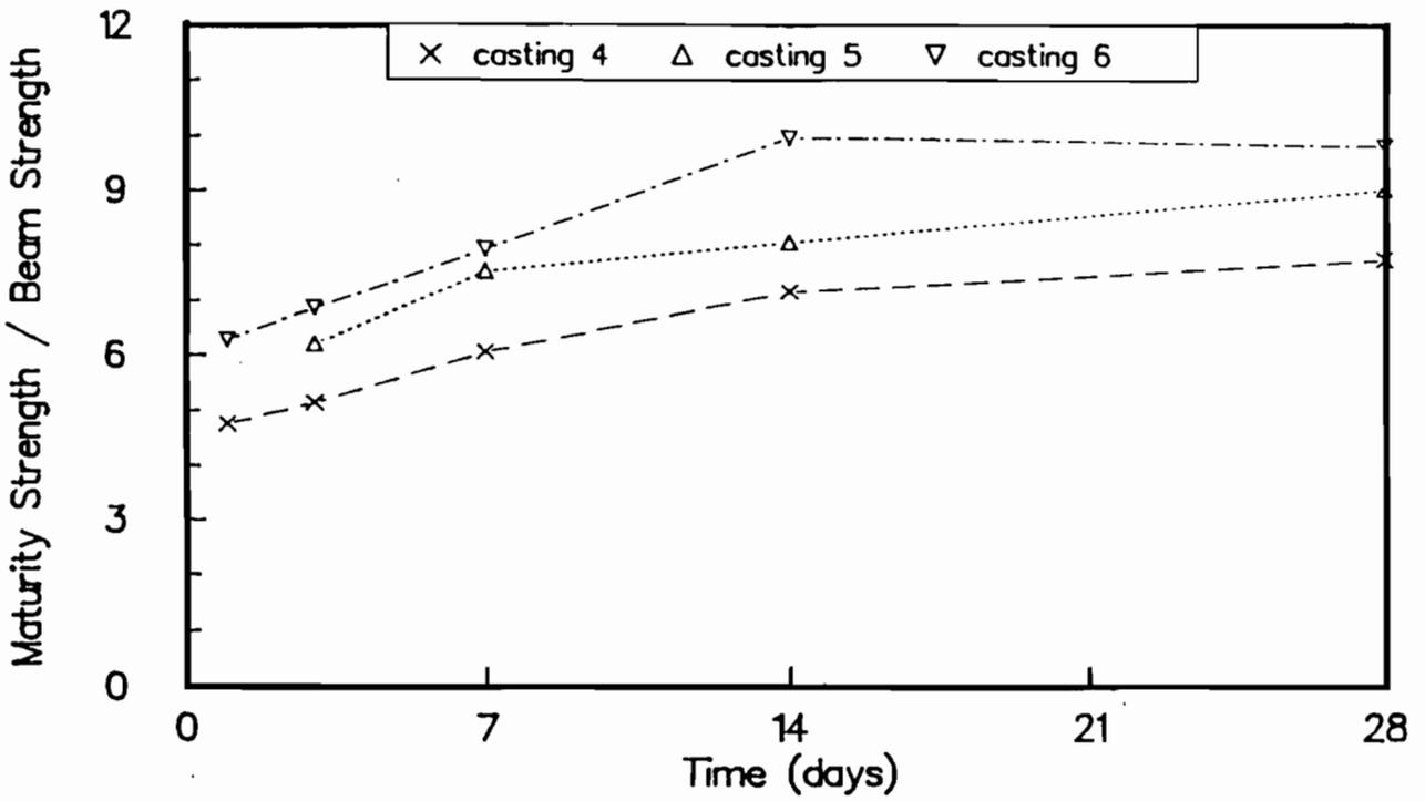
Fig B-29. Ratio of maturity method strengths to flexural strengths of wetroom-cured beams for castings 4, 5, and 6. Maturity curve based on wetroom-cured cylinders.
