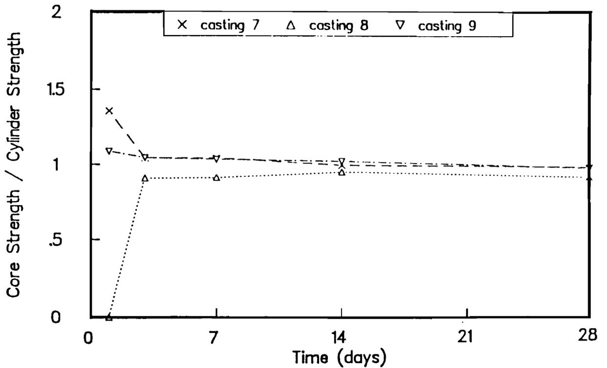
Fig C-2. Ratio of strengths of cores to strengths of wetroom-cured cylinders for castings 7, 8, and 9.
