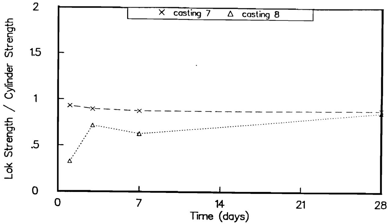
Fig C-5. Ratio of "Lok-Test" pullout strengths to strengths of wetroom-cured cylinders for castings 7, 8, and 9.
