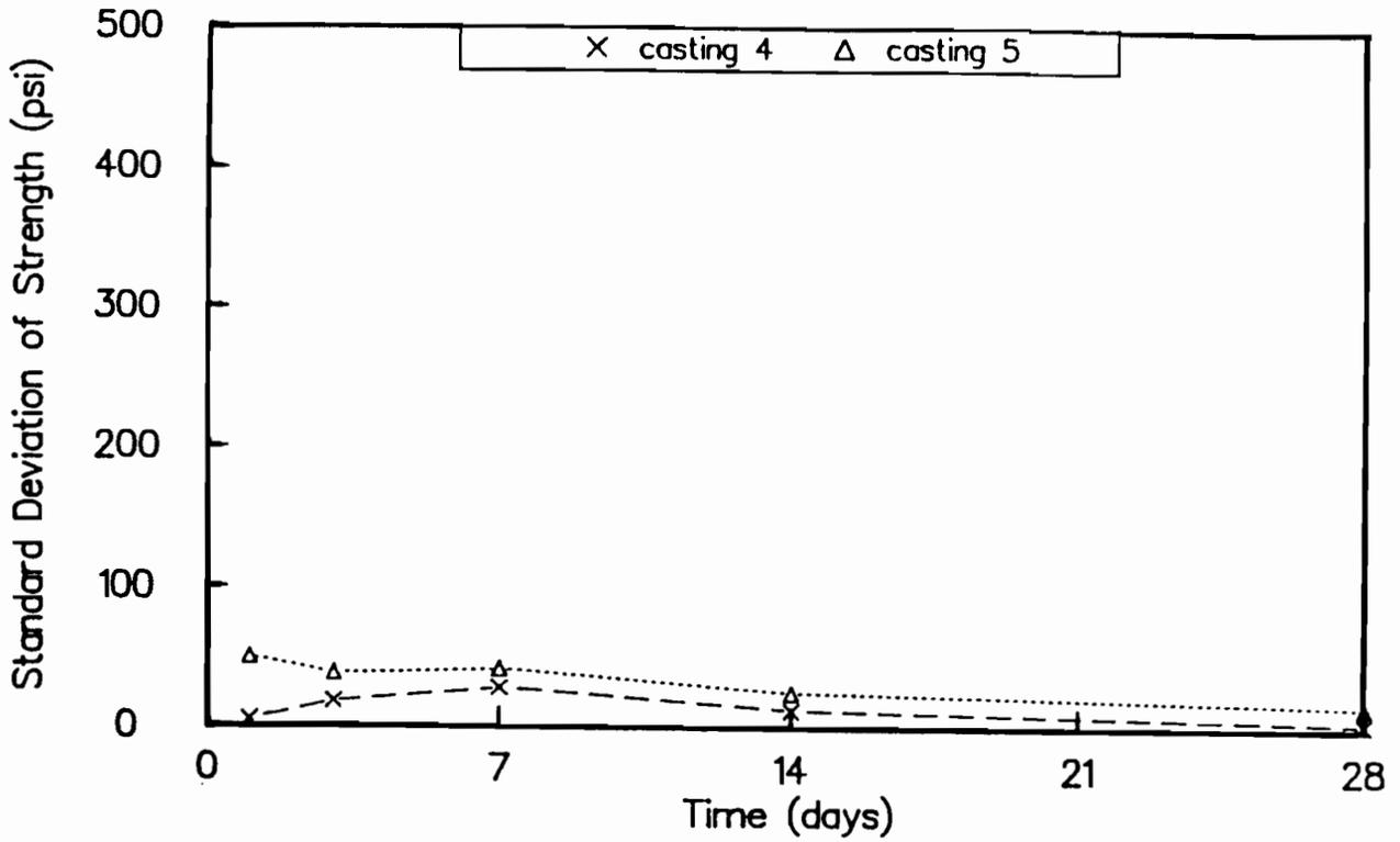
Fig B-66. Standard deviation of maturity method strengths for castings 4 and 5. Maturity curve based on cores drilled from slabs.
