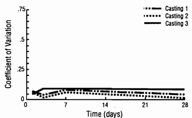
Fig 5-15. Coefficient of variation of wetroom-cured flexural beam strengths for castings 1, 2, and 3.
