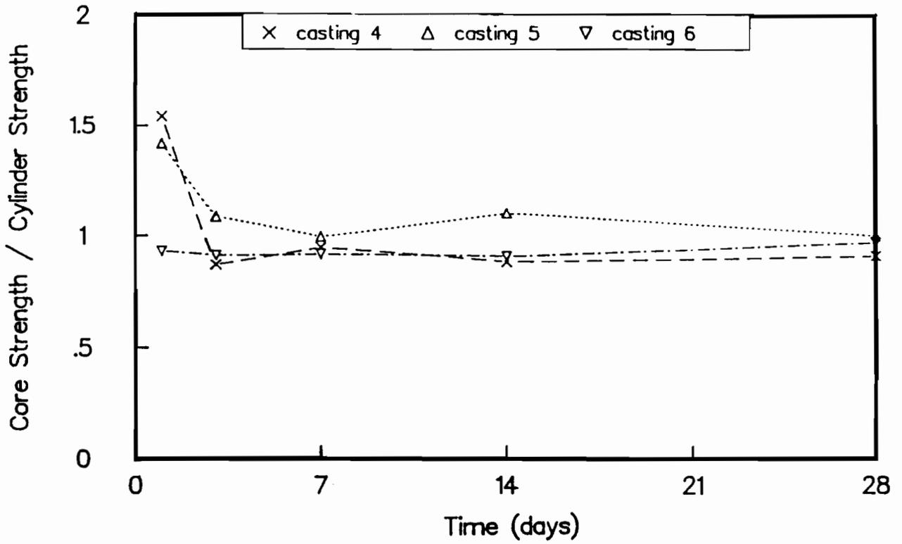
Fig B-2. Ratio of strengths of cores to strengths of wetroom-cured cylinders for castings 4, 5, and 6.
