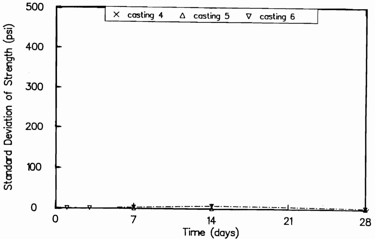
Fig B-59. Standard deviation of cores drilled from slabs for castings 4, 5, and 6.
