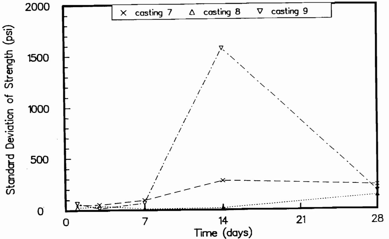
Fig C-58. Standard deviation of outdoor-cured cylinder strengths for castings 7, 8, and 9.
