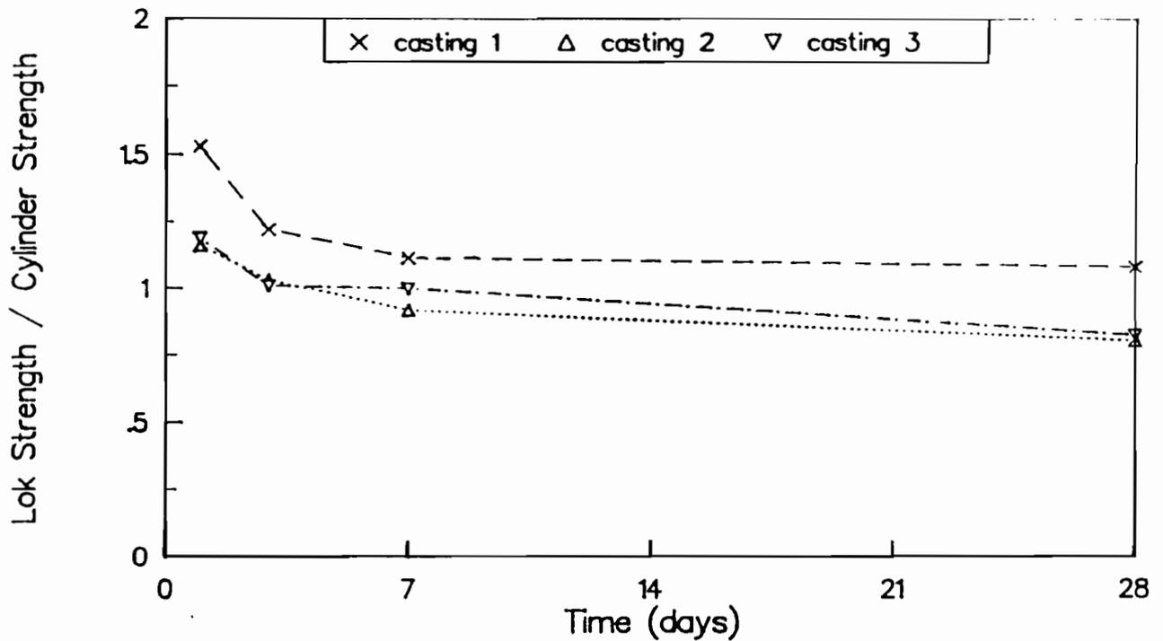
Fig A-3. Ratio of "Lok-Test" pullout strengths to strengths of wetroom-cured cylinders for castings 1, 2, and 3.
