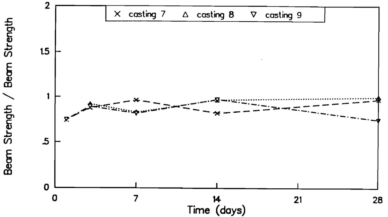
Fig C-26. Ratio of flexural strengths of outdoor-cured beams to flexural strengths of wetroom-cured beams for castings 7, 8, and 9.
