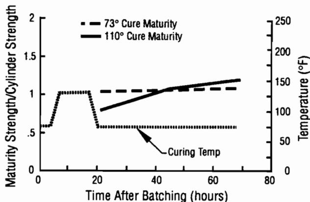
**Fig 5-37. Ratio of maturity method strength to cylinder strength for casting 11.**
