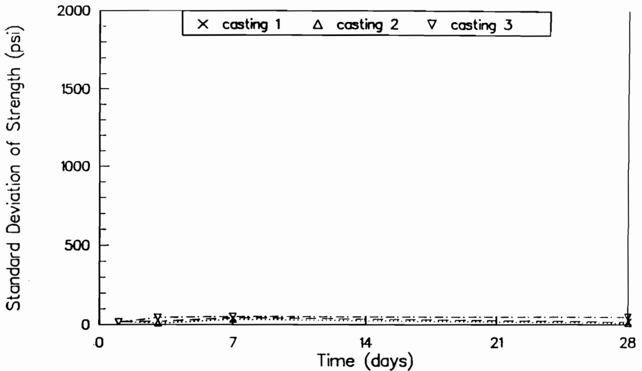
Fig A-21. Standard deviation of flexural strength of wetroom-cured beams for castings 1, 2, and 3.
