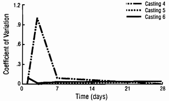
Fig 5-28. Coefficient of variation of Windsor probe penetration resistance strength for castings 4, 5, and 6.
