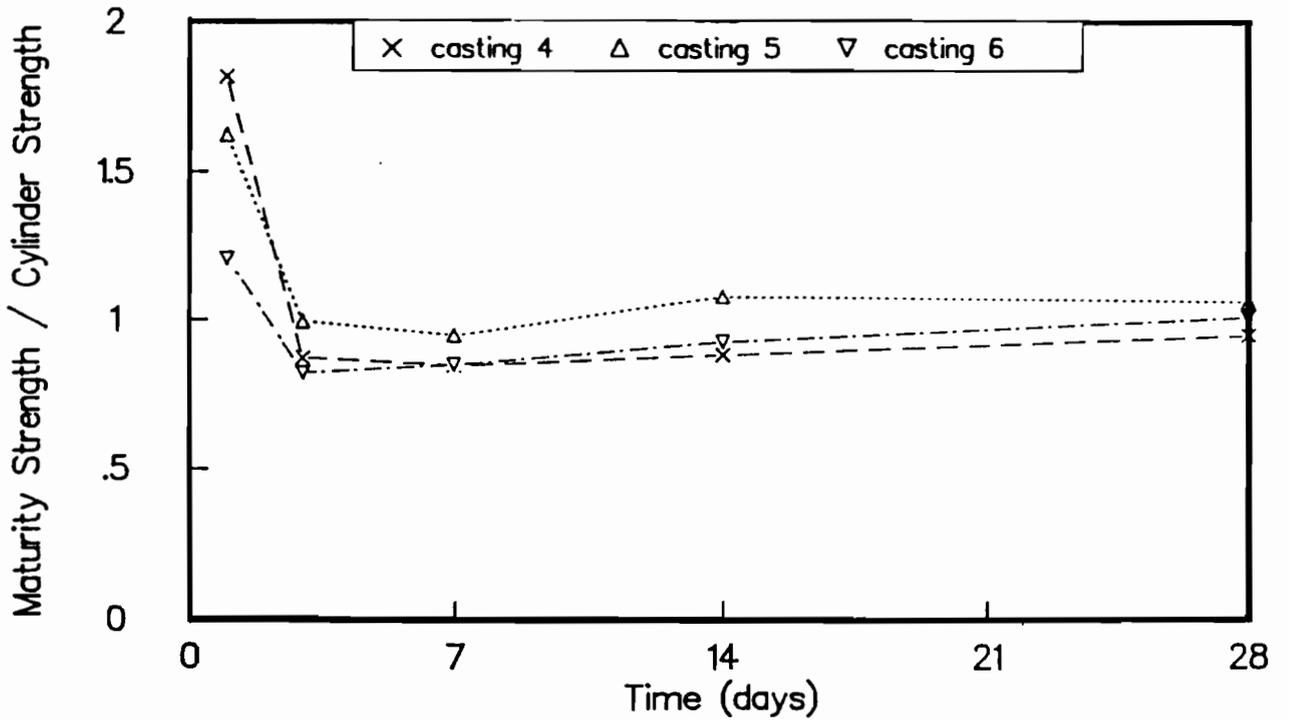
Fig B-9. Ratio of maturity method strengths to strengths of wetroom-cured cylinders for castings 4, 5, and 6. Maturity curve based on cores drilled from slabs.
