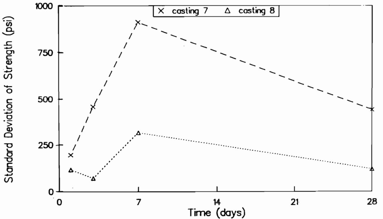
Fig C-62. Standard deviation of "Lok-Test" pullout strengths for castings 7 and 8.
