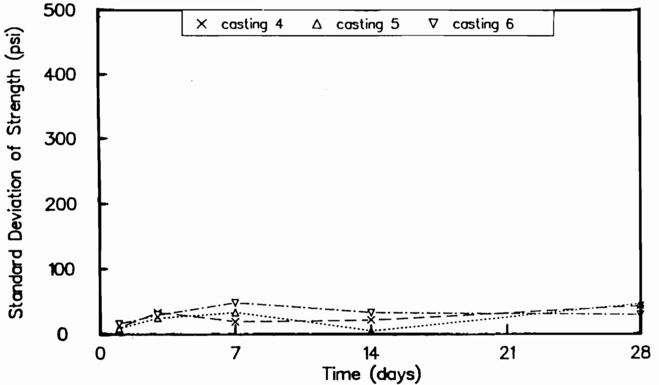
Fig B-64. Standard deviation of maturity method strengths for castings 4, 5, and 6. Maturity curve based on wetroom-cured cylinders.
