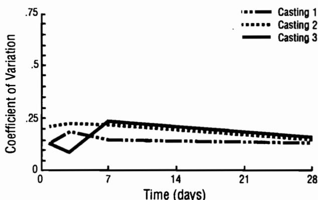
Fig 5-4. Coefficient of variation of "Lok-Test" pullout strengths for castings 1, 2, and 3.
