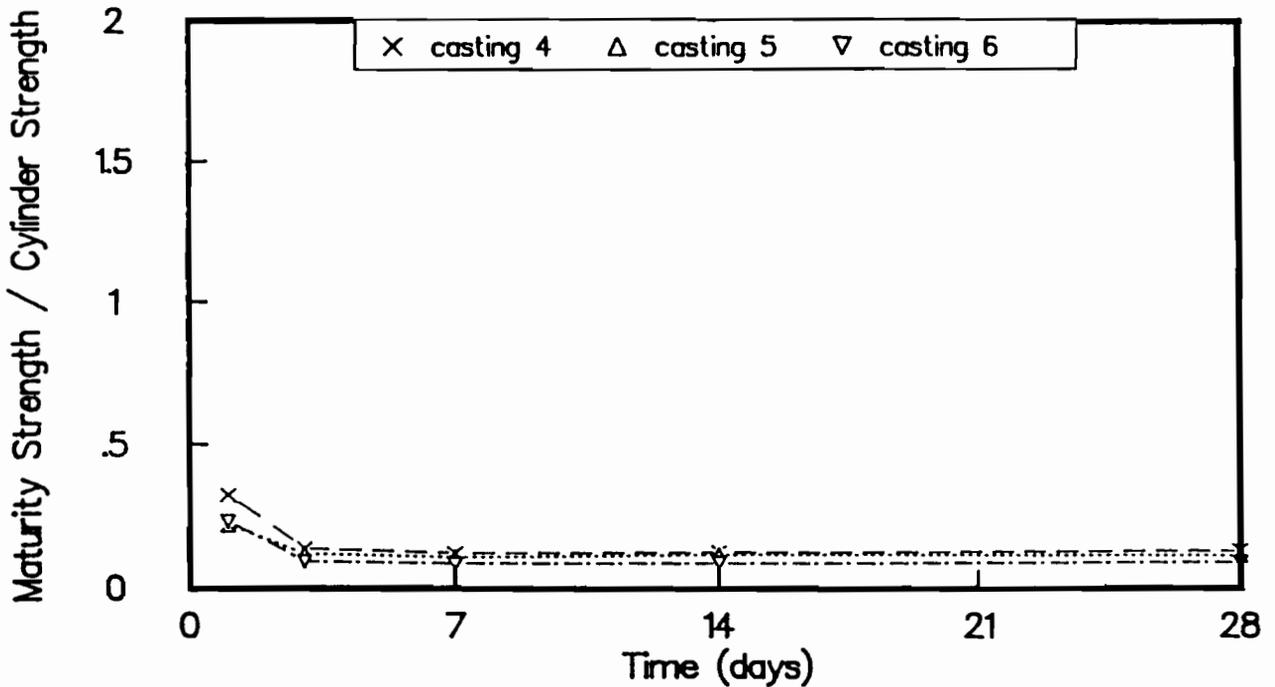
Fig B-11. Ratio of maturity method strengths to strengths of wetroom-cured cylinders for castings 4, 5, and 6. Maturity curve based on outdoor-cured beams.
