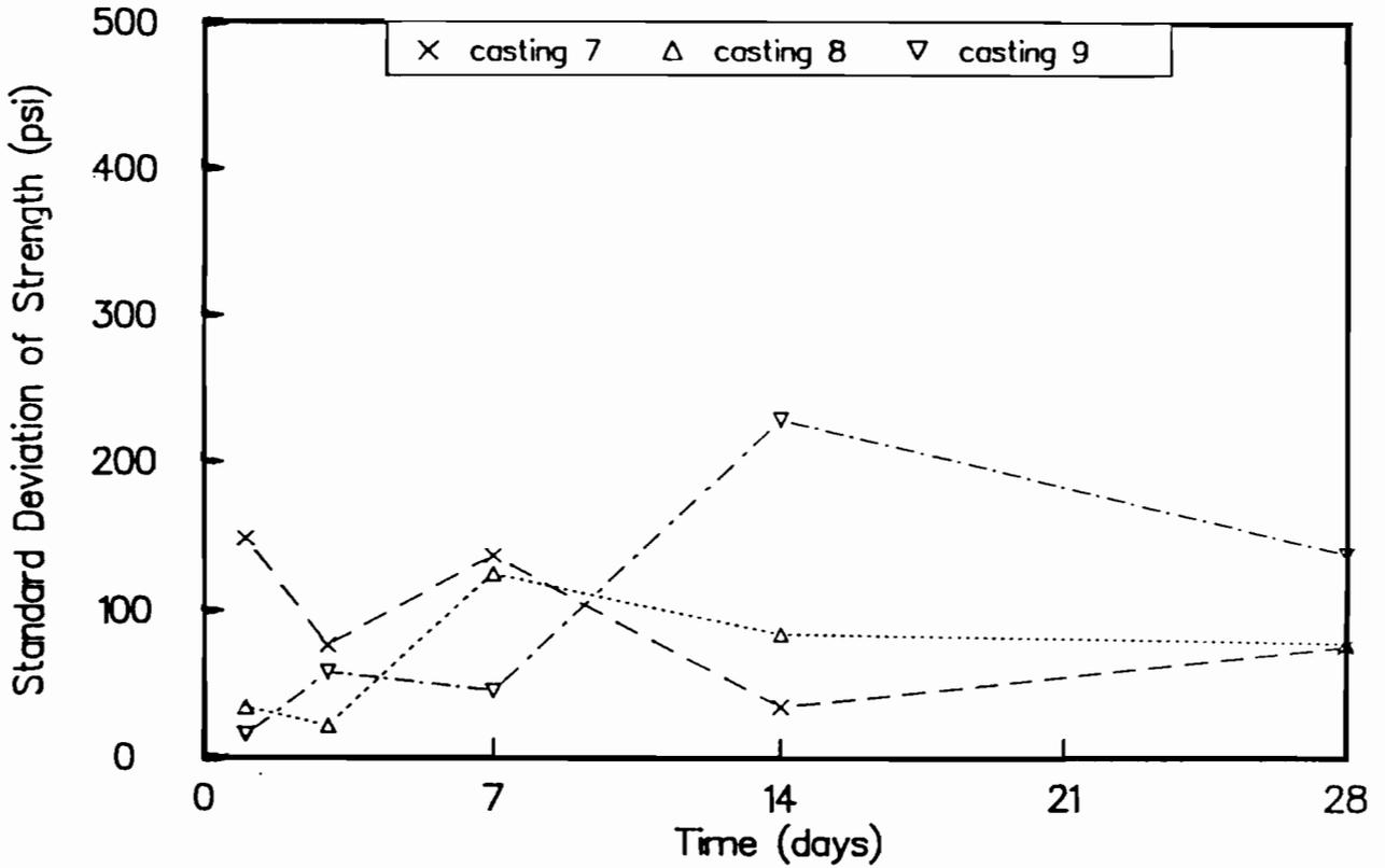
Fig C-57. Standard deviation of wetroom-cured cylinder strengths for castings 7, 8, and 9.
