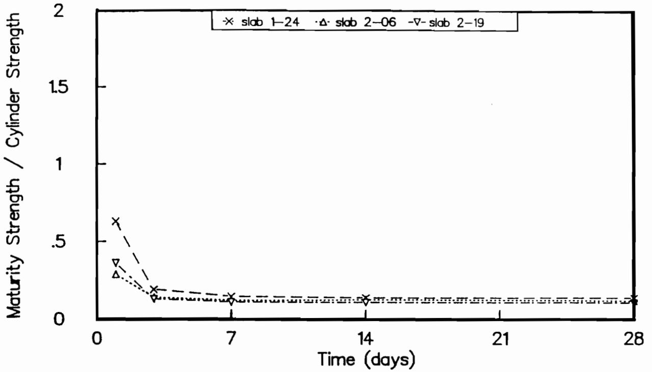
Fig B-10. Ratio of maturity method strengths to strengths of wetroom-cured cylinders for castings 4, 5, and 6. Maturity curve based on wetroom-cured beams.
