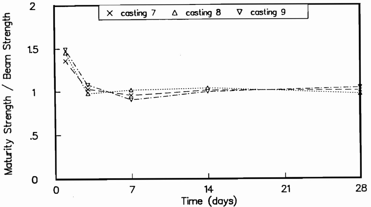
Fig C-32. Ratio of maturity method strengths to flexural strengths of wetroom-cured beams for castings 7, 8, and 9. Maturity curve based on wetroom-cured beams.
