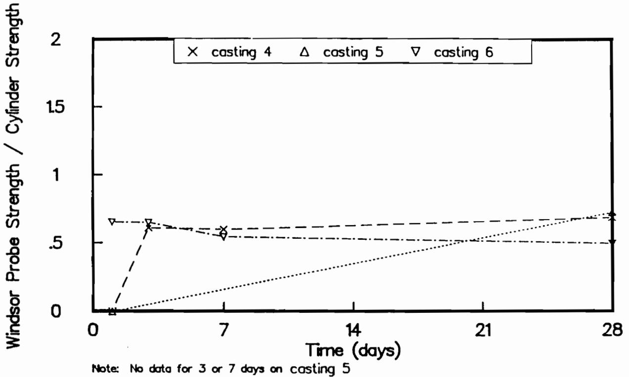
Fig B-6. Ratio of Windsor probe penetration resistance strengths to strengths of wetroom-cured cylinders for castings 4, 5, and 6.
