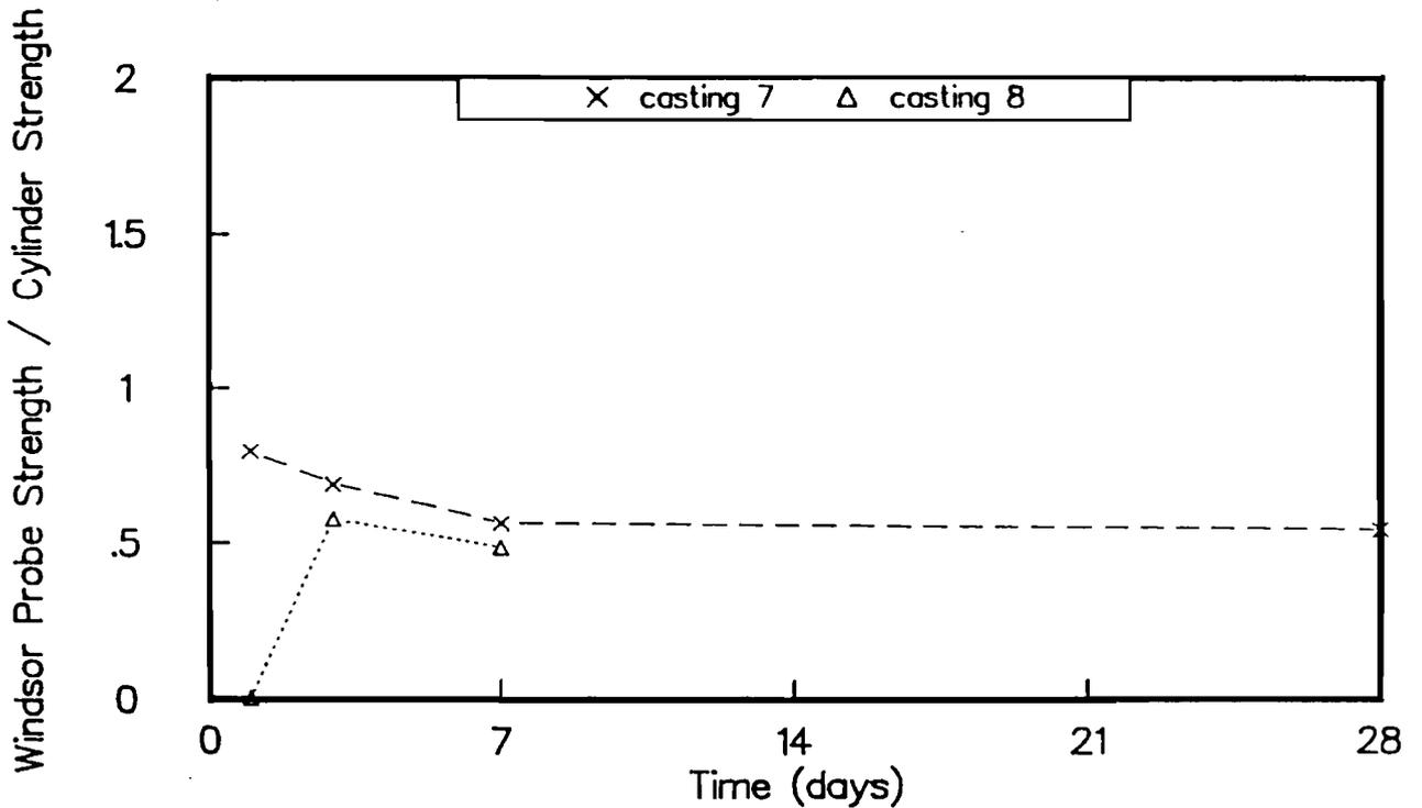
Fig C-6. Ratio of Windsor probe penetration resistance strengths to strengths of wetroom-cured cylinders for castings 7 and 8.
