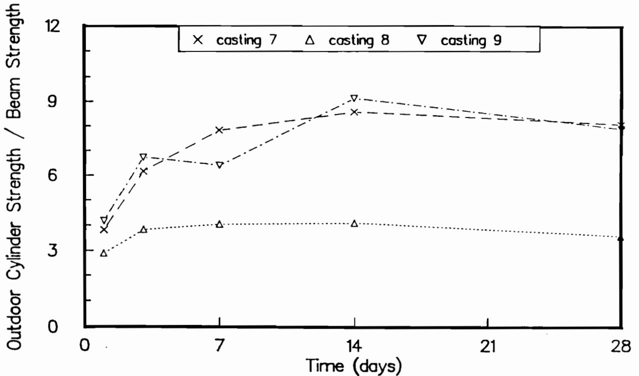
Fig C-24. Ratio of strengths of outdoor-cured cylinders to flexural strengths of wetroom-cured beams for castings 7, 8, and 9.
