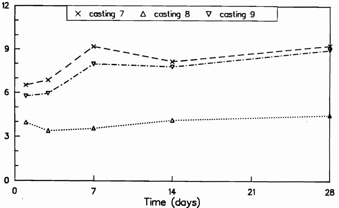
Fig C-40. Ratio of maturity method strengths to flexural strengths of outdoor-cured beams for castings 7, 8, and 9. Maturity curve based on wetroom-cured cylinders.
