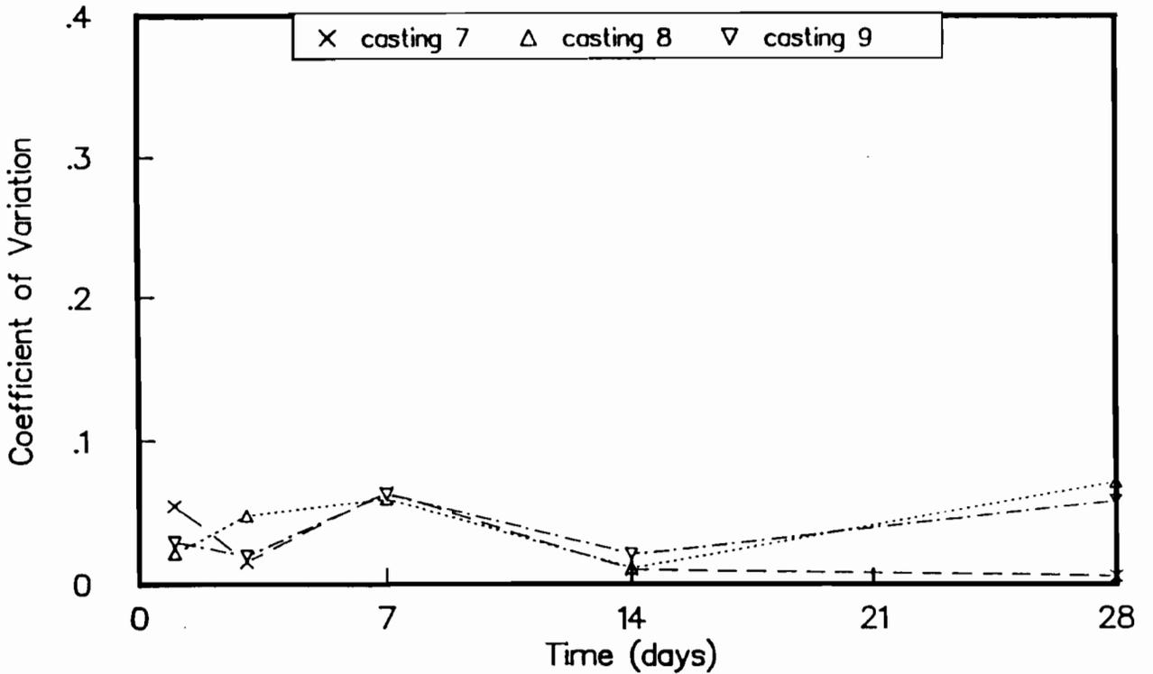
Fig C-48. Coefficient of variation of flexural strengths of wetroom-cured beams for castings 7, 8, and 9.
