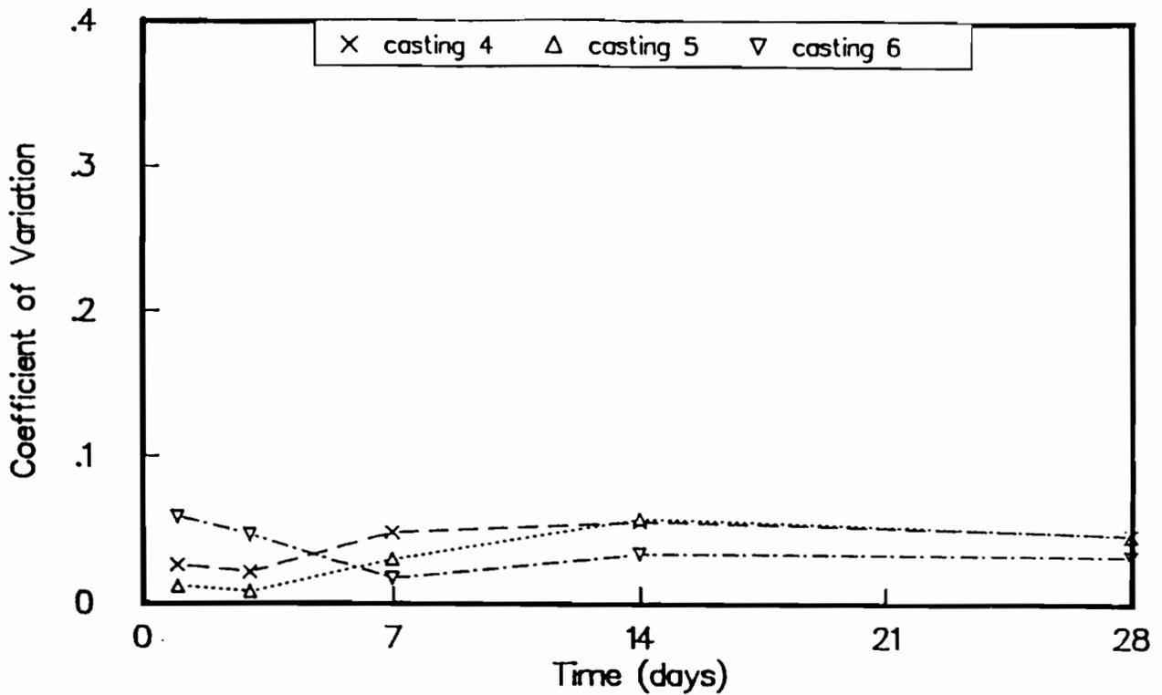
Fig B-46. Coefficient of variation of outdoor-cured cylinder strengths for castings 4, 5, and 6.
