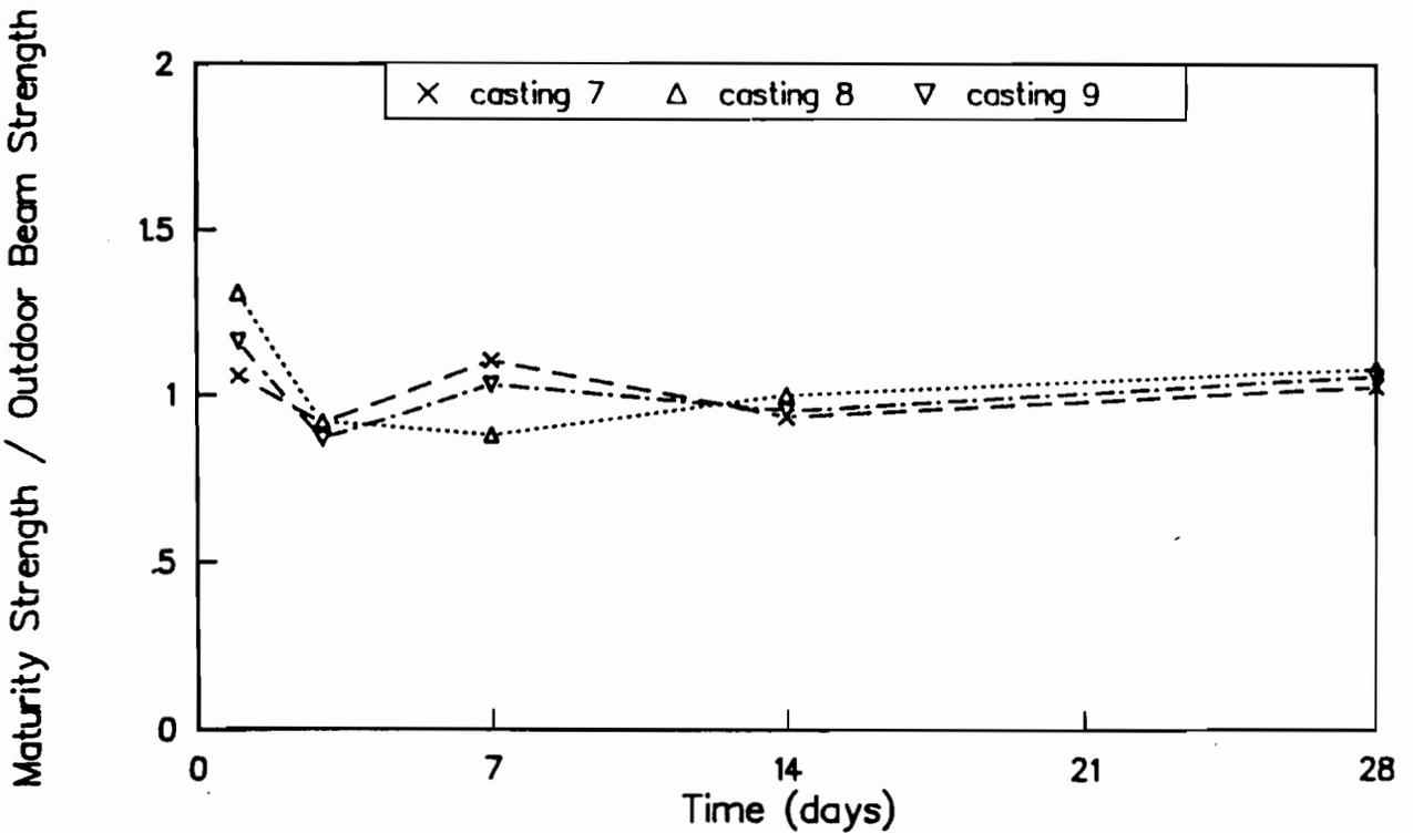
Fig C-44. Ratio of maturity method strengths to flexural strengths of outdoor-cured beams for castings 7, 8, and 9. Maturity curve based on outdoor-cured beams.
