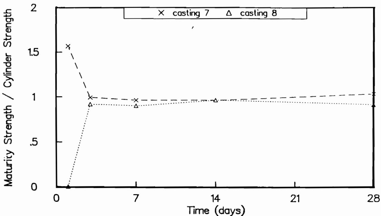
Fig C-9. Ratio of maturity method strengths to strengths of wetroom-cured cylinders for castings 7 and 8. Maturity curve based on cores drilled from slabs.
