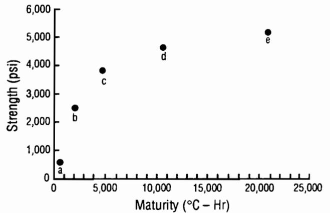
Fig 5-29. Relationship between maturity and strength of wetroom-cured cylinders for casting 4.
