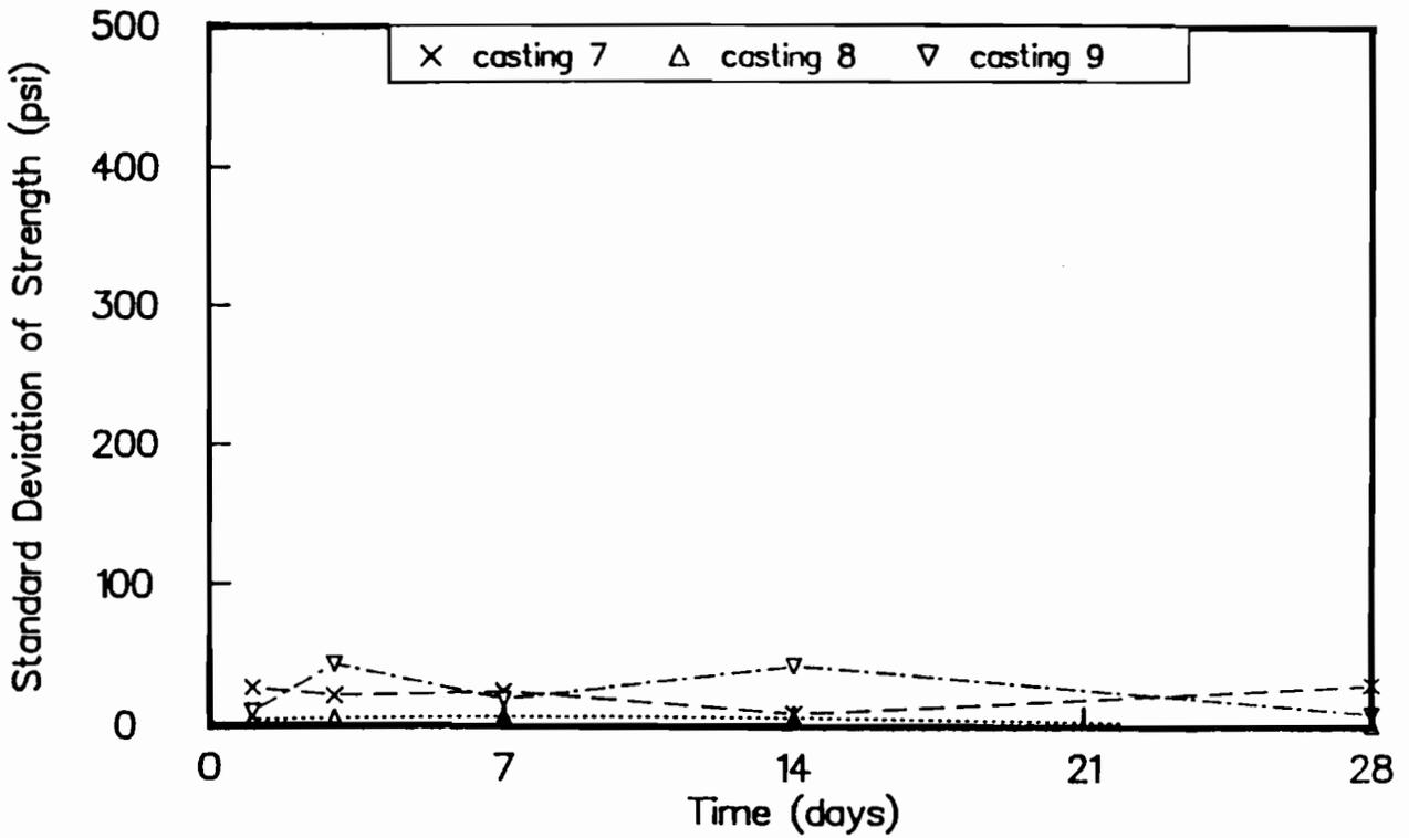
Fig C-64. Standard deviation of maturity method strengths for castings 7, 8, and 9. Maturity curve based on wetroom-cured cylinders.
