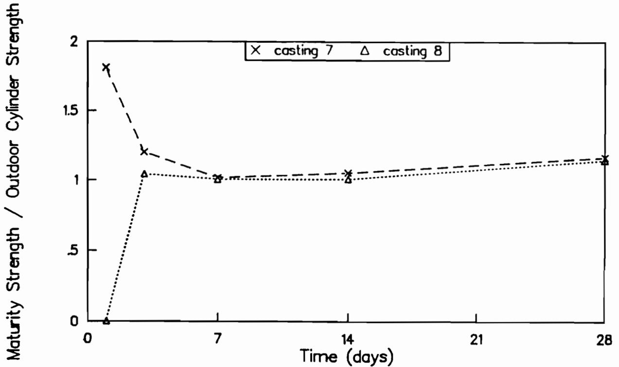
Fig C-20. Ratio of maturity method strengths to strengths of outdoor-cured cylinders for castings 7 and 8. Maturity curve based on cores drilled from slabs.
