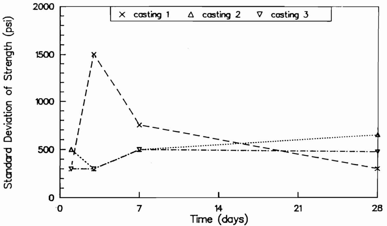
Fig A-25. Standard deviation of rebound number strengths for castings 1, 2, and 3.
