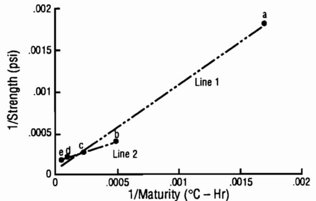
Fig 5-32. Relationship between maturity and strength for casting 4, used to determine  $S_u$ .
