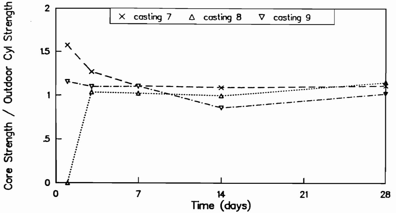
Fig C-13. Ratio of strengths of cores to strengths of outdoor-cured cylinders for castings 7, 8, and 9.
