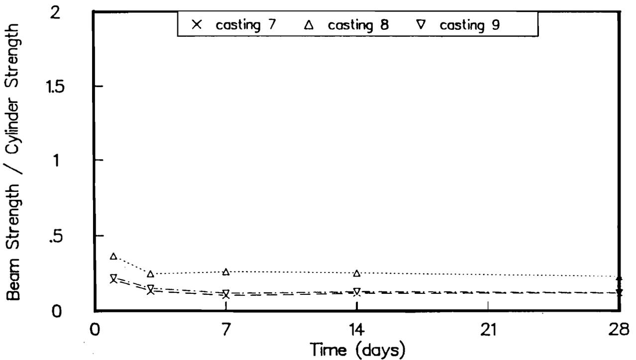
Fig C-4. Ratio of flexural strengths of outdoor-cured beams to strengths of wetroom-cured cylinders for castings 7, 8, and 9.
