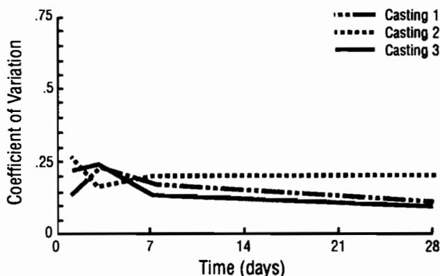
Fig 5-3. Coefficient of variation of "CAPO test" pullout strengths for castings 1, 2, and 3.
