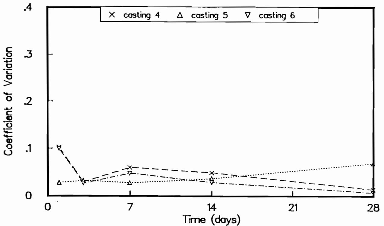
Fig B-47. Coefficient of variation of cores drilled from slabs for castings 4, 5, and 6.
