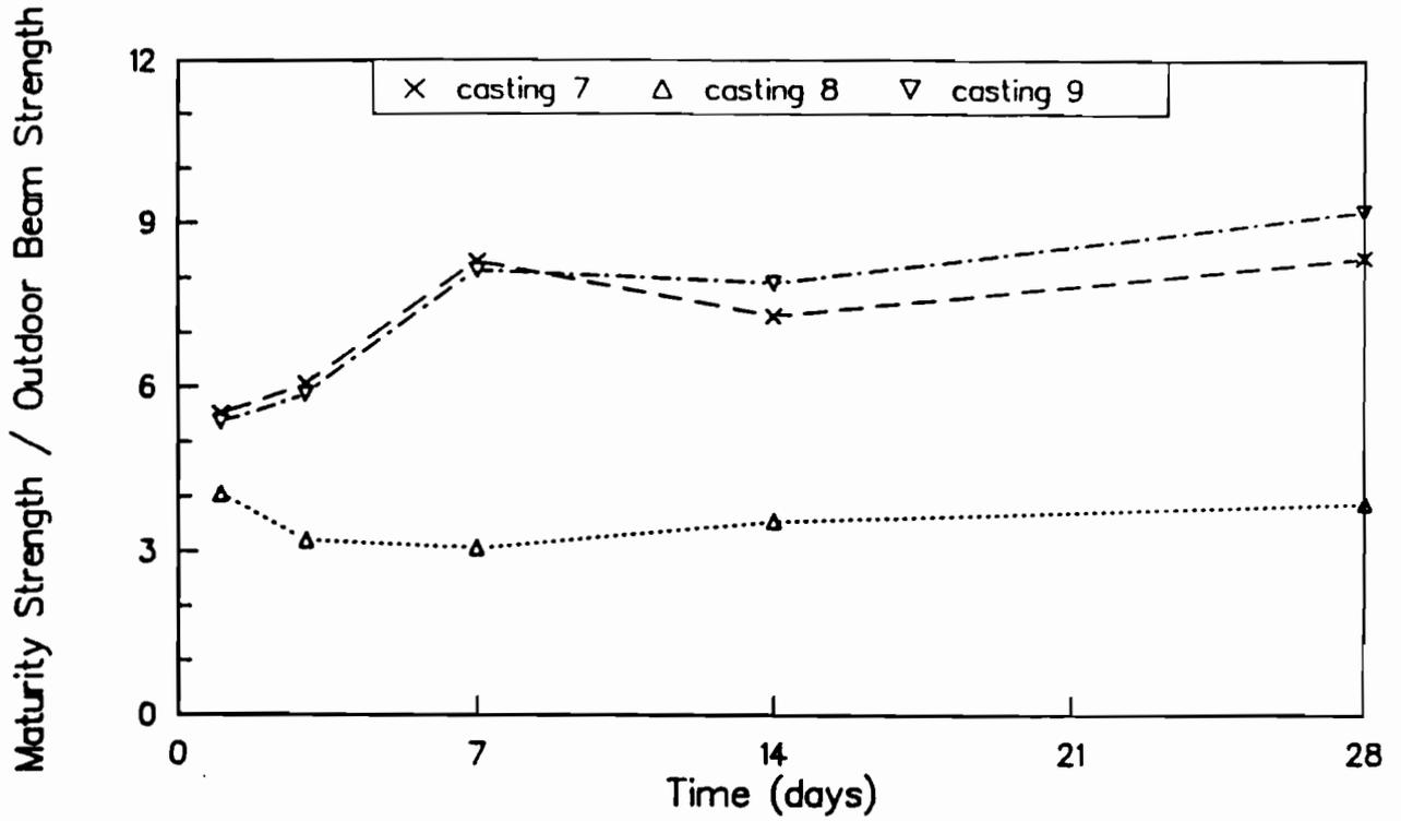
Fig C-41. Ratio of maturity method strengths to flexural strengths of outdoor-cured beams for castings 7, 8, and 9. Maturity curve based on outdoor-cured cylinders.
