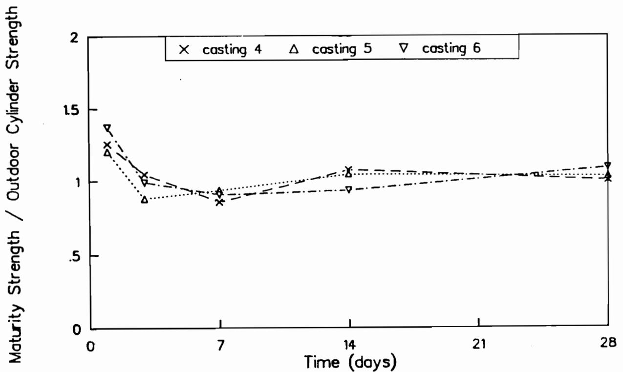
Fig B-19. Ratio of maturity method strengths to strengths of outdoor-cured cylinders for castings 4, 5, and 6. Maturity curve based on outdoor-cured cylinders.
