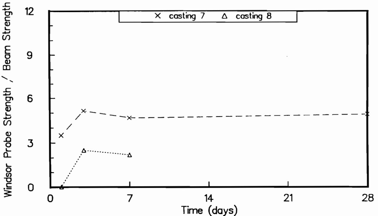
Fig C-28. Ratio of Windsor probe penetration resistance strengths to flexural strengths of wetroom-cured beams for castings 7 and 8.
