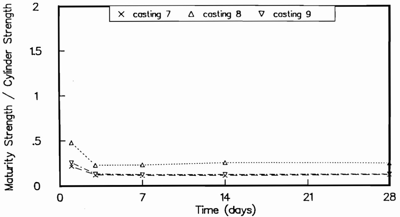
Fig C-11. Ratio of maturity method strengths to strengths of wetroom-cured cylinders for castings 7, 8, and 9. Maturity curve based on outdoor-cured beams.
