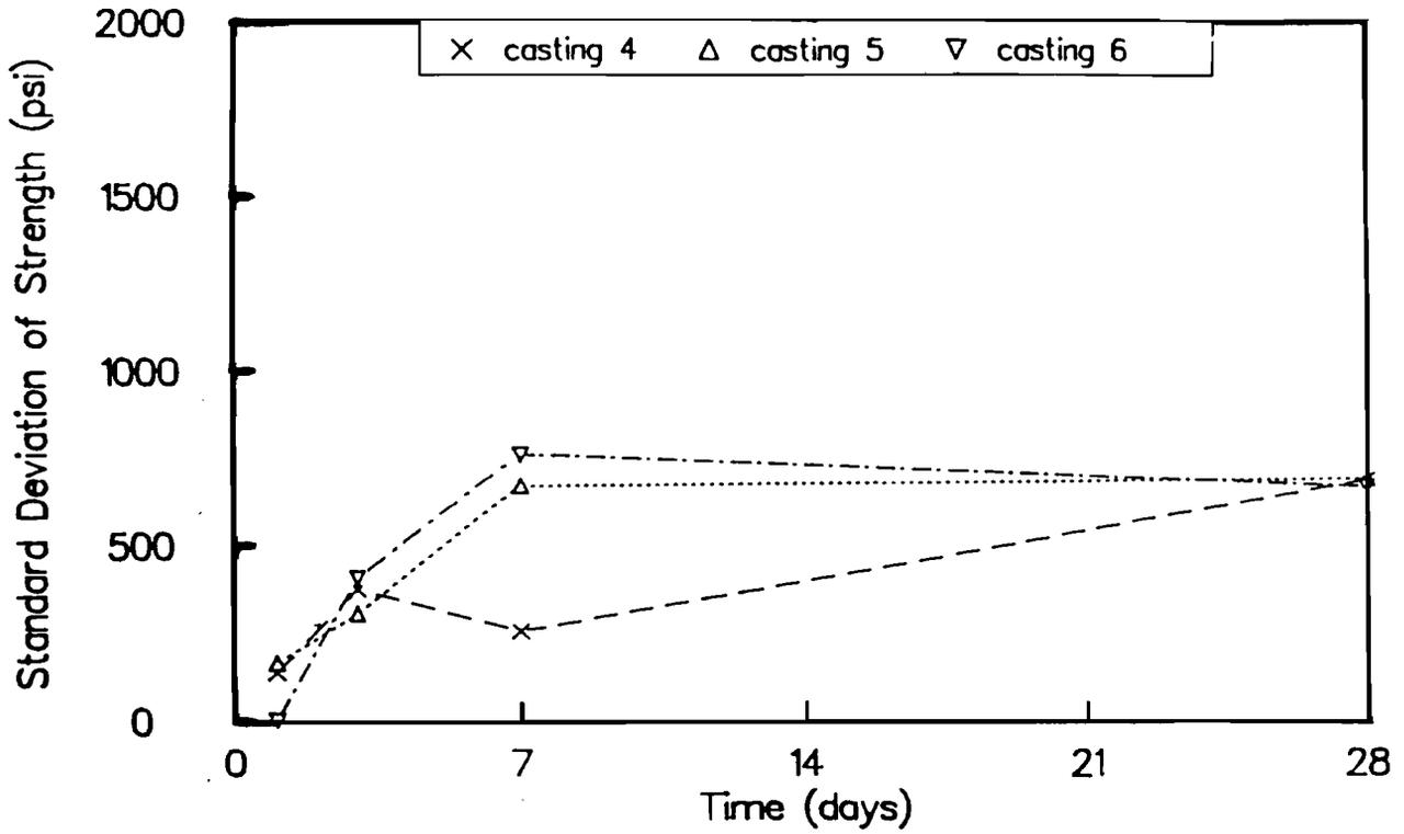
Fig B-62. Standard deviation of "Lok-Test" pullout strengths for castings 4, 5, and 6.
