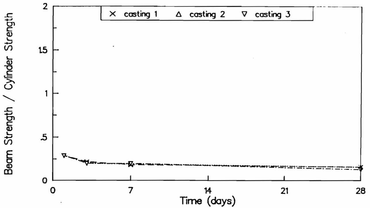
Fig A-1. Ratio of flexural strengths of wetroom-cured beams to strengths of wetroom-cured cylinders for castings 1, 2, and 3.
