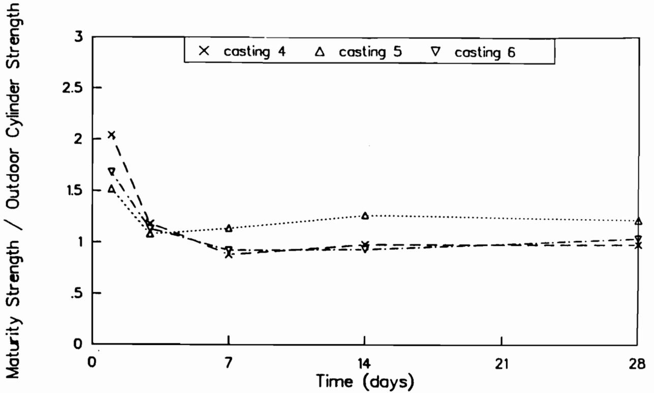
Fig B-20. Ratio of maturity method strengths to strengths of outdoor-cured cylinders for castings 4, 5, and 6. Maturity curve based on cores drilled from slabs.
