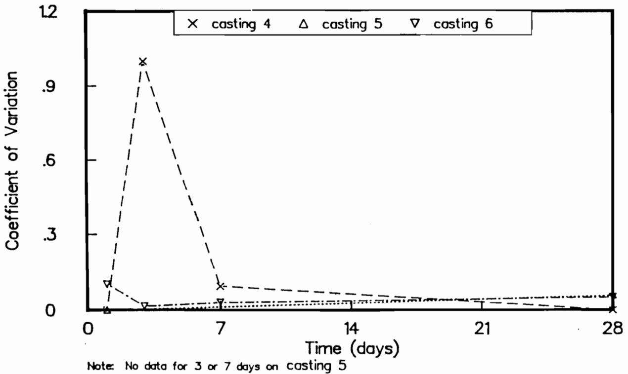
Fig B-51. Coefficient of variation of Windsor probe penetration resistance strengths for castings 4, 5, and 6.
