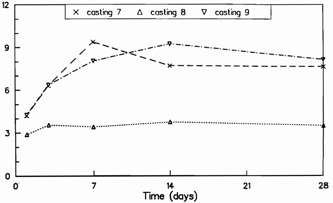
Fig C-35. Ratio of strengths of outdoor-cured cylinders to flexural strengths of outdoor-cured beams for castings 7, 8, and 9.
