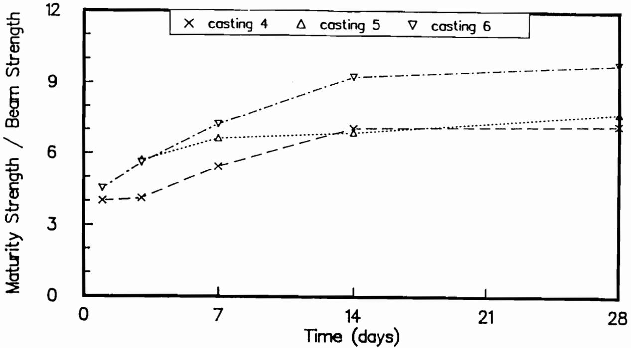
Fig B-30. Ratio of maturity method strengths to flexural strengths of wetroom-cured beams for castings 4, 5, and 6. Maturity curve based on outdoor-cured cylinders.
