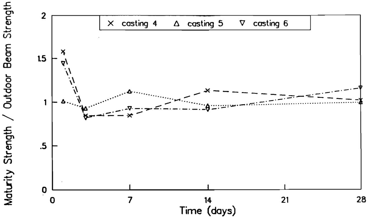
Fig B-44. Ratio of maturity method strengths to flexural strengths of outdoor-cured beams for castings 4, 5, and 6. Maturity curve based on outdoor-cured beams.
