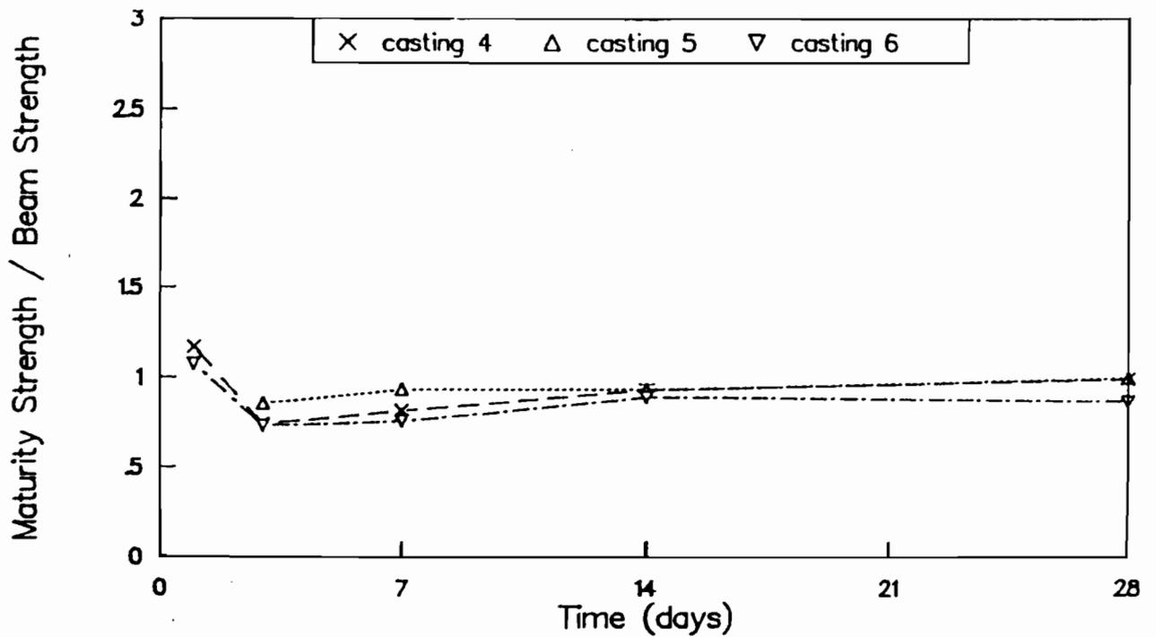
Fig B-33. Ratio of maturity method strengths to flexural strengths of wetroom-cured beams for castings 4, 5, and 6. Maturity curve based on outdoor-cured beams.
