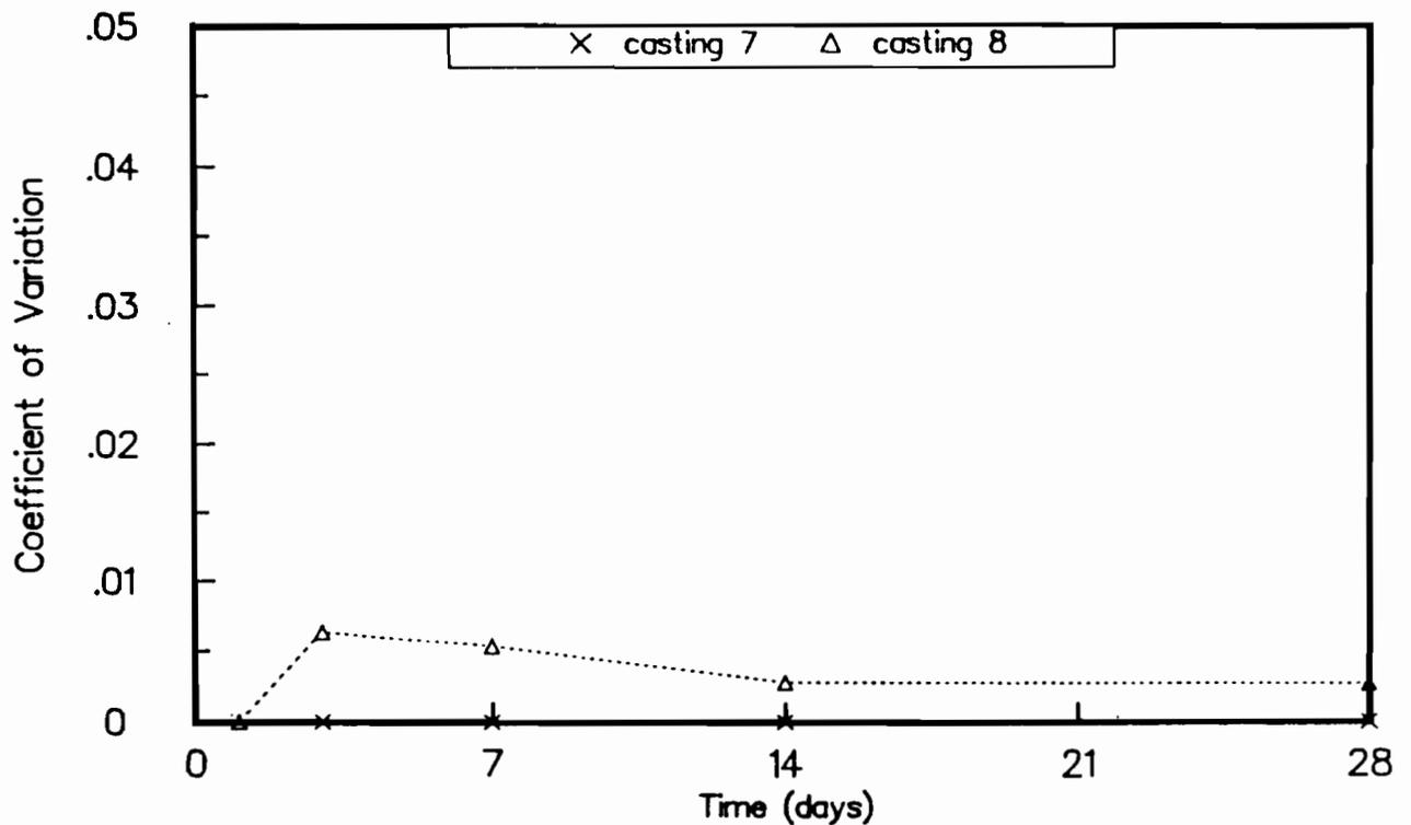
Fig C-54. Coefficient of variation of maturity method strengths for castings 7 and 8. Maturity curve based on cores drilled from slabs.
