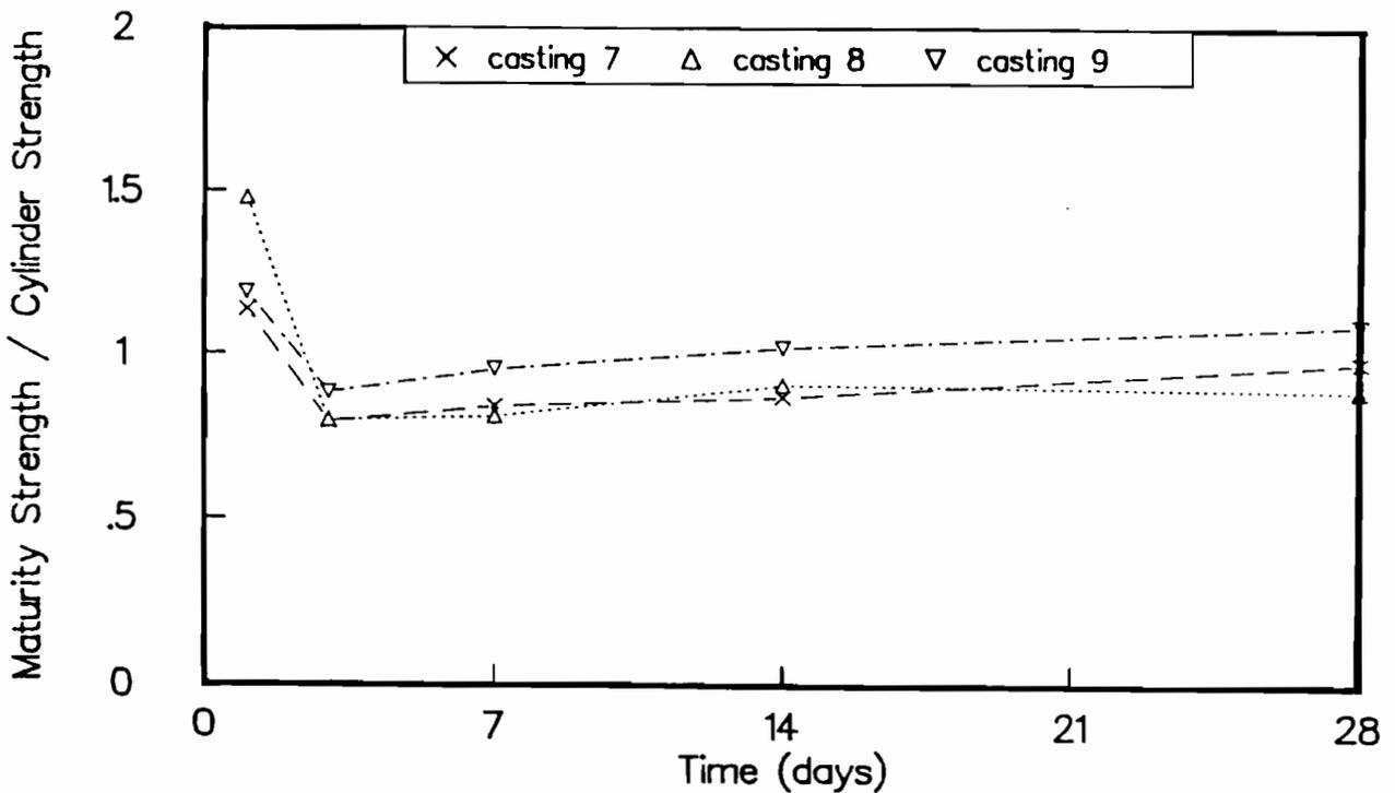
Fig C-8. Ratio of maturity method strengths to strengths of wetroom-cured cylinders for castings 7, 8, and 9. Maturity curve based on outdoor-cured cylinders.
