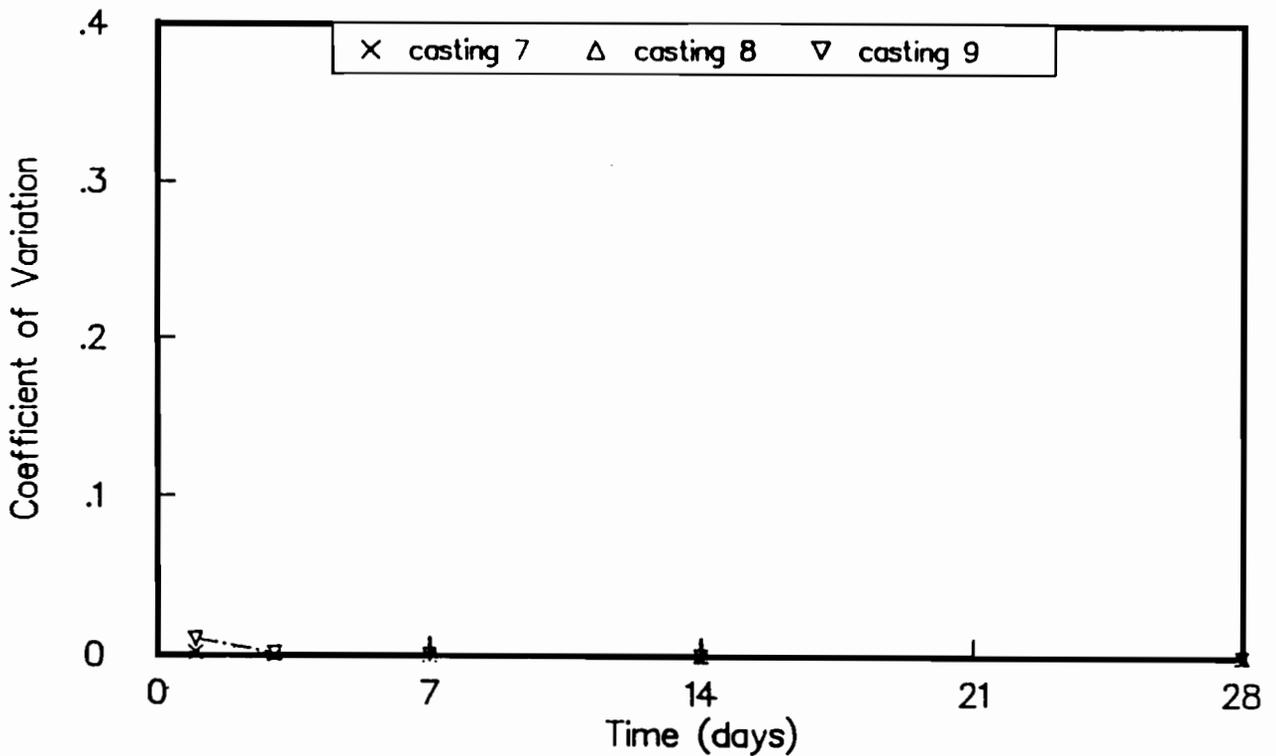
Fig C-52. Coefficient of variation of maturity method strengths for castings 7, 8, and 9. Maturity curve based on wetroom-cured cylinders.
