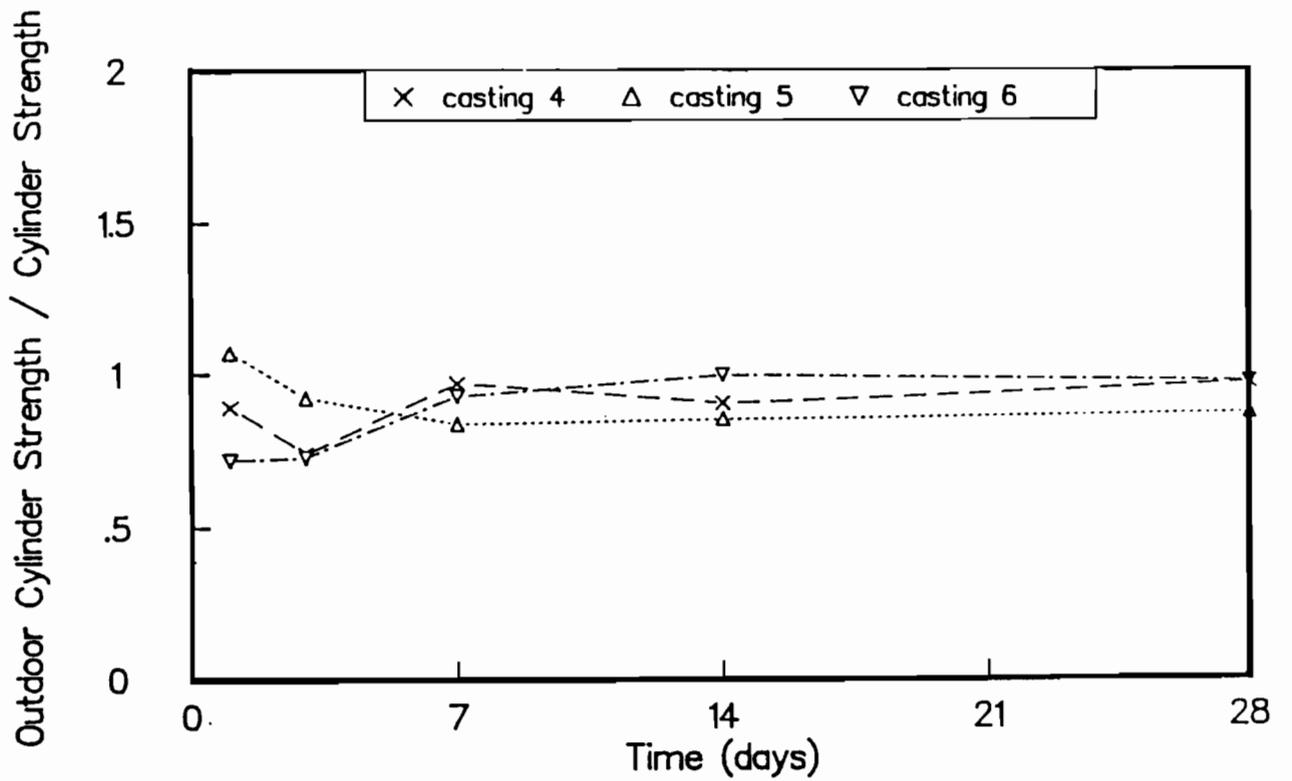
Fig B-1. Ratio of strengths of outdoor-cured cylinders to strengths of wetroom-cured cylinders for castings 4, 5, and 6.
