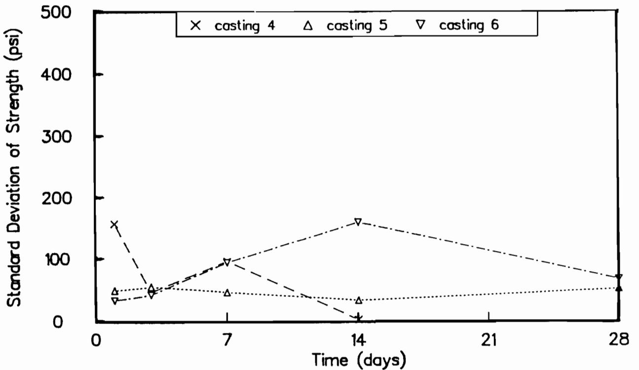
Fig B-65. Standard deviation of maturity method strengths for castings 4, 5, and 6. Maturity curve based on outdoor-cured cylinders.
