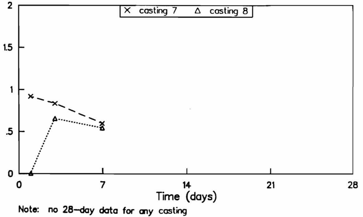
Fig C-17. Ratio of Windsor probe penetration resistance strengths to strengths of outdoor-cured cylinders for castings 7 and 8.
