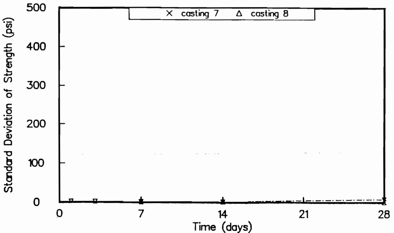
Fig C-68. Standard deviation of maturity method strengths for castings 7 and 8. Maturity curve based on outdoor-cured beams.
