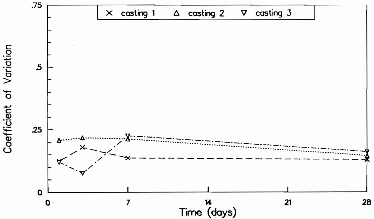
Fig A-16. Coefficient of variation of "Lok-test" pullout strengths for castings 1, 2, and 3.
