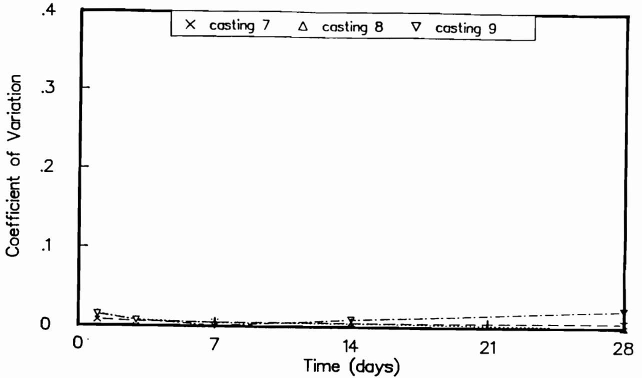
Fig C-53. Coefficient of variation of maturity method strengths for castings 7, 8, and 9. Maturity curve based on outdoor-cured cylinders.
