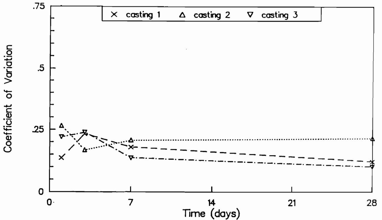
Fig A-15. Coefficient of variation of "CAPO-test" pullout strengths for castings 1, 2, and 3.
