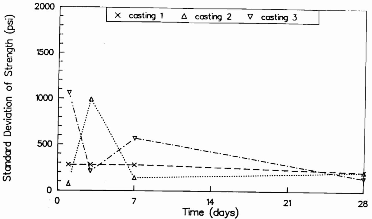
Fig A-24. Standard deviation of Windsor probe penetration resistance strengths for castings 1, 2, and 3.
