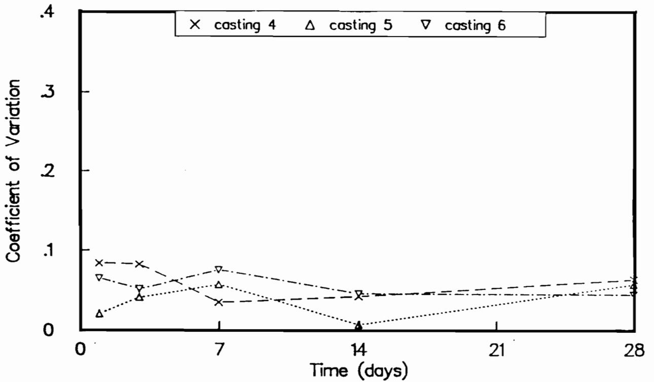
Fig B-49. Coefficient of variation of flexural strength of outdoor-cured beams for castings 4, 5, and 6.
