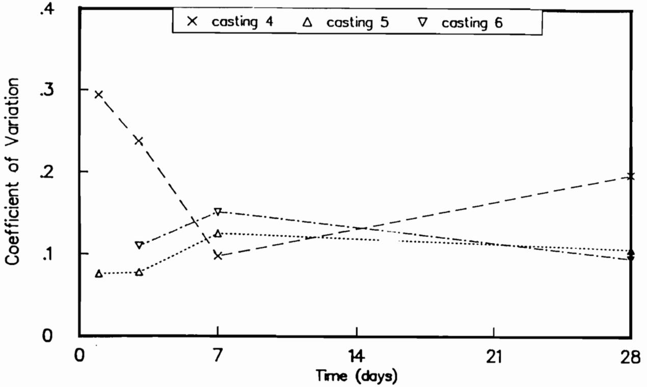
Fig B-50. Coefficient of variation of "Lok-Test" pullout strengths for castings 4, 5, and 6.
