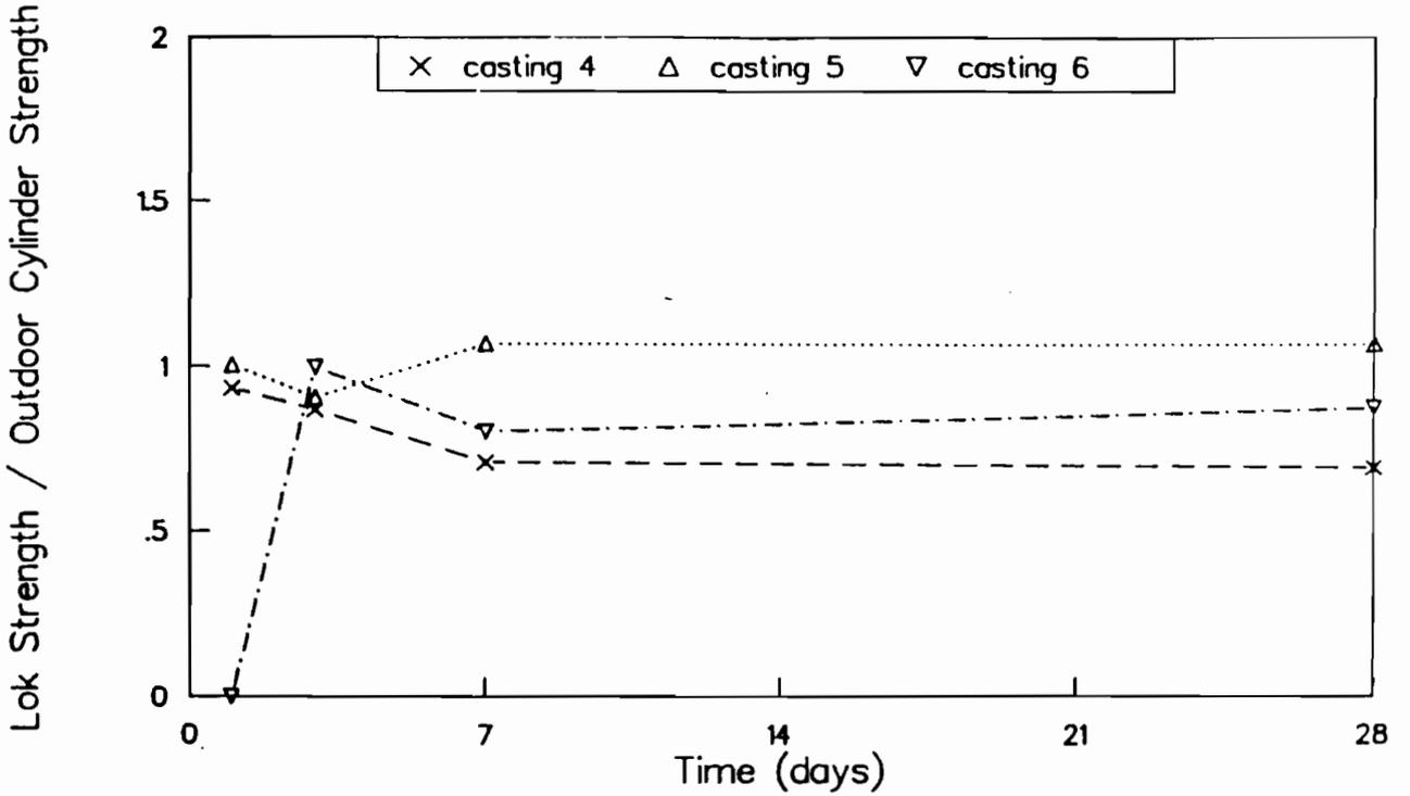
Fig B-16. Ratio of "Lok-Test" pullout strengths to strengths of outdoor-cured cylinders for castings 4, 5, and 6.
