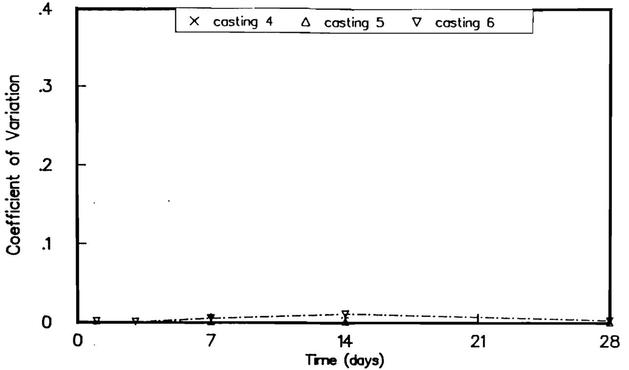
Fig B-56. Coefficient of variation of maturity method strengths for castings 4, 5, and 6. Maturity curve based on outdoor-cured beams.
