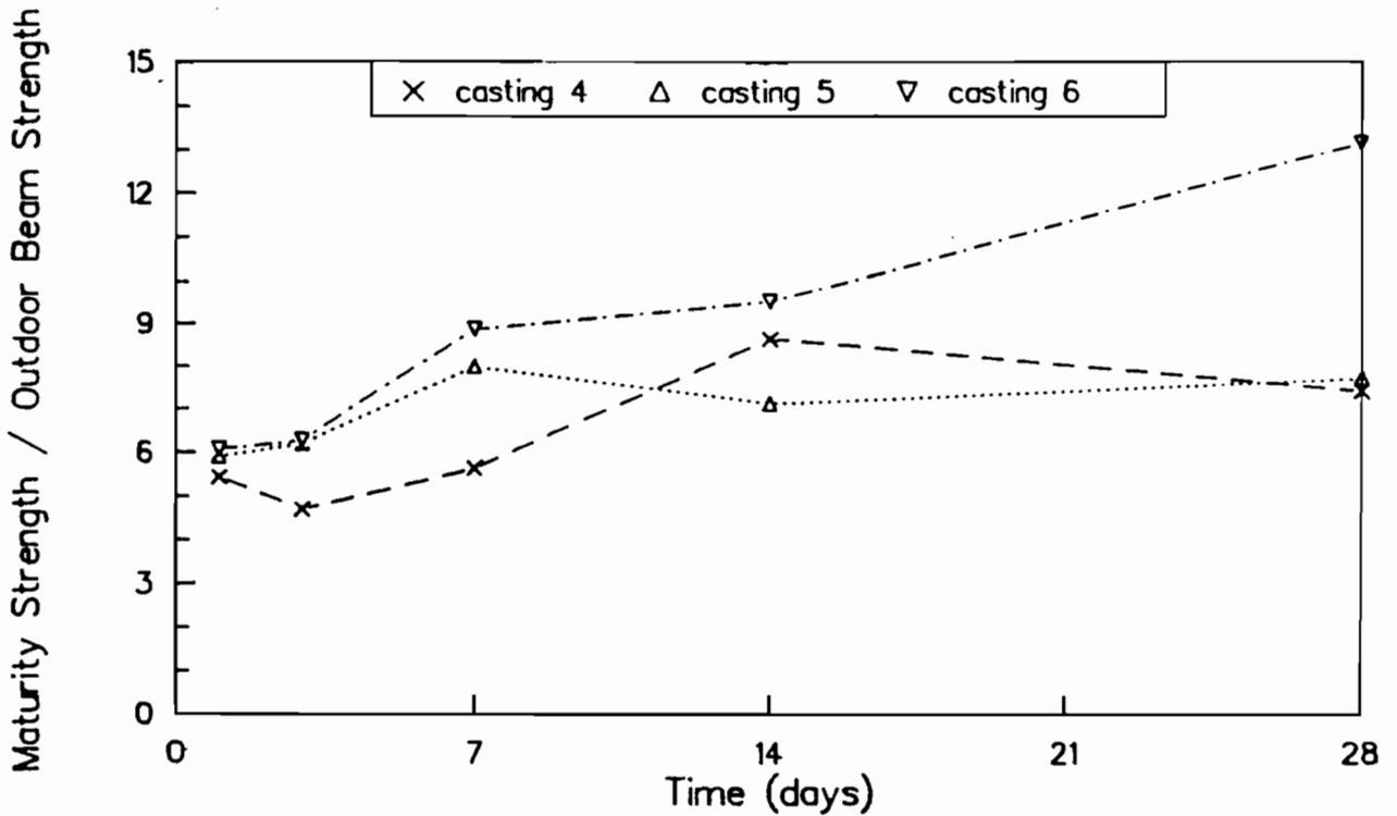
Fig B-41. Ratio of maturity method strengths to flexural strengths of outdoor-cured beams for castings 4, 5, and 6. Maturity curve based on outdoor-cured cylinders.
