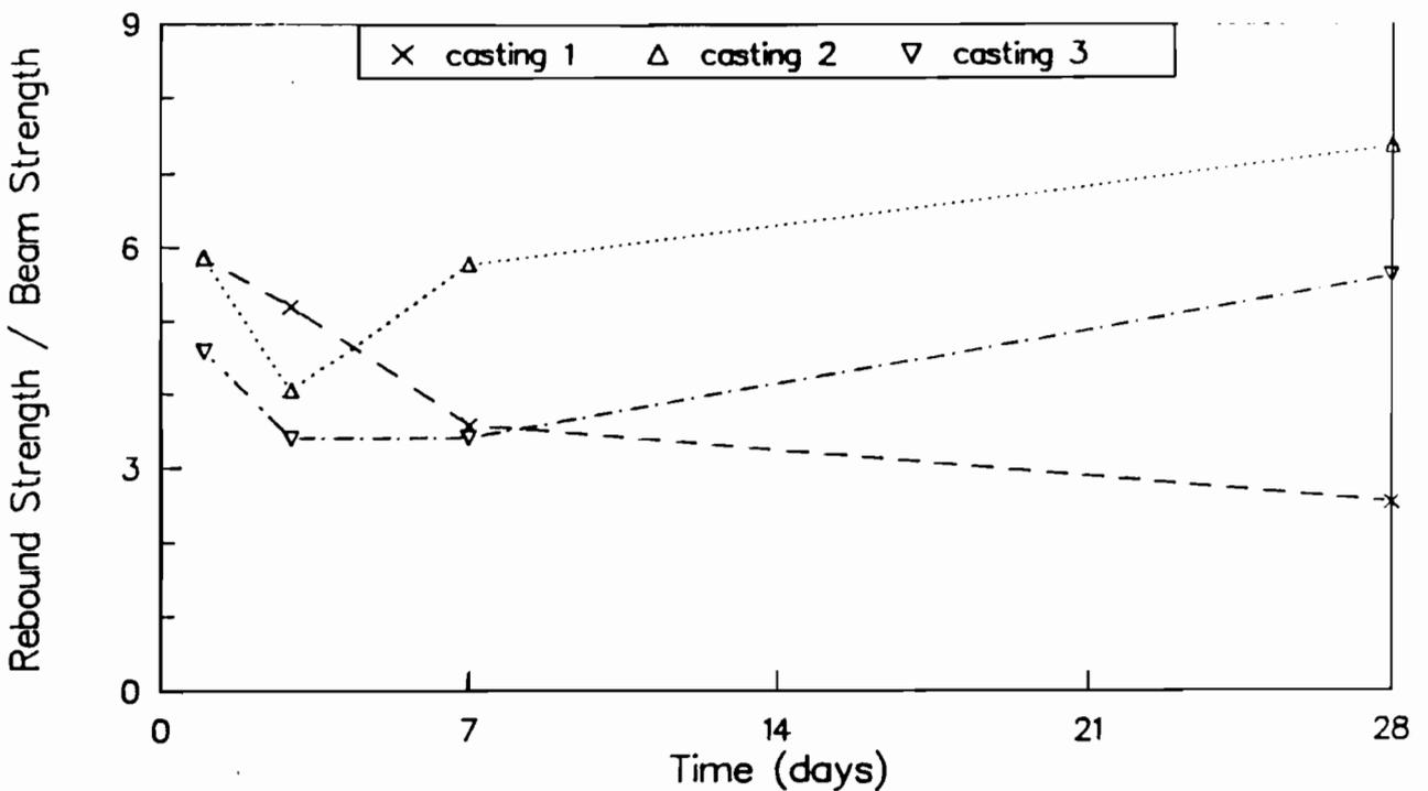
Fig A-11. Ratio of rebound number strengths to flexural strengths of wetroom-cured beams for castings 1, 2, and 3.
