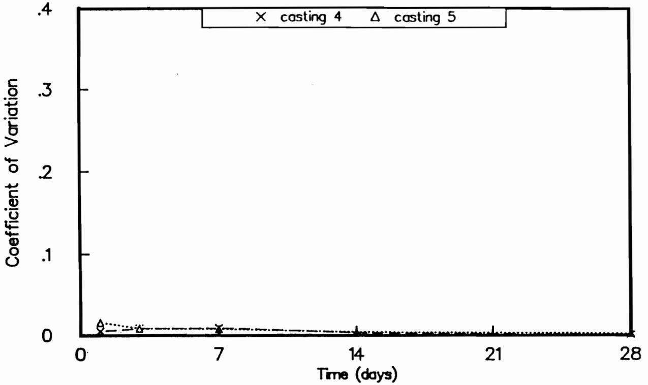
Fig B-54. Coefficient of variation of maturity method strengths for castings 4 and 5. Maturity curve based on cores drilled from slabs.
