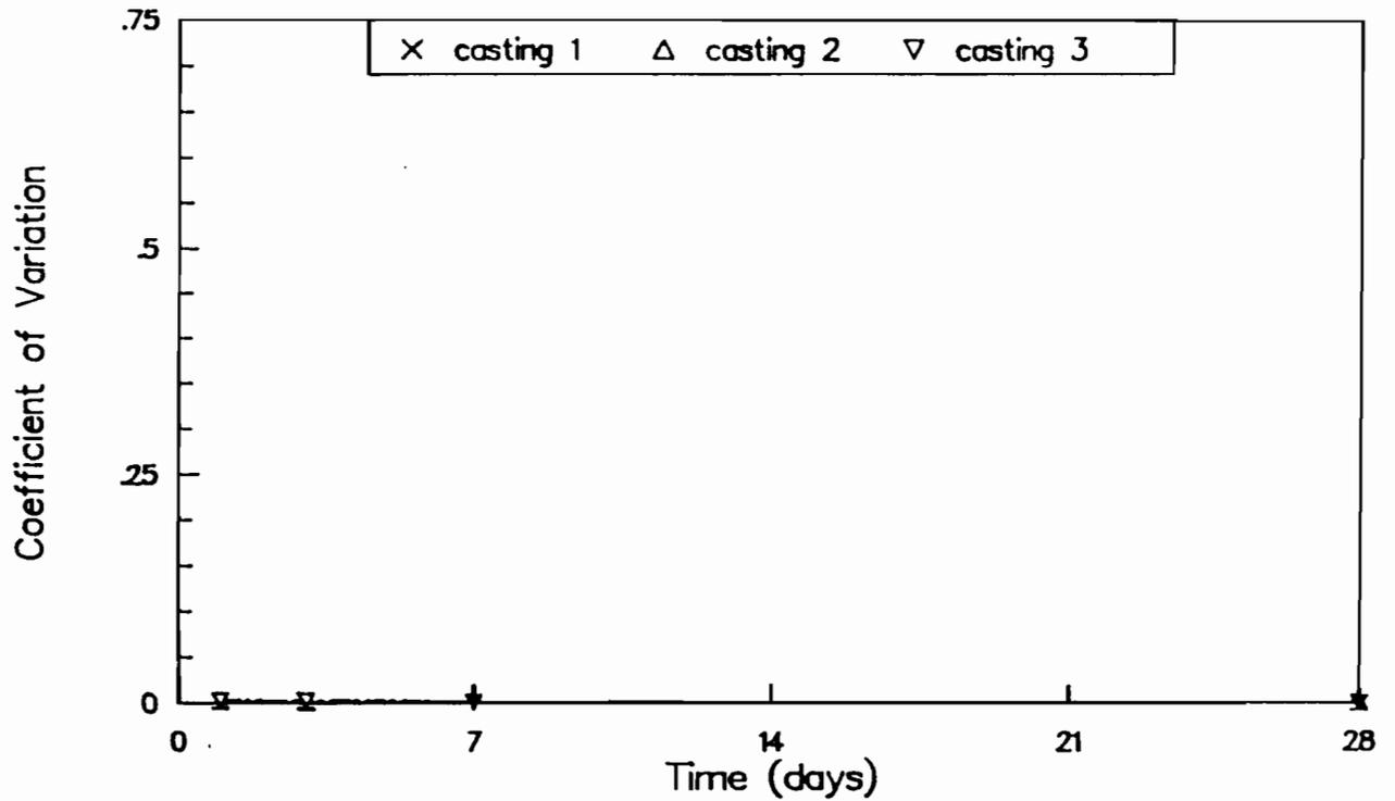
Fig A-19. Coefficient of variation of maturity method strengths for castings 1, 2, and 3.
