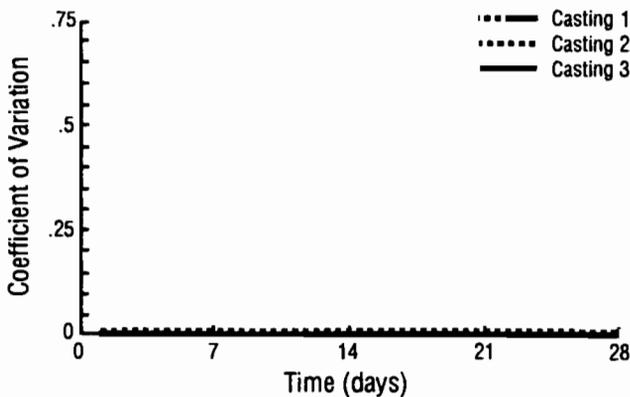
**Fig 5-11. Coefficient of variation of maturity method strengths for castings 1, 2, and 3.**
