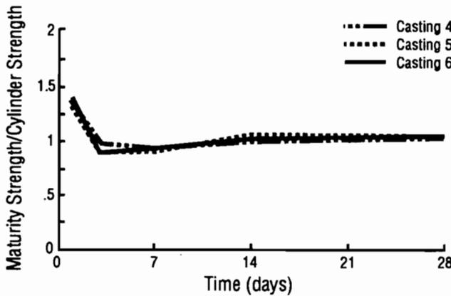
**Fig 5-20. Ratio of strength by maturity method to strength of wetroom-cured cylinders for castings 4, 5, and 6. Maturity curve based on wetroom-cured cylinders.**
