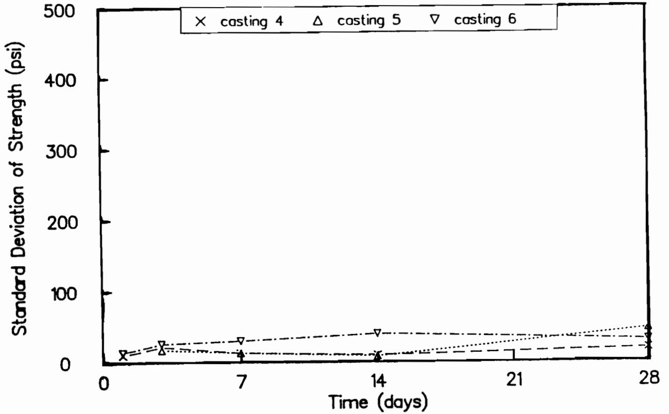
Fig B-60. Standard deviation of flexural strength of wetroom-cured beams for castings 4, 5, and 6.
