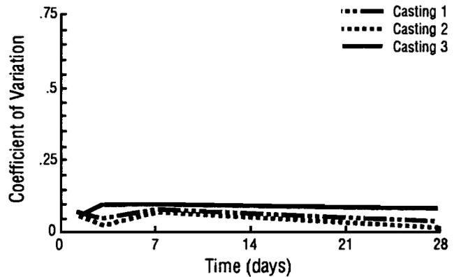
**Fig 5-9. Coefficient of variation of flexural strength of wetroom-cured beams for castings 1, 2, and 3.**
