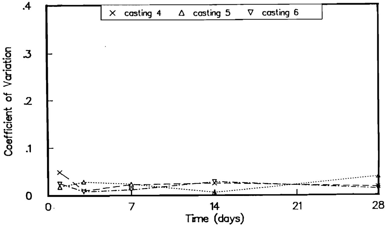
Fig B-45. Coefficient of variation of wetroom-cured cylinder strengths for castings 4, 5, and 6.
