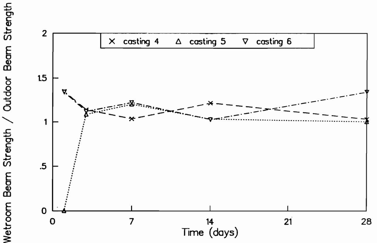
Fig B-37. Ratio of flexural strengths of wetroom-cured beams to flexural strengths of outdoor-cured beams for castings 4, 5, and 6.
