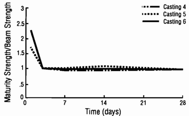
**Fig 5-22. Ratio of strength by maturity method to strength of wetroom-cured flexural beams for castings 4, 5, and 6. Maturity curve based on wetroom-cured beams.**
