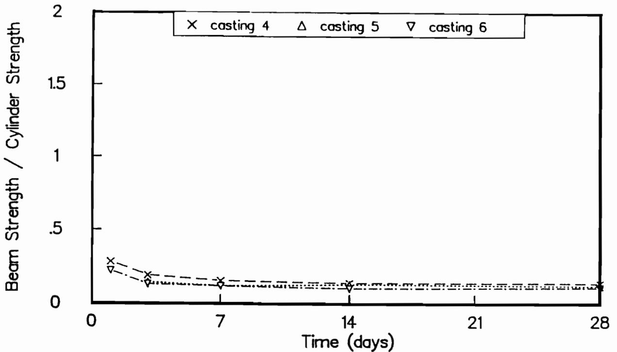
Fig B-3. Ratio of flexural strengths of wetroom-cured beams to strengths of wetroom-cured cylinders for castings 4, 5, and 6.
