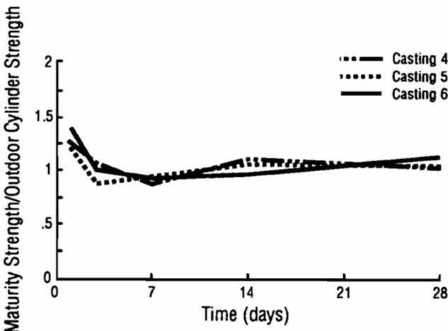
**Fig 5-21. Ratio of strength by maturity method to strength of outdoor-cured cylinders for castings 4, 5, and 6. Maturity curve based on outdoor-cured cylinders.**
