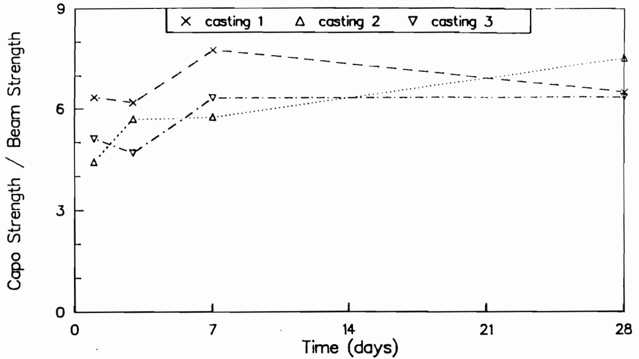
Fig A-8. Ratio of "CAPO-test" pullout strengths to flexural strengths of wetroom-cured beams for castings 1, 2, and 3.
