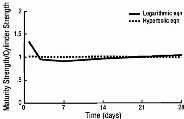
Fig 5-35. Ratio of maturity method strength to strength of wetroom-cured cylinders using two different maturity relationships.
