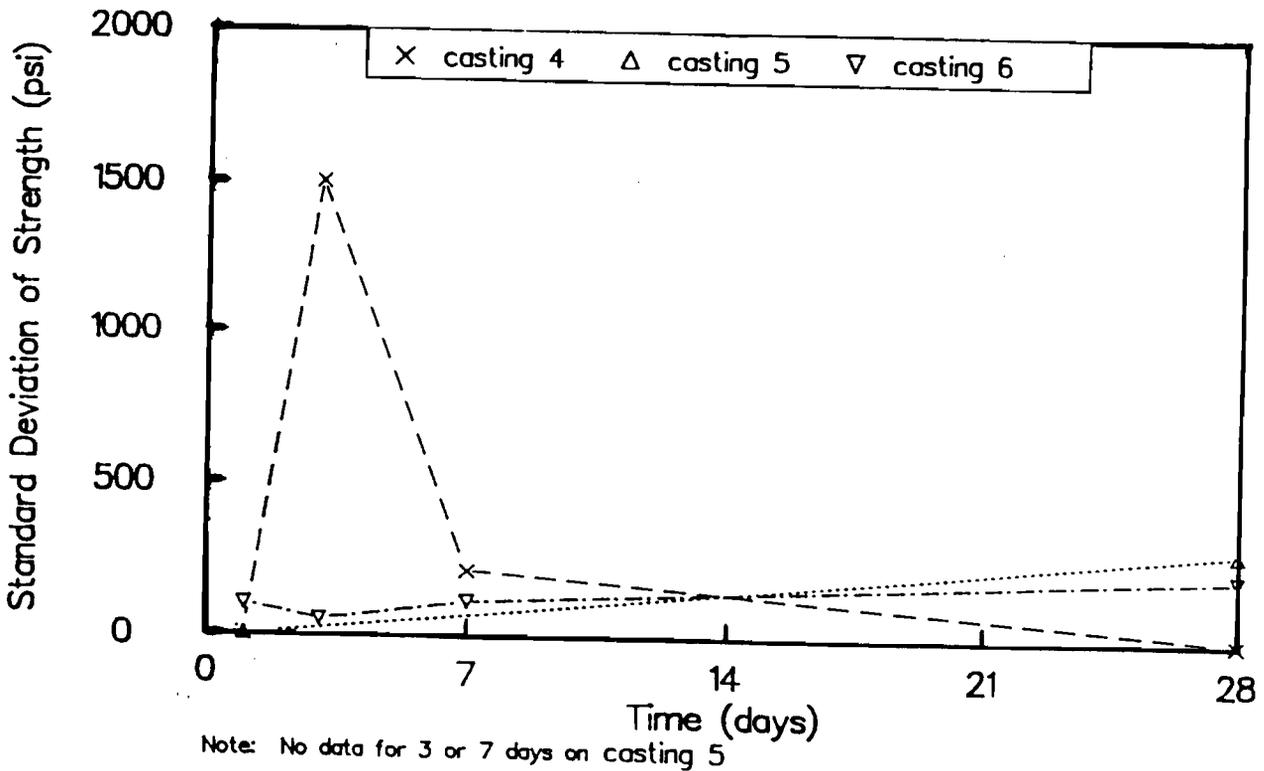
Fig B-63. Standard deviation of Windsor probe penetration resistance strengths for castings 4, 5, and 6.
