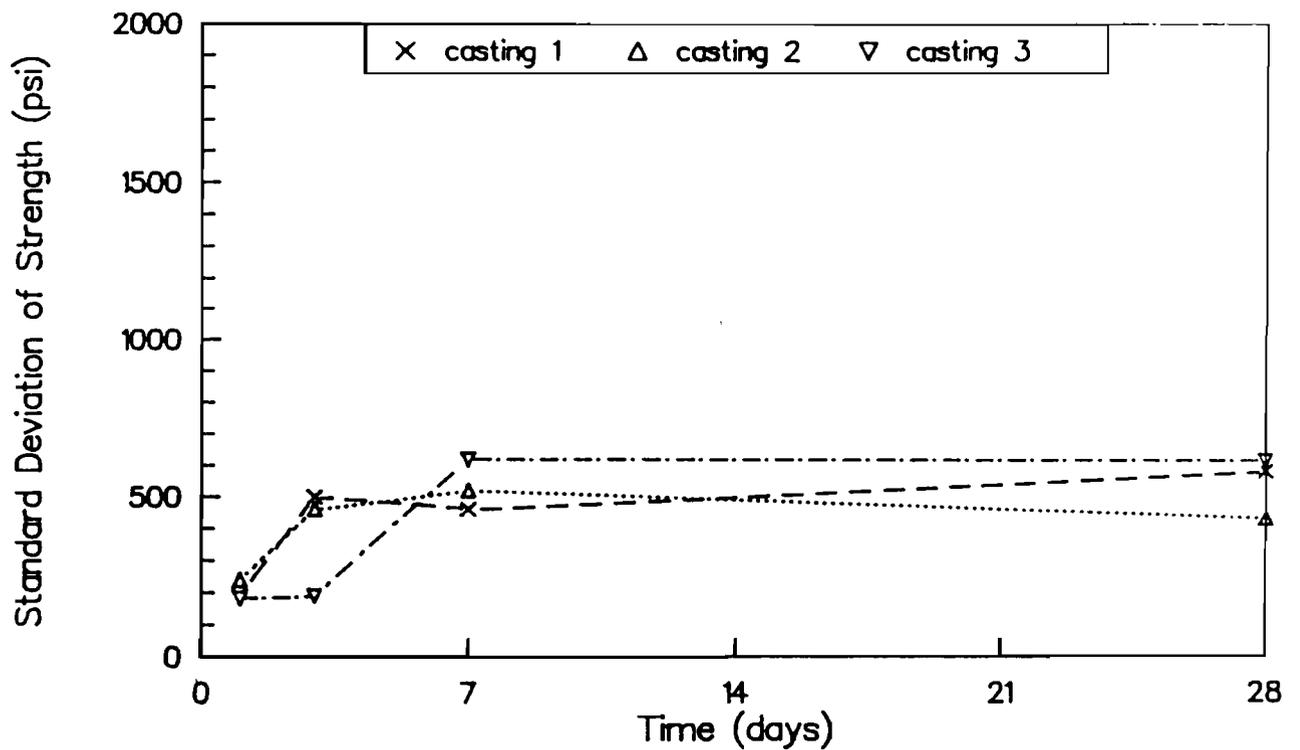
Fig A-23. Standard deviation of “Lok-Test” pullout strengths for castings 1, 2, and 3.
