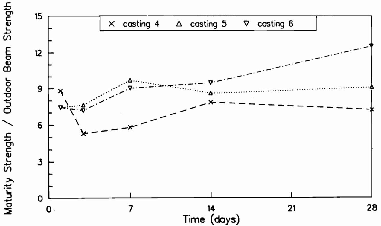
Fig B-42. Ratio of maturity method strengths to flexural strengths of outdoor-cured beams for castings 4, 5, and 6. Maturity curve based on cores drilled from slabs.
