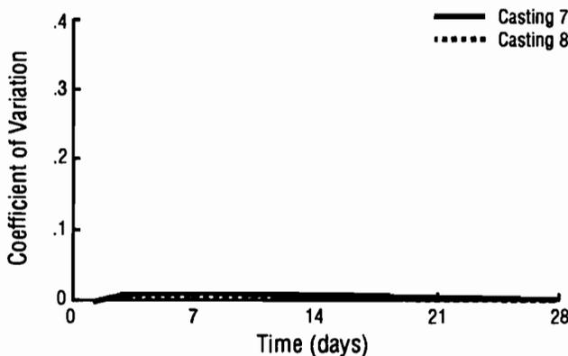
**Fig 5-25.** Coefficient of variation of maturity method strengths for castings 7 and 8. Maturity curves based on cores drilled from slabs.
