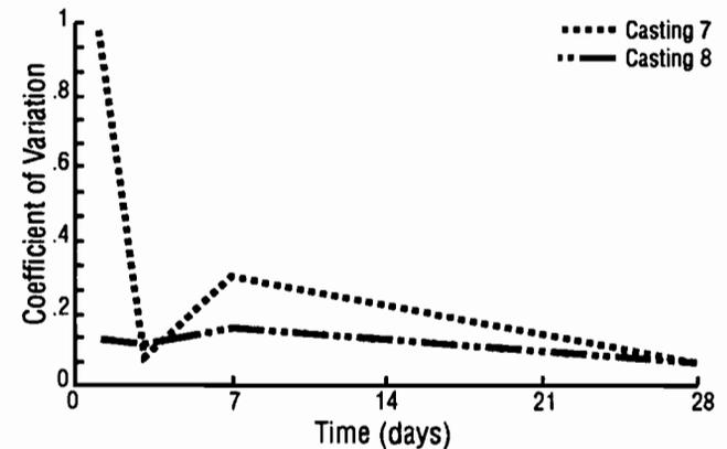
**Fig 5-27.** Coefficient of variation of “Lok-Test” pullout strengths for castings 7 and 8.
