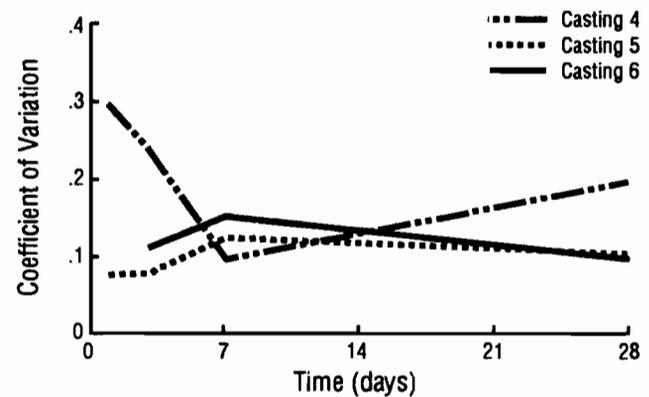
**Fig 5-26.** Coefficient of variation of “Lok-Test” pullout strengths for castings 4, 5, and 6.
