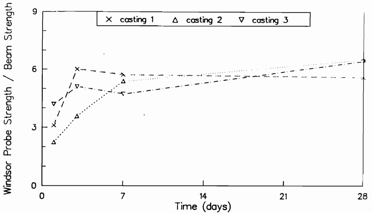
Fig A-10. Ratio of Windsor probe penetration resistance strengths to flexural strengths of wetroom-cured beams for castings 1, 2, and 3.
