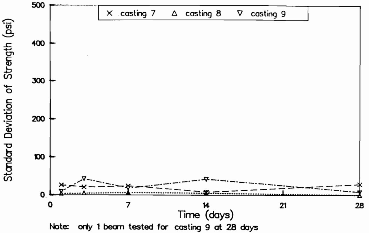
Fig C-61. Standard deviation of flexural strength of outdoor-cured beams for castings 7, 8, and 9.
