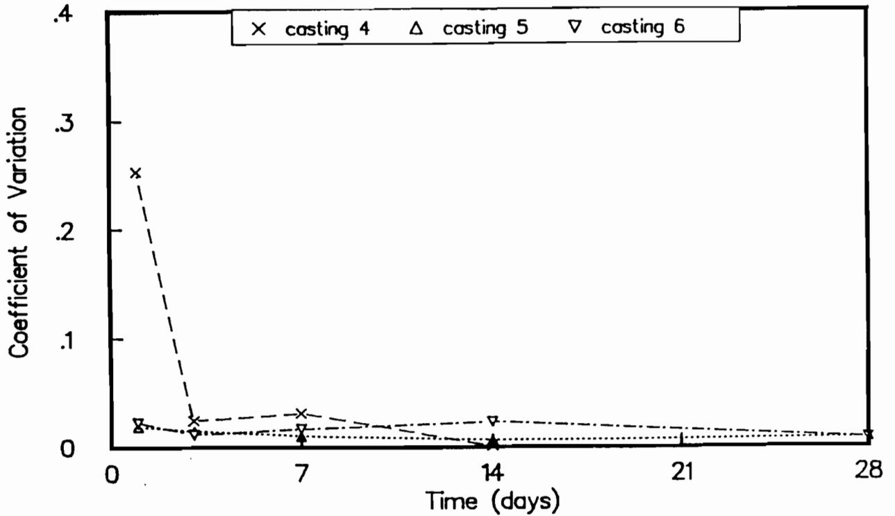
Fig B-53. Coefficient of variation of maturity method strengths for castings 4, 5, and 6. Maturity curve based on outdoor-cured cylinders.
