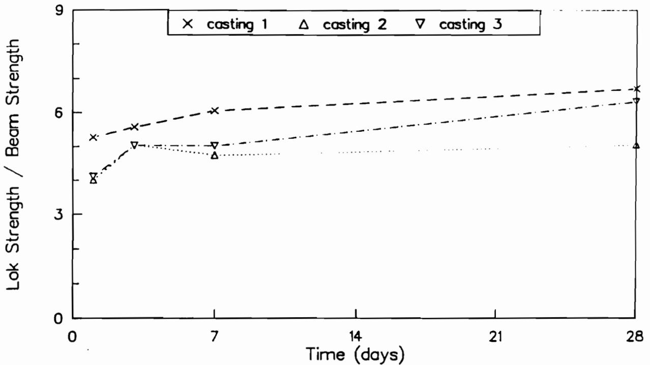
Fig A-9. Ratio of "Lok-Test" pullout strengths to flexural strengths of wetroom-cured beams for castings 1, 2, and 3.
