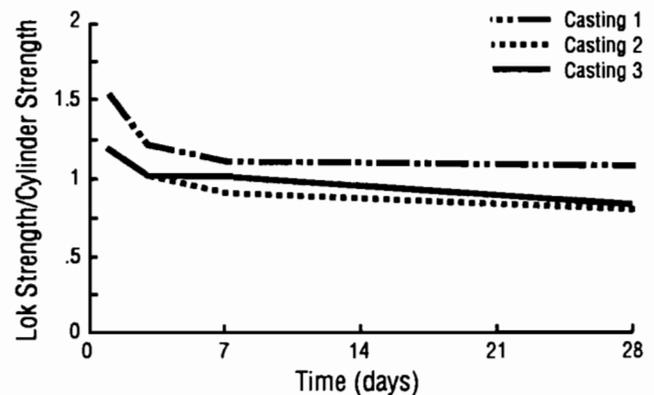
Fig 5-2. Ratio of "Lok-Test" pullout strength to strength of wetroom-cured cylinders of castings 1, 2, and 3.
