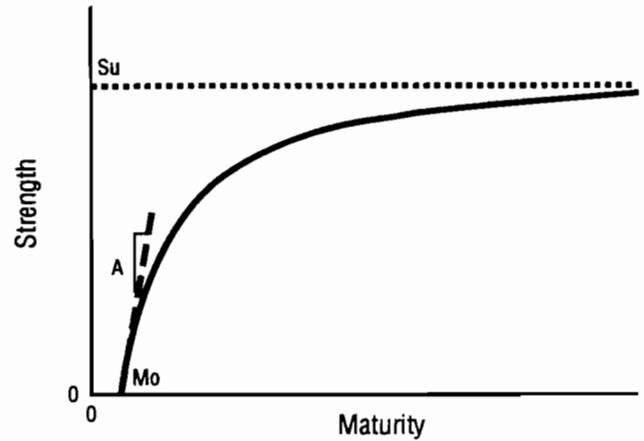
Fig 5-31. Typical relationship between maturity and strength with hyperbolic constants defined.
