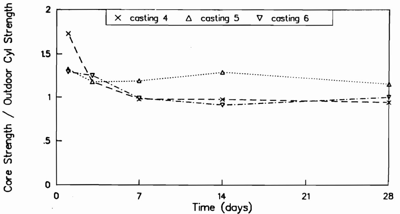
Fig B-13. Ratio of strengths of cores to strengths of outdoor-cured cylinders for castings 4, 5, and 6.
