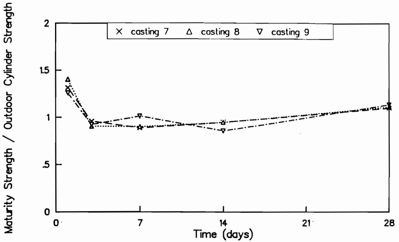
Fig C-19. Ratio of maturity method strengths to strengths of outdoor-cured cylinders for castings 7, 8, and 9. Maturity curve based on outdoor-cured cylinders.
