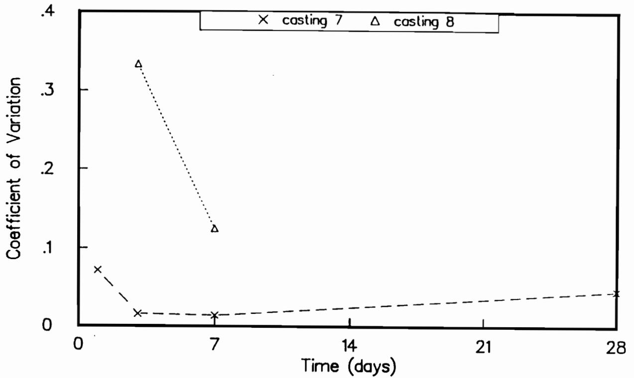
Fig C-51. Coefficient of variation of Windsor probe penetration resistance strengths for castings 7 and 8.
