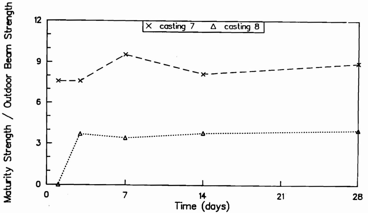
Fig C-42. Ratio of maturity method strengths to flexural strengths of outdoor-cured beams for castings 7 and 8. Maturity curve based on cores drilled from slabs.
