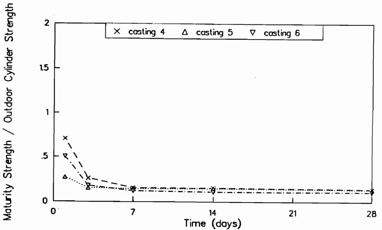
Fig B-21. Ratio of maturity method strengths to strengths of outdoor-cured cylinders for castings 4, 5, and 6. Maturity curve based on wetroom-cured beams.
