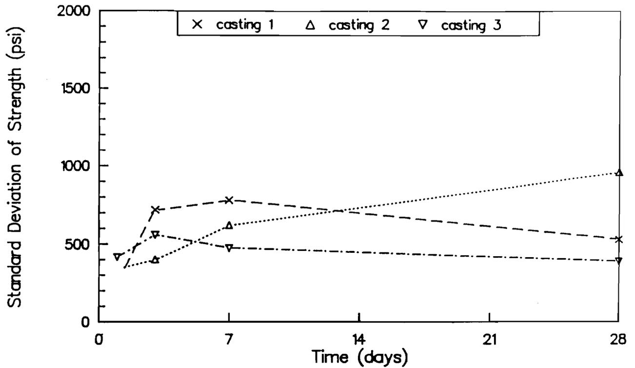
Fig A-22. Standard deviation of “CAPO-test” pullout strengths for castings 1, 2, and 3.
