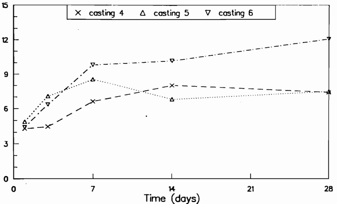
Fig B-35. Ratio of strengths of outdoor-cured cylinders to flexural strengths of outdoor-cured beams for castings 4, 5, and 6.
