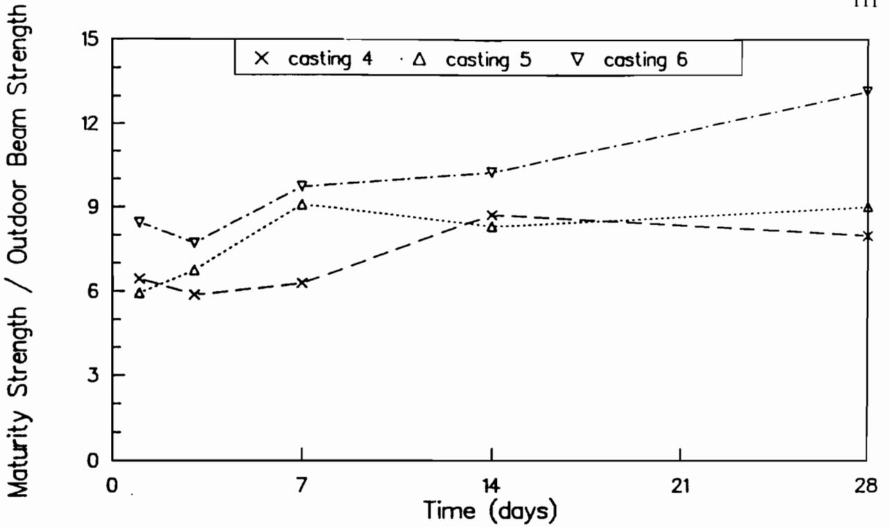
Fig B-40. Ratio of maturity method strengths to flexural strengths of outdoor-cured beams for castings 4, 5, and 6. Maturity curve based on wetroom-cured cylinders.
