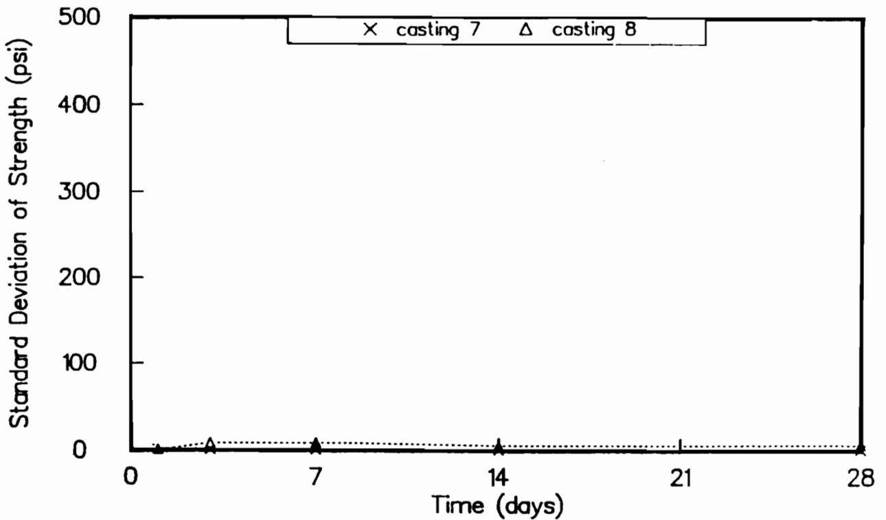
Fig C-66. Standard deviation of maturity method strengths for castings 7 and 8. Maturity curve based on cores drilled from slabs.
