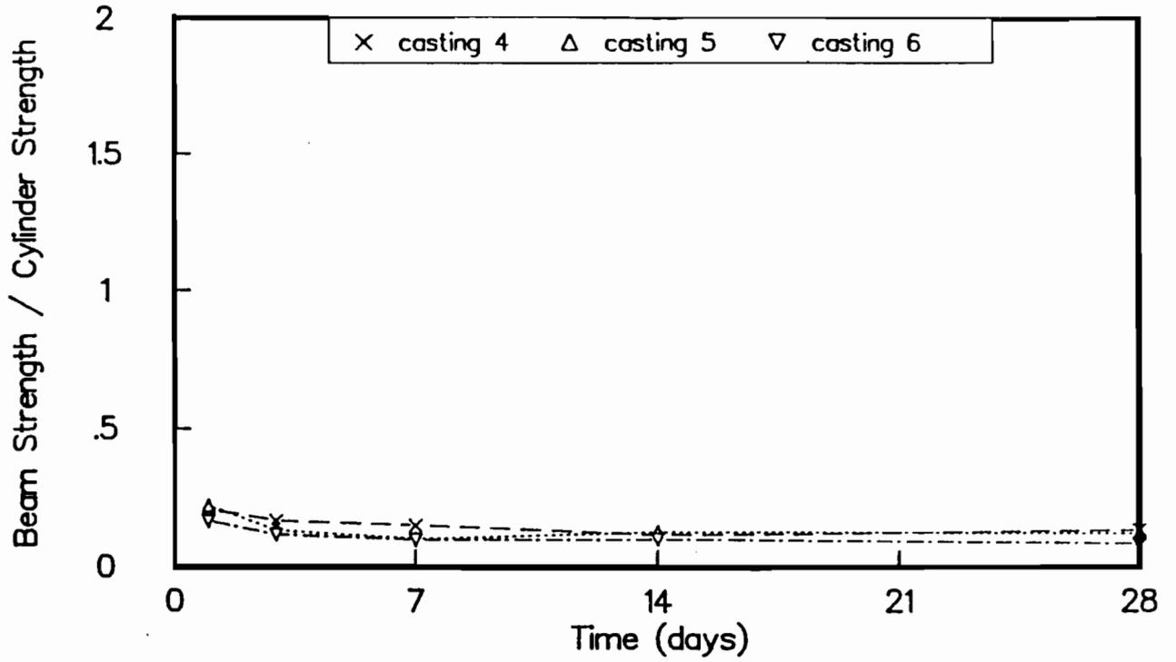
Fig B-4. Ratio of flexural strengths of outdoor-cured beams to strengths of wetroom-cured cylinders for castings 4, 5, and 6.
