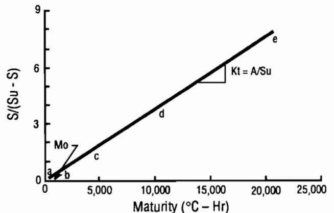
Fig 5-33. Relationship between maturity and  $S/S_u - S$  used to determine  $K_t$ ,  $A$  and  $M_o$ .
