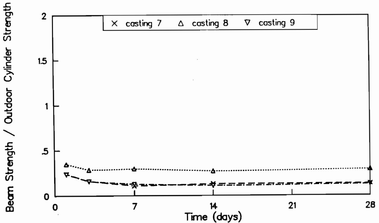
Fig C-15. Ratio of flexural strengths of outdoor-cured beams to strengths of outdoor-cured cylinders for castings 7, 8, and 9.
