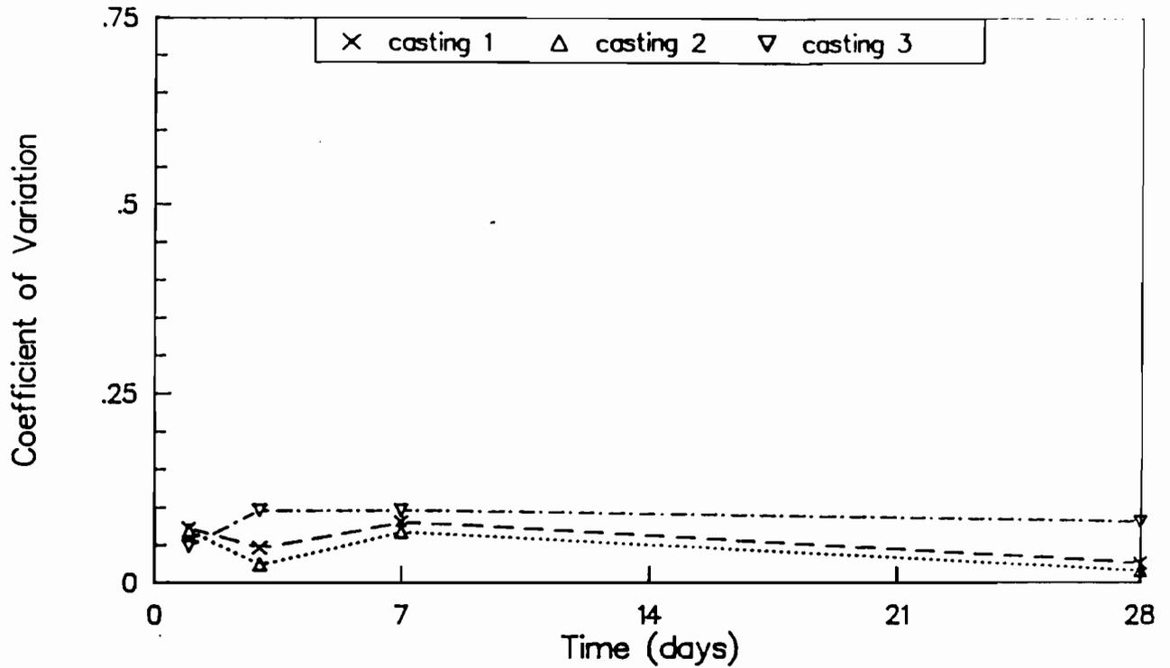
Fig A-14. Coefficient of variation of flexural strength of wetroom-cured beams for castings 1, 2, and 3.
