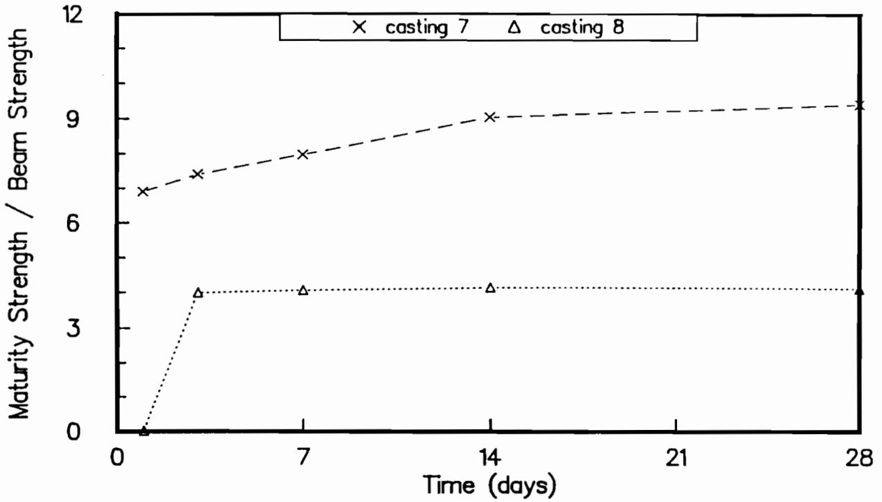
Fig C-31. Ratio of maturity method strengths to flexural strengths of wetroom-cured beams for castings 7 and 8. Maturity curve based on cores drilled from slabs.
