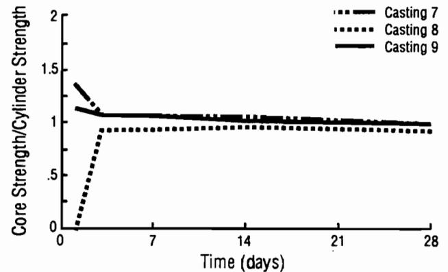
**Fig 5-19. Ratio of strength of cores drilled from slabs to strength of wetroom-cured cylinders for castings 7, 8, and 9.**
