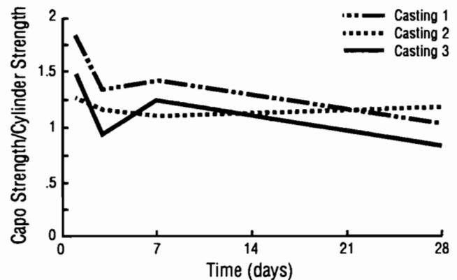
Fig 5-1. Ratio of "CAPO test" strength to strength of wetroom-cured cylinders for castings 1, 2, and 3.
