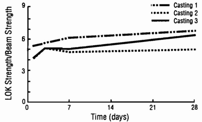
Fig 5-14. Ratio of "Lok-Test" pullout strength to strength of wetroom-cured flexural beams for castings 1, 2, and 3.
