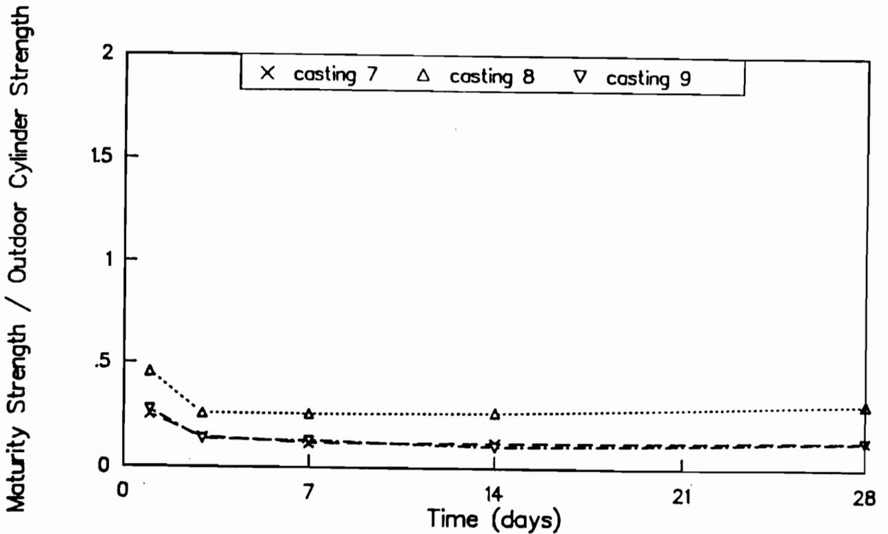
Fig C-22. Ratio of maturity method strengths to strengths of outdoor-cured cylinders for castings 7, 8, and 9. Maturity curve based on outdoor-cured beams.
