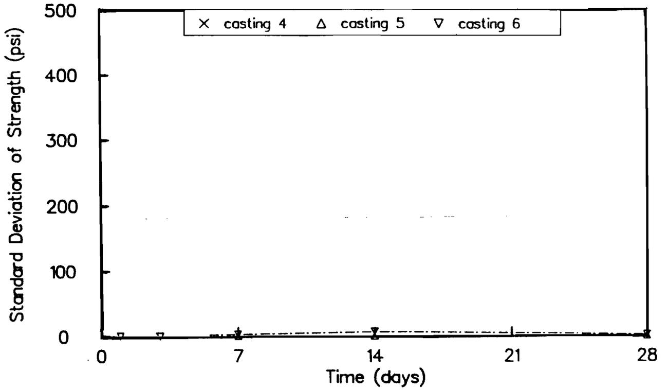
**Fig B-68. Standard deviation of maturity method strengths for castings 4, 5, and 6. Maturity curve based on outdoor-cured beams.**
