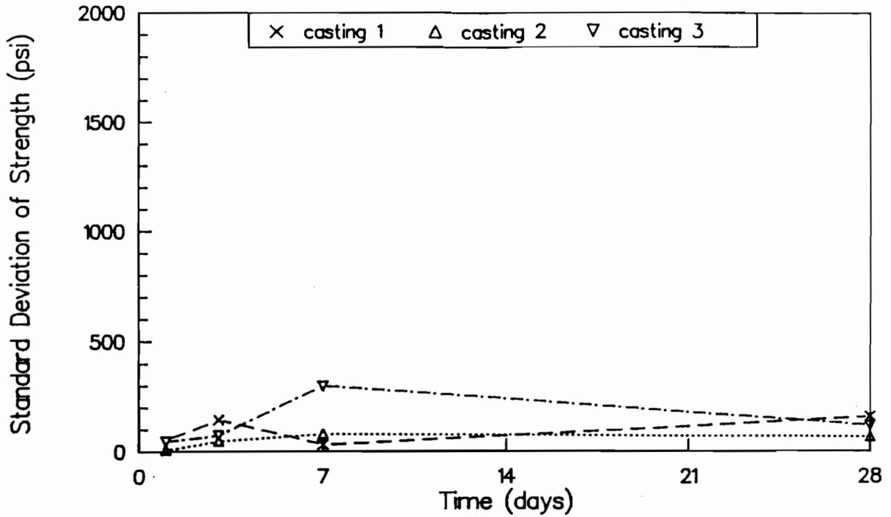
Fig A-20. Standard deviation of wetroom-cured cylinder strengths for castings 1, 2, and 3.
