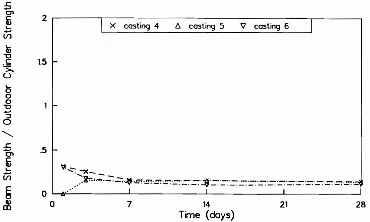
Fig B-14. Ratio of flexural strengths of wetroom-cured beams to strengths of outdoor-cured cylinders for castings 4, 5, and 6.
