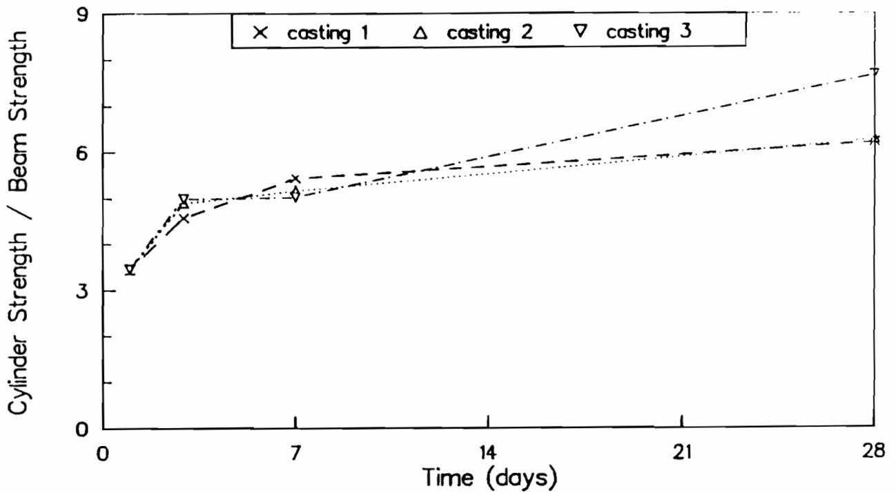
Fig A-7. Ratio of strengths of wetroom-cured cylinders to flexural strengths of wetroom-cured beams for castings 1, 2, and 3.
