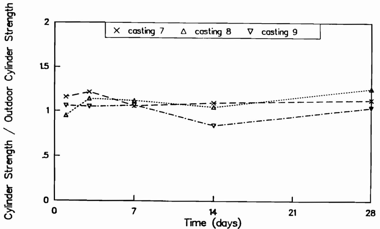
Fig C-12. Ratio of strengths of wetroom-cured cylinders to strengths of outdoor-cured cylinders for castings 7, 8, and 9.
