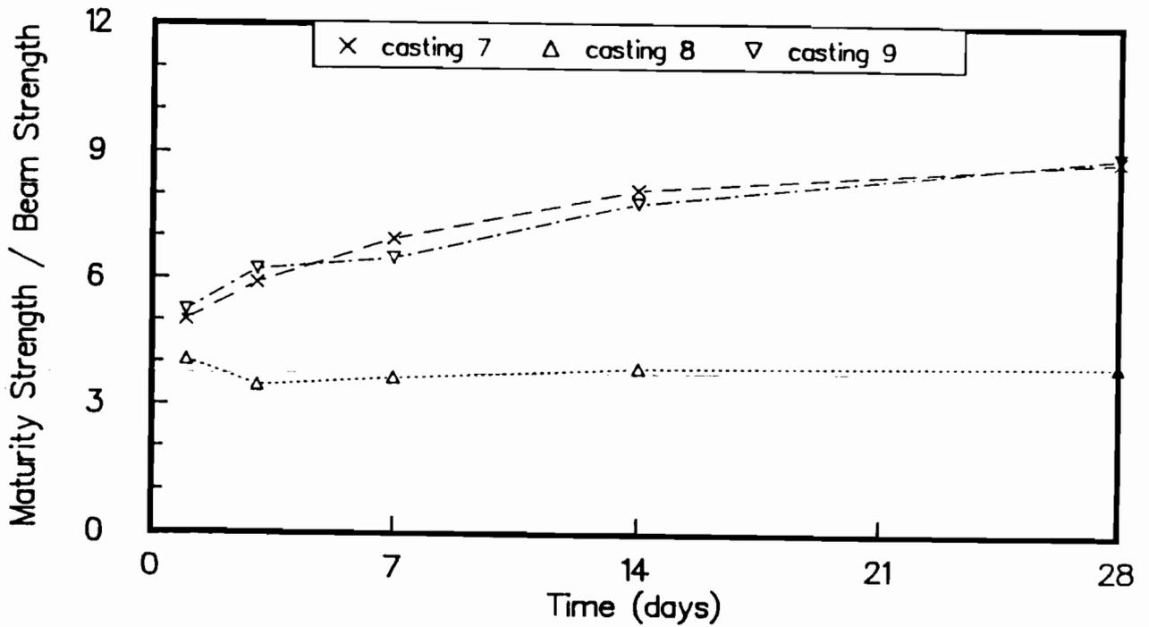
Fig C-30. Ratio of maturity method strengths to flexural strengths of wetroom-cured beams for castings 7, 8, and 9. Maturity curve based on outdoor-cured cylinders.
