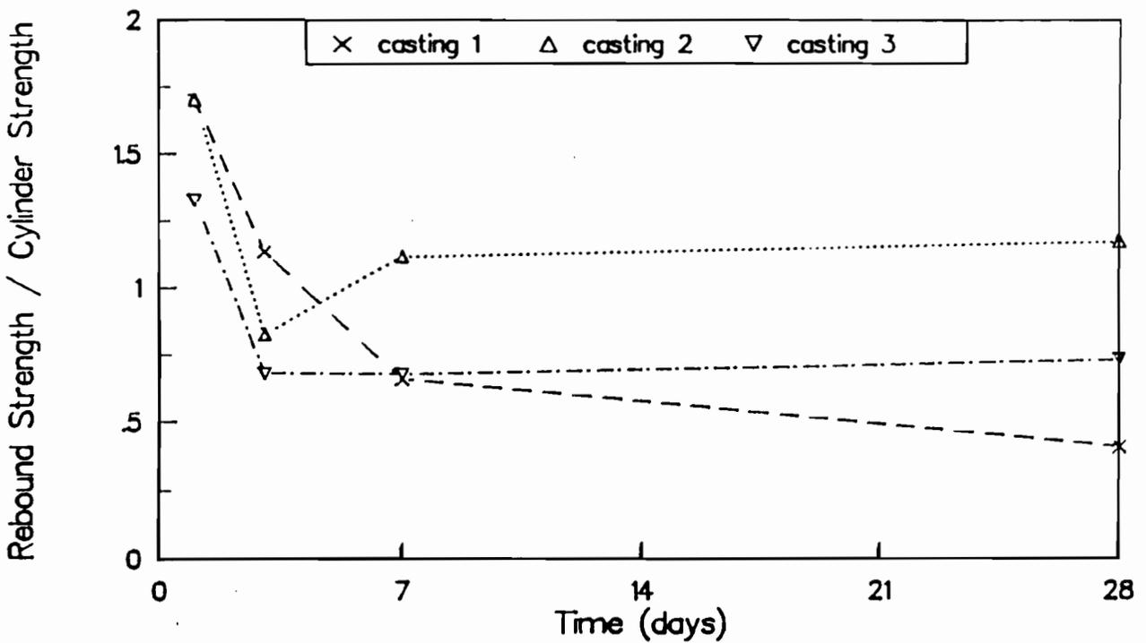
Fig A-5. Ratio of rebound number strengths to strengths of wetroom-cured cylinders for castings 1, 2, and 3.
