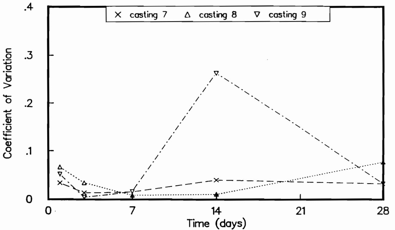
Fig C-46. Coefficient of variation of outdoor-cured cylinder strengths for castings 7, 8, and 9.
