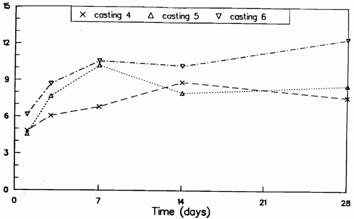
Fig B-34. Ratio of strengths of wetroom-cured cylinders to flexural strengths of outdoor-cured beams for castings 4, 5, and 6.
