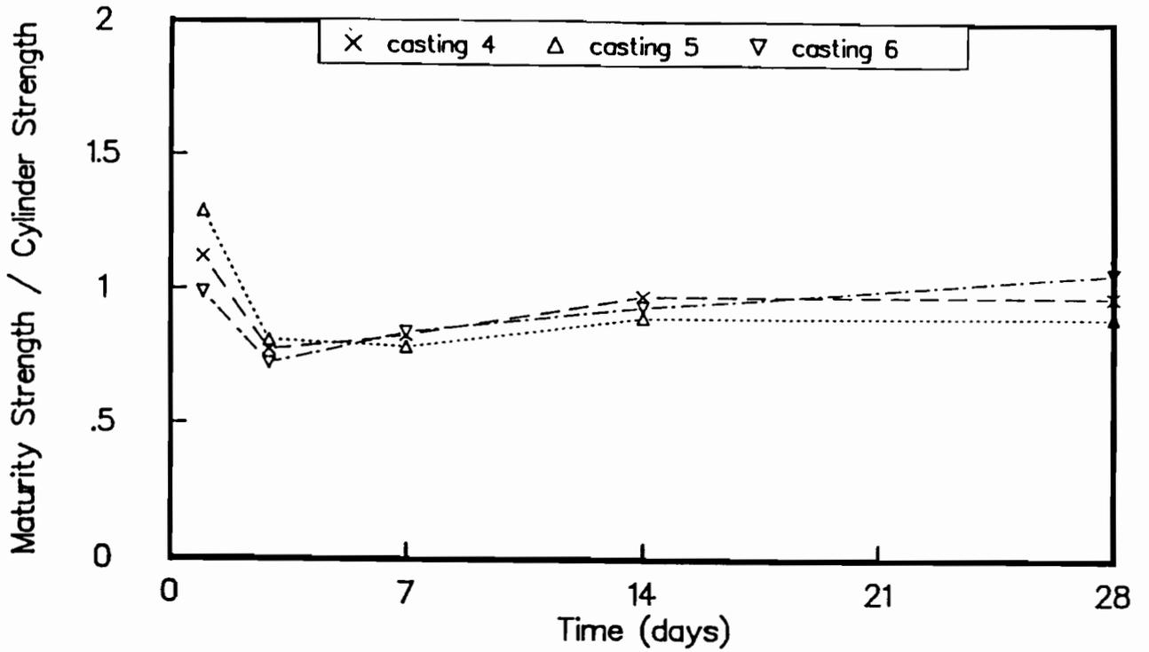
Fig B-8. Ratio of maturity method strengths to strengths of wetroom-cured cylinders for castings 4, 5, and 6. Maturity curve based on outdoor-cured cylinders.
