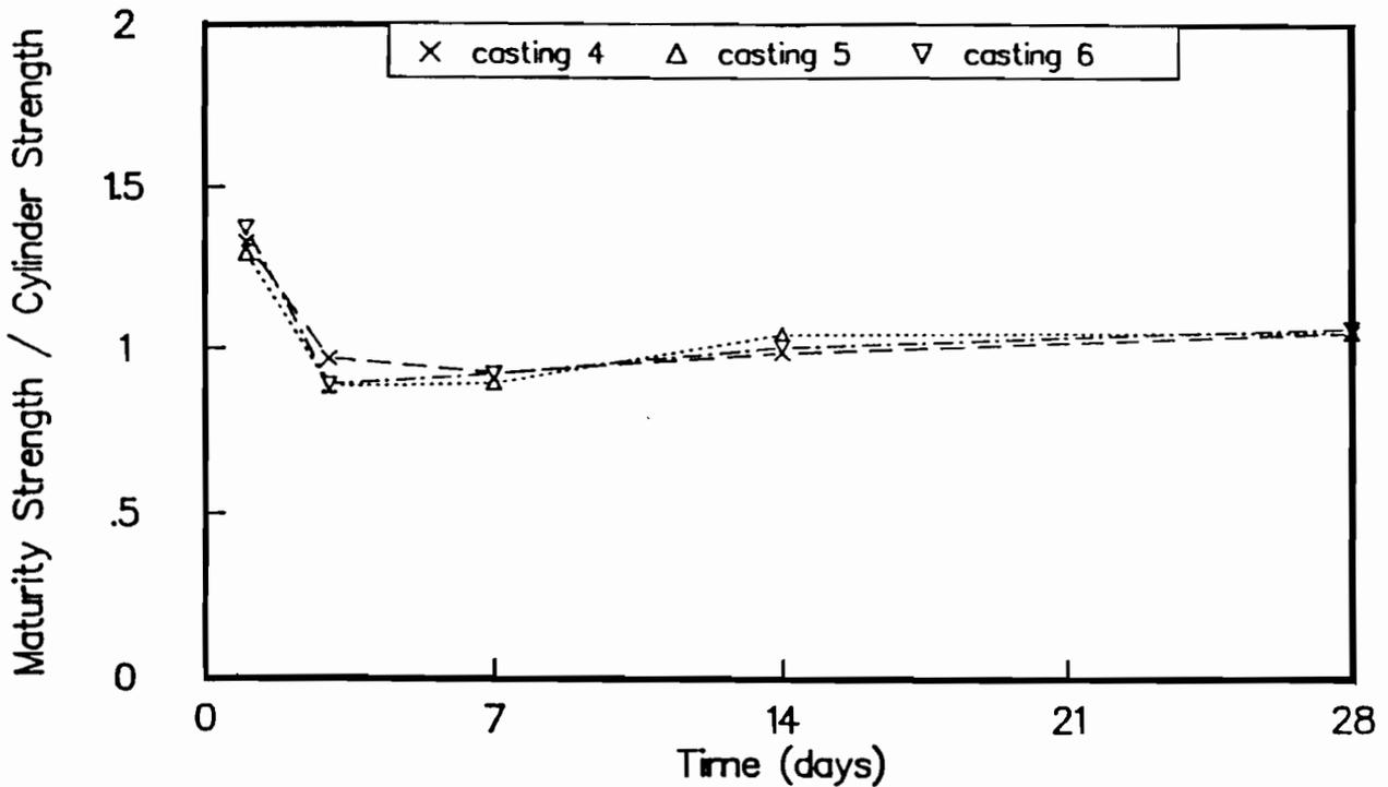
Fig B-7. Ratio of maturity method strengths to strengths of wetroom-cured cylinders for castings 4, 5, and 6. Maturity curve based on wetroom-cured cylinders.
