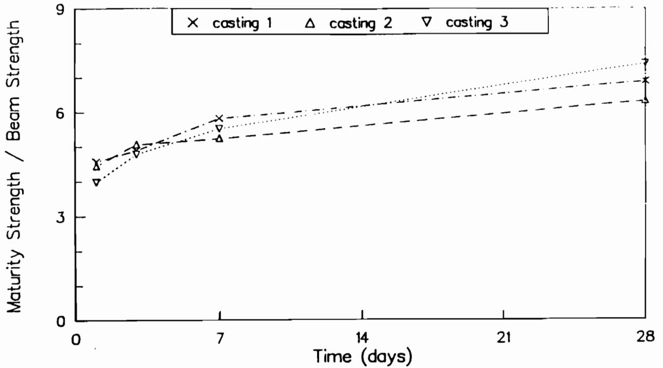
Fig A-12. Ratio of maturity method strengths to flexural strengths of wetroom-cured beams for castings 1, 2, and 3.
