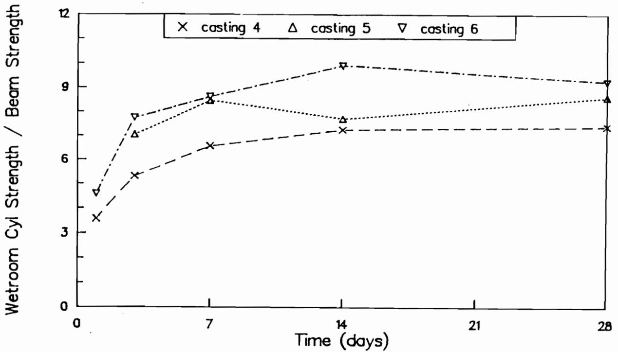
Fig B-23. Ratio of strengths of wetroom-cured cylinders to flexural strengths of wetroom-cured beams for castings 4, 5, and 6.
