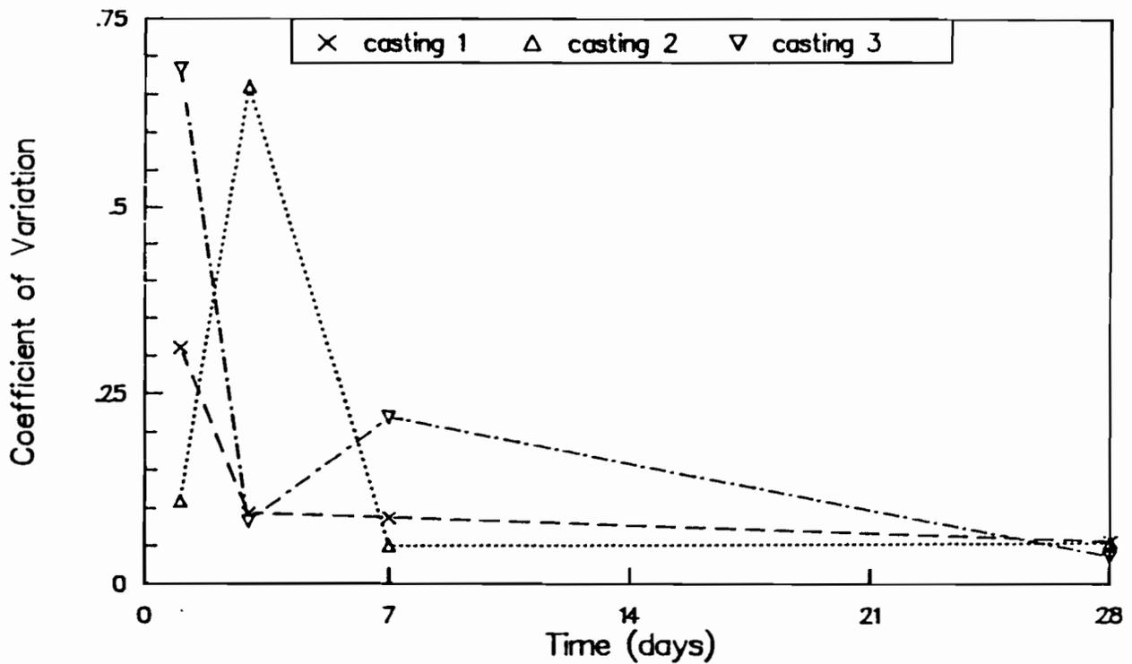
Fig A-17. Coefficient of variation of Windsor probe penetration resistance strengths for castings 1, 2, and 3.
