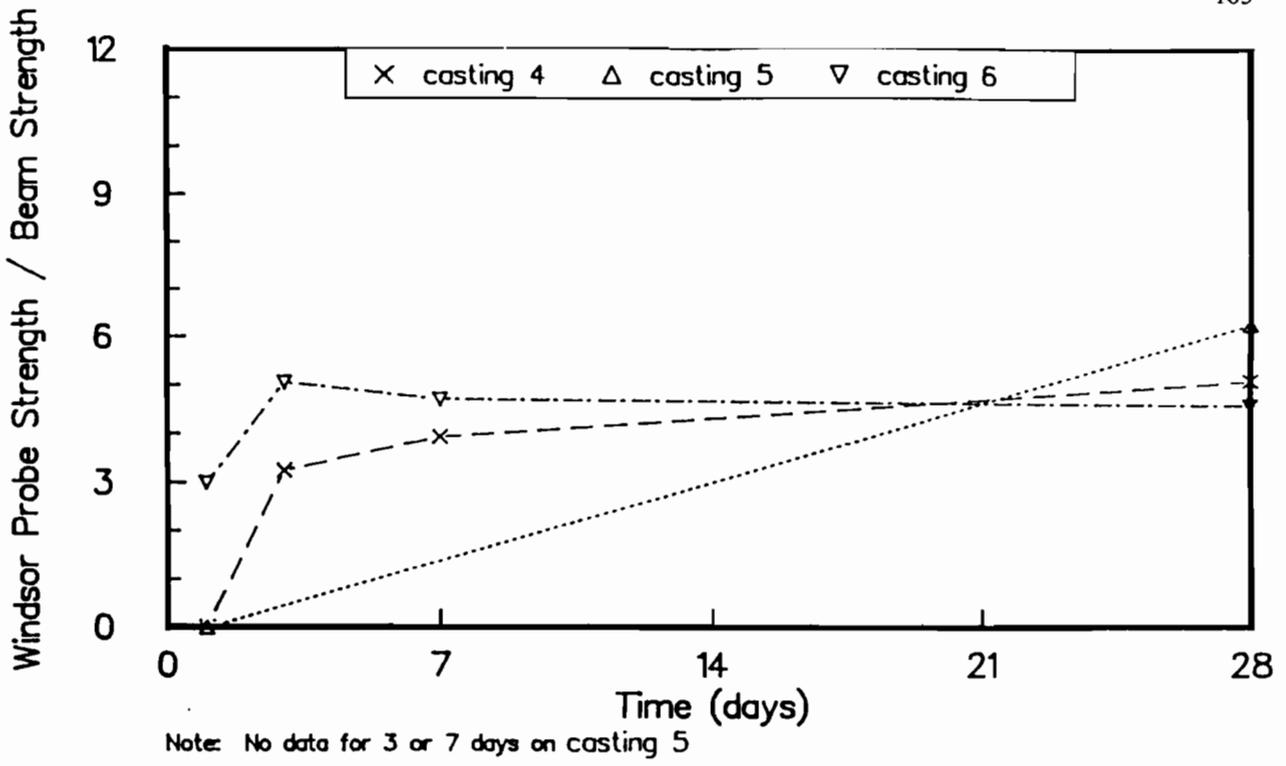
Fig B-28. Ratio of Windsor probe penetration resistance strengths to flexural strengths of wetroom-cured beams for castings 4, 5, and 6.
