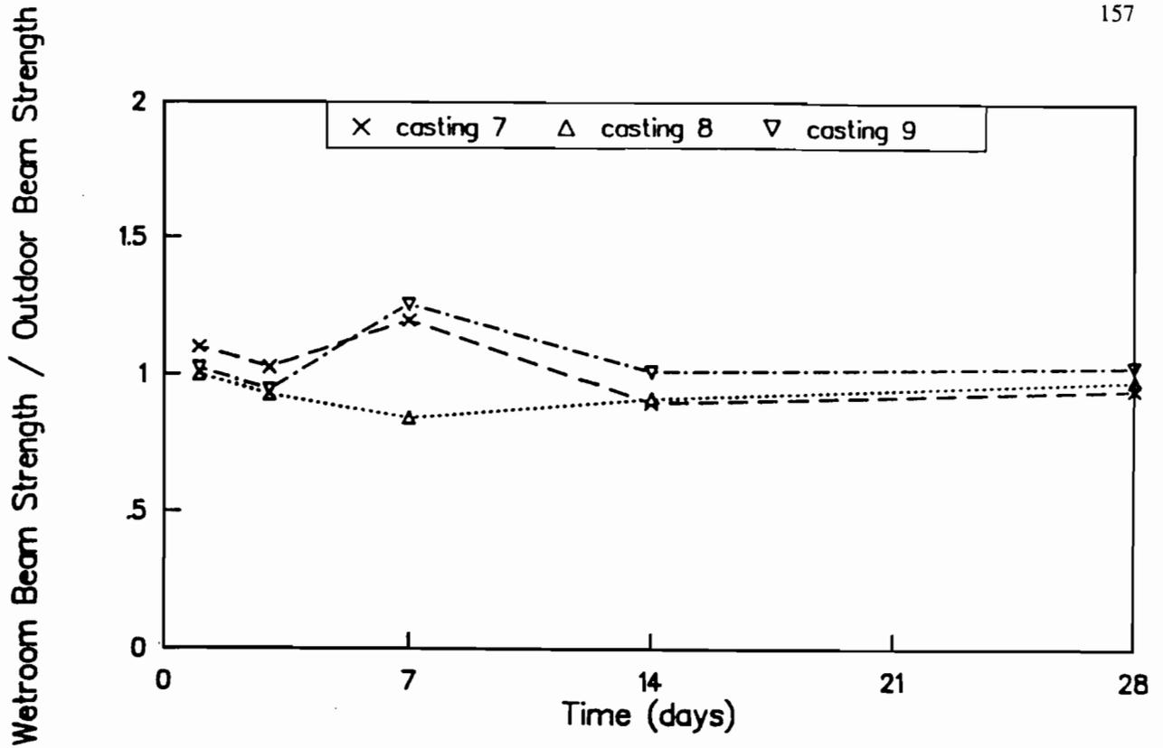
Fig C-37. Ratio of flexural strengths of wetroom-cured beams to flexural strengths of outdoor-cured beams for castings 7, 8, and 9.
