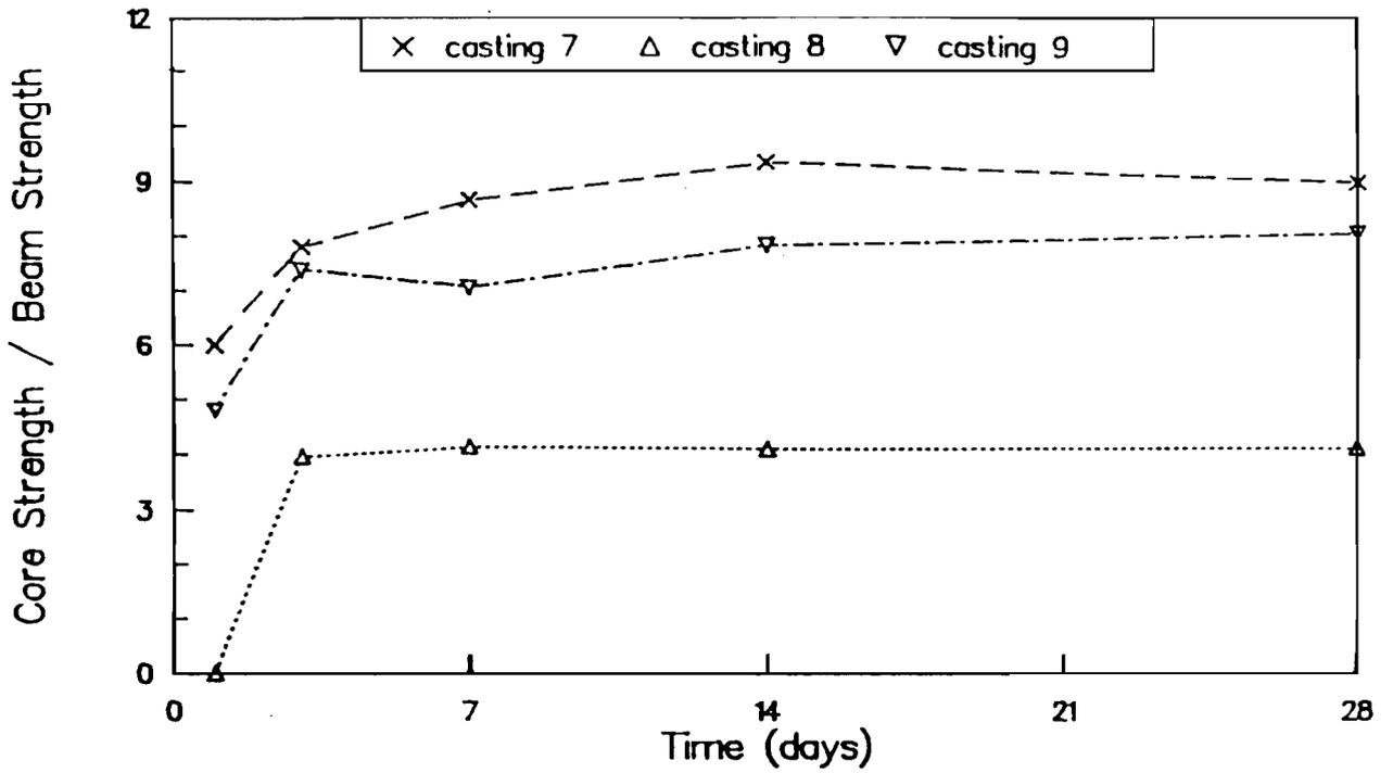
Fig C-25. Ratio of strengths of cores to flexural strengths of wetroom-cured beams for castings 7, 8, and 9.
