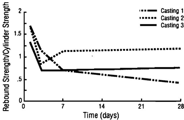
**Fig 5-6. Ratio of rebound hammer strengths to strengths of wetroom-cured cylinders for castings 1, 2, and 3.**
