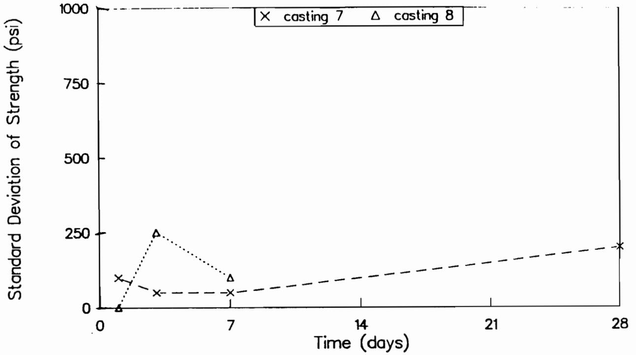
Fig C-63. Standard deviation of Windsor probe penetration resistance strengths for castings 7 and 8.
