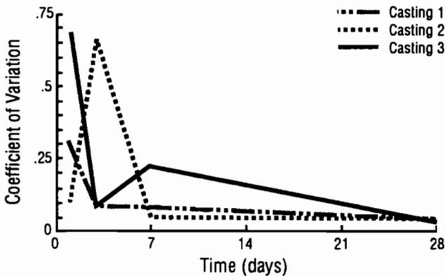
Fig 5-13. Coefficient of variation of Windsor probe penetration resistance strengths for castings 1, 2, and 3.
