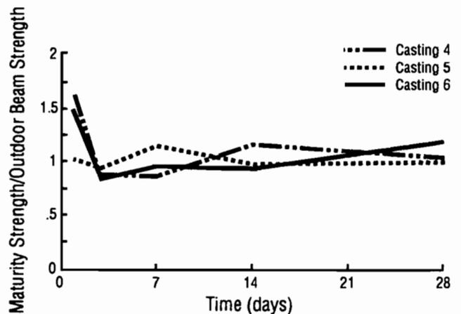
**Fig 5-23. Ratio of strength by maturity method to strength of outdoor-cured beams for castings 4, 5, and 6. Maturity curve based on outdoor-cured beams.**
