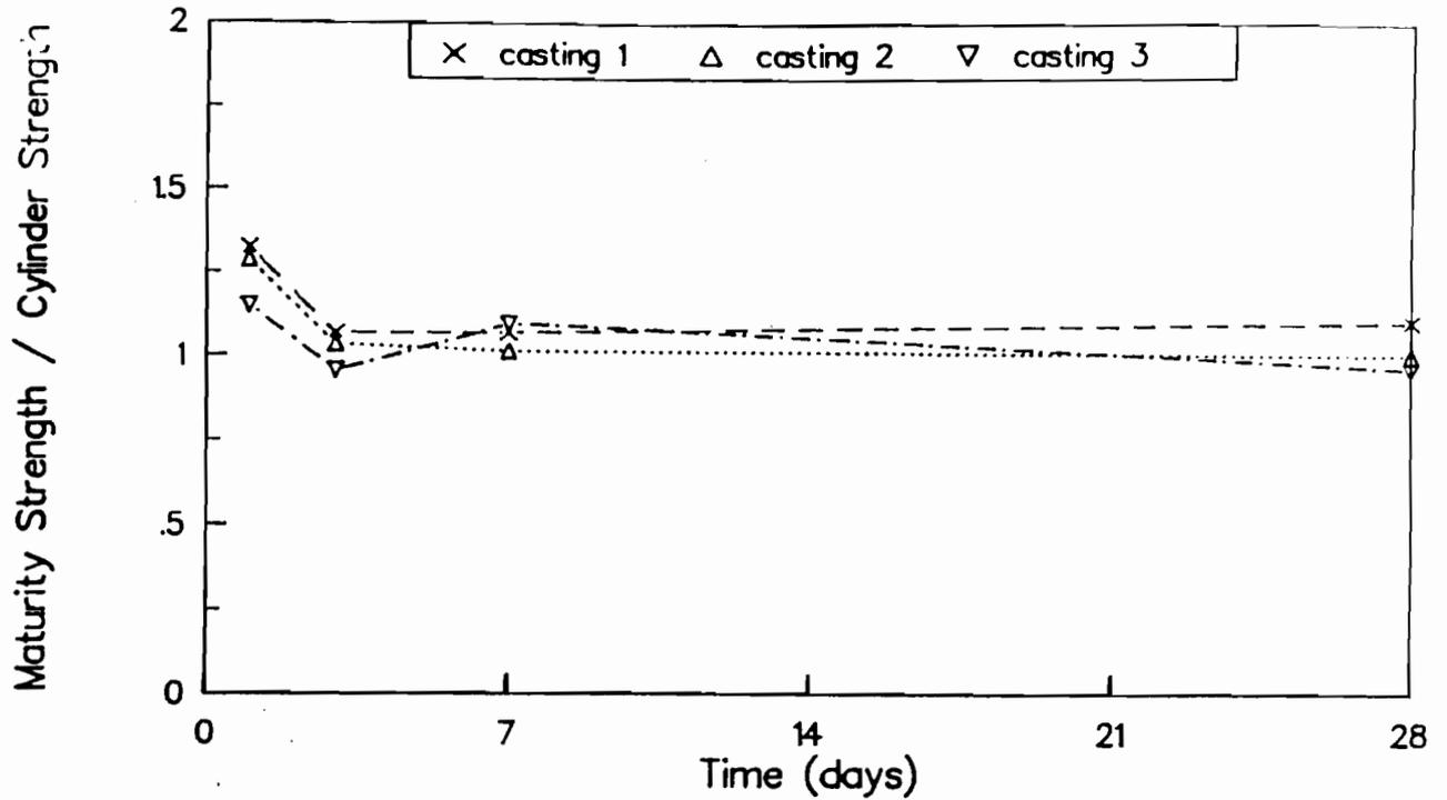
Fig A-6. Ratio of maturity method strengths to strengths of wetroom-cured cylinders for castings 1, 2, and 3.
