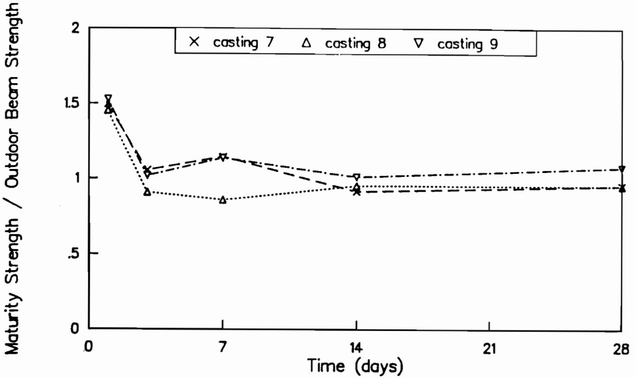
Fig C-43. Ratio of maturity method strengths to flexural strengths of outdoor-cured beams for castings 7, 8, and 9. Maturity curve based on wetroom-cured beams.
