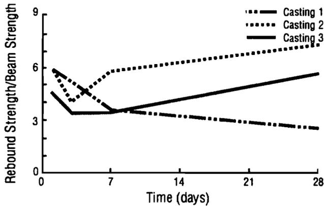
**Fig 5-7. Ratio of rebound number strength to flexural strength of wetroom-cured beams for castings 1, 2, and 3.**
