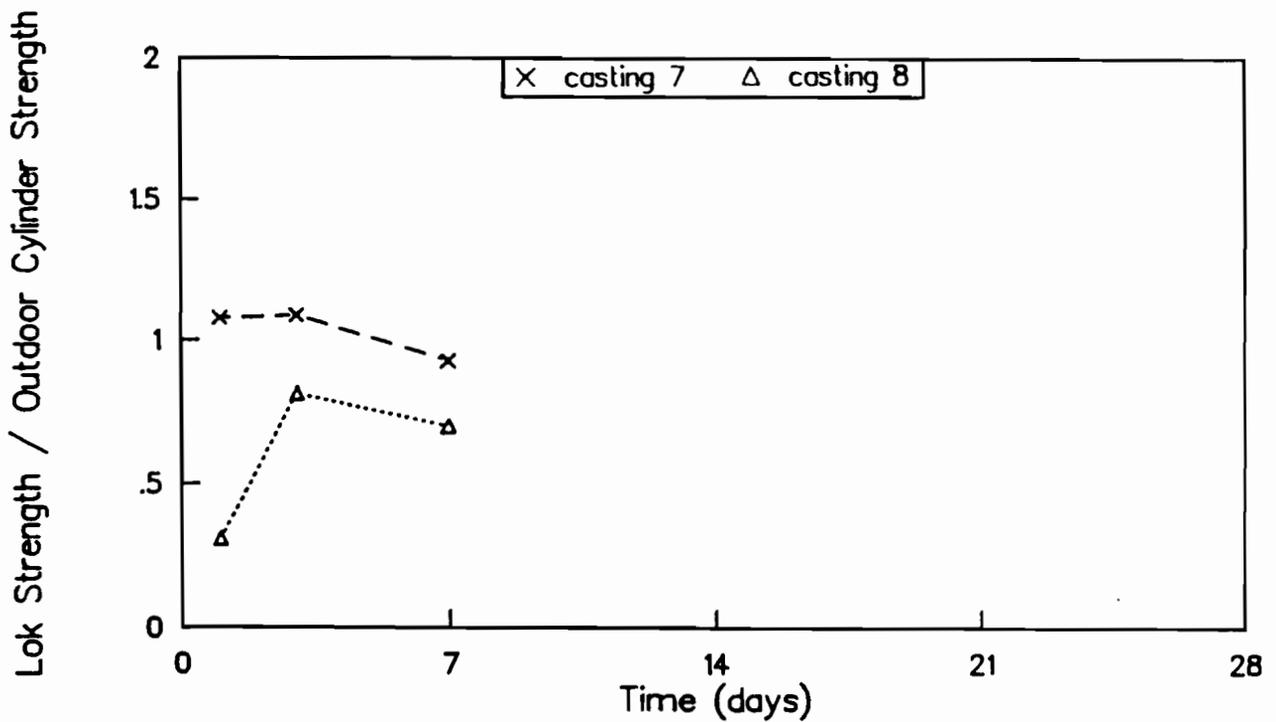
Fig C-16. Ratio of "Lok-Test" pullout strengths to strengths of outdoor-cured cylinders for castings 7 and 8.
