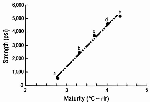
Fig 5-30. Relationship between logarithm of maturity and strength of wetroom-cured cylinders for casting 4.
