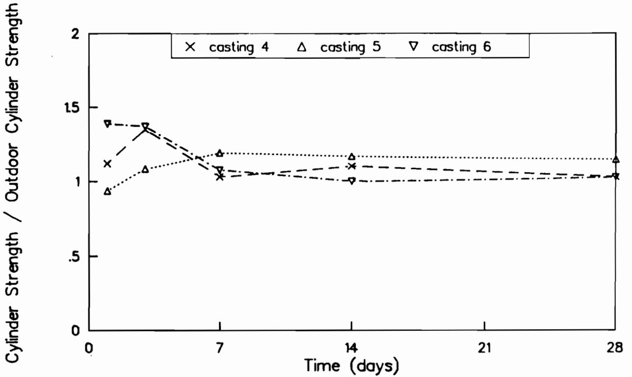
Fig B-12. Ratio of strengths of wetroom-cured cylinders to strengths of outdoor-cured cylinders for castings 4, 5, and 6.
