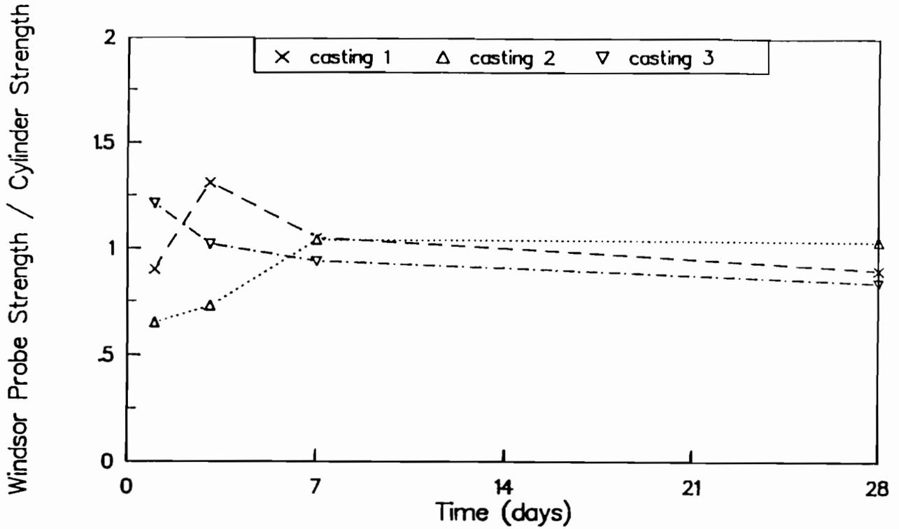
Fig A-4. Ratio of Windsor probe penetration resistance strengths to strengths of wetroom-cured cylinders for castings 1, 2, and 3.
