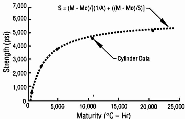
Fig 5-34. Comparison of hyperbolic prediction curve with actual cylinder maturities and strength.
