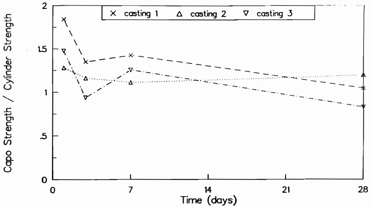
Fig A-2. Ratio of "CAPO-test" pullout strengths to strengths of wetroom-cured cylinders for castings 1, 2, and 3.
