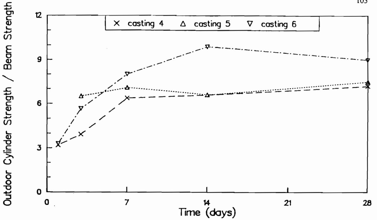
Fig B-24. Ratio of strengths of outdoor-cured cylinders to flexural strengths of wetroom-cured beams for castings 4, 5, and 6.
