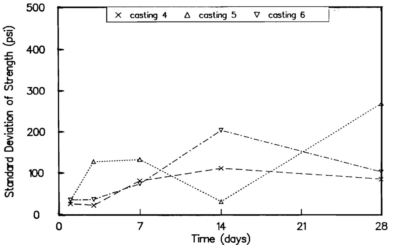
Fig B-57. Standard deviation of wetroom-cured cylinder strengths for castings 4, 5, and 6.
