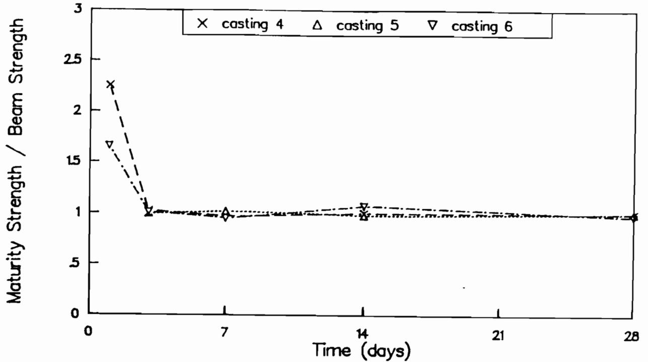
Fig B-32. Ratio of maturity method strengths to flexural strengths of wetroom-cured beams for castings 4, 5, and 6. Maturity curve based on wetroom-cured beams.
