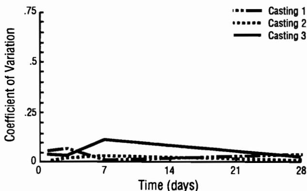
Fig 5-5. Coefficient of variation of wetroom-cured cylinder strengths for castings 1, 2, and 3.
