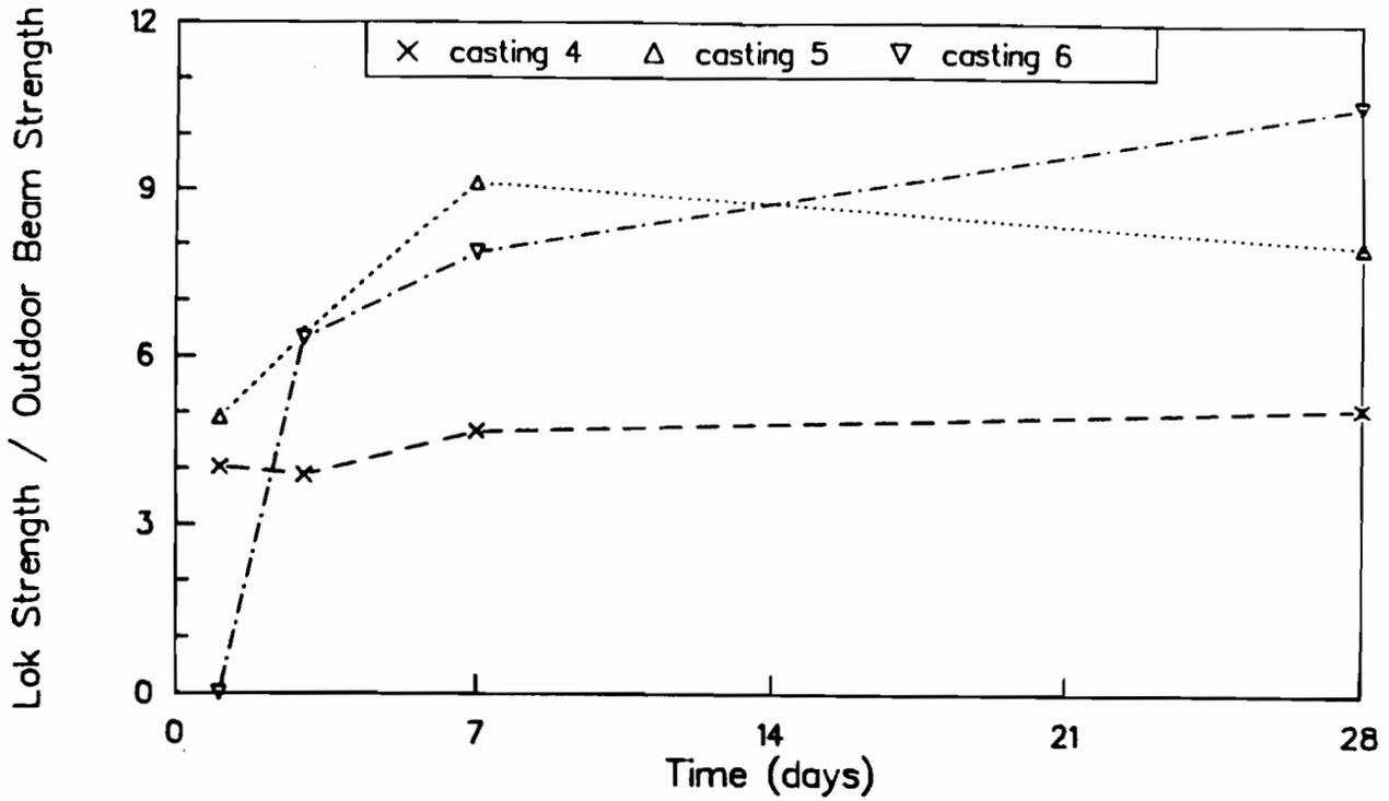
Fig B-38. Ratio of "Lok-Test" pullout strengths to flexural strengths of outdoor-cured beams for castings 4, 5, and 6.
