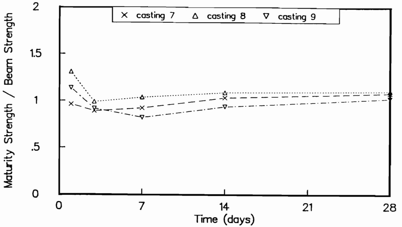
Fig C-33. Ratio of maturity method strengths to flexural strengths of wetroom-cured beams for castings 7, 8, and 9. Maturity curve based on outdoor-cured beams.
