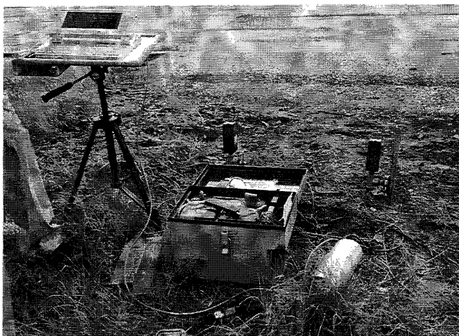
Fig 2.12. Traffic data acquisition system equipment.
