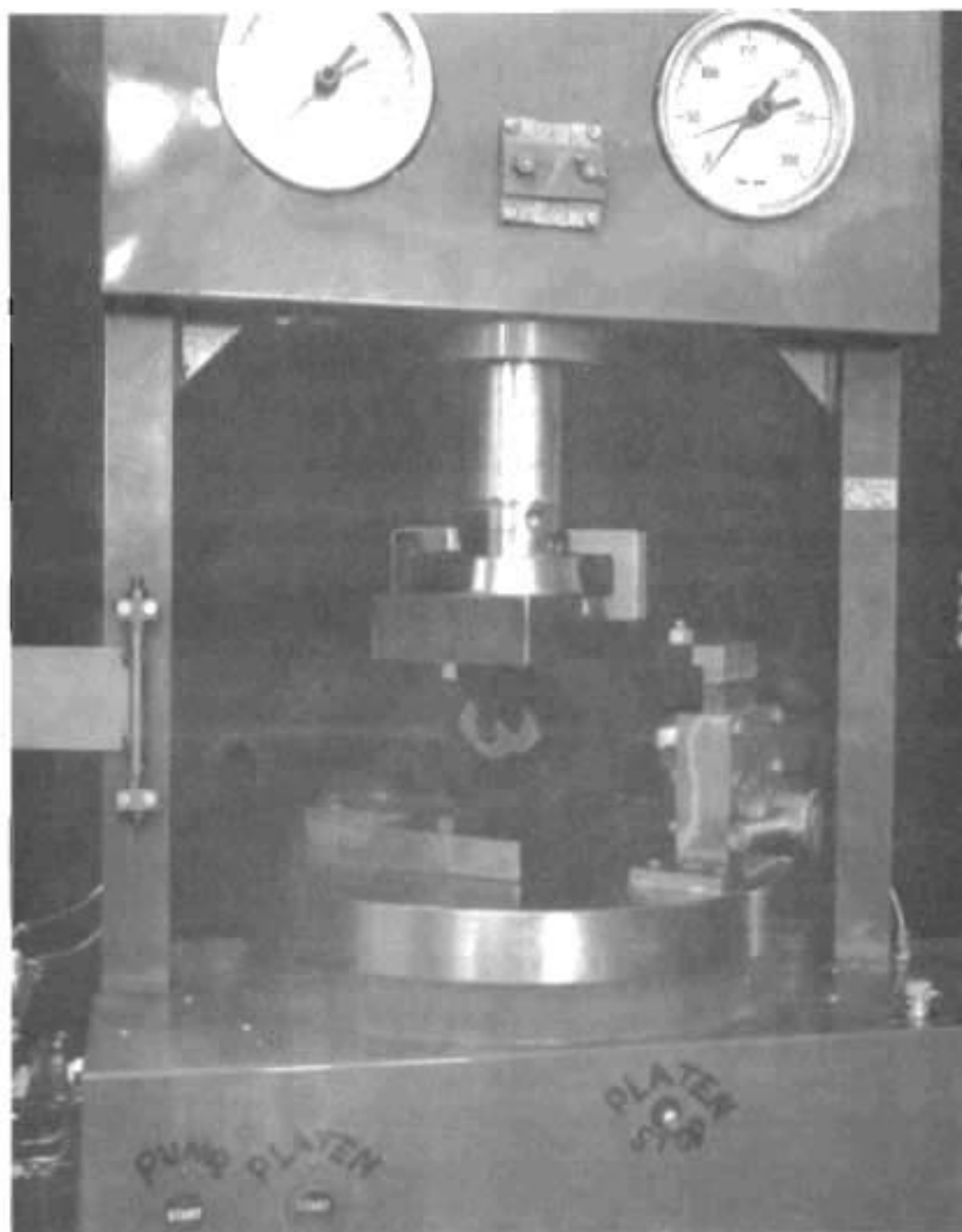
Fig 7. Motorized gyratory press with upper and lower loading plates and strips.
