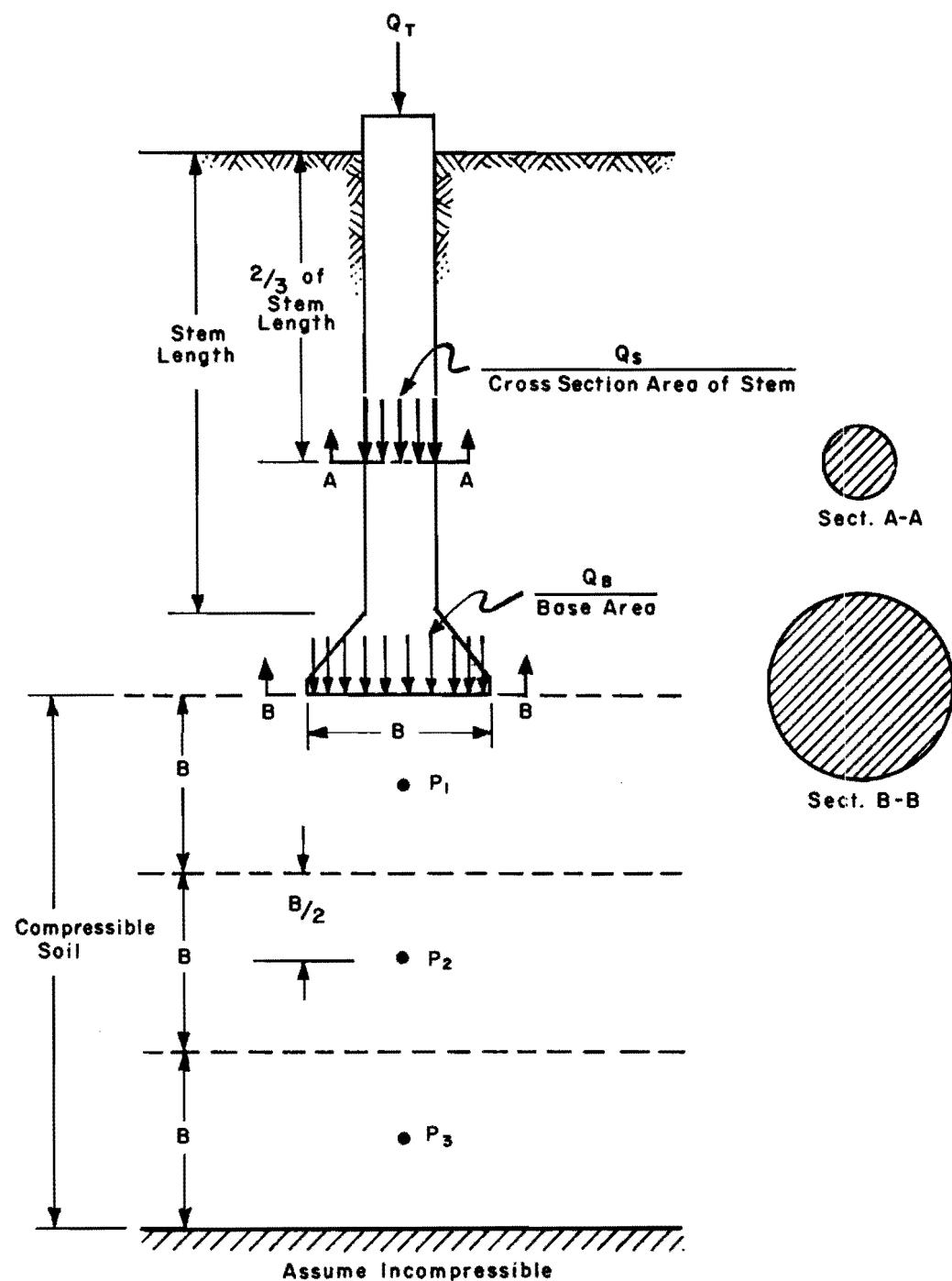
Fig. 4.5. Idealization of Shaft-Soil System for Settlement Computations
