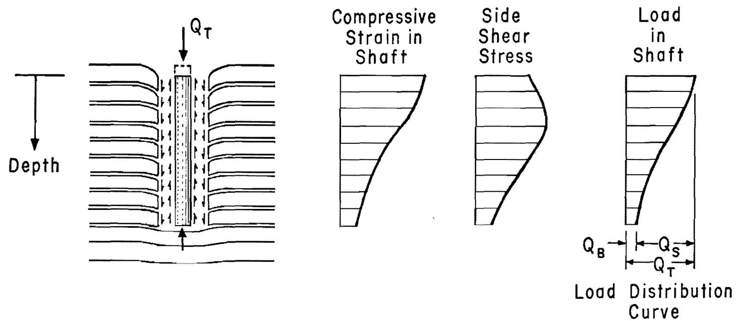
Fig. 3.1. Action of Drilled Shaft-Soil System Under Axial Load
