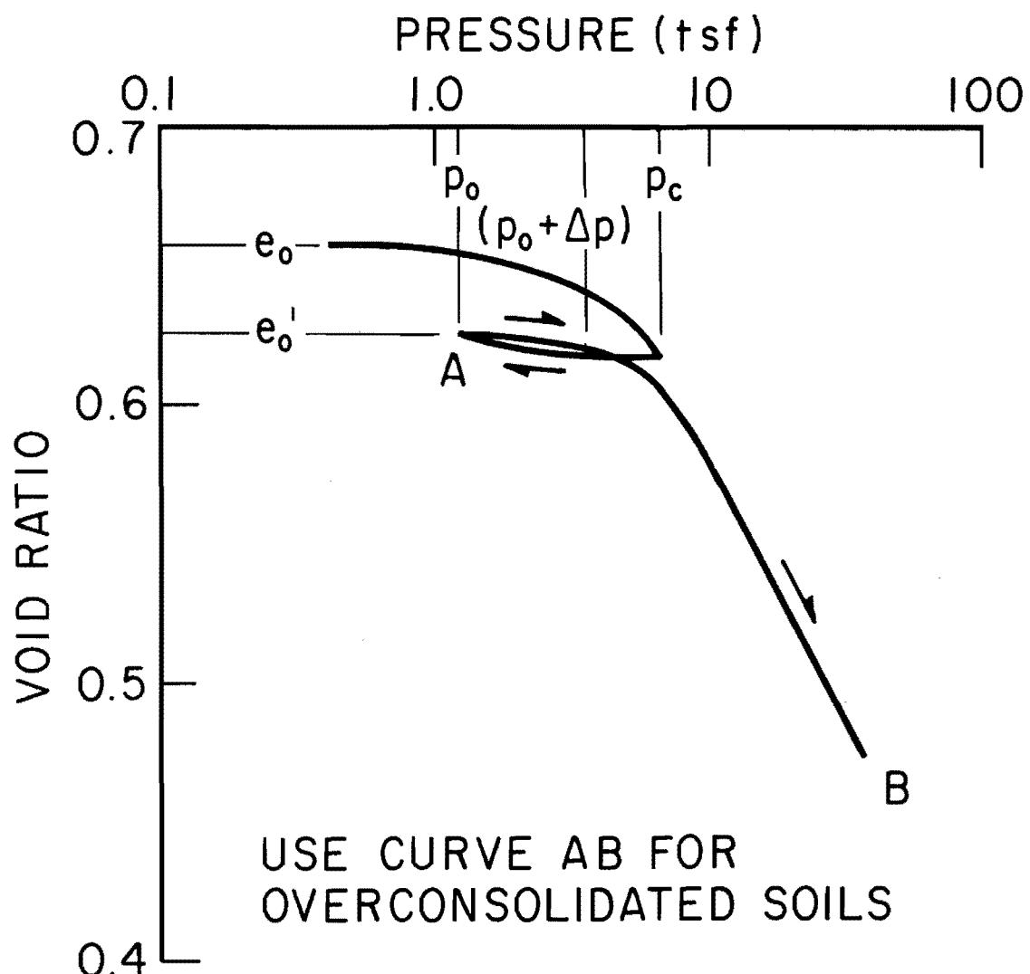
Fig. 4.6. Cyclic  $e$ -log  $p$  Curve for Use in Computing Settlements in Overconsolidated Clays
