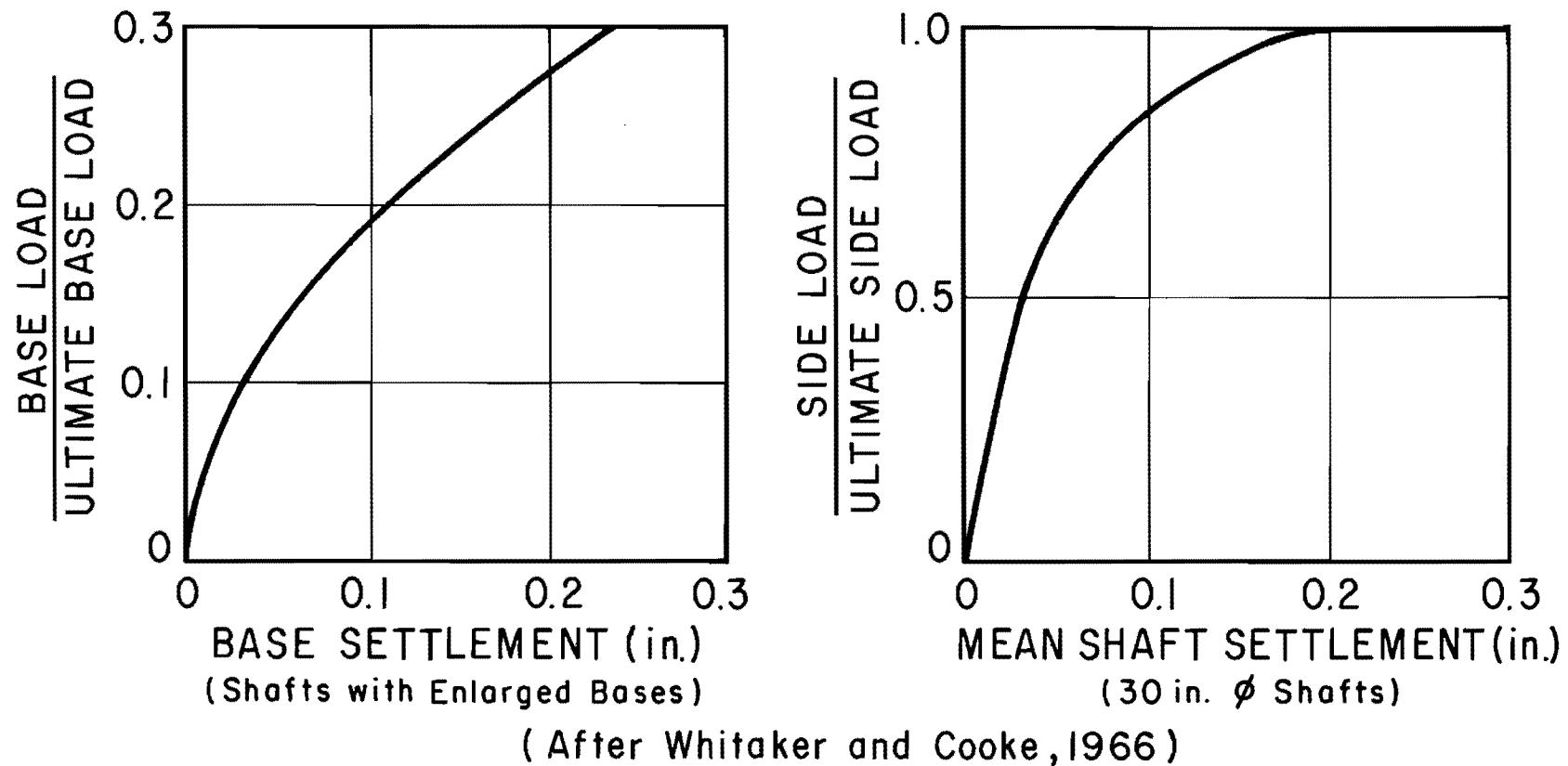
Fig. 4.4. Normalized Side and Base Load-Settlement Curves for 30-Inch Shafts in London Clay
