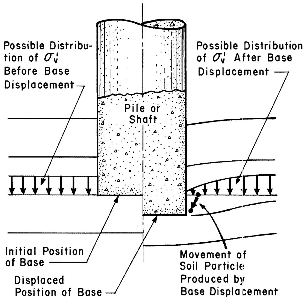
Fig. 4.1. Action of Soil Near Base of Drilled Shaft
