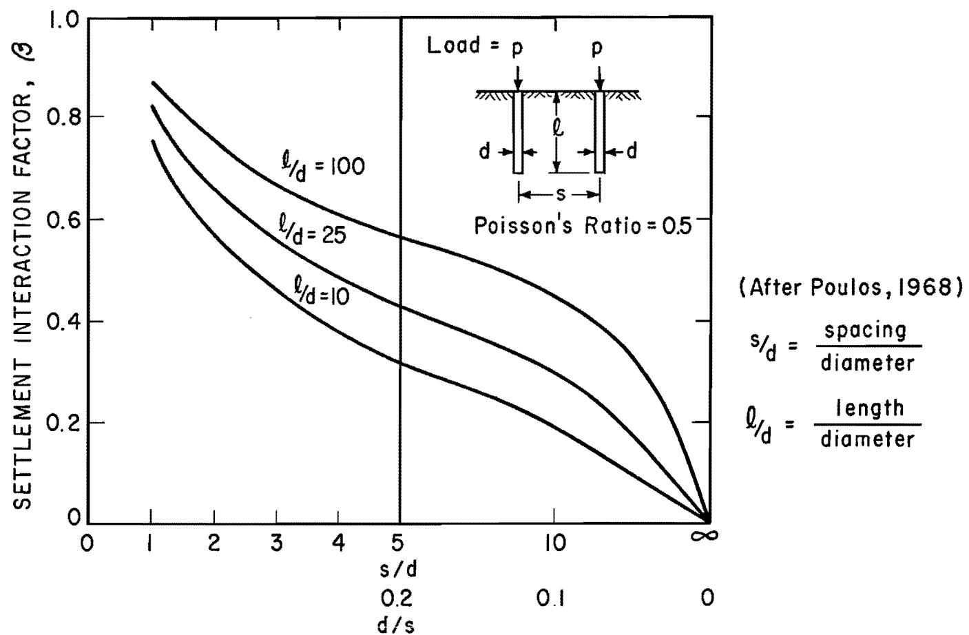
Fig. 4.7. Settlement Interaction Between Two Shafts or Piles in a Semi-Infinite, Elastic Mass
