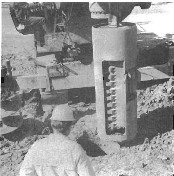
b. Belling Tool in Closed Position
