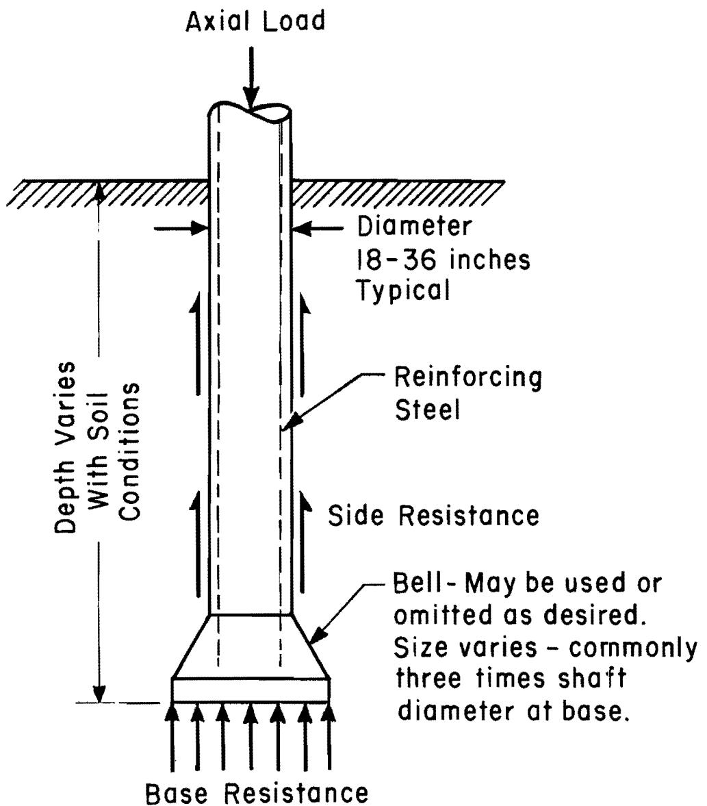
Fig. 1.1. Typical Drilled Shaft
