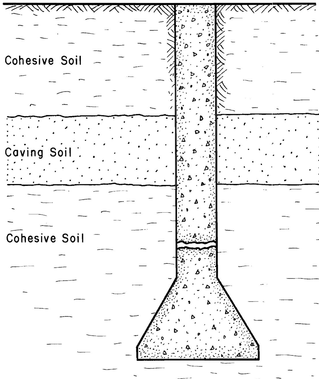
Fig. 2.5. Separated Shaft
