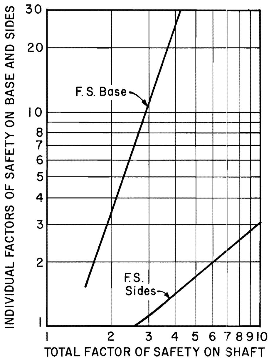
Fig. 3.5. Relationship Between Base, Side, and Total Factors of Safety on a Drilled Shaft
