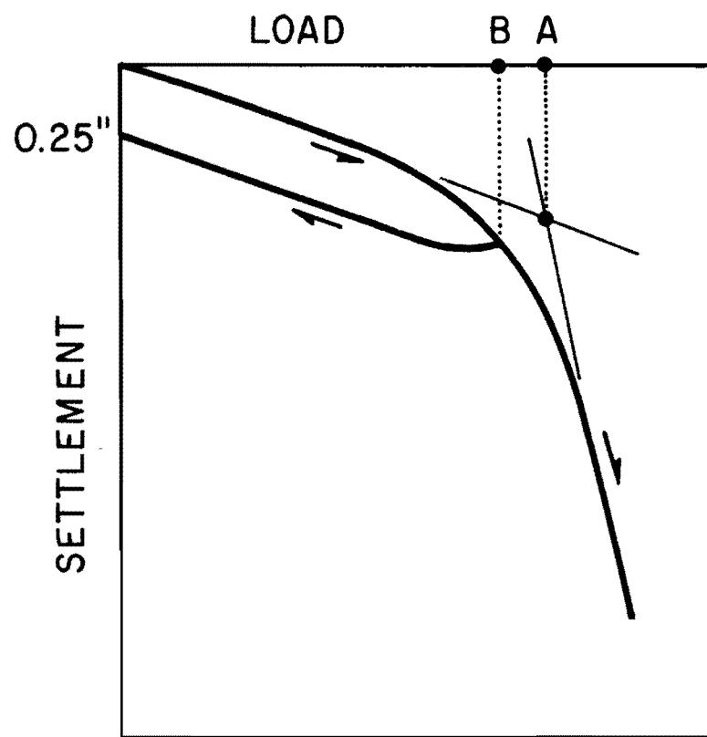
Fig. 4.3. Methods of Estimating Failure Load
