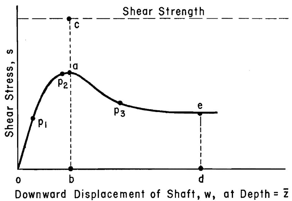
Fig. 3.3. Load Transfer Curve
