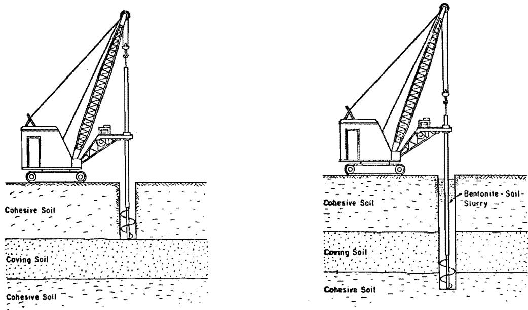
a. Dry Drilling Through Cohesive Soil
