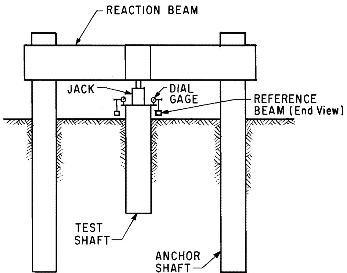
Fig. 4.2. Typical Arrangement for Testing a Drilled Shaft
