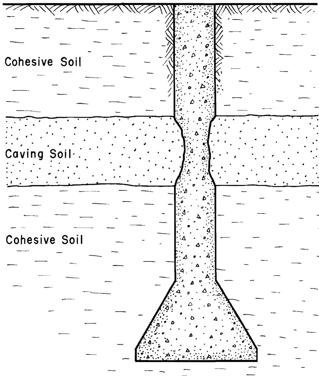
Fig. 2.4. Shaft with Necked Section
