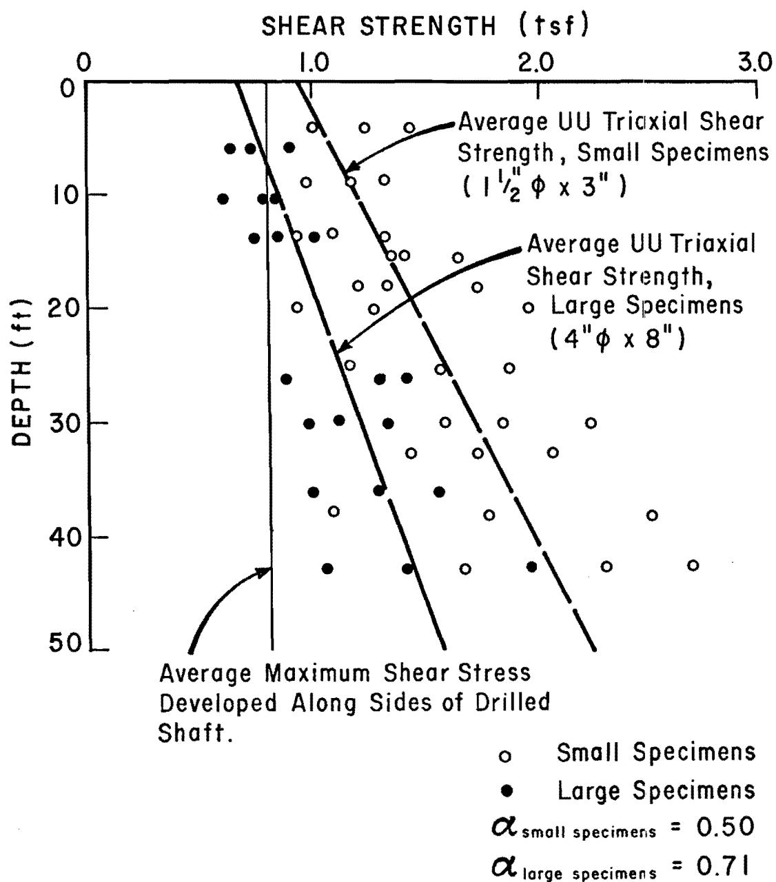
Fig. 5.1. Hypothetical Comparison of Average Shear Strengths Indicated by Tests on Small Specimens and on Large Specimens
