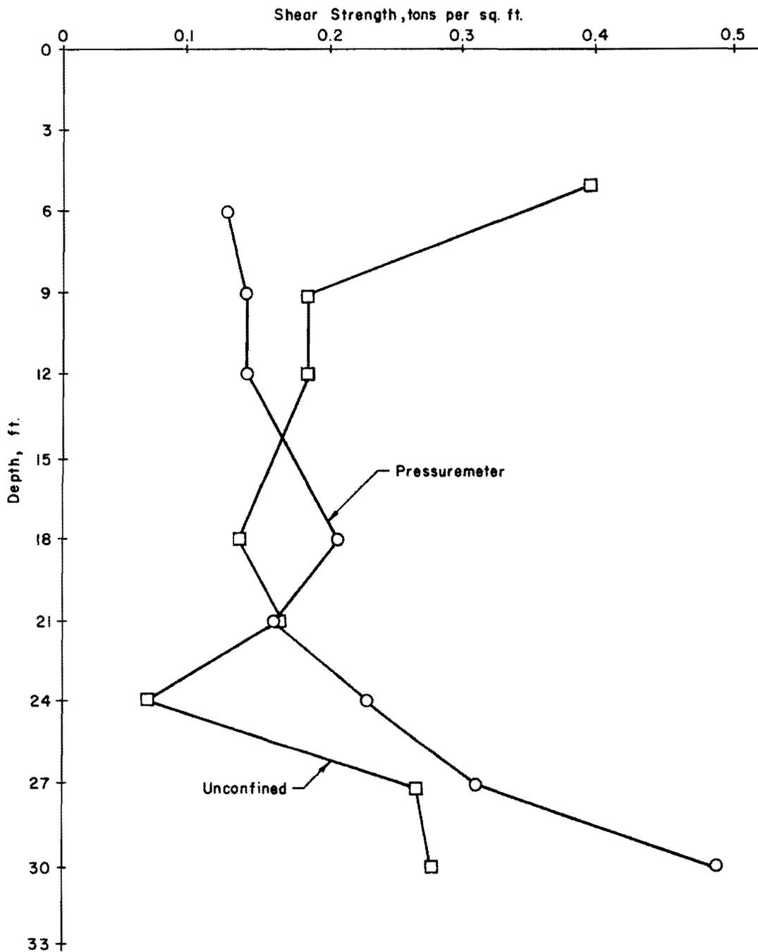
Fig. 2.3. Comparison of Shear Strengths Obtained by Menard Pressuremeter and Unconfined Compression Tests, Plaquemine Test Site (After Higgins)
