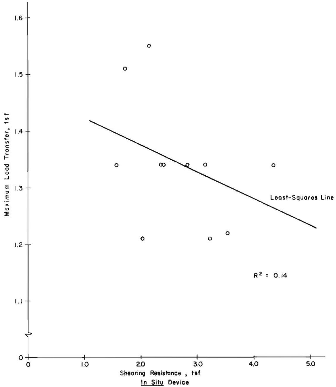
Fig. 5.6. Correlation of Load Transfer and Shearing Resistances Measured with UT In Situ Device, Montopolis Site
