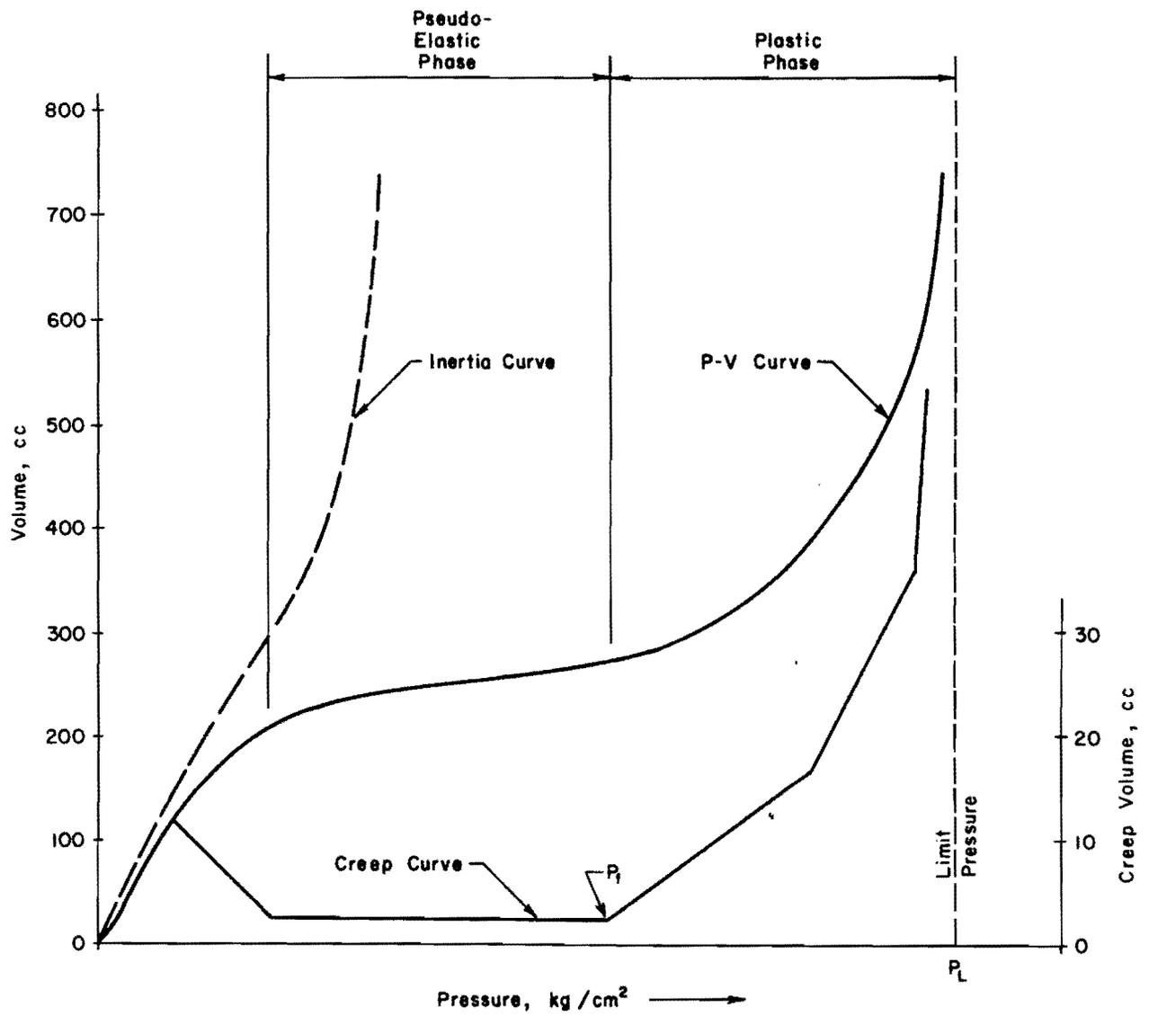
Fig. 2.2. Curves Derived from Menard Pressuremeter Data
