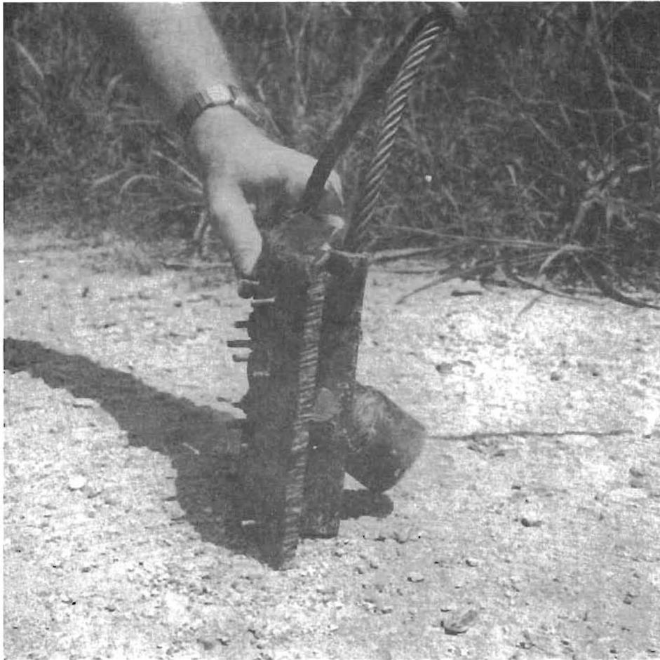
Fig. 4.2. Shear Plate for UT In Situ Device
