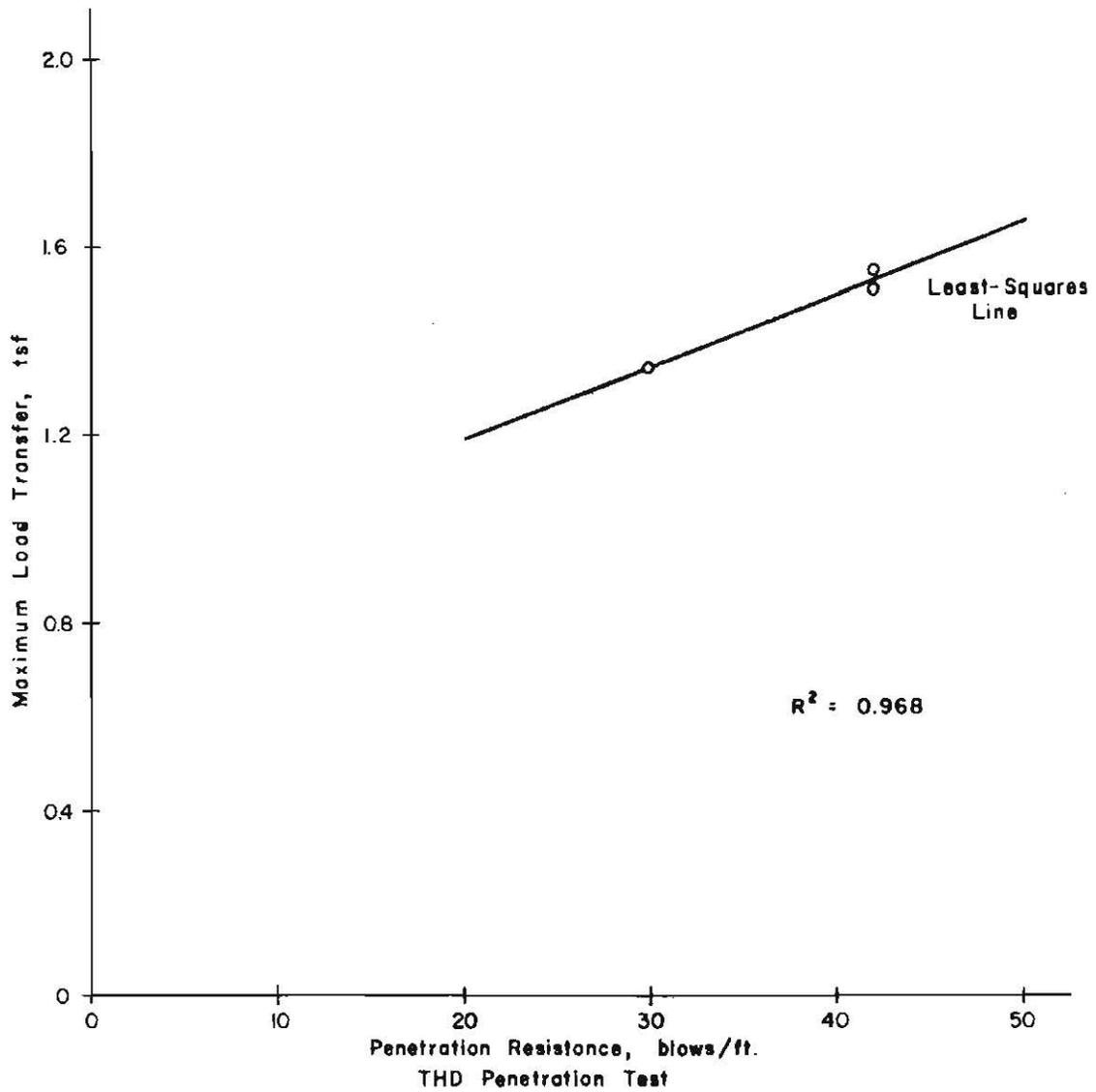
Fig. 5.8. Correlation of Load Transfer and Penetration Resistance, Montopolis Site
