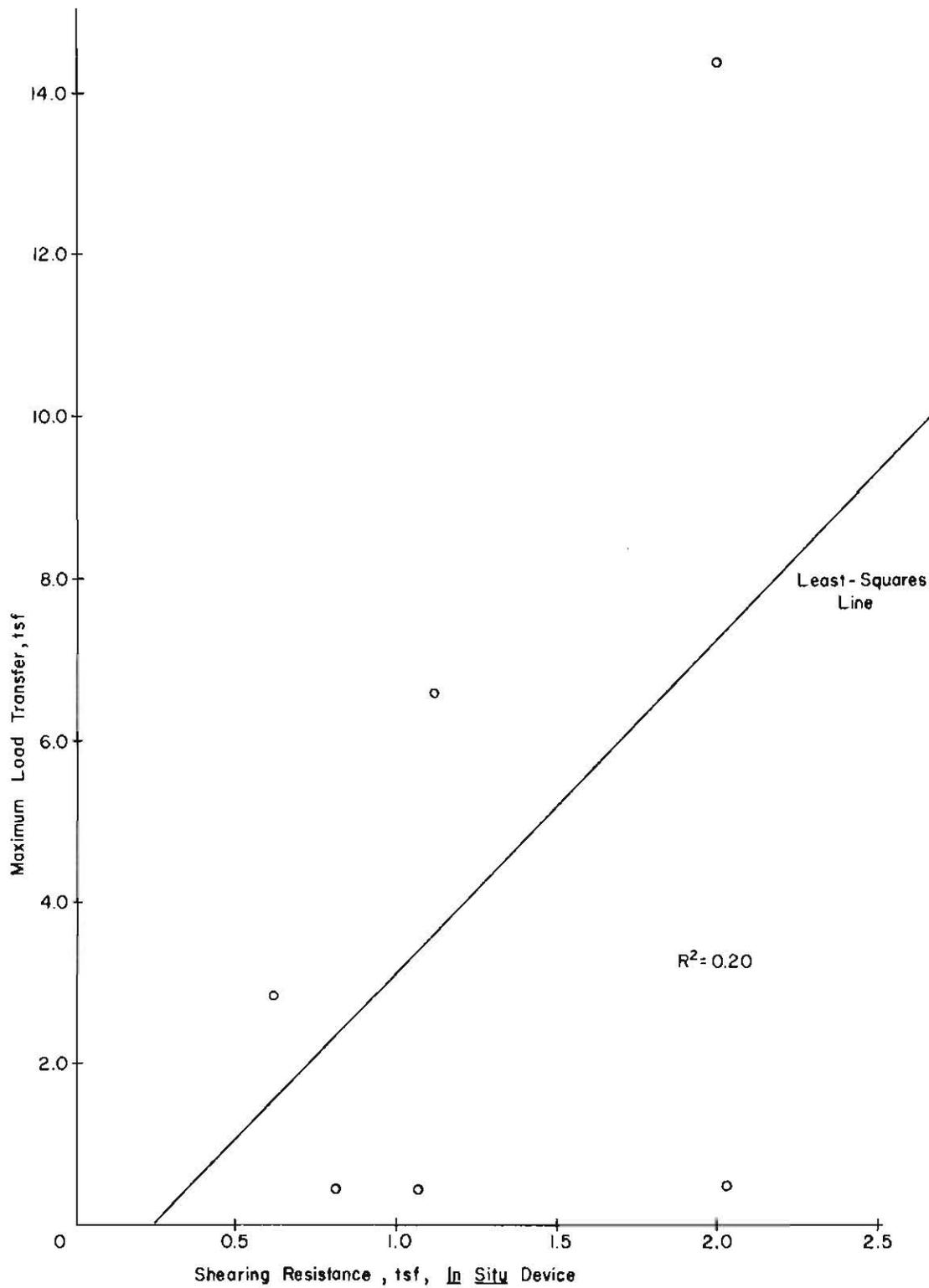
Fig. 5.7. Correlation of Load Transfer and Shearing Resistances Measured with UT In Situ Device, San Antonio Site
