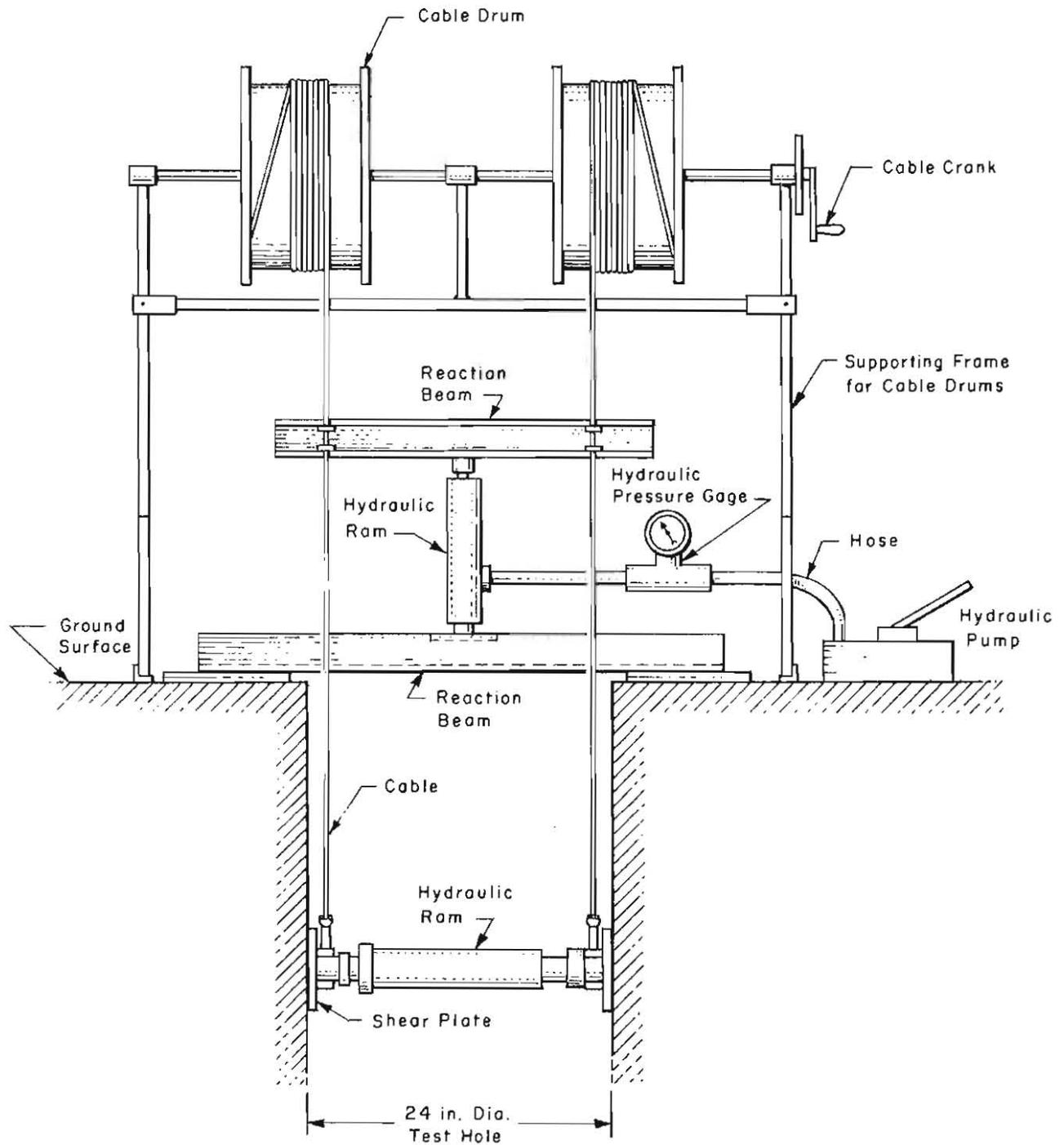
Fig. 4.4. Pull-out System for UT In Situ Device
