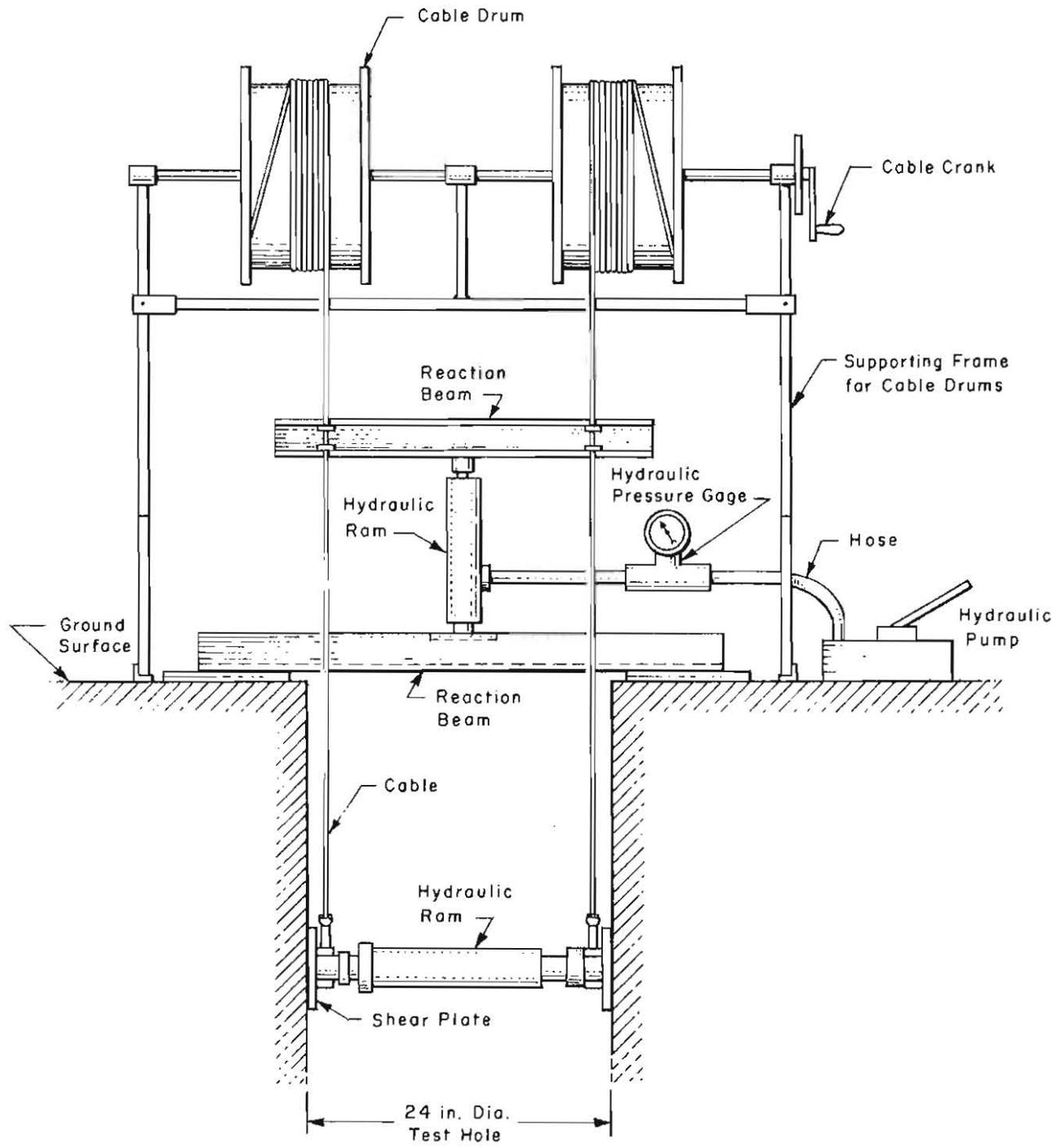
Fig. 4.4. Pull-out System for UT In Situ Device
