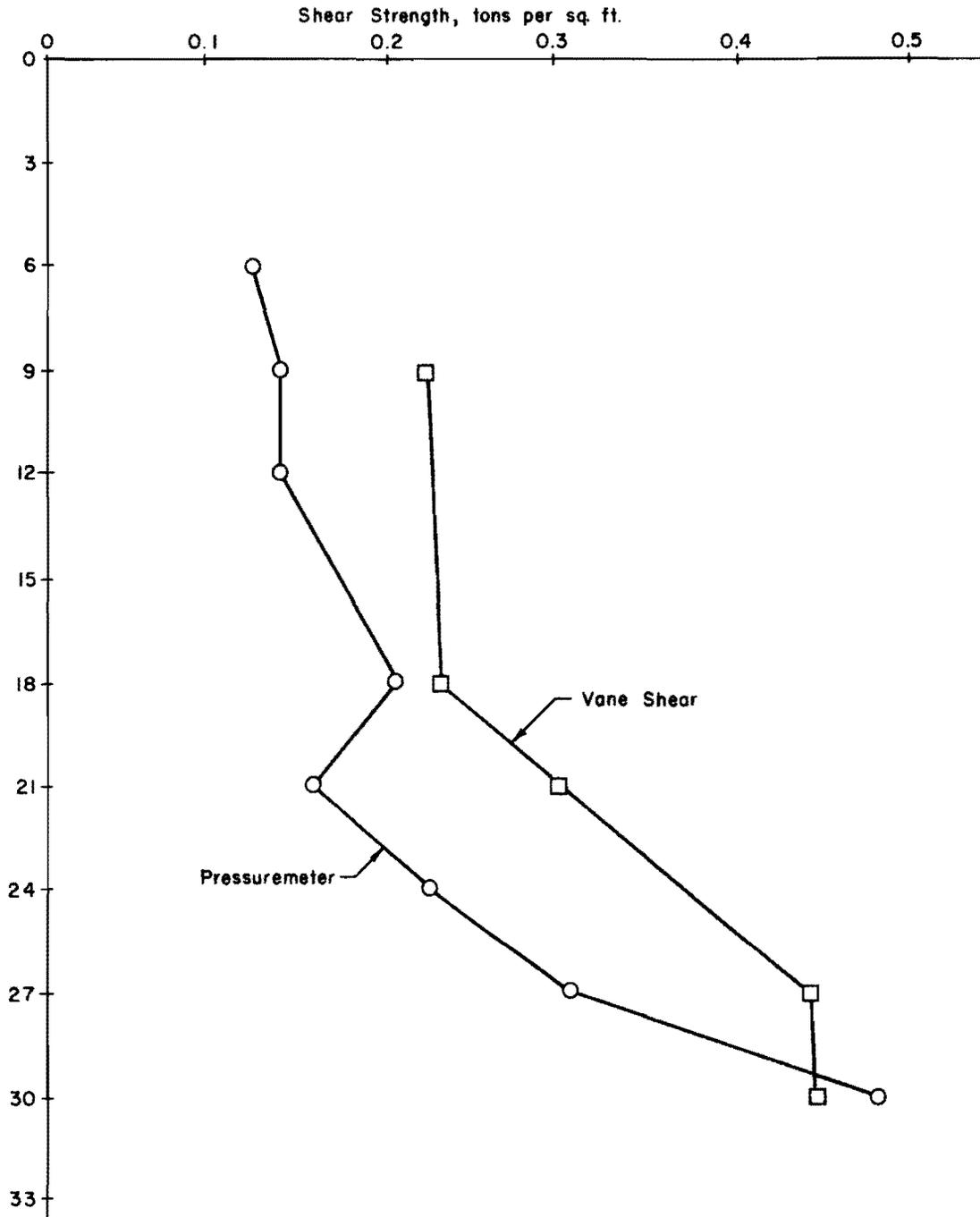
Fig. 2.4. Comparison of Shear Strengths Obtained by Menard Pressuremeter and Vane Shear Tests, Plaquemine Test Site (After Higgins)
