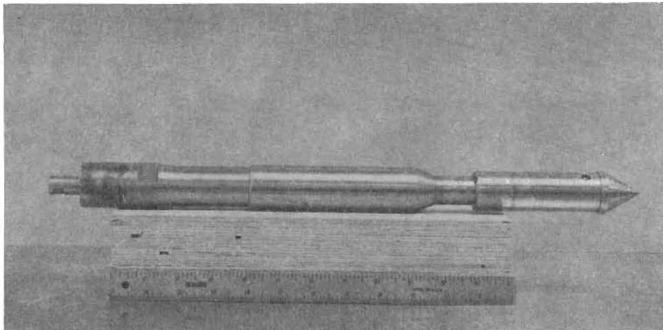
Fig. 3.1. Dutch Cone Penetrometer
