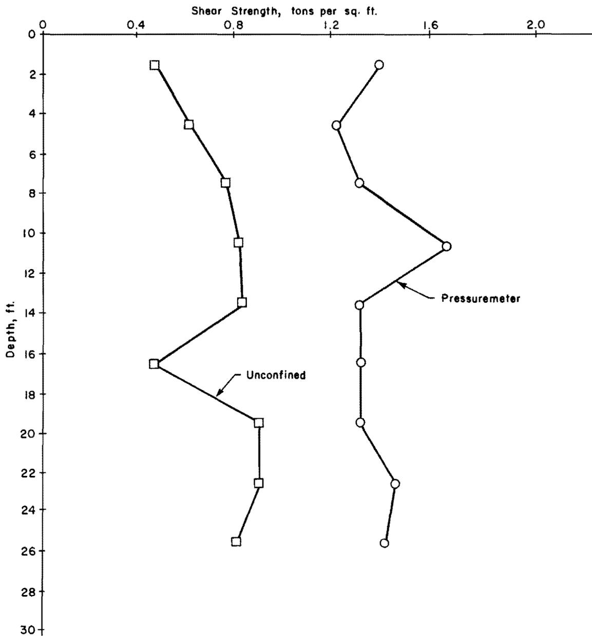
Fig. 2.5. Comparison of Shear Strengths Obtained by Menard Pressuremeter and Unconfined Compression Tests, Lake Charles Test Site (After Higgins)
