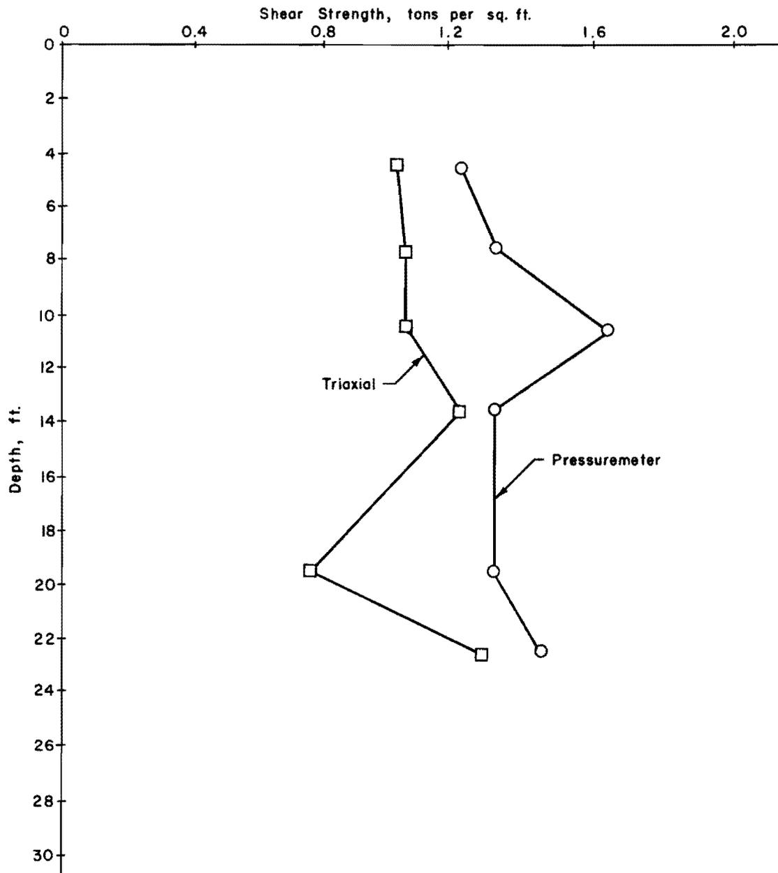
Fig. 2.6. Comparison of Shear Strengths Obtained by Menard Pressuremeter and Triaxial Tests, Lake Charles Test Site (After Higgins)
