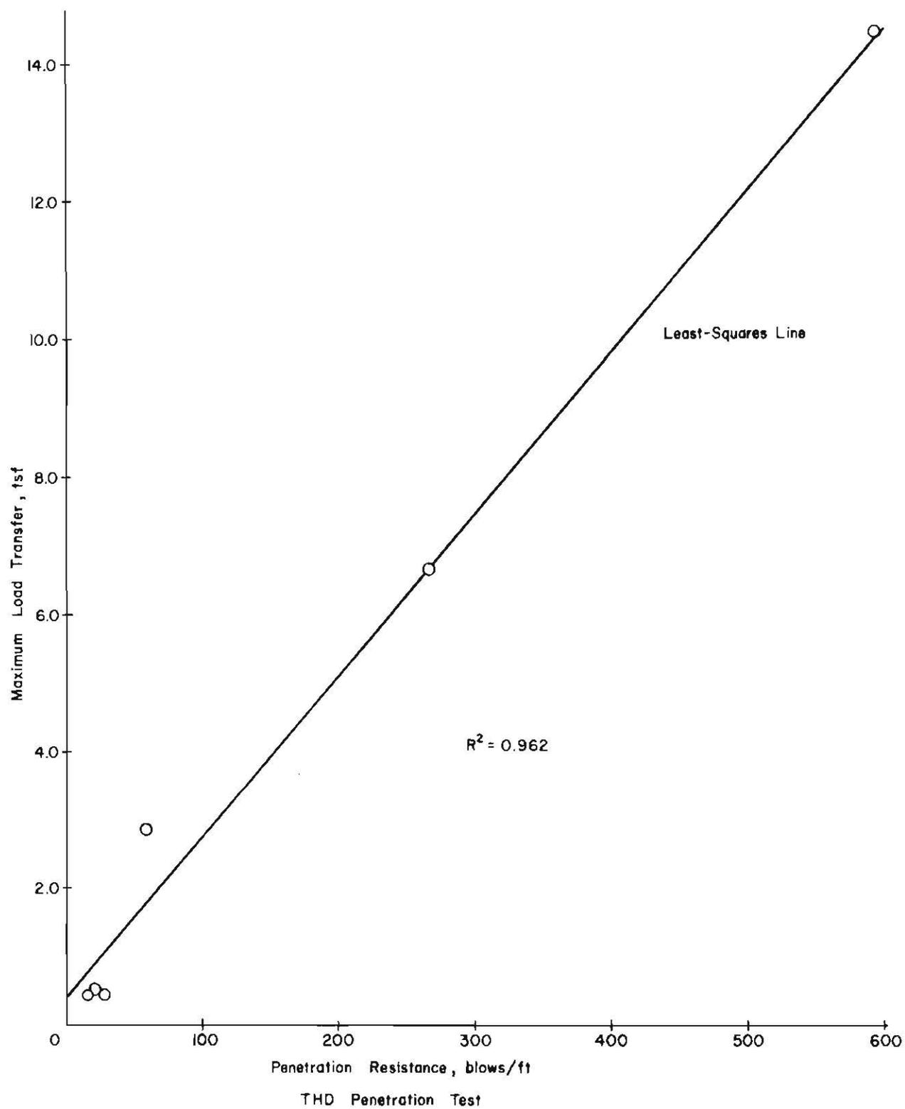
Fig. 5.9. Correlation of Load Transfer and Penetration Resistance, San Antonio Site
