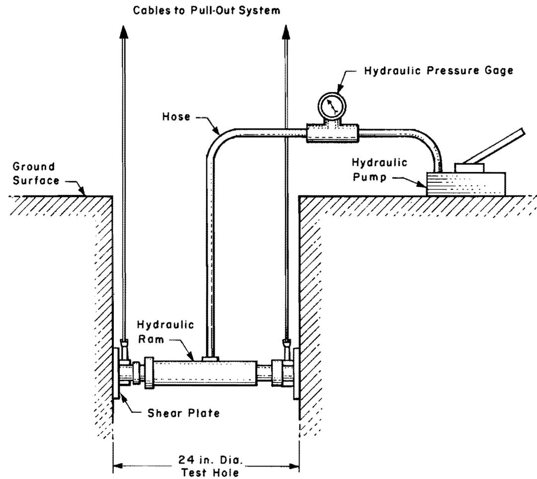
Fig. 4.3. Normal Force System for UT In Situ Device
