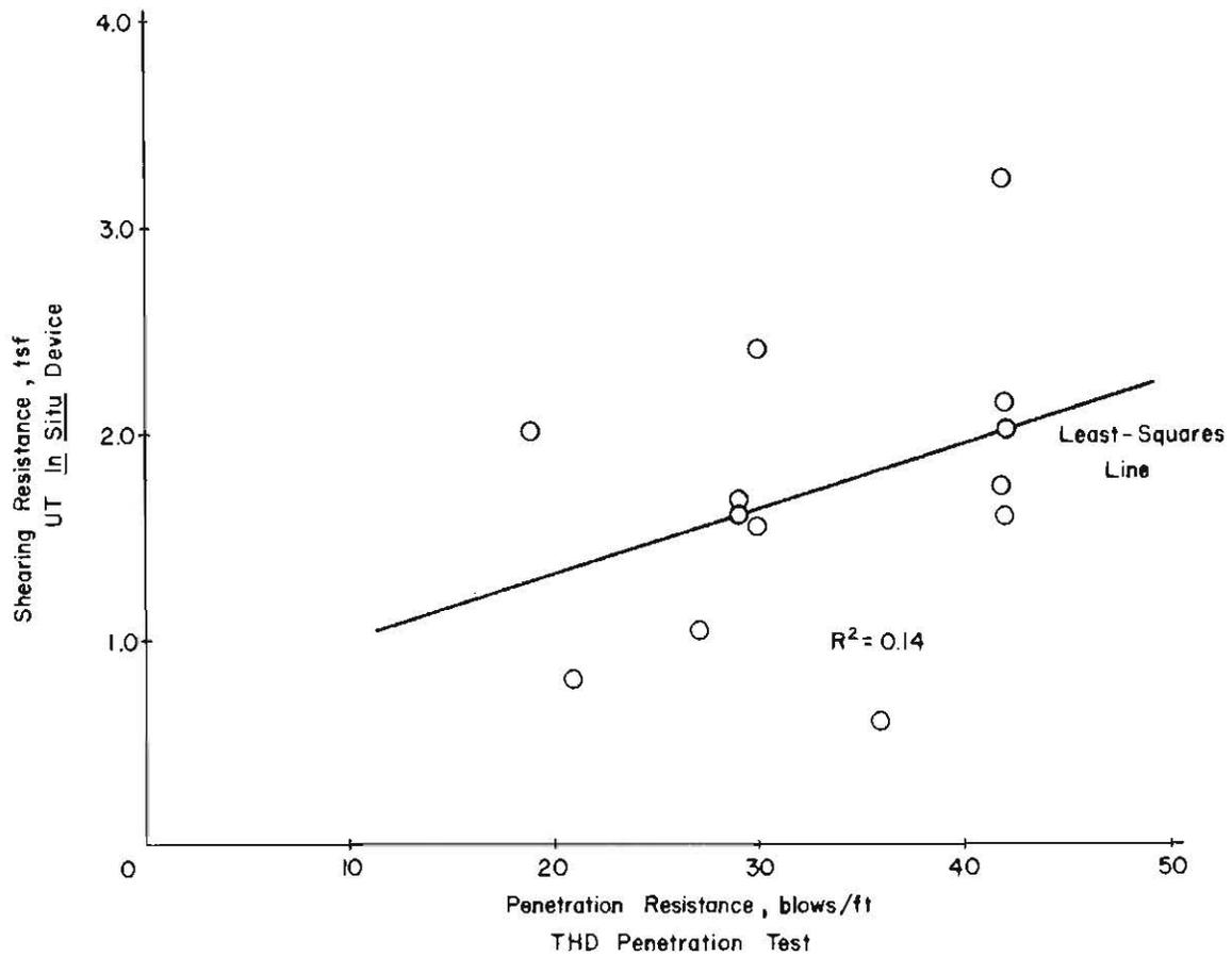
Fig. 5.5. Correlation of Shearing Resistances Measured with UT In Situ Device and Penetration Resistance Measured by THD Penetrometer, Montopolis and San Antonio Sites
