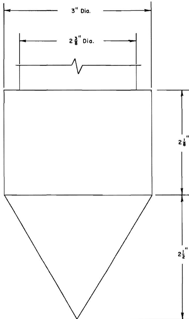
Fig. 3.5. Details of THD Cone Penetrometer
