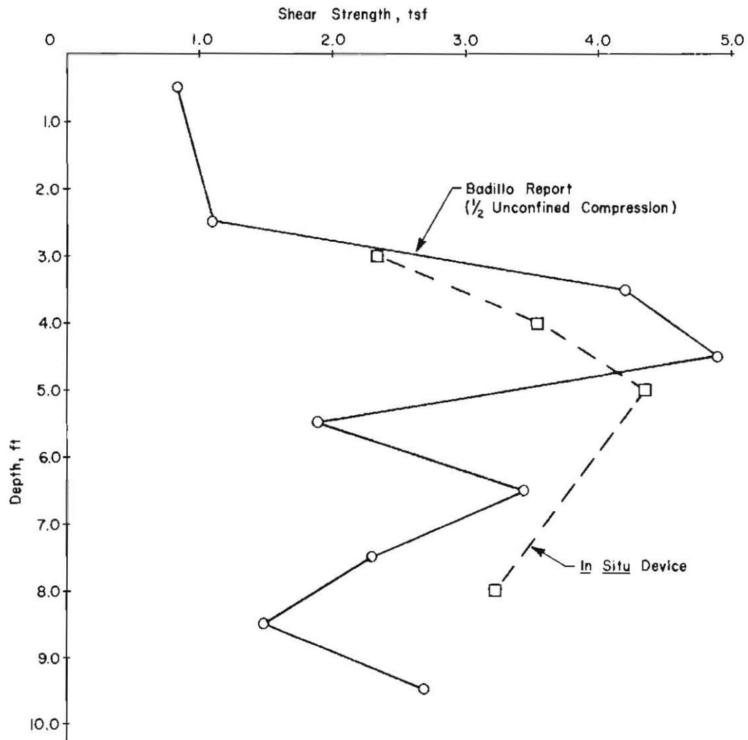
Fig. 5.2. Comparison of Shearing Resistances Measured with UT In Situ Device and One-half Unconfined Compression Tests Results, Montopolis Site
