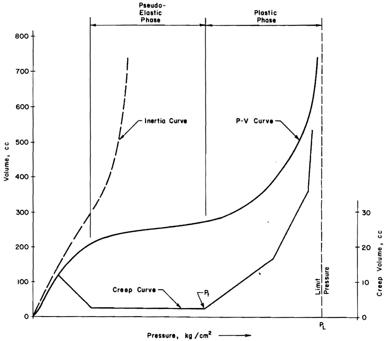
Fig. 2.2. Curves Derived from Menard Pressuremeter Data
