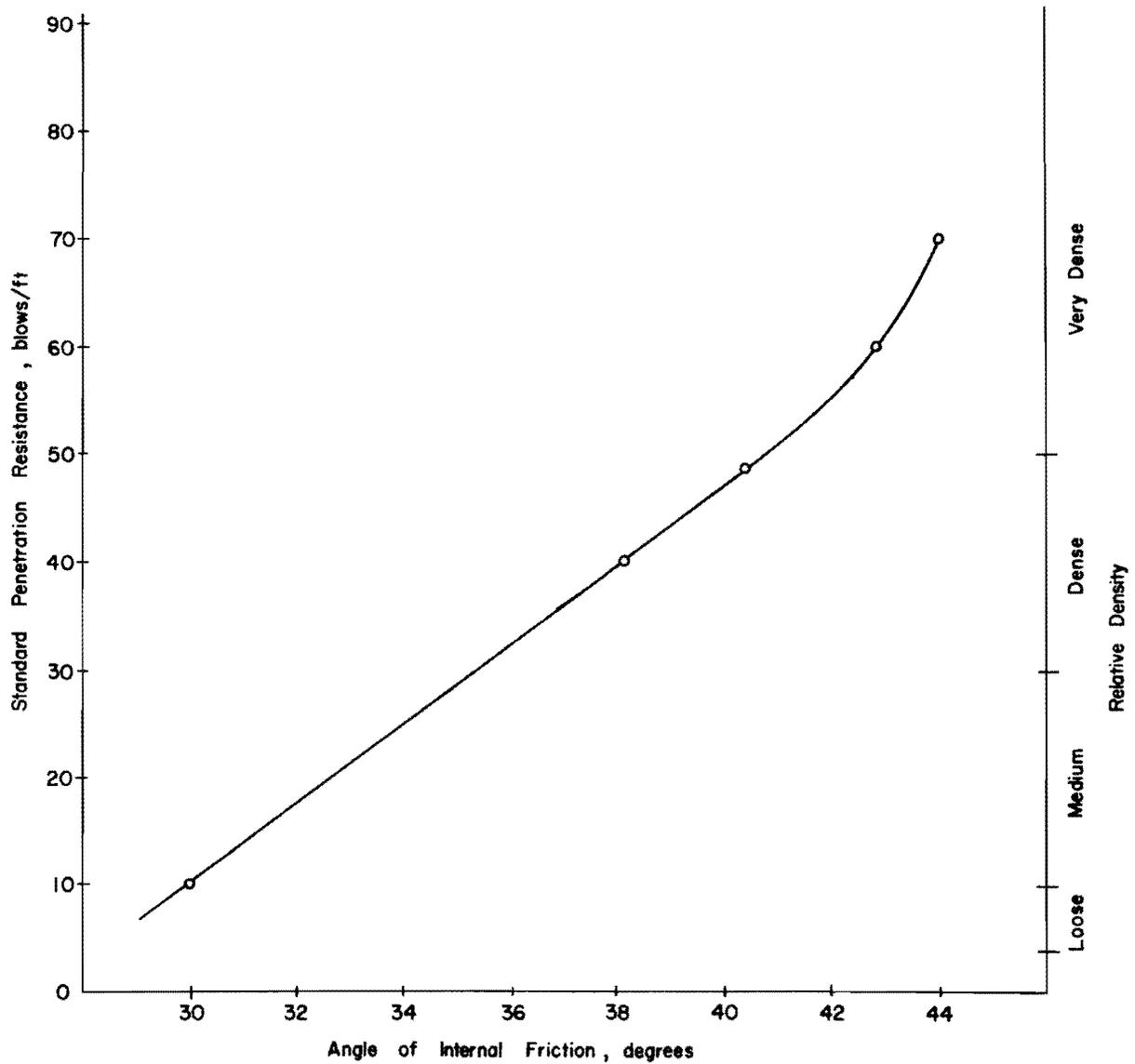
Fig. 3.4. Relationship Between Penetration Resistance and Angle of Internal Friction of Cohesionless Soils
