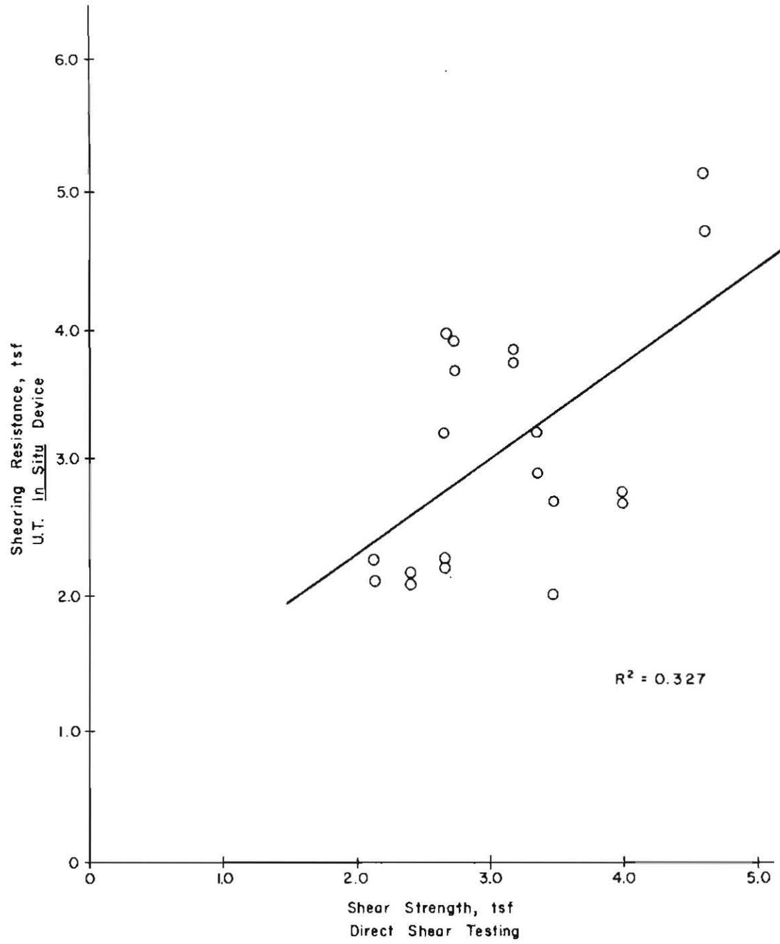
Fig. 5.3. Correlation of Shearing Resistances Measured with UT In Situ Device and Direct Shear Test Results, Montopolis Site
