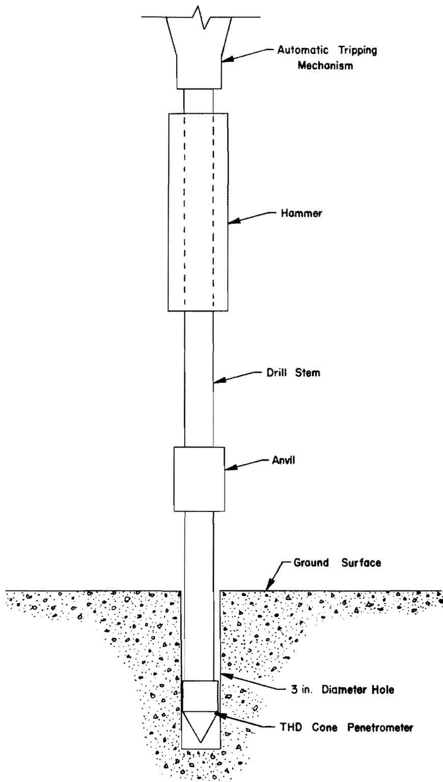
Fig. 3.6. THD Cone Penetration Test Arrangement
