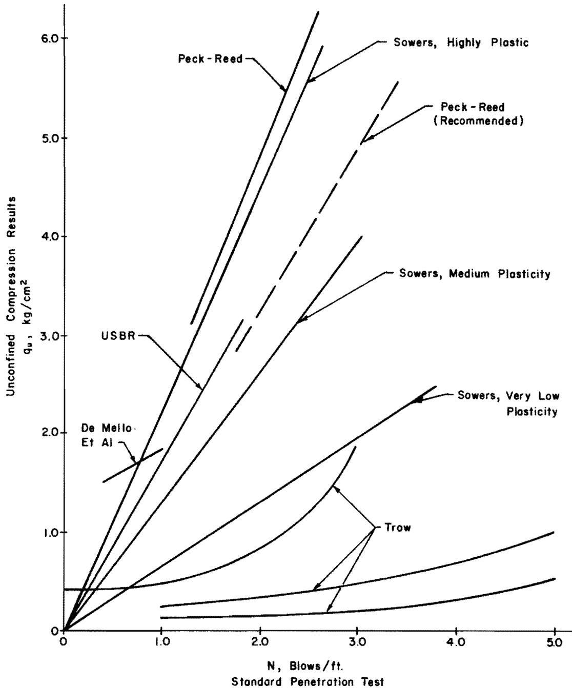
Fig. 3.3. Attempted Correlations Between  $N$  and  $q_u$  ( $\text{kg}/\text{cm}^2$ ) for Clays (After De Mello)
