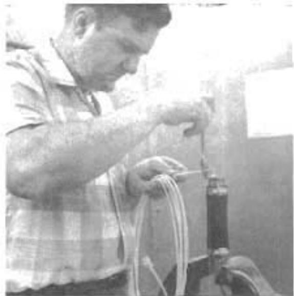
Fig. 2.12. Steps in Assembly of a Mustran Cell
