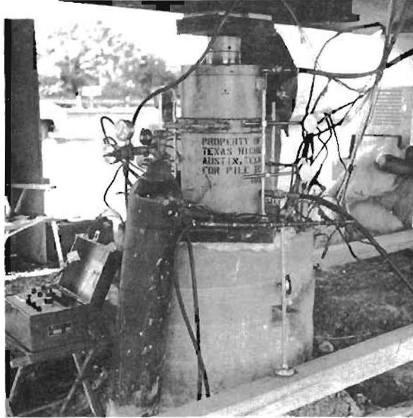
Fig. 4.8a. Shaft Head and Loading Jack
