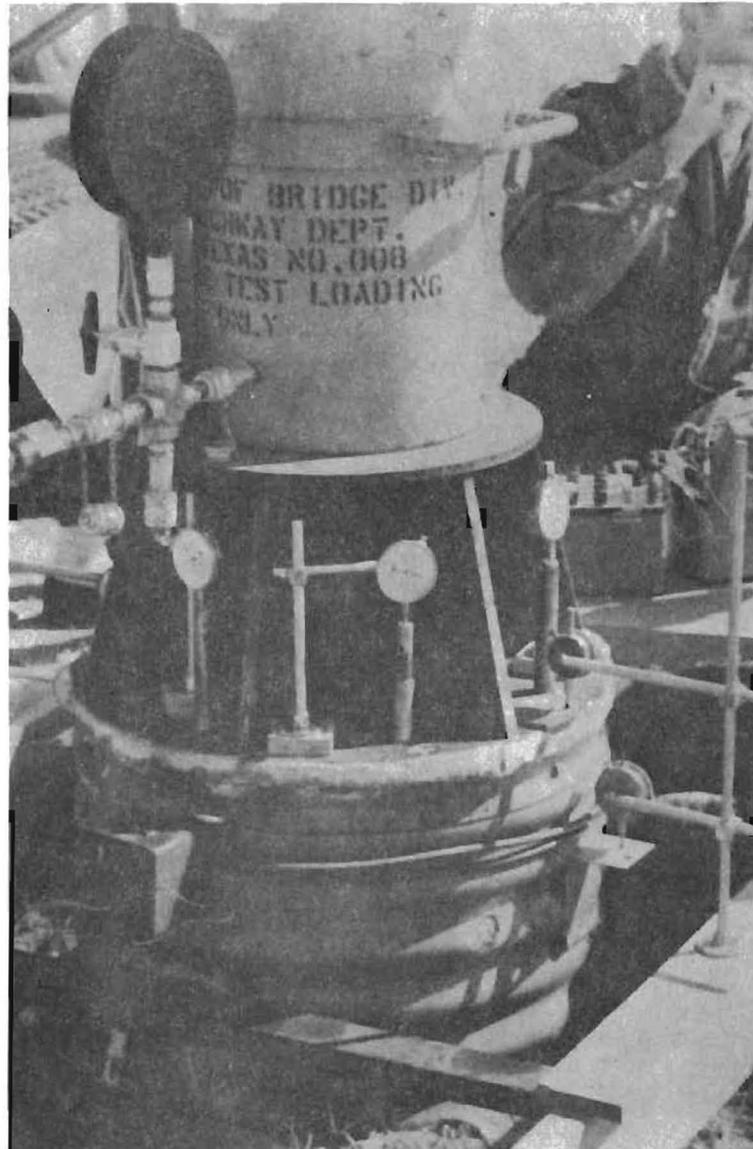
Fig. 3.2. View of Loading Head, Settlement Gages, and Telltales at the Montopolis Site (After Reese and Hudson, Ref. 13)
