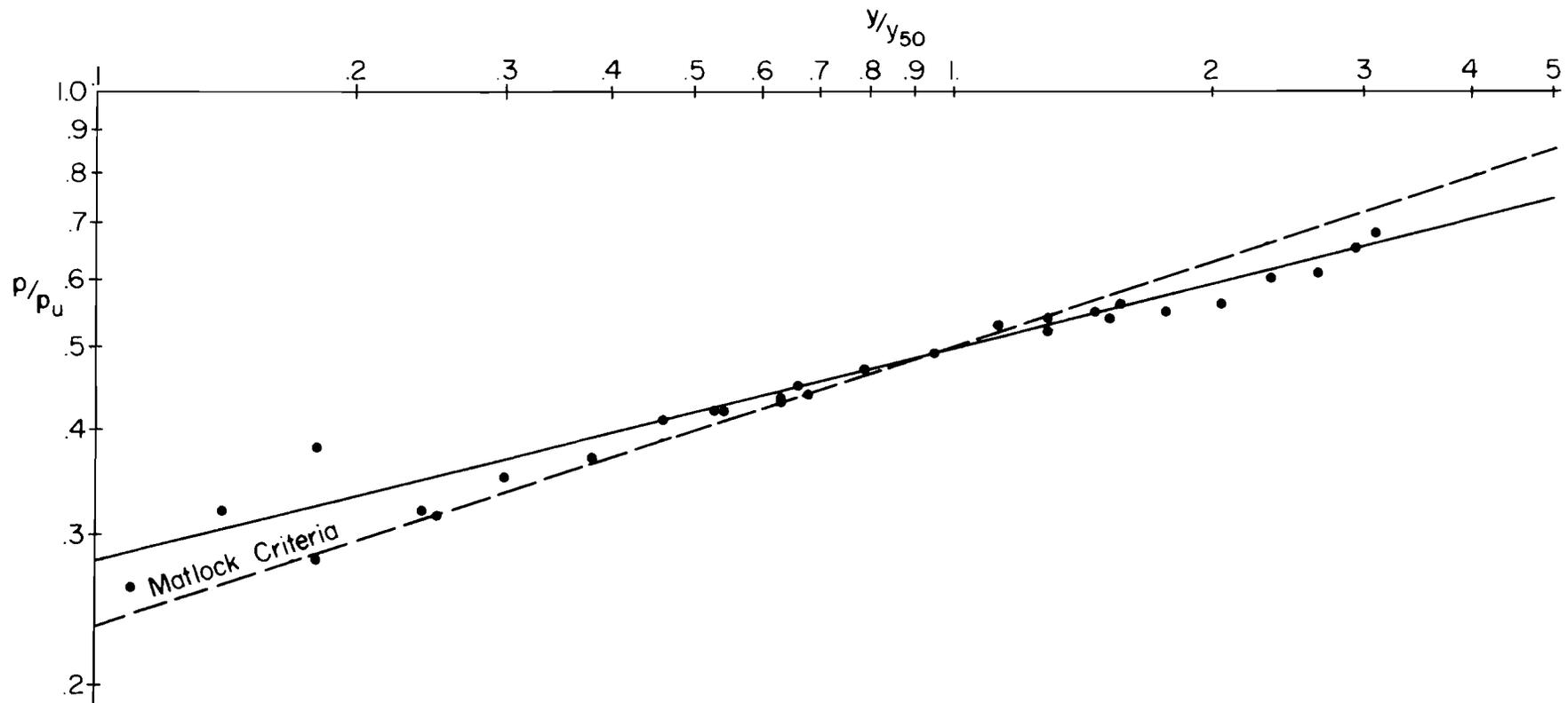
Fig. 7.14 Graphical Determination of Nondimensional p-y Curve
