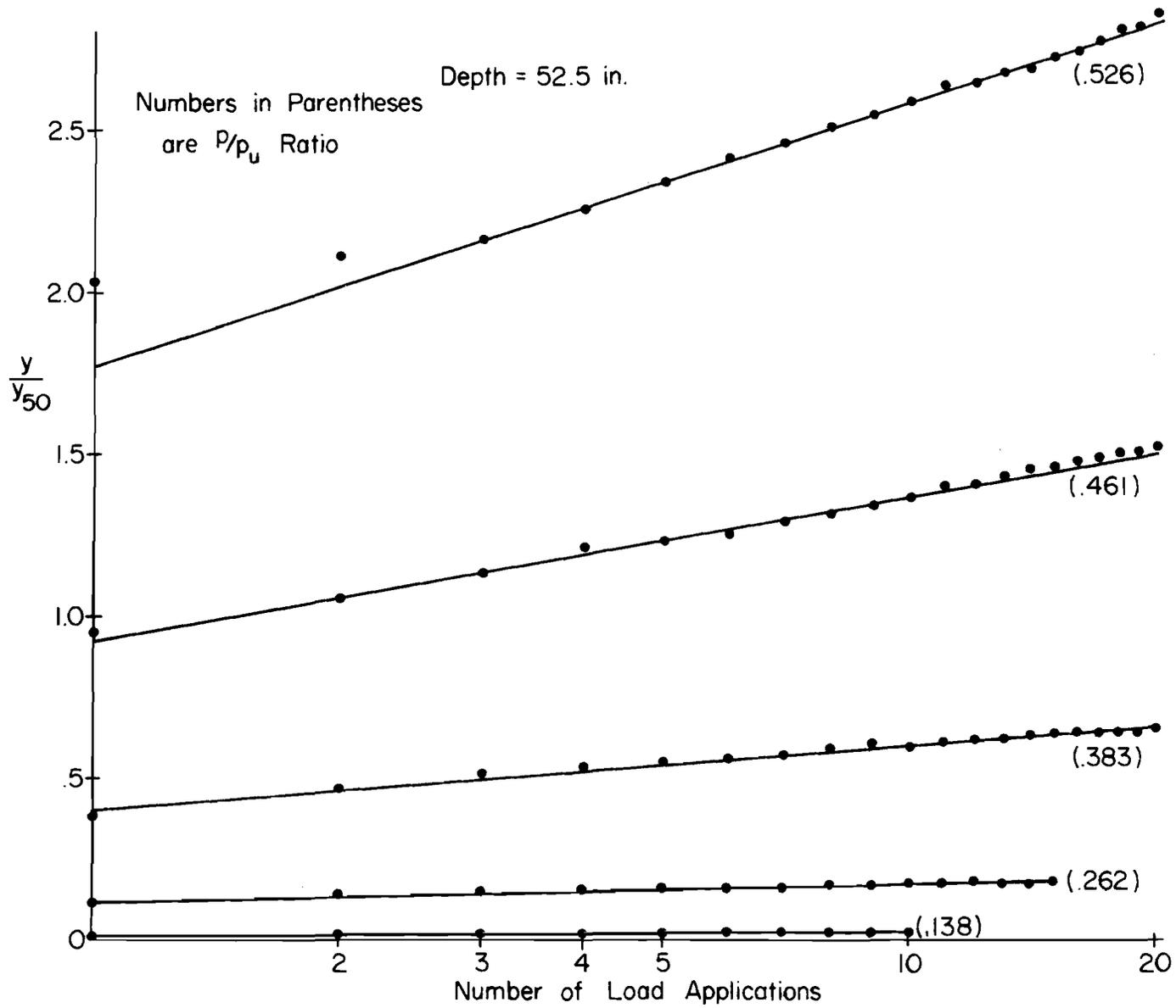
Fig. 7.15e Effect of Stress Level on Deformation Under Repeated Loading,
