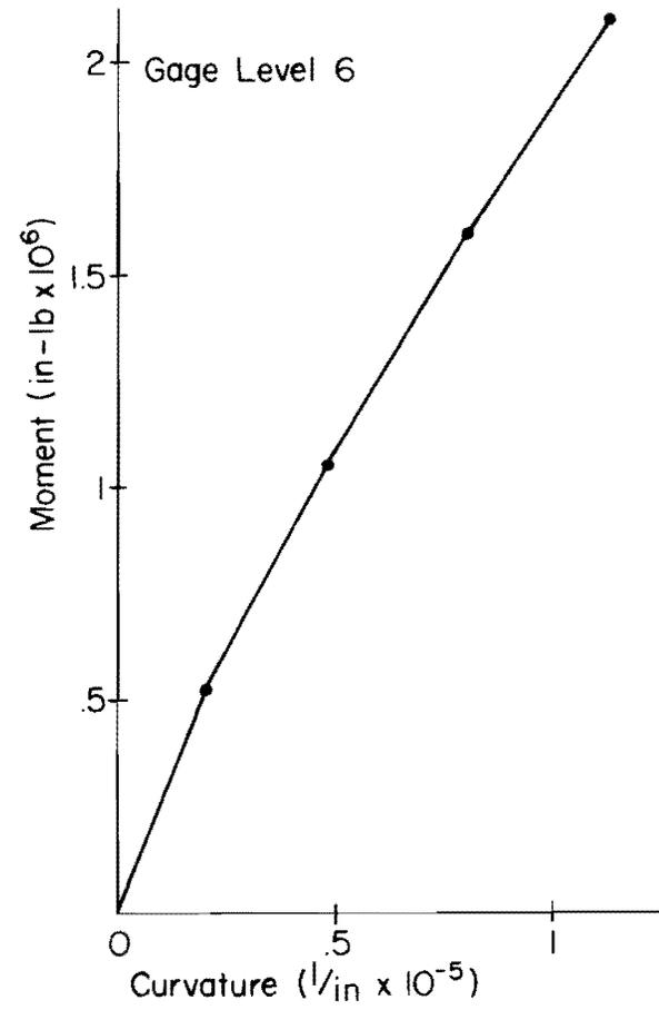
Fig. A.2 Measured Moment-Curvature Relationships
