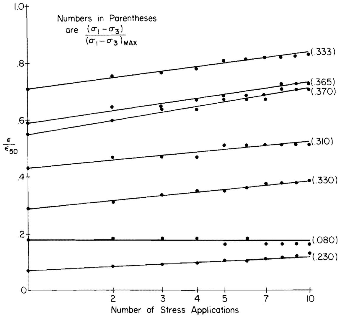
Fig. 8.4a Effect of Stress Level on Deformation Under Repeated Loading
