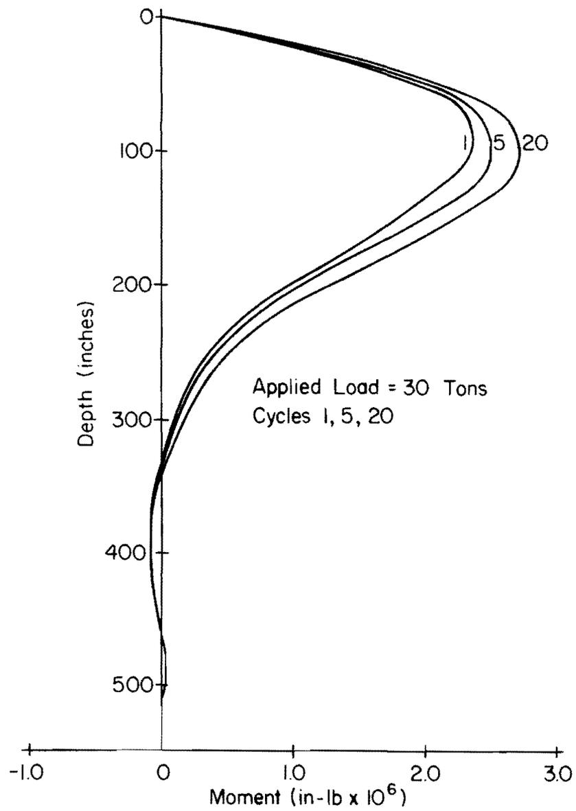
Fig. 7.8 Effect of Repeated Loading on Moment
