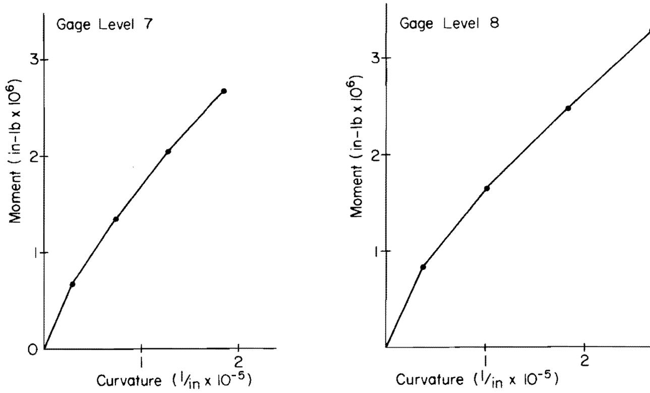
Fig. A.3 Measured Moment-Curvature Relationships
