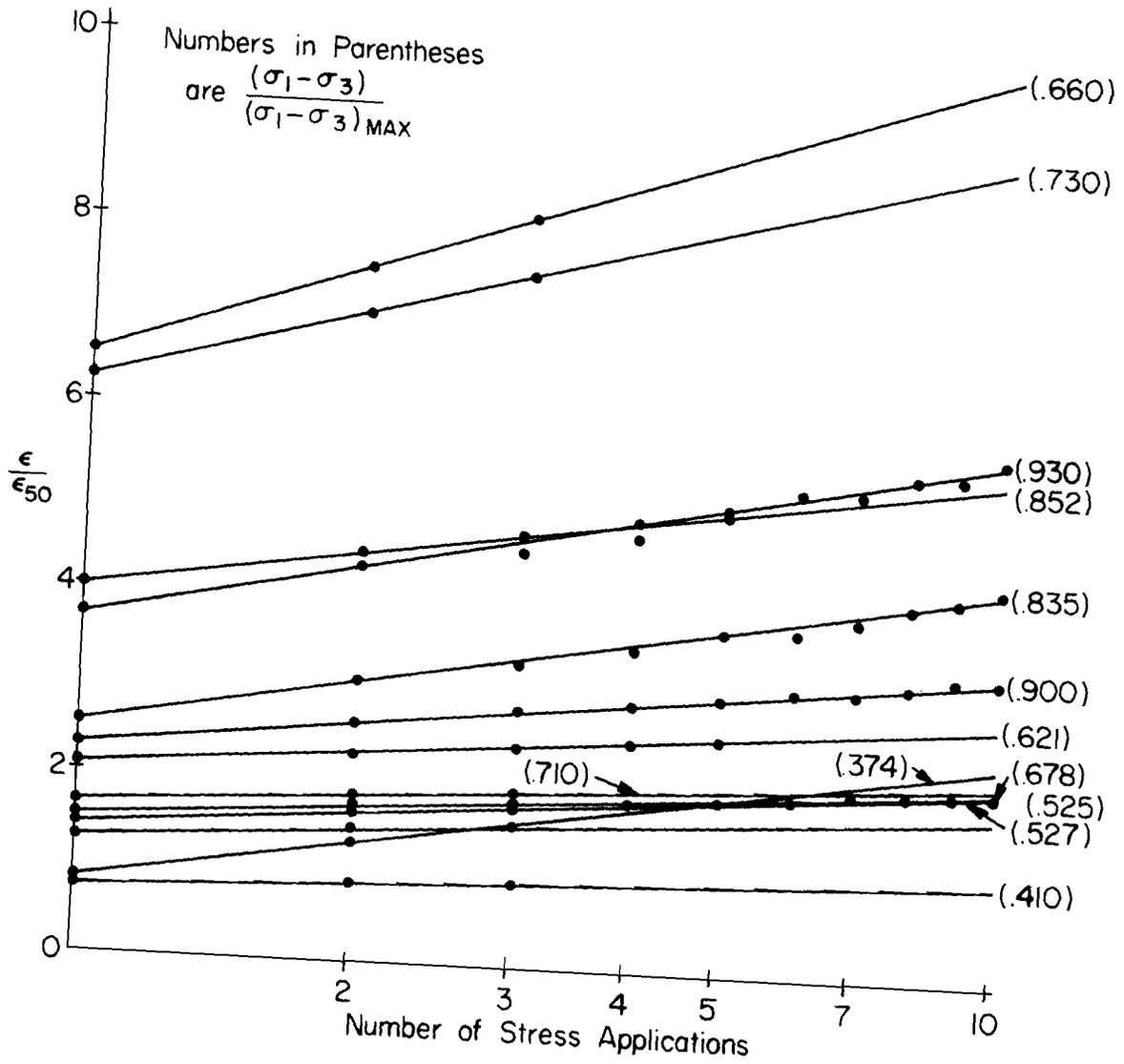
Fig. 8.4b Effect of Stress Level on Deformation Under Repeated Loading
