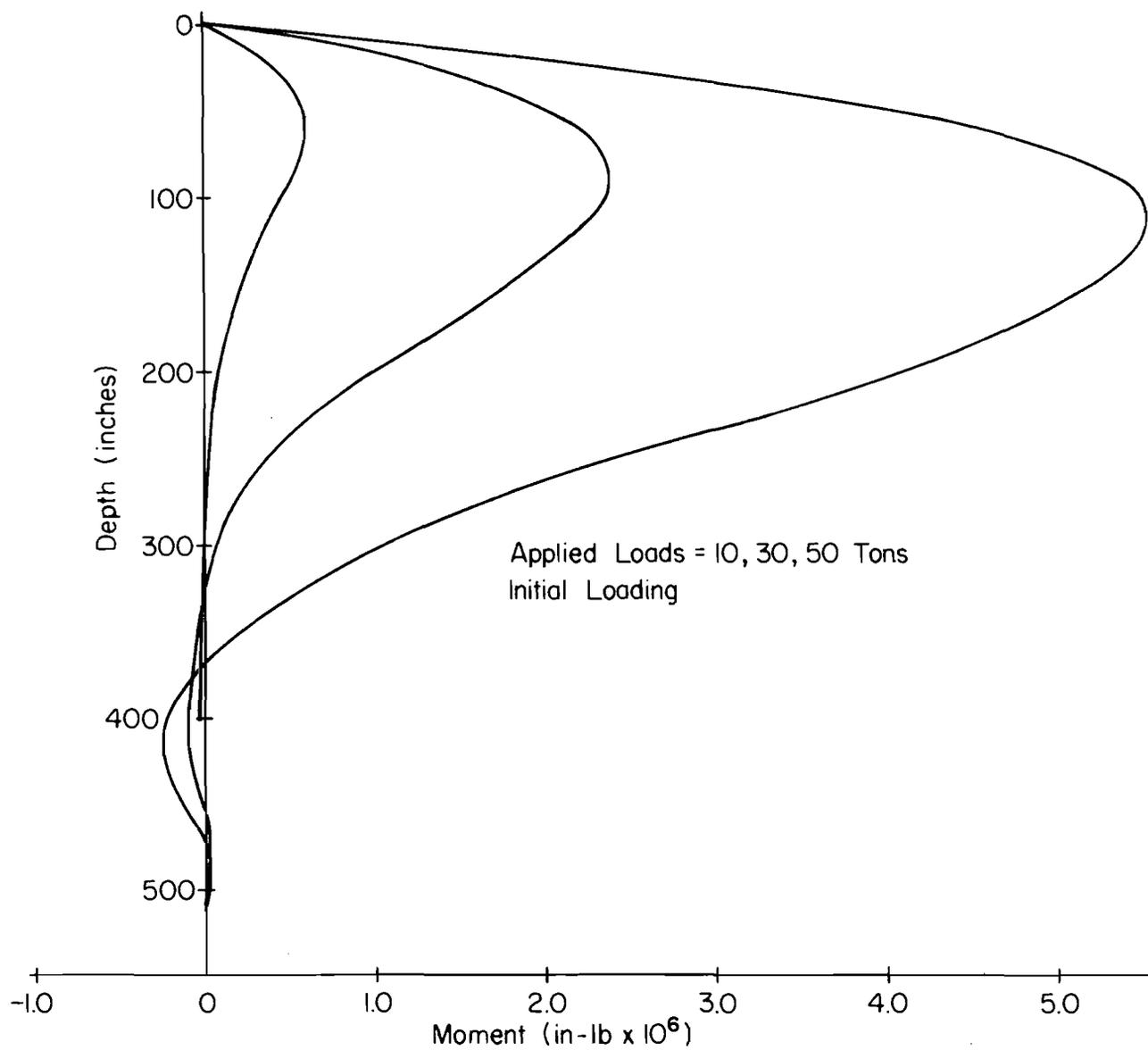
Fig. 7.9 Effect of Increasing Loads on Moment
