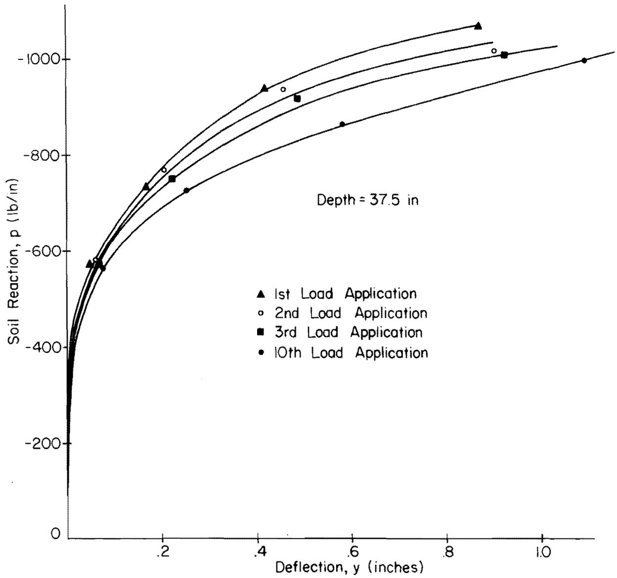
Fig. 7.13 Effect of Repeated Loading on  $p$ - $y$  Curves
