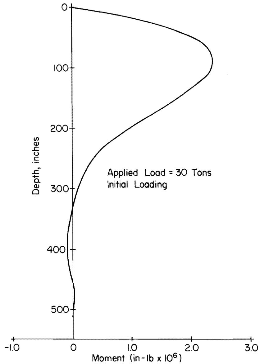
Fig. 7.7 Typical Variation of Moment with Depth
