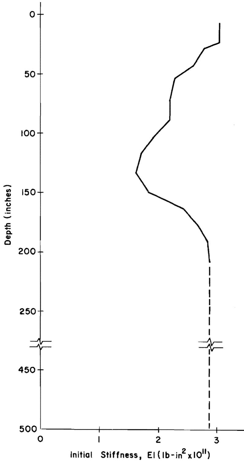
Fig. 7.5 Variation of Shaft Stiffness with Depth
