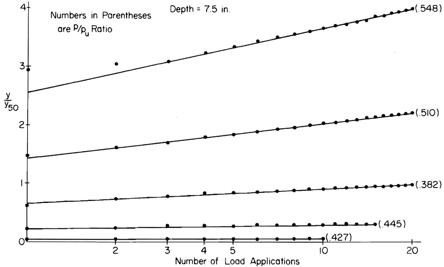
Fig. 7.15b Effect of Stress Level on Deformation Under Repeated Loading,
