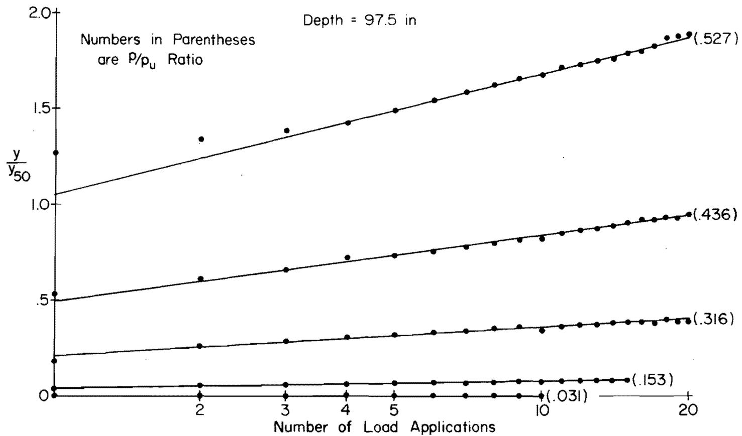
Fig. 7.15h Effect of Stress Level on Deformation Under Repeated Loading,
