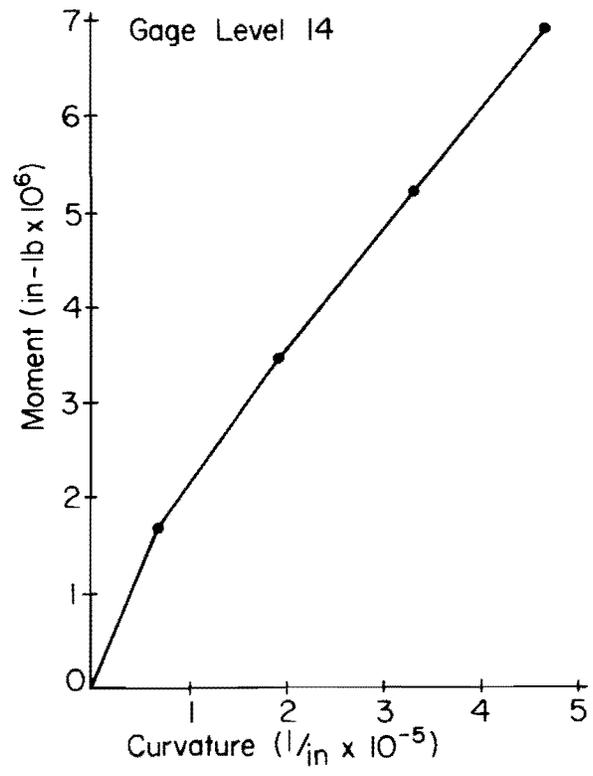
Fig. A.6 Measured Moment-Curvature Relationships
