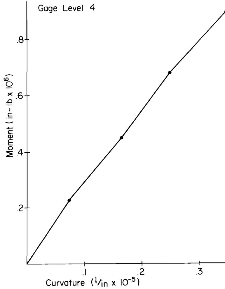
Fig. A.1 Measured Moment-Curvature Relationships
