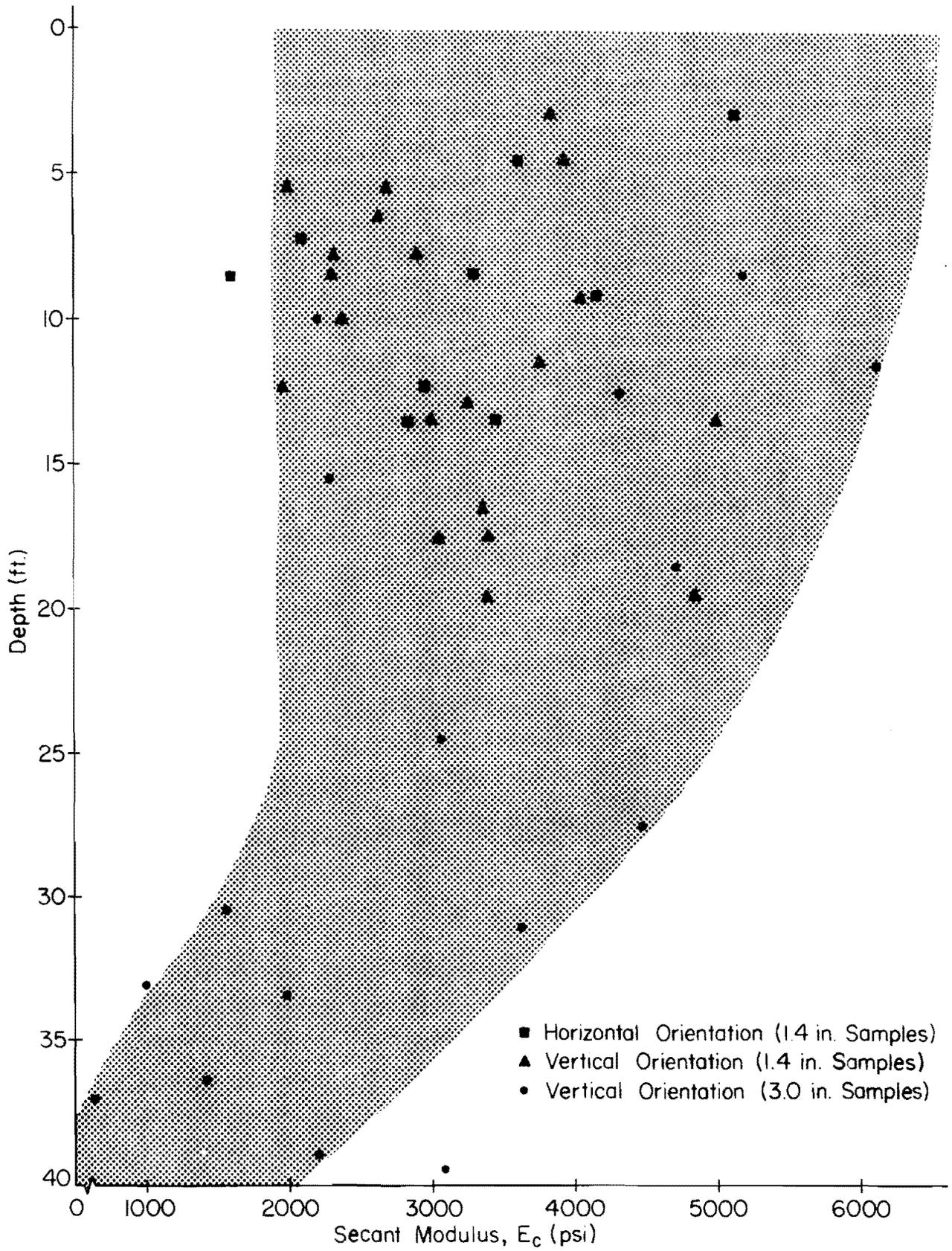
Fig. 8.2 Soil Stiffness Variation with Depth
