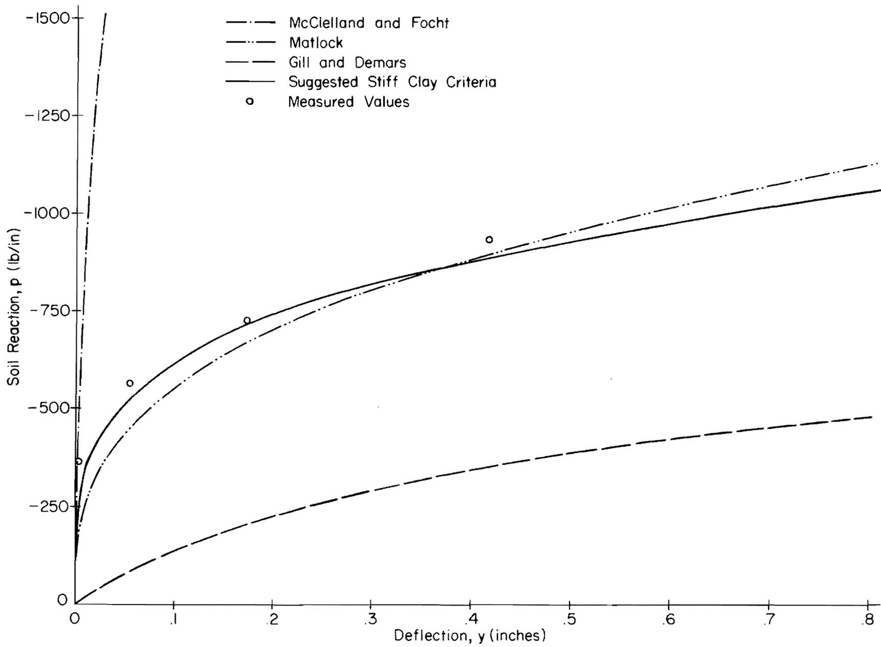
Fig. 9.5 Comparison of Various Criteria
