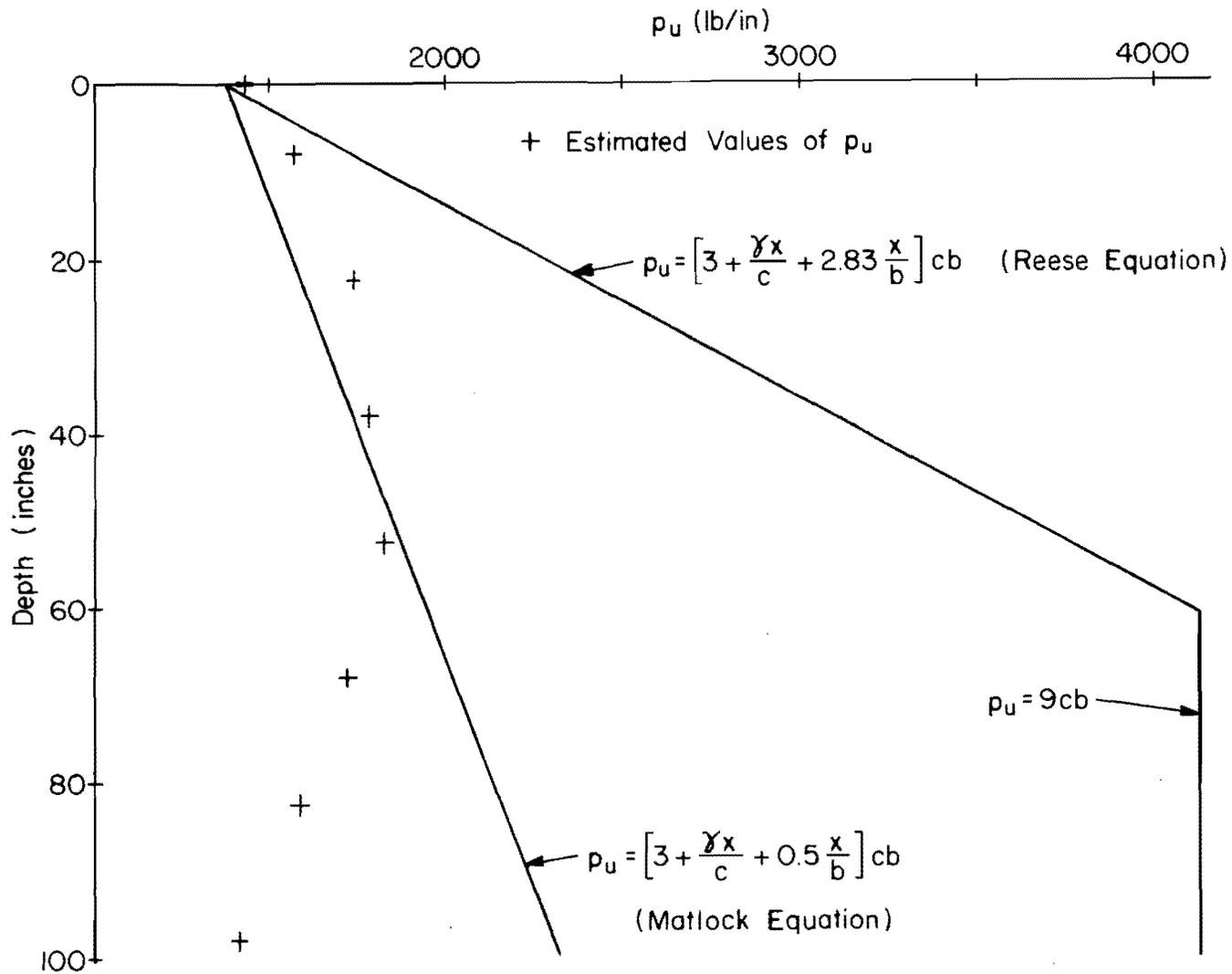
Fig. 7.16 Variation of Ultimate Soil Resistance with Depth
