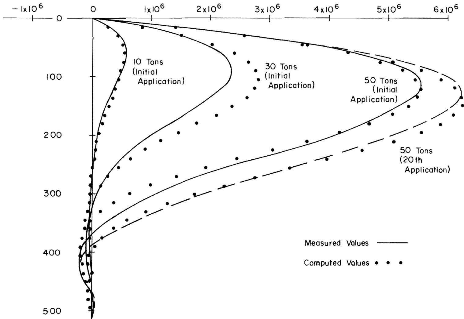
Fig. 9.4 Computed and Measured Values of Moment vs. Depth
