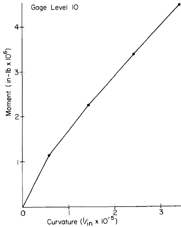
Fig. A.4 Measured Moment-Curvature Relationships
