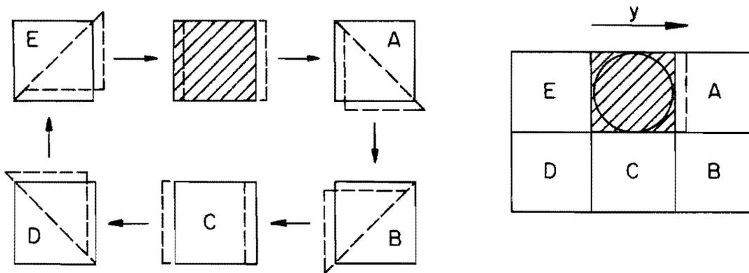
b. Flow-Around Failure (after Reese, 1958).
