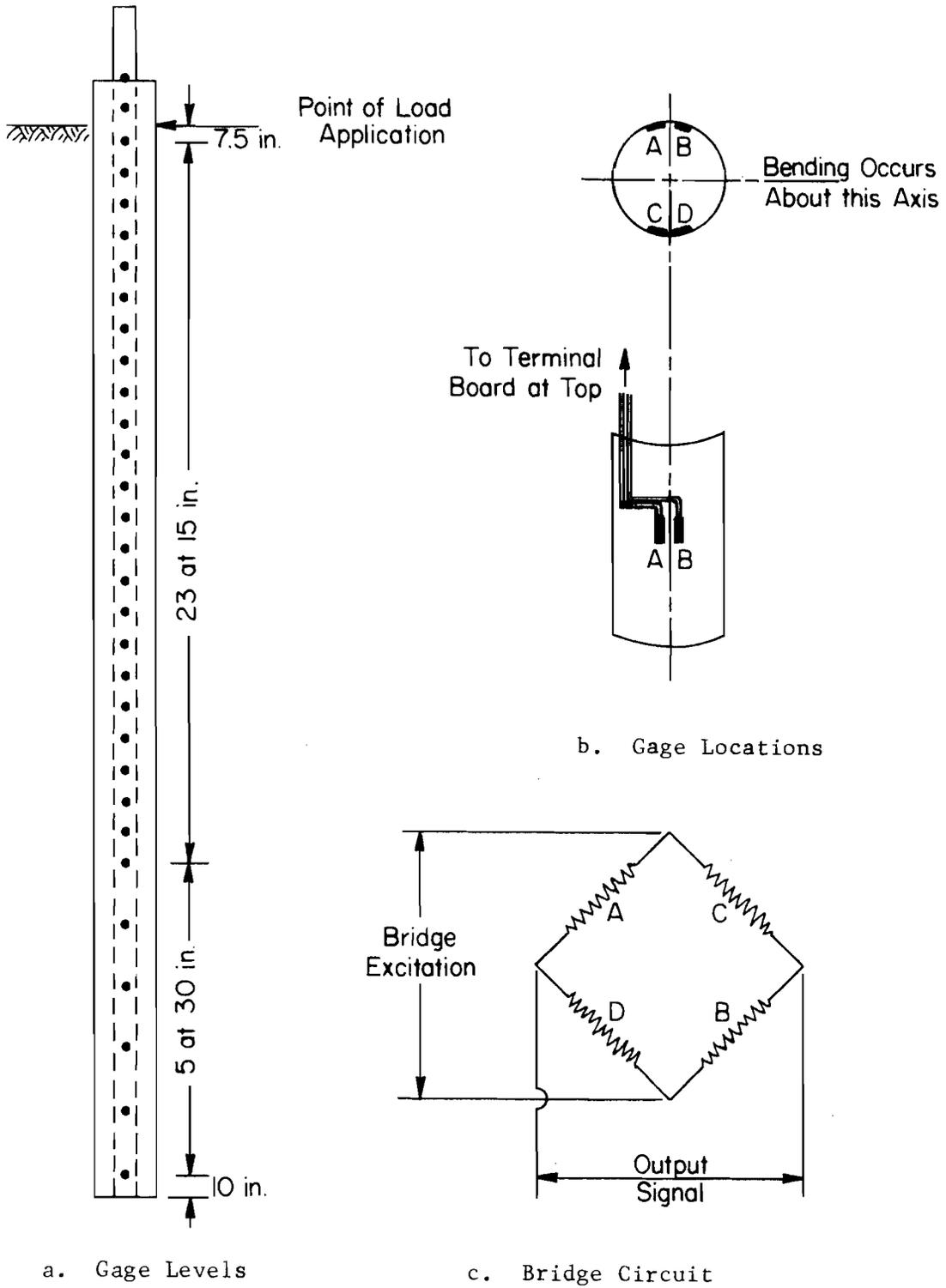
Fig. 6.3 Gage Locations and Circuits
