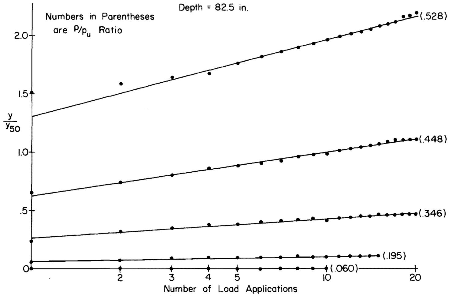
Fig. 7.15g Effect of Stress Level on Deformation Under Repeated Loading, Depth = 82.5 in.
