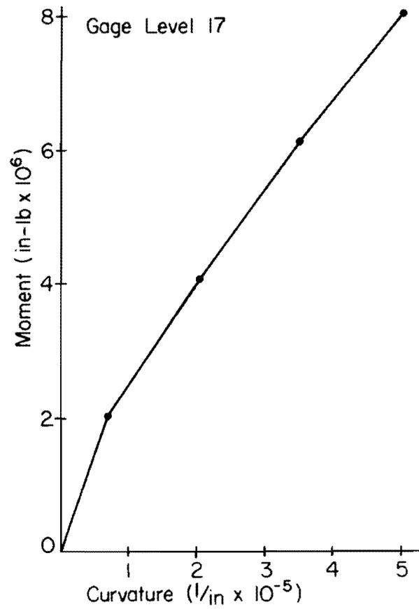
Fig. A.8 Measured Moment-Curvature Relationships
