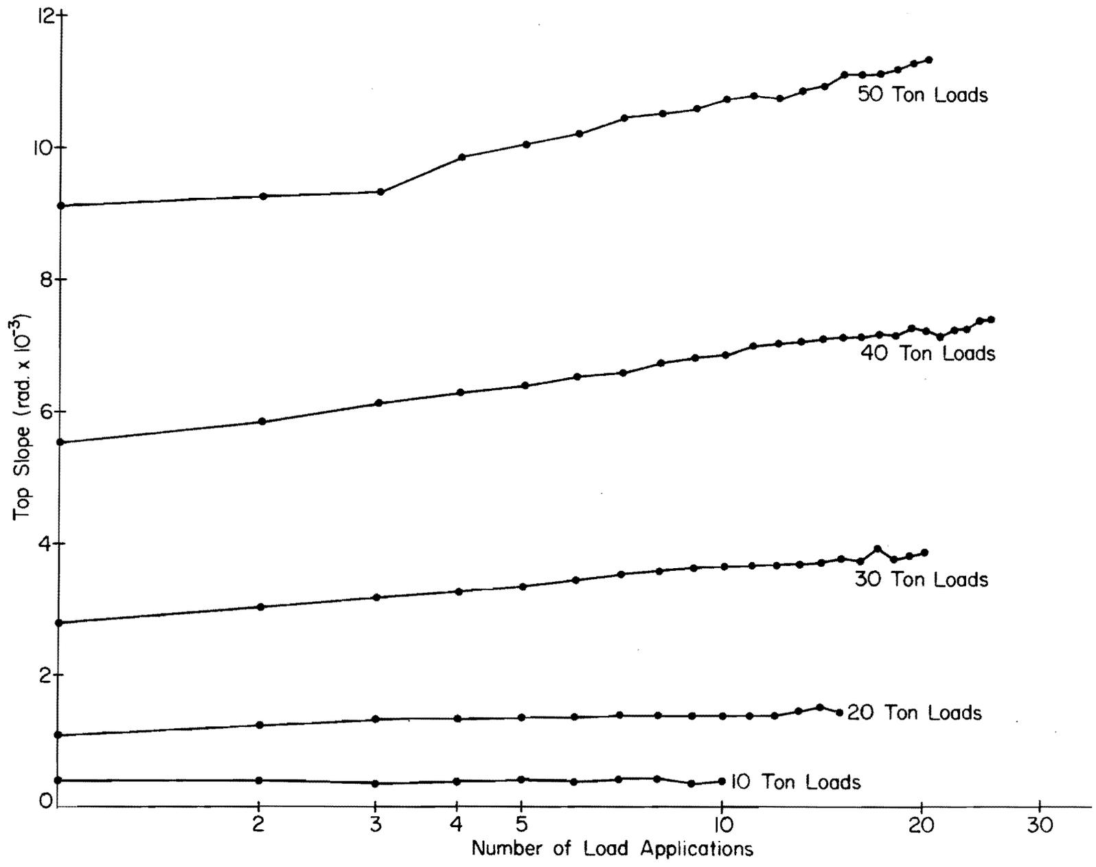
Fig. 7.4 Effect of Repeated Loading on Top Slope
