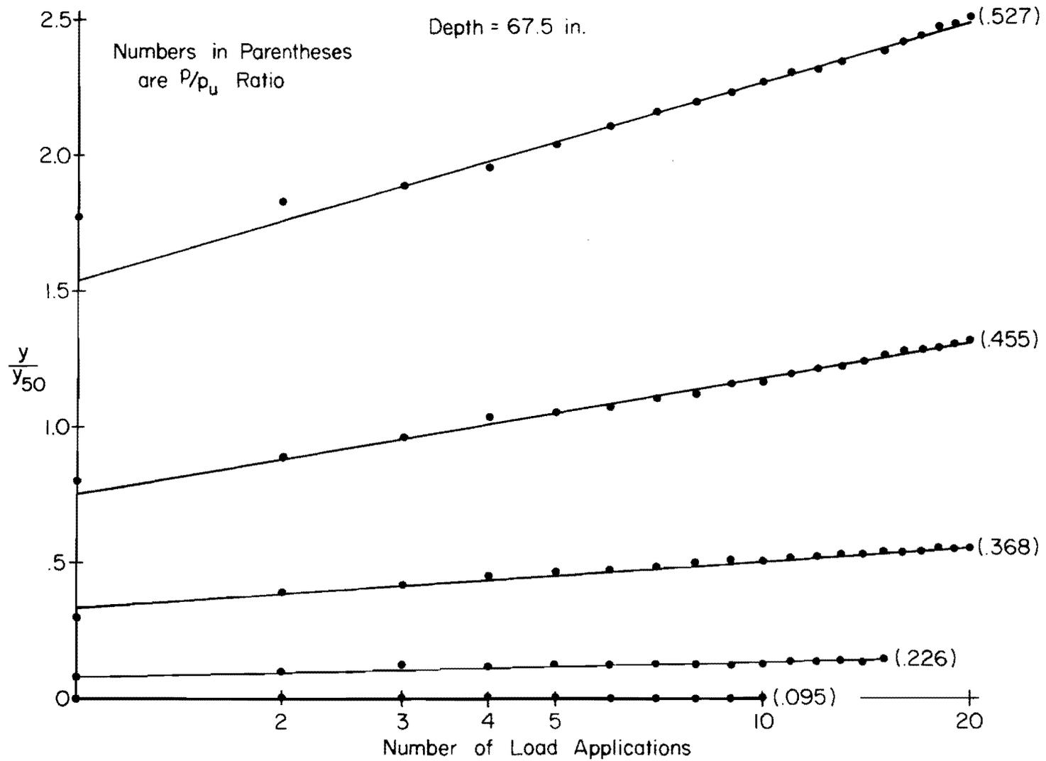
Fig. 7.15f Effect of Stress Level on Deformation Under Repeated Loading,
