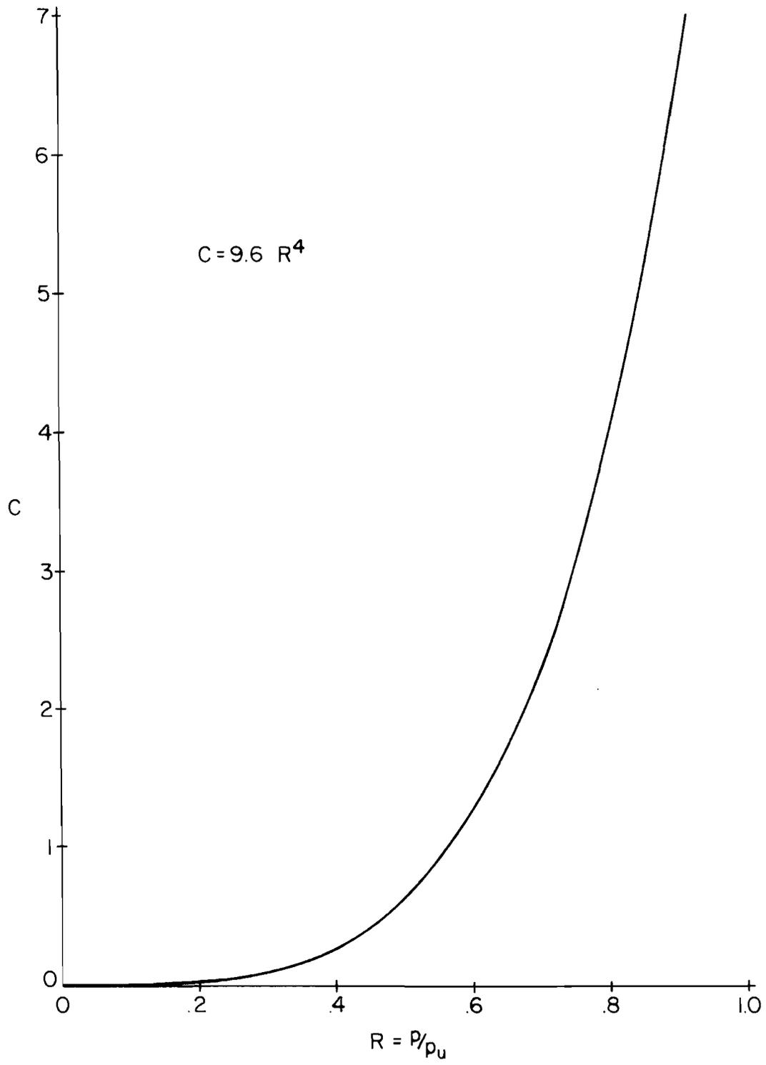
Fig. 9.3 Stress Ratio - Parameter C Relationship
