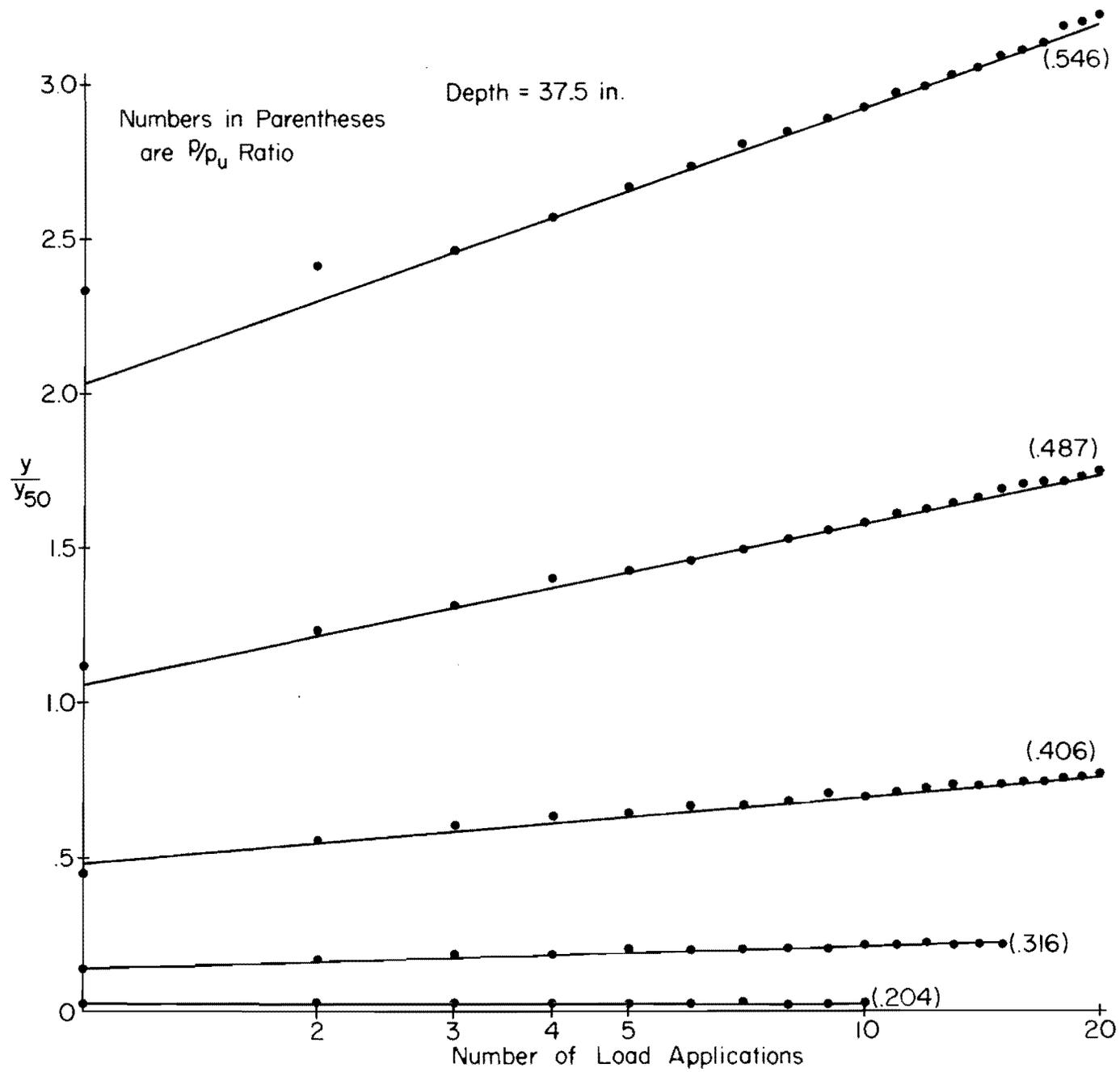
Fig. 7.15d Effect of Stress on Deformation Under Repeated Loading,
