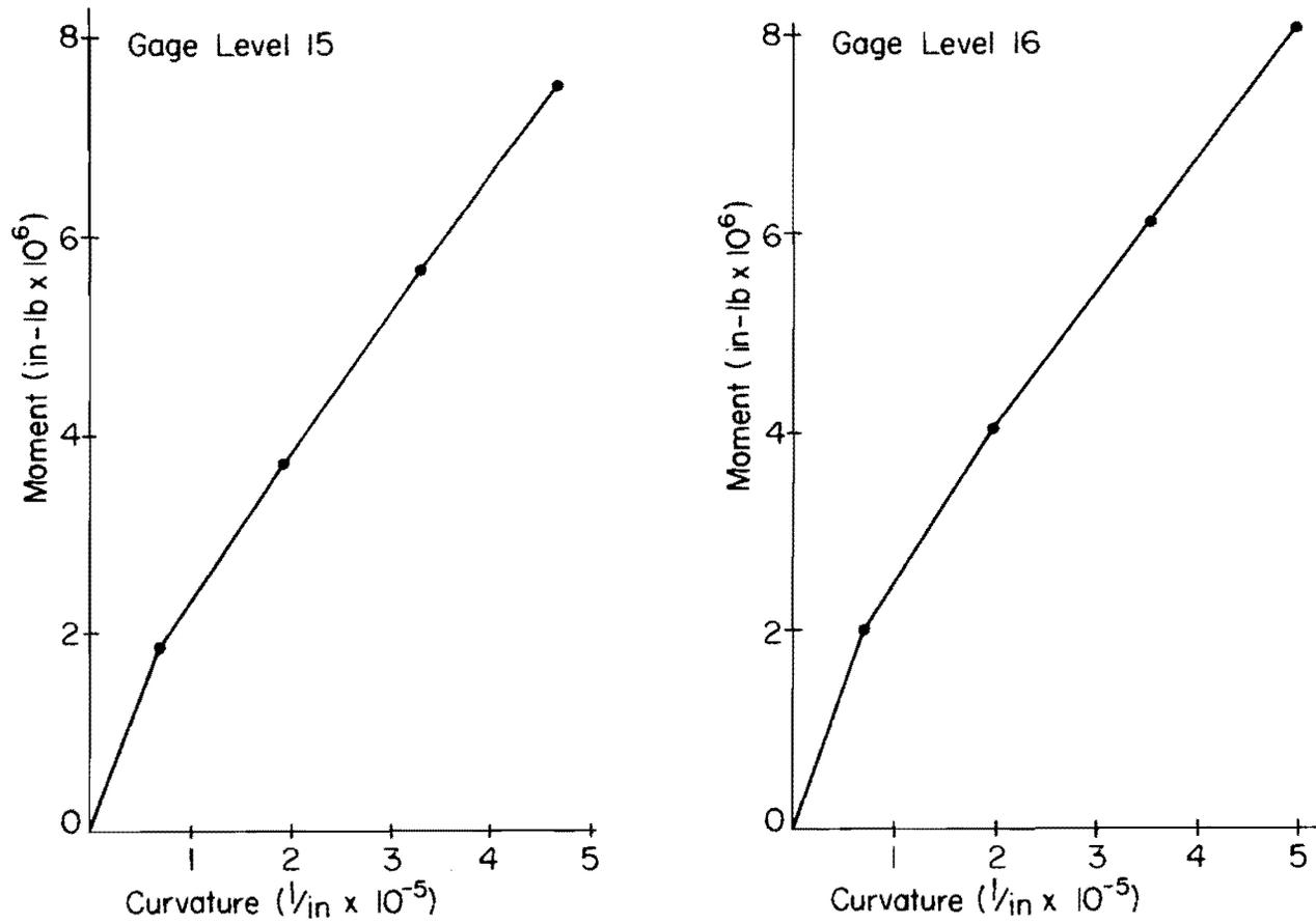
Fig. A.7 Measured Moment-Curvature Relationships
