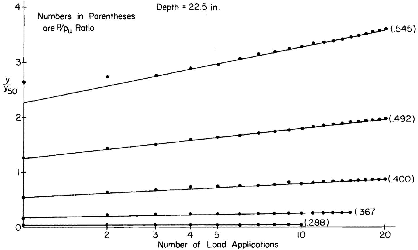
Fig. 7.15c Effect of Stress Level on Deformation Under Repeated Loading, Depth = 22.5 in.
