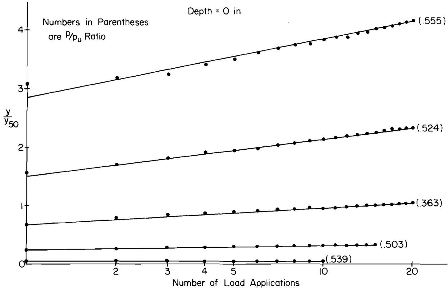
Fig. 7.15a Effect of Stress Level on Deformation Under Repeated Loading,
