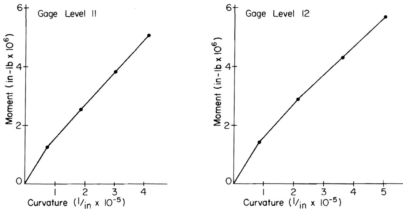
Fig. A.5 Measured Moment-Curvature Relationships
