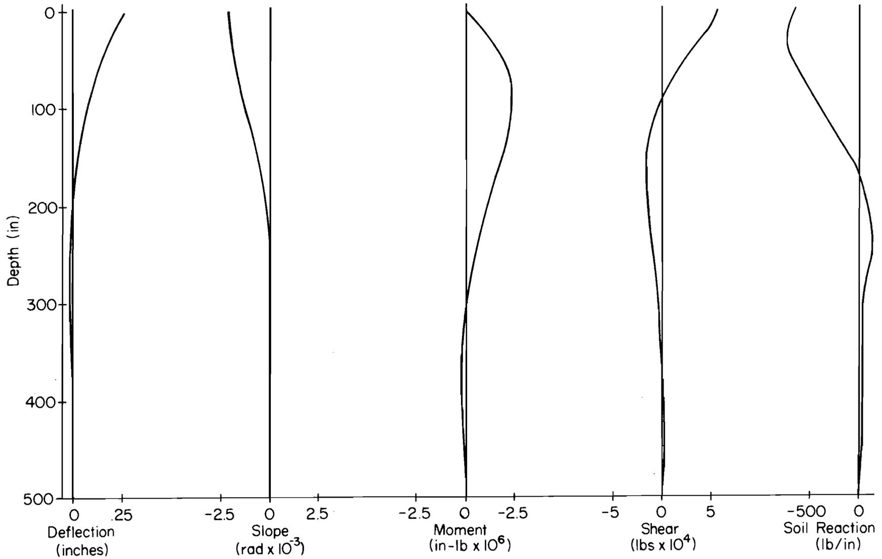
Fig. 7.12 Complete Solution of Laterally Loaded Drilled Shaft
