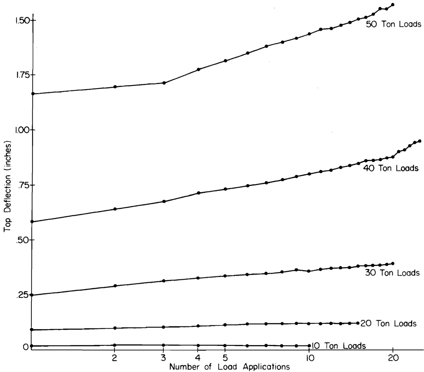
Fig. 7.2 Effect of Repeated Loading on Top Deflection
