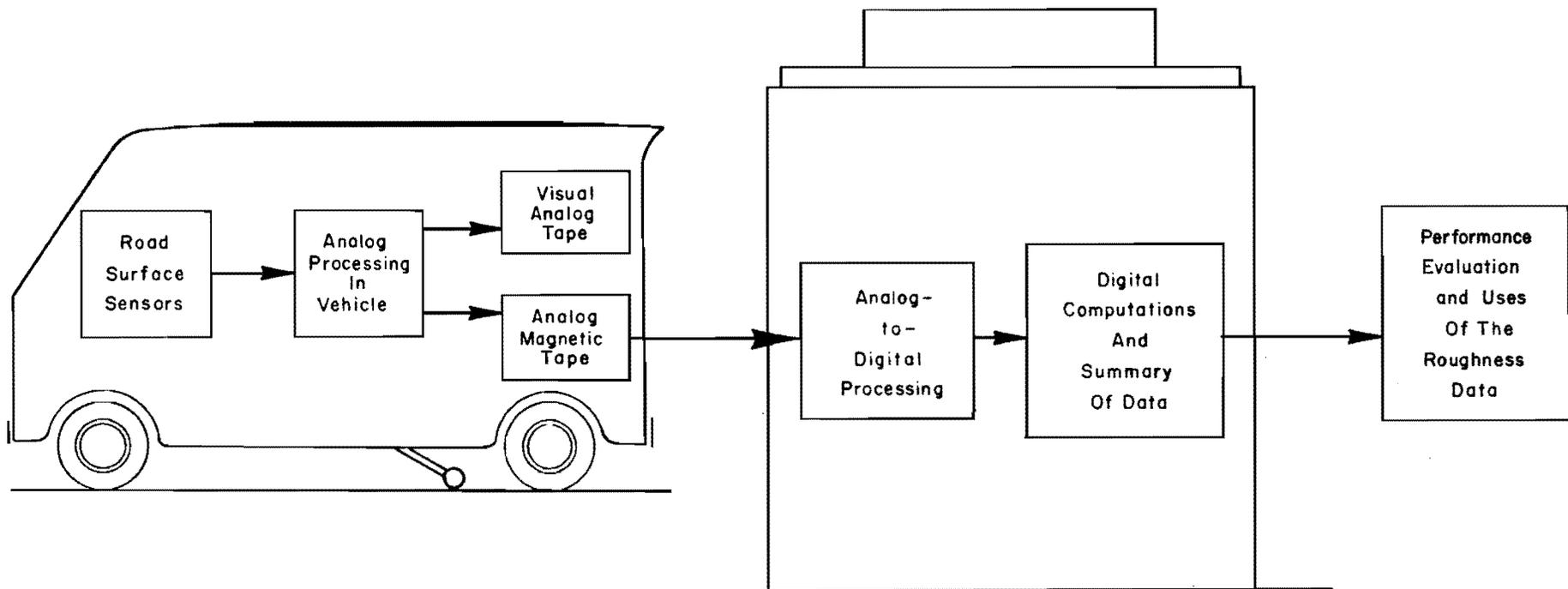
Fig 2. Profilometer measurement system.
