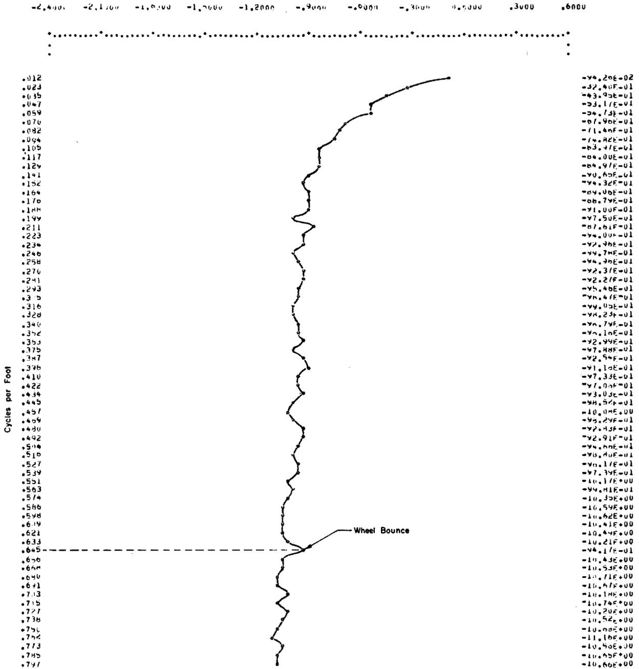
Fig 6. Power spectral plot for right wheel path.
