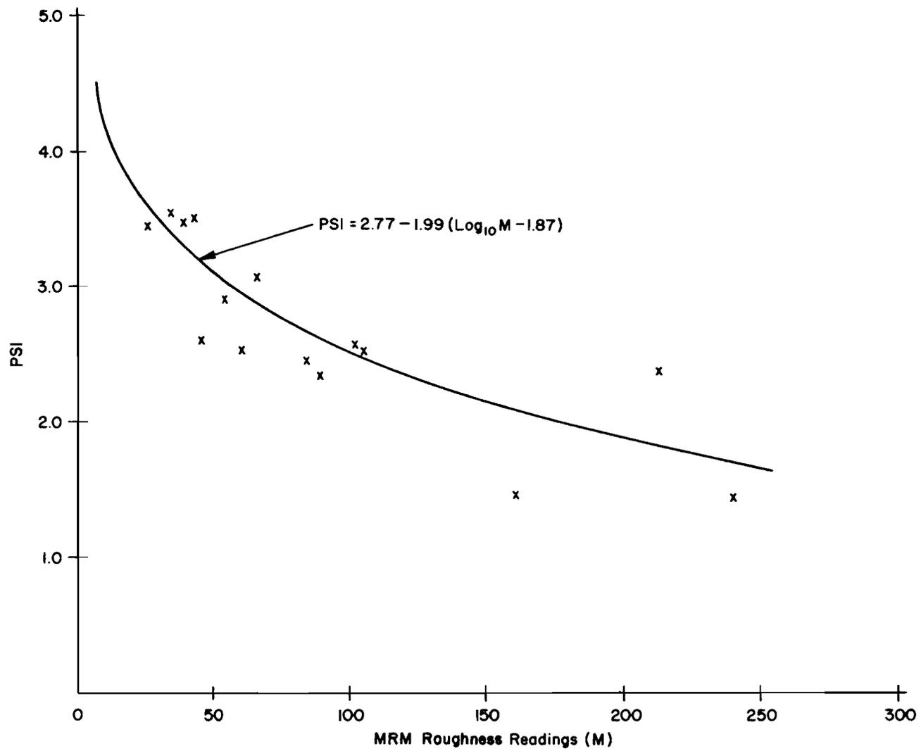
Fig 3. Surface Dynamics Profilometer PSI versus MRM roughness.
