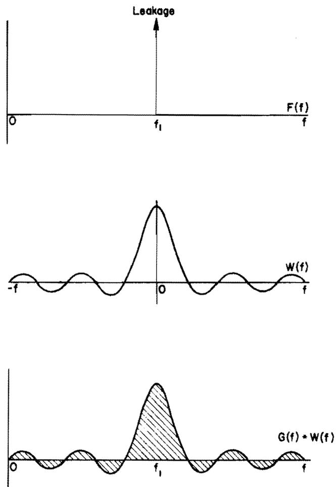
Fig 13. Results of convoluting rectangular data window with sine wave (after Ref 18).
