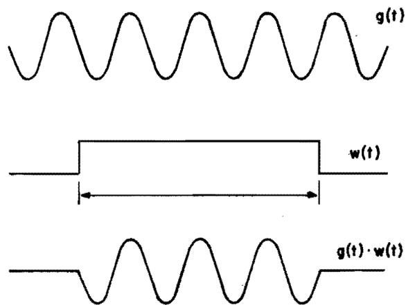
Fig 12. The rectangular data window result when using finite data record (after Ref 18).
