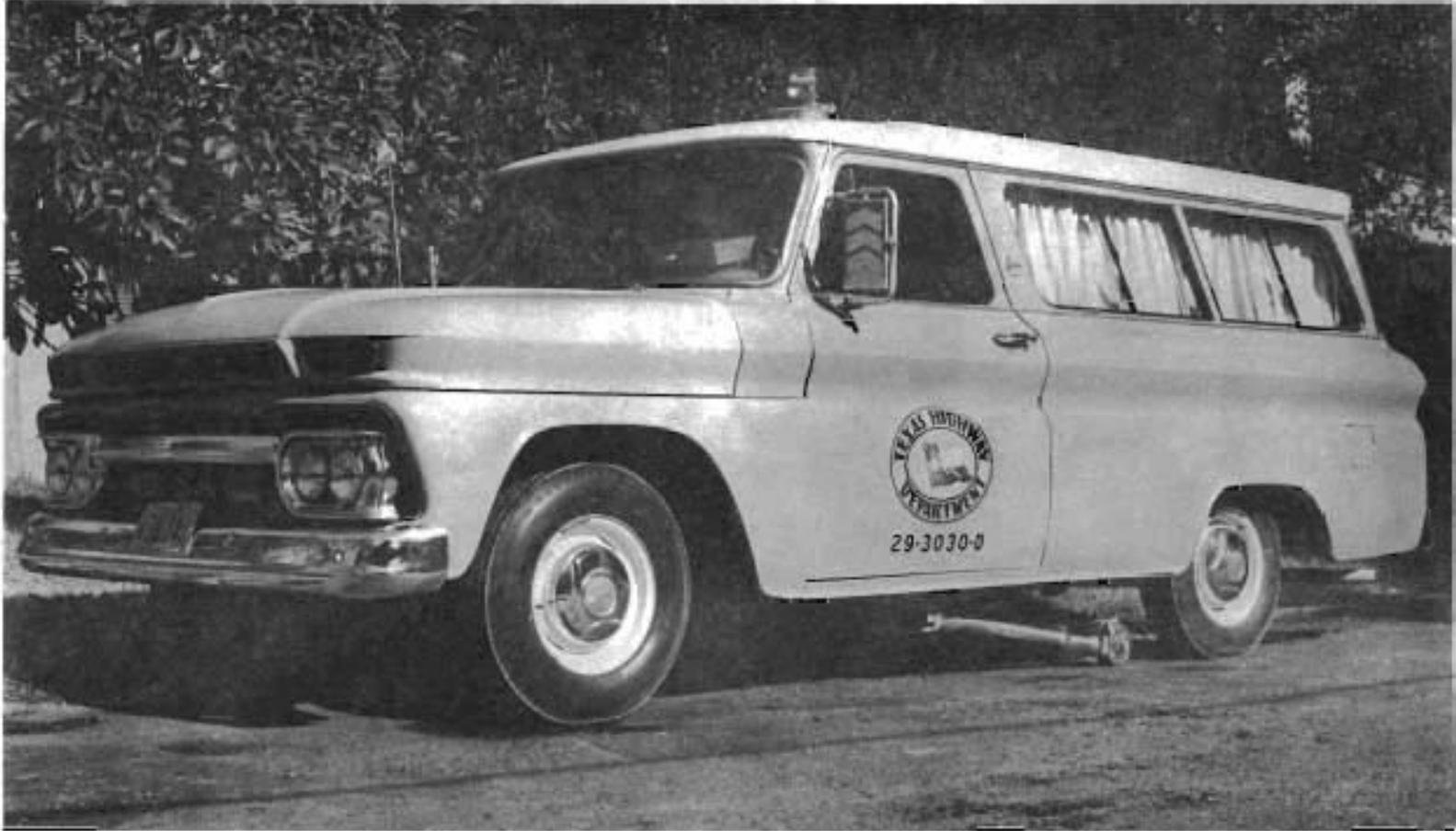
Fig 1. Surface Dynamics Profilometer.
