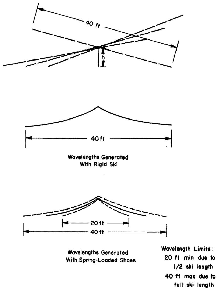
Fig 8. Wavelengths generated by longitudinal grade reference ski transversing abrupt bump.
