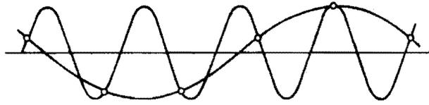
Fig 11. Aliasing effect of high-frequency wave (after Ref 18).
