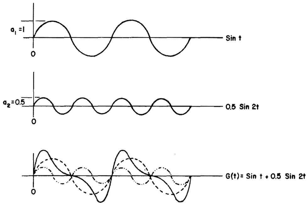
Fig 10. Complex wave consisting of first and second sine terms of its Fourier coefficients.
