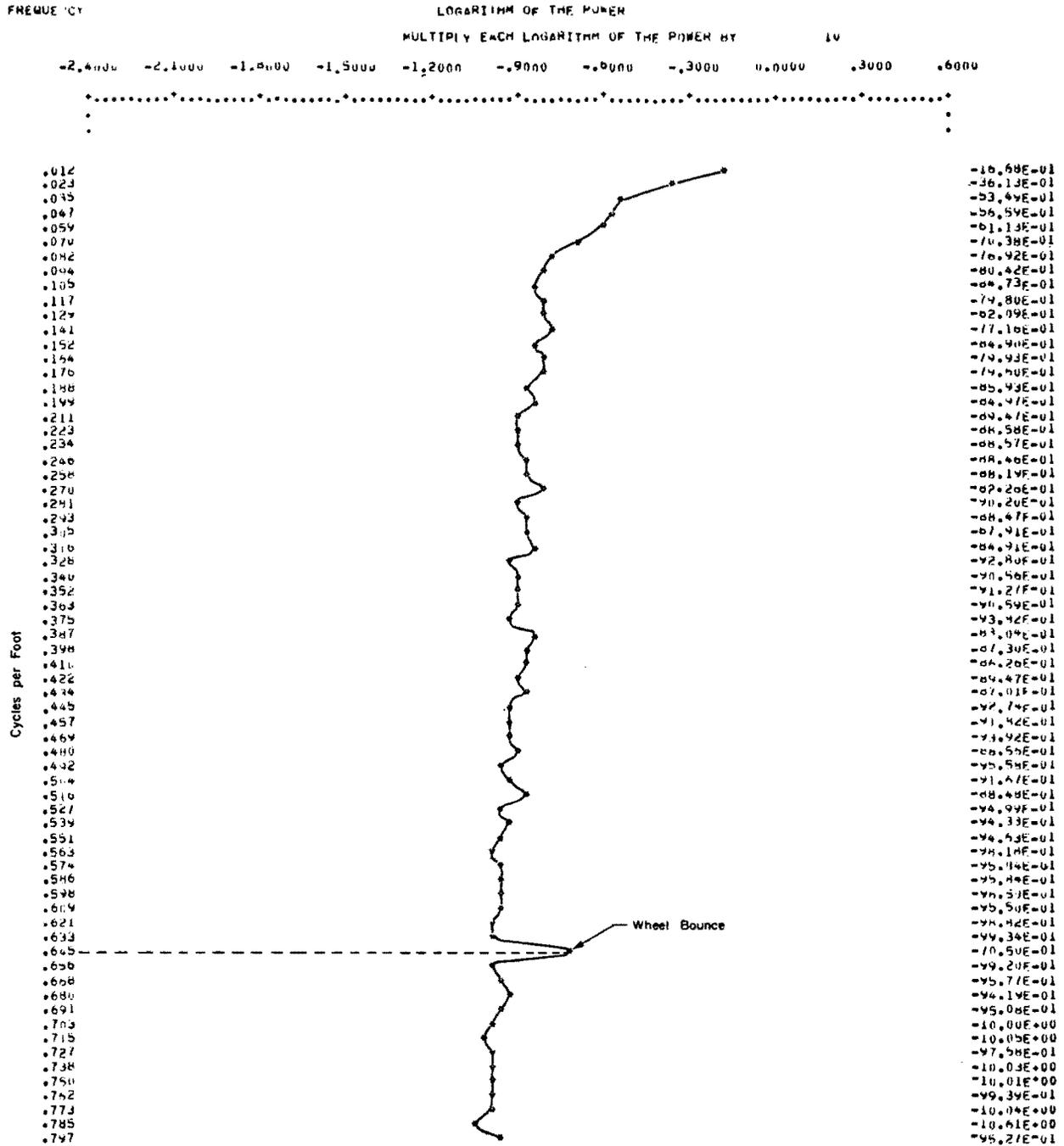
Fig 5. Power spectral plot for left wheel path.
