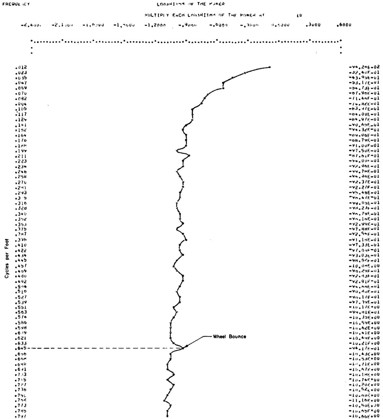
Fig 6. Power spectral plot for right wheel path.
