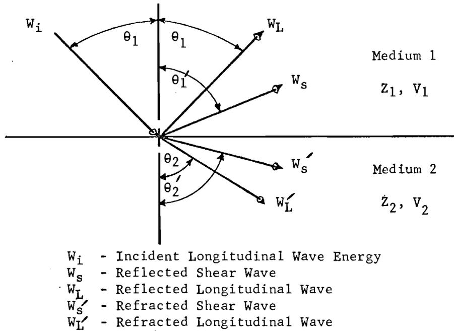
Figure II. Reflection & Refraction with Mode Conversion
