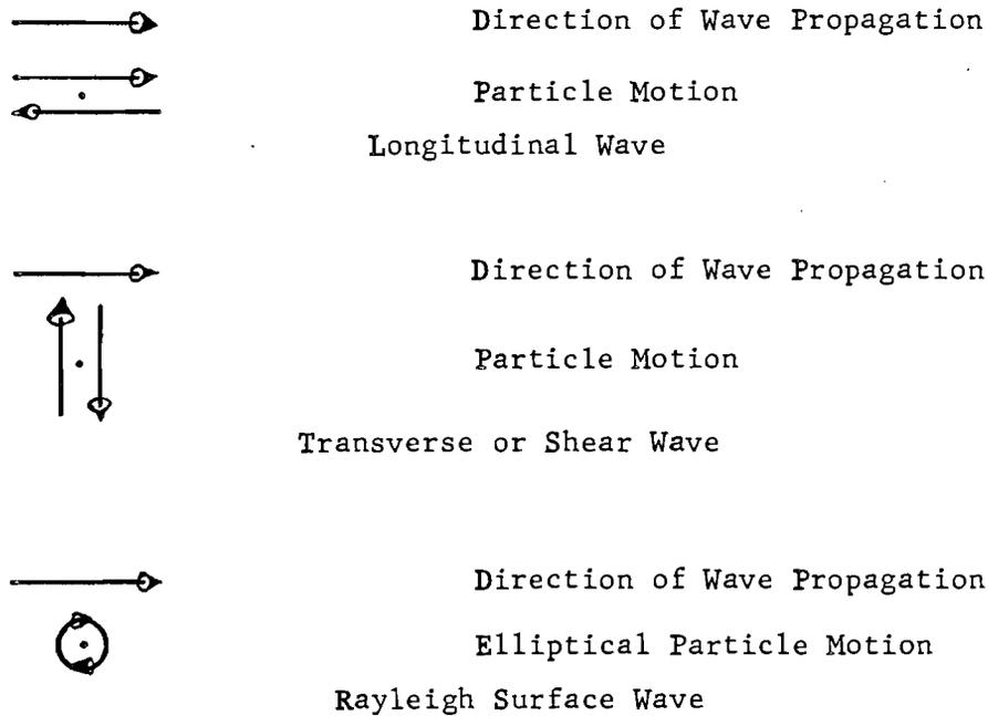
Figure I. Particle Motion for Various Modes of Wave Propagation
