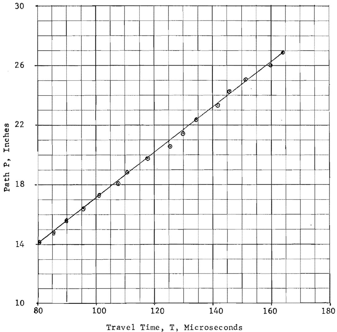
Figure VIII. Path, P, of Reflected Longitudinal Wave
