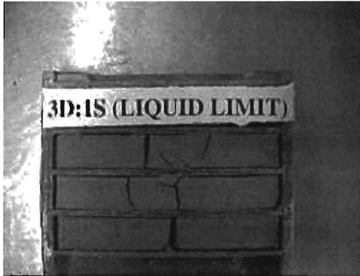
Figure C.5 Linear Shrinkage Mold of CMT 1 (DM_75) at Liquid Limit
