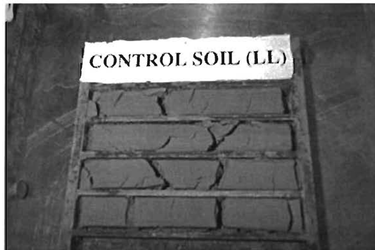
Figure C.2 Linear Shrinkage Mold of Control Soil at Liquid Limit
