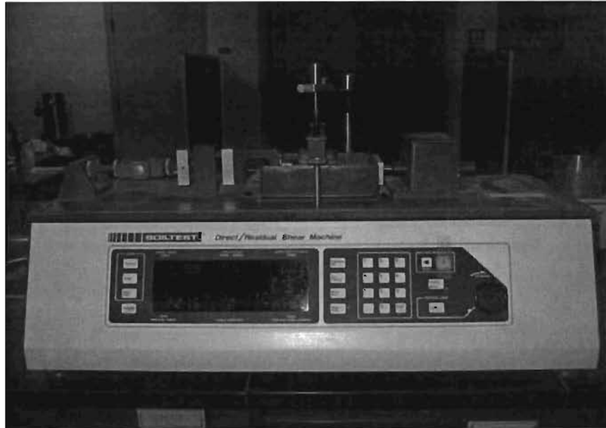
Figure 3.5 Direct Shear Test Setup
