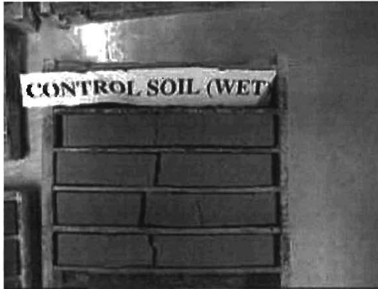
Figure C.1 Linear Shrinkage Mold of Control Soil at Optimum Moisture Content
