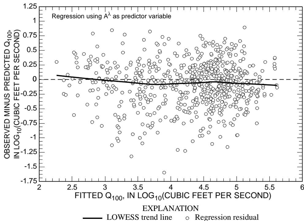
**Figure 5. Residual plot of regression of 100-year peak streamflow using power transformation of drainage area using drainage area as the only predictor variable.**
