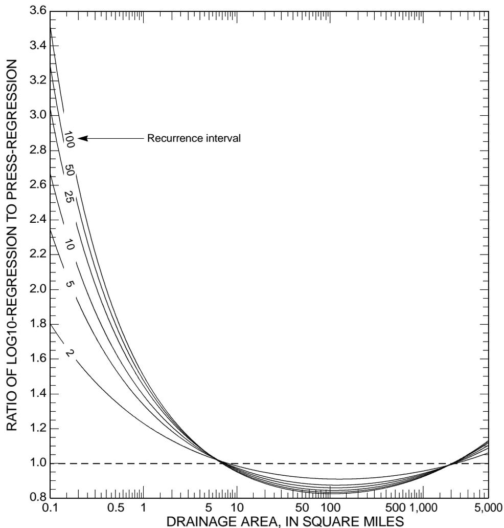
**Figure 7. Relation between bias ratio and drainage area by recurrence interval for the regressions using drainage area as the only predictor variable.**
