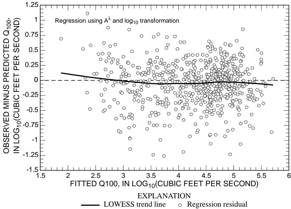
**Figure 4. Residual plot of regression of 100-year peak streamflow using power transformation of drainage area using three predictor variables.**
