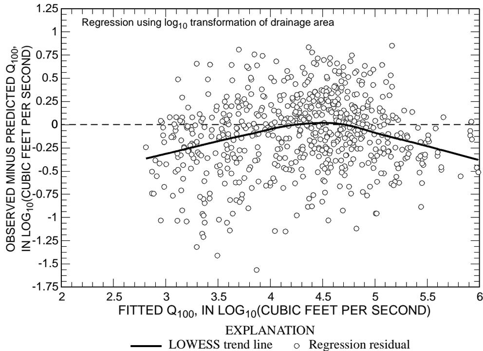
**Figure 2. Residual plot of regression of 100-year peak streamflow using  $\log_{10}$  transformation of drainage area using drainage area as the only predictor variable.**
