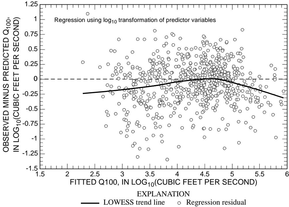
**Figure 1. Residual plot of regression of 100-year peak streamflow using  $\log_{10}$  transformation of drainage area using three predictor variables.**
