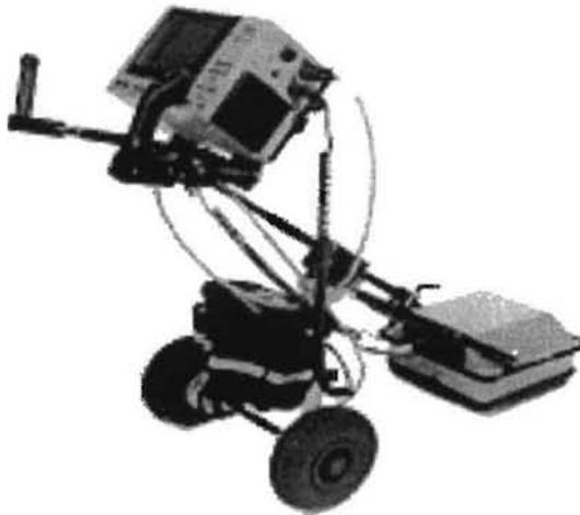
**Figure 10** SPR Scan GPR System from ERA Technology, UK
