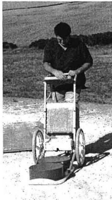
**Figure 16** GPR Cart System-Geo Radar Inc., CA.
