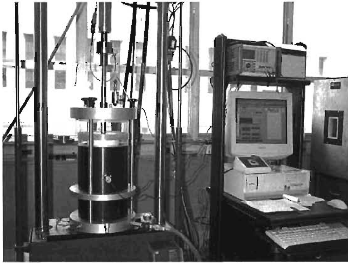
Figure 4.14 - Test Set-up for Resilient Modulus
