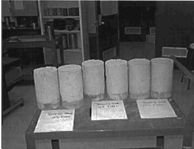
Figure 4.4 - Compacted Samples for TST Prior to Placing in the Triaxial Cells
