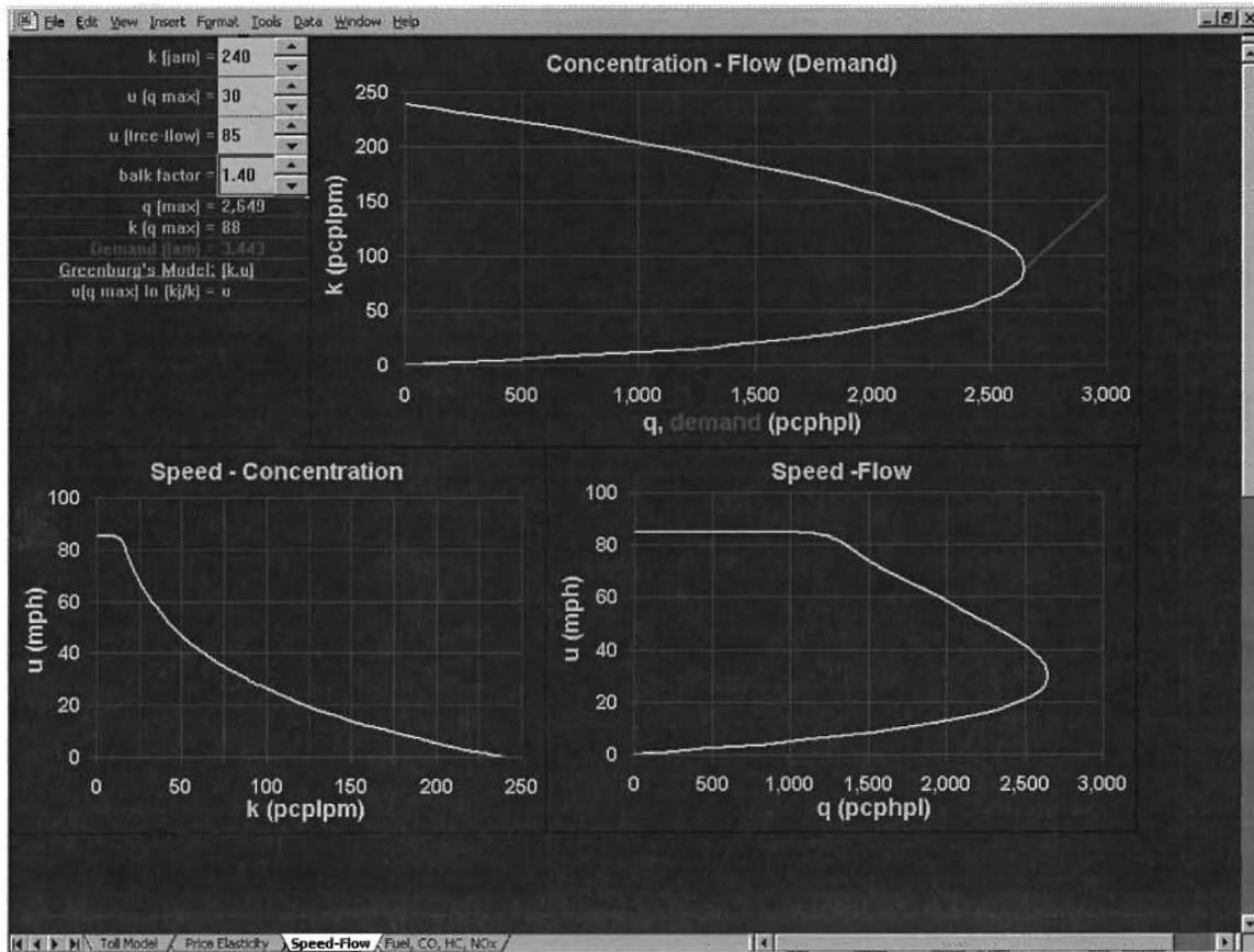
Once the above inputs are provided, the model user can observe the impacts of pricing on toll revenue, traffic conditions (including flow, speed, travel time, and delay) on both the GP and managed lanes, as well as on emission.
