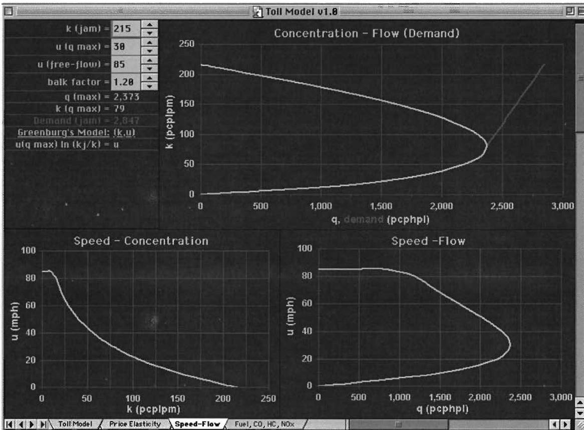
The effects of low and high input values on the Speed-Flow sheet are shown in Figures 6.7 and 6.8. The values of the above variables can be calibrated from local traffic count data. In the absence of pertinent local data, the values of 220 pcplpm, 30 mph, 75 mph, and 1.2 are recommended for the  $k$  (jam),  $u$  (q max),  $u$  (free flow), and the balk factor, respectively.<sup>4</sup>
