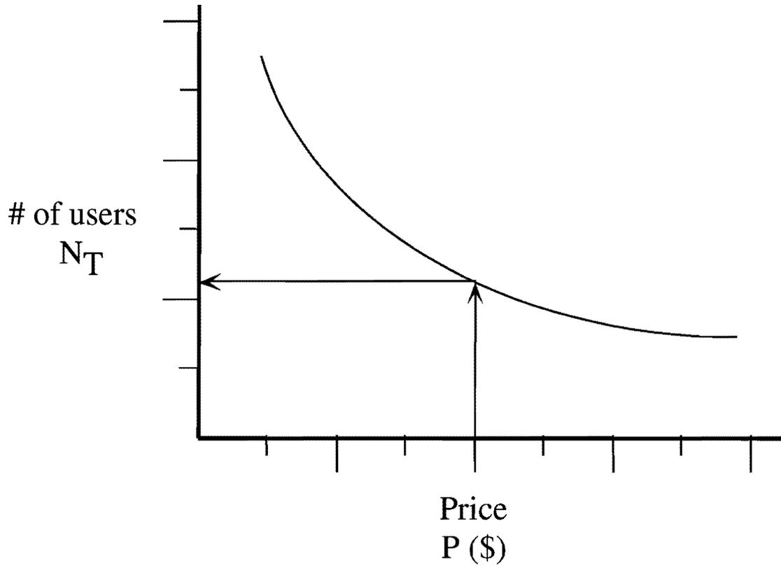
For example, on the toll lanes, the more users, the slower the speeds, and the longer the travel time. Conversely, on the GP lanes, the fewer users, the faster the speeds, and the shorter the travel time. Hence, the savings in travel time for using the toll lanes decline (See Figure 3.2).
