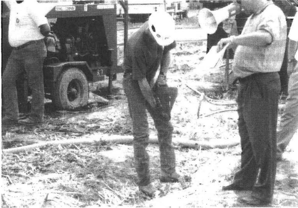
**Fig. 6.1. Flow cone test for grout.**
