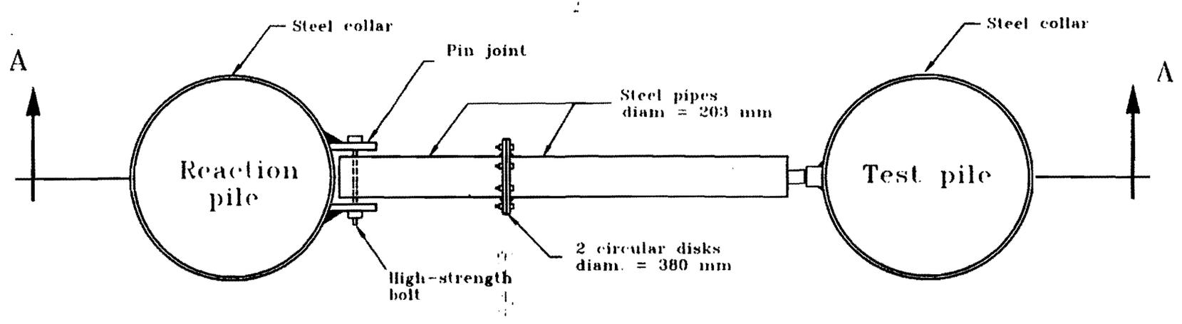
**Fig. 2.10. Detail of the loading test reaction system**
