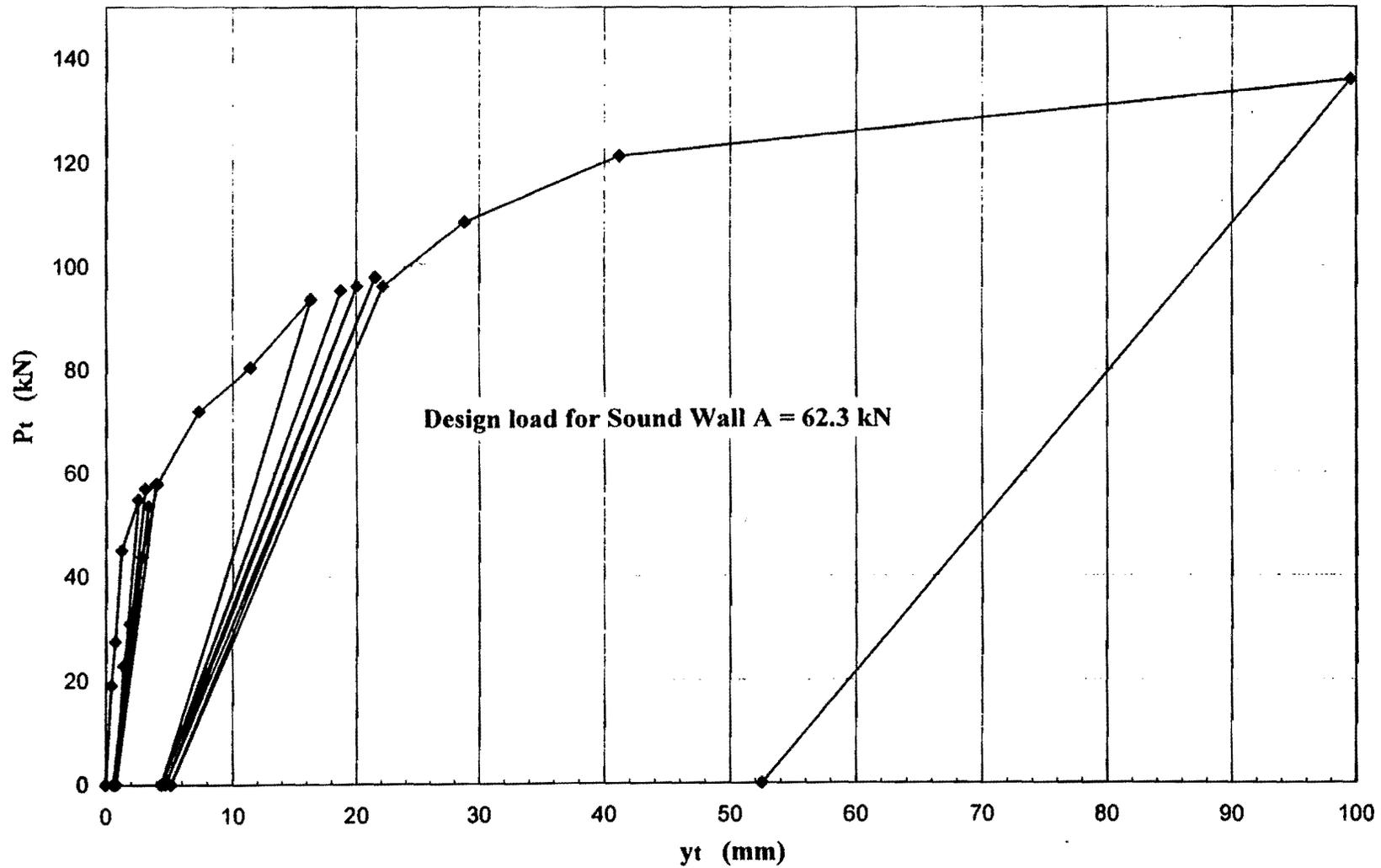
**Fig. 2.14. Lateral load-deflection curve for Test Pile West
