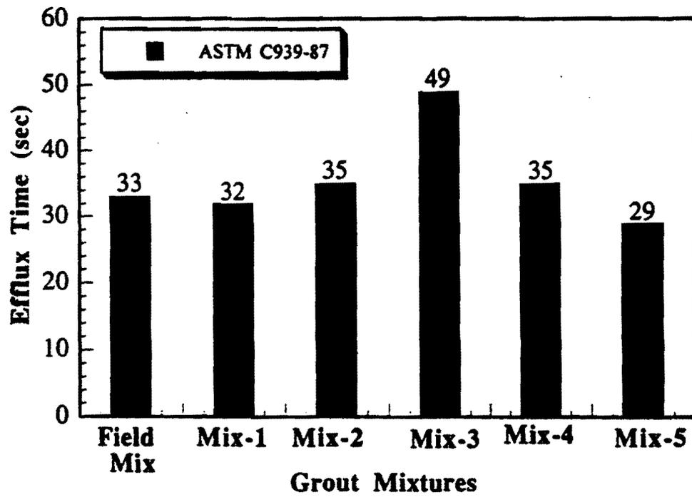
**Fig. 5.1. Variation of efflux time with fiber type, silica fume and fluidizer**
