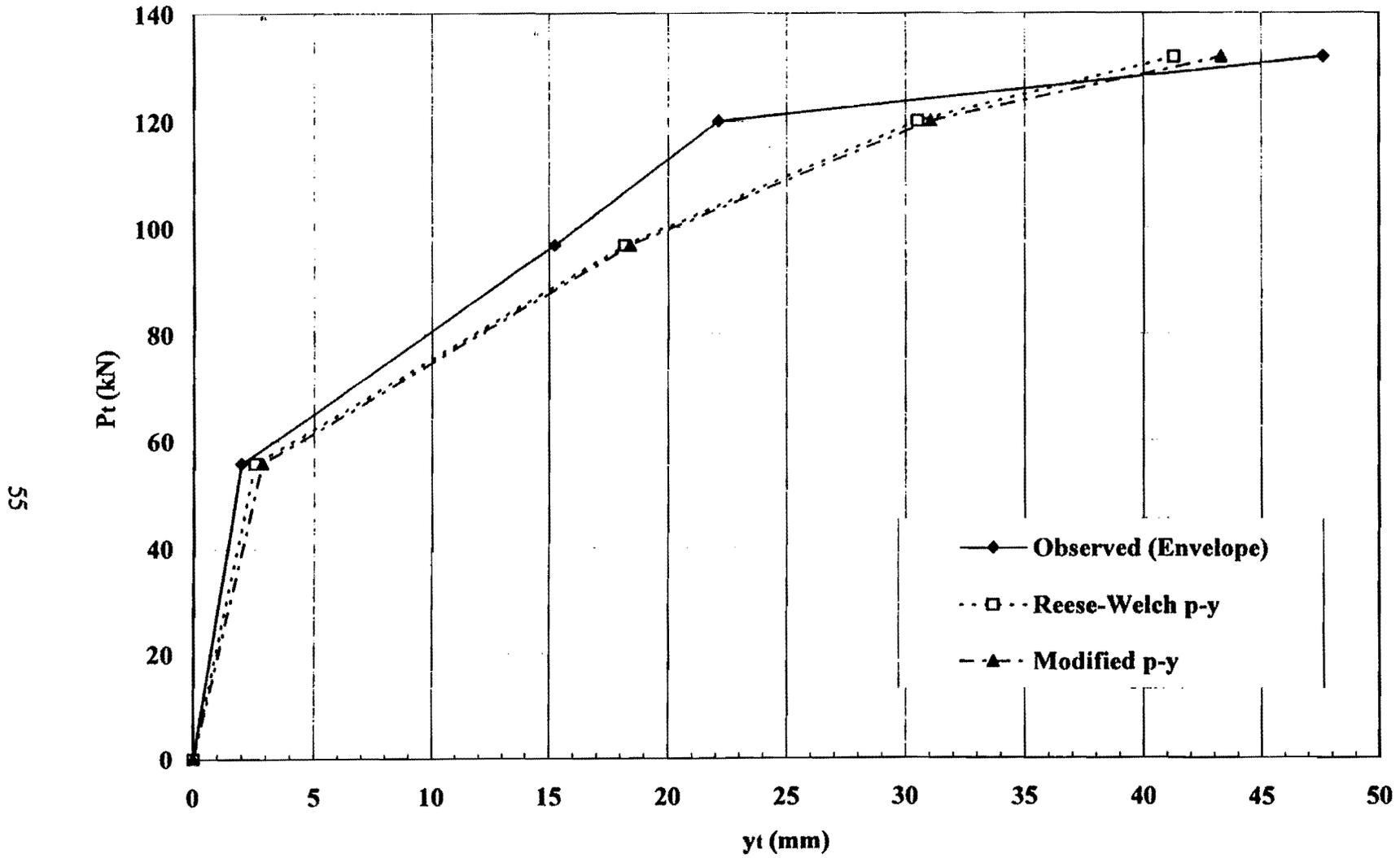
**Fig. 3.5. Comparison of computed load-deflection curves for Pile East**
