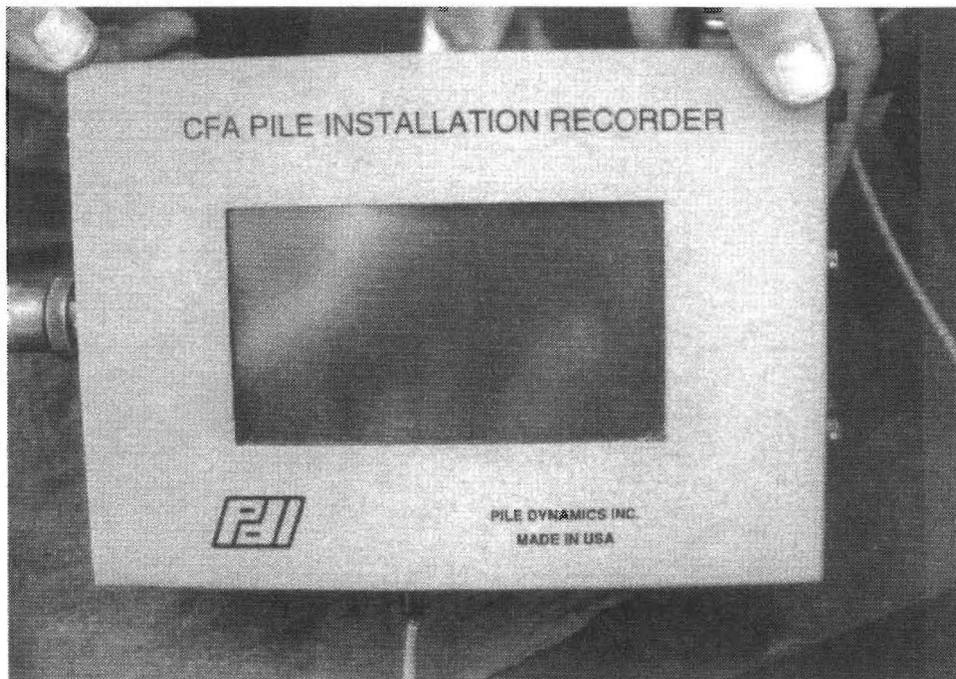
**Fig. 6.6. View of output display for automated monitoring instruments.**
