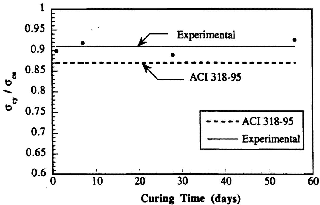
Fig. 5.5. Variation of compressive and tensile strengths of various grout mixes
