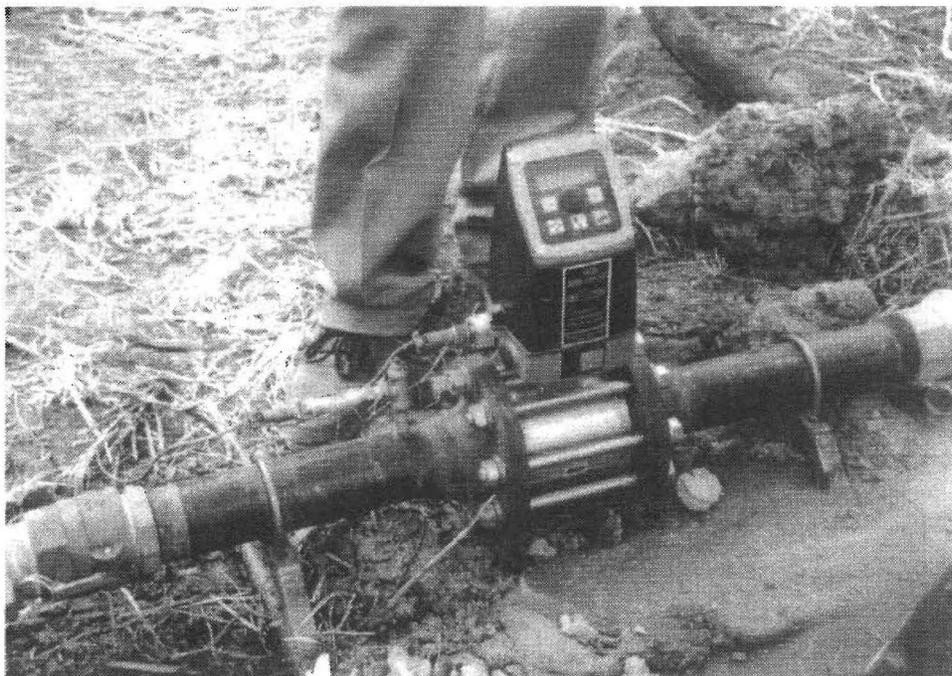
**Fig. 6.4. View of flowmeter and pressure transducer in grout line.**
