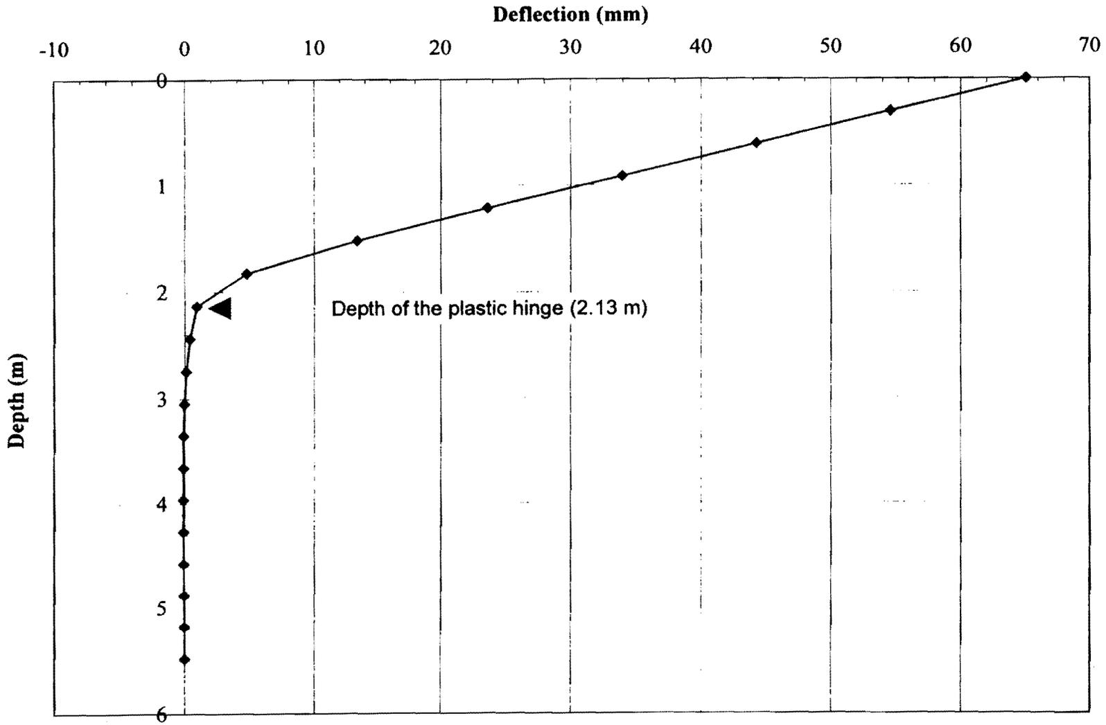
Fig. A.4. Corrected profile of permanent lateral displacement along Pile East
