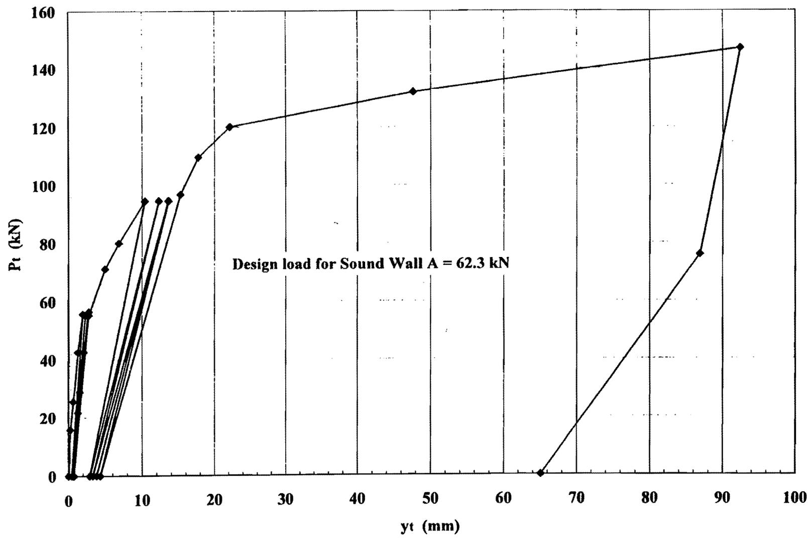
**Fig. 2.13. Lateral load-deflection curve for Test Pile East (Diameter = 457 mm and Length = 6.1 m)**
