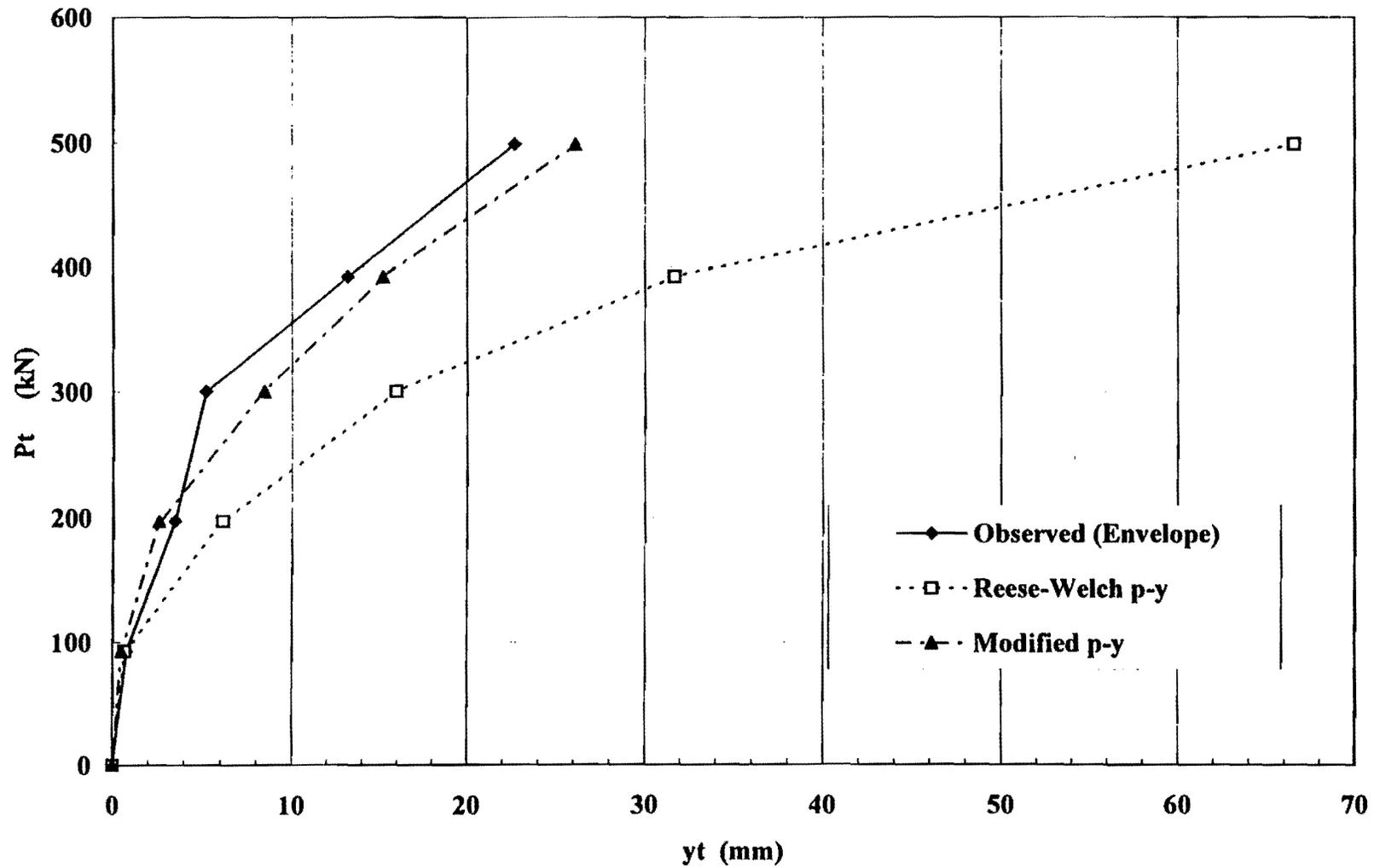
Fig. 3.7. Comparison of computed load-deflection curves for Pile South
