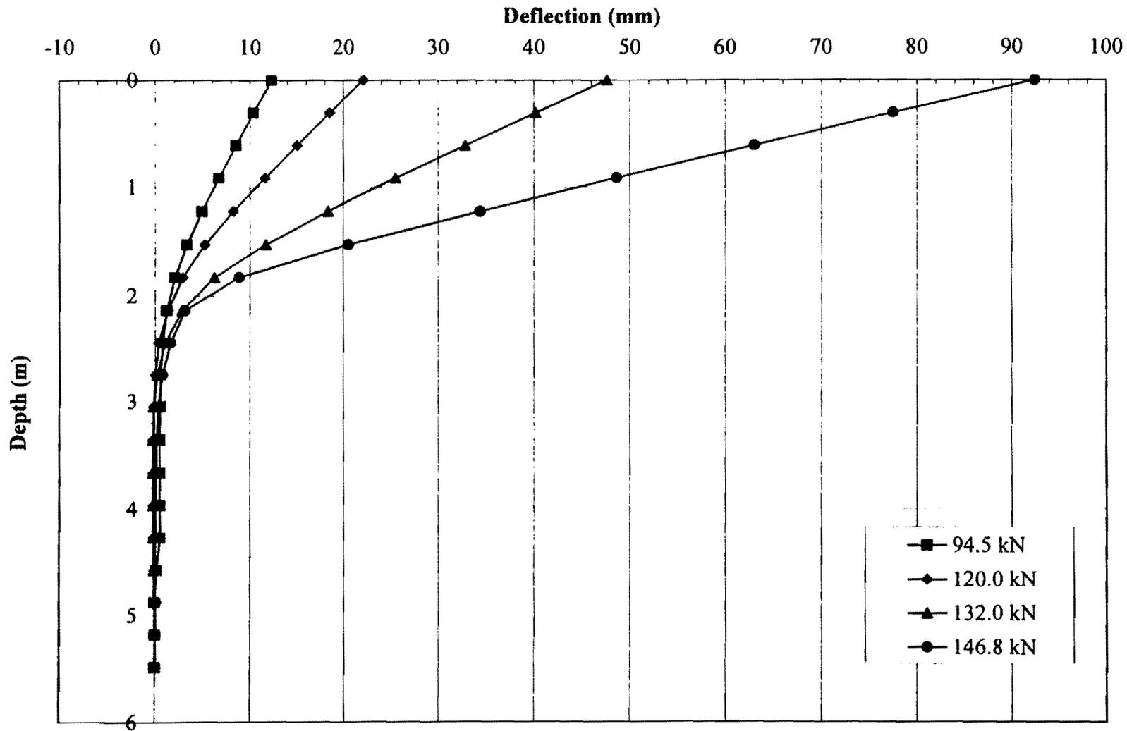
**Fig. A.3. Corrected profile of lateral displacement along Pile East
