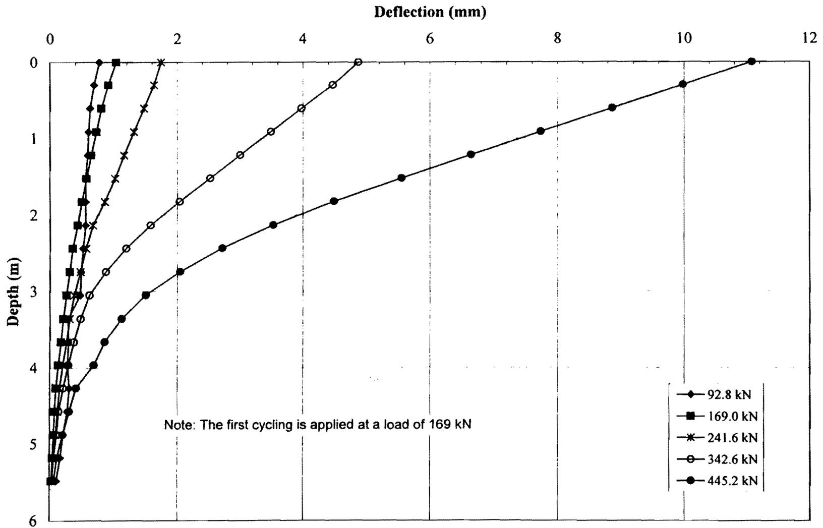
Fig. A.9. Measured profile of lateral deflection along Pile South
