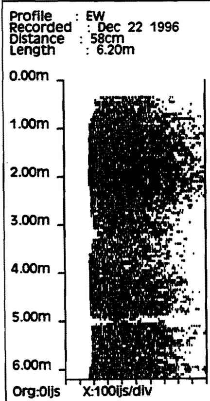
**Fig. A.18. Cross-hole ultrasonic log of Test Pile South**
