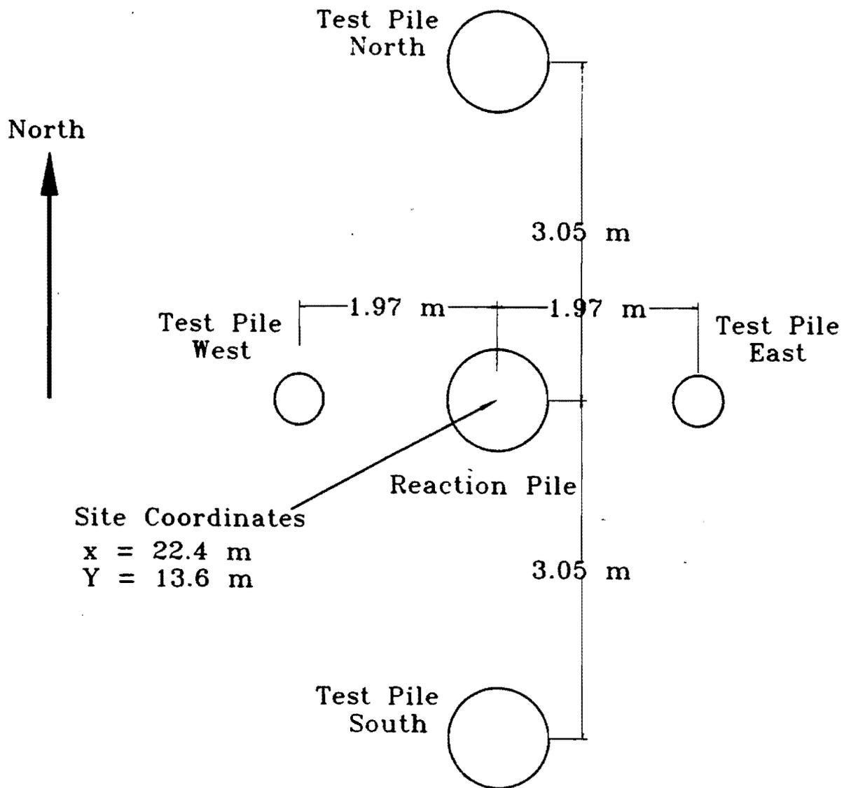
**Fig. 2.4. Arrangement of the test and reaction piles**
