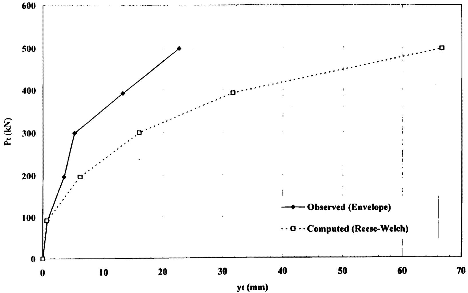
**Fig. 3.3. Observed and computed load-deflection curves for Pile South**
