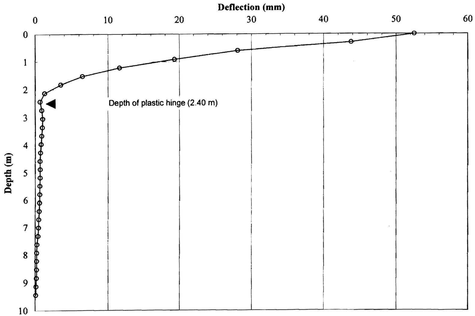
**Fig. A.8. Corrected profile of permanent lateral displacement along Pile West**
