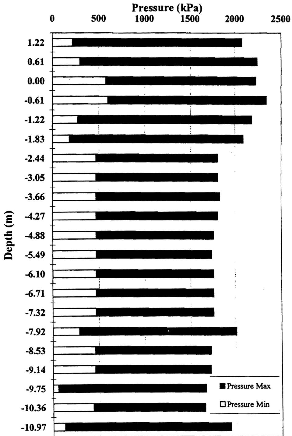
**Fig. 2.8. Records of maximum and minimum pump grout pressure vs. depth for Pile Test North**
