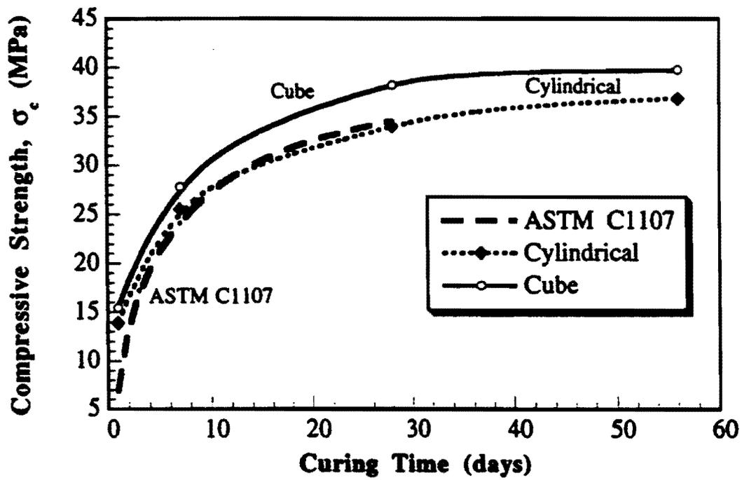
Fig. 5.3. Variation of compressive strength with curing time for the field grout mix and comparison to ASTM C1107-91
