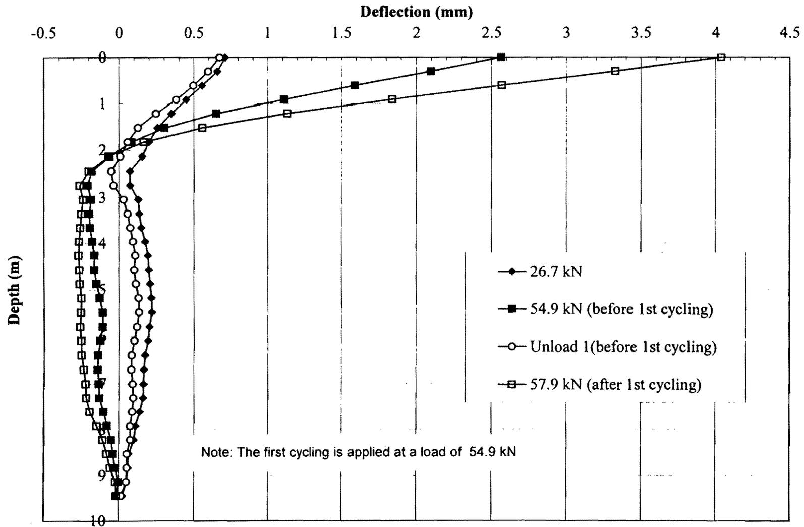
**Fig. A.6. Corrected profile of lateral displacement along Pile West
