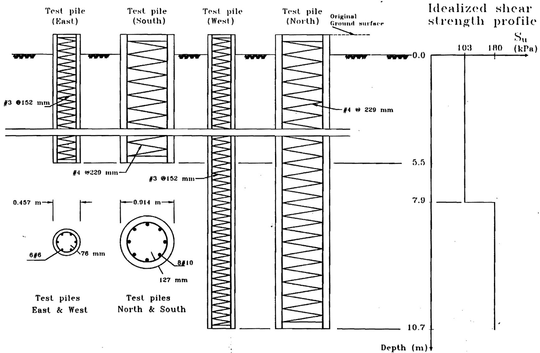
Fig. 2.5. Details of the pile reinforcement and the idealized shear strength profile
