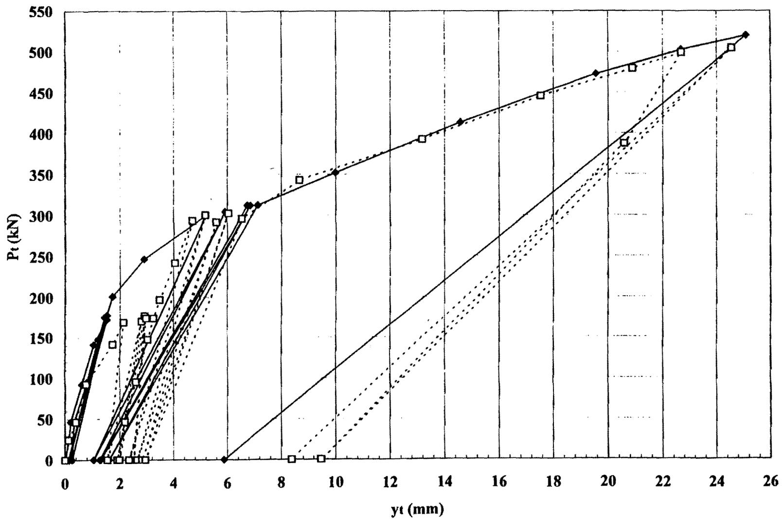
Fig. 2.18. Comparison of lateral load-deflection curves for Test Piles South and North
