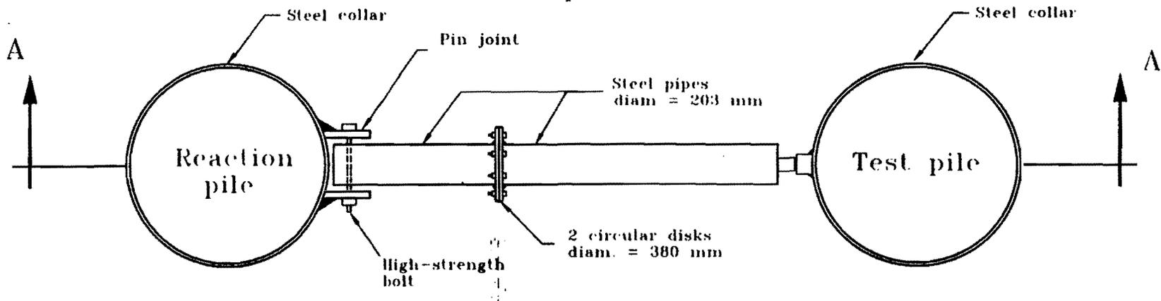
**Fig. 2.10. Detail of the loading test reaction system**
