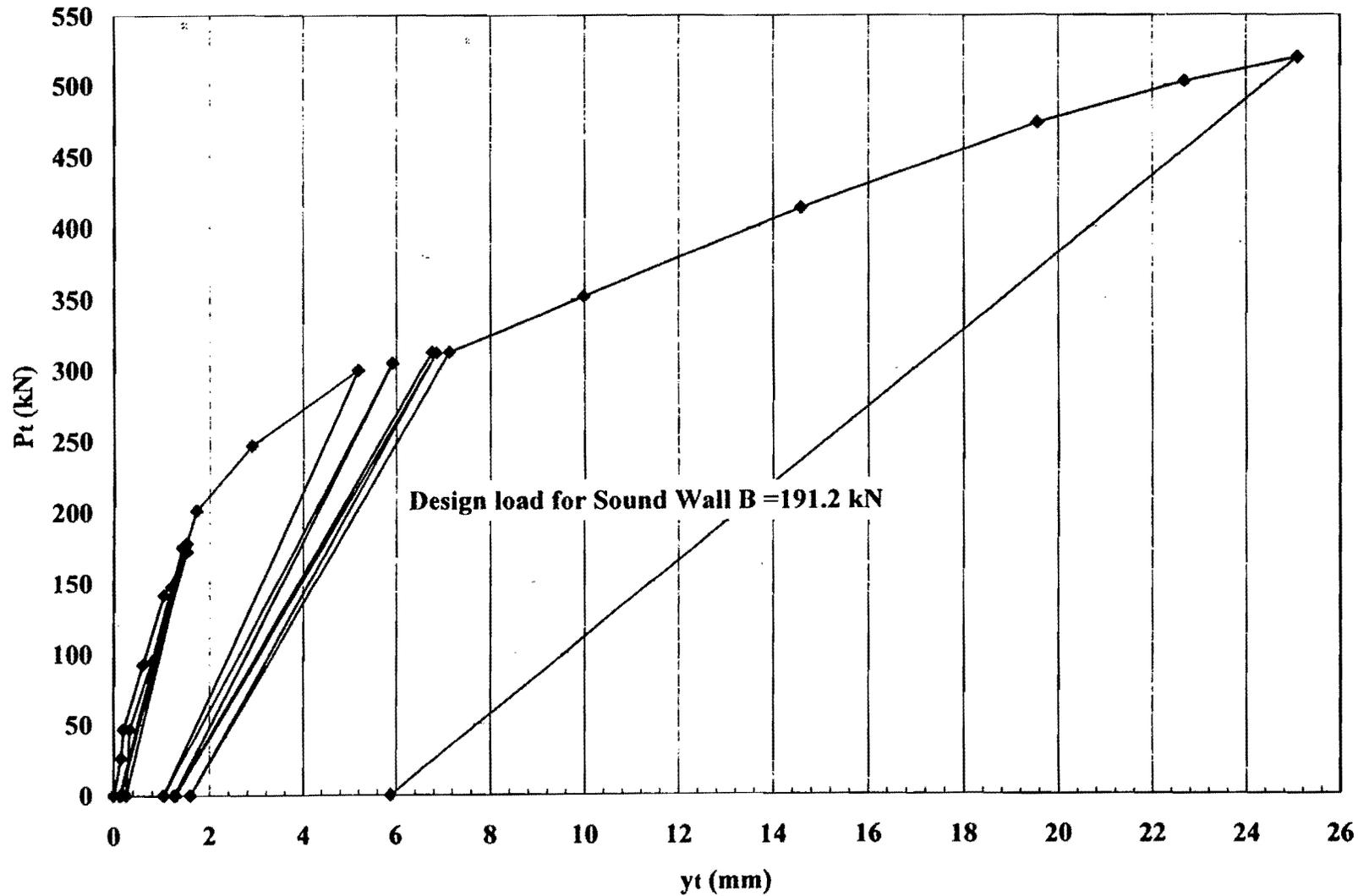
**Fig. 2.16. Lateral load-deflection curve for Test Pile North
