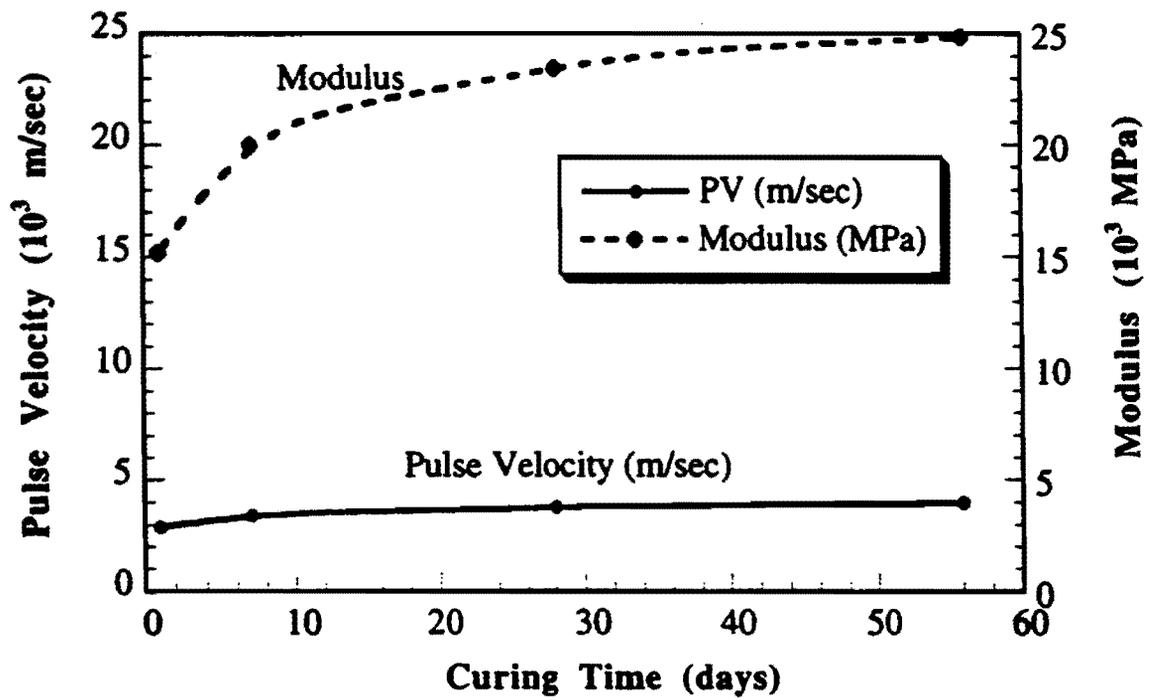
Fig. 5.2. Variation of compressive modulus and pulse velocity of the field grout mix with curing time
