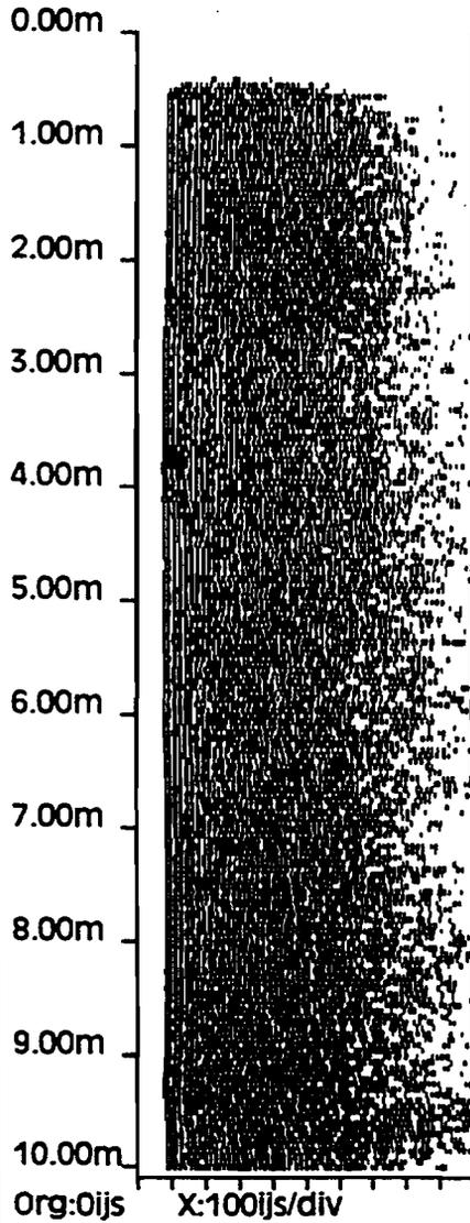
Fig. A.16. Cross-hole ultrasonic log of Test Pile West
