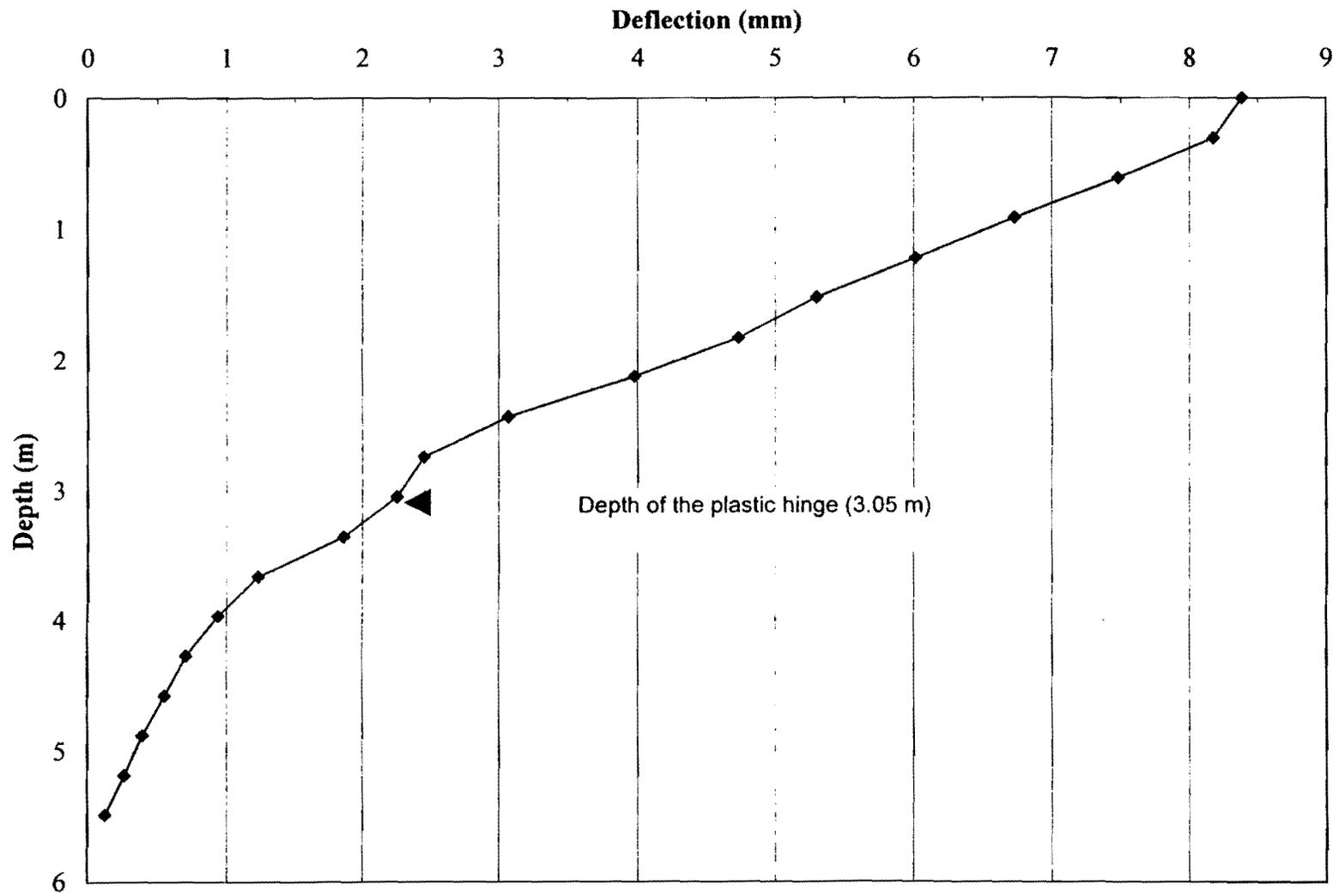
**Fig. A.11. Corrected profile of permanent lateral displacement along Pile South**
