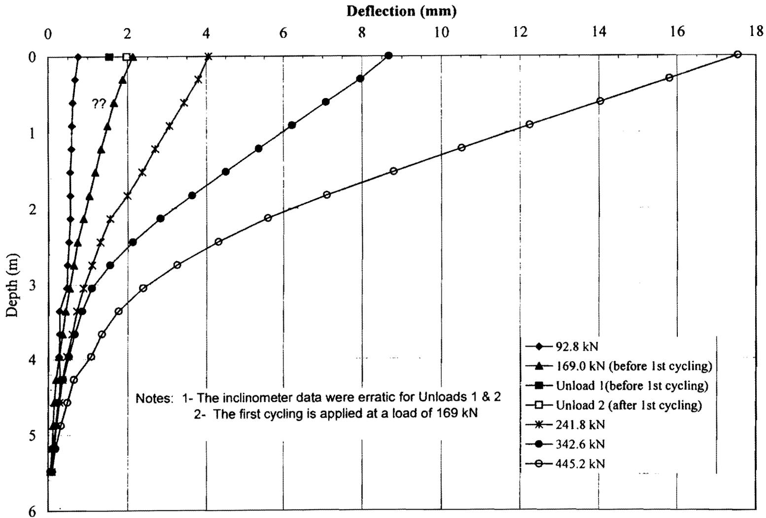
Fig. A.10. Corrected profile of lateral displacement along Pile South
