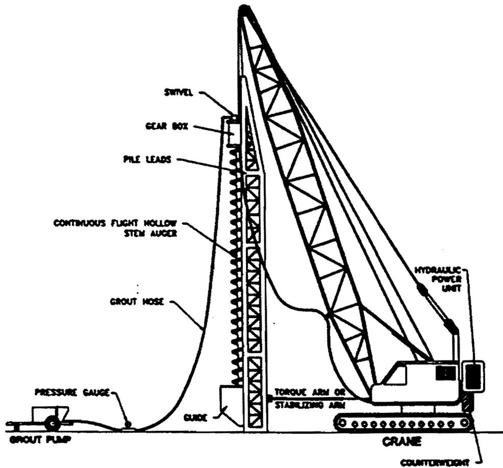
Fig. 2.6. Schematic arrangement for the CFA pile rig, after Deep Foundations Institute (1994)
