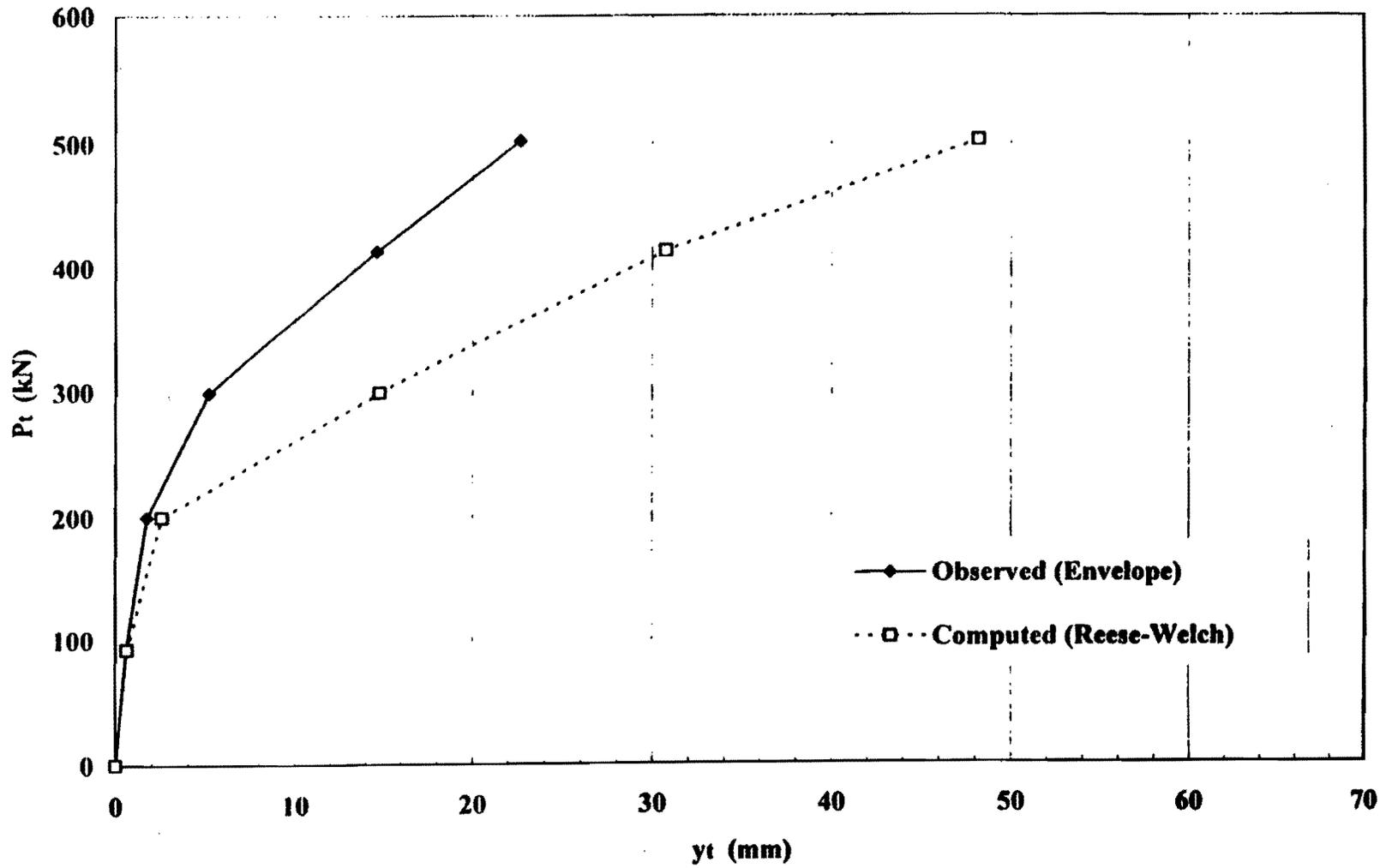
**Fig. 3.4. Observed and computed load-deflection curves for Pile North**
