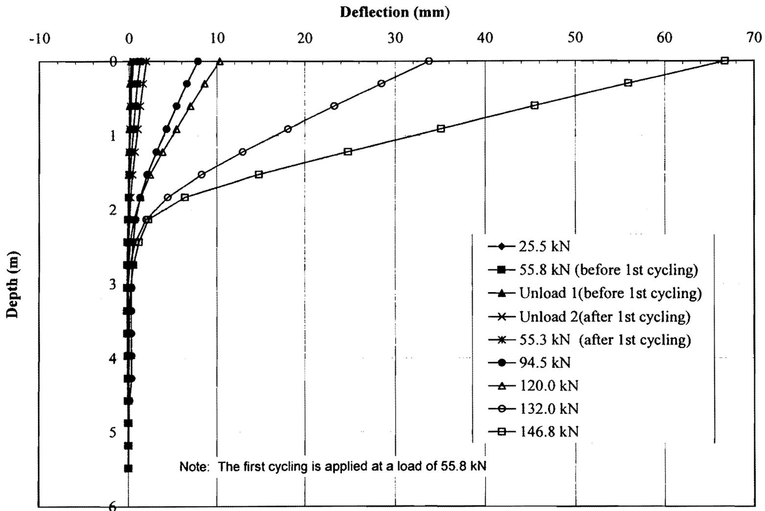
**Fig. A.1. Measured profile of lateral displacement along Pile East**
