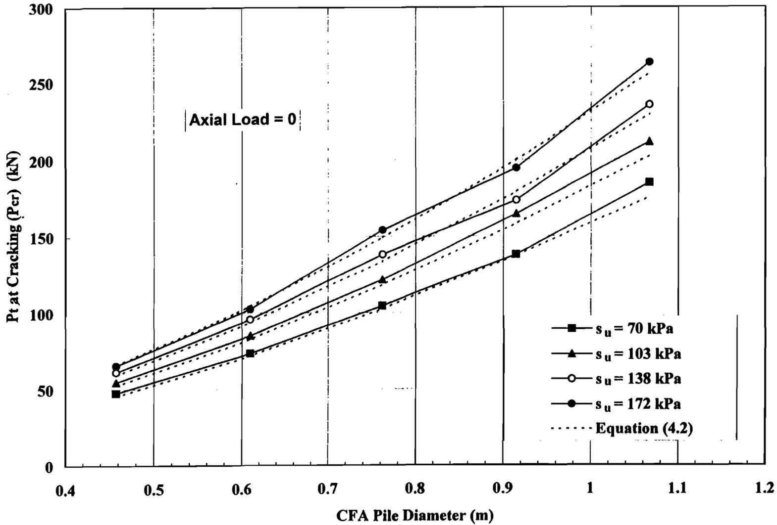
**Fig. 4.1. Relationship between ground-line shear at cracking, pile diameter and  $s_u$**
