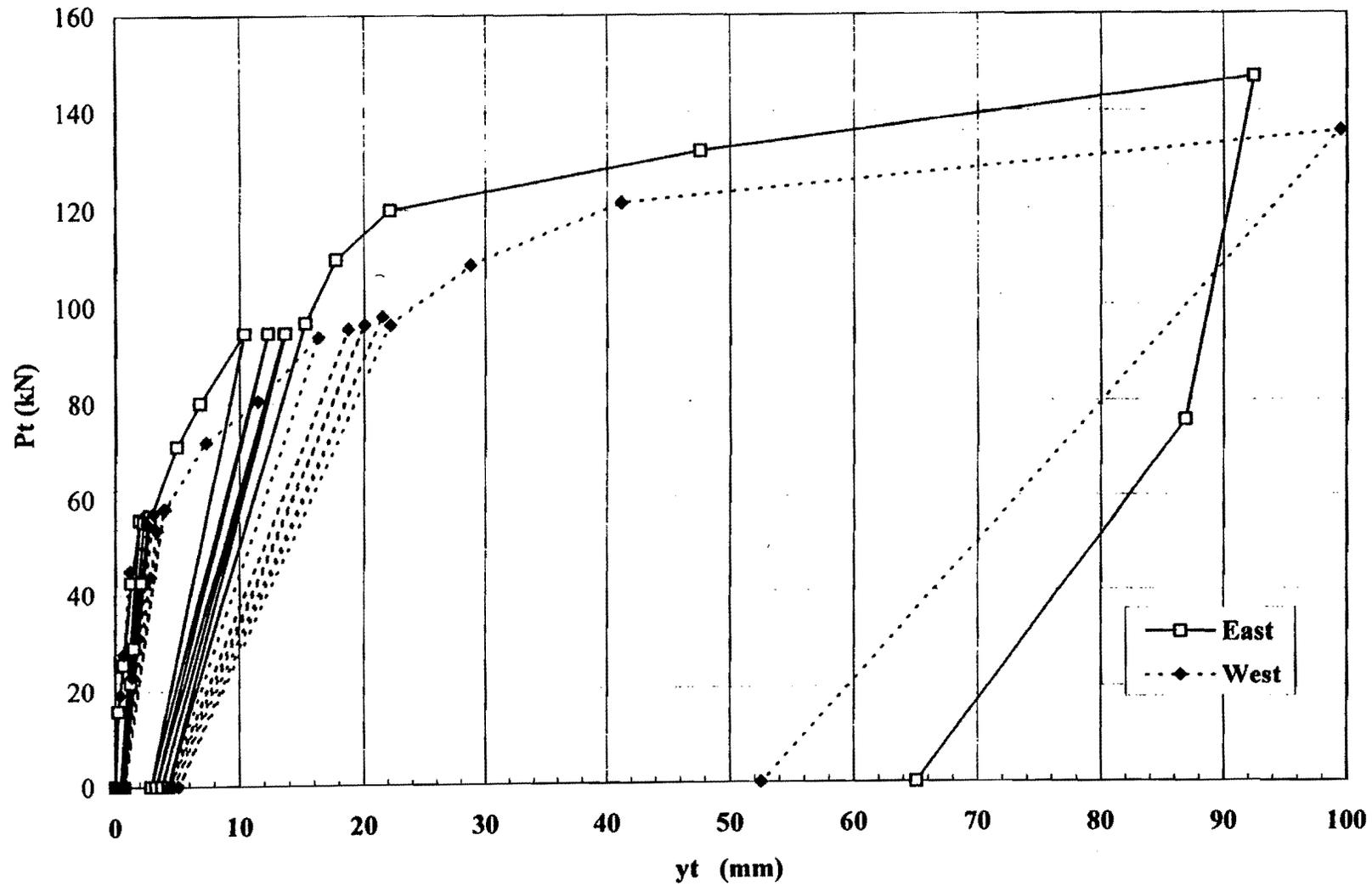
Fig. 2.17. Comparison of the lateral load-deflection curves for Test Piles East and West
