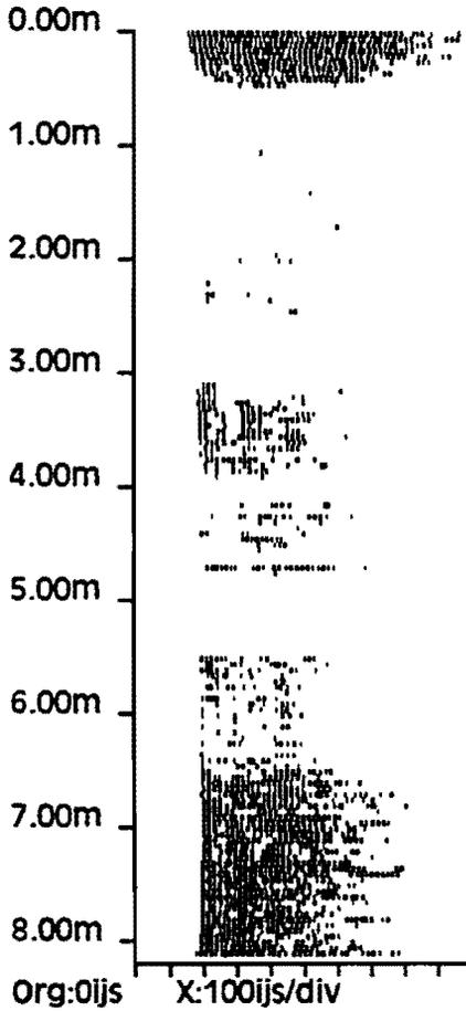
Fig. A.20. Cross-hole ultrasonic log of Test Pile North
