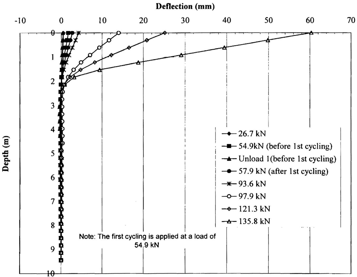
**Fig. A.5. Measured profile of lateral defelection along Pile West**
