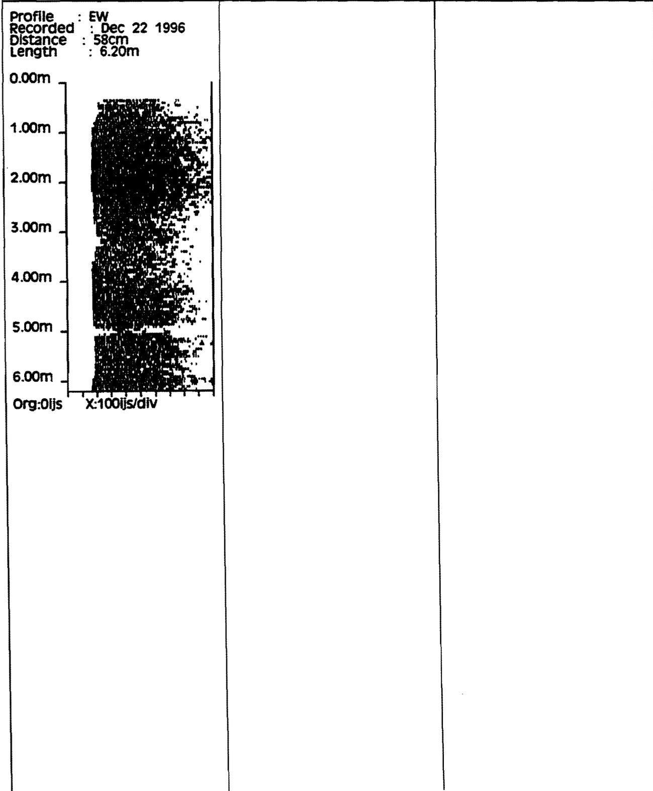
**Fig. A.18. Cross-hole ultrasonic log of Test Pile South**
