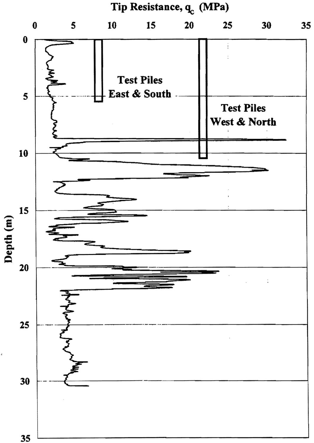
**Fig. 2.2. Results of electronic CPT log**
