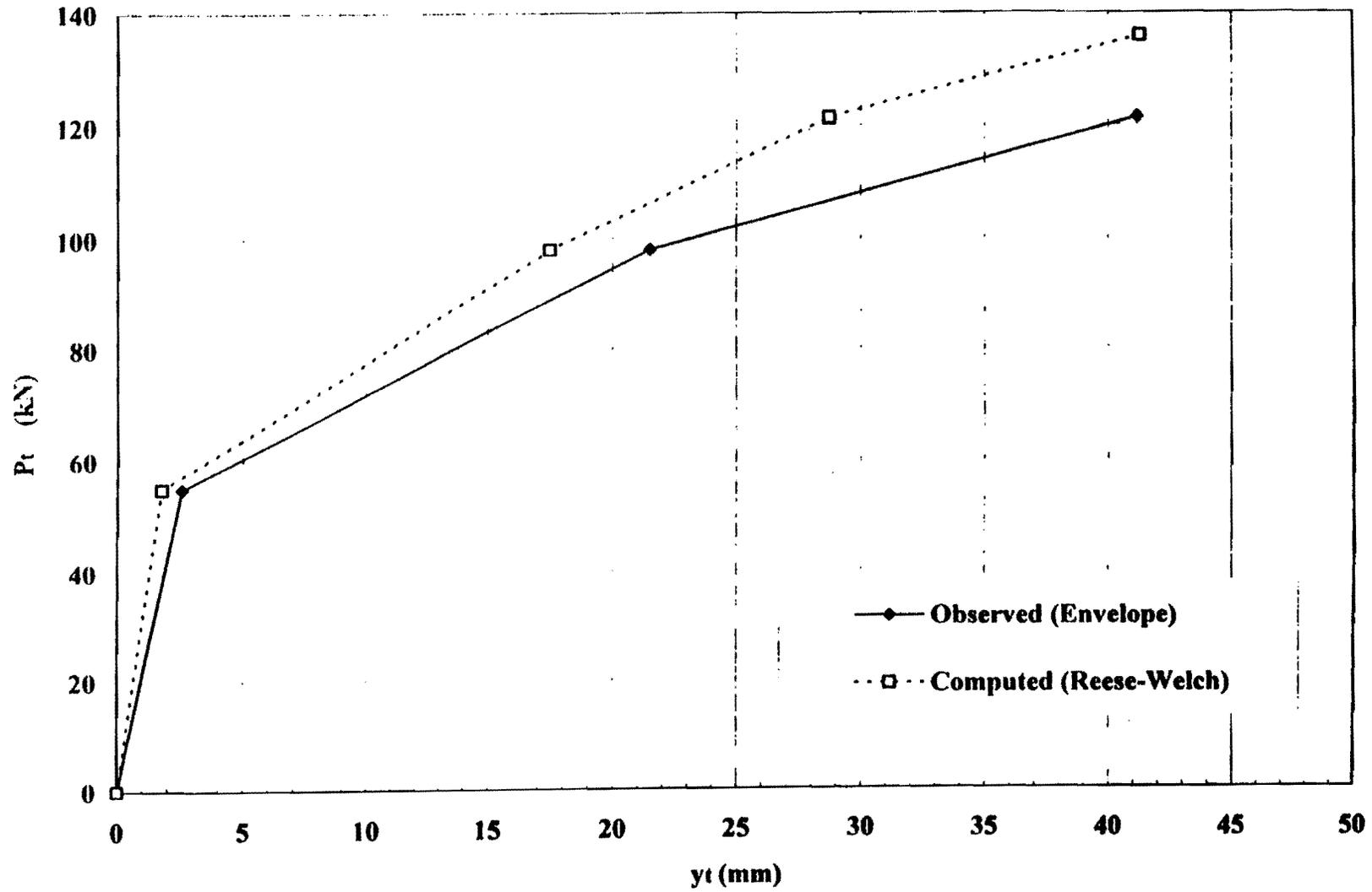
Fig. 3.2. Observed and computed load-deflection curves for Pile West
