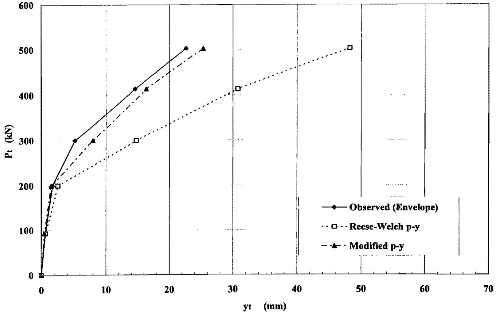
Fig. 3.8. Comparison of computed load-deflection curves for Pile North
