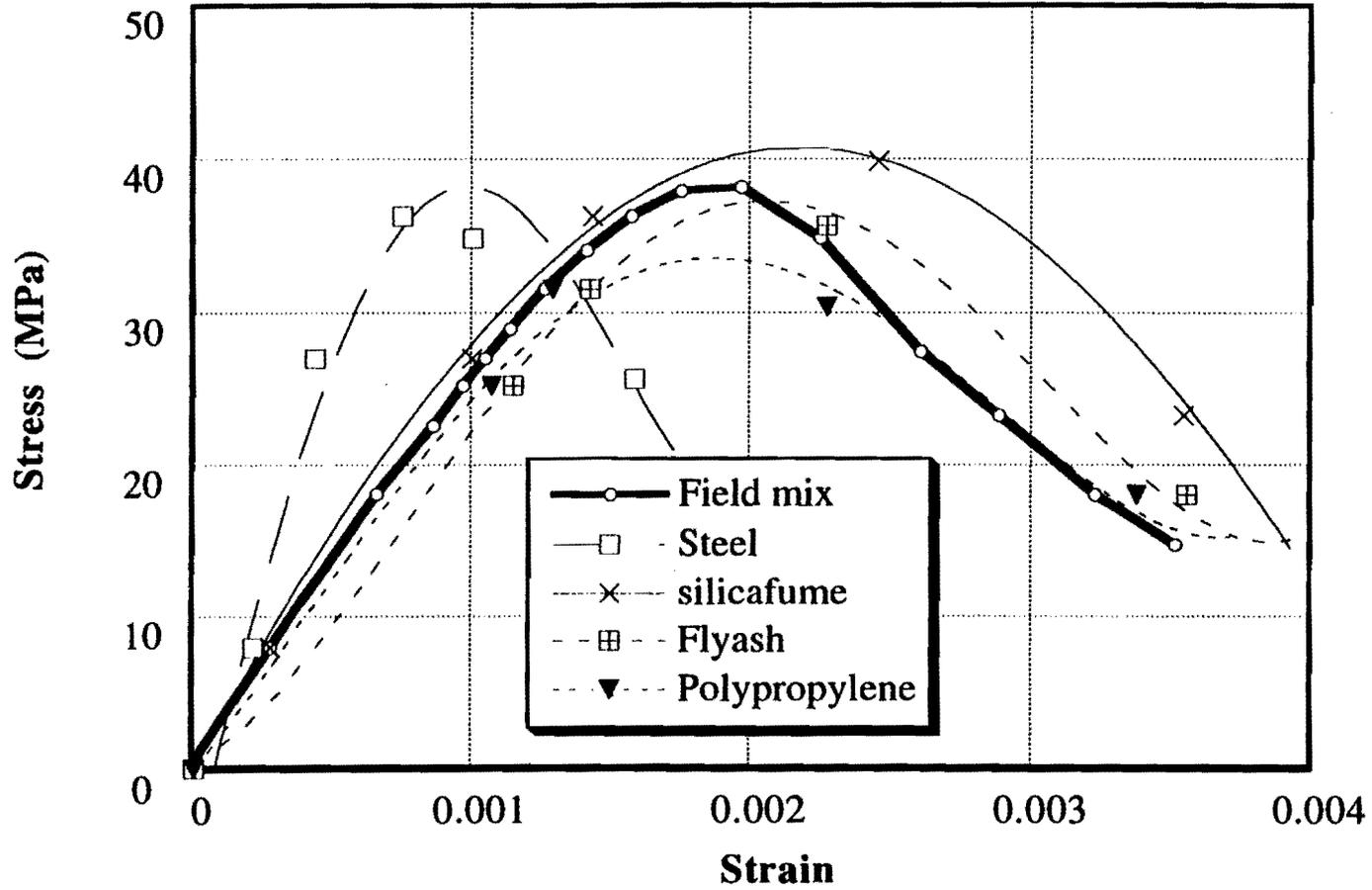
**Fig 5.7 Compressive Stress-Strain Relationships for Various Grout Mixtures after 28 days of Curing**
