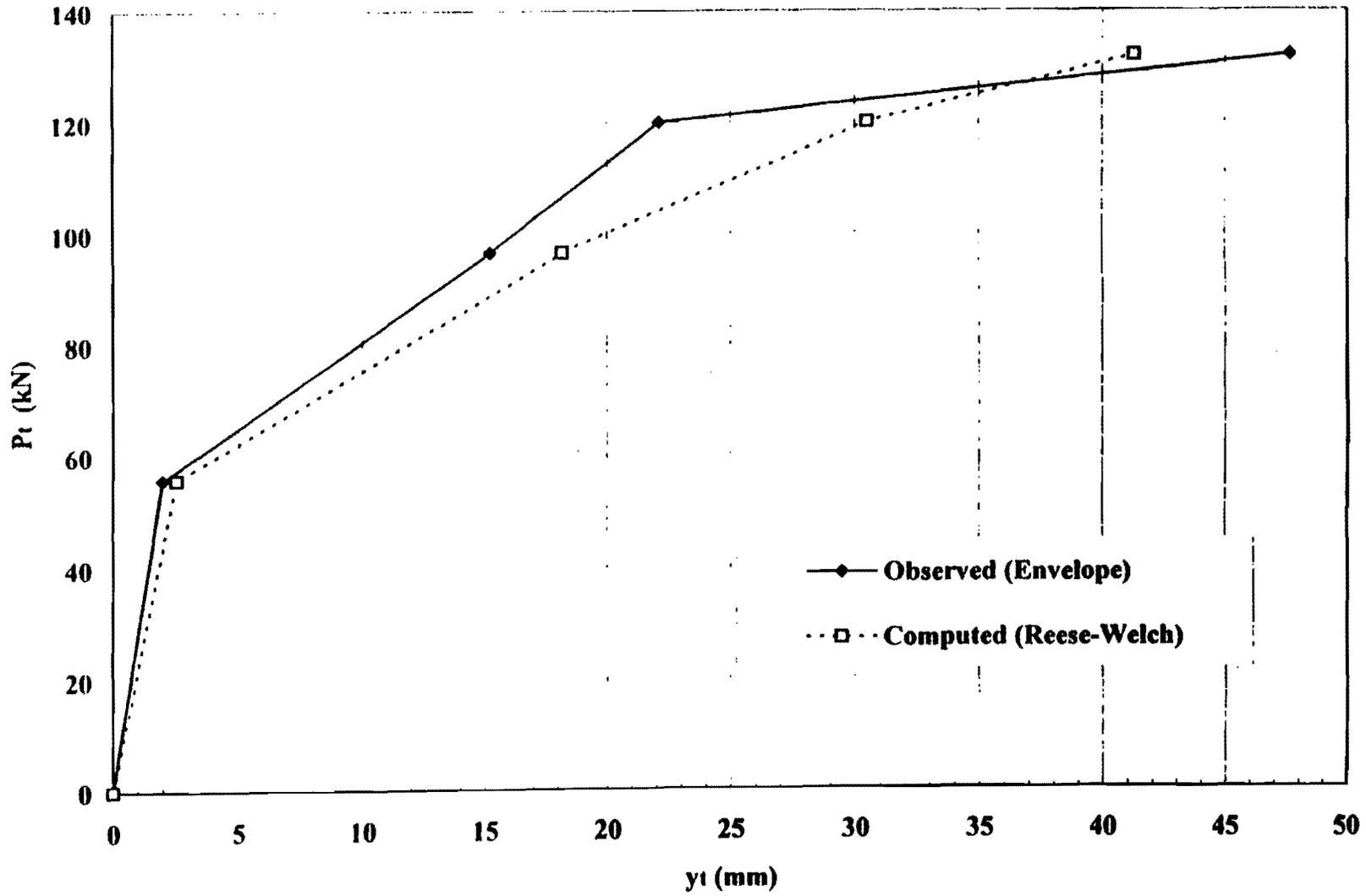
Fig. 3.1. Observed and computed load-deflection curves for Pile East
