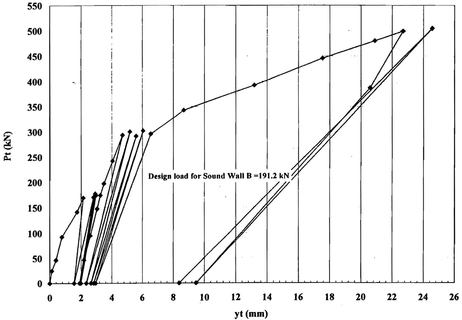
**Fig. 2.15. Lateral load-deflection curve for Test Pile South
