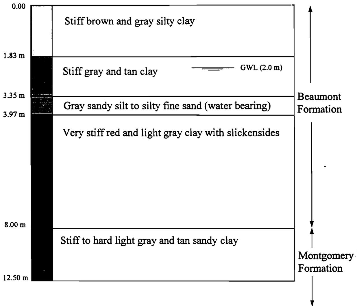
**Fig. 2.1. General soil profile for the test site**
