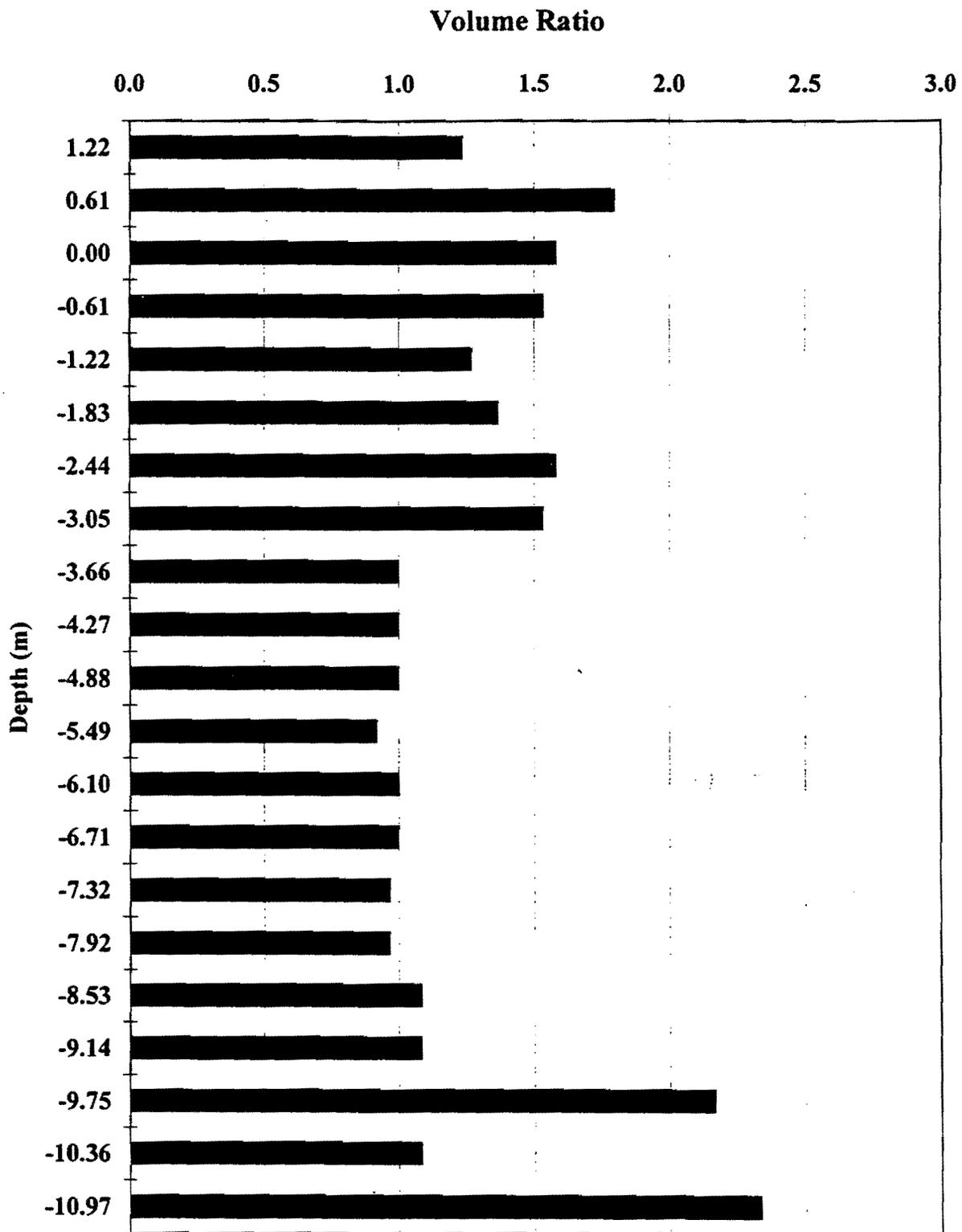
**Fig. 2.7. Record of grout volume ratio vs. depth for Test Pile North**
