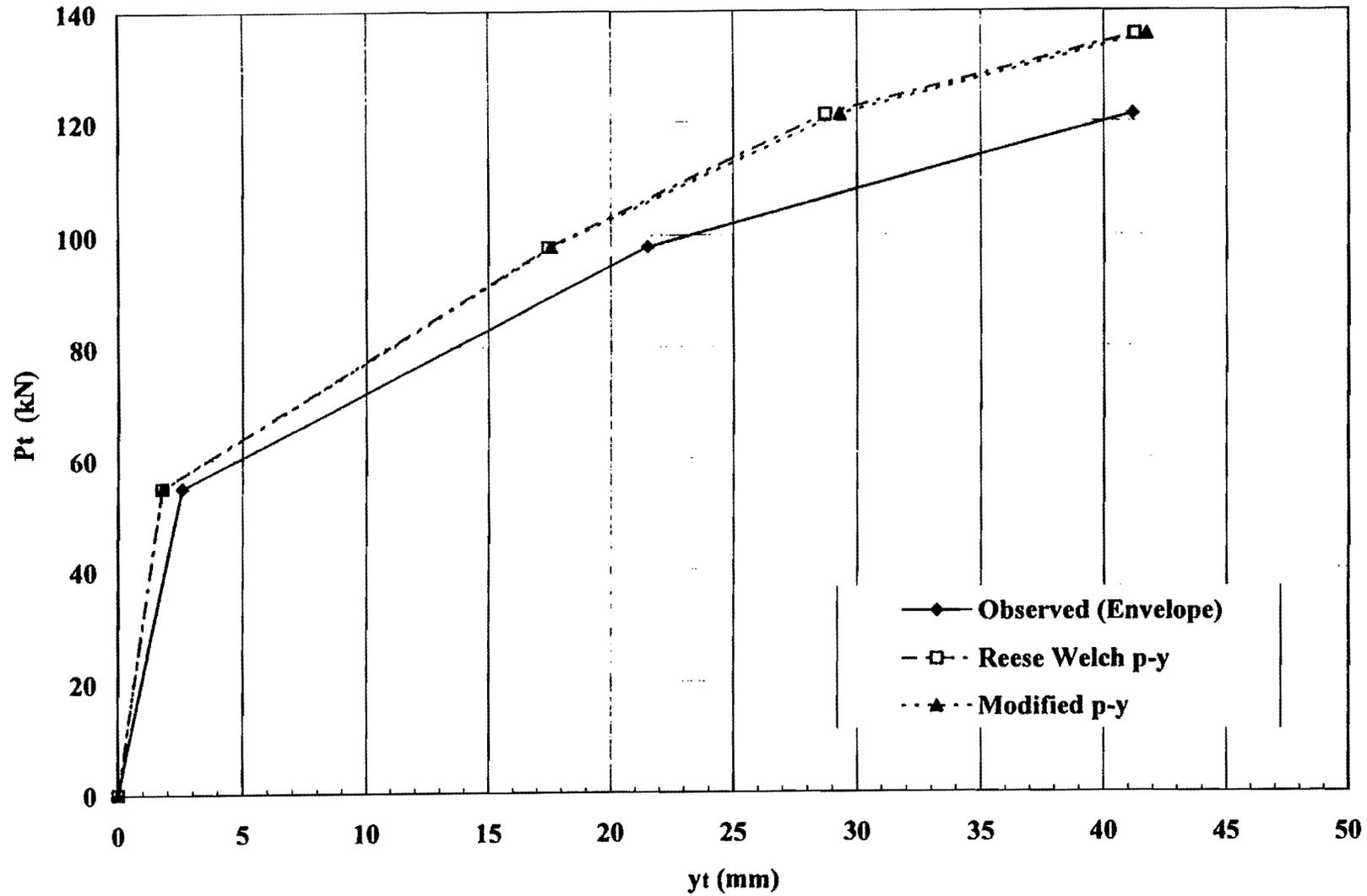
Fig. 3.6. Comparison of computed load-deflection curves for Pile West
