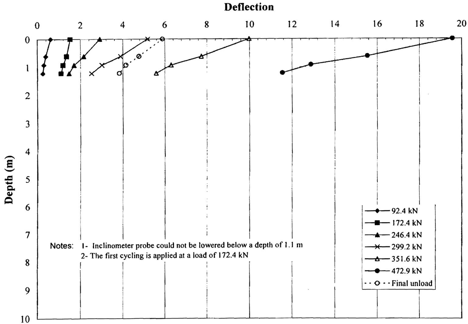
**Fig. A. 12. Measured profile of lateral displacement along Pile North**
