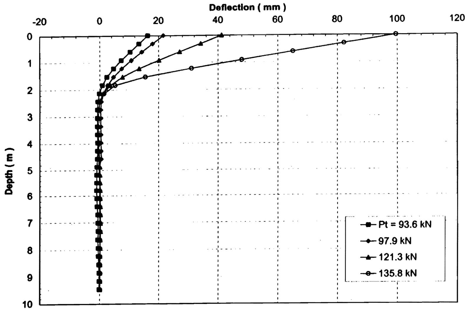
Fig. A.7. Corrected profile of lateral displacement along Pile West
