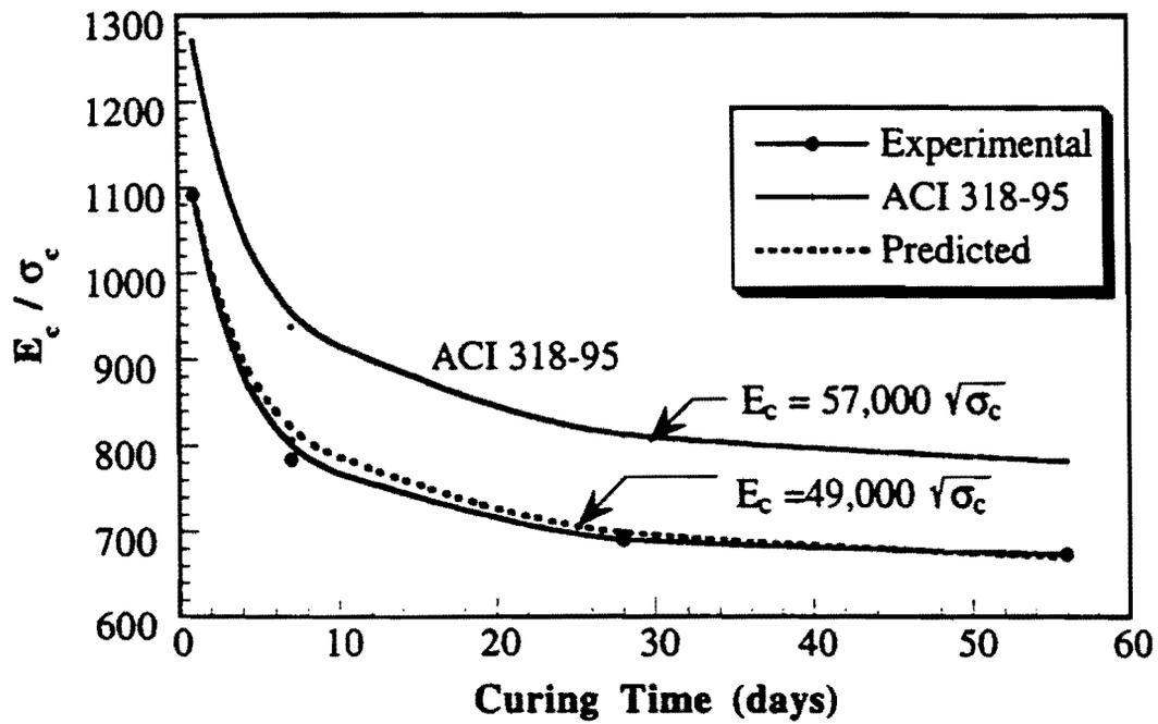
Fig. 5.6. Variation of modulus-to-strength ratio with curing time
