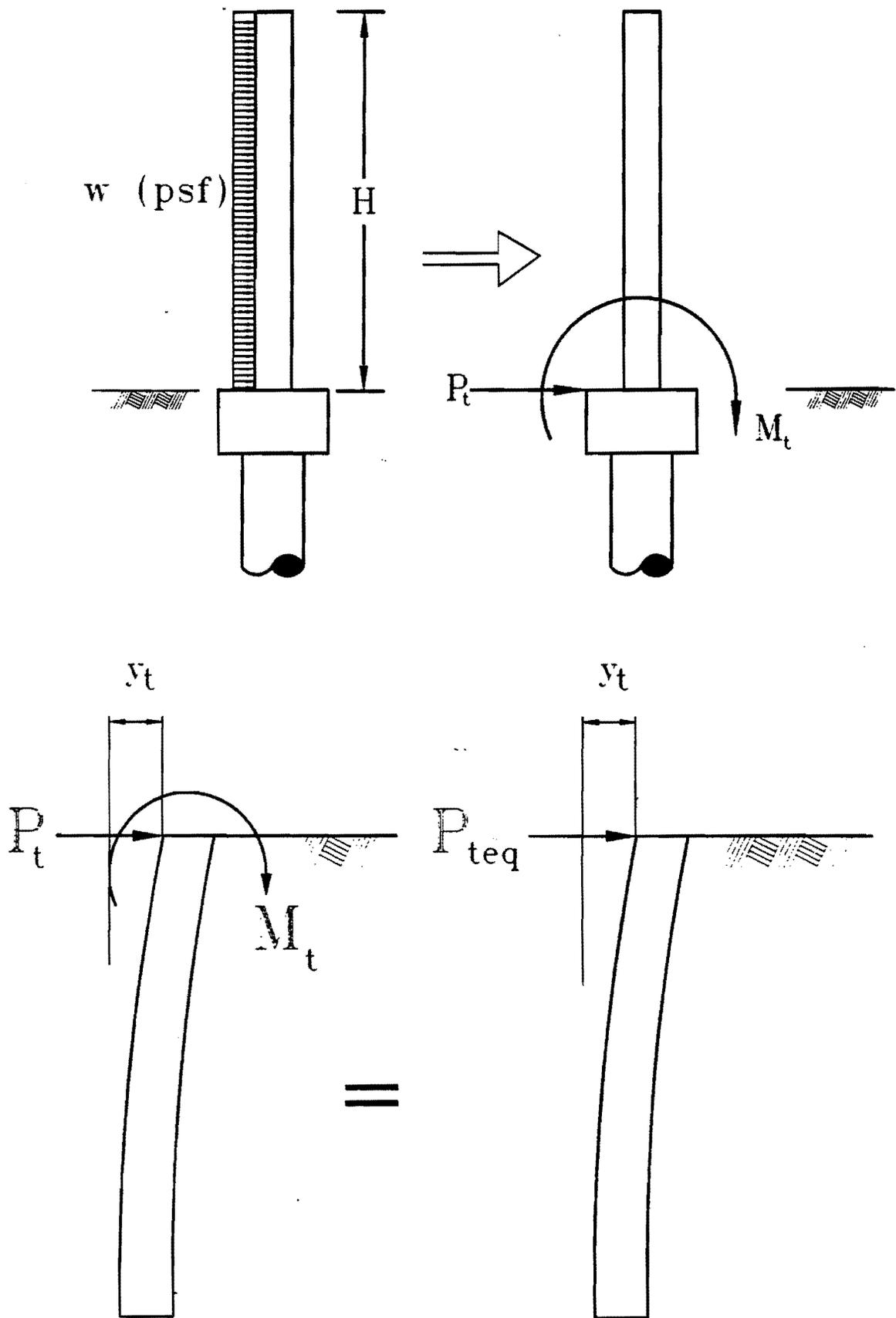
**Fig. 2.11. A schematic diagram of the concept of design load determination**
