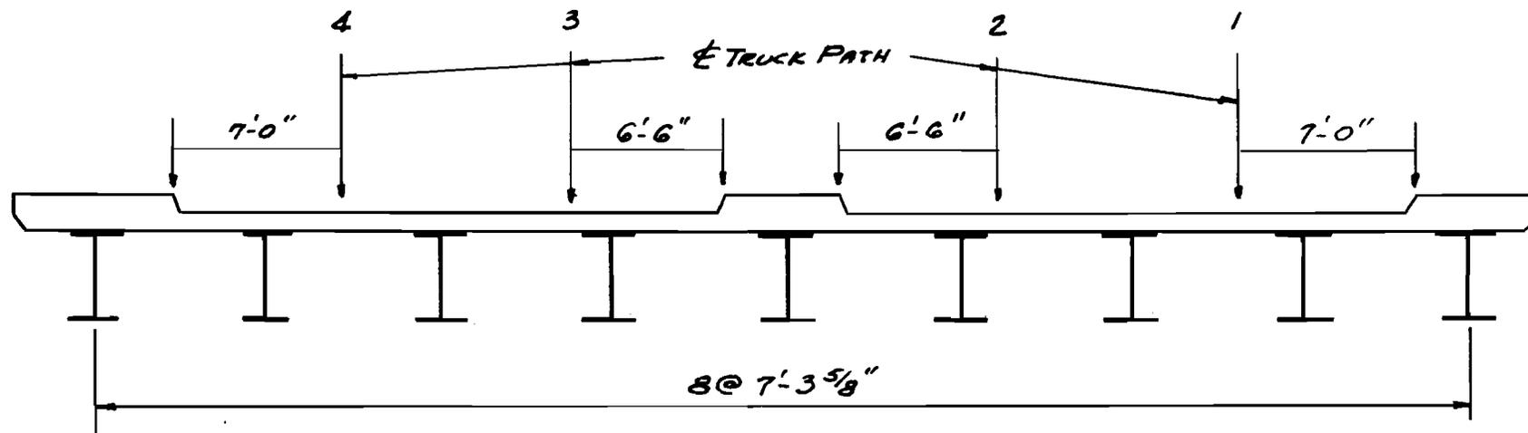
Figure 4 Truck Position During Test Runs
