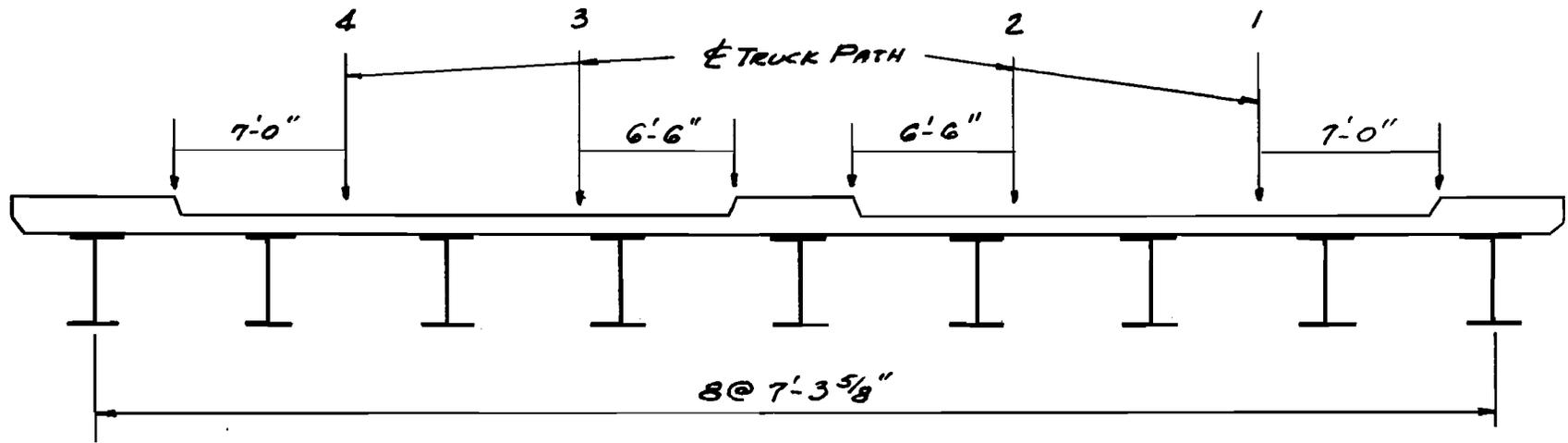
Figure 4 Truck Position During Test Runs
