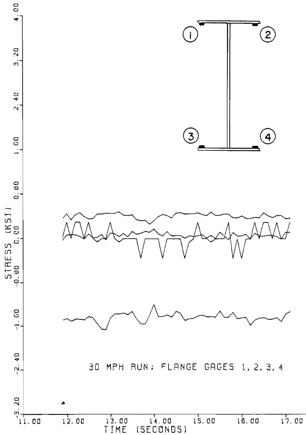
Fig. 3.1 Faulty behavior of gage 4.
