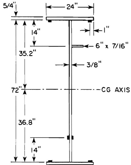
Fig. 3.3 Section with stiffener
