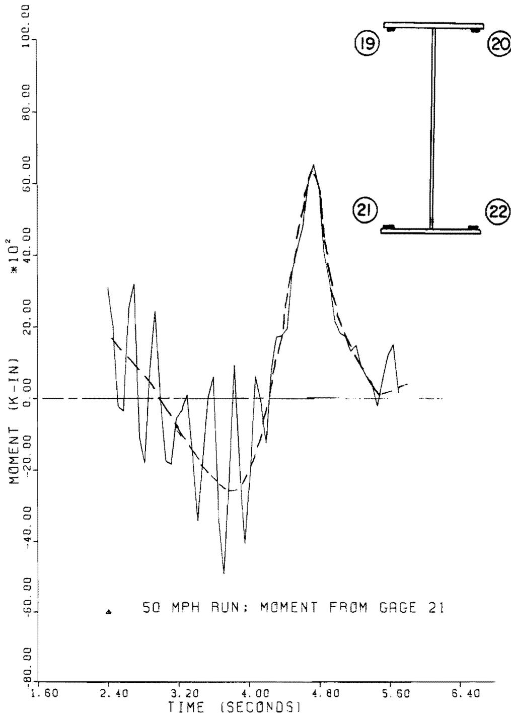
Fig. E.16 50 mph run: moment from gage 21
