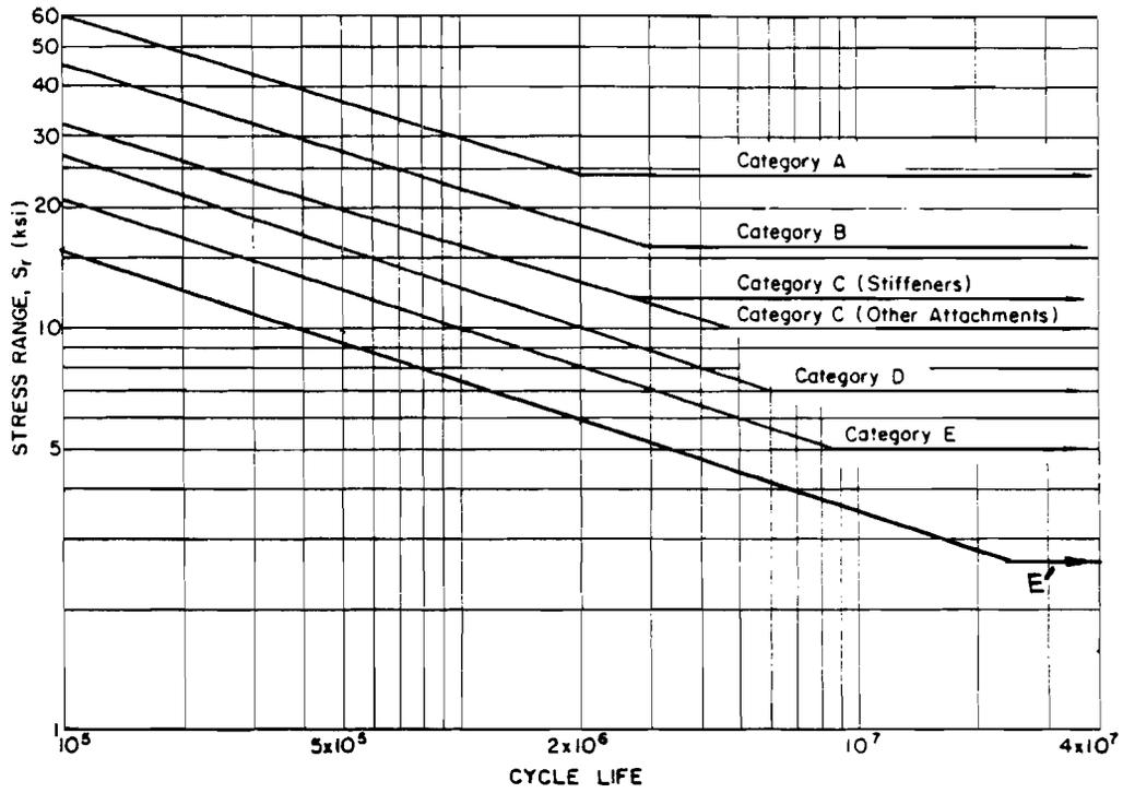
Fig. 1.2 Design stress range curves for Categories A to E' (from Ref 2)
