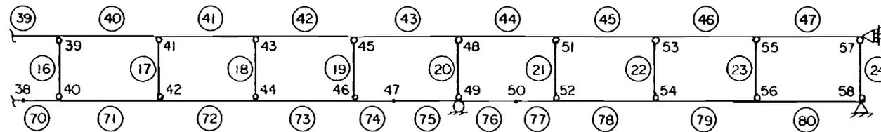
Fig. 4.1 Frame model of the bridge
