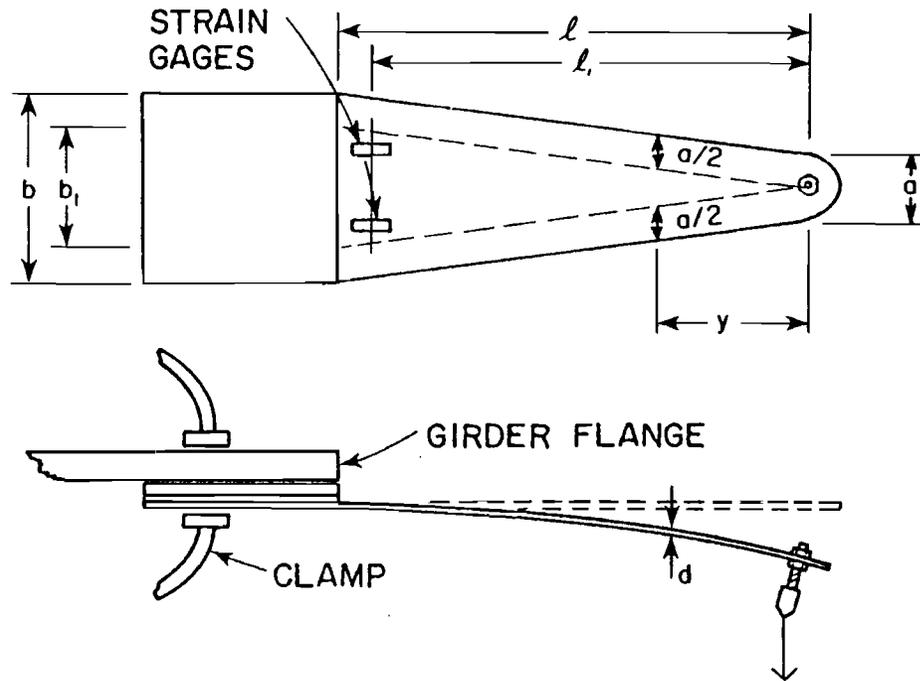
Fig. A1 Cantilever-type deflection gage
