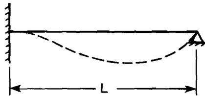
Fig. C1 Propped Cantilever
