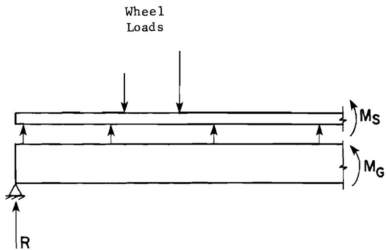
Fig. 4.3 Reactions due to the truck load
