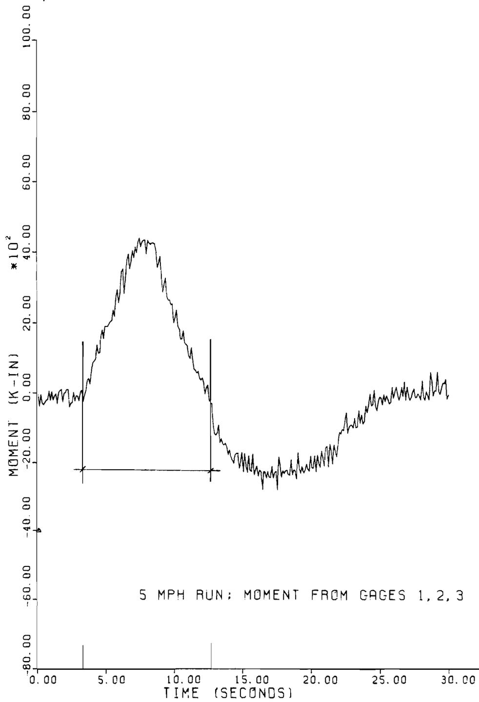
Fig. C.3 Time period of fluctuation = 0.31 secs
