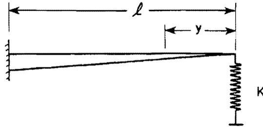
Fig. A2 Analytical model of deflection gage
