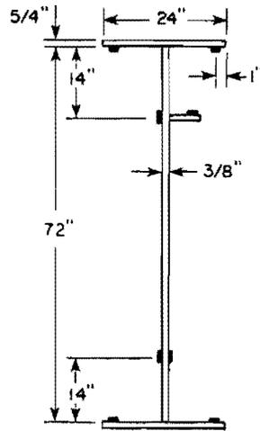
Fig. 2.5 Gaged sections on F18S
