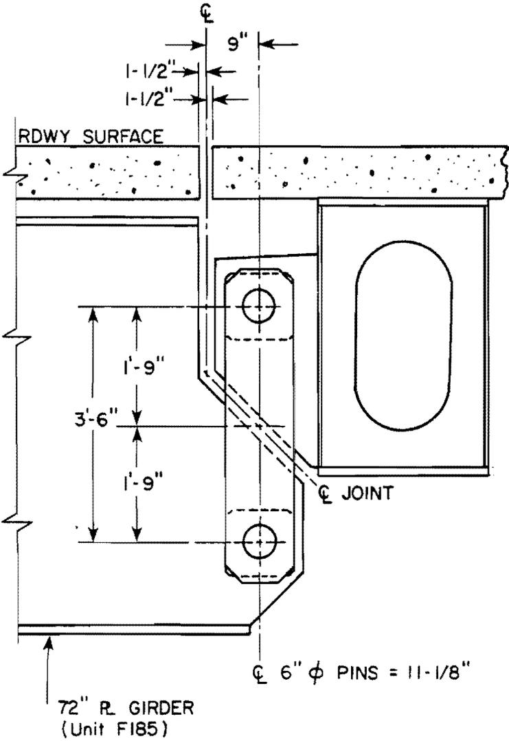
Fig. 2.4b Hanger support detail
