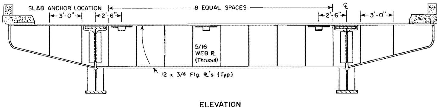
Fig. 1.3b Typical elevation of a crossbeam with connected deck
