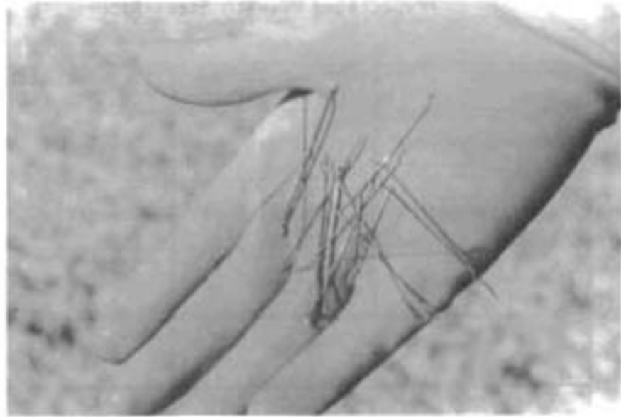
Fig. 7.37 Steel Fiber Using User-Formulated Prepackaged PC with Steel Fiber
