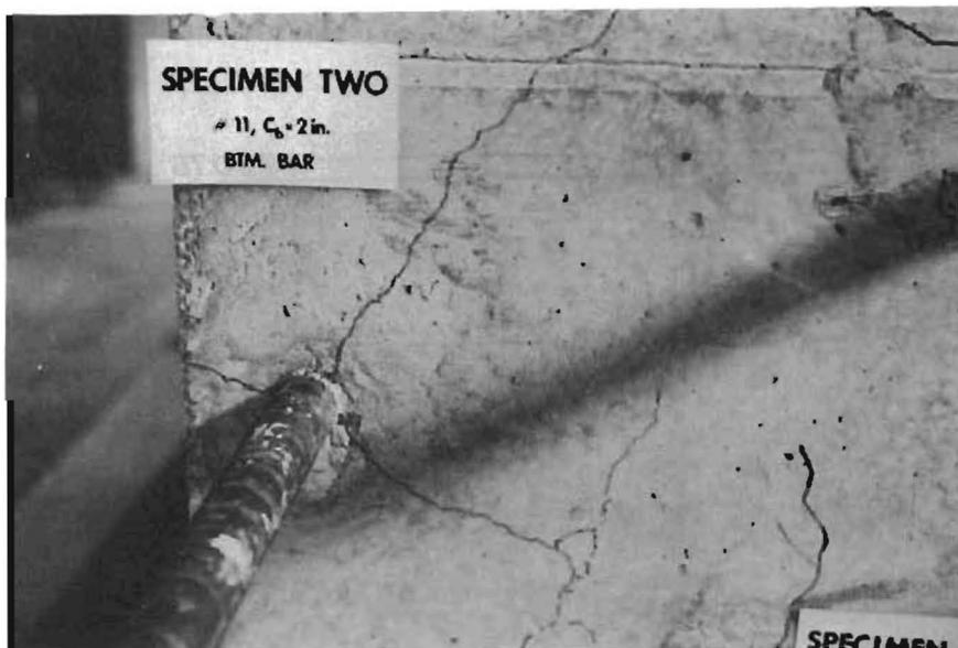
Fig. A.13 Typical crack pattern of the middle top and bottom bars of trial Specimen T2
