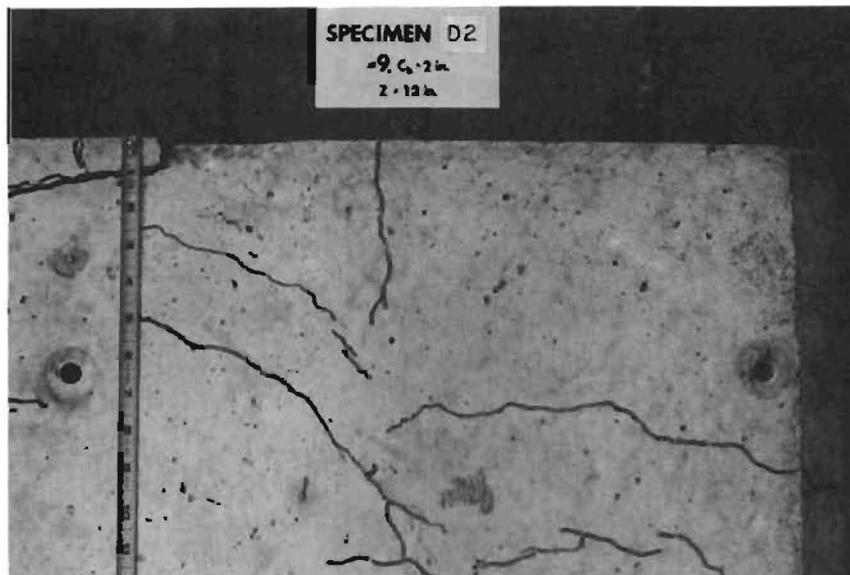
Fig. 5.5 Corner-splitting mode of failure of the #9 bar at  $z = 12$  in. in test Specimen D2
