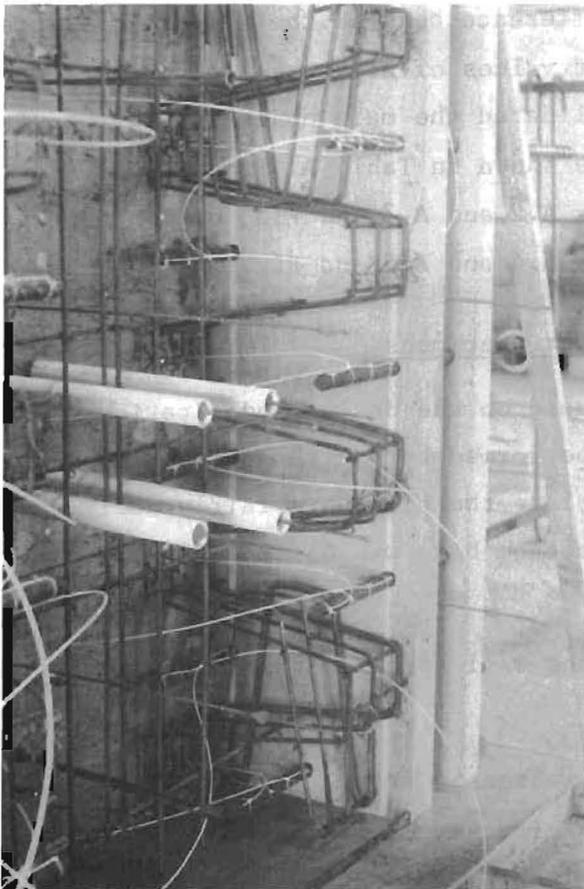
Fig. A.11 Additional #3 reinforcement on one side of Specimen T3
