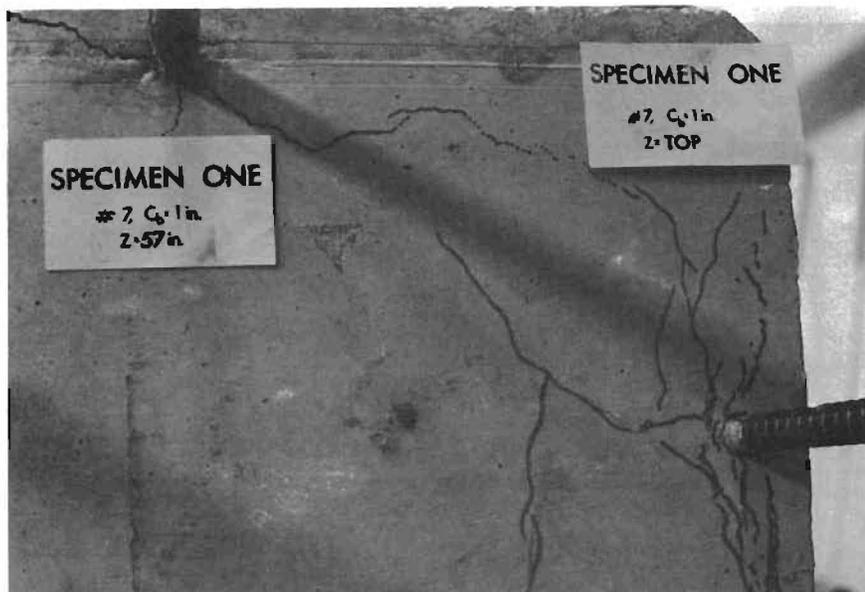
Fig. A.8 Cracks from bar at  $z = 57$  in. spreading into the test zone of the middle top bar, Specimen T1
