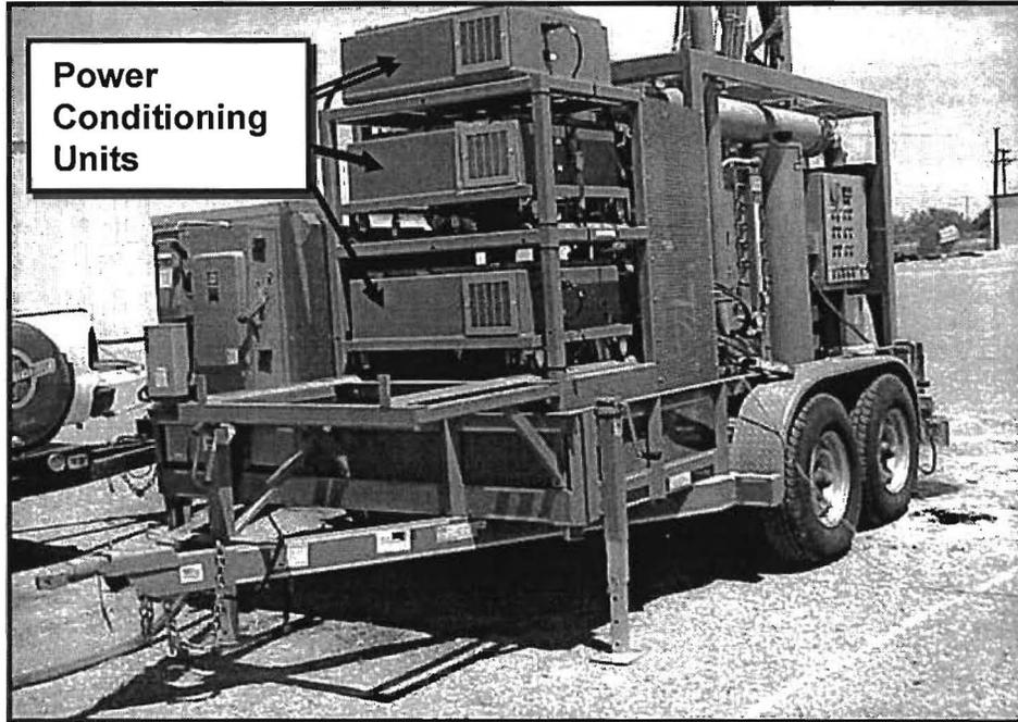
**Figure 3. Power Conditioning Unit**
