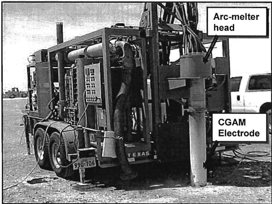
**Figure 1. Mobile, Trailer-Mounted SOVIT System**
