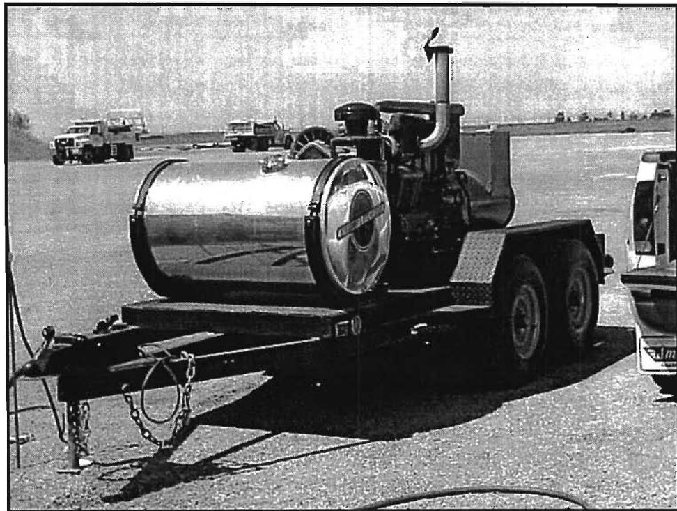
**Figure 2. Electric Power Generator Used with SOVIT**
