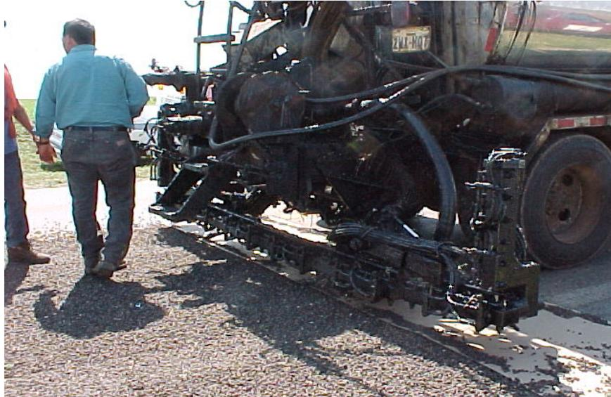
**Figure 3.** Distributor Spray Bar
