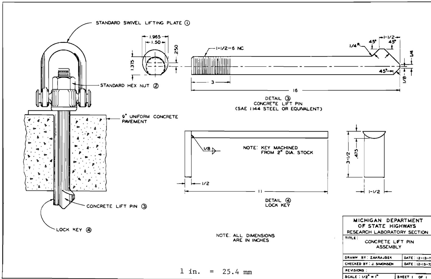
Fig 3.9. Concrete lift pin assembly (Ref 2).
