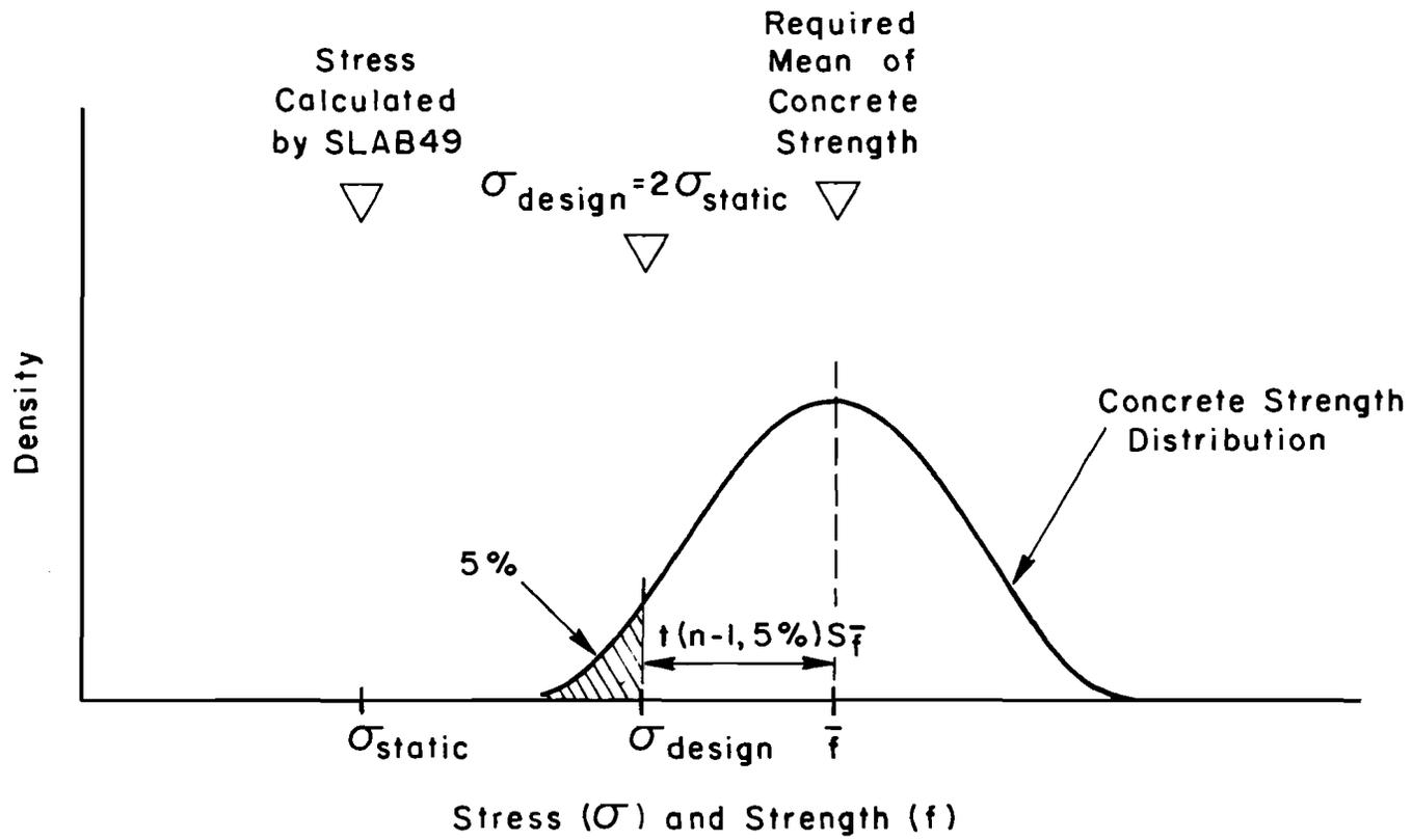
Fig A3.17. Selection of required concrete strength for lifting concrete slabs.
