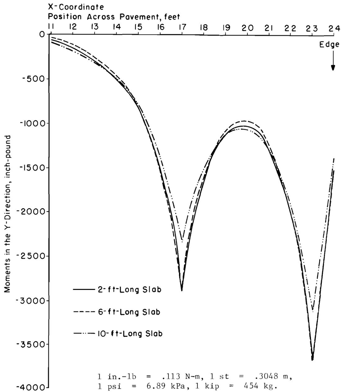
Fig A2.21. Moments in the Y-direction due to 9-kip loads at 17 and 23 ft. Modulus of elasticity at splice locations equals  $10.0 \times 10^6$  psi. Varying slab length.
