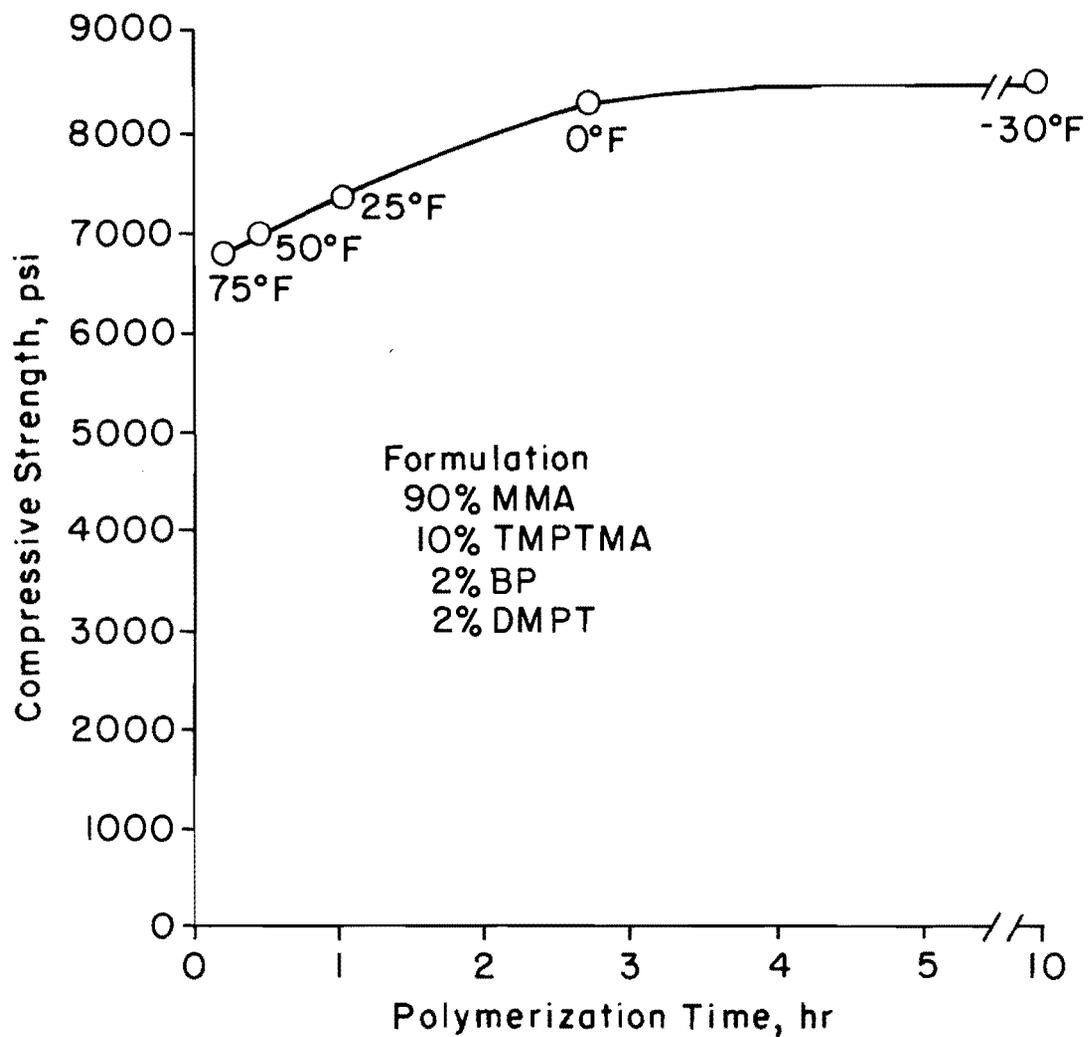
Fig 3.7. Effect of polymerization time on compressive strength of polymer concrete (Ref 29).
