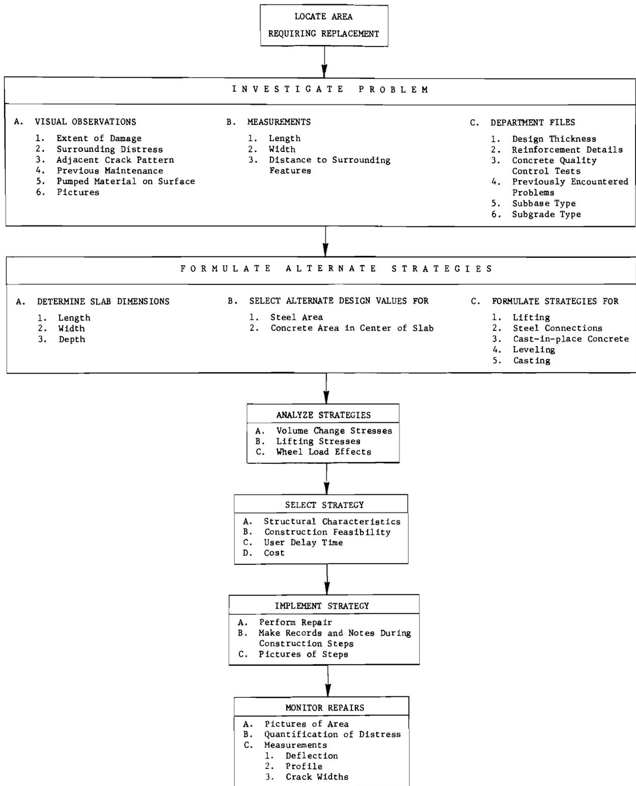
Fig 5.1. Flowchart of precast slab repair design process.
