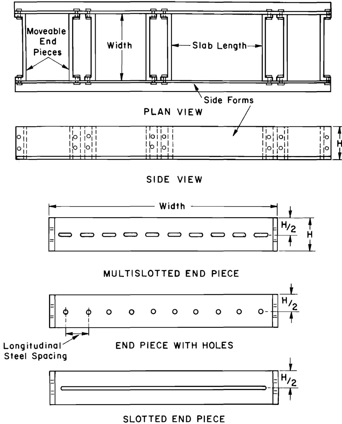
Fig 3.1. Multi-casting slab forms with alternate types of end pieces.
