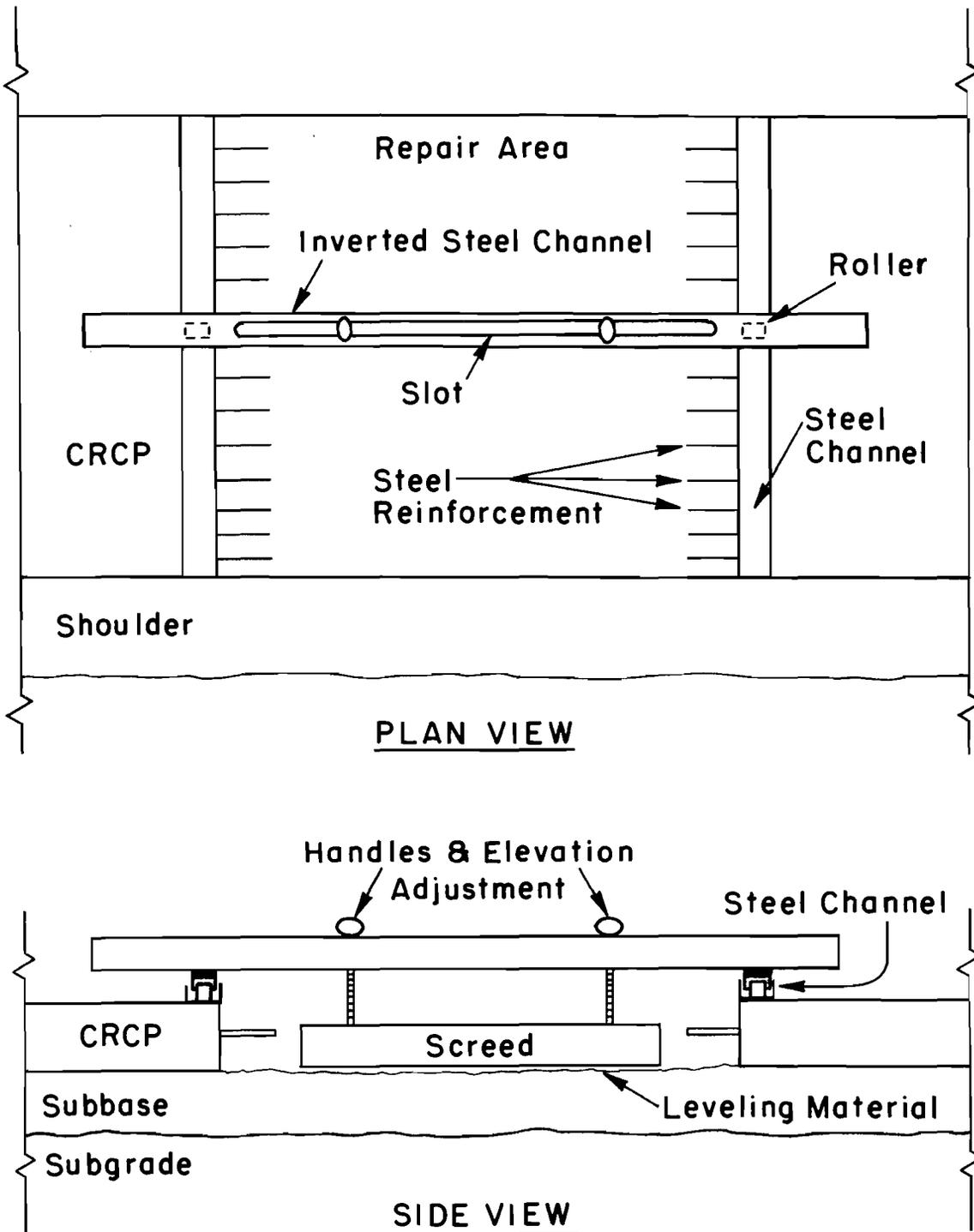
Fig 3.11. Conceptual diagram of tracked screed for striking leveling material.
