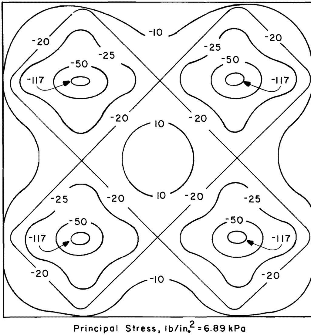
Fig A3.10. Stresses in a 12 X 12-foot (3.66 X 3.66-m) slab with lift points at 1/4 span.
