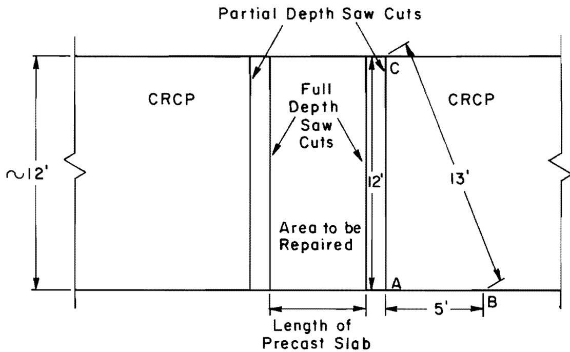
Fig 3.8. Right triangle techniques for laying out saw cuts.
