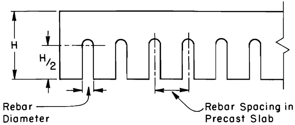
Slots in Bond Breaker to Fit Over Reinforcement
