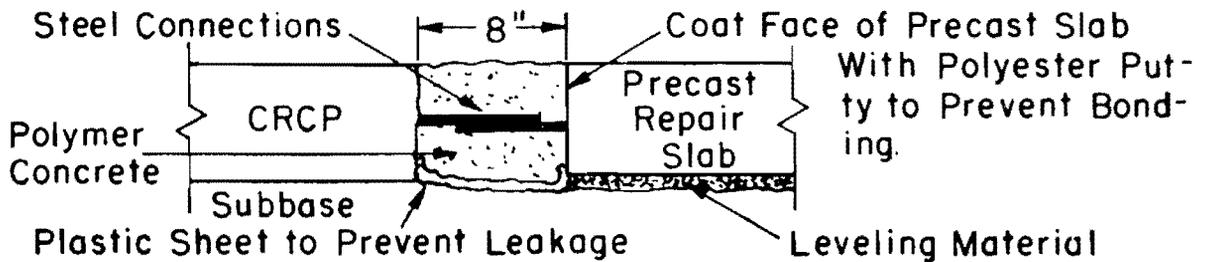
Side View of Anchorage Zone With Polymer Concrete Filler
