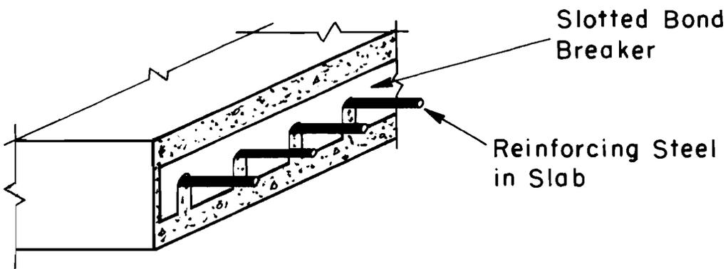
Oblique Section Showing Orientation of Bond Breaker
