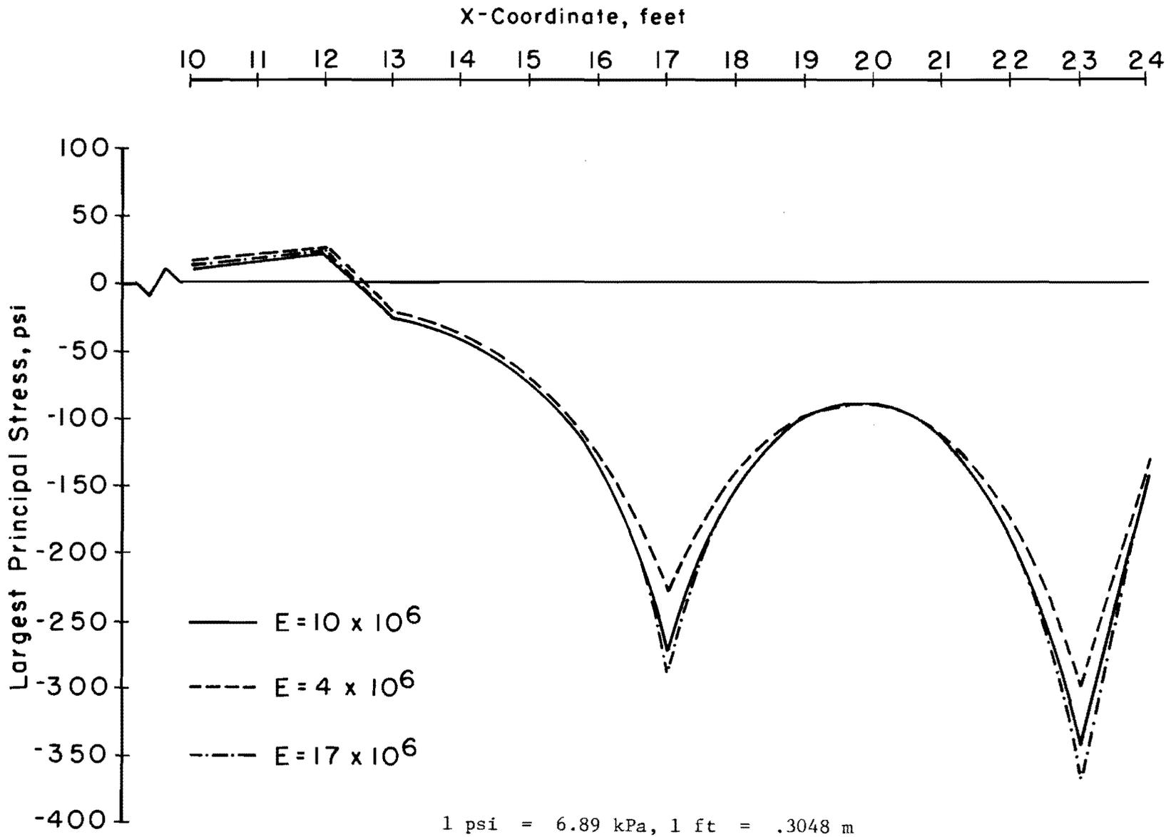
Fig A2.11. Distribution of principal stress across slab with varying splice modulus.
