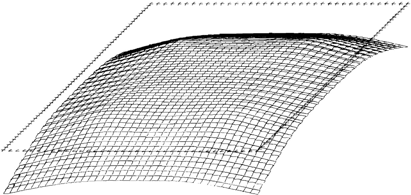
Fig A3.16. Distorted 3-D deflection profile for 12 X 14-foot (3.66 X 4.27-m) slab with lift points at 1/4 span.
