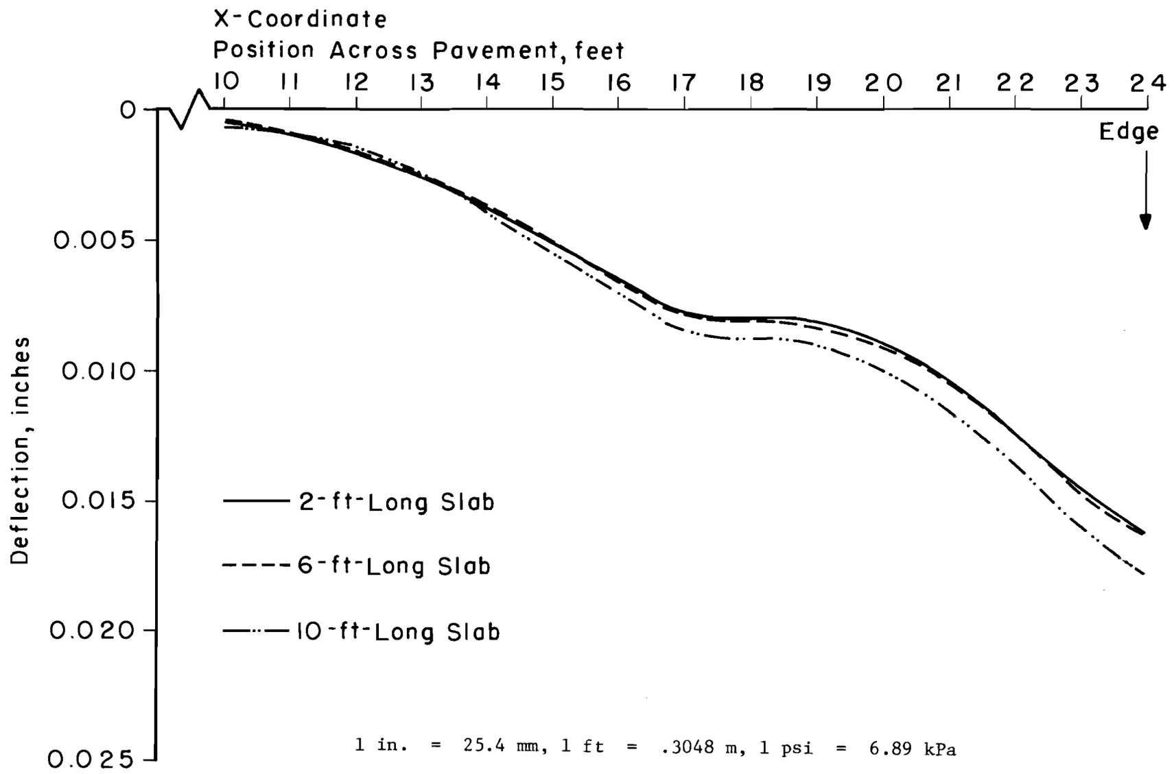
Fig A2.24. Deflection due to 9-kip loads at 17 and 23. Modulus of elasticity at splice locations equals  $10.0 \times 10^6$  PSI varying slab length.
