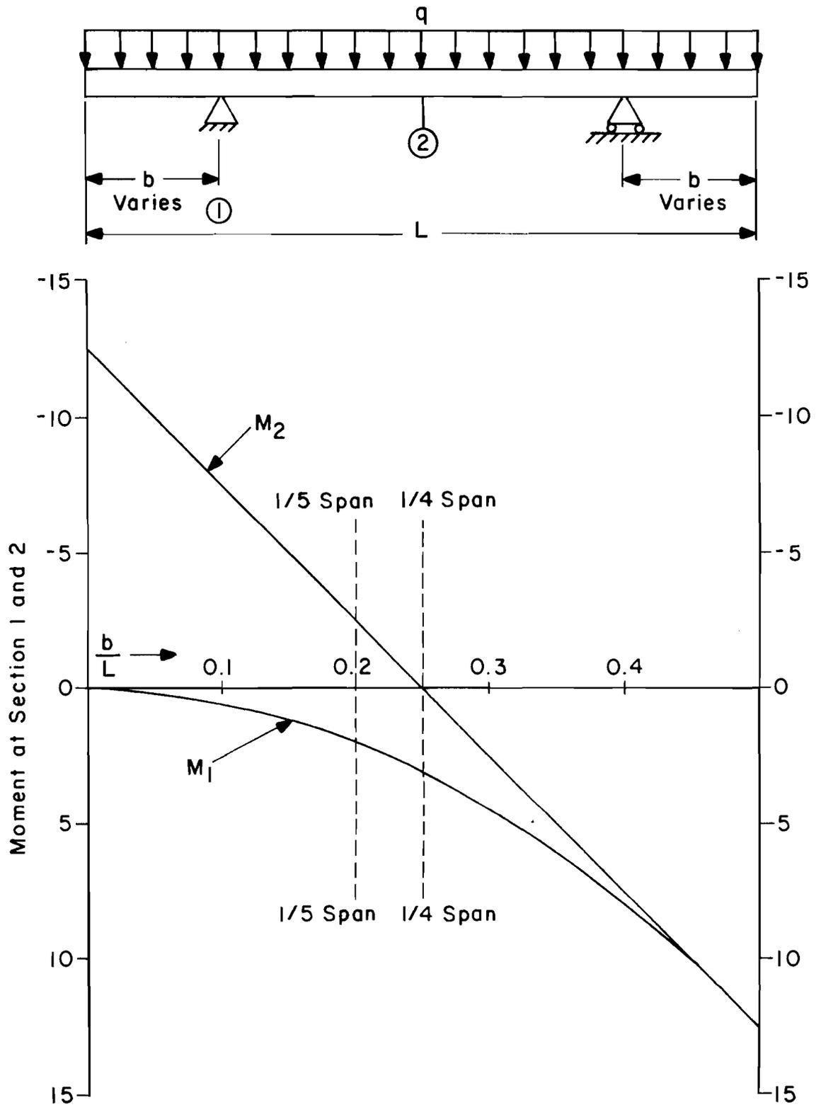
Fig A3.2. Moment analysis of simply supported beam with uniformly distributed load.
