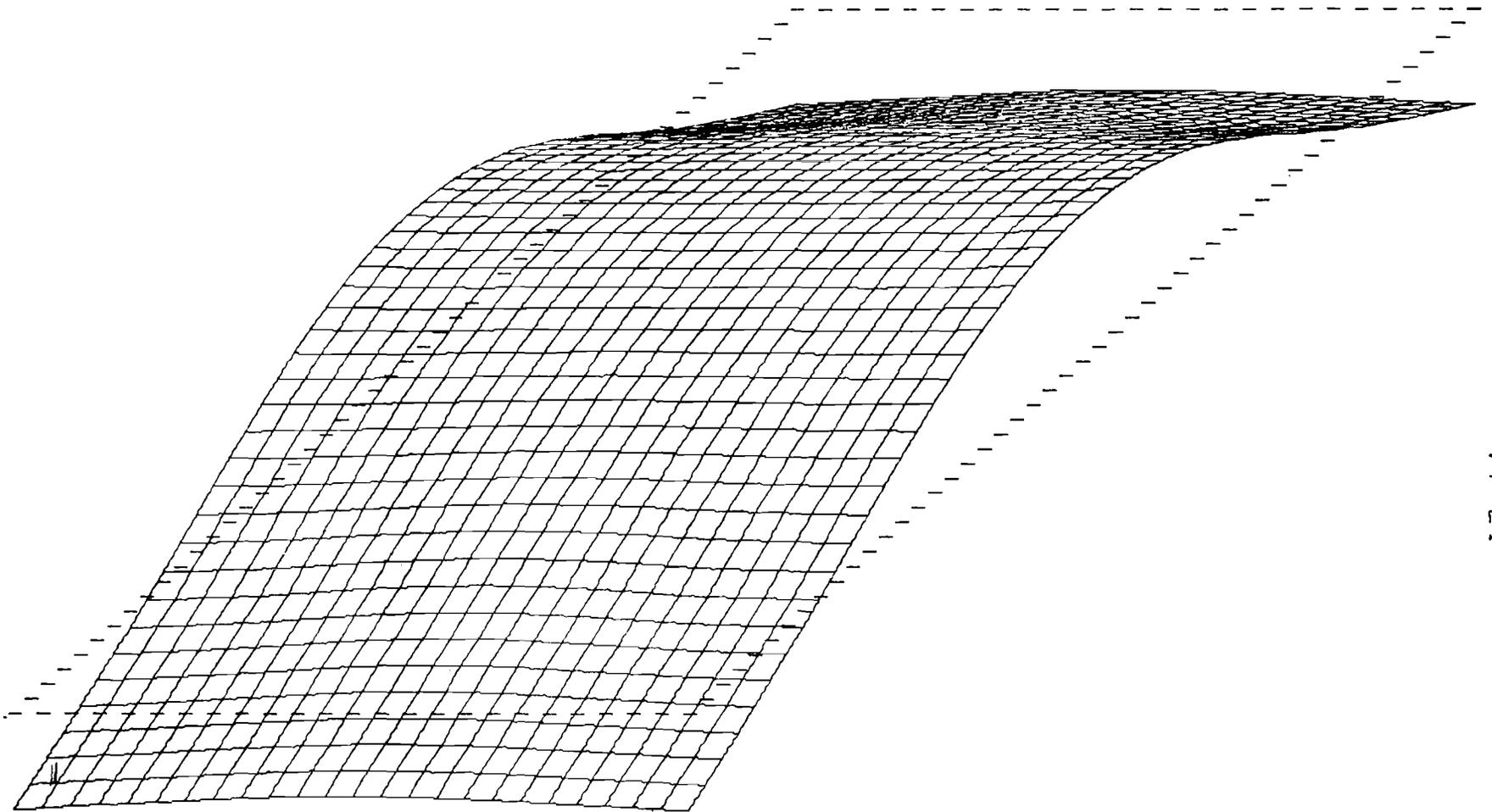
Fig A3.6. Distorted 3-D deflection profile for 6 x 12-foot (1.83 x3.66 m) concrete slab with lifting points at 1/6 span.
