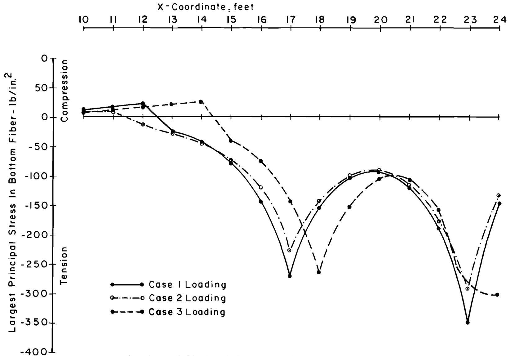
Fig A2.6. Largest principal stress in bottom fiber-critical position of load.
