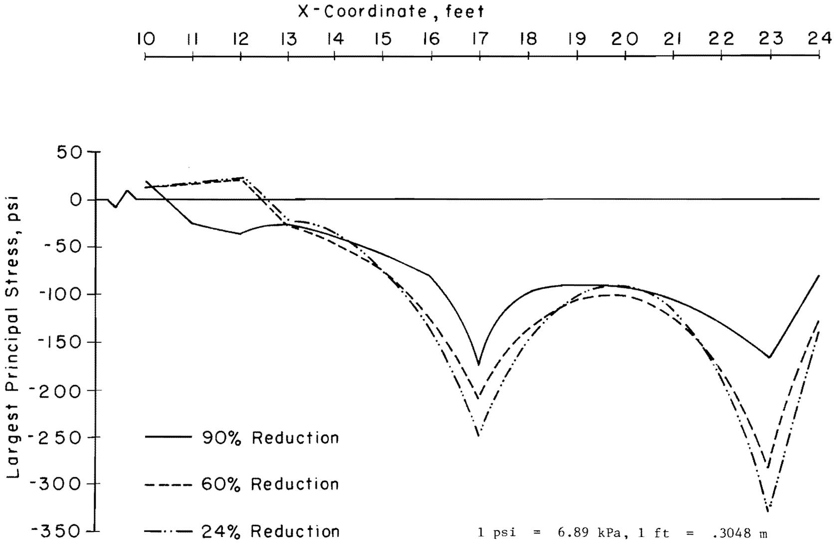
Fig A2.17. Distribution of principal stress across slab with reduced splice bending stiffness  $E_{SPL} = 10 \times 10^6$  psi.
