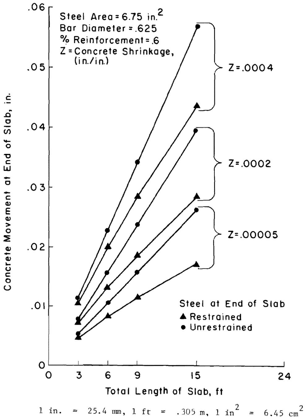
Fig A5.4. Comparison of concrete movement at end of slab for restrained and unrestrained slabs.
