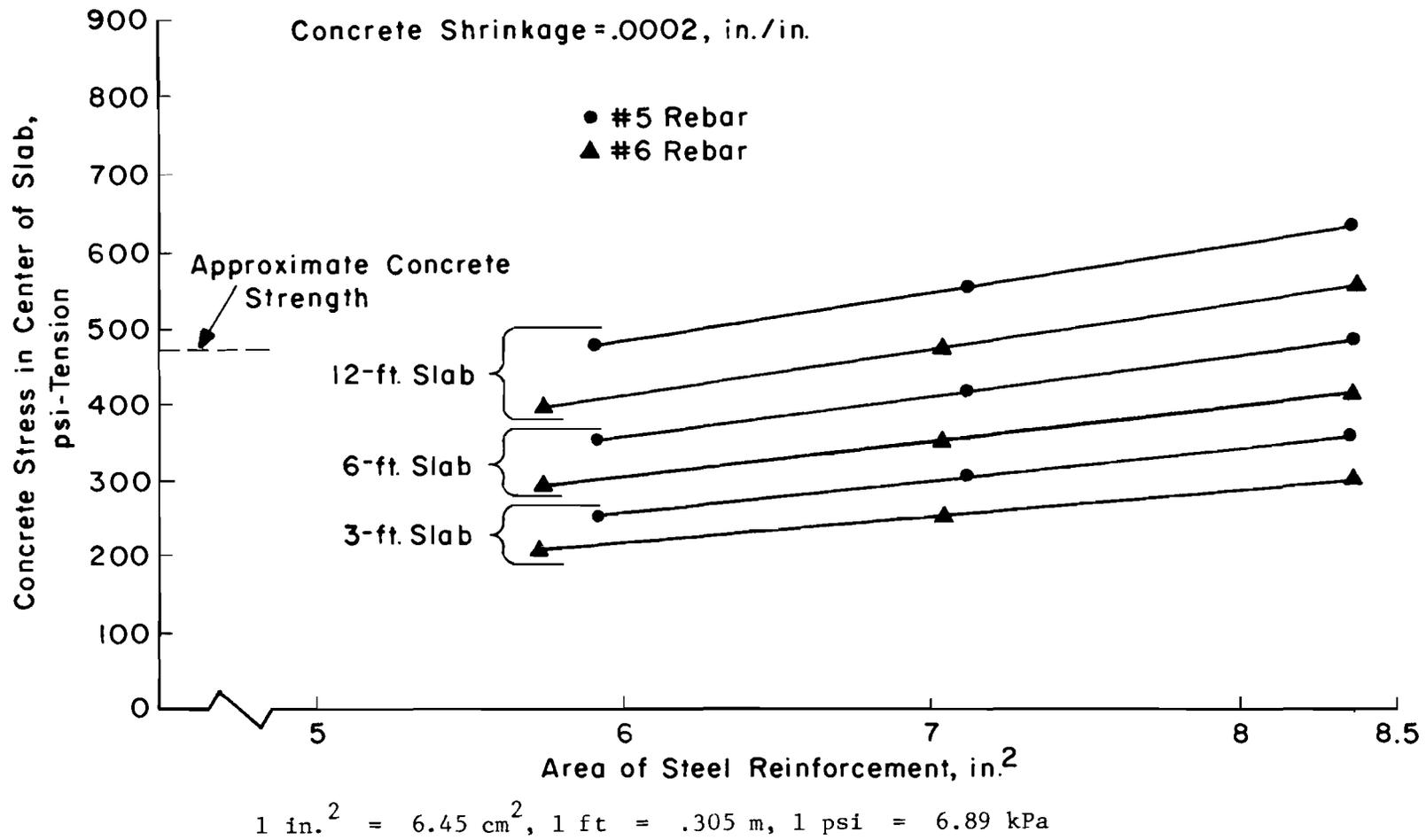
Fig A5.11. Concrete stress versus area of steel reinforcement, general analysis.
