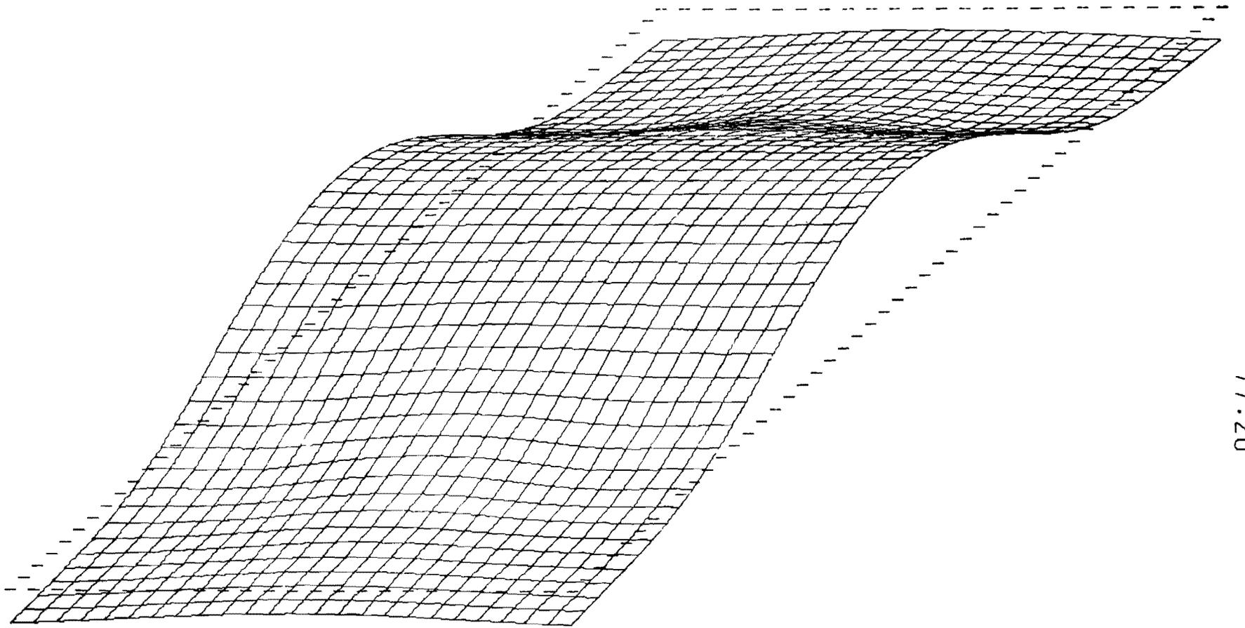
Fig A3.7. Distorted 3-D deflection profile for 6 x 12-loot (1.83 x 3.66 m) concrete slab with lifting points at 1/5 span.
