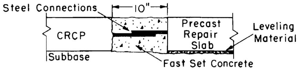
Side View of Anchorage Zone With Fast Set Concrete Filler
