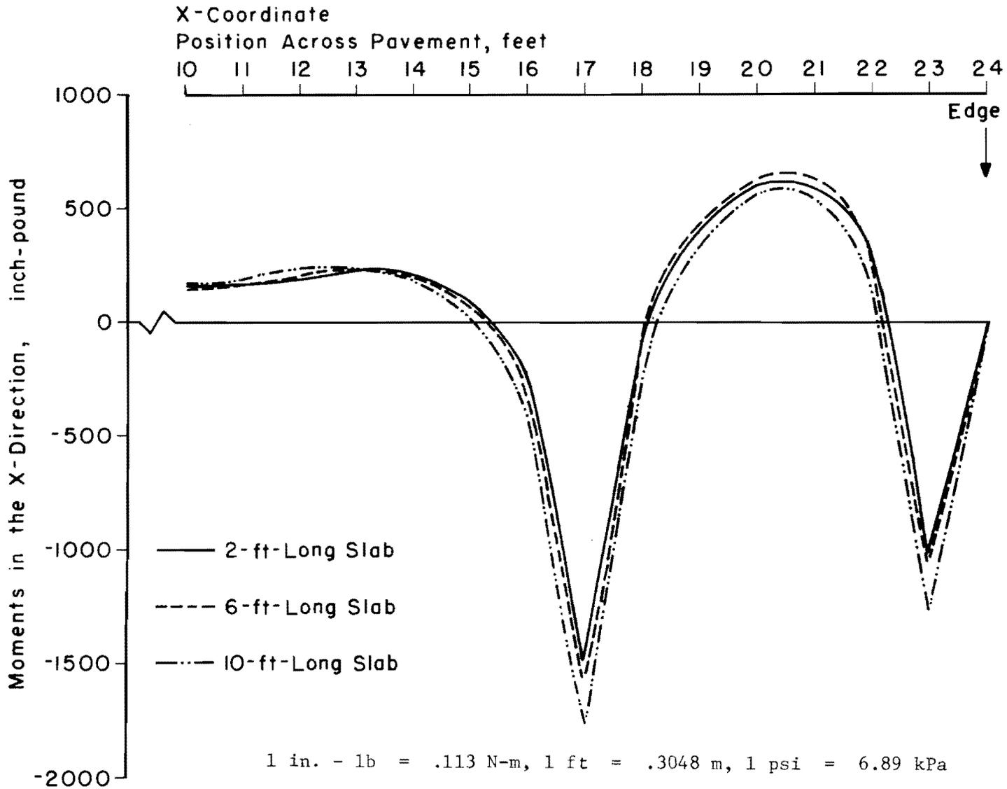
Fig A2.22. Moments in the X-direction due to 9-kip loads at 17 and 23. Modulus of elasticity at splice locations equal to  $10.0 \times 10^6$  psi, varying slab lengths.
