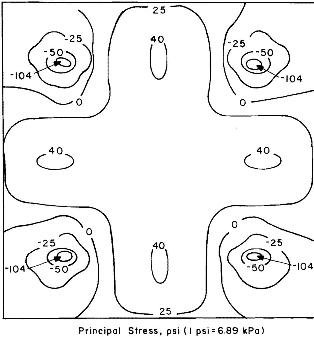
Fig A3.9. Stresses in a 12 X 12-foot (3.66 X 3.66-m) slab with lift points at 1/5 span.
