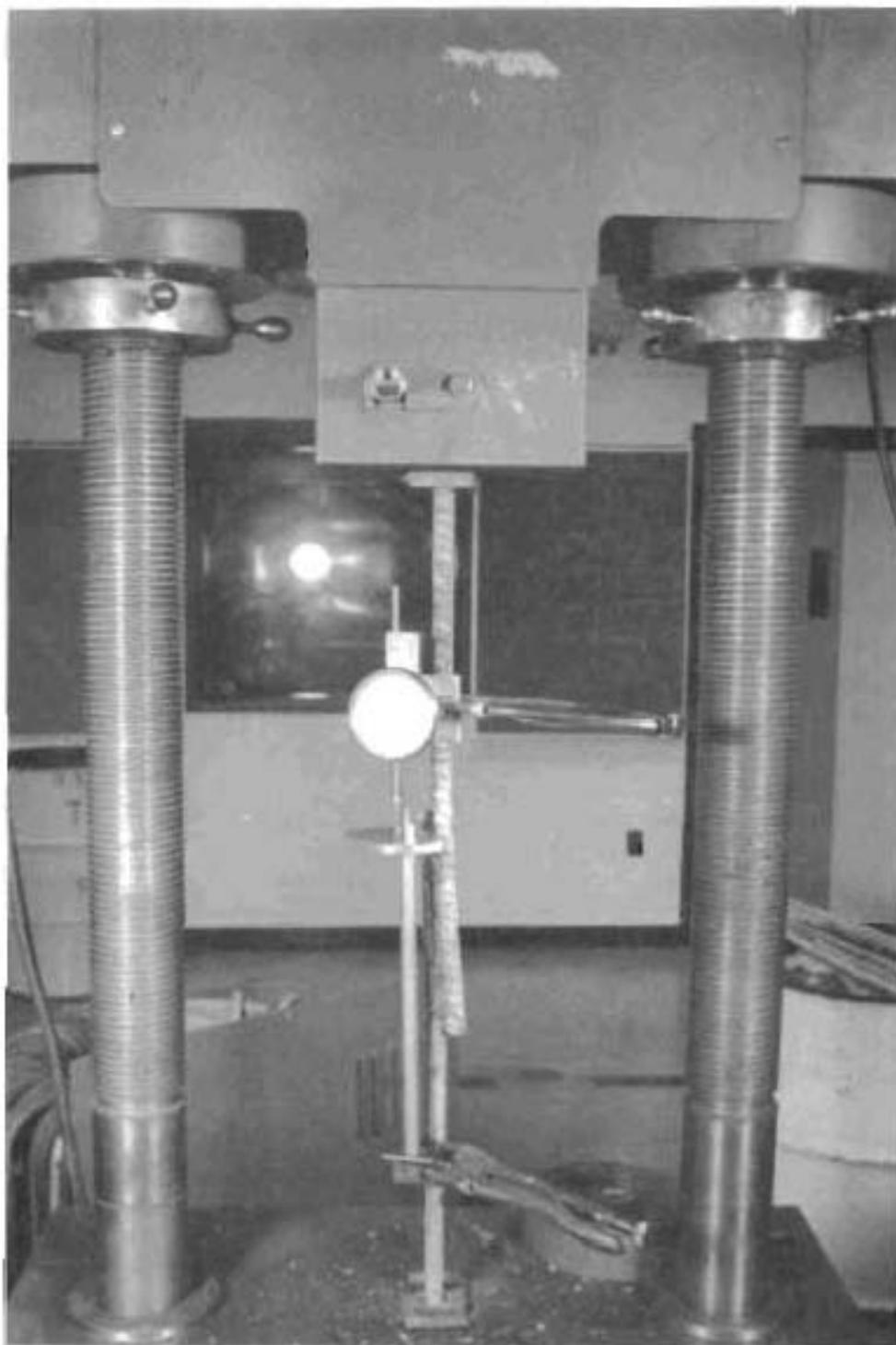
Fig A6.1. Welded reinforcing bar in test machine.
