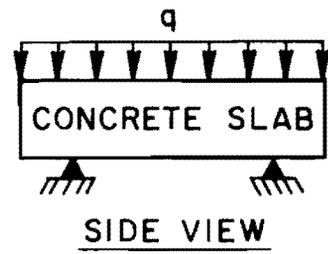
Fig 4.4. SLAB49 Lifting model for precast slabs.
