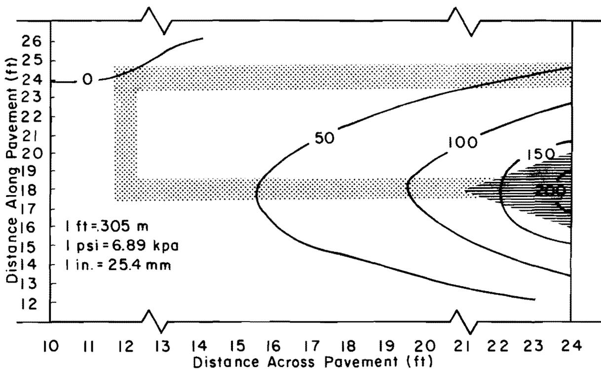
Fig A4.3. Principal stress and deflection contours for case 1.
