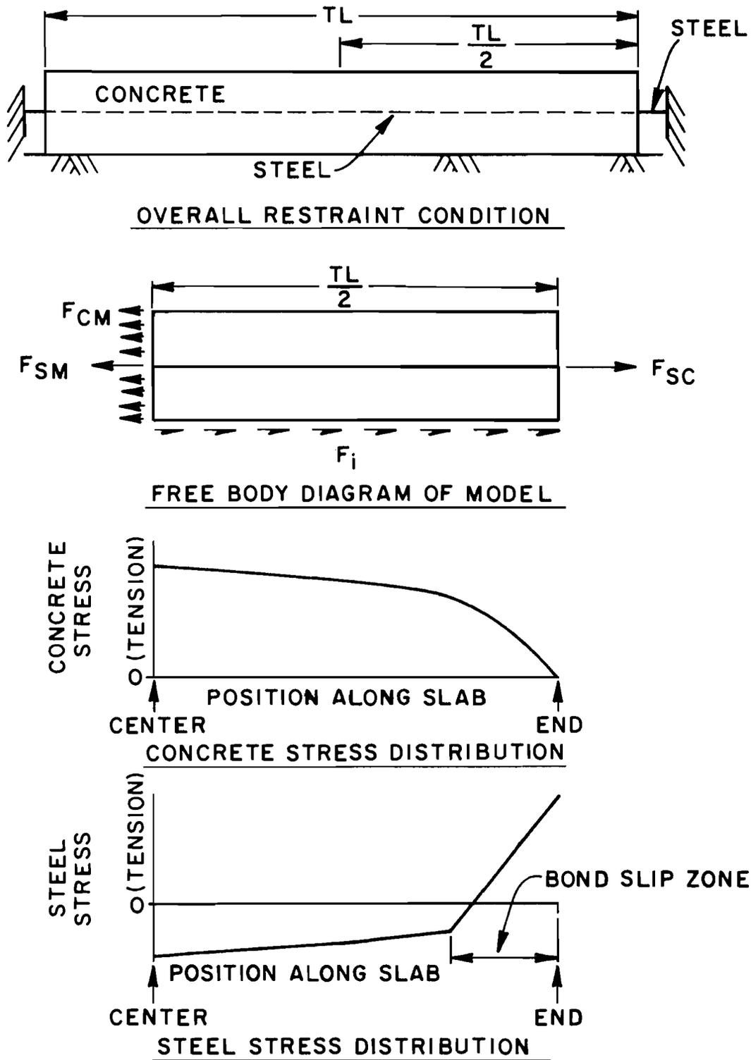
Fig 4.3. VCARCS equilibrium model and stress distribution in restrained concrete slab.
