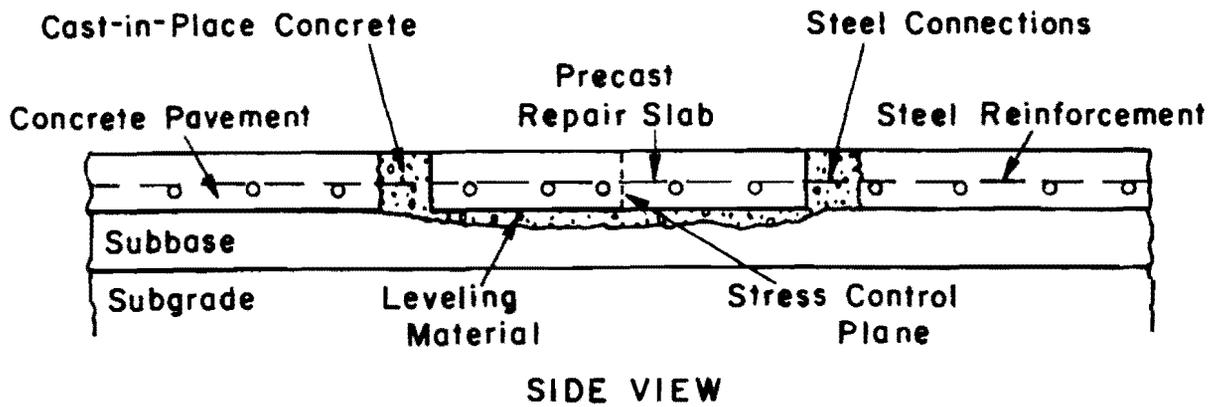
Fig 1.4. Precast repair methodology applied to CRCP.
