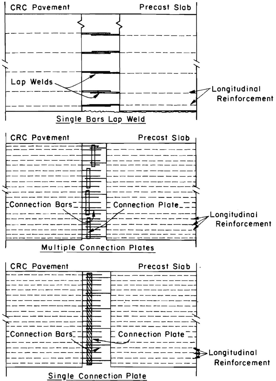
Fig 3.3. Welded steel connection alternatives.
