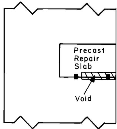
CASE 2. Rectangular Void at Steel Connections
