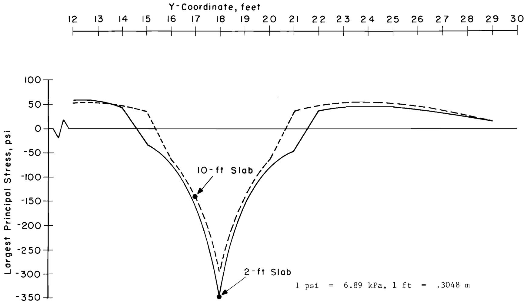
Fig A2.25. Largest principal stress versus Y-coordinate with two and 10-foot long slabs. X = 23.
