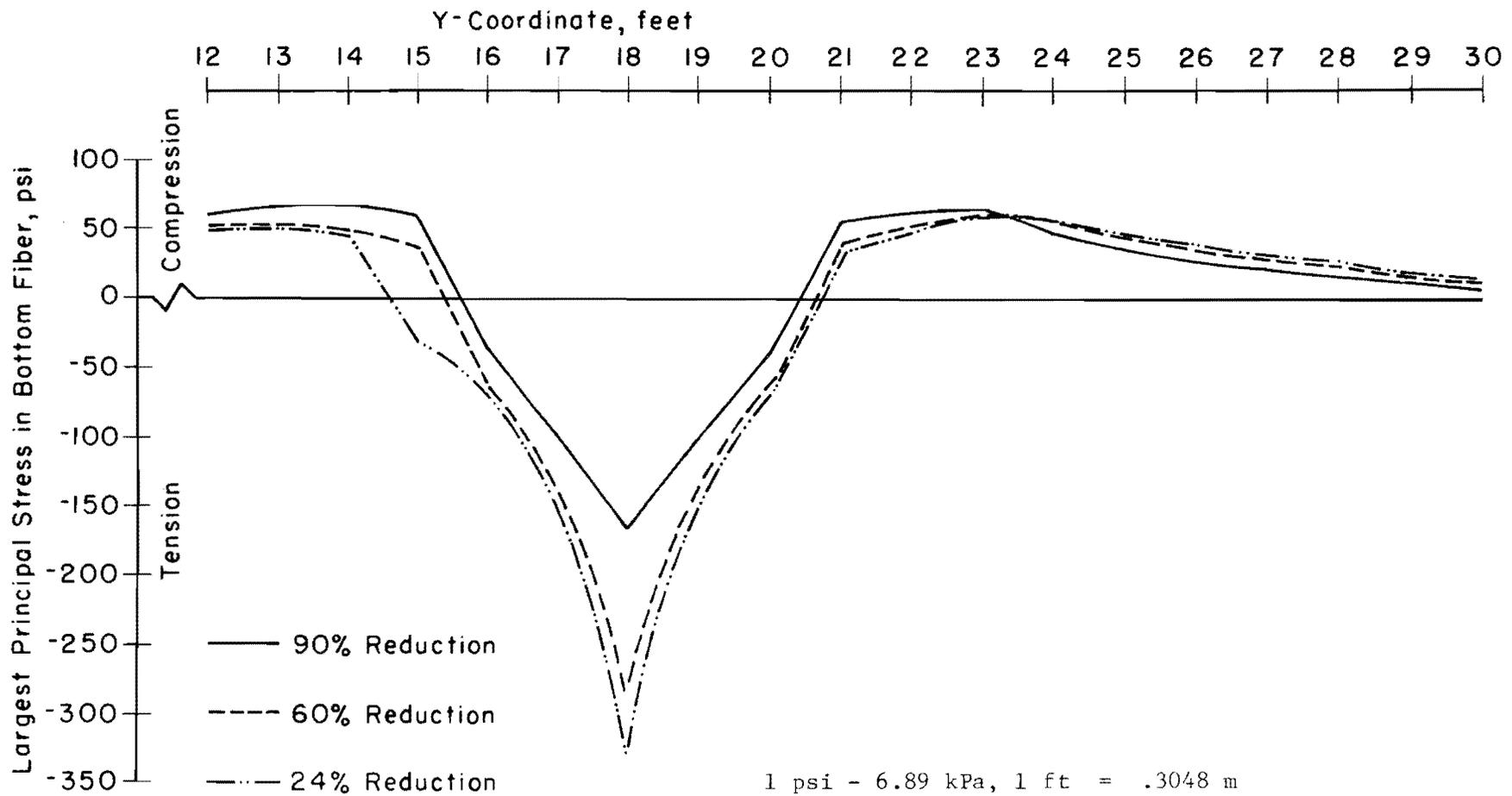
Fig A2.18. Distribution of principal stress along slab with reduced splice bending stiffness.  $E_{SPL} = 10 \times 10^6$  PSI
