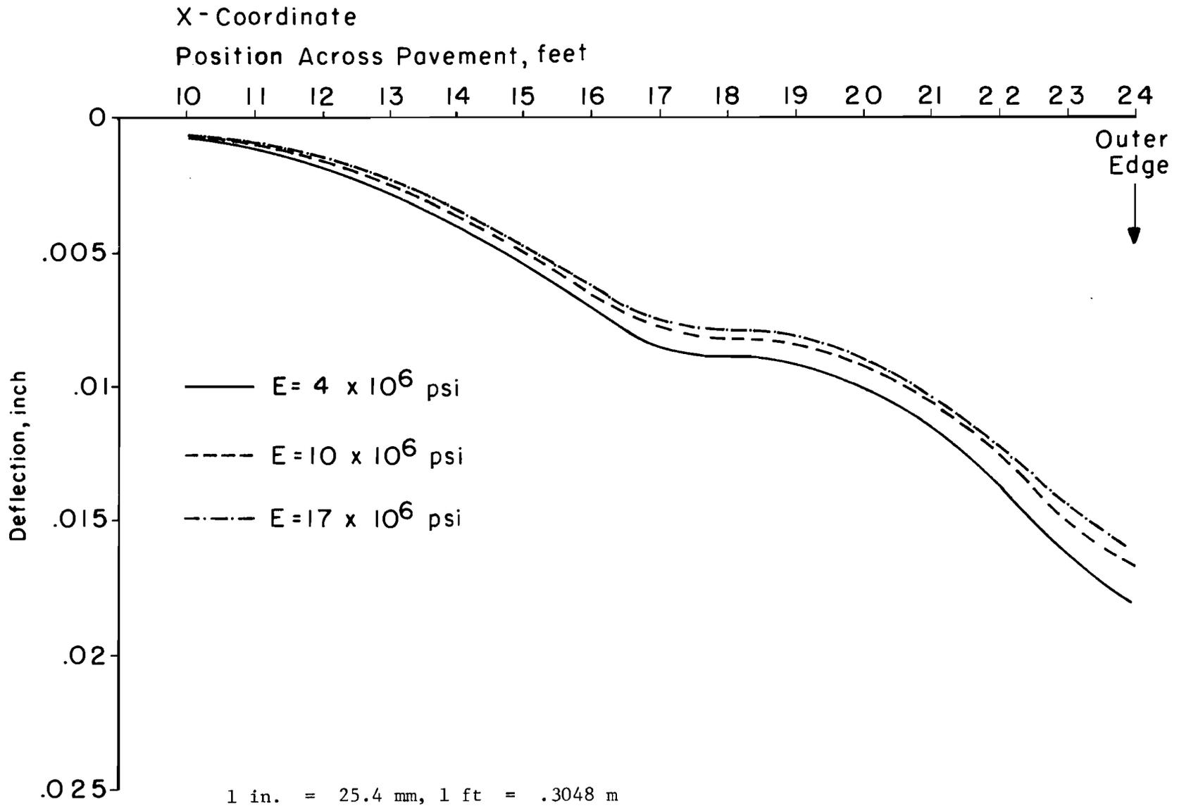
Fig A2.12. Deflection due to 9-kip loads at 17 and 23. Varying modulus of elasticity at splice locations.
