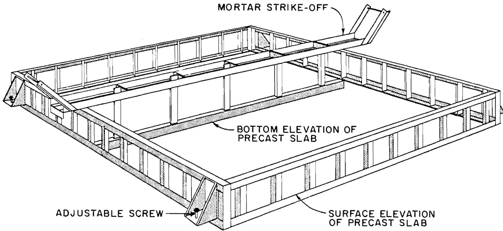
Fig 3.12. Frame for setting precast slab elevation (Ref 2).
