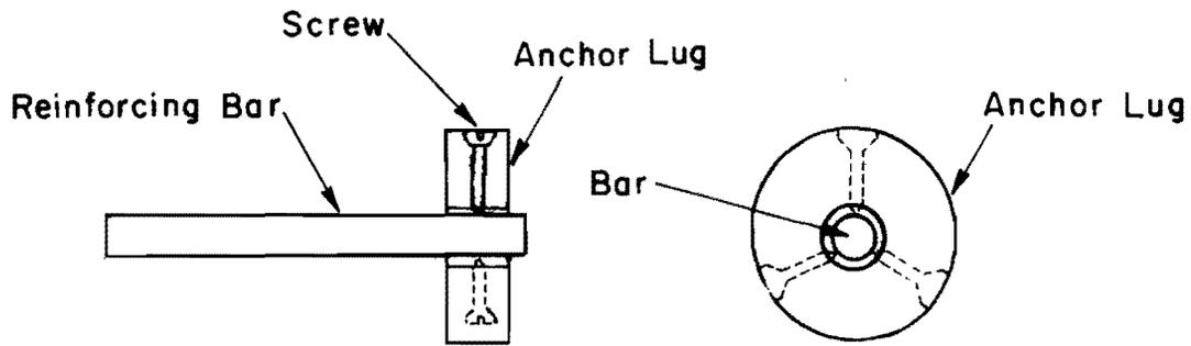
SPHERICAL BEARING SURFACE ATTACHMENT
