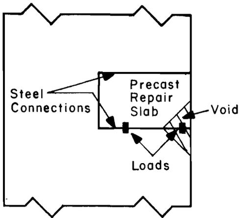
CASE 1. Triangular Void at Steel Connections
