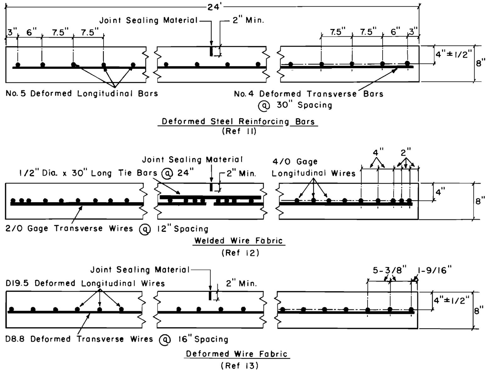
Fig 2.2. Example CRCP cross sections. 1 ft = .305 m, In. = 25.4 mm
