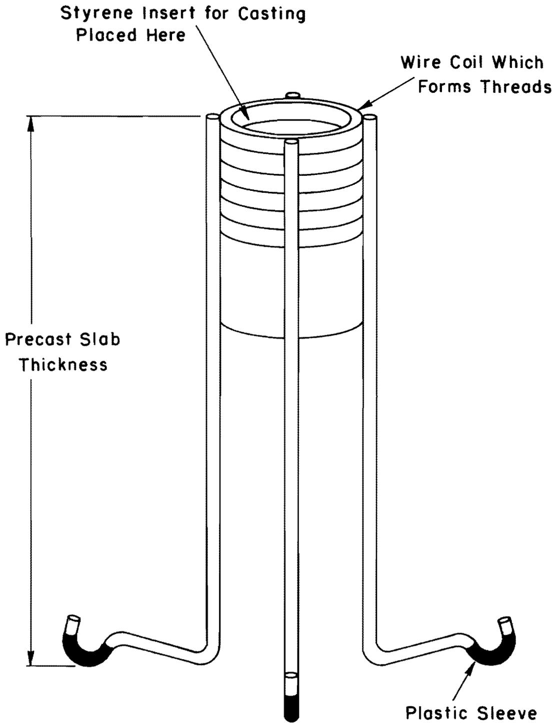
Fig 3.10 Sketch of threaded inserts for lift connections (Ref 2).
