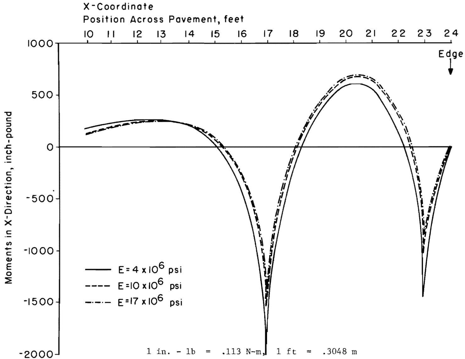
Fig A2.10. Moments in the X-direction due to two 9-kip loads at 17 and 23. Slab with varying modulus of elasticity at splice locations.
