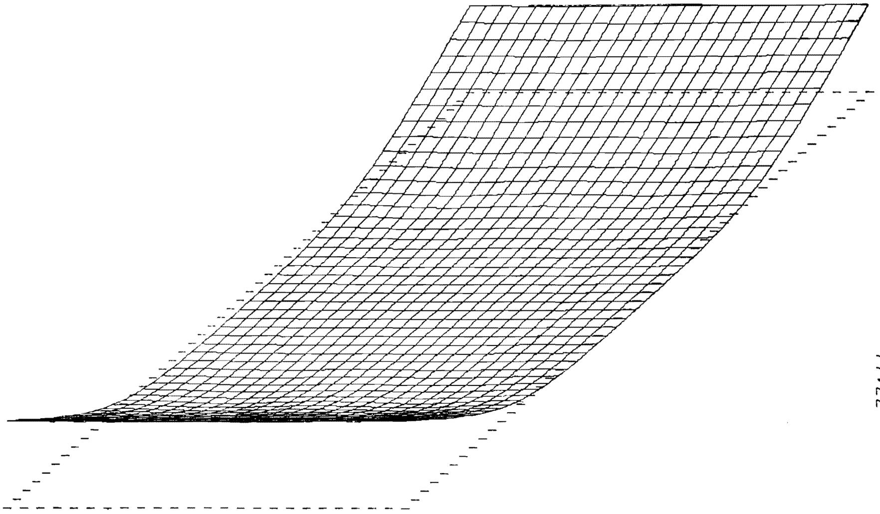
Fig A3.8. Distorted 3-D deflection profile for 6 x 12 foot (1.83 x 3.66 m) concrete slab with lifting points at 1/4 span.
