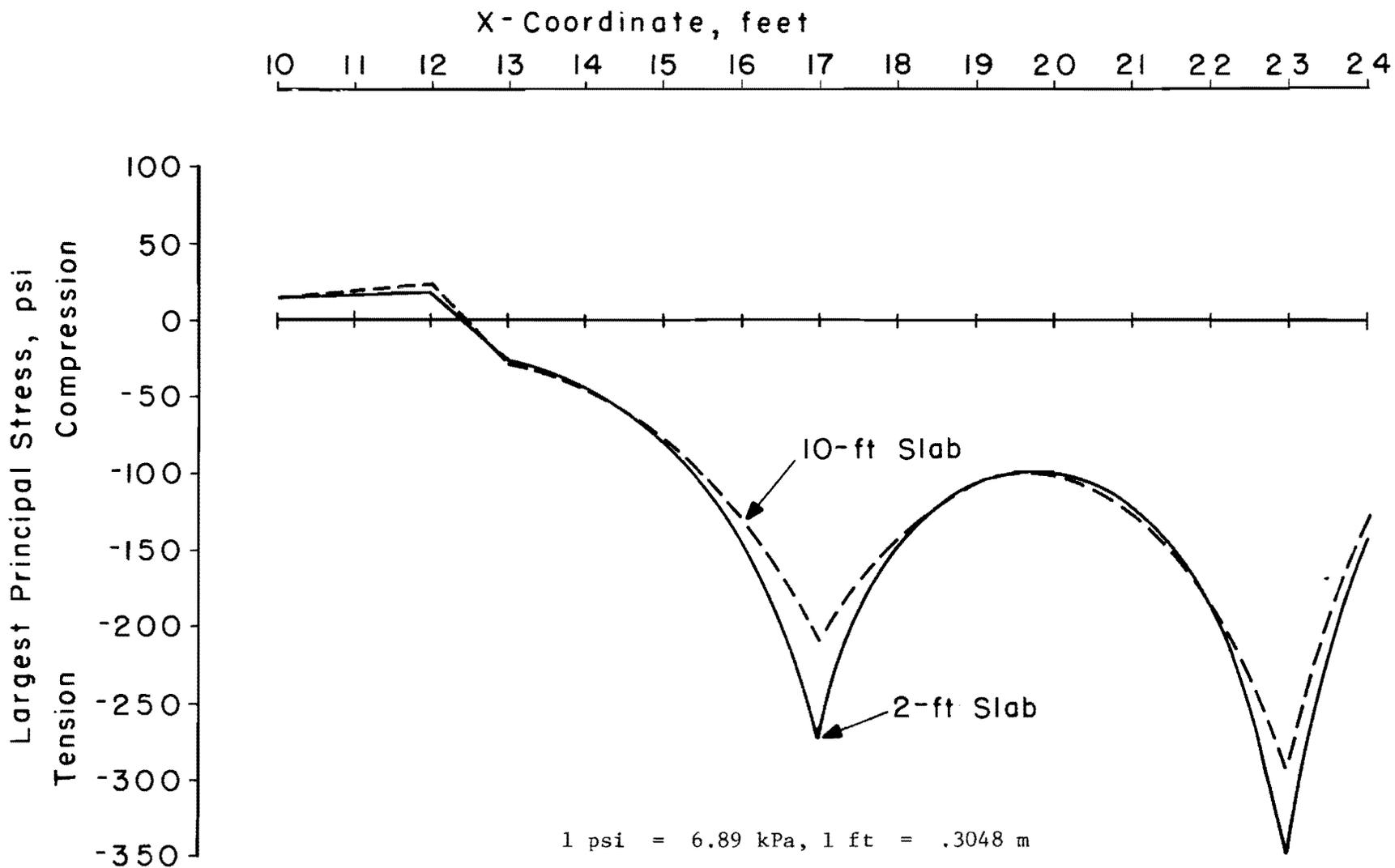
Fig A2.23. Largest principal stress in bottom of slab versus X-coordinate for two and ten-foot long slabs.
