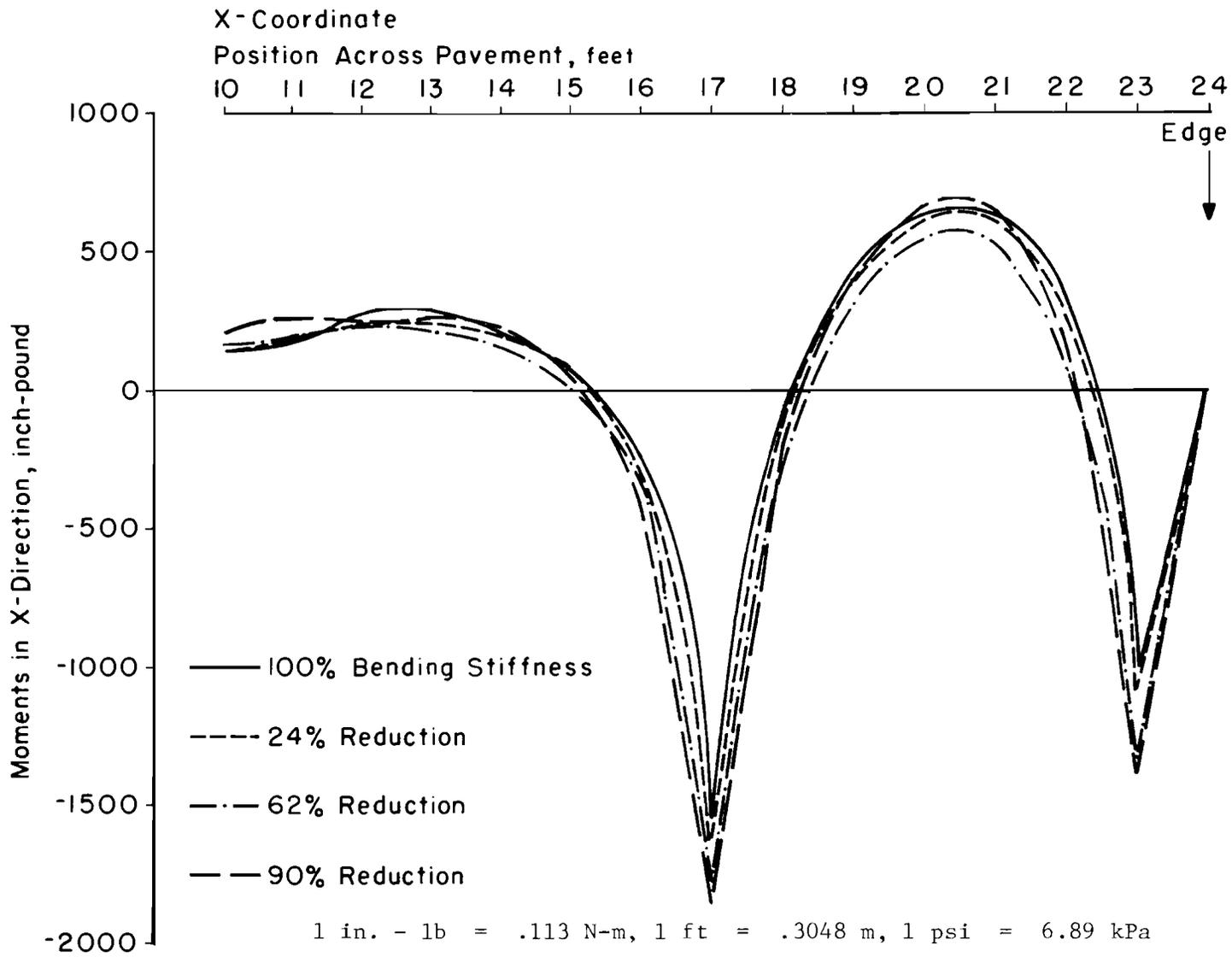
Fig A2.16. Moments in the X-direction due to 9-kip loads at 17 and 23. Modulus of elasticity at splice locations equal to  $10 \times 10^6$  psi, varying bending stiffness.
