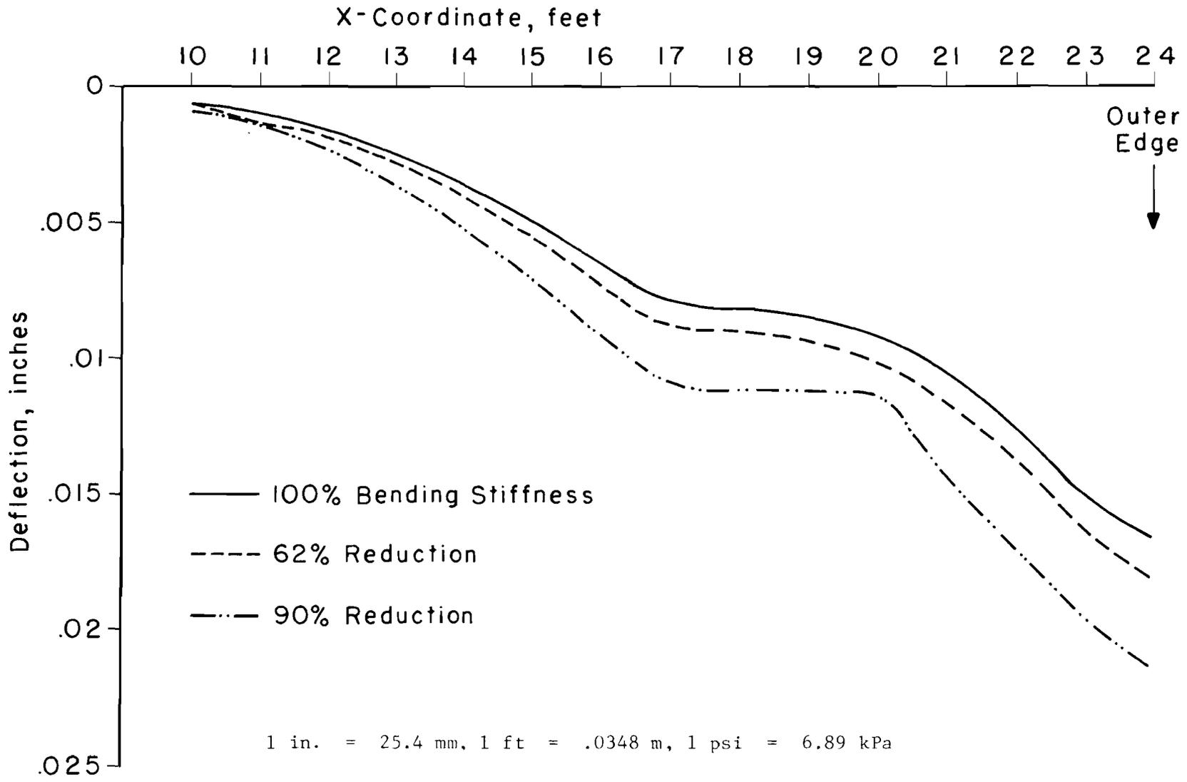
Fig A2.19. Deflection due to 9-kip loads at 17 and 23. Modulus of elasticity at splice locations equal to  $10 \times 10^6$  PSI varying bending stiffness.
