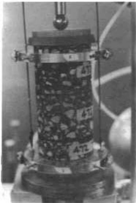
Fig A-11.1. Photographs of dynamic modulus testing equipment.
