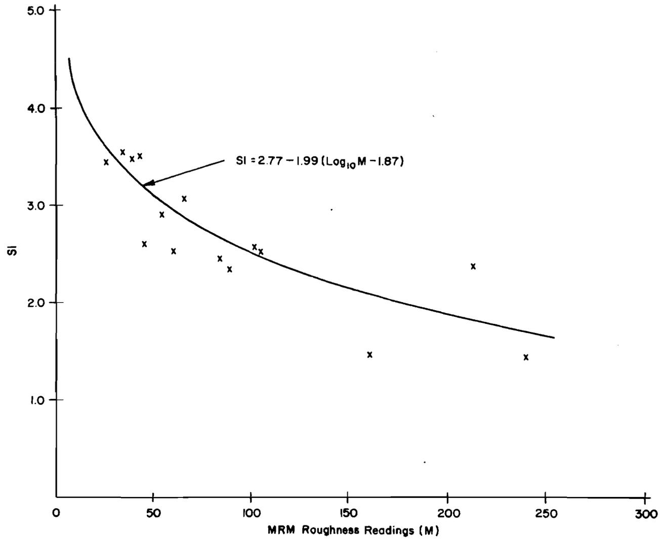
Fig 1.1. Surface Dynamics Profilometer SI versus MRM roughness.
