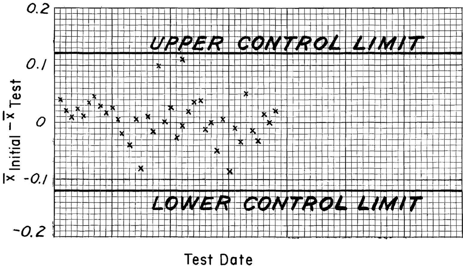
Fig C. Typical MRM control chart for mean.
