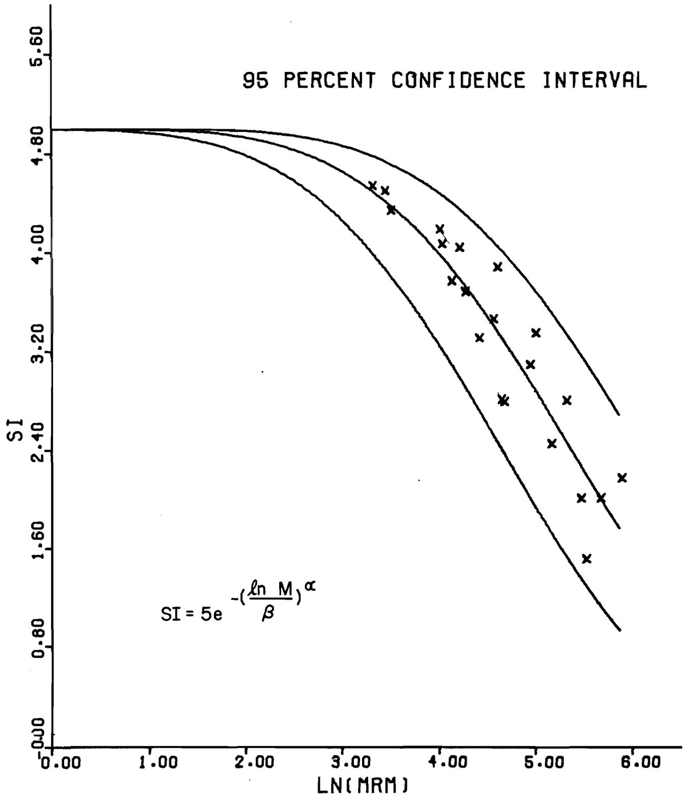
Fig 3.2. SDP-SI values versus log Mays road roughness readings.
