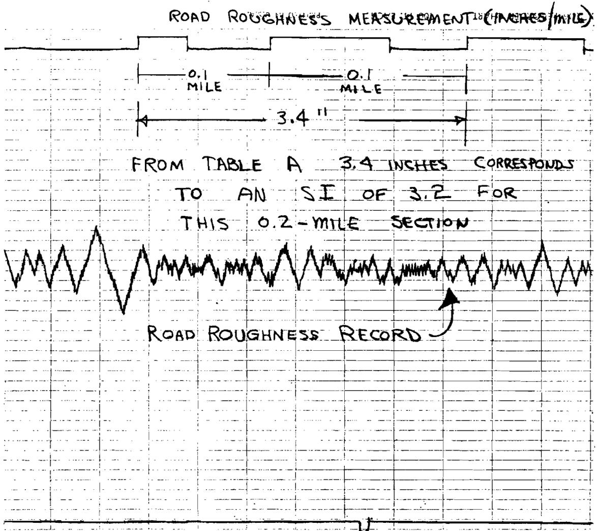
Fig A. Typical MRM road roughness measurements.
