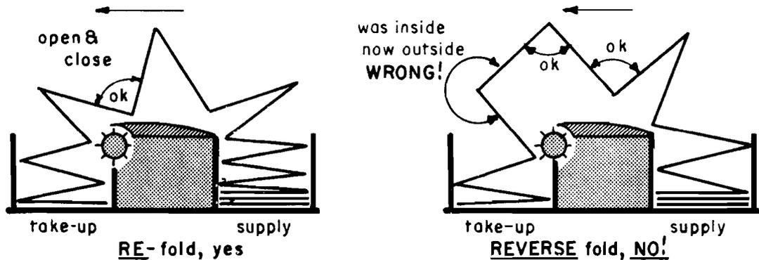
Never open a fresh package until it is needed because the chart can get soggy and lose the necessary spring hinge action.
