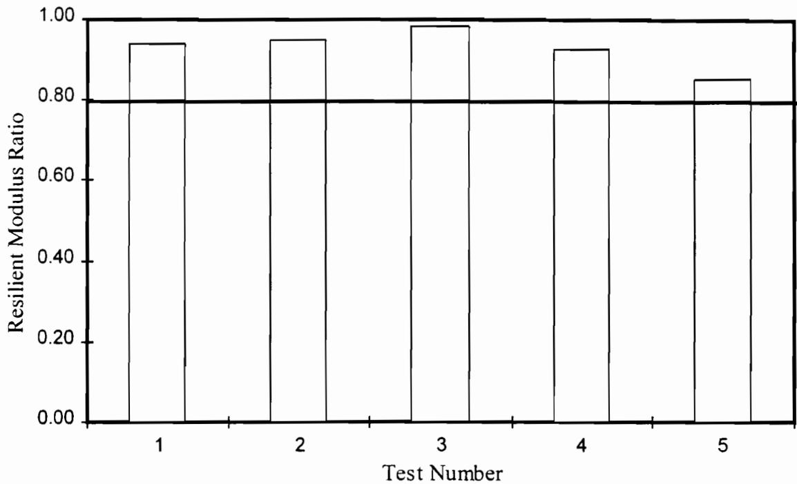
**Figure 5.1 - Resilient Modulus Ratio of the Austin Mix**
