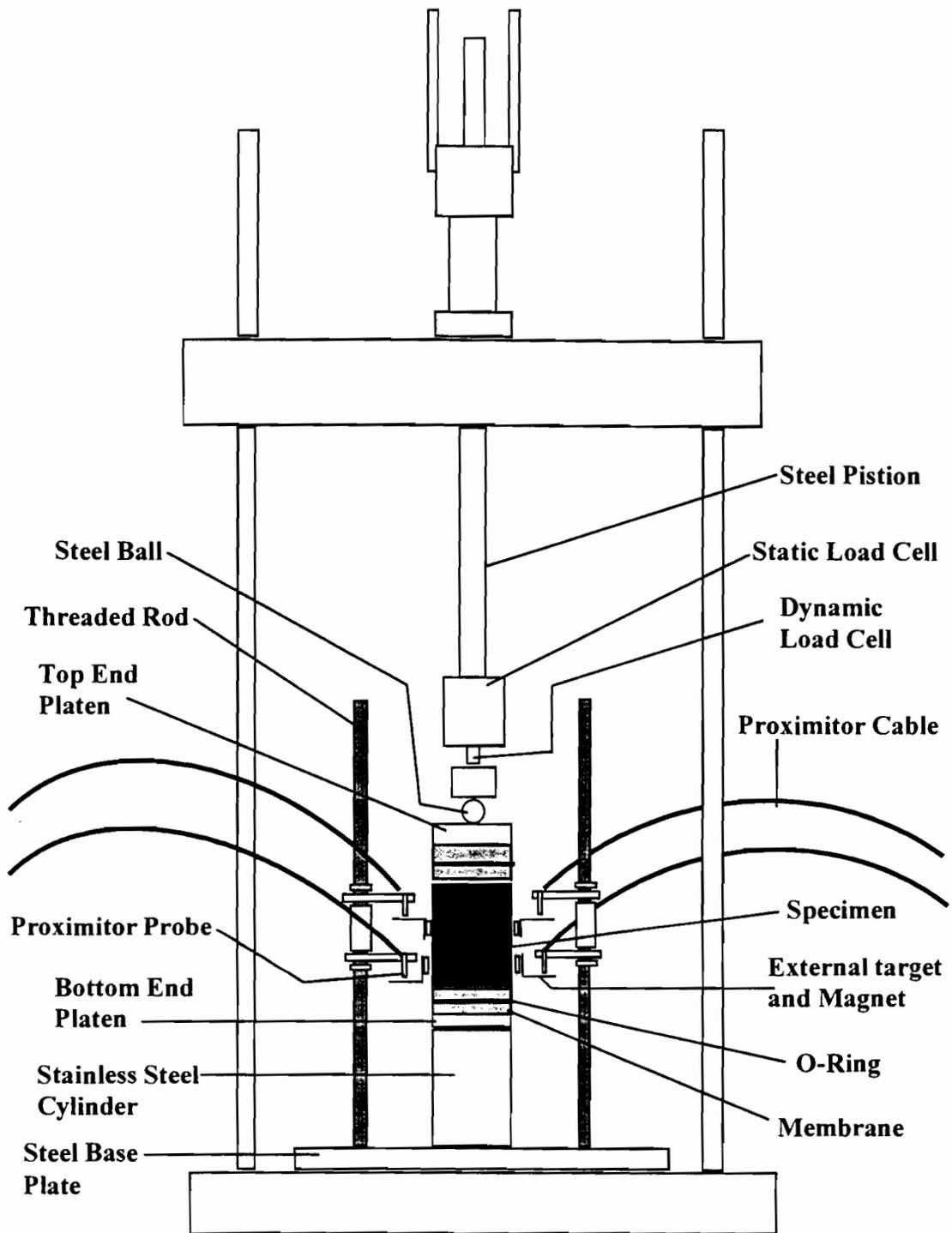
Figure 4.1 - Sketch of Resilient Modulus Test Setup (Not to the Scale)
