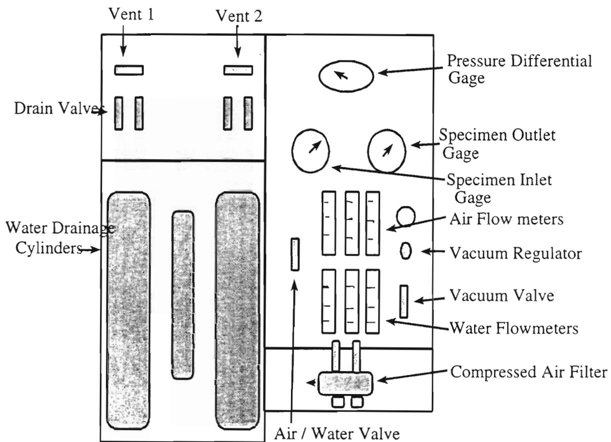
**Figure B.3 - Fluid Control Panel (Front View)**
