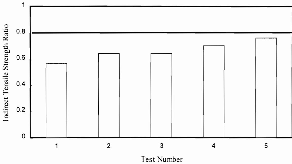
**Figure 5.4 - Indirect Tensile Strength Ratio of the El Paso II Mix**
