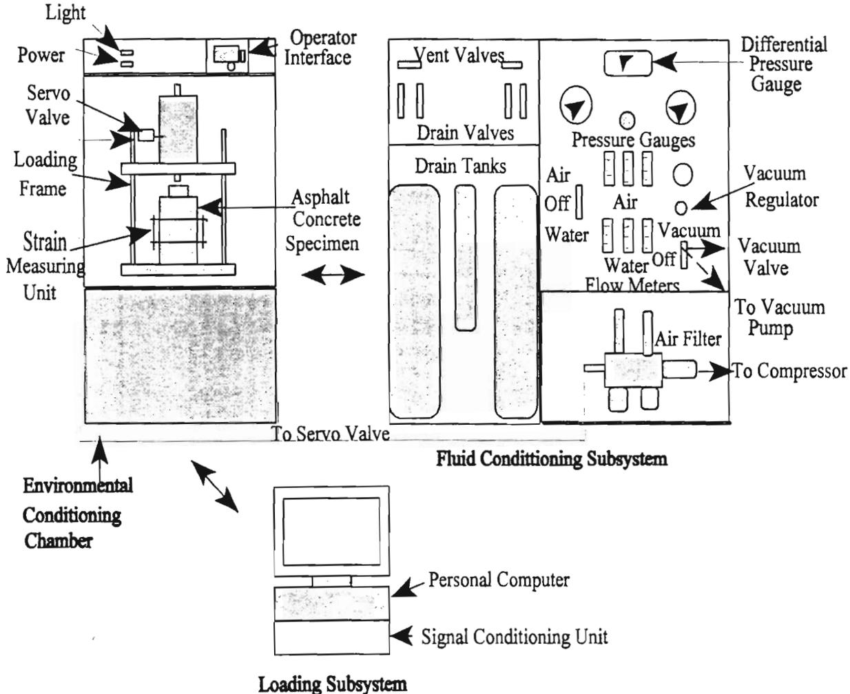
Figure 2.1 - Schematic Diagram of Environmental Conditioning System (ECS)
