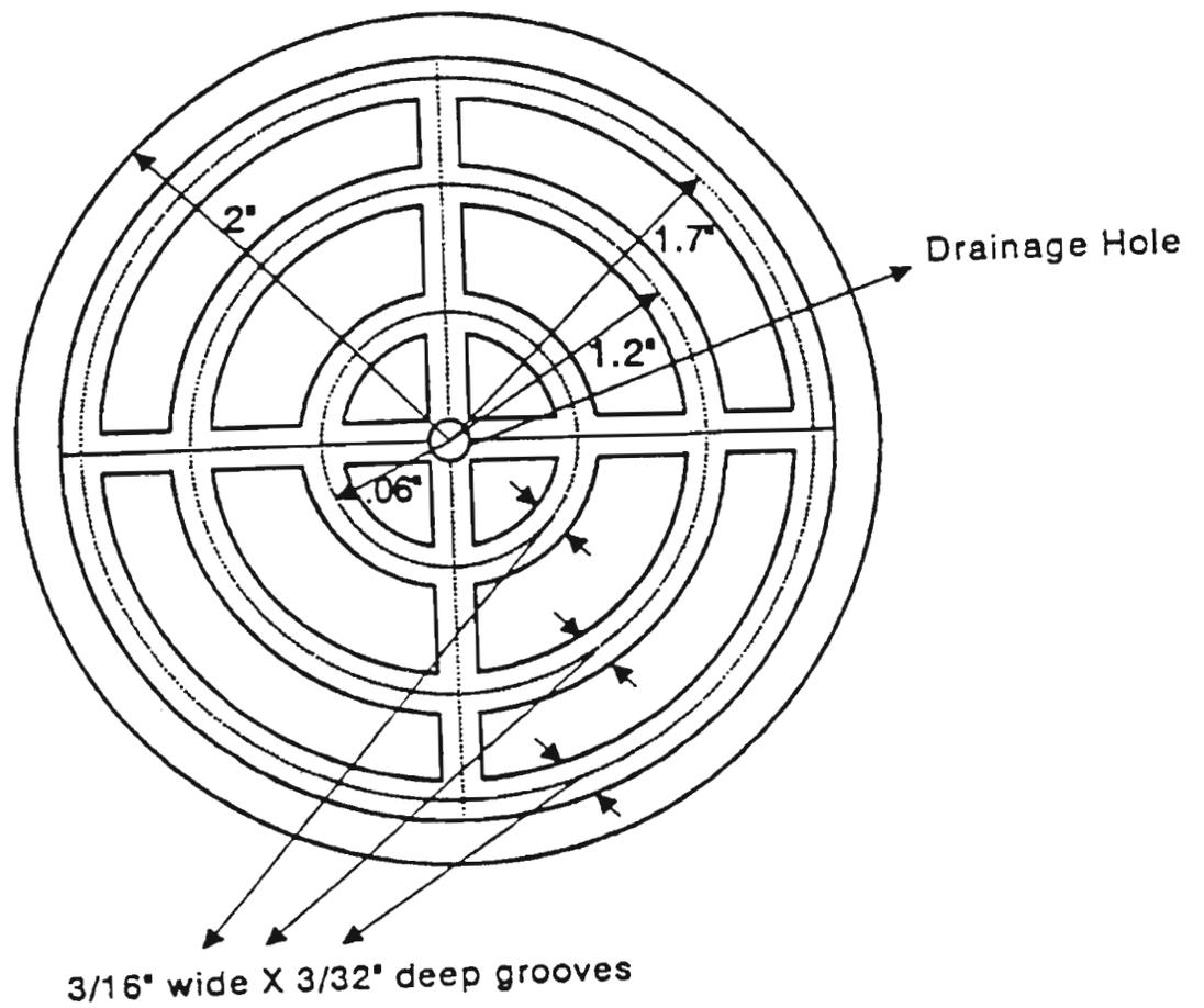
Figure B.4 - Groove Pattern for End Platens
