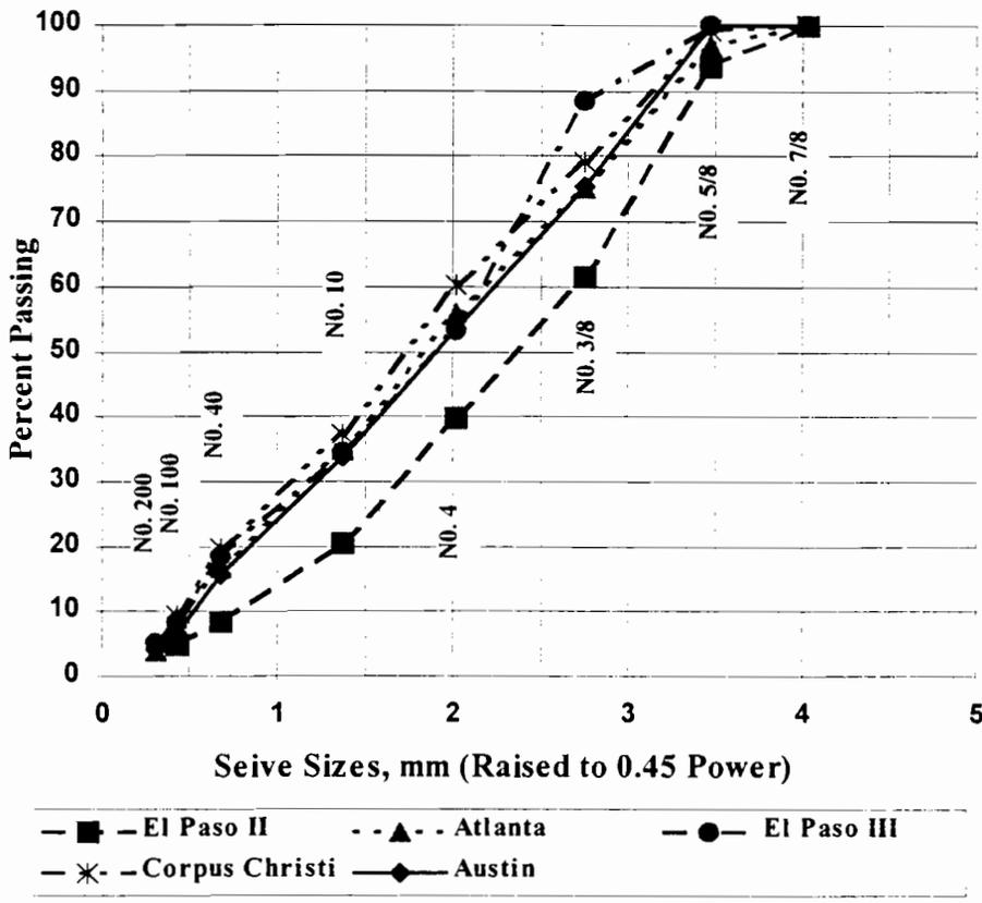
Figure 2.2 - Gradation Chart for the Aggregate of the Mixes
