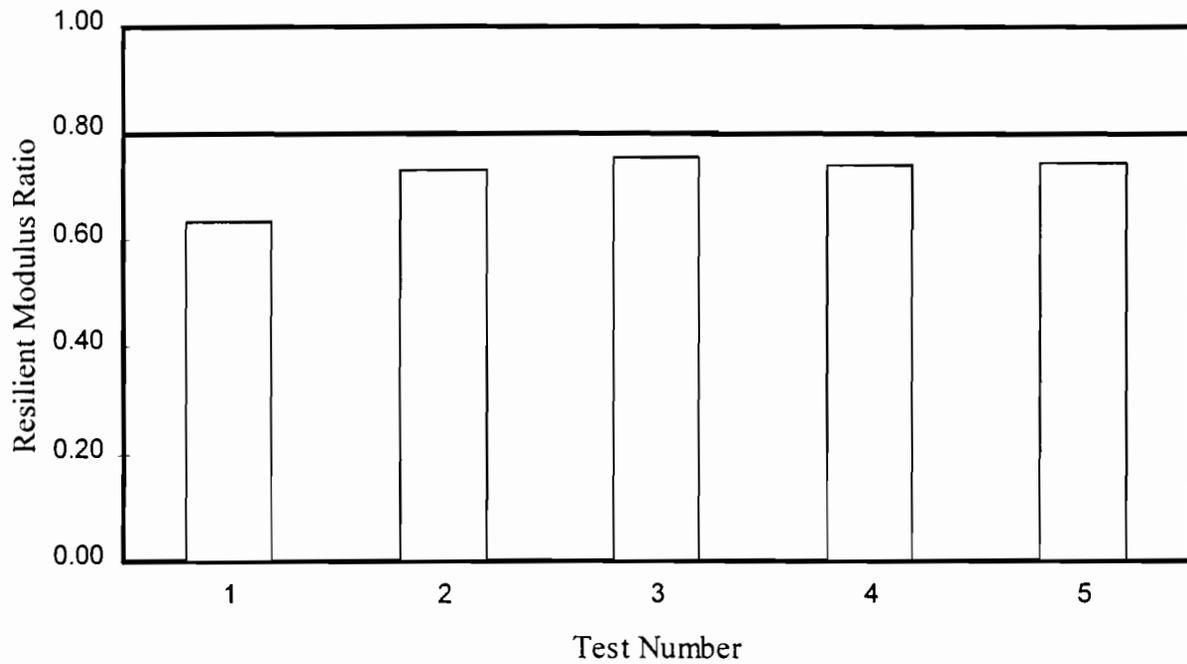
**Figure 5.2 - Resilient Modulus Ratio of the El Paso II Mix**
