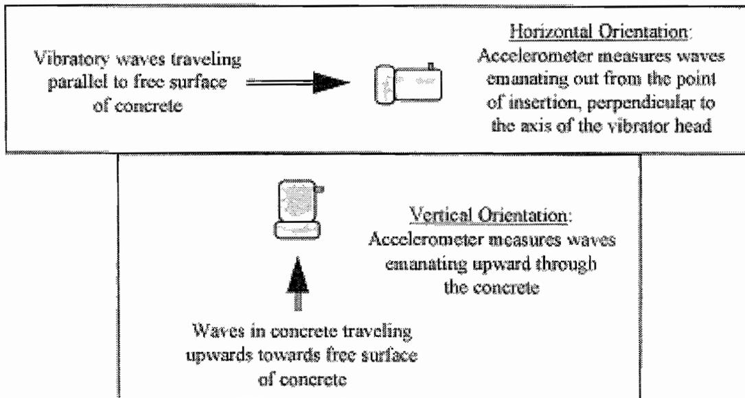
Figure 3.5 Accelerometer orientation
