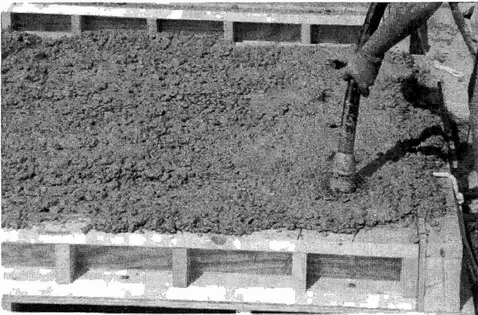
*Figure 2. 15 Consolidating slab specimen*
