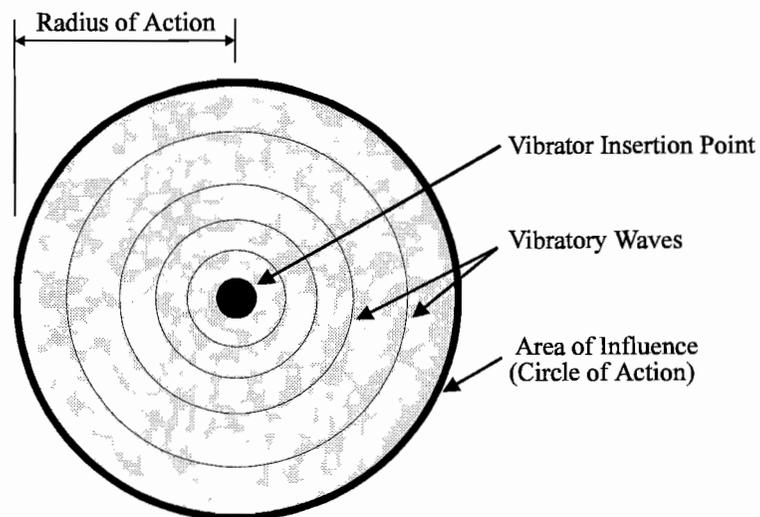
*Figure 1.4 Area of influence for concrete vibrator*
