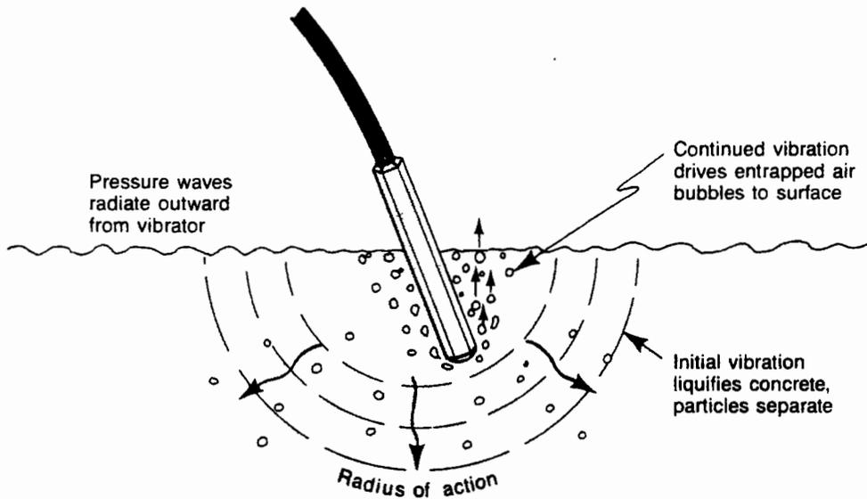
Figure 1.6 *Action of internal vibrator*<sup>8</sup>
