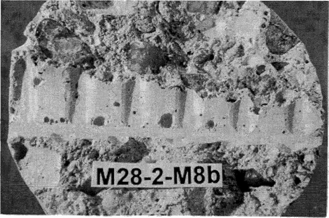
*Figure 4. 24 Large voids under #8 rebar*
