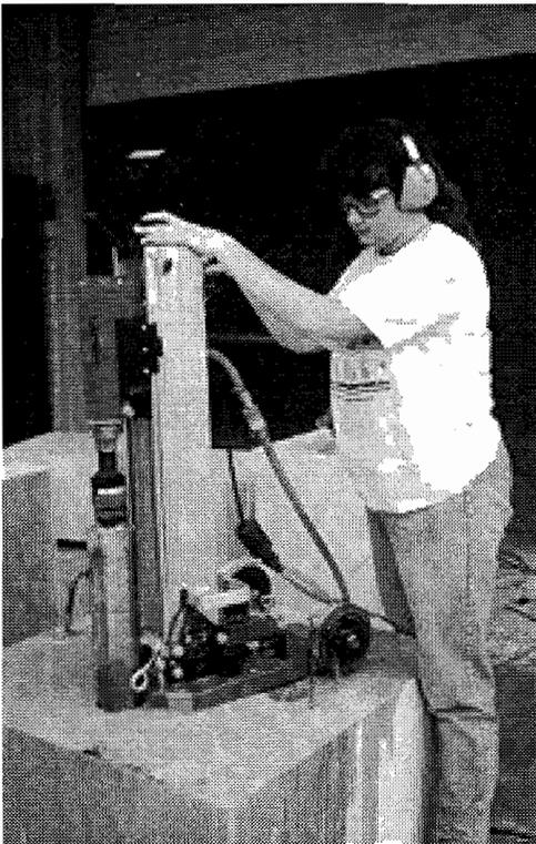
*Figure 4. 13 Coring reinforced concrete test specimen*
