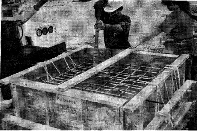
*Figure 2. 12 Consolidating footing specimen*
