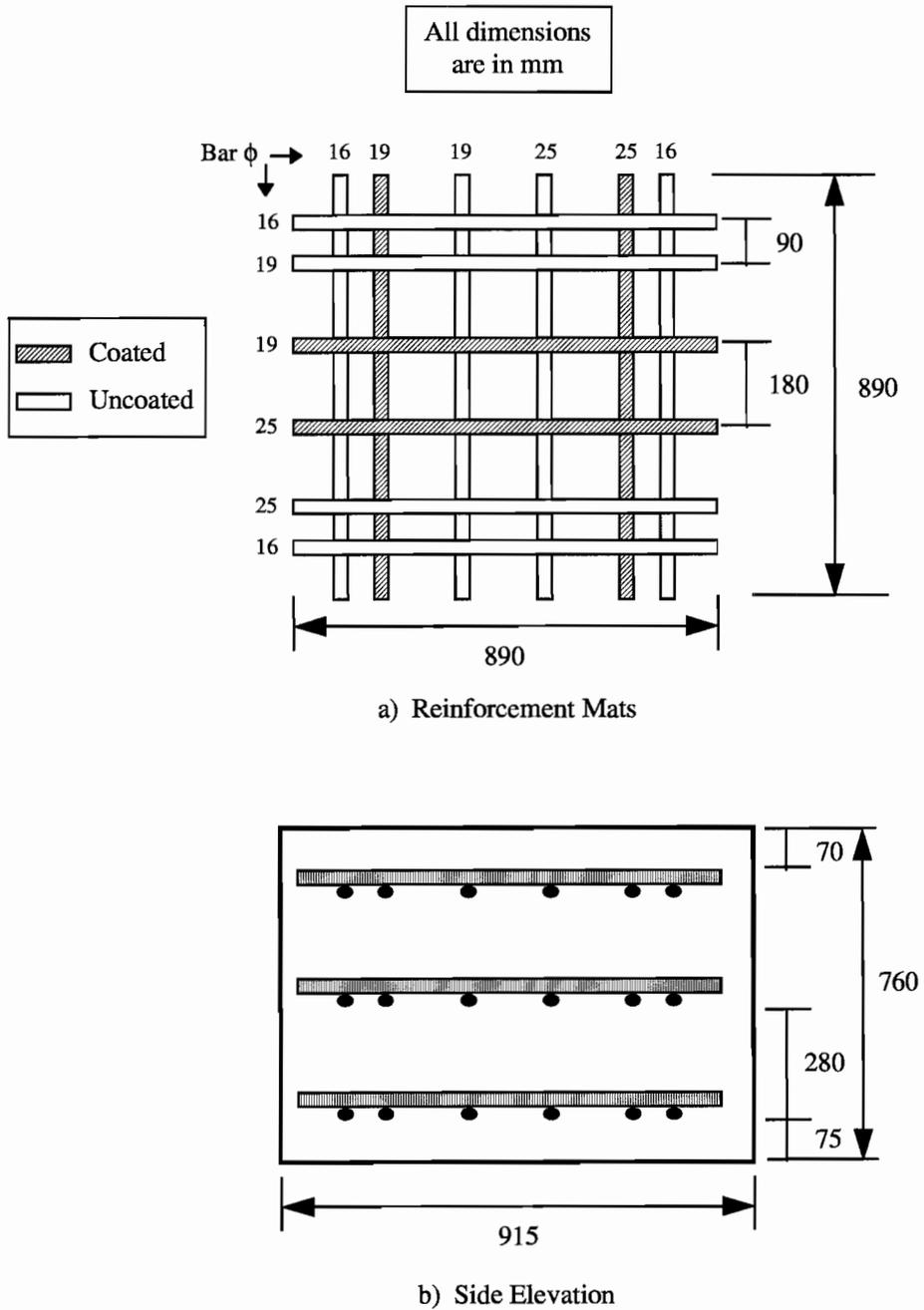
Figure 4.9 Layout of reinforcement in Specimen R30
