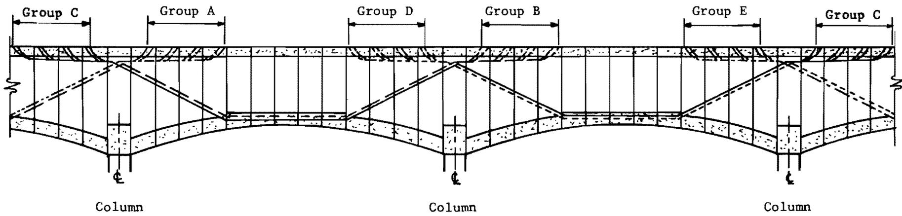
Fig. 4. Hammersmith Flyover--cable profile.
