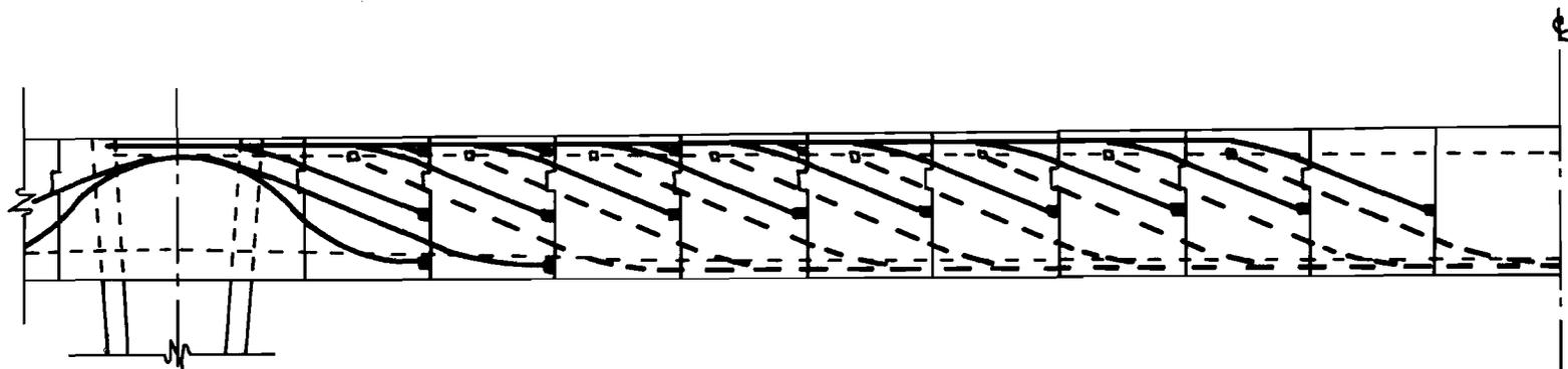
Fig. 14. Choisy-le-Roi Bridge--longitudinal cable profile.
