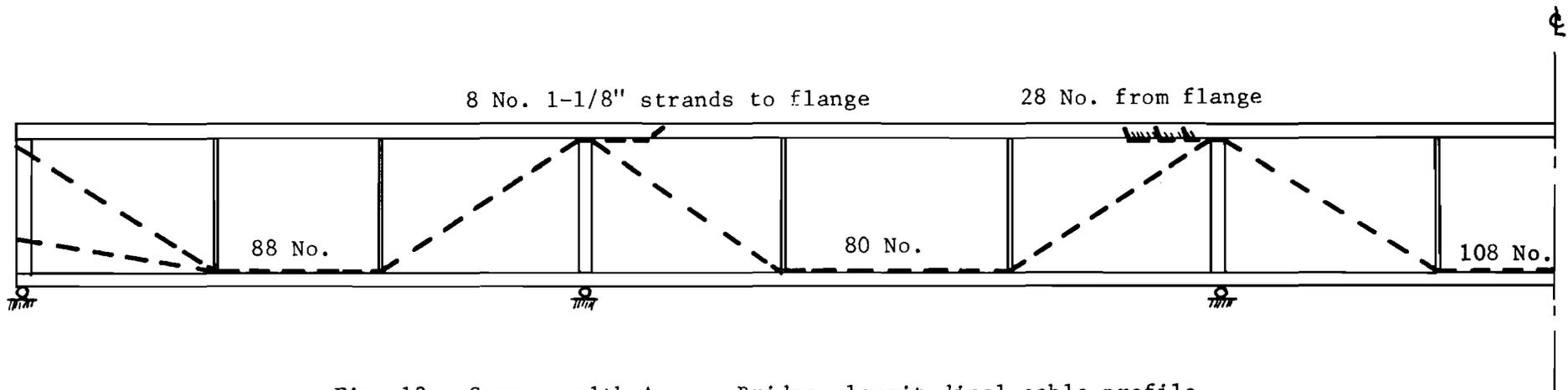
Fig. 13. Commonwealth Avenue Bridge--longitudinal cable profile.
