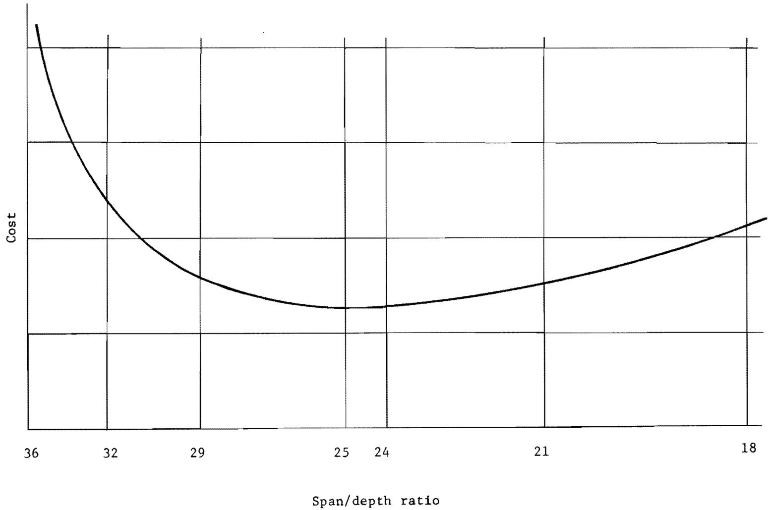
Fig. 16. Relation between cost and depth for a box girder bridge.
