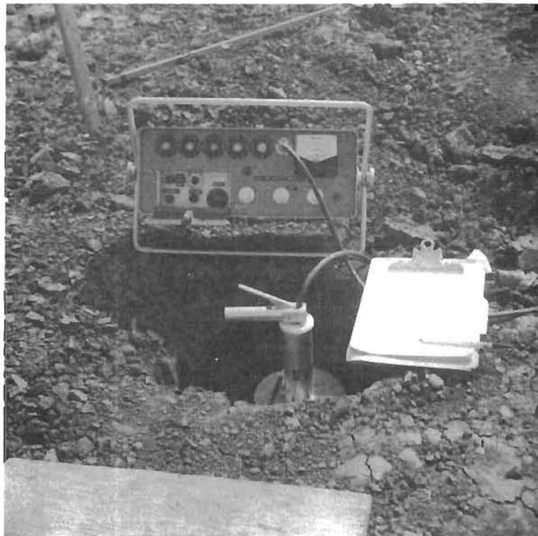
Fig 4.14. Readings in access tube with density probe.
