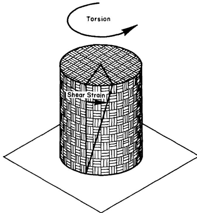
Fig 5. Schematic representation of Test No. 5 to determine shear modulus function  $\phi_3$ .
