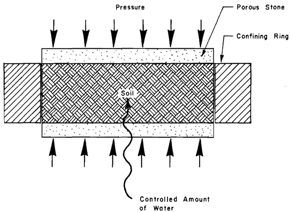
Fig 3. Schematic representation of Test No. 3, zero swell test, to measure  $(\phi_2 + \phi_5)$ .
