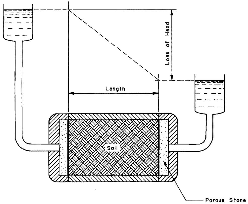
Fig 1. Schematic representation of Test No. 1, the permeability test, to measure  $K$  as a function of  $\sigma_L$ .
