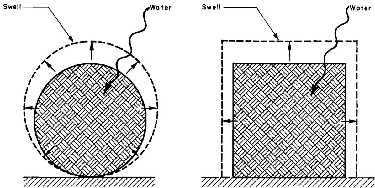
Fig 2. Schematic representation of Test No. 2 to determine  $\frac{\phi_2}{\phi_1}$  and  $\frac{\phi_5}{\phi_4}$ .
