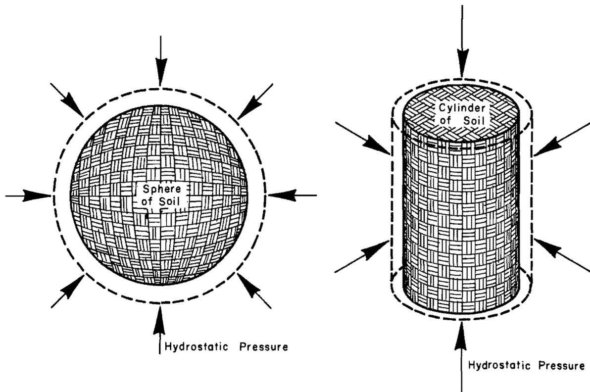
Fig 4. Schematic representation of Test No. 4, compression test, to determine the relations between  $(\phi_2, \phi_3)$  and  $(\phi_4, \phi_5)$ .
