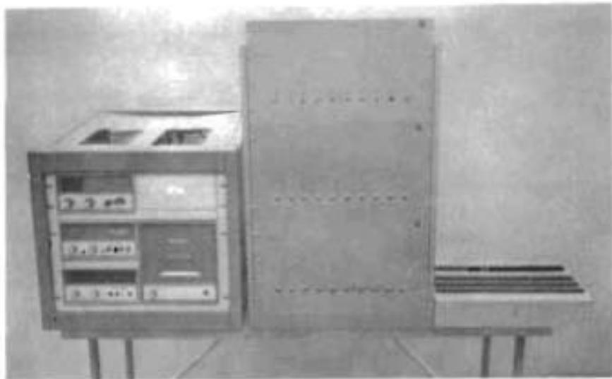
Fig. D.3. Honeywell 620 Data Logging System, Balance Circuits, and Switching System.
