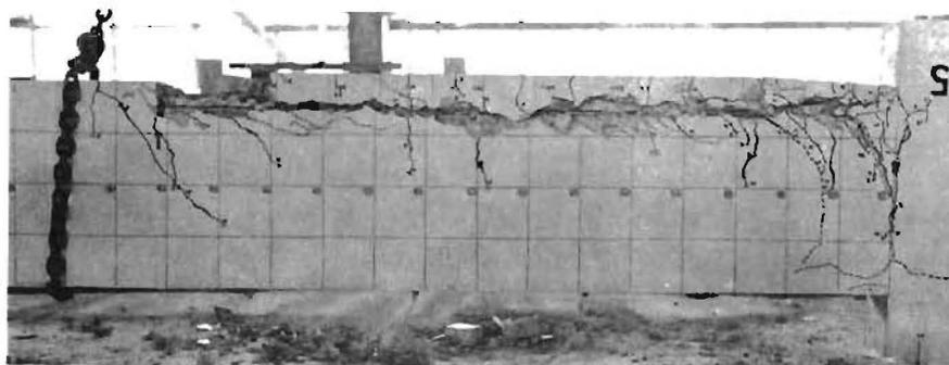
FIG.3. SIDE SPLIT FAILURE OF BEAM NO.5
